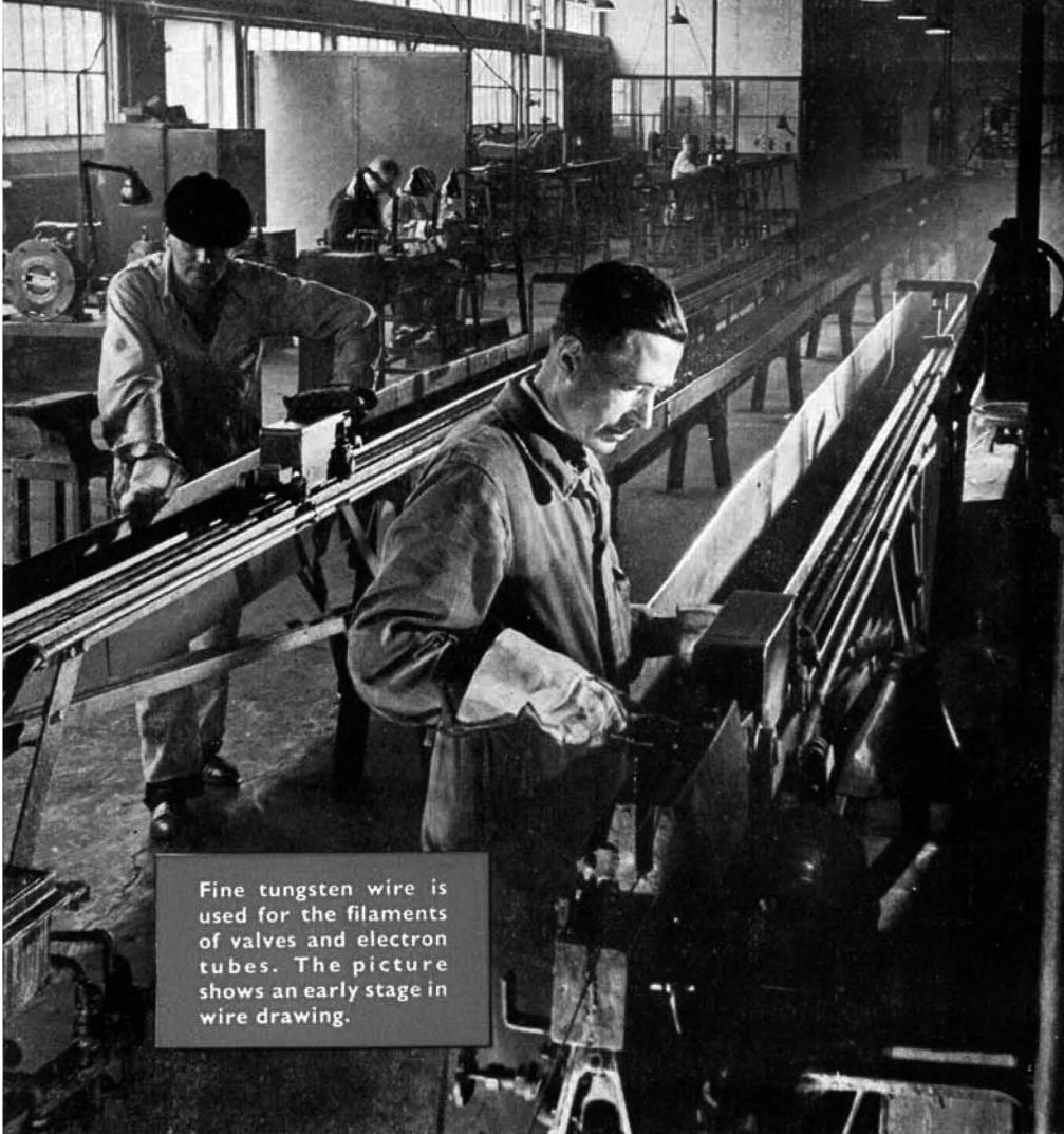
Fine tungsten wire is used for the filaments of valves and electron tubes. The picture shows an early stage in wire drawing.
