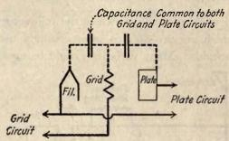
Fig. 36-Inter-electrode tube capacitance.
