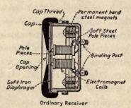
Fig. 21—Construction of a typical telephone receiver.
