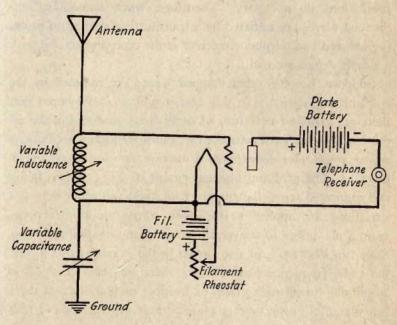
Fig. 22-Simple detector circuit.
