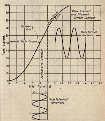
Fig. 30-Amplification of continuous oscillations
