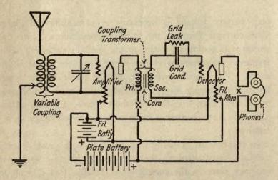
Fig. 45—Two circuits for radio-frequency amplification and detection.
