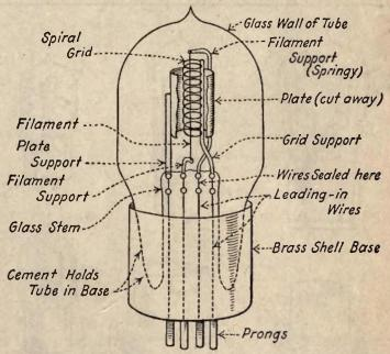
Fig. 12—Construction of a typical vacuum tube.
