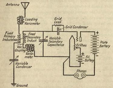
Fig. 39-Two Circuit Receiver, Inductive Coupling.
