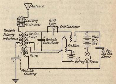
Fig. 40-Two Circuit Regenerative Receiver, Inductive Coupling.
