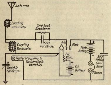
Fig. 38-Single Circuit Regenerative Receiver.
