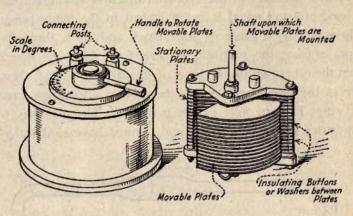
Fig. 7—Typical variable condenser with air dielectric.
