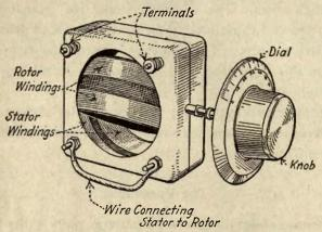
Fig. 35—Construction of a typical variometer.
