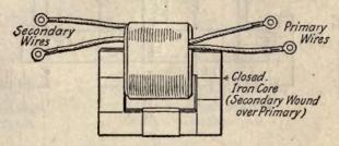
Fig. 44-Typical audio-frequency coupling transformer.
