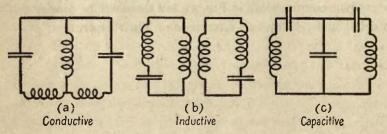
Fig. 34-Methods of coupling.
