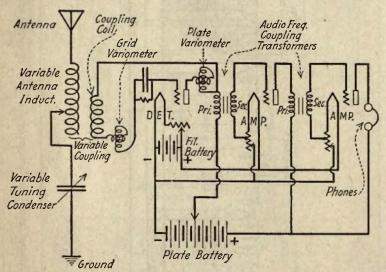
Fig. 47—Suggestion for Short Wave Regenerative Receiver and Two Stage
