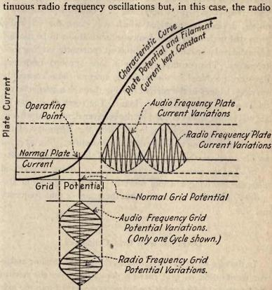
Fig. 24-Detection of modulated continuous oscillations at a constant group frequency.
