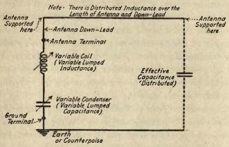
Fig. 11-Scheme of antenna as a complete circuit.
