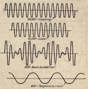
Fig. 27-The principle of heterodyne action.
