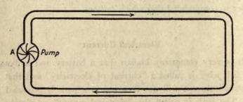
Fig. 2-Water analogy of simple electrical circuit.
