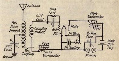
Fig. 41-Three Circuit Regenerative Receiver for Short Waves.
