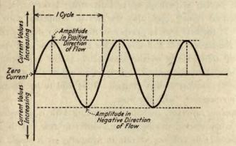
Fig. 9-Continuous oscillations.
