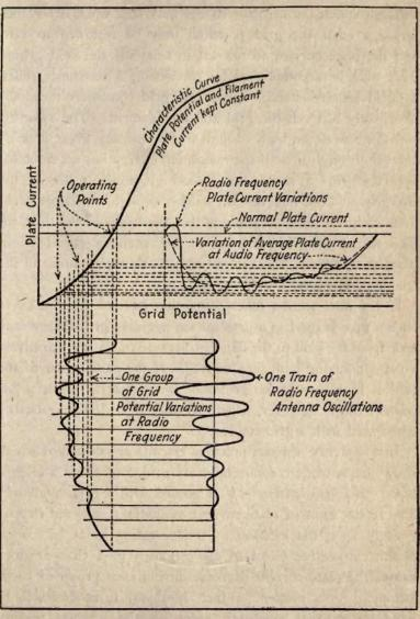
Fig. 26—Rectification or detection of damped oscillations with a grid condenser.
