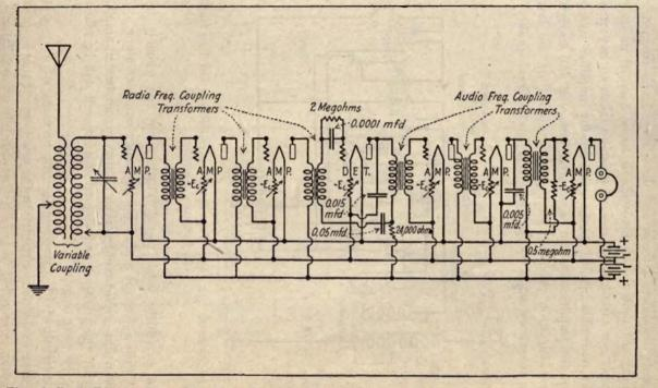
Fig. 46-Radio Frequency Amplifier, Detector and Audio-frequency Amplifier connected to Two Circuit Receiver.
