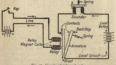
Fig. 17—Circuits of telegraph relay.
