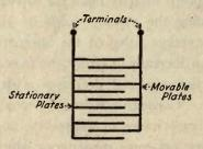
Fig. 6—Scheme of a variable condenser. (If the movable plates are made stationary it is a "fixed" condenser.)
