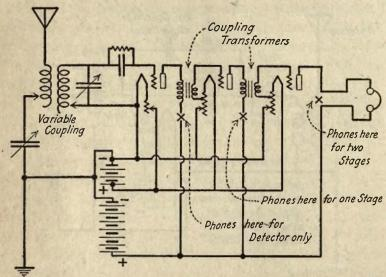
Fig. 43—Two Circuit Receiver with Two-Stage Audio-frequency Amplifier.
