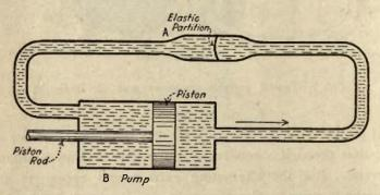
Fig. 8—Water analogy of alternating current in a circuit containing a condenser.
