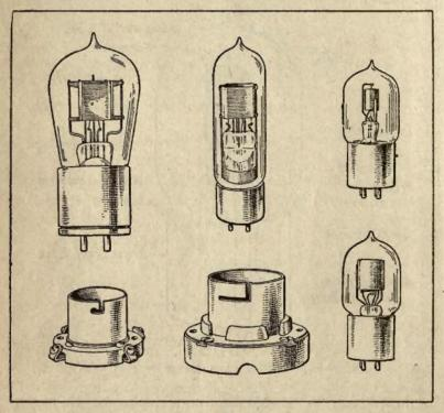
Fig. 13-Various forms of vacuum tubes and sockets.
