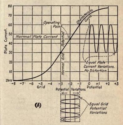
Fig. 29 (a)—Amplification of continuous oscillations.
