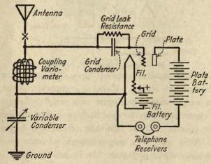
Fig. 37-Simple Single Circuit Receiver.
