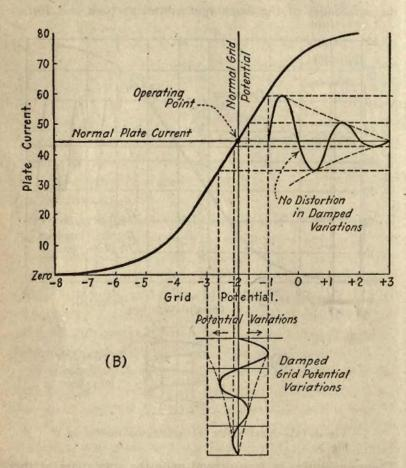
Fig. 29 (b)-Amplification of damped oscillations.
