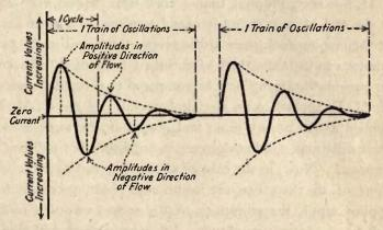
Fig. 10-Damped oscillations.
