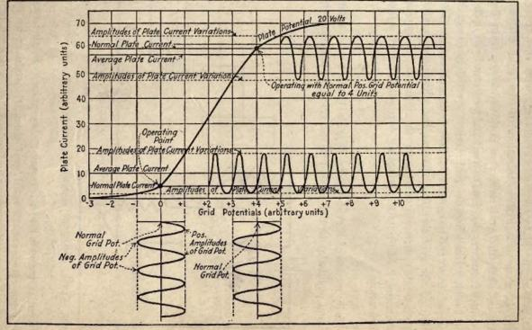
Fig. 19-Variations of plate current with variations of grid potential.
