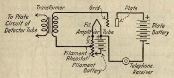
Fig. 31—Customary method of placing a normal negative potential on the grid of an amplifier tube.
