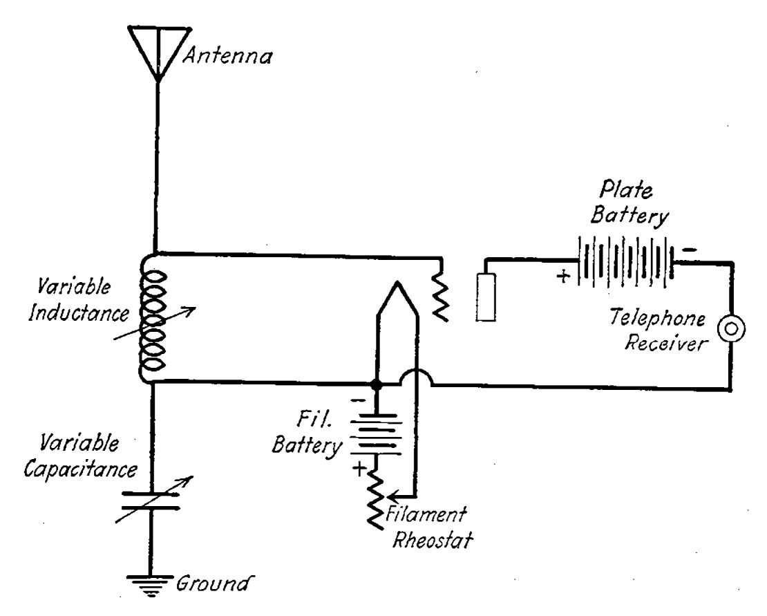
Fig. 22—Simple detector circuit.
