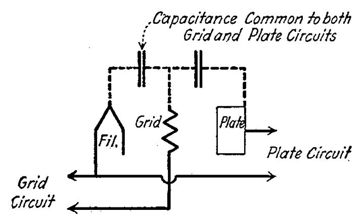
Fig. 36—Inter-electrode tube capacitance.
