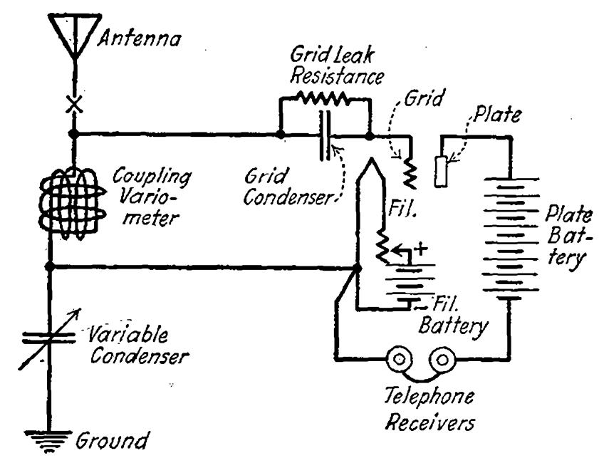
Fig. 37—Simple Single Circuit Receiver.
