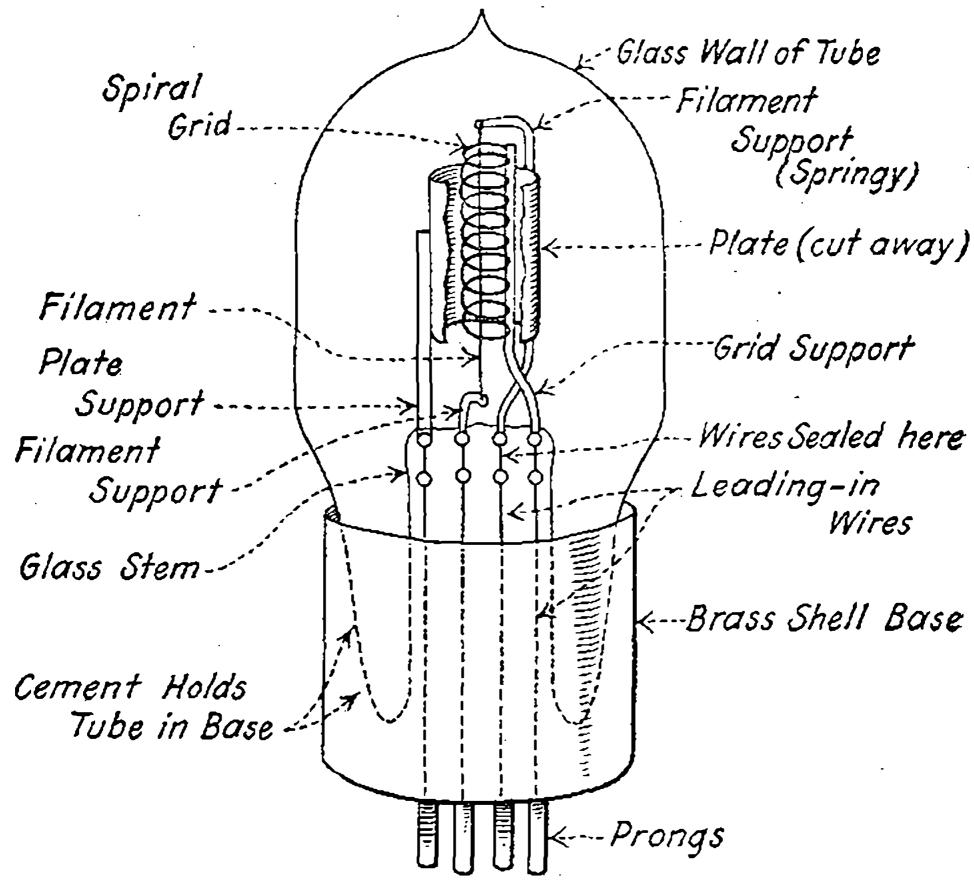
Fig. 12—Construction of a typical vacuum tube.
