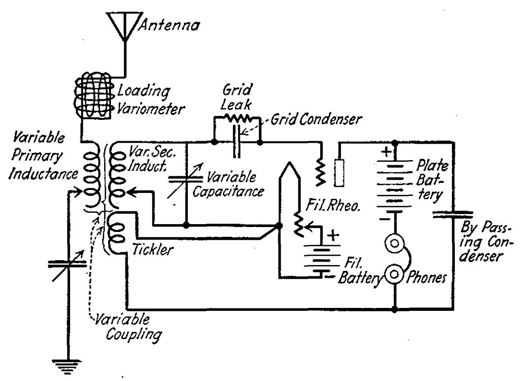
Fig. 40—Two Circuit Regenerative Receiver, Inductive Coupling.
