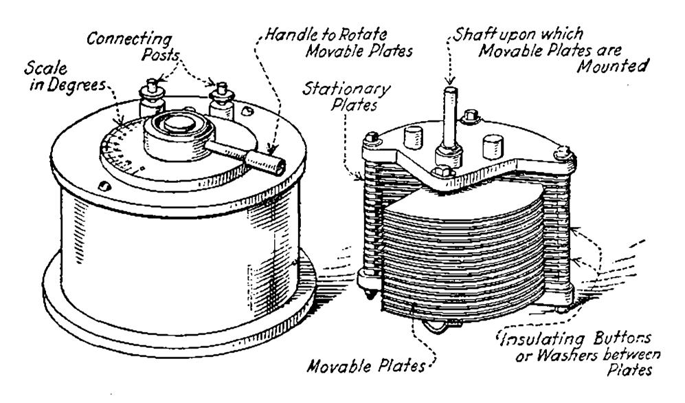
Fig. 7—Typical variable condenser with air dielectric.
