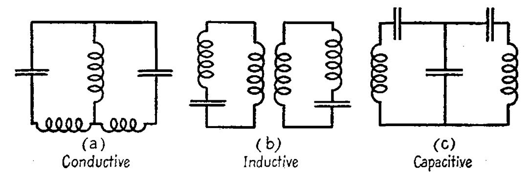
Fig. 34—Methods of coupling.
