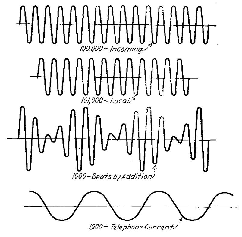
Fig. 27—The principle of heterodyne action.
