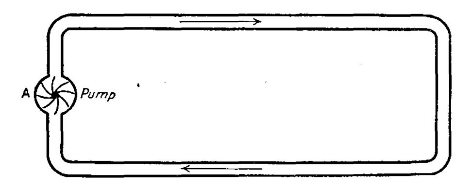
Fig. 2—Water analogy of simple electrical circuit.
