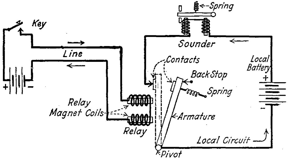
Fig. 17—Circuits of telegraph relay.
