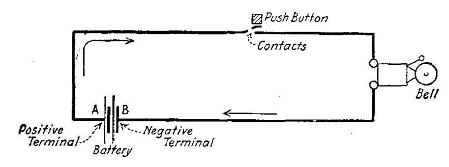
Fig. 1—Simple electrical path or circuit.
