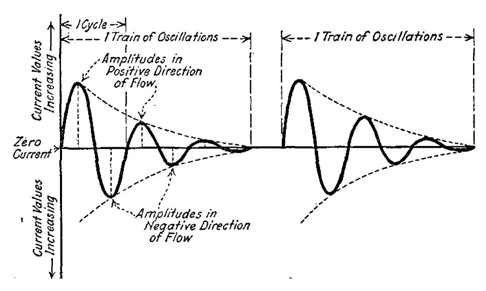
Fig. 10—Damped oscillations.
