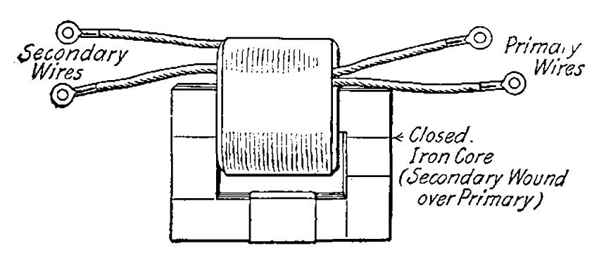
Fig. 44—Typical audio-frequency coupling transformer.
