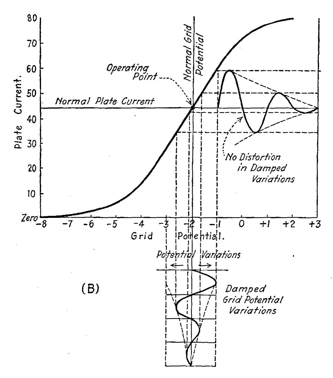
Fig. 29 (b)—Amplification of damped oscillations.
