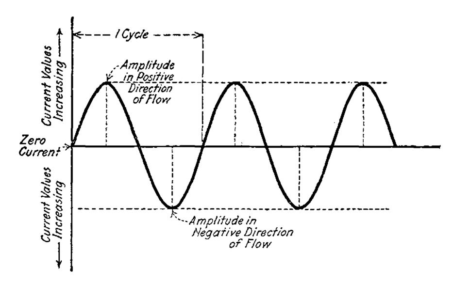
Fig. 9—Continuous oscillations.
