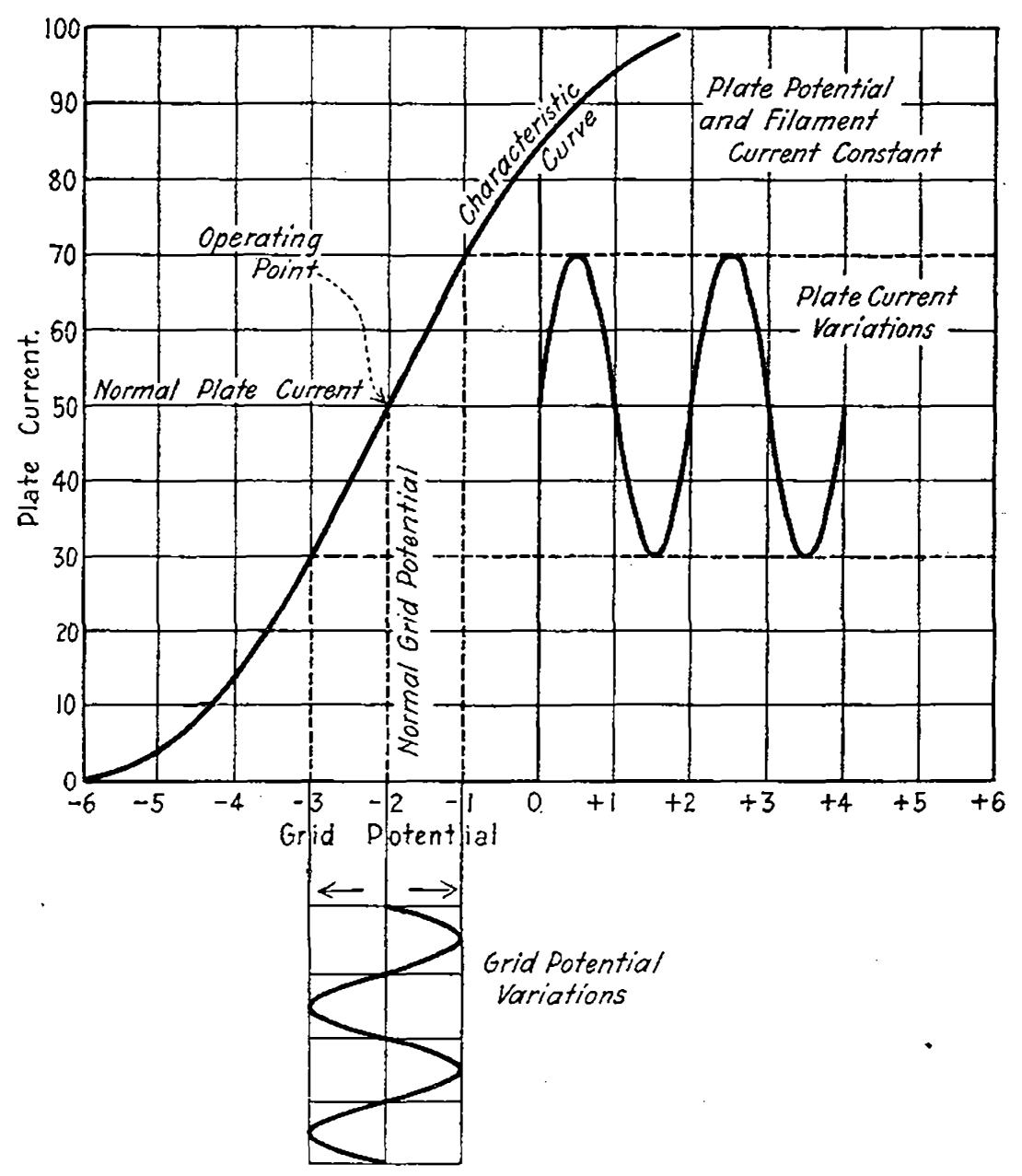
Fig. 30—Amplification of continuous oscillations
