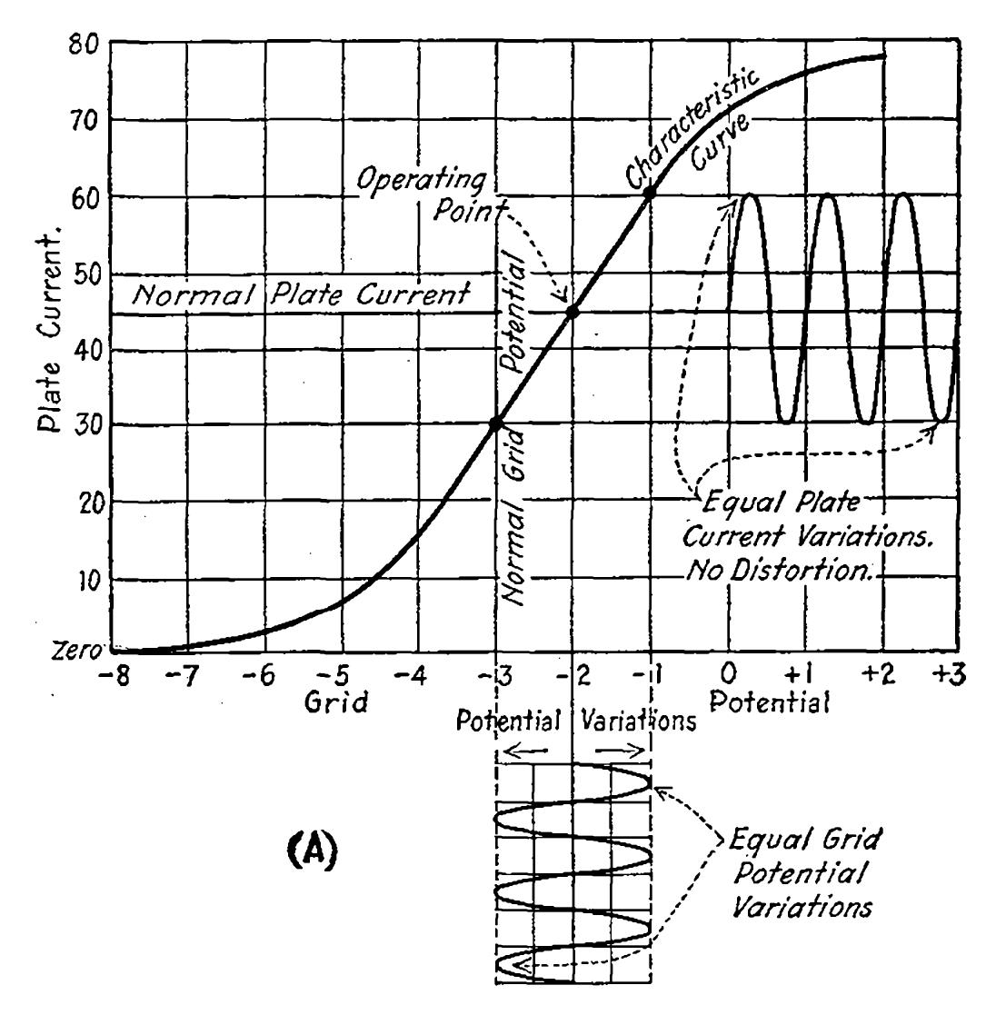
Fig. 29 (a)—Amplification of continuous oscillations.
