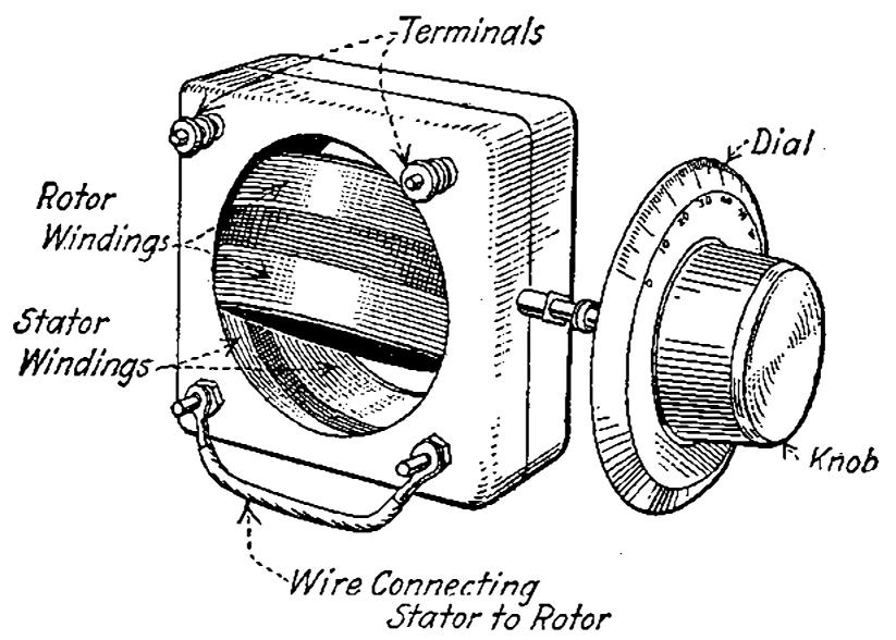
Fig. 35—Construction of a typical variometer.
