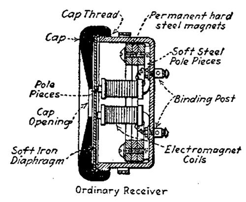
Fig. 21—Construction of a typical telephone receiver.
