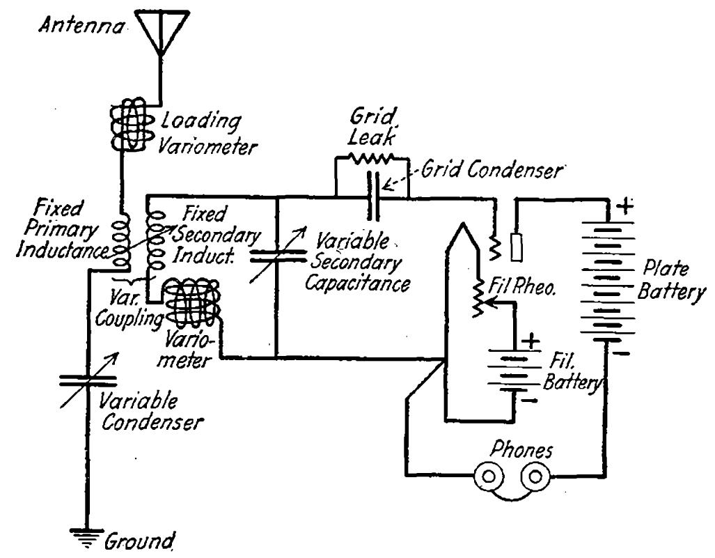
Fig. 39—Two Circuit Receiver, Inductive Coupling.
