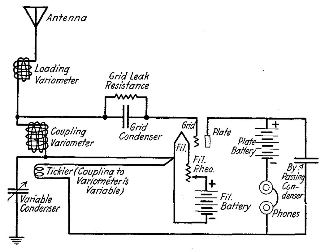
Fig. 38—Single Circuit Regenerative Receiver.
