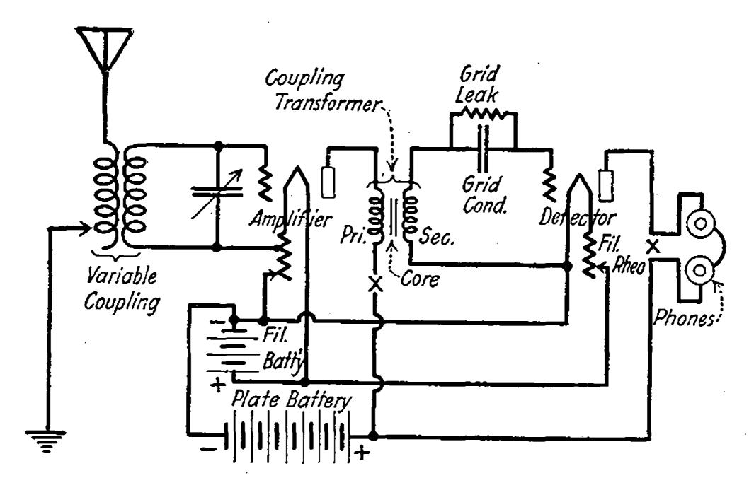
Fig. 45—Two circuits for radio-frequency amplification and detection.
