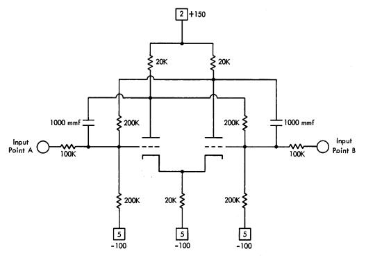
Figure 62. Desensitized Triggers, Types TR41 and TR42
