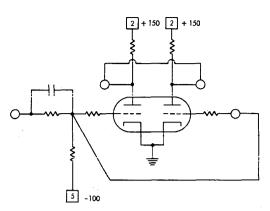
Figure 40. A Semi-Power Arrangement Using Two Triodes in Parallel
