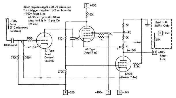
Figure 71. Schematic Diagram of the 604 Reset Circuit
