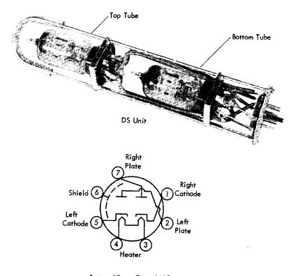
Bottom View, Type 6AL5 Figure 49. A Diode Switch Pluggable Unit and the Base Diagram for Type 6AL5 Tubes
