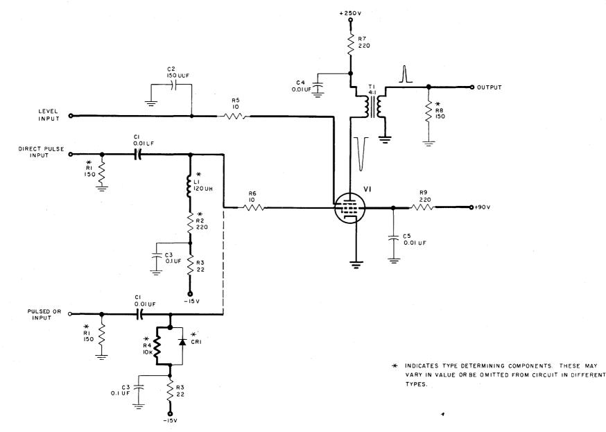
Figure 3-34. Gate Tube, Model A, Schematic Diagram
