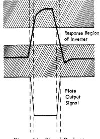
Figure 34. Signal Reshaping
