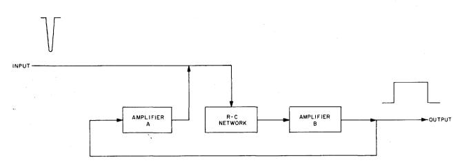
Figure 3—46. Single-Shot, Simplified Block Diagram
