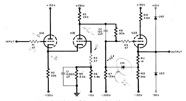
Figure 3-10. D-C Level Setter, Model A, Schematic Diagram
