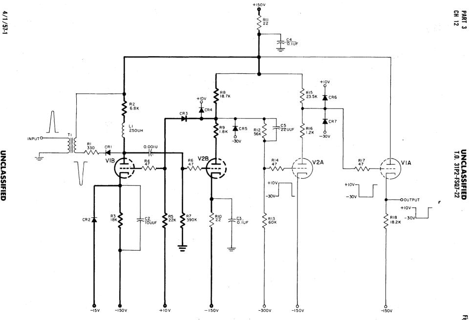
Figure 3—51. Single-Shot, Model C, Schematic Diagram
