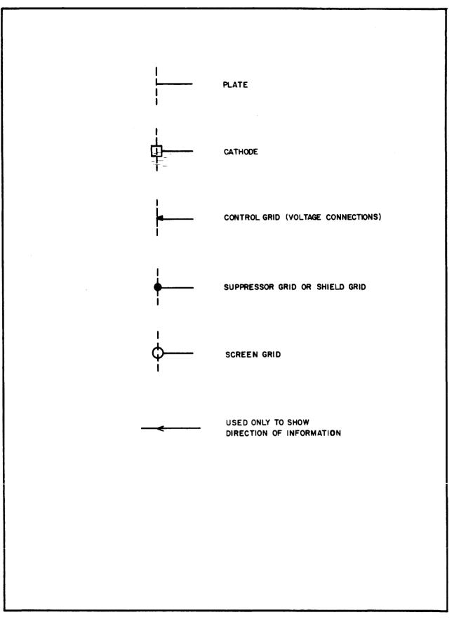
Figure 2. Tube Element Connections. PX 131
