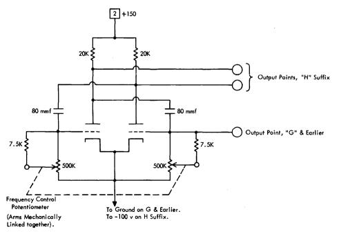
Figure 67. 604 Multivibrator Circuit
