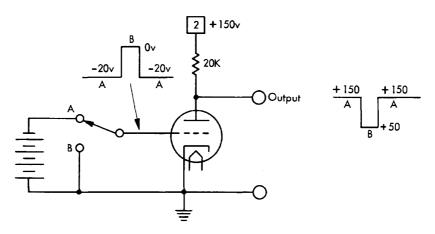
Figure 21. Basic Inverter Circuit
