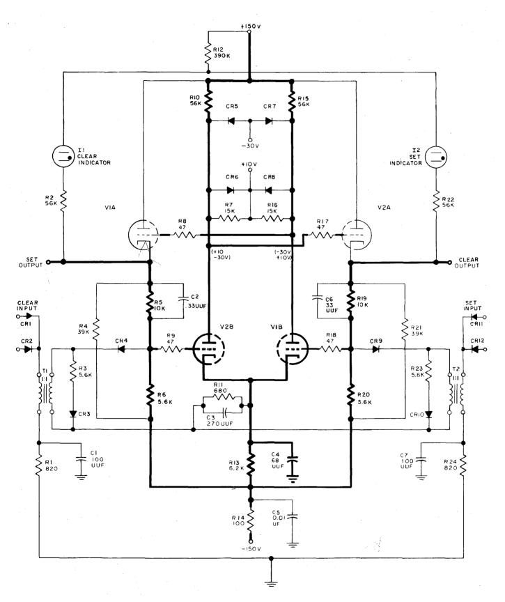
Figure 3–44. Flip-Flop, Model A, Schematic Diagram
