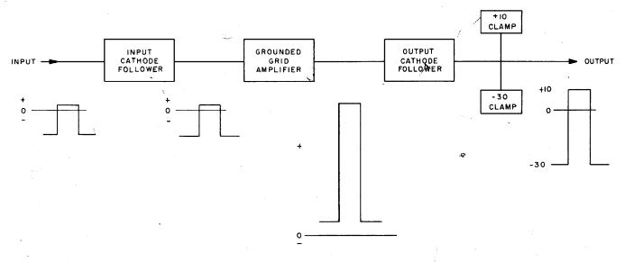
Figure 3–8. D-C Level Setter, Block Diagram
