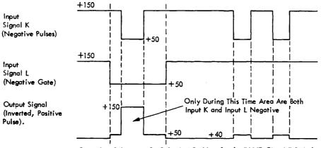
Control or Selection of a Pulse is a Problem for the "AND Circuit" Switch. Waveshapes Drawn are Representative of an Inverter Switch.
