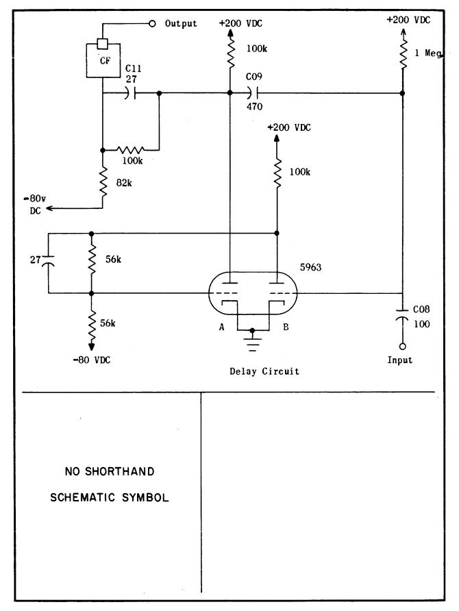
Figure 11. STANDARD Delay Circuit (Vacuum Tube) PX 131 UNCLASSIFIED
