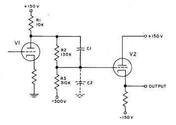
Figure 2-15. Compensated D-C Coupling Network, Simplified Schematic Diagram
