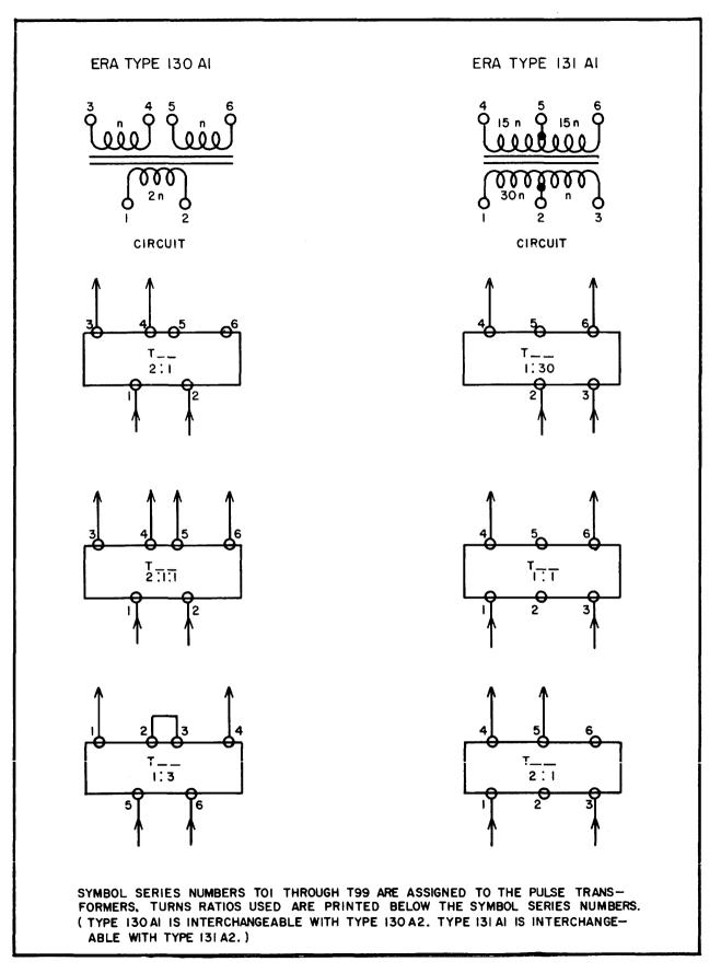
Figure 8. STANDARD Pulse Transformer Stages PX 131 (7) SHAPER. - A shaper is used to change the form of a pulse to a desired level, duration, or shape. This is done in order to facilitate the use of the pulse in a special application or circuit. Shapers differ in their purpose and circuitry. For this reason, shapers are indicated by the symbol shown in Figure 9, and their operations are not detailed unless necessary for the explanation of **a**n associated circuit.
