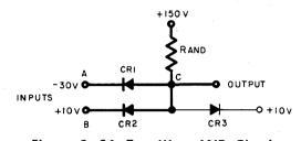
Figure 3—26. Two-Way AND Circuit, Schematic Diagram
