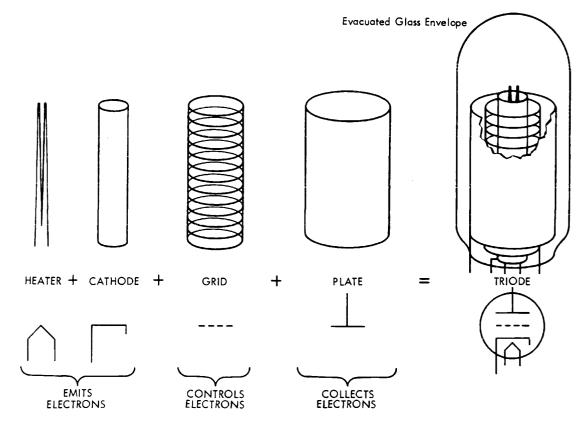
Figure 20. Development of the Triode Tube
