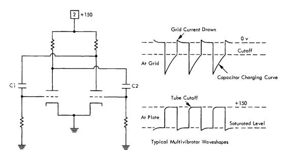
Figure 66. The Basic Multivibrator and Typical Waveshapes
