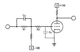
Figure 24. The Compensating Capacitor
