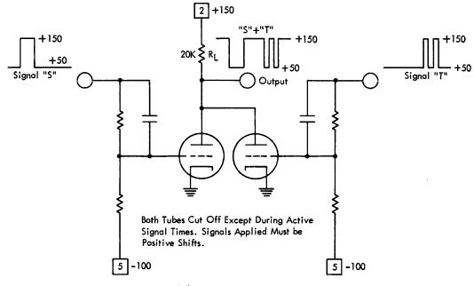
Figure 37. The Inverter OR Circuit (Mixer)
