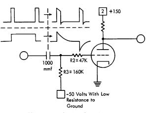
Figure 28. The Coupling Capacitor
