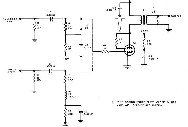
Figure 3-13. Pulse Amplifier, Model B, Schematic Diagram
