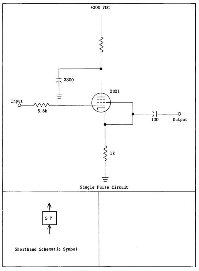
Figure 10. STANDARD Single Pulse Circuit PX 131
