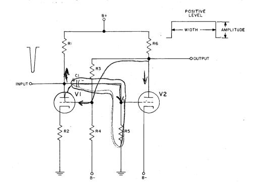
Figure 3–47. Single-Shot, Simplified Schematic Diagram
