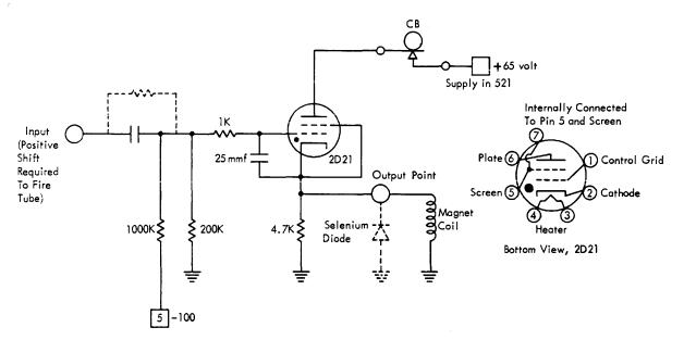
Figure 54. A Typical Thyratron Unit Circuit and the Base Diagram for the Type 2D21 Tube
