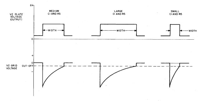
Figure 3–49. Plate and Grid Voltages of V2 for Varying Values of C1 and R5
