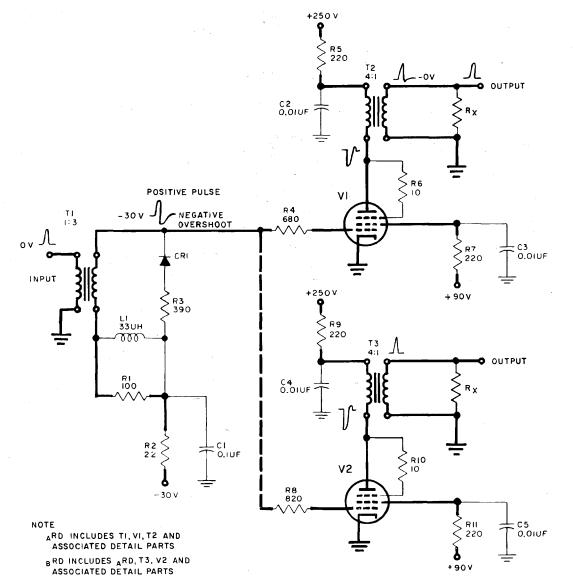
Figure 3–15. Register Driver, Models A and B, Schematic Diagram
