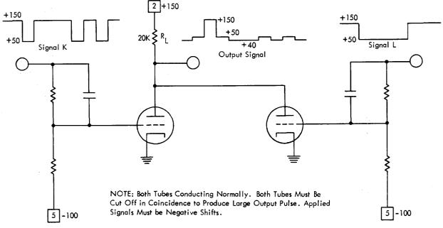
Figure 39. The Inverter AND Circuit (Switch)
