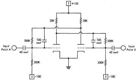
NOTE: Capacitive input triggers in the 604 respond only to negative shifts. Figure 63. A Capacitive Input Trigger
