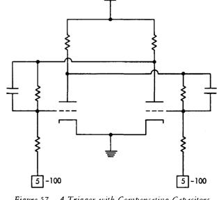
NOTE: The convention used for designating a trigger as ON or OFF: left side conducting is ON; right side conducting is OFF.
