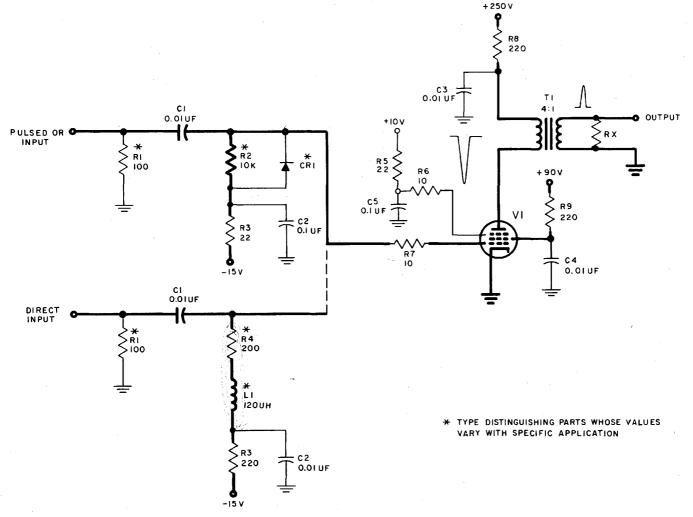
Figure 3–12. Pulse Amplifier, Model A, Schematic Diagram
