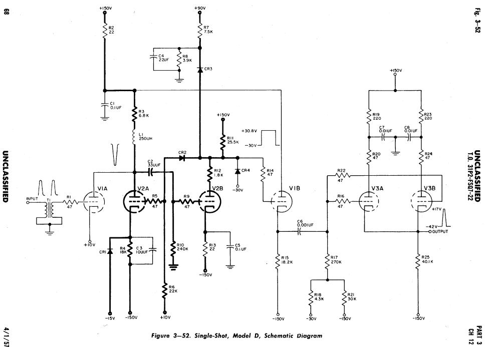
Figure 3-52. Single-Shot, Model D, Schematic Diagram
