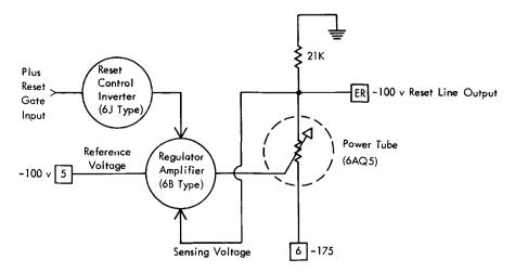
Figure 70. Basic Workings of the Reset Regulator
