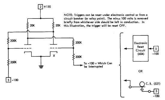
Figure 59. Trigger Unit Reset
