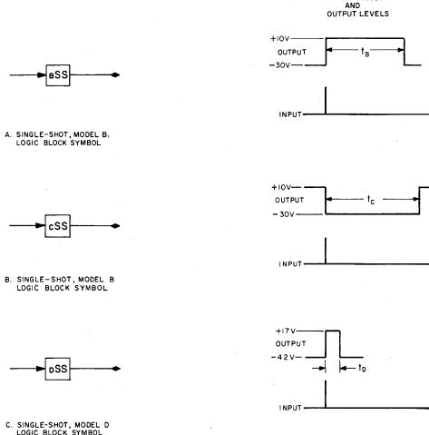
Figure 3-45. Single-Shot, Logic Block Symbols and Output Waveforms
