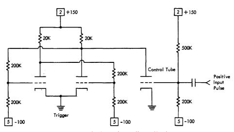
Figure 60. The Basic Plate Pullover Circuit
