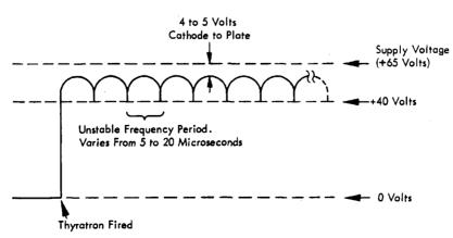
Figure 55. Thyratron Flutter or Oscillation
