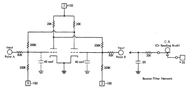
Figure 61. The Direct Coupled Trigger Input
