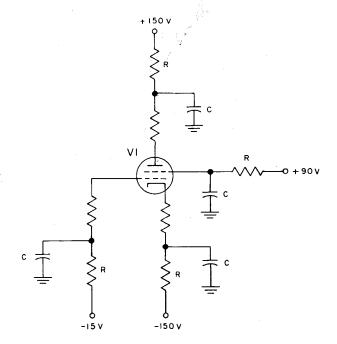
Figure 2—10. RC Decoupled Returns, Simplified Schematic Diagram
