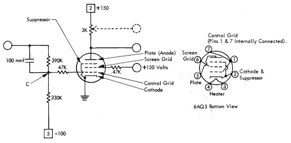
Figure 41. A Power Unit Using a 6AQ5
