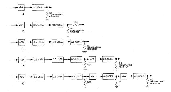
Figure 3-59. Typical Arrangements of Delay Units
