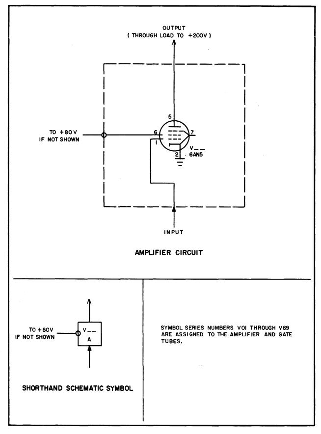
Figure 7. STANDARD Amplifier Stage PX 131
