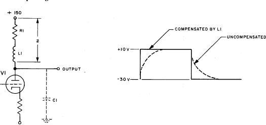
Figure 2—17. Peaking Coil Compensated Plate Circuit, Simplified Schematic Diagram with Waveform UNCLASSIFIED
