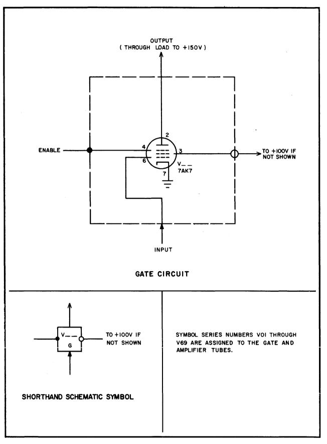
Figure 6. STANDARD Gate Stage PX 131
