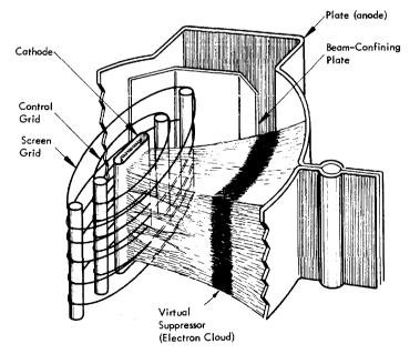
Figure 42. A Beam Power Pentode
