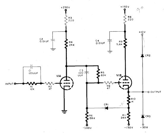
Figure 3–38. D-C Inverter, Model A, Schematic Diagram
