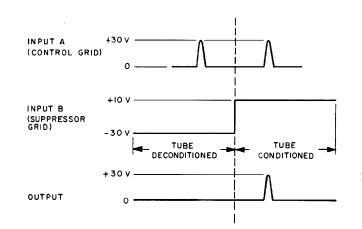
Figure 3–35. Gate Tube, Model A, Input-Output Relationship
