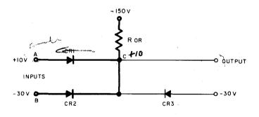
Figure 3—29. Two-Way OR Circuit, Schematic Diagram
