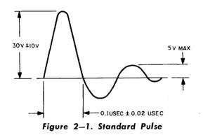
(nominal) with a tolerance of  $\pm 10$  volts. The pulse shape approaches that of the positive half of a sine wave, with a negative tail of indefinite value. The pulse width measured at the base has a nominal value of 0.1 microsecond and a tolerance of  $\pm 0.02$  microsecond. It is evident that a standard pulse is defined by its amplitude, pulse width, and shape.
