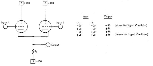
Figure 44. The Cathode Follower Switch Circuit
