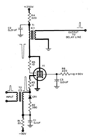
Figure 3-58. Delay Line Driver, Model A
