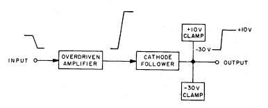
Figure 3-37. D-C Inverter, Simplified Block Diagram A positive level between 0 and  $\pm 12$  volts applied to the overdriven amplifier input is amplified and inverted and fed to the cathode follower, whose output circuit clamps the inverted level of  $\pm 30$  volts. Similarly, a negative level between  $\pm 8$  and  $\pm 30$  volts applied to the overdriven amplifier is amplified, inverted, and clamped at  $\pm 10$  volts at the cathode follower output.
