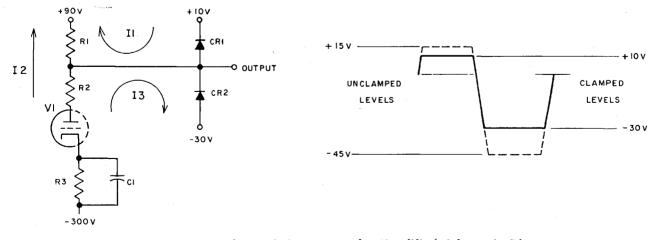
Figure 2–13. Diode Clamped Output Levels, Simplified Schematic Diagram
