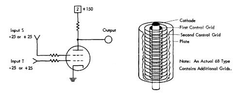
Figure 47. The Basic Circuit of the Pentagrid Switch Unit and a Cutaway View of a Simplified Tube for Use in the Circuit
