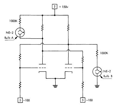
Figure 69. Neon Indicator Bulb Circuits for Triggers
