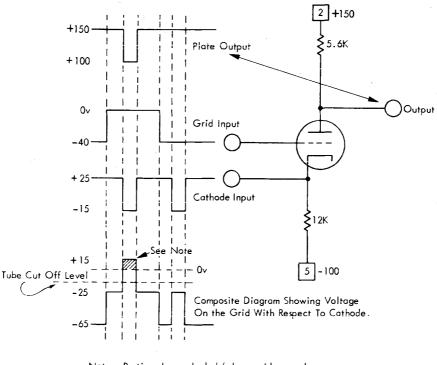
Note: Portion shown shaded (where grid goes plus with respect to cathode) will, if cathode is hot, be swamped due to grid current flow.
