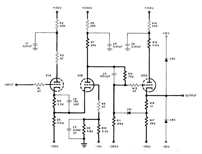
Figure 3-11. D-C Level Setter, Model B, Schematic Diagram
