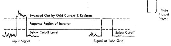
Figure 33. Clipping and Shaping
