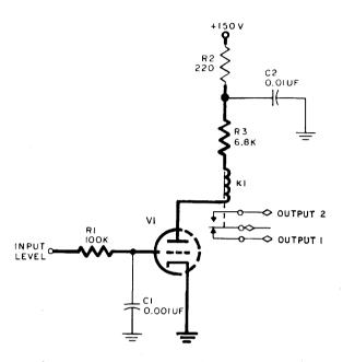
Figure 3-19. Vacuum-Tube Relay Driver, Model B, Schematic Diagram
