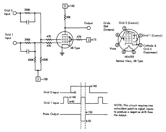
Figure 48. A Practical Pentagrid Switch Circuit Showing All Five Grids and the Base Connections for IBM 6B Class of Tubes
