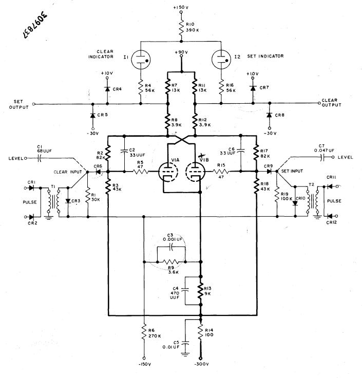
Figure 3-43. Flip-Flop, Model C, Schematic Diagram
