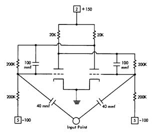
Figure 64. A Binary. Commoned Input Trigger
