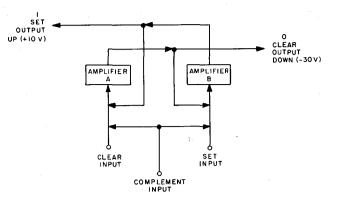
Figure 3–39. Flip-Flop, Block Diagram
