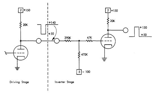
Figure 23. A Practical Inverter Circuit
