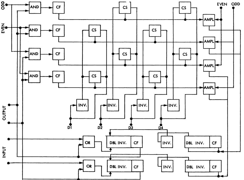
Fig. 29 - Capacitor Storage Cells Combined into a Matrix
