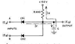
IF = ELECTRON FLOW DURING FALL TIME IR = ELECTRON FLOW DURING RISE TIME
