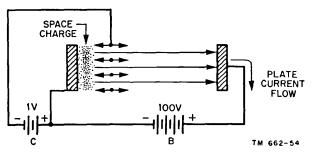
Figure 45. Electron flow in triode with control grid negative in relation to cathode.
