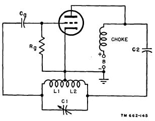
Figure 136. Shunt-fed Hartley oscillator.
