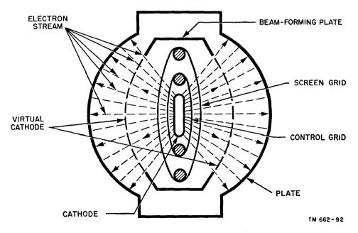
Figure 83. Effect of beam-forming plates on electron flow through beam power tube.
