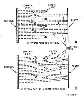
Figure 82. Electron paths in tetrode and beam-power tube.
