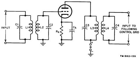
Figure 130. Transformer-coupled triode amplifier.
