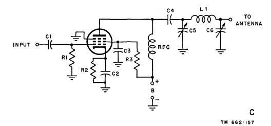
Figure 148. Single-ended power amplifier circuits.
