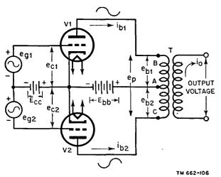
Figure 97. Push-pull triode amplifier circuit.
