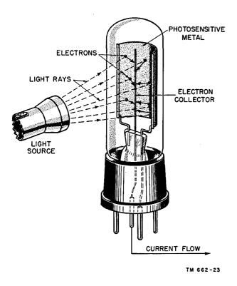
Figure 14. Photoelectric emission of electrons.
