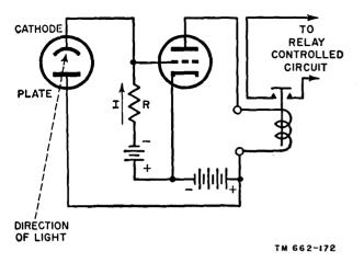
Figure 163. Basic phototube control circuit.
