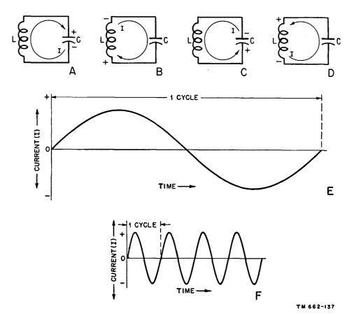
Figure 128. Oscillatory current in an L-C circuit.
