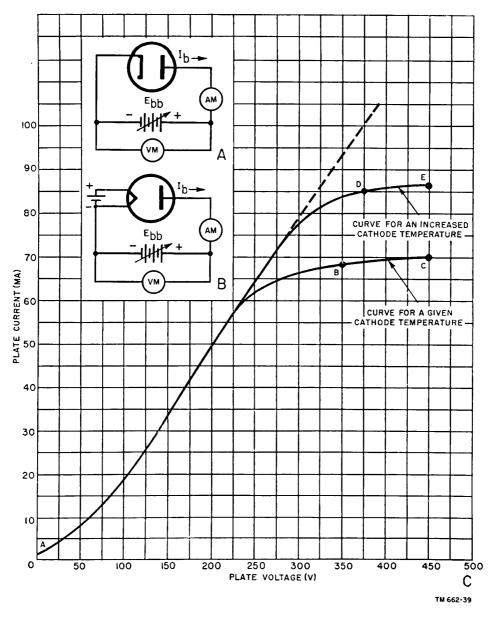
Figure 30. Plate-current plate-voltage characteristic curves.
