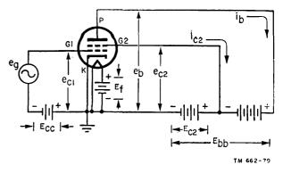
Figure 70. Circuit representation of tetrode.
