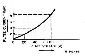
Figure 27. Curve illustrating completely nonlinear characteristic.
