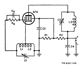
Figure 137. Electron-coupled oscillator.
