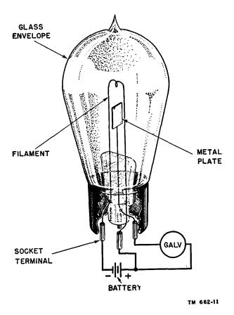
Figure 2. Circuit of Edison's two-electrode tube.
