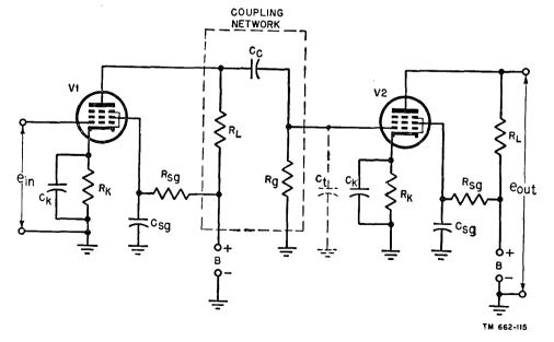
Figure 106. Typical R-C coupled amplifier using pentodes.
