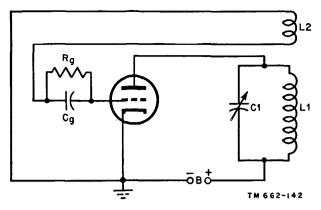
Figure 133. Tuned-plate oscillator.
