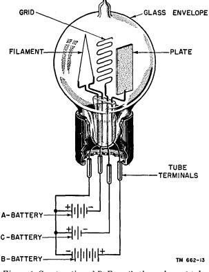
Figure 4. Construction of DeForest's three-element tube, or triode.
