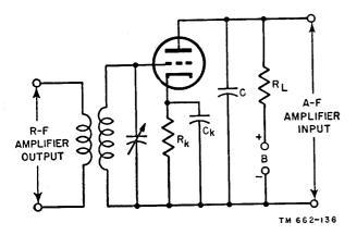
Figure 127. Diagram of plate detector.
