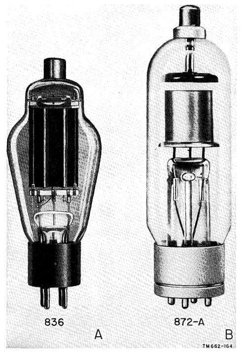
Figure 155. Typical transmitter half-wave rectifiers.
