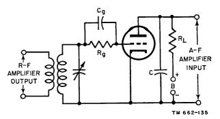
Figure 126. Circuit of grid-leak detector.
