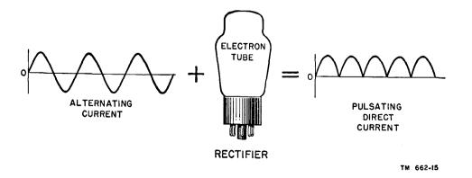
Figure 6. Function of tube as rectifier of alternating current.
