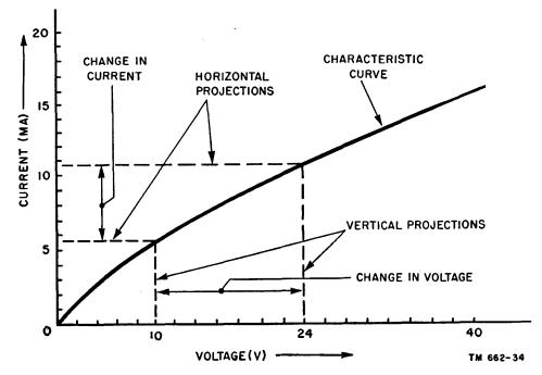
Figure 25. Plot of simple characteristic curve.
