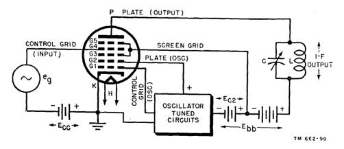
Figure 90. Pentagrid converter circuit.
