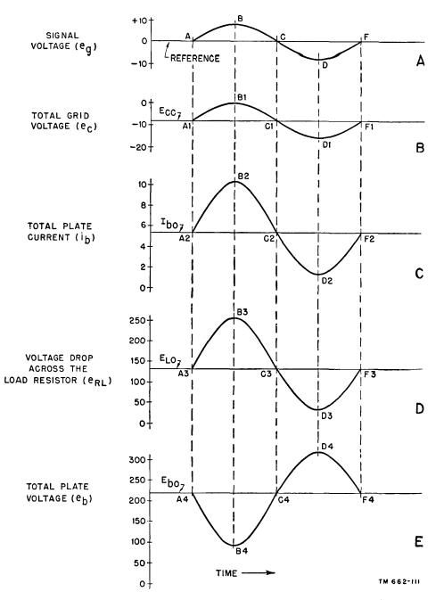
Figure 102. Waveforms in triode amplifier circuit.
