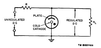
Figure 157. Simple voltage regulator circuit.
