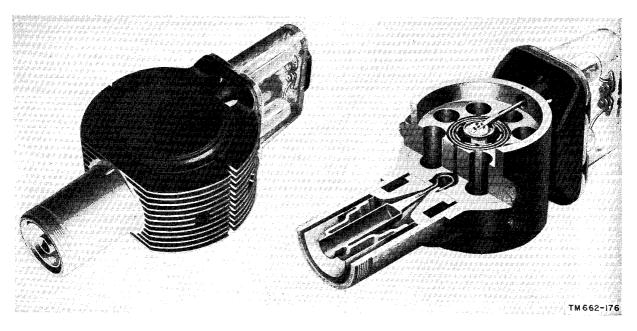
Figure 167. Operational and cutaway view of typical magnetron.
