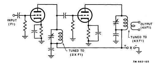
Figure 146. Frequency multiplier system with output frequency four times input frequency.
