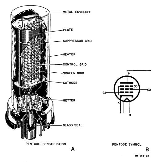
Figure 73. Physical construction (metal-type) and symbol of pentode.
