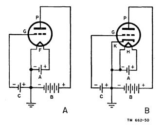
Figure 41. D-c supply voltages of directly and indirectly heated triodes.
