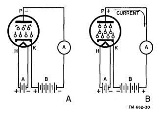
Figure 21. Different conditions of current flow through diode.
