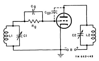
Figure 134. Tuned-plate tuned-grid oscillator.
