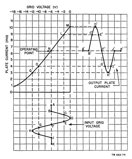
Figure 65. Operating on linear portion of 6J5 dynamic transfer characteristic (R<sub>L</sub> equal to 25,000 ohms).
