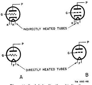
Figure 40. Symbols for directly and indirectly heated triodes.
