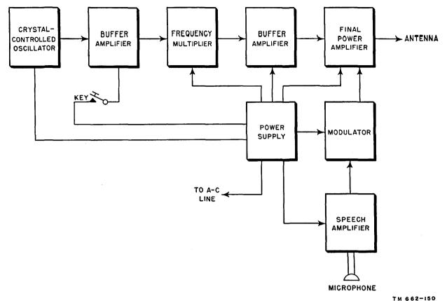
Figure 141. Block diagram of typical transmitter.
