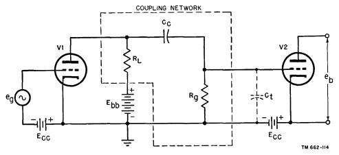
Figure 105. R-C coupling network between two triode amplifiers.
