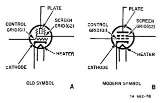
Figure 69. Tube symbols for tetrode.
