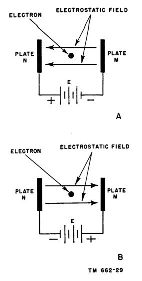
Figure 20. Electrostatic fields resulting from two plates and a battery.
