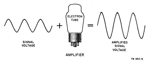
Figure 7. Function of tube as amplifier.
