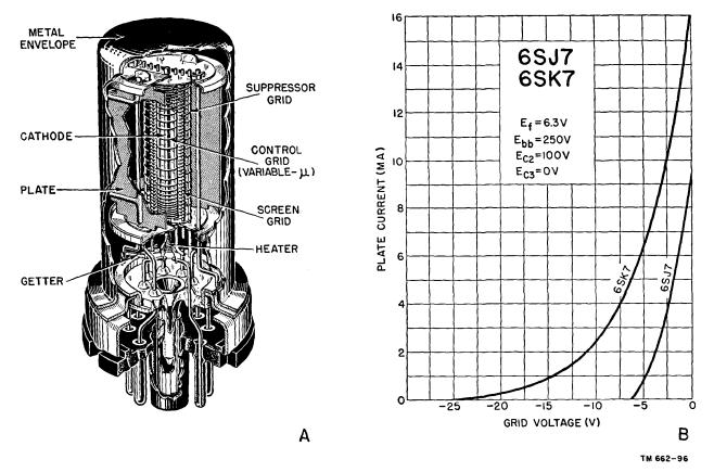
Figure 87. Construction of variable- $\mu$  pentode and its plate-current grid-voltage characteristic.
