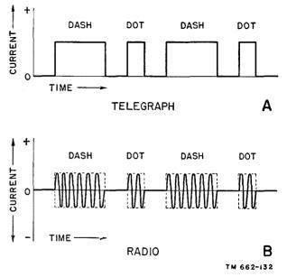
Figure 123. Current waveforms for code letter C.
