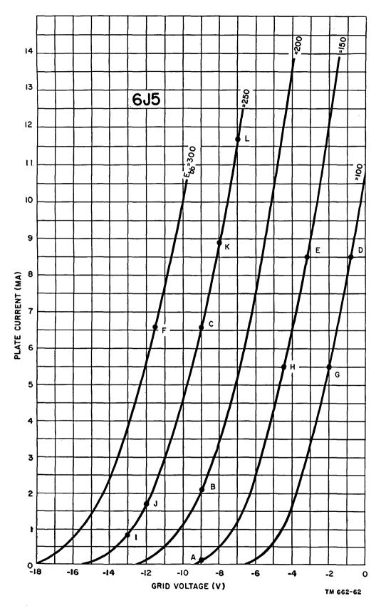
Figure 53. Grid family of characteristic curves for 6J5 triode.
