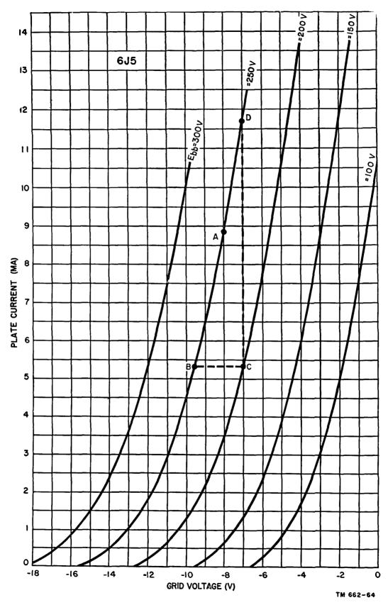
Figure 55. Grid family of curves used to determine amplifiaction factor of 6J5 triode.
