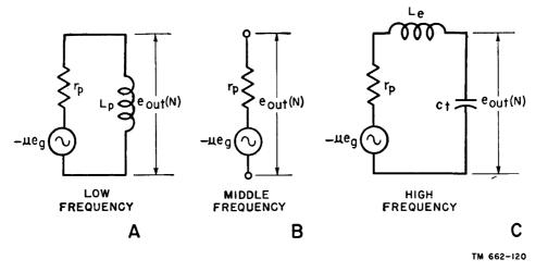
Figure 111. Equivalent circuits of transformer-coupled amplifier.
