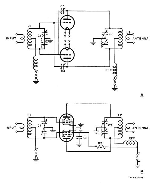
Figure 149. Push-pull power amplifier circuits.
