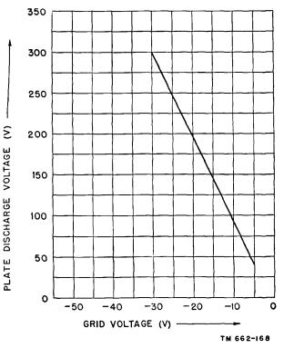
Figure 159. Grid-control characteristic of the 884.
