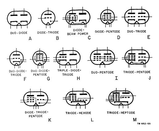
Figure 92. Tube symbols for multiunit tubes.
