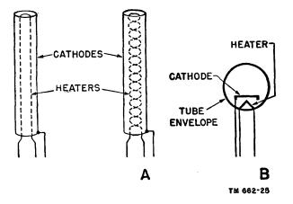
Figure 16. Indirectly heated emitter and schematic symbol.
