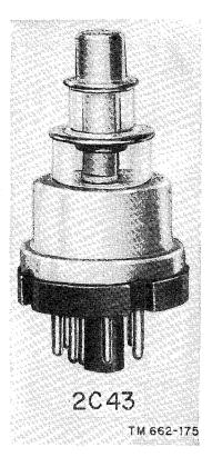
Figure 166. Lighthouse tube 2C43.
