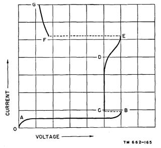
Figure 156. Graphical relations in gaseous conduction.
