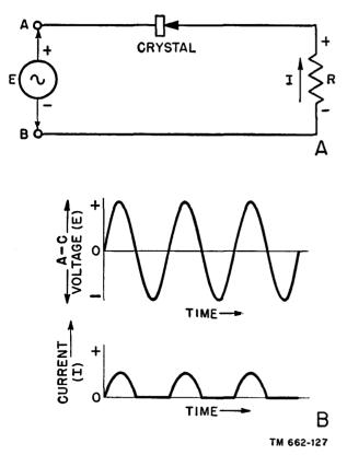
Figure 118. Crystal rectifier circuit and operating waveforms.
