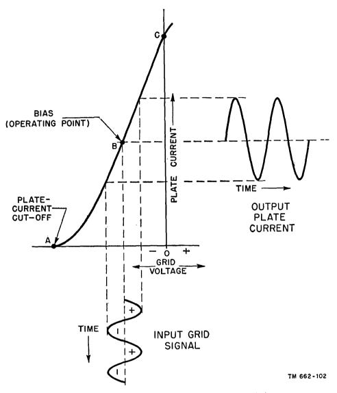
Figure 93. Class A operation on dynamic characteristic.
