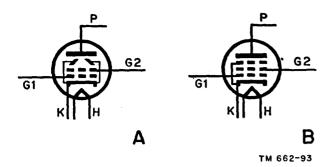
Figure 84. Symbols for beam power tubes.
