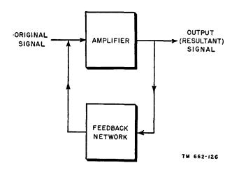
Figure 117. Block diagram of feedback amplifier.
