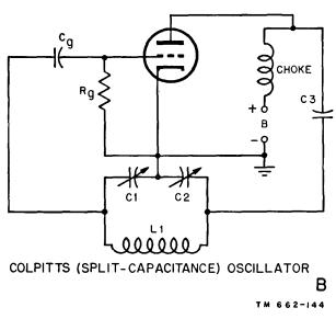
Figure 135. Split-tank oscillators.
