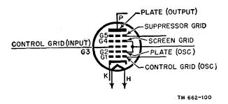
Figure 91. Another form of pentagrid converter.
