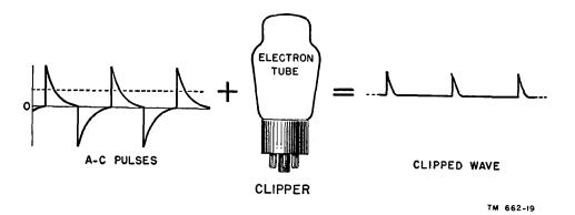
Figure 10. Another type of waveshaping. Only parts of the positive peaks of the input signal are present in the output.
