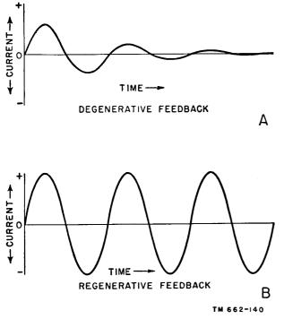
Figure 131. Waveforms showing effect of feedback.
