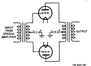
Figure 152. Class B amplifier, a high-level modulator.
