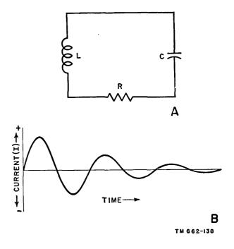
Figure 129. Damped oscillatory current in R-L-C circuit.
