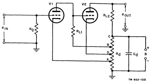
Figure 114. Typical direct-coupled amplifier using triodes.
