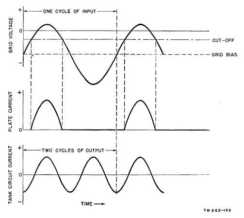
Figure 147. Voltage and current relationships in class C doubler.
