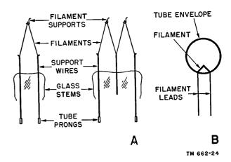
Figure 15. Directly heated filaments and schematic symbol.
