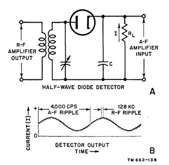
Figure 125. Half-wave diode detector circuit.
