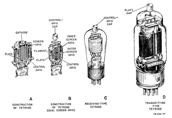
Figure 68. Physical construction of tetrodes.
