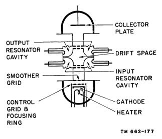
Figure 168. Operation of typical klystron.
