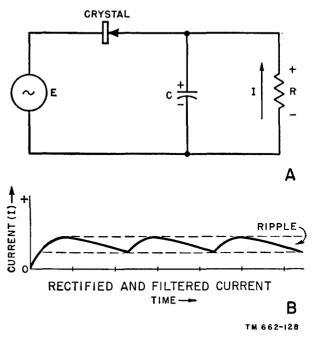
Figure 119. Crystal rectifier and filter.
