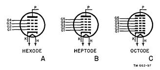
Figure 88. Schematic symbols of multigrid tubes.
