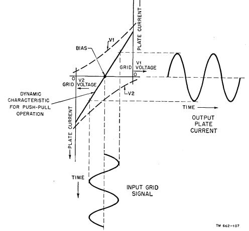
Figure 98. Dynamic characteristic of two tubes in push-pull class A operation.
