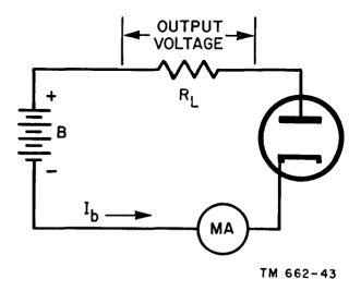
Figure 34. Adding a load resistor,  $R_L$ , to a diode circuit to obtain an output voltage.
