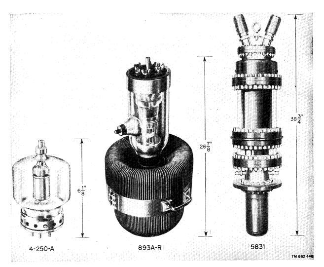
Figure 139. Three typical transmitting tubes.
