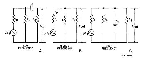
Figure 108. Equivalent circuit of R-C coupled amplifier.
