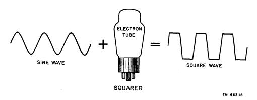
Figure 9. One type of waveshaping accomplished by electron tubes. The input signal is a sine wave; the output is a square wave.
