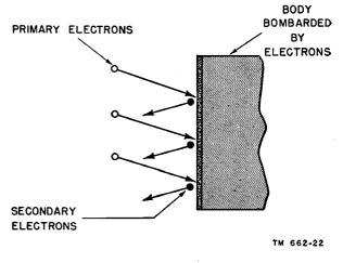
Figure 13. Secondary emission caused by electron bombardment.
