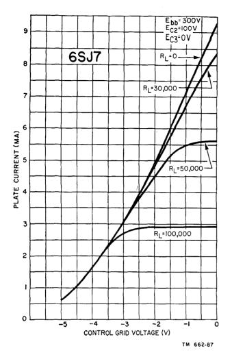
Figure 78. Dynamic transfer characteristic curves of 6SJ7 pentode.
