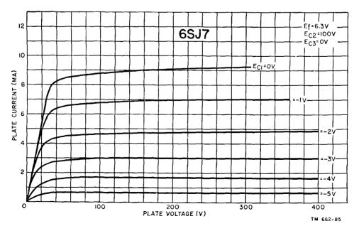
Figure 76. Plate family of characteristic curves for pentode.
