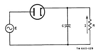
Figure 120. Half-wave diode rectifier circuit.
