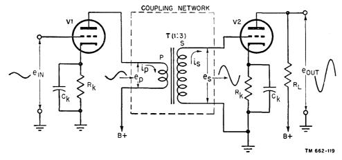
Figure 110. Transformer-coupled amplifier using triodes.
