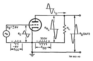
Figure 101. Current and voltage phase relations in triode amplifier circuit.
