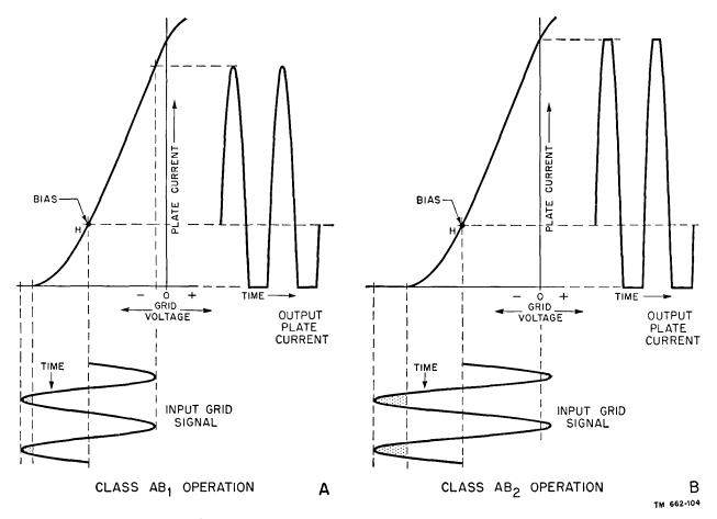
Figure 95. Class AB operation on dynamic characteristic.
