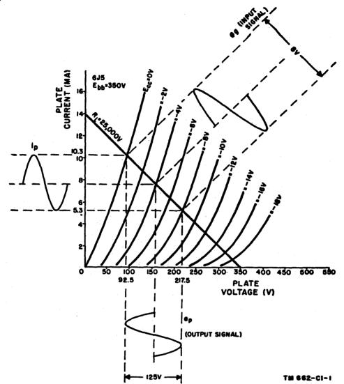
Figure 61.1. (Added) Plate characteristics showing signal voltage amplification.
