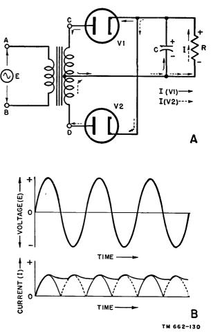
Figure 121. Full-wave diode rectifier circuit.
