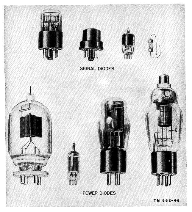
Figure 37. Various types of high-vacuum diodes.
