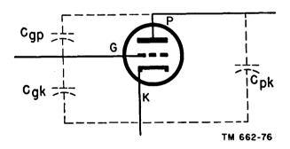
Figure 67. Location of interelectrode capacitances within triode.
