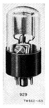
Figure 160. Typical phototube.
