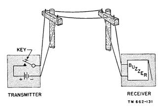
Figure 122. Simple telegraph circuit for communication.
