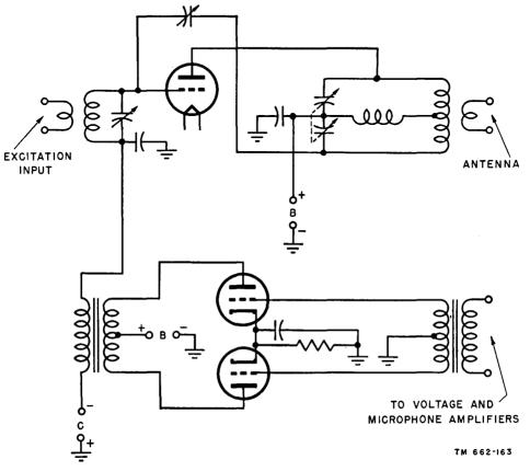
Figure 154. Grid-modulated amplifier.
