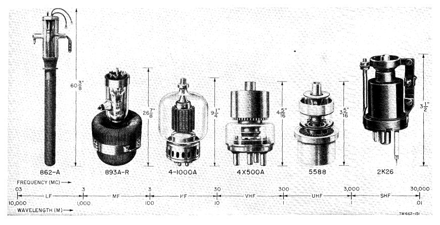
Figure 142. Typical transmitting tubes used in r-f spectrum.
