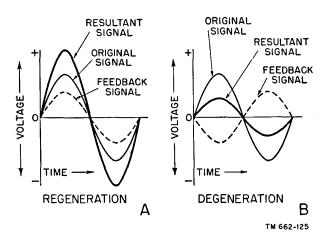
Figure 116. Phase relationships of signals producing regeneration and degeneration.
