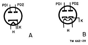
Figure 19. Other schematic representations of duo-diodes.
