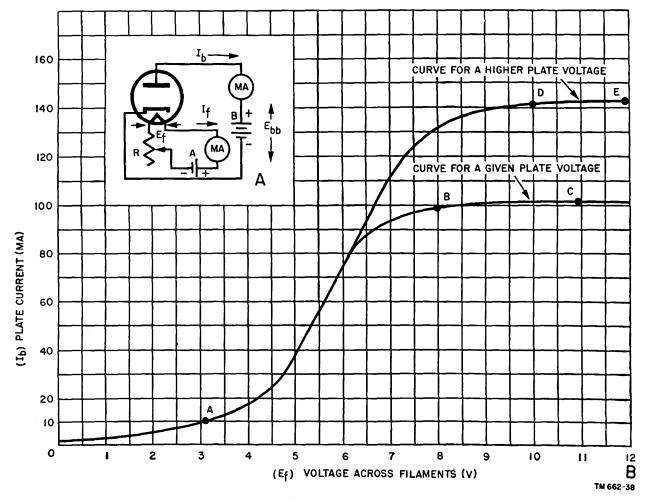
Figure 29. Plate-current filament-voltage characteristic curves.
