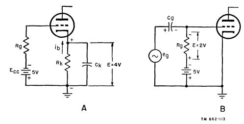
Figure 104. Circuits showing combination bias.
