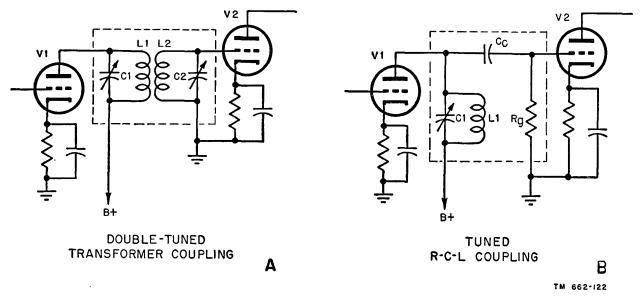
Figure 113. Tuned-circuit coupling system.
