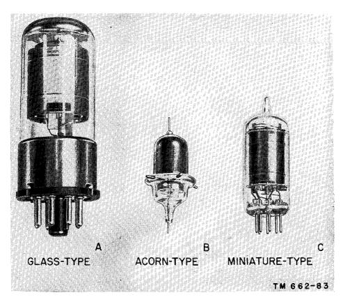
Figure 74. Different types of receiving pentodes.
