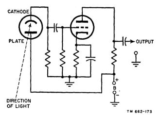
Figure 164. Phototube circuit for reproduction of sound.
