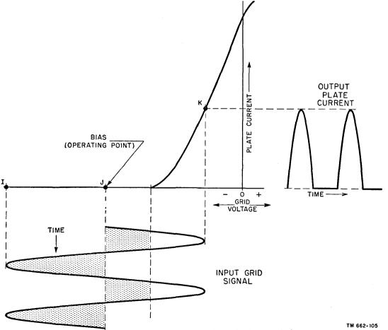
Figure 96. Class C operation on dynamic characteristic.
