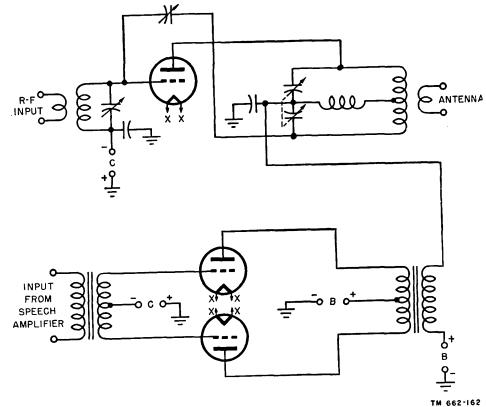
Figure 153. Plate-modulated power amplifier.
