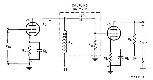
Figure 109. R-C-L coupled amplifier using triodes.
