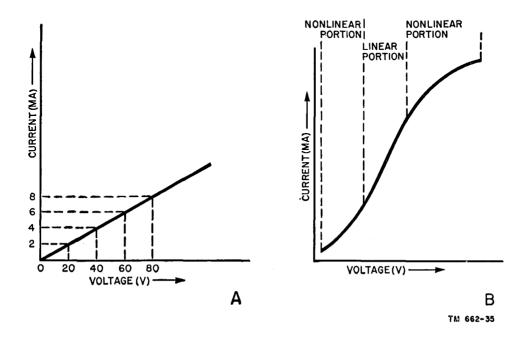
Figure 26. Linear and nonlinear characteristic curves.
