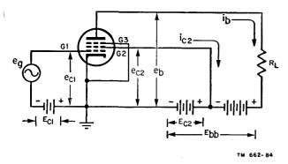
Figure 75. Circuit representation of pentode.
