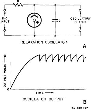
Figure 158. Relaxation oscillator and waveform produced.
