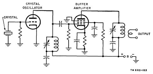
Figure 144. Crystal oscillator and buffer amplifier.
