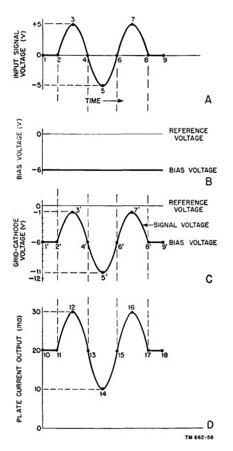
Figure 49. Waveshapes illustrating bias, signal voltage, and plate current.
