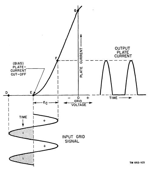
Figure 94. Class B operation on dynamic characteristic.
