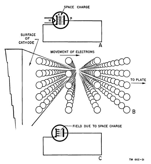
Figure 22. Electron accumulation in diode.
