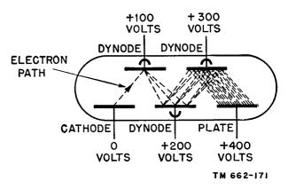
Figure 162. Operation of secondary-emission multiplier.
