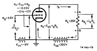
Figure 64. Basic circuit of triode, including input signal and load.
