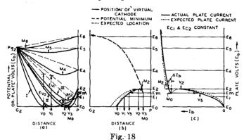
(a)—Potential distribution in a tetrode with high space-charge density between screen and plate.
