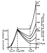
Fig. 10-Calculated effective potentials in a typical power pentode.
