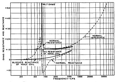
Fig. 1-Electrical characteristics of a dynamic loud-speaker.
