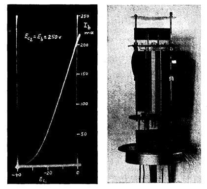
Fig. 27—Transfer characteristic of type 6L6 beam power tube.
