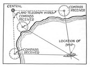
Showing how the radio compass functions.
