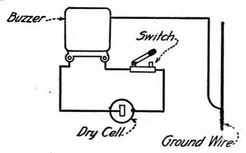
Details of a busser testing oufit used in the adjustment of crystal detectors.
