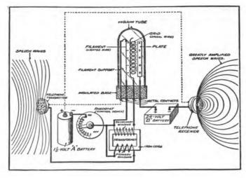
A diagrammatic explanation of the operation of the vacuum tube amplifier for the deaf.
