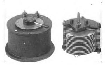
The type of variable condenser used in radio receiving circuits
