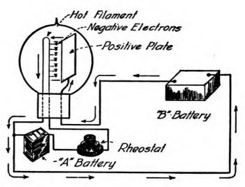
Diagram showing principle of the two-element vacuum tube.
