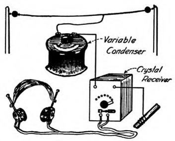
How a variable condenser is connected between the aërial and receiving outfit to reduce the wave-length.
