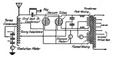
Transmitter No. 4. A ten-watt combination telegraph transmitter.
