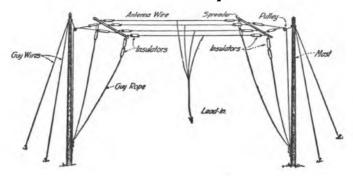
Constructional details of a large four-wire aërial suitable for general amateur use.
