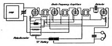
Connections for a radio-frequency amplifier using the loop or indoor antenna. This is receiving outfit No. 8.
