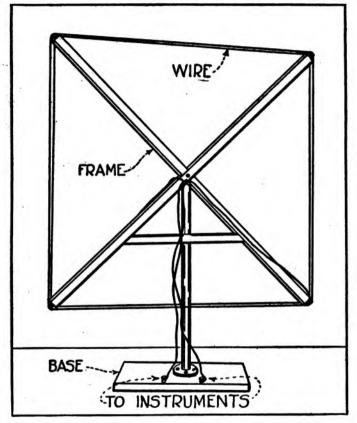
Construction of a loop antenna. It is made by winding several turns of wire around a four-foot frame.
