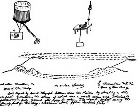
A particularly significant sketch copied from Dr. Loomis's notebook. The apparatus shown in the upper right-hand corner closely resembles the oscillator used in the early Marconi experiments. It has both the aërial and the ground connection. The lower sketch illustrates the Loomis theory of radio transmission. The upper left-hand corner illustrates the receiver. The handwriting is that of Dr. Loomis.
