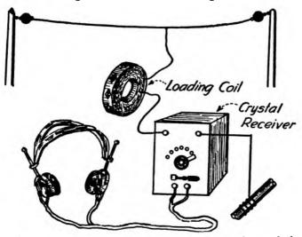
How a loading coil is connected between the aërial and ground of a crystal receiver to increase the wave-length.
