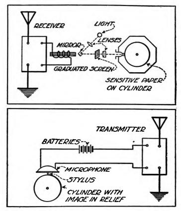
A diagram of the transmitting and receiving apparatus used in the Belin system.
