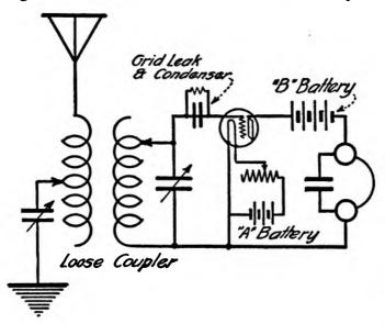
A simple vacuum tube receiver employing the grid leak and grid condenser. This is receiving outfit No. 5.
