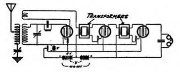
Connections for a two-stage vacuum tube amplifier using the regenerative principle. This is receiving outfit No. 7.
