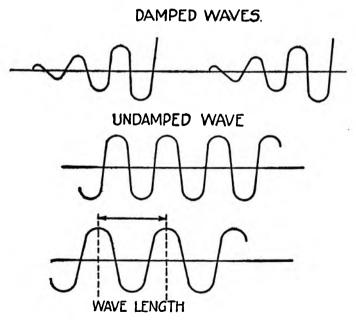
A diagrammatic representation of damped and undamped waves. The meaning of wave-length will be gathered from the bottom diagram
