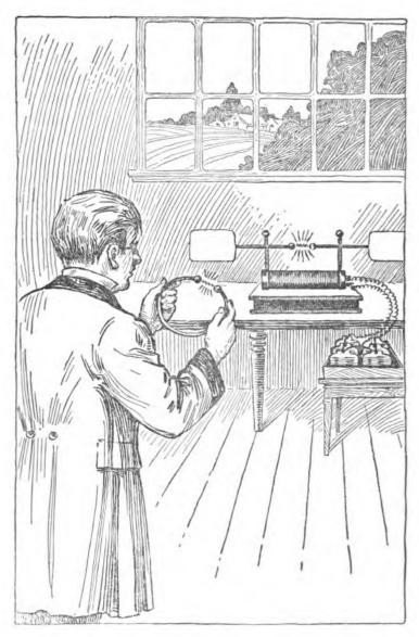
The first wireless or radio transmitter and receiver used by Professor Hertz. Hertz, working this simple apparatus, paved the way for the later triumphs over space and time in the transmission of human intelligence.
