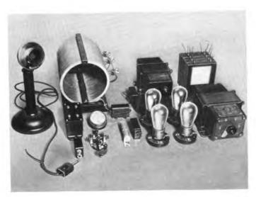
Neccessary apparatus for a twenty-watt vacuum tube telephone transmitter
