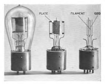
The various parts of a vacuum tube
