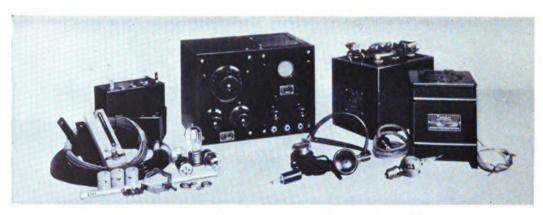
Complete set of apparatus necessary for a two-stage amplifying receiver. The auxiliary apparatus pictured follows: Storage battery, "B" batteries, three vacuum tubes, charging outfit for storage battery, telephones, aërial wire, lightning arrester, and insulators. A loud speaker can be used in place of the telephones
