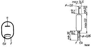
Fig. 2 Electrode connections and dimensions of the EY 51.
