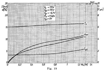
Anode current, screen-grid current, input voltage and total distortion of **pentode section** plotted against output power for anode and screen-grid voltage of 170 V.
