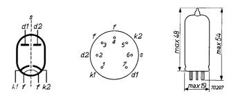
Fig. 6 Base connections and dimensions of the EB 91.
