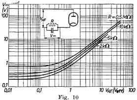
Fig. 10 Direct voltage at the load resistor plotted against the H.F. signal, with the load resistance as parameter. The curves refer to one diode section.
