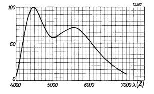
Fig. 9 Spectral energy emission characteristic of the screen.
