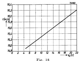
Relation between the multivibrator frequency and the anode voltage of the coincidence detector.
