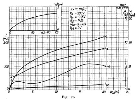
Anode current, screen-grid current, input voltage and total distortion plotted against output power of two valves PL 81 in push-pull B for anode and screengrid supply voltage of 200 V.
