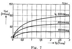
The intercarrier voltage at the load of the detector diode plotted against the picture carrier voltage at the input of the detector, with the sound carrier voltage at the input of the detector as parameter.
