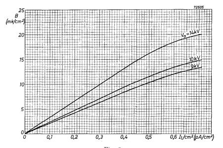
Fig. 8 Brightness plotted against beam current per square em screen area with the anode potential as parameter.
