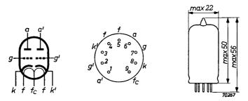
Fig. 6 Base connections and dimensions of the ECC 81.
