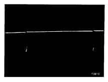
Fig. 51 Anode current pulses of the triode section of  $V_{19}$ . The pulse amplitude is 110 mA.
