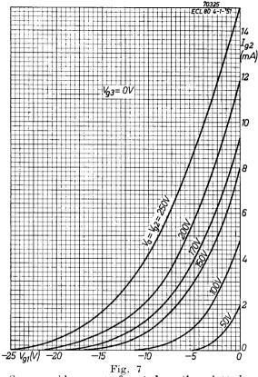
Fig. 7 Screen-grid current of **pentode section** plotted against control-grid voltage for anode and screen-grid voltages between 50 V and 250 V.
