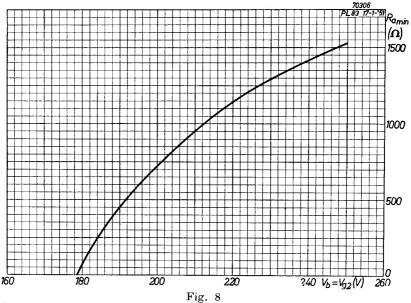
Minimum permissible anode load resistance plotted against supply and screengrid voltage.
