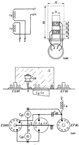
Fig. 14 a. Dimensions in mm of the transformer  $L_{\mathfrak{g}}L_{7}$ . b. Position on the receiver chassis. a
