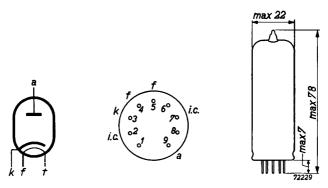
Fig. 2 Base connections and dimensions of the PY 82.
