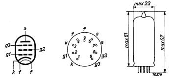
Fig. 8 Base connections and dimensions of the EF 80 pentode.
