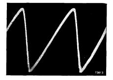
Fig. 44 Saw tooth current in the line coils. The peak-to-peak value is 1050 mA.
