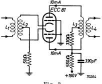
Fig. 3 The ECC 81 as R.F. amplifier in a grounded-grid circuit, with the two sections in push-pull.
