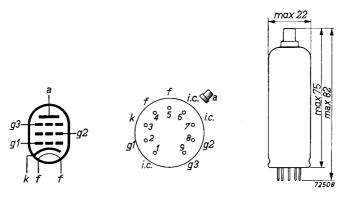
Fig. 18 Base connections and dimensions of the PL 81.
