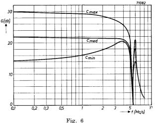
The video gain plotted against frequency. The curve marked  $c_{\max}$  corresponds to the condition when  $R_{10}$  is adjusted for maximum contrast,  $c_{med}$  to an average contrast control setting and  $c_{\min}$  to minimum contrast.
