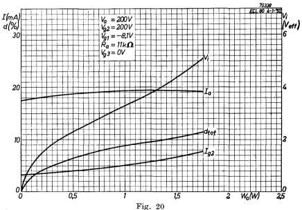
Anode current, screen-grid current, input voltage and total distortion of **pentode section** plotted against output power for anode and screen-grid voltage of 200 V.
