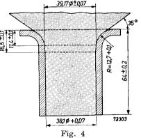
Reference line gauge (dimensions in mm). The deflection coils may not extend into the shaded area.
