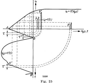
Operation of the EQ 80 as phase detector. This figure represents the case when the fifth grid is connected to the cathode.
