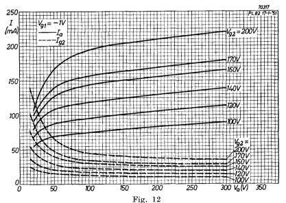
Anode current and screen-grid current plotted against anode voltage for control-grid voltage of -1 V, with screen-grid voltage as parameter.
