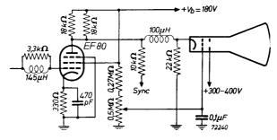
Fig. 7 The EF 80 as a video amplifier with cathode compensation.
