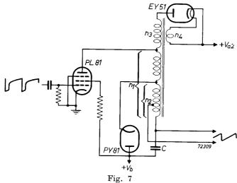
Line-output circuit in which the PY 80 is replaced by a PY 81 booster diode. With the PY 81 it is no longer necessary to feed the heater via a bifilar winding.
