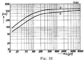
A.F. voltage  $V_0$  at the video detector load plotted against the R.F. signal  $V_i$  at the aerial terminals. The curves were measured in channel 2 at the picture carrier frequency and with a 30 % modulated signal. Curve *a* refers to the contrast control adjusted for maximum contrast and curve *b* to minimum contrast.
