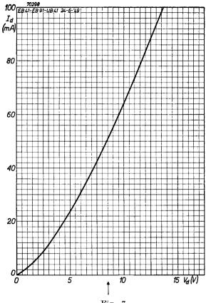
Fig. 7 Anode current plotted against anode voltage for each diode.
