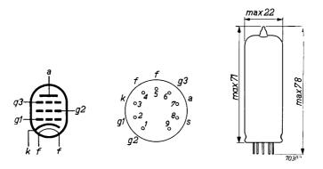
Fig. 4 Base connections and dimensions of the PL 83.
