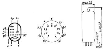
Fig. 4 Base connections and dimensions of the ECL 80.
