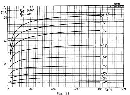
Anode current of **pentode section** plotted against anode voltage for screen-grid voltage of 200 V, with control-grid voltage as parameter.
