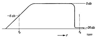
Fig. 3 Required shape of the response curve for intercarrier sound.
