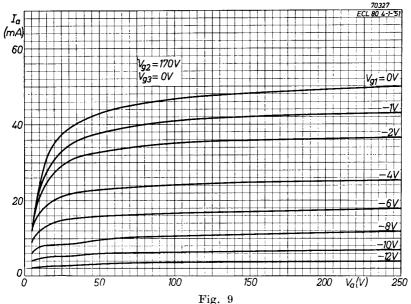
Anode current of pentode section plotted against anode voltage for screengrid voltage of 170 V, with control-grid voltage as parameter.
