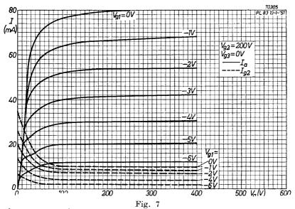
Anode current and screen-grid current plotted against anode voltage for screen-grid voltage of 200 V, with control-grid voltage as parameter.
