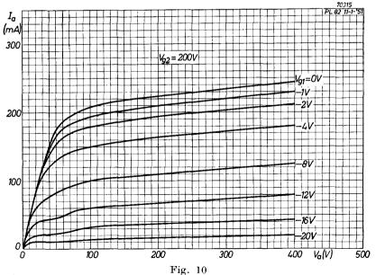
Anode current plotted against anode voltage for screen-grid voltage of 200 V, with control-grid voltage as parameter.
