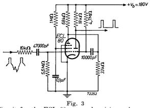
Circuit for the ECL 80 as synchronizing pulse separator and amplifier.
