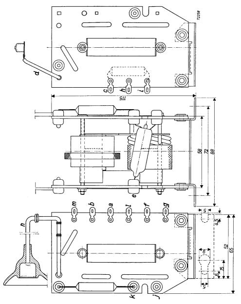
Fig. 15 Dimensions of the line-output transformer Type AT 2000. The indications at the various terminals correspond to those of the circuit diagram of Fig. 8.
