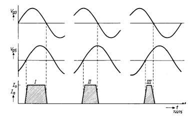
Fig. 9 Anode current of the EQ 80 for different phase angles between the signal voltages at the third and the fifth grids.
