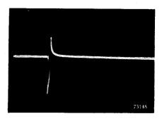
Fig. 52 Flyback voltage at the anode of the triode section of  $V_{19}$ . The peakto-peak value is 375 V.
