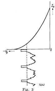
Signal at the control grid of the single video stage.
