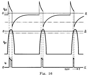
Voltages on the third and the first grids of the pentode and the resulting anode current pulses.
