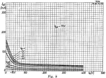
Screen-grid current plotted against anode voltage for screen-grid voltage of 170 V, with control-grid voltage as parameter.
