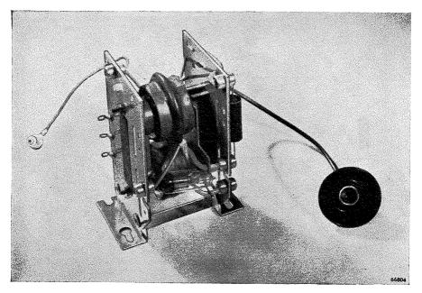
Fig. 14 The line-output transformer Type AT 2000
