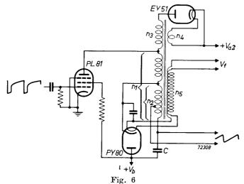
Line-output circuit with booster diode in which an autotransformer is used. The heater of the PY 80 booster must be fed via a bifilar winding on the transformer.
