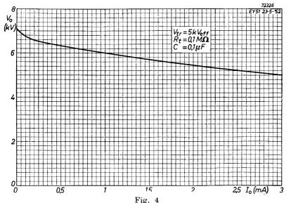
Fig. 4 Rectified output voltage of the EY 51 plotted against the output current, for a sinusoidal input voltage of 5 kV<sub>rms</sub> and a limiting resistance of 0.1 M $\Omega$ .
