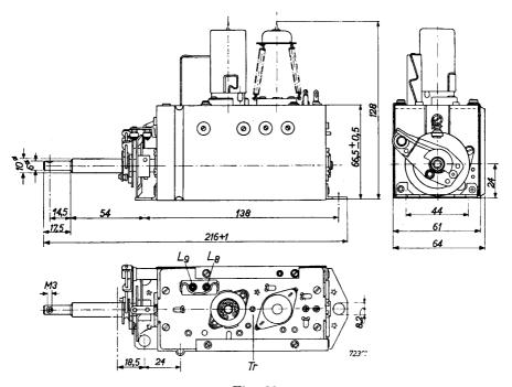
Fig. 31 Dimensions of the channel selector Type AT 7501.
