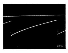
Fig. 56 Saw-tooth voltage across the charge capacitor  $C_{131}$ . The peak-to-peak value of the saw-tooth is 145 V, the negative voltage at the end of the stroke being 35 V.
