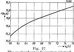
The multivibrator frequency plotted against the anode voltage of the phase detector.
