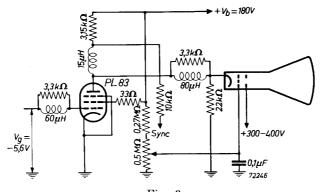
Fig. 3 The PL 83 as video amplifier with anode compensation. The stopper resistor in the screen-grid lead should not be higher than 33  $\Omega$ .
