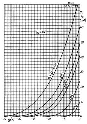
Fig. 5 Anode current of **pentode section** plotted against control-grid voltage for anode and screen-grid voltages between 50 V and 250 V.
