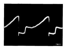
Fig. 47 Cathode current (peak-to-peak value 270 mA) of the output pentode PL 81.
