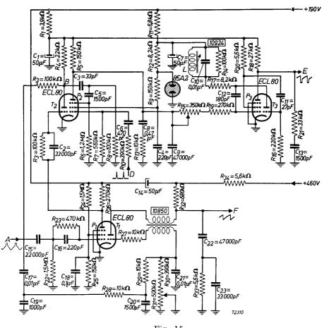
Fig. 15 Circuit for flywheel synchronization, with the pentode section of an ECL 80 triode pentode as coincidence detector.
