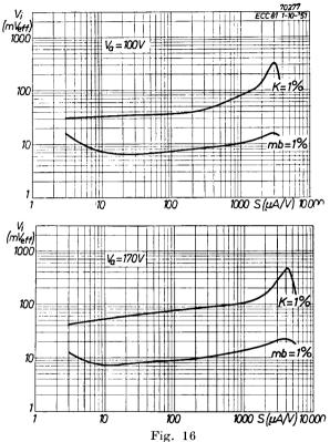
R.m.s. value of an interfering signal which results in a cross modulation of K = 1%, and hum voltage giving a modulation hum of 1%, plotted against the mutual conductance, for anode voltages of 100 and 170 V respectively.
