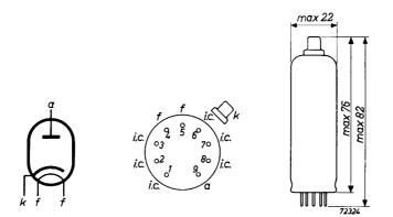
Fig. 2 Base connections and dimensions of the PY 81.
