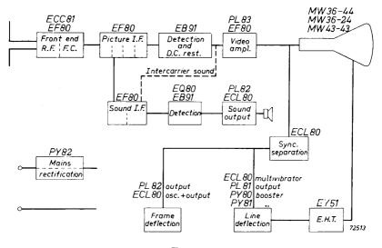
Fig. 1 Block diagram of a typical television receiver.
