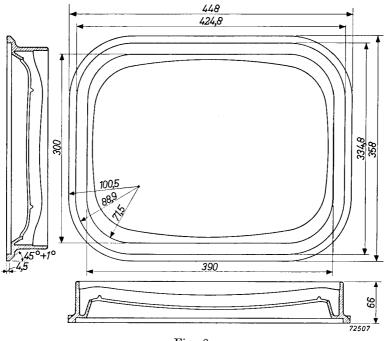
Fig. 8 Dimensions in mm of the mask Type 55404.
