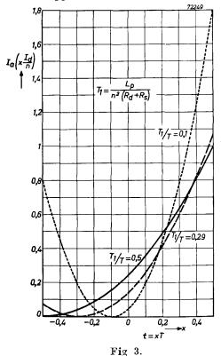
Shape of the total anode current required to give a linear deflection current, for different values of  $T_1/T$ .
