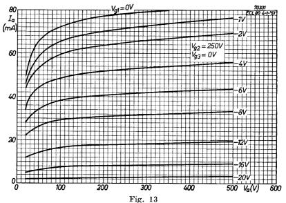
Anode current of pentode section plotted against anode voltage for screen-grid voltage of 250 V, with control-grid voltage as parameter.
