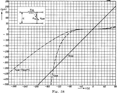
Voltage-current characteristics of the VDR resistor  $R_{114}$ , the fixed resistor  $R_{113}$  and of the combination of these two.
