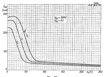
Fig. 23 Screen-grid current plotted against anode voltage for screen-grid voltage of 200 V, with control-grid voltage as parameter.
