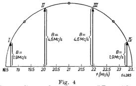
Stagger diagram for a three-stage I.F. amplifier centred at 21 Mc/s.
