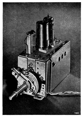
Fig. 30 Channel selector Type AT 7501.
