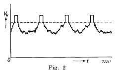
Polarity of the signal required at the cathode of the picture tube.
