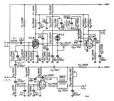
Fig. 21 Circuit for flywheel synchronization with the EQ 80 enneode as phase detector.
