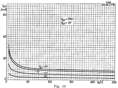
Screen-grid current of **pentode section** plotted against anode voltage for screen-grid voltage of 170 V, with control-grid voltage as parameter.
