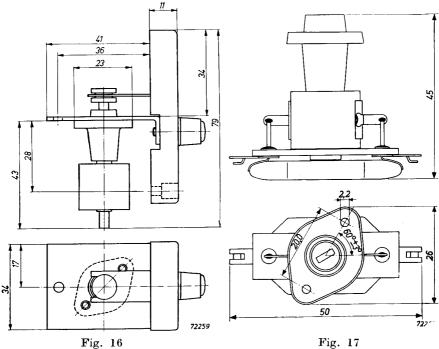
Dimensions of the picture width control Type AT 4000.
