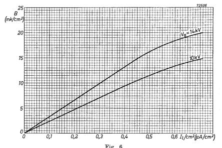
Fig. 6 Brightness plotted against the beam current per square cm screen area, for anode potentials of 10 and 14 kV.
