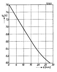
Fig. 28 Anode voltage at the phase detector plotted against the horizontal displacement of the picture. The displacement corresponds to a total picture width of 29 cm.
