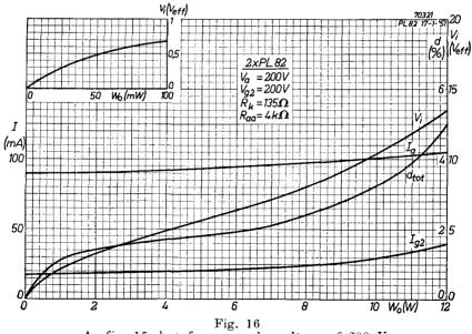
As fig. 15, but for a supply voltage of 200 V.
