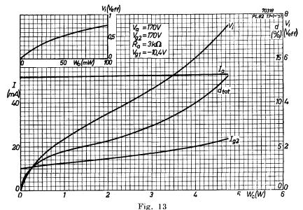
Anode current, screen-grid current, input voltage and total distortion of one PL 82 valve in Class A, plotted against output power for anode and screen-grid voltage of 170 V.
