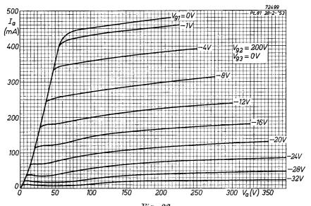
Fig. 22 Anode current plotted against anode voltage for screen-grid voltage of 200 V, with control-grid voltage as parameter.
