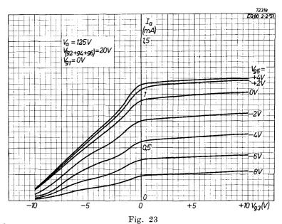
Anode current of the EQ 80 enneode plotted against the voltage on the third grid, with the voltage on the fifth grid as parameter.
