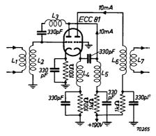
Fig. 4 The ECC 81 as cascode amplifier.
