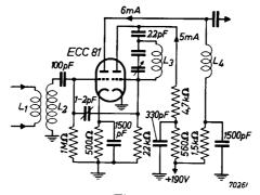
Fig. 5 Frequency changer circuit using the ECC 81, in which one section serves as mixer and the other as local oscillator.
