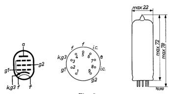
Fig. 5 Base connections and dimensions of the PL 82.
