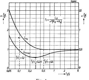
Fig. 4 Peak anode current and average anode current plotted against  $T_1/T$ .
