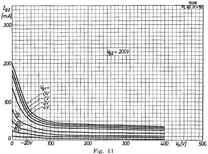
Screen-grid current plotted against anode voltage for screen-grid voltage of 200 V, with control grid voltage as parameter.
