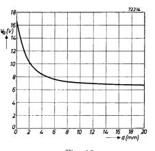
Fig. 19 Anode voltage of the coincidence detector plotted against the horizontal displacement of the picture. This displacement corresponds to a total picture width of 29 cm, as on an MW 36-24 picture tube.
