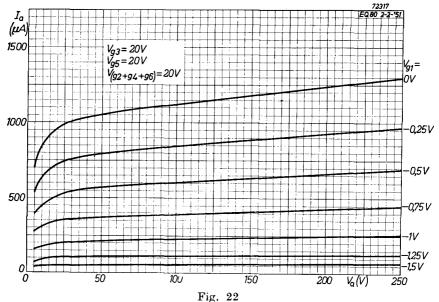
Anode current of the EQ 80 enneode plotted against the anode voltage, with the voltage on the first grid as parameter.
