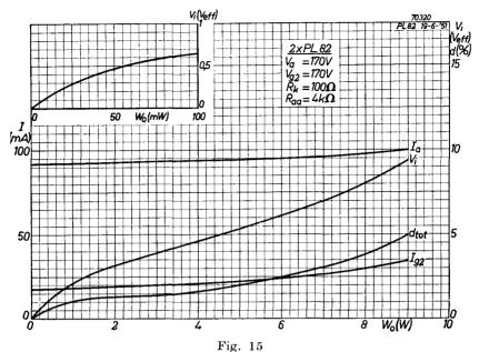
Anode current, screen-grid current, input voltage and total distortion plotted against output power of two valves PL 82 in push-pull for anode and screengrid voltage of 170 V. The currents indicated are of the two valves together.
