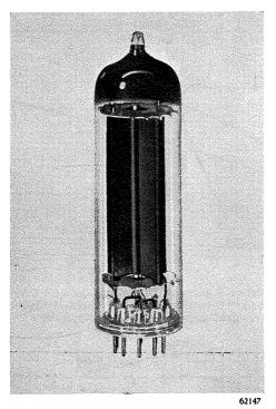
Fig. 1 The booster diode PY 80 (about actual size).
