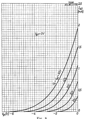
Fig. 8 Screen-grid current of **pentode section** plotted against control-grid voltage for anode and screen-grid voltages between 10 V and 50 V.
