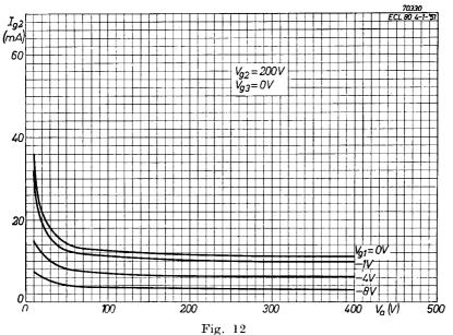
Screen-grid current of **pentode scetion** plotted against anode voltage for screengrid voltage of 200 V, with control-grid voltage as parameter.
