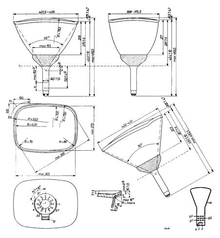
Fig. 2 Dimensional outline of the MW 43.43 (dimensions in mm). Notes:
