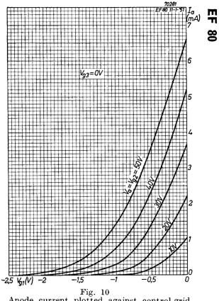
Fig. 10 Anode current plotted against control-grid voltage for anode and screen-grid voltages between 10 V and 50 V.
