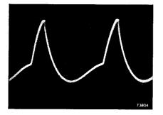
Fig. 36 Saw-tooth voltage at the third grid of the EQ 80 tube. The peak-to-peak value is 24 V.
