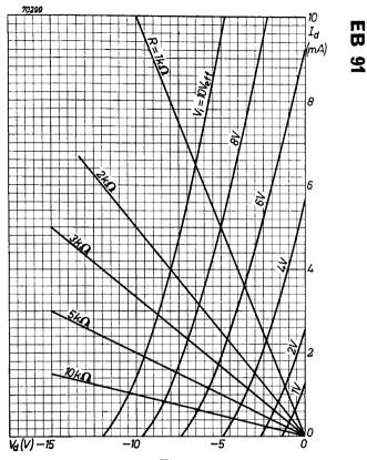
Fig. 8 Output characteristics for each diode, for input voltages between 1 and 10 V.
