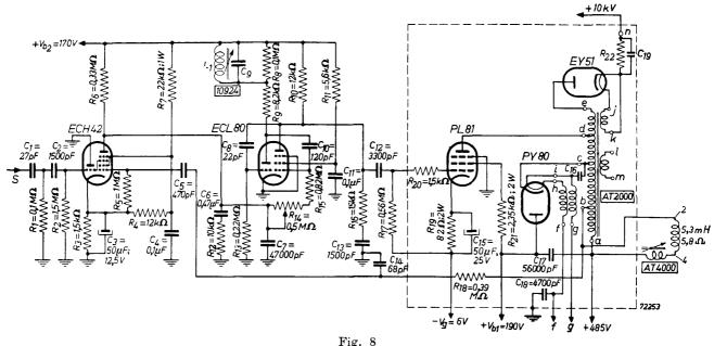
Fig. 8 Complete circuit for horizontal deflection and an E.H.T. of 10 kV.
