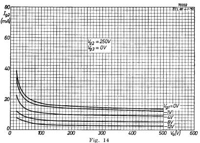
Screen-grid current of **pentode section** plotted against anode voltage for screen-grid voltage of 250 V, with control-grid voltage as parameter.
