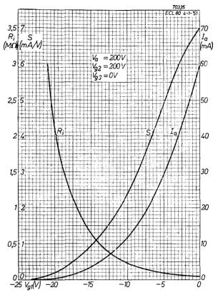
Anode current, mutual conductance and internal resistance of **pentode section** plotted against control-grid voltage for anode and screen-grid voltage of 200 V.
