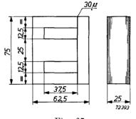
Fig. 67 Dimensions of the laminations of the output transformer for vertical deflection  $T_2$ . The thickness of the laminations is 0.5 mm.
