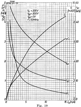
Control-grid voltage, mutual conductance, internal resistance, input capacitance variation and input damping (at 50 Mc/s) plotted against anode current for anode and screen-grid voltage of 200 V.
