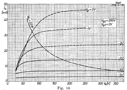
Anode current plotted against anode voltage for screen-grid voltage of 250 V, with control-grid voltage as parameter.
