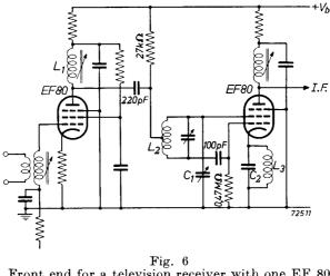
Front end for a television receiver with one EF 80 as R.F. amplifier and the other as self-oscillating frequency changer.
