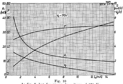
As fig. 9, but for an anode voltage of 170 V.
