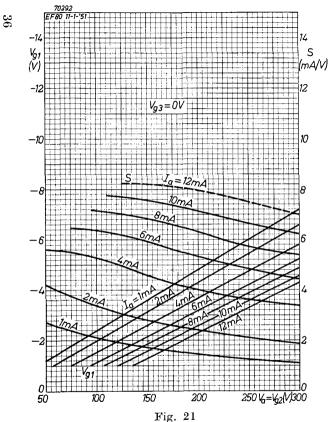
Fig. 21 Relation between control-grid voltage and mutual conductance and anode and screengrid voltage, with anode current as parameter.
