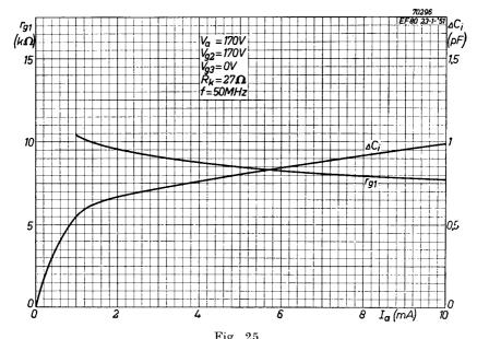
Fig. 25 Input capacitance variation and input damping at 50 Mc/s plotted against anode current in a cathode-compensated circuit ( $R_k = 27 \Omega$ ).
