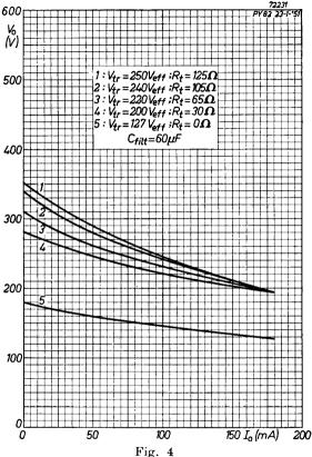
Rectified output voltage of the PY 82 plotted against the output current, with the alternating input voltage and the limiting resistor as parameters.
