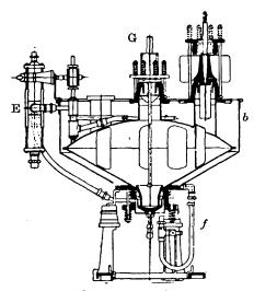
Fig. 84.—A.E.G. Rectifier for 500 amps.
