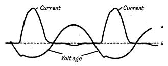
Fig. 58.—Current and Voltage Curves of a Glow Discharge Rectifier with Alkali Cathode. 120 Volts A.C. Input.
