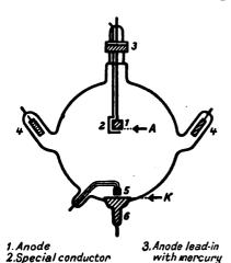
Fig. 8.—Large Spherical Vessel for the Elimination of Wall Disturbances.
