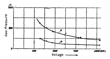
Fig. 64.—Dependence of Back-firing Voltage on Pressure.
