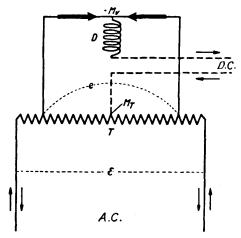
Fig. 34.—Transformer Circuit for Single-phase A.C.
