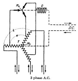
Fig. 35.—Transformer Circuit for Three-phase A.C.
