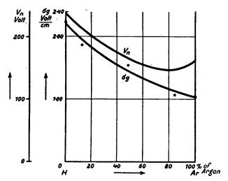
Fig. 7.—Variation of Normal Cathode Fall  $V_n$  and Normal Gradient  $\sigma_q$  with Composition of the Mixture of  $H_2$ -Ar.
