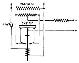
Fig. 50.—Connections of Pendulum Rectifier of the Hydrawerke for 100-130 Volts A.C.
