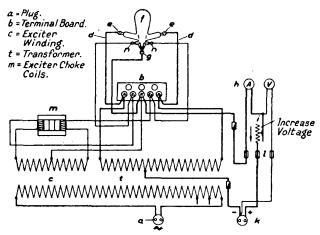
Fig. 80.—Connections of 5-10 amps. Accumulator Charging Rectifier.
