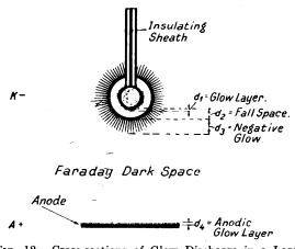
Fig. 12.—Cross-sections of Glow Discharge in a Large Vessel.
