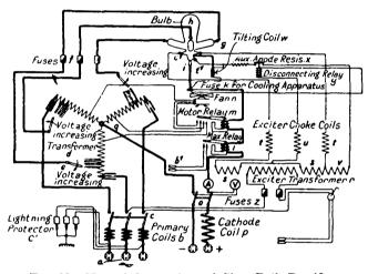
Fig. 66.—Normal Connections of Glass Bulb Rectifier.
