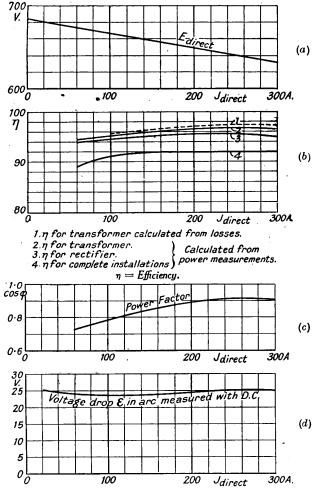
Fig. 73.—Various Graphs obtained by Idelberger and Schenkel.
