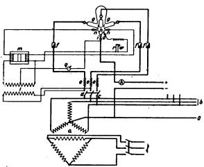
a-Main Transformer. b=3-phase Mains. e-Primary Choke Coils. 1-Exciter Transformer. o-Mains Neutral Wire. r-Exciting Switch.
