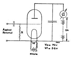
Fig. 91.—Connections of Moullin Voltmeter, Type B.
