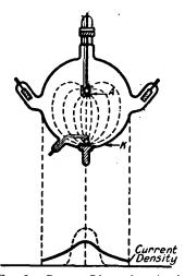
Fig. 9.—Current Lines of an Arc in a Large Vessel containing Pure Mercury Vapour.
