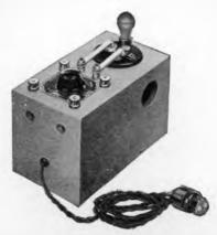
Fig. 55.—Tantalum Rectifier for Trickle Charging.
