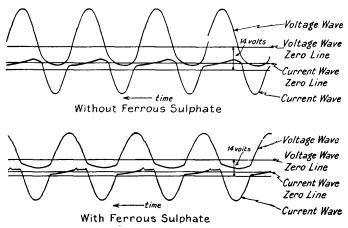
Fig. 54.—Effect of adding Ferrous Sulphate to Tantalum Rectifier.
