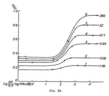
is a resistance across  $k_1k_2$ , representing the load.  $R_1$  is the resistance between the condenser and the valves. The curves show that v approximates more and more closely to  $V_0$ , and the voltage fluctuations become smaller and smaller, as  $R_2$ , w and C increase and  $R_1$  decreases.
