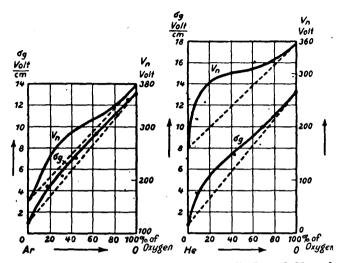
Fig. 5.—Variation of Normal Cathode Fall  $V_n$  and Normal Gradient  $\sigma_q$  with Constitution of Mixtures of Argon and Oxygen.
