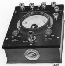
Fig. 90.—Moullin Voltmeter, Type B.
