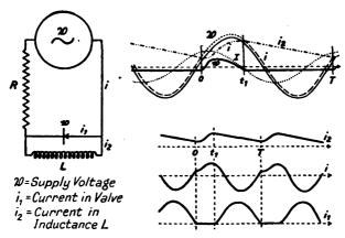
Fig. 47.—Resistance in Series and Inductance in Parallel with Valve.
