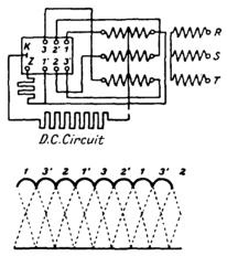
Fig. 36.—Connections and Output Curve of Haxaphase Rectifier.
