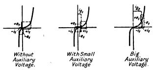
Fig. 31.—Influence of Auxiliary Voltage on Rectification.
