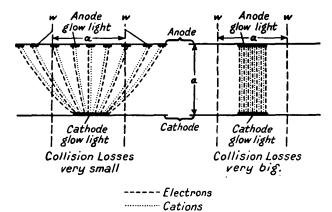
Fig. 4.—Lines of Flow of Electrons and Cations between Plane Parallel Electrodes.
