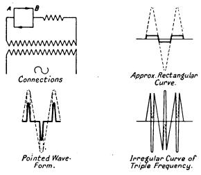
Fig. 94.—Production of any Wave Form.
