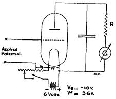
Fig. 88.—Connections of Moullin Voltmeter, Type A.
