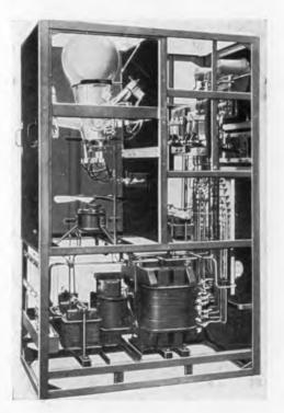
A.E.G. GLASS BULB RECTIFIER INSTALLATION.
