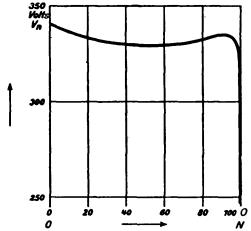
Fig. 17.—Normal Cathode Fall  $V_n$  in the Mixture  $O_2$ — $N_2$  using an Iron Cathode.
