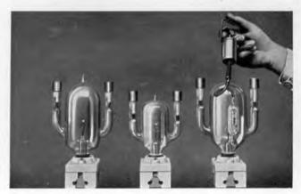
Fig. 86.—Wehnelt High Voltage Valves.
