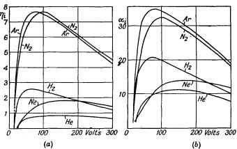
Fig. 14.—Curves obtained by Hughes and Klein, showing  $\eta_i$  the number of pairs of ions produced by an electron per cm. (at 1 mm. pressure) and  $a_i$  the percentage of ionising collisions.
