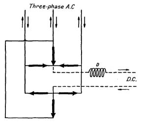
Fig. 33.—Grätz Circuit for Three-phase A.C.
