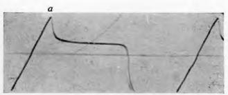
Fig. 25.—Voltage at One Arm of a 10 Amp. Multiphase Rectifier.
