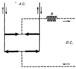
Fig. 32.—Grätz Circuit for Single-phase A.C.
