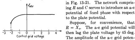
FIG. 13-20. The average plate current in a thyratron as a function of the d-c grid-bias potential.
