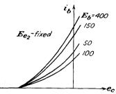
tial variation in which the plate current decreases with increasing plate potential. This region is one of negative plate resistance, since an increasing plate potential is accompanied by a decreasing plate
