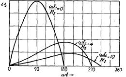
FIG. 14-2. The effect of changing inductance on the wave form of the current in a half-wave rectifier with inductor filter. The load  $R_l$  is assumed constant.
