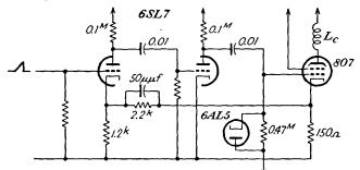
FIG. 21-16. A feed-back sweep-current amplifier.
