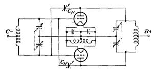
FIG. 11-15. Neutralization of a push-pull tuned amplifier.
