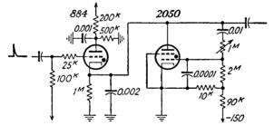
FIG. 19-37. A thyratron pulse generator with thyratron clipper.
