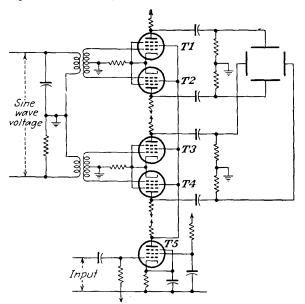
FIG. 21-22. A circular-sweep generator circuit.
