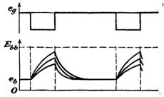
FIG. 20-12. The voltage across the capacitor C in the circuit of Fig. 20-11.
