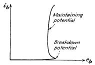
FIG. 2-19. Volt-ampere characteristic of a glow discharge.
