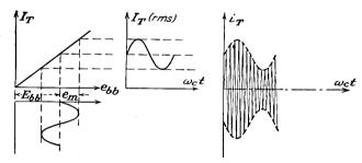
FIG. 15-11. The conditions during plate modulation.
