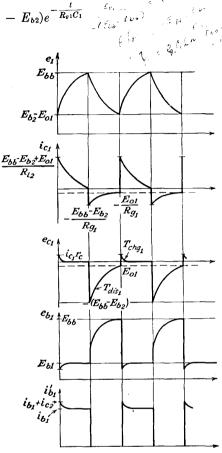
FIG. 18-7. The potential and current wave forms at various points in a symmetrical multivibrator.
