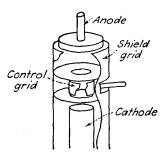
FIG. 2-28. Electrode structure of the FG-98 shield-grid thyratron.
