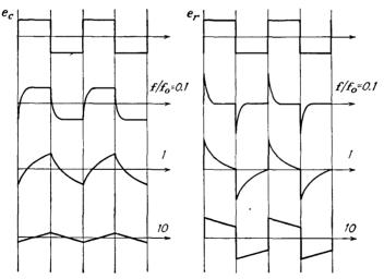
FIG. 7-16. The voltage forms  $e_c$  and  $e_r$  for an applied square wave on a differentiating circuit, with  $f/f_0$  as parameter.
