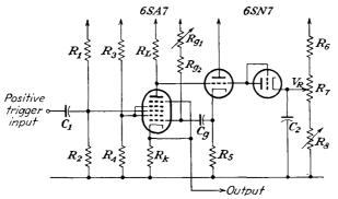
FIG. 19-33. A second version of the phantastron delay circuit.
