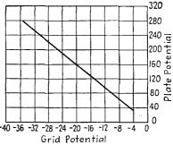
acting as a dummy electrode, the cylin- Fig. 2-27. Critical grid characterdrical grid now serving as the anode. istic of an 884 argon-filled thyratron. It is because of this that a large current-
