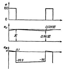
A comparison of the above examples shows that, the lower the clamp impedance relative to the circuit impedance, the "tighter" the clamp
