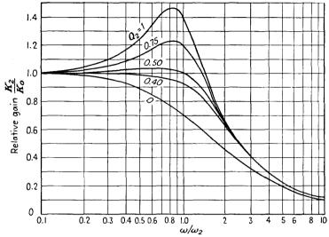
FIG. 6-5. Dimensionless relative gain curves for the shunt-compensated amplifier. (Adapted from Bedford and Fredendall.<sup>1</sup>)
