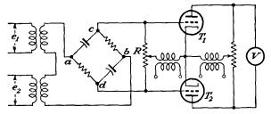
FIG. 22-18. A double-triode phasemeter.
