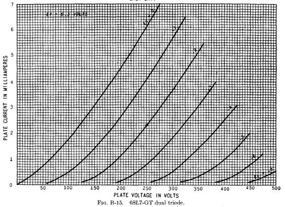
Class A amplifier:  $E_b = 250$  volts,  $E_c = -2$  volts,  $I_b = 2.3$  ma,  $\mu = 70$ ,  $r_p = 44,000$  ohms,  $g_m = 1,600 \mu$ mhos. Interelectrode capacitances: Unit 1:  $C_1 = 3.0 \mu\mu$ f,  $C_2 = 3.8 \mu\mu$ f,  $C_3 = 2.8 \mu\mu$ f. Unit 2:  $C_1 = 3.4 \mu\mu$ f,  $C_2 = 3.2 \mu\mu$ f.
