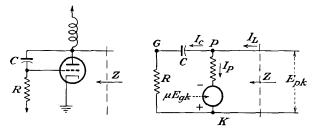
FIG. 17-10. The reactance tube and its equivalent circuit.
