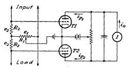
so that the voltage drop across them does not appreciably reduce the load voltage. The resistor  $R_1$  is high in order to prevent appreciable power loss.
