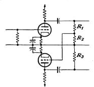
FIG. 9-25. A single-tube paraphase amplifier.
