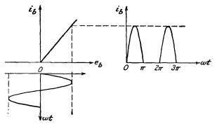
The method of obtaining the output-current wave form from the dynamic Fig. 13-3. characteristic.
