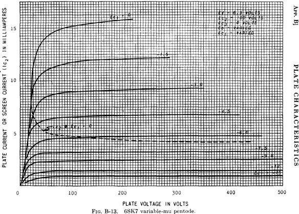
Class A amplifier:  $E_b = 250$  volts,  $E_{c2} = 100$  volts,  $E_c = -3$  volts,  $I_b = 9.2$  ma,  $I_{c2} = 2.6$  ma,  $r_p = 0.8$ megohm approx,  $g_m = 2,000 \ \mu$ mhos. Interelectrode capacitances:  $C_1 = 6.0 \ \mu\mu$ f,  $C_2 = 7.0 \ \mu\mu$ f,  $C_3 = .003 \ \mu\mu$ f.
