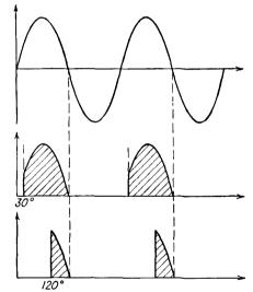
FIG. 13-14. The character of the conduction in a thyratron for various angles of initiation of the arc.
