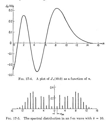
A plot of the spectrum corresponding to Eq. (17-19) is given in Fig. 17-5. Notice that this is just a plot of the spectral lines, without regard for sign, as dictated by the Bessel function plot of Fig. 17-4. The separation between individual side bands is 7.5 kc, the modulating frequency. It is evident from this plot that the total band width necessary to include all significant side-bands is 210 kc.
