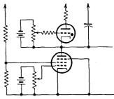
FIG. 20-16. A thyratron sawtooth generator with a pentode charging circuit.
