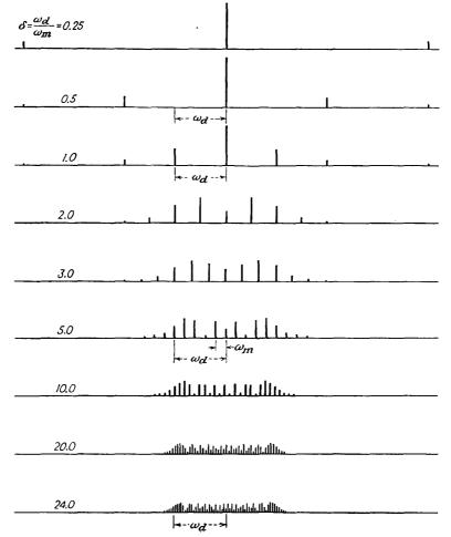
FIG. 17-7. The spectral distribution in an f-m wave for different values of  $\delta$ , fixed  $\omega_{d_i}$  and different  $\omega_m$ .
