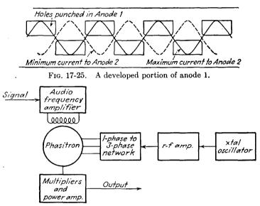
FIG. 17-26. The General Electric phasitron f-m transmitter.
