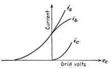
FIG. 2-5. Total space, plate, and grid current in a triode, as a function of grid voltage, with fixed plate voltage.
