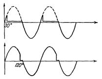
FIG. 13-15. The potential across the thyratron for various current-conduction periods.
