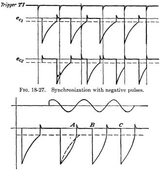
FIG. 18-28. Synchronization with sine-wave voltage.
