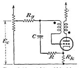
former. For a given transformer, C is the most important circuit element, larger values of C being accompanied by longer pulses. For example, a certain transformer, when used in the circuit of Fig. 18-20, yielded pulses which could be varied from approximately 0.2 to 20  $\mu$ sec by changing the size of the capacitor C.
