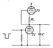
Assume that the beam resistance of T2 is  $r_b$  when the tube conducts and is infinite when the gate is applied.
