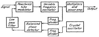
FIG. 17-18. The Federal center frequency-stabilization system.
