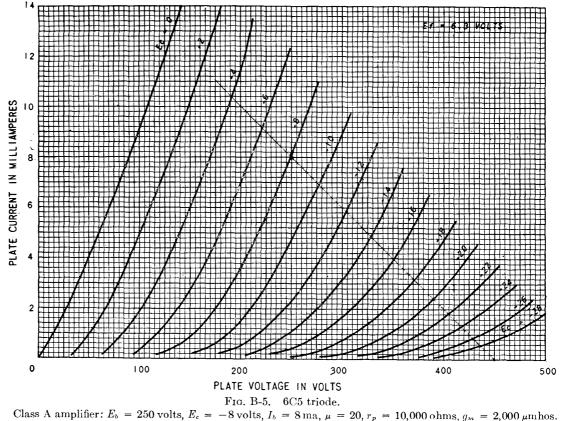
Class A amplifier:  $E_b = 250$  volts,  $E_c = -8$  volts,  $I_b = 8 \text{ ma}, \mu = 20, r_p = 10,000 \text{ ohms}, g_m = 2,000 \mu\text{mhos}.$ Interelectrode capacitances:  $C_1 = 3 \mu\mu$ f,  $C_2 = 11 \mu\mu$ f,  $C_3 = 2.0 \mu\mu$ f.
