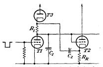
FIG. 20-23. The use of a diode in the plate circuit to reduce any d-c shift and to maintain the feed-back gain.
