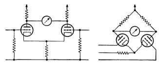
FIG. 6-21. A difference amplifier in conventional form, and also drawn in a manner to indicate the equivalent bridge character of the circuit.
