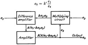
FIG. 8-15. A circuit which divides two voltages.
