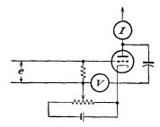
shown in Fig. 22-7. The 6J7 is satisfactory for use to several megacycles, but where the voltmeter is intended for use across highimpedance tuned circuits at frequencies as high as 10 megacycles, and in cases where the input ca-
