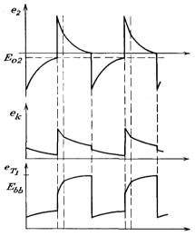
charging continues at a slower rate. The equivalent charging circuits are shown in Fig. 18-15. As C charges, the bias on T2 decreases, causing  $i_{b2}$ to decrease. This in turn causes  $e_k$  to decrease. The grid of T1 is held constant at ground potential so that this tube remains cut off as
