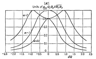
FIG. 10-7. The response characteristics of a double-tuned amplifier for various values of coupling.
