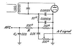
FIG. 16-12. A diode detector and automatic-volume-control circuit.
