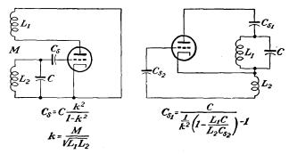
FIG. 12-11. Impedance-stabilized oscillators.
