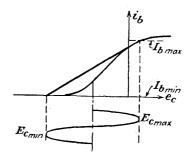
FIG. 12-2. Sketch for defining the average transconductance  $\overline{g_m}$ .
