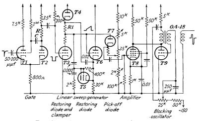
FIG. 19-35. A 150-µsec linear-sweep delay circuit.
