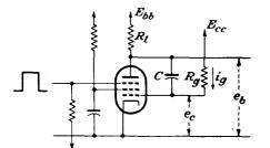
FIG. 19-24. The basic Miller integrating circuit.
