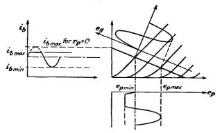
FIG. 7-9. Saturation limiting in a triode.
