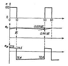
figure. These sketches show the potential variations across the capacitor and across the grid-cathode resistor after steady-state conditions have been reached.
