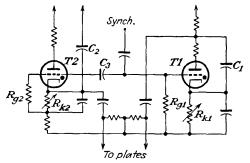
FIG. 20-31. Two thyratron saw-tooth generators operating in push-pull.
