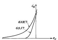
FIG. 2-16. The transfer curves of a 6SJ7 sharp-cutoff pentode and a 6SK7 remote-cutoff pentode.
