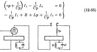
FIG. 12-25. The equivalent and simplified circuit of the negative-resistance oscillator.
