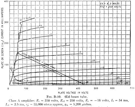
Interelectrode capacitances:  $C_1 = 10 \ \mu\mu f$ ,  $C_2 = 12 \ \mu\mu f$ ,  $C_3 = 0.4 \ \mu\mu f$ .
