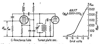
FIG. 17-12. A reactance-tube f-m oscillator, and the curve showing the variation of  $g_m$  with grid potential.
