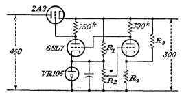
14-13. Design a regulated power supply that will supply 150 ma at 250 volts from a 450-volt rectified and filtered source, with a ripple not to exceed 0.1 per cent and with a stabilization ratio of 15,000. What is the rms ripple voltage in the output of this regulated source if a II filter consisting of two 8- $\mu$ f capacitors and a 12-henry choke is used? The effective output resistance is 650 ohms.
