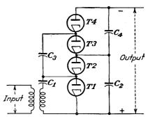
FIG. 13-9. A half-wave voltage-doubling circuit.
