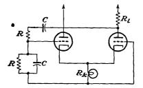
this problem. Determine the critical value of  $R_l$  at which oscillations will just start.
