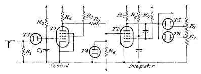
FIG. 19-28. The sanatron delay circuit.
