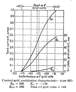
class C amplifier are given in the sketch. Calculate for m = 1.0 the following:
