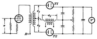
FIG. 22-16. An electronic phasemeter.
