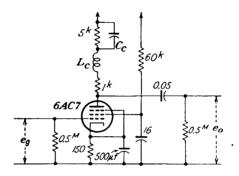
$L_c$  that will yield the same gain at the upper frequency  $f_2$  as at the mid-band. Assuming the stray wiring capacitances to be 20  $\mu\mu$ f, the tube capacitances of the 6AC7 are  $C_{gp} = 0.015 \,\mu\mu$ f,  $C_{pk} = 5 \,\mu\mu$ f,  $C_{gk} = 11 \,\mu\mu$ f. Calculate also  $f_1$  under the optimum conditions for the l-f compensation.
