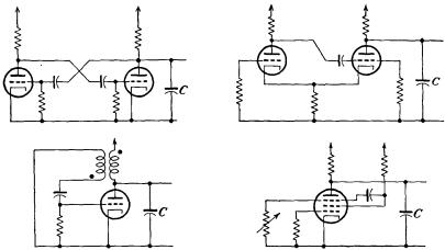
FIG. 20-10. Free-running vacuum-tube sweep generators.
