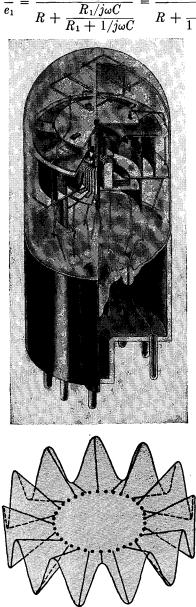
FIG. 17-24. The General Electric 2H21 phasitron.
