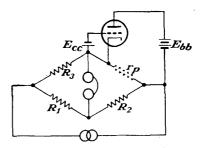
FIG. 3-10. A Wheatstone bridge for determining the plate resistance of a triode under operating conditions.
