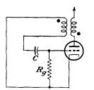
FIG. 18-18. A simple blocking oscillator.
