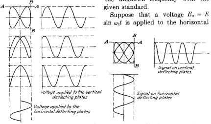
FIG. 22-20. Lissajous figure for 1:2 frequency ratio.
