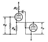
**6-13.** Show that the h-f cutoff of the anode-follower amplifier is approximately one-half that of the cathode follower. Show also that the l-f cutoff is approximately the same as that of the cathode-follower amplifier, for  $Z_1 = R_g$  in Circuit Fig. 6-10.
