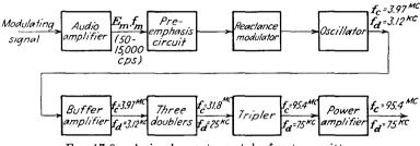
FIG. 17-9. A simple reactance-tube f-m transmitter.
