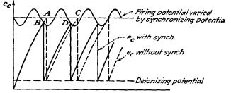
FIG. 20-9. Synchronizing a thyratron saw-tooth generator with a sine wave.
