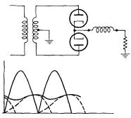
FIG. 14-3. Full-wave rectifier circuit with inductance choke, and the wave shape of the load current.
