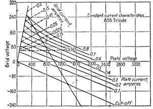
FIG. 11-12. Constant-current characteristics of an 806 triode.
