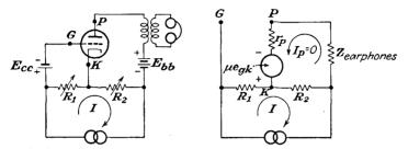
FIG. 3-8. The Miller bridge and its equivalent circuit, for determining the amplification factor of a triode under operating conditions.
