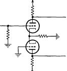
FIG. 20-27. A cathodecoupled paraphase amplifier.
