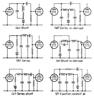
FIG. 6-7. Various h-f-compensating coupling circuits. (D. L. Jaffee, Electronics, April, 1942.)
