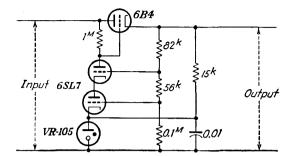
FIG. 14-24. A voltage regulator employing a "cascode" amplifier.
