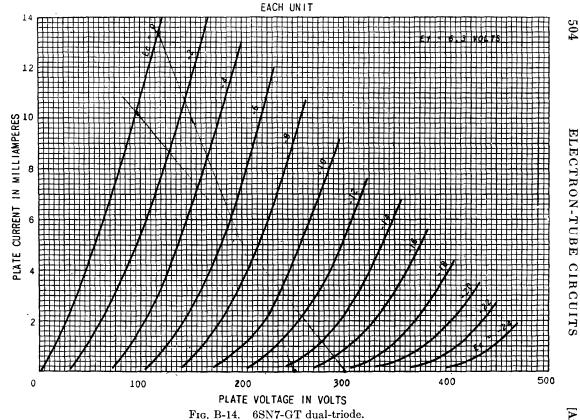
[App. Class A amplifier:  $E_b = 250$  volts,  $E_c = -8$  volts,  $I_b = 9$  ma,  $\mu = 20$ ,  $r_p = 7,700$  ohms,  $g_m = 2,600$   $\mu$ mhos. Interelectrode capacitances: Unit 1:  $C_1 = 3.2 \ \mu\mu$ f,  $C_2 = 3.4 \ \mu\mu$ f,  $C_3 = 4 \ \mu\mu$ f. Unit 2:  $C_1 = 3.8 \ \mu\mu$ f, в  $C_2 = 2.6 \ \mu\mu f, \ C_3 = 4 \ \mu\mu f.$
