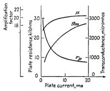
FIG. 2-9. The parameters  $\mu$ ,  $r_p$ , and  $g_m$  of a 6C5 triode as a function of plate current.
