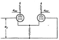
Fig. 6-25. A cathode-coupled paraphase amplifier.
