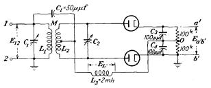
FIG. 17-32. A center-tuned discriminator circuit.
