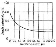
Transfer characteristic FIG. 2-22. of an RCA OA4G cold-cathode triode.
