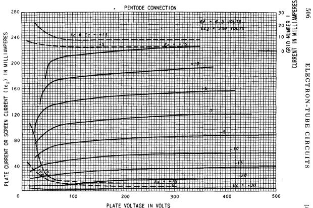
FIG. B-16. 6V6 beam tube.
