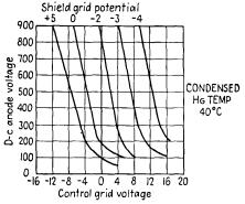
FIG. 2-29. Control characteristics of an FG-98 shield-grid thyratron.
