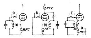
12-10. An amplitude-controlled oscillator uses a 6J5 tube. It operates at 5 megacycles. A measurement of the network and rectifier when the oscillator \*Butler, F., *Wireless Eng.*, 23, 157 (1946).
