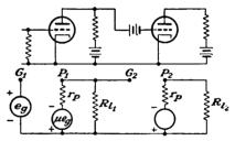
FIG. 6-17. Basic battery-coupled amplifier circuit.
