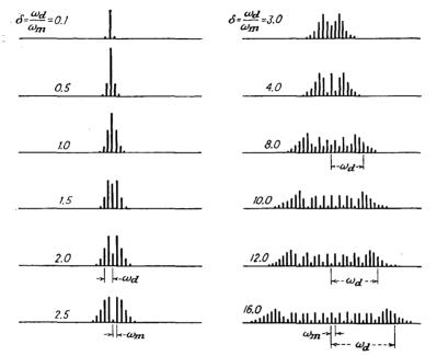
FIG. 17-6. The spectral distribution in an f-m wave for different values of  $\delta$ , different  $\omega_{d}$ , and fixed  $\omega_{m}$ .
