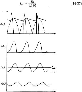
FIG. 14-10. The tube current in the full-wave rectifier with L-section filter, for (a) L = 0, (b) L less than critical inductance  $L_{c_1}(c) L$  equal to  $L_{c_2}(d) L$  greater than  $L_c$ .
