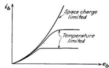
FIG. 2-2. The volt-ampere characteristics of a typical diode.
