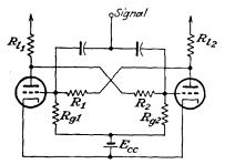
FIG. 19-14. The Eccles-Jordan trigger circuit.
