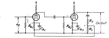
FIG. 5-21. A two-stage RC coupled amplifier with current feedback in the first stage and voltage feedback between stages.
