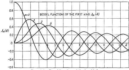
FIG. 17-3. Bessel functions of the first kind.
