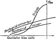
FIG. 16-15. Typical transconductance curves of different types of tubes.
