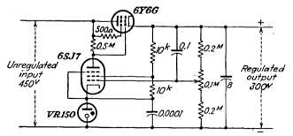
FIG. 14-21. An electronically regulated power supply.
