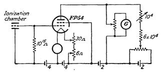
FIG. 22-13. An electrometer circuit using an FP-54 tube.
