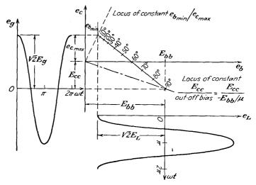
FIG. 11-10. The operating characteristics of a class C amplifier.
