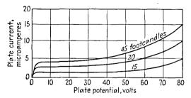
FIG. 1-7. The volt-ampere characteristics of a type PJ-23 gas-filled phototube, with light intensity as a parameter.
