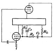
FIG. 12-17. An *RC* coupled oscillator.
