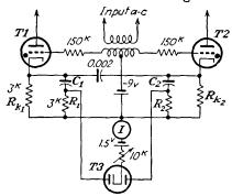
FIG. 22-23. An electronic frequency meter.
