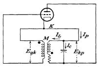
FIG. 12-5. Tuned-plate oscillator.
