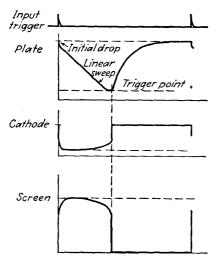
FIG. 19-31. The potentials at various points of the phantastron.
