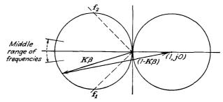
FIG. 5-23. The locus in the complex plane of  $K\beta$  for the circuit of Fig. 5-19.
