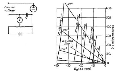
FIG. 16-9. The rectification characteristic of a 6H6 diode, and the circuit used for its determination.
