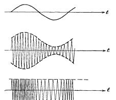
FIG. 17-2. The output of a sinusoidally modulated a-m and f-m transmitter.
