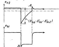
FIG. 19-9. The grid potential of T2and the plate potential of T1 in the cathode-coupled delay multivibrator of Fig. 19-8.
