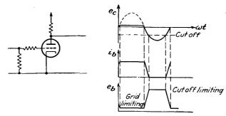
FIG. 7-11. Formation of a square wave by grid-circuit and cutoff limiting.
