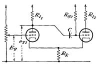
FIG. 19-8. A cathode-coupled delay multivibrator.
