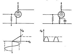
FIG. 7-10. Cutoff limiting in a strongly biased amplifier.
