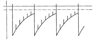
FIG. 18-30. The grid-voltage wave form of a blocking oscillator synchronized with positive pulses.
