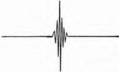
FIG. 1.3.—Modulated alternating voltage (short a-c pulse).
