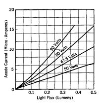
and anode current in a typical gasfilled phototube.
