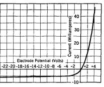
Fig. 50. Volt-ampere characteristic of an auxiliary electrode immersed in an arc discharge.
