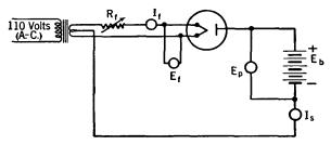
Fig. 10. Circuit for measuring the emission of a high-vacuum tube.
