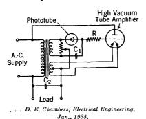
Fig. 77. A phototube relay or control circuit using a high-vacuum tube and a phototube.
