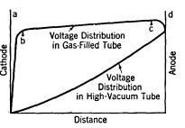
tribution in a high-vacuum tube and in a gas-filled tube.
