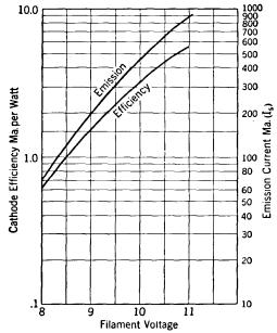
Fig. 9. The emission efficiency and emission of a pure tungsten filament.
