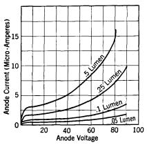
The relation between the anode Fig. 19. voltage and current for a typical gasfilled phototube.
