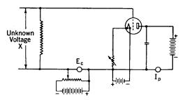
Fig. 37. The circuit for the slide-back voltmeter using a high-vacuum, three-electrode tube.
