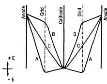
Fig. 23. The potential distribution in a hypothetical high-vacuum tube. Curve B shows the grid above normal space potential; in C the grid is at space potential; A shows the grid enough negative to produce a negative field at the cathode. from the cathode as a
