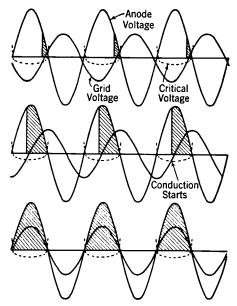
Fig. 72. The variable conduction period obtained by shifting the phase relation of the grid and anode voltages. The phase-shift method permits complete control of the average current flow in a gas-filled tube.
