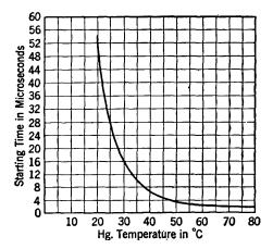
Fro. 54. The time required to establish full conductivity, that is, the "ionization time," and the effect of the mercury-vapor pressure.
