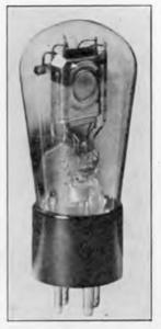
Fig. 39. A three-electrode high-vacuum tube designed to have a minimum of undesired disturbances in the plate current flow; that is, a "low-noise" tube.
