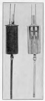
Fig. 83. A single-pole, doublethrow vacuum switch.
