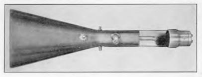
Fig. 82. A cathode-ray oscillograph tube.
