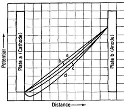
Fig. 14. The potential distribution between plane parallel plates with various degrees of space charge.
