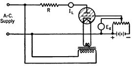
Fig. 71. Circuit for measuring the control characteristic of a three-electrode gas-filled tube.
