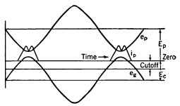
Fig. 42. The relation between plate current, plate voltage, and grid voltage for the Class C mode of operation.
