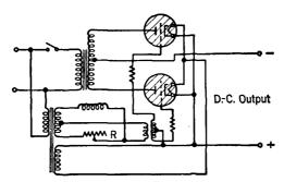
Fig. 75. A circuit for a controlled rectifier using gas-filled tubes.
