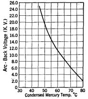
Curve illustrating the effect of mercury-vapor pressure on arcback voltage.
