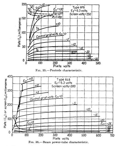
In Figs. 35 and 36 are shown the characteristics for a pentode and beam power tube, respectively.
