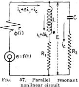
method by which the present  $\Delta i_L$  and  $i_c$  are to be found. With this in mind we write down the equations
