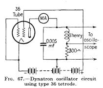
struction of Sec. 11 is to be used. circuit and value The of parameters employed are shown in Fig. 67. The inductance had an ohmic resistance of 500 ohms. so that the total resistance of that branch was 800 ohms. The screen voltage was maintained constant at 130 volts, and the plate supply voltage at each of three values, 45, 22.5, and 13.5 volts.
