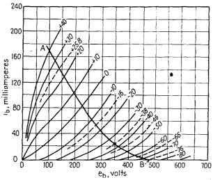
FIG. 79.-Push-pull load line for 6F6 tube-sliding-rule method.
