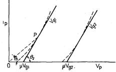
FIG. 7.-Linear and actual tube-plate characteristics.
