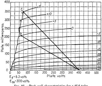
FIG. 85.—Push-pull characteristics for a 6L6 tube.
