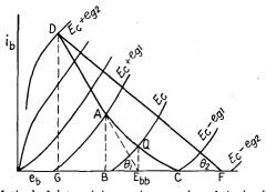
F10. 84.—Method of determining optimum value of the load resistance. has reached the value of AB. Its load line (for increased grid swing) continues along the straight line AD, corresponding to a value of  $R_L/4$ . Thus, for a grid swing  $e_{g_2}$ , point D is reached and the current is DG, while, for the other tube, point F is reached and its current is zero.
