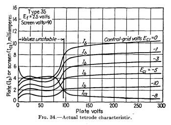
curvature; this break has been called a "knee" in the characteristic. Obviously this knee should be as sharp and as close to the  $i_b$  axis as possible, in order that increased power output may be obtained. (This is the case for Fig. 33.)
