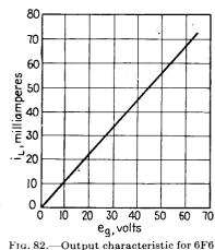
Fig. 82.—Output characteristic for 6F6 balanced amplifier.
