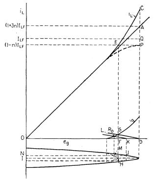
FIG. 99.—Graphical constructions for determining permissible driver resistance.
