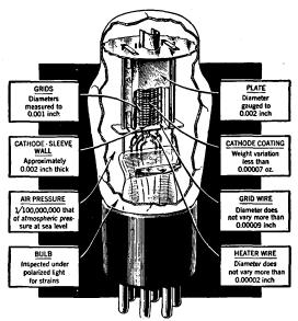
FIG. 4.-Typical triode construction. (Courtesy of RCA.)
