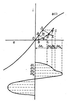
FIG. 47.—Graphical solution for Lr nonlinear circuit.
