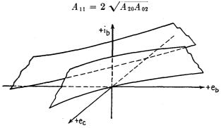
FIG. 90.-Tube surface of the form of a hyperbolic paraboloid.
