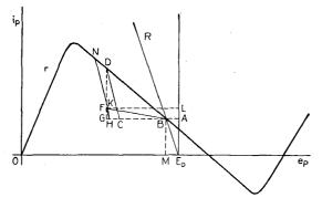
FIG. 68.—Graphical construction for dynatron oscillator circuit.
