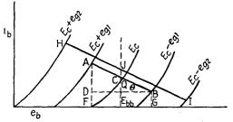
FIG. 83.—Sliding-rule method showing paths of operation for the output and mid-branch currents.
