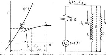
FIG. 53.—Series circuit having linear L, C, and R and nonlinear r.
