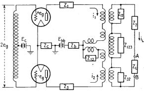
FIG. 89.—Generalized balanced-amplifier circuits.
