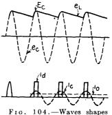
FIG. 104.—Waves shapes of current and voltage in diode detection for fixed-carrier amplitude.
