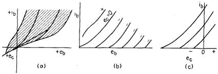
FIG. 18.-Triode surface and characteristic curves.
