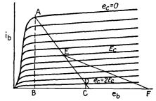
FIG. 125.—Graphical constructions for the case of lower a.c. than d.c. plate-load resistance—pentode tube.
