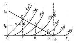
FIG. 22.-Two-dimensional graphical solution for triode circuit.
