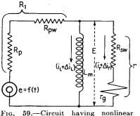
Fig. 59.—Circuit having nonlinear parallel resistor.
