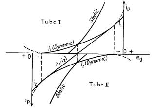
FIG. 94.—Push-pull operation beyond cutoff for parabolic tubes.
