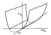
FIG. 92.-Tube surface of the form of a parabolic cylinder.
