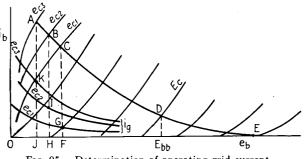
FIG. 95.—Determination of operating grid current.
