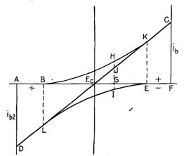
FIG. 77.-Individual and composite dynamic characteristics.
