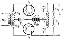
FIG. 72.-Idealized push-pull circuit.
