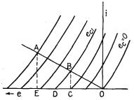
FIG. 103.—Rectification diagram and load line for a diode detector.
