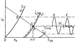
FIG. 40.-Shifting of operating point due to self-rectification, plate characteristic.
