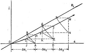
FIG. 61.—Graphical solution for nonlinear parallel resistor.
