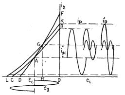
FIG. 43.—Correction to load line—inductive plate feed, transfer characteristics.
