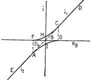
FIG. 78.—Dynamic characteristics for extreme class AB (class B) operation.
