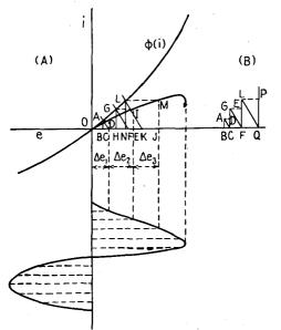
FIG. 50.—Graphical solution for rC nonlinear circuit.
