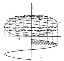
FIG. 48.—Displaced ellipse obtained for pure linear inductance.
