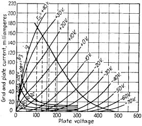
FIG. 100.—Grid-current determination for a 6F6 tube.
