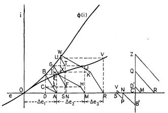
FIG. 58.—Graphical solution for parallel resonant circuit.
