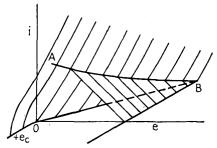
FIG. 21.—Three-dimensional graphical solution for triode circuit.
