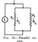
*i.e.*, I should be known, and then the component currents  $I_1$  and  $I_2$  through  $R_1$  and  $R_2$ , respectively, as well as  $E_1$  can be determined. In practice, however,  $E_1$  is usually given, and I,  $I_1$ , and  $I_2$  are to be determined. Hence, the method will differ
