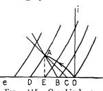
FIG. 115.—Graphical construction for a diode circuit having appreciable shunting capaci-
