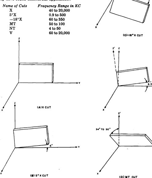
Figure 1-19. The X group. (The second rotations of the MT, NT, and V cuts are shown only for the positive angles) \*
