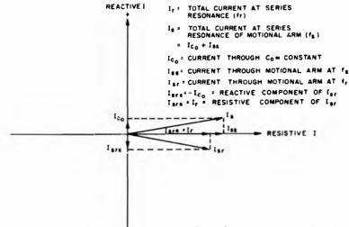
Figure 1-99. Phasor representation (greatly exaggerated) of current through arms of crystal unit at the series-resonant frequencies, f, and f... Distributed inductance of the crystal leads is assumed to be negligible
