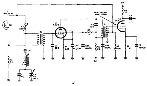
Figure 1-163. Meacham bridge-stabilized oscillators
