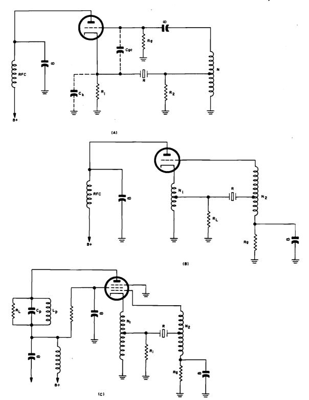
Figure 1-180. Grounded-plate oscillators. (A) Basic circuit. (B) Circuit for increased power output. (C) Electron-coupled circuit
