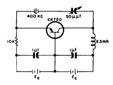
Figure 1-224. Junction transistor crystal-feedback oscillator
