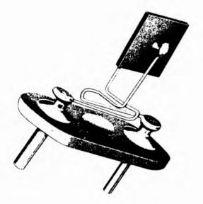
Figure 1-85. Solder-cone wire mounting of face-shear element
