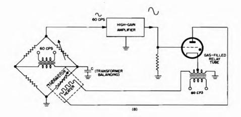
Figure 4-9. On-off heater control circuits
