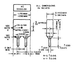
Figure 3-23. Crystal Holder for Crystal Unit CR-1A/AR
