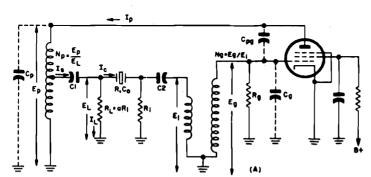
Figure 1-176. (A) Basic circuit of transformer-coupled oscillator
