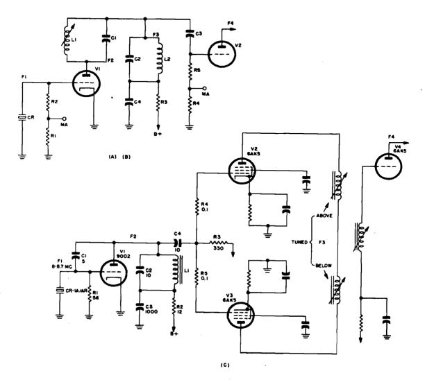
Figure 1-150. Modified Miller oscillators using triodes
