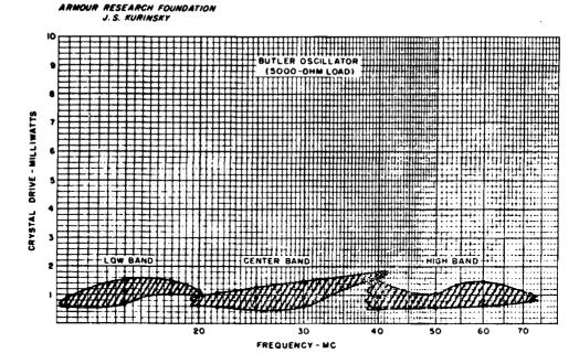
Figure 1-252. Typical drive levels and operating tolerances to be expected for crystal units connected in the Butler circuit of Gruen packet series. The values shown assume a 5000-ohm load resistance
