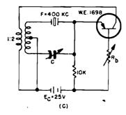
Figure 1-234. Transformer-coupled transistor
