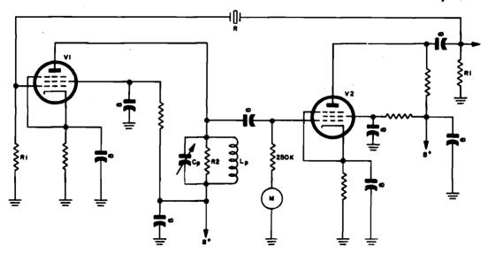
Figure 1-183. Grounded-cathode two-stage feed-back oscillator
