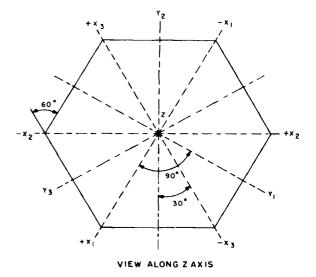
Figure 1-6. XY plane of quartz showing three sets of rectangular axes: X<sub>1</sub>Y<sub>1</sub>Z<sub>1</sub>, X<sub>2</sub>Y<sub>2</sub>Z<sub>1</sub>, X<sub>2</sub>Y<sub>2</sub>Z (Z axis is perpendicular to plane of paper)
