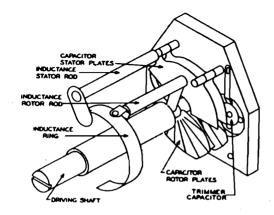
Figure 1-204. Construction of r-f tuner employed in Radio Receiver R-278/GR
