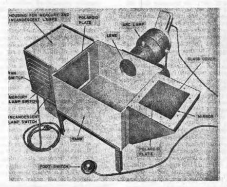
Figure 1-57. Palariscope-inspectoscope. Used for examining raw quartz
