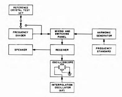
Figure 2-92. System recommended for Government inspection measurements of crystal frequencies at room temperature. The measurements are made visually with the oscilloscope and interpolation oscillator. The speaker is used principally as an aid in determining whether the crystal frequency under test is greater or less than the standard harmonic
