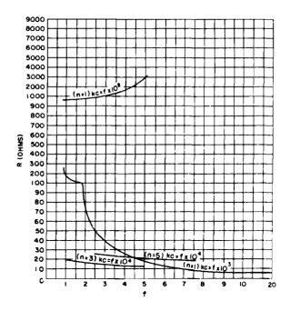
Figure 1-96. Typical curves of the series-arm resistance of plated crystals versus frequency. Actual series-arm resistances will vary between R/3 and 3R, where R is the value shown, except when R is less than 10 ohms, in which case the minimum resistance will be approximately one-half the value indicated. Values indicated are average for fundamental modes and approximately ½ the average for overtone modes
