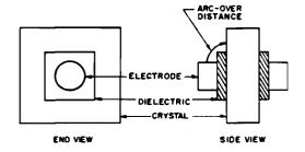
Figure 1-74. Center-pressure type of dielectric sandwich for mounting crystals
