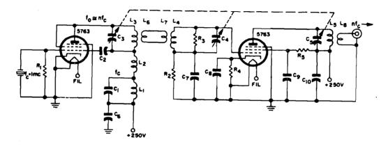
$R_1 = 30.000 \text{ ohms}$  $C_t = 112 \, \mu \mu f$  $L_1 = 114 \mu h$  $f_a = 1 \text{ mc}$  $R_a = 15,000 \text{ ohms}$  $C_1 = 10 \mu\mu f$  $L_z = 37 \,\mu h$  $f_0 = 20-30 \text{ mc}$  $C_{s}$ ,  $C_{s}$ ,  $C_{s} = 6-80 \,\mu\mu f$  $R_a = 2.200 \text{ ohms}$  $L_{3}$ ,  $L_{4}$ ,  $L_{6} = 0.8 \, \mu f$  $R_{\star} = 150 \text{ ohms}$  $C_{0}$ ,  $C_{7}$ ,  $C_{8}$ ,  $C_{9}$ ,  $C_{10} = .01 \, \mu f$  $L_{1}$ ,  $L_{2} = 0.12 \, \mu h$  $R_4 = 68,000 \text{ ohms}$ L - 0.17 uh
