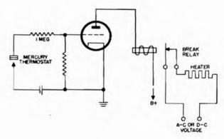
Figure 4-8. Heater control circuit using mercury thermostat
