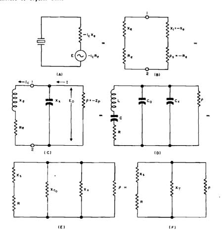
Figure 1-108. Generalized crystal oscillator circuit
