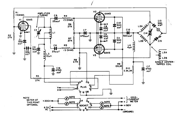
Figure 1-171. A multitube capacitance-bridge oscillator which is practical for operation in the 50–200-mc range.
