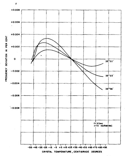
Figure 1-113. Large clockwise angle of rotation of frequency-temperature curve of harmonic-mode A element caused by small increments (3 minutes of arc) in the cutting orientation angle about the X axis
