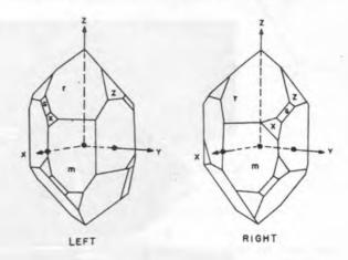
Figure 1-4. Left and right quartz crystals
