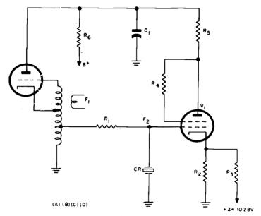
Figure 1-159. Crystal and magic-eye resonance indicator
