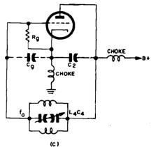
Figure 1-220. (A) Schematic diagram of Hahnel spectrum generator in which two oscillator circuits are combined in one stage; (B) Simplified schematic diagram of the crystal oscillator circuit of the spectrum generator; (C) Simplified schematic diagram of the v-f-o circuit of the spectrum generator
