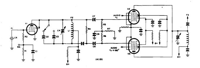
Figure 1-153 Miscellaneous Miller-oscillator modifications
