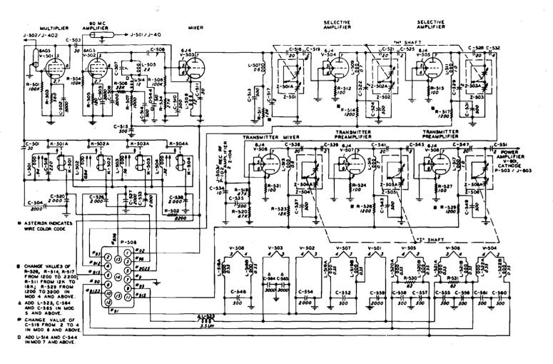
Figure 1-215. Spectrum amplifier and transmitter preamplifier subassembly, Receiver-Transmitter RT-178/ARC-27. See figure 1-212 for functional operation of spectrum generator stages V501, V502, V503, V504, and V505. See figure 1-211 for functional operation of transmitter stages V506, V507, and V508
