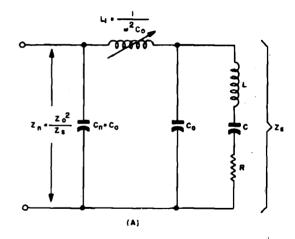
Figure 1-182. Impedance-inverting oscillator circuits.
