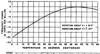
Figure 1-35. Frequency-temperature characteristics of element M \*
