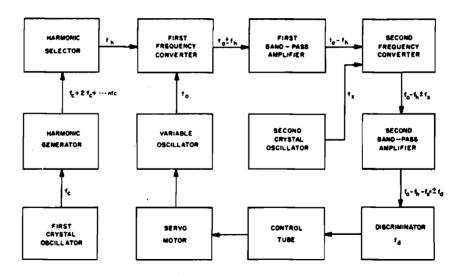
Figure 1-191, Block diagram of frequency-synthesizer circuit
