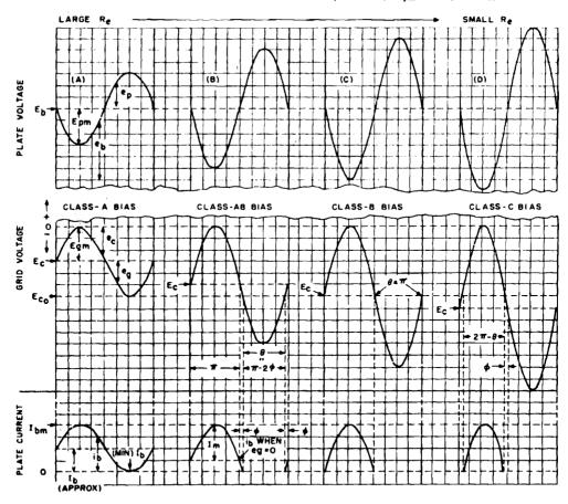
Figure 1-132. Change of state of Pierce oscillator with a C<sub>v</sub>/C<sub>p</sub> ratio of one, under no-load conditions when E<sub>p</sub> is held constant and the effective resistance of the crystal changes
