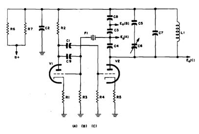
Figure 1-184. Modifications of two-stage feed-back oscillator to improve sine-wave output
