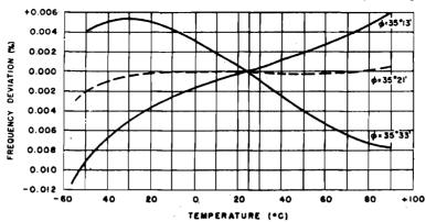
Figure 1-49. Temperature-frequency characteristics of element A
