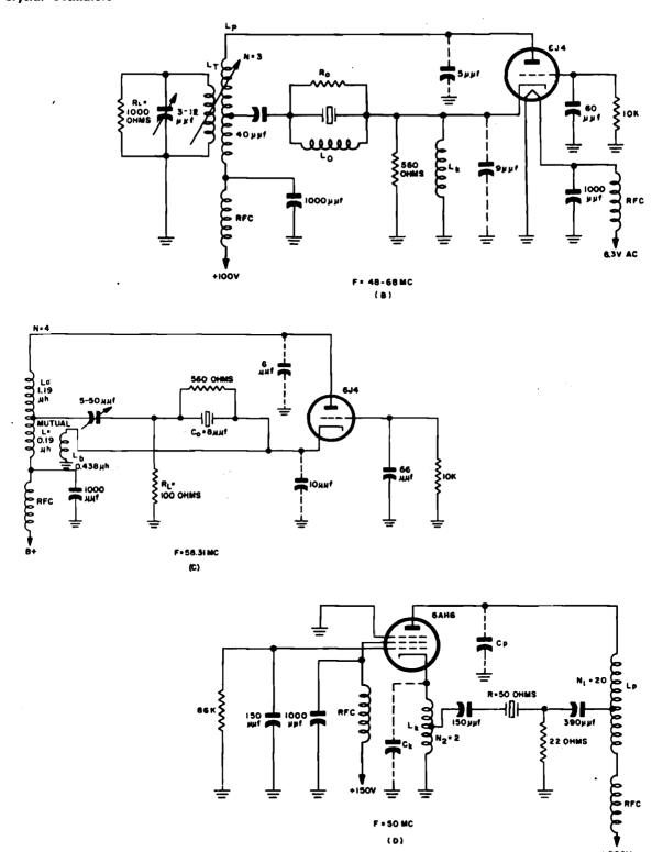
Figure 1-179. Modifications of grounded-grid oscillator. (B) Broad-band circuit. (C) Circuit for compensating crystal capacitance by mutual inductance. (D) High-efficiency class-C circuit
