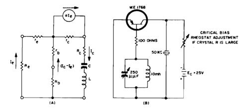
Figure 1-232. (A) Equivalent a-c circuit of tuned-collector negative-resistance oscillator. For crystal control, L, C, and R, can be interpreted as being the series-arm parameters of a crystal unit; (B) Crystal-controlled tuned-collector negative-resistance oscillator. The parallel tuned tank is inserted in the base circuit in lieu of a resistor in order to obtain negative resistance values in excess of 40,000 ohms
