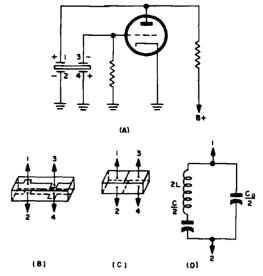
Figure 1-156. Basic circuit of oscillator using crystal with two pairs of electrodes
