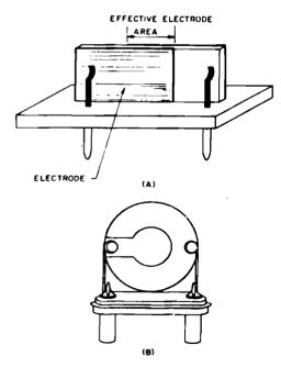
Figure 1-88. Edge-clamped systems of mounting. (A)
