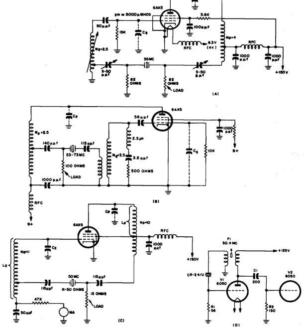
Figure 1-177. Modifications of transformer-coupled oscillator for: (A) High stability.
