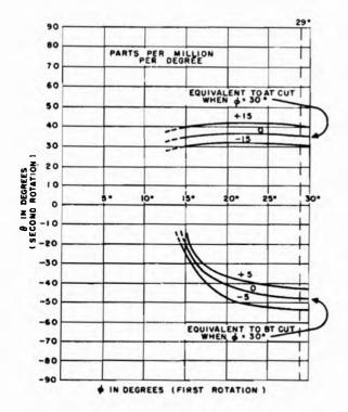
Figure 1-40. Relations of  $\theta$  to  $\phi$ , for thickness-shear mode of V cut, which provide the temperature coefficients indicated for each curve
