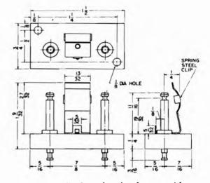
Figure 3-17. Crystal socket for use with HC-10/U holder
