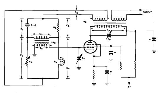
Figure 1-160. Basic circuit of Meacham bridge-stabilized oscillator
