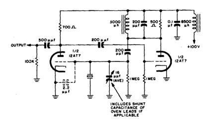
Figure 2-50. Schematic diagram of typical oscillator designed for use with Crystal Unit CR-46/U
