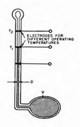
Figure 4-7. Diagram of typical mercury thermostat
