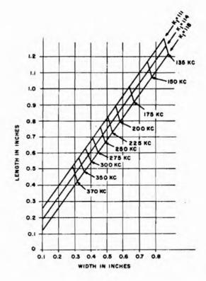
Figure 1-22. Frequency characteristics of X-cut crystal vibrating in width-extensional mode, where the width is parallel to the Y axis. w/l ratios not included between the two outer curves will have interfering modes. K, is in kc-inches
