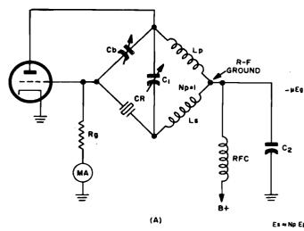
Figure 1-165. (A) Basic circuit of capacitance-bridge oscillator. (B) Equivalent circuit of capacitance-bridge oscillator
