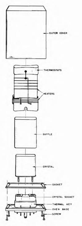
Figure 4-2. Small crystal oven equivalent to Milltary
