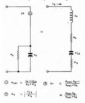
Figure 1-128. Equivalent Pierce feed-back circuit
