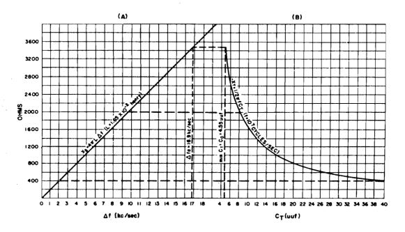
Figure 1-103. Reactance curves of: (A)  $X_i$  versus  $\Delta f_i(B) = X_i$  versus  $C_i$
