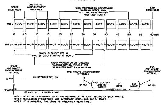
Figure 2-87. Chart showing standard time and frequency signals broadcast by Stations WWV and WWVH (Subject to change)
