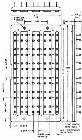
Figure 3-16. Multiple crystal socket for use with HC-6/U, HC-13/U, and HC-14/U holders
