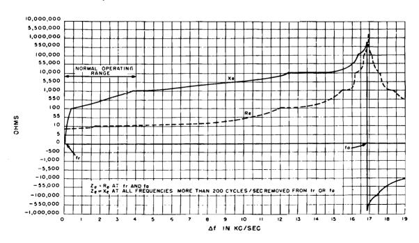
Figure 1-104. Typical characteristic curves for X<sub>o</sub> and R<sub>o</sub> of 10-mc crystal unit. (Shunt resistance, R<sub>I</sub>, across crystal is assumed to be negligible)
