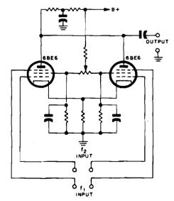
Figure 1-218. Balanced modulator circuit, which is useful as a mixer stage when maximum attenuation of the input frequencies in the output is desired
