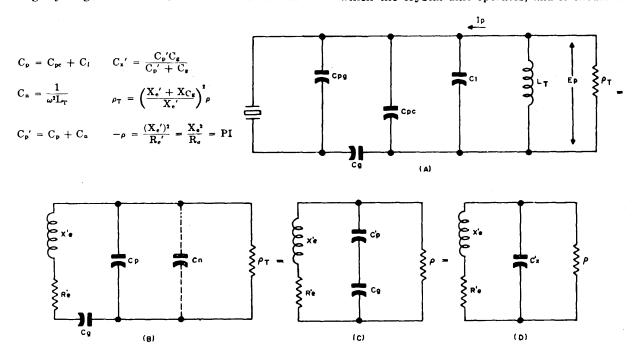
Figure 1-121. Generalized Pierce oscillator.  $X_0'$  and  $R_0'$  are the effective impedance parameters of the crystal unit based upon the assumption that  $C_{pp}$  is a part of  $C_0$ .  $C_n$  is an equivalent negative capacitance having a positive reactance equal to that of  $L_T$ .  $L_p$  is the r-f plate current of the vacuum tube.
