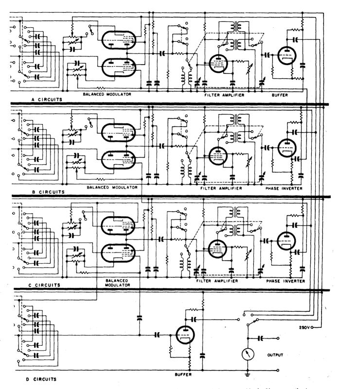
Figure 1-190. Schematic diagram of the 100-kc synchronized multivibrator used in the Plessey synthesizer as a decade divider of a 1000-kc standard and as a 100-kc harmonic generator 293-294
