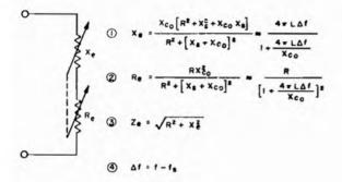
Figure 1-98. Equivalent circuit of crystal unit when represented as an effective reactance in series with an effective resistance. The ganged arrows indicate that  $X_c$  and  $R_c$  will vary together with changes in the frequency, as indicated by the approximate formulas given as functions of  $\Delta f$ . ( $X_{co}$  is negative.)
