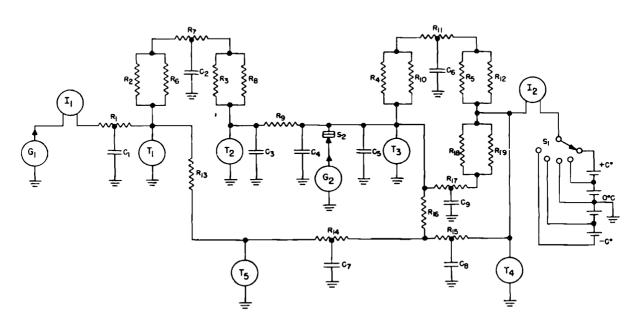
Figure 4-12. Equivalent electrical circuit of crystal oven
