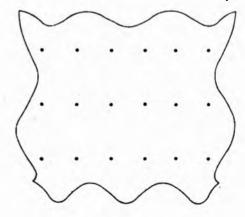
Figure 1-13. Faco-shear mode for m=6, n=3.
