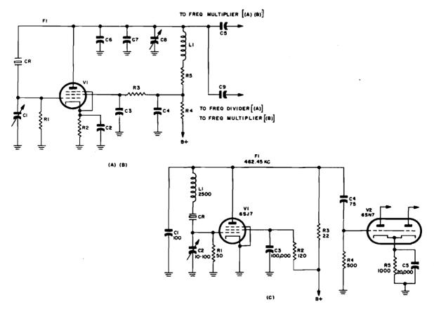
Figure 1-136. Modifications of Pierce oscillator using screen-grid tubes
