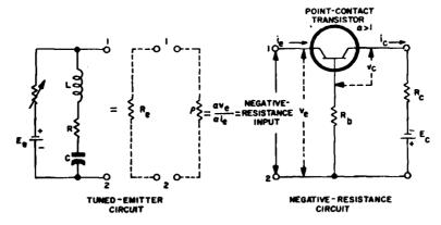
Figure 1-228. Tuned-emitter negative-resistance circuit. Essential features are that alpha be greater than unity, the insertion of an external resistance, R<sub>b</sub>, in the common-base circuit to increase the collector-to-emitter energy feedback; and for oscillations to build up, the effective positive resistance, R<sub>c</sub>, of the tuned-emitter circuit must be less, numerically, than the negative resistance, at the emitter input
