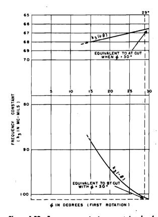
Figure 1-39. Frequency constant versus  $\phi$  (angle of rotation about Z axis) for the thickness-shear mode of V-cut crystals when  $\theta$ , the second angle of rotation, is so chosen that a zero temperature coefficient is obtained. The upper and lower curves are for positive and negative values of  $\theta$ , respectively
