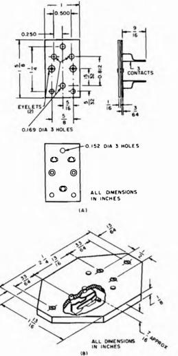
Figure 3-14. Crystal sockets for use with HC-5/U holder
