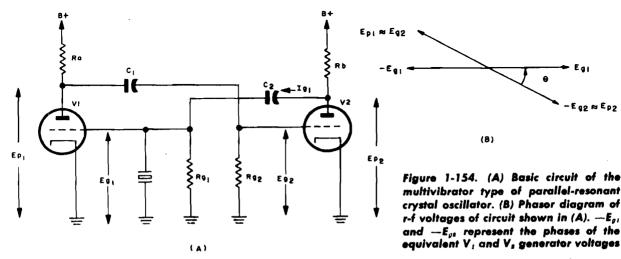
the less will be the leading (inductive) component of  $E_{g1}$  with respect to  $I_{g1}$ . Hence, the smaller the angle  $\theta$ , the more nearly must the crystal approach parallel resonance with the input capacitance of  $V_1$ . Any change in the  $V_1$  plate circuit that tends to decrease  $\theta$  therefore tends to raise the frequency.  $C_{g1}$  can be increased by the insertion of a fixed capacitance to make the total approach the rated load capacitance of the crystal unit.
