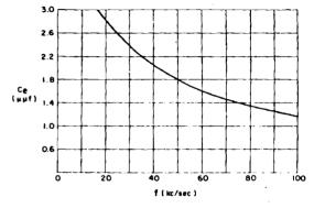
Figure 1-94. C, versus frequency for typical wiremounted N elements
