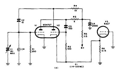
Figure 1-155. Two-stage parallel-resonant escillators of the multivibrator type.
