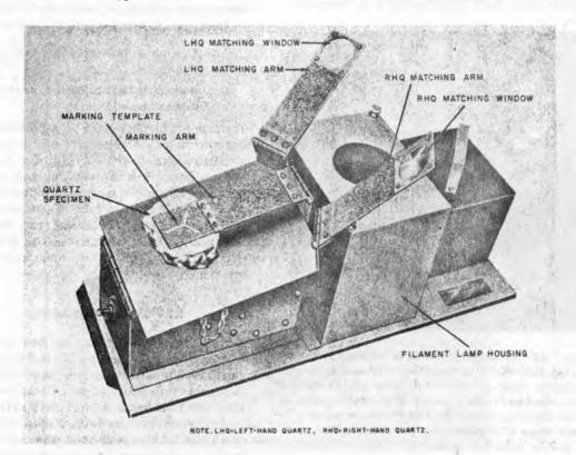
Figure 1-63. Pinhole oriascope with matching and marking arms for use on 4 sections
