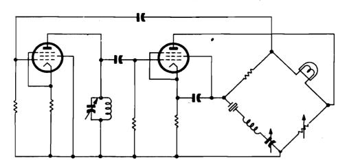
Figure 1-164. Two-stage Meacham bridge-stabilized oscillator
