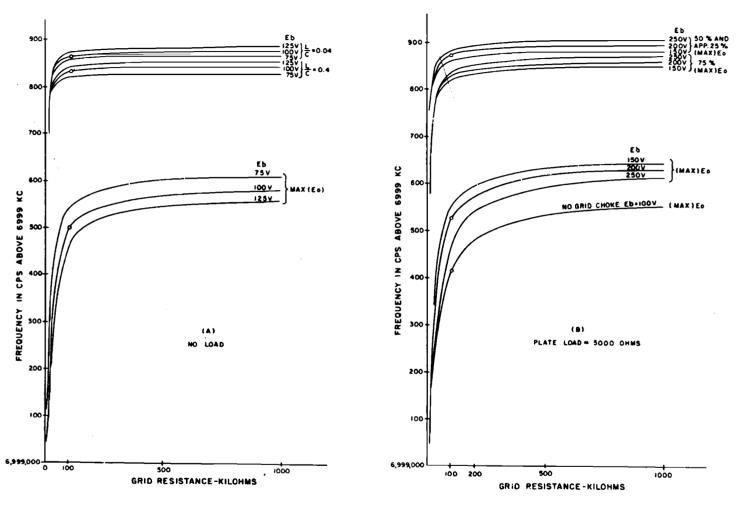
Figure 1-146. Frequency of experimental Miller oscillator versus d-c plate voltage and grid resistance for various plate-tuned load capacitances. (Max) E, represents the plate tuning adjustment that provided maximum output voltage when grid resistance and d-c plate voltage were values indicated by zero reference point. A 7-mc CR-18/U crystal unit was used, having a PI of 49,000 ohms when operating into a rated load capacitance of 32 μμf
