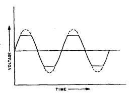
Figure 1-241. Voltage waveform after clipping of both peaks by diode rectiflers
