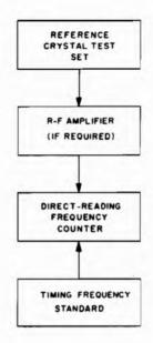
Figure 2-89. System for measuring crystal frequencies visually with a direct-reading electronic counter
