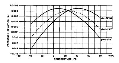
Figure 1-52. Temperature-frequency characteristics of element D
