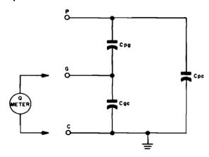
Figure 1-126. Equivalent network formed by the stray static capacitances of a vacuum-tube circuit. A minimum of three different measurements is required. The individual capacitances can be determined by solving simultaneously any three of the nine equations above when the respective terminal capacitances are known
