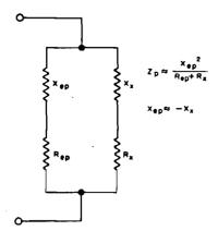
Figure 1-101. Equivalent parallel-resonant circuit of crystal unit  $(X_{cp},\,R_{cp})$  shunted by load  $(X_{cp},\,R_{c})$ . Normally  $f_r < f_p < f_a$ , so that  $X_{cp}$  is inductive and  $X_c$  is capacitive
