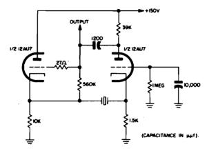
Figure 2-4. Schematic diagram of typical oscillator designed for use with Crystal Unit CR-16/U
