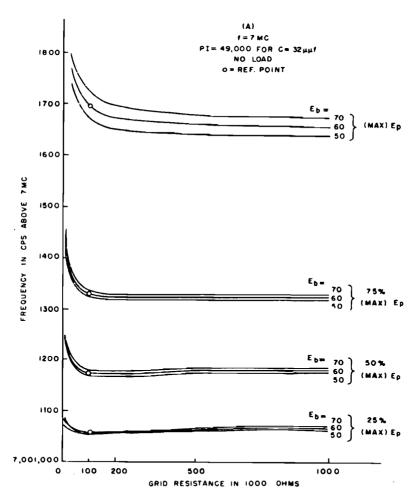
Figure 1-129. Frequency of tuned Pierce oscillator versus plate voltage and grid resistance for various platetuned load capacitances. (Max) E, represents plate tuning adjustment that provided maximum r-f plate voltage when grid resistance and d-c plate voltage were values indicated by zero reference point. A 7-mc CR-18/U crystal unit was used, having a PI of 49,000 ohms when operating into a rated load capacitance of 32 μμf
