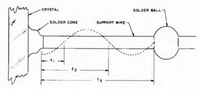
Figure 1-84. Solder-cone resonant-wire support. The solder ball "tunes" the wire to the crystal frequency if it is placed at a distance equal to an odd multiple of a quarter wavelength (l<sub>1</sub>, l<sub>2</sub>, etc.) from the peak of the solder cone \*
