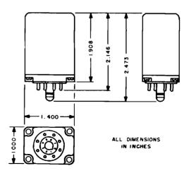
Figure 4-20. Dimensions of Crystal Oven HD-54/U
