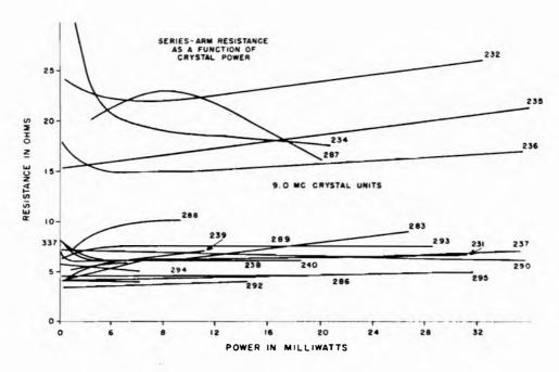
Figure 1-116. Resistance deviation versus drive for a random sample of 9-mc A elements. Curves are for the same sample of crystal units whose frequency-drive characteristics are shown in figure 1-115. Correspondingly numbered curves are those of the same crystal unit
