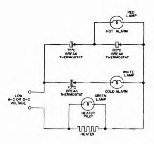
Figure 4-10. Thermostat monitoring and alarm circuit
