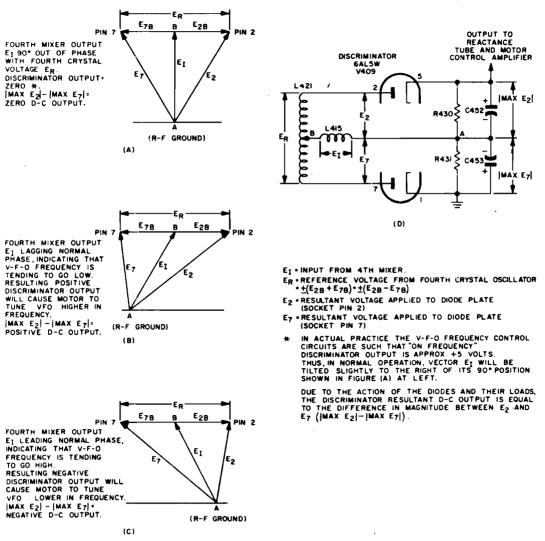
Figure 1-197. Discriminator operation as a function of the phase difference between the input voltages
