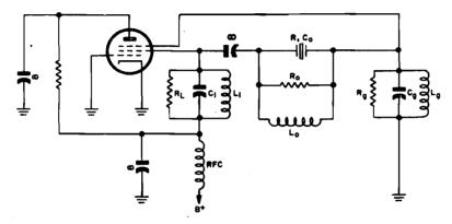
Figure 1-181. Transitron crystal oscillator
