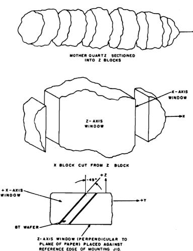
Figure 1-61. X-block method of cutting waters from unfaced stone. Waters, on being diced, provide crystal blanks of the proper orientation
