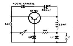
Figure 1-236. Frequency-stabilized circuit for single battery supply
