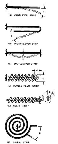
Figure 4-4. Basic types of bimetallic strips
