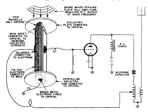
Figure 1-1. The first crystal- (Rochelle salt) controlled oscillator. Invented by A. M. Nicolson, 1918
