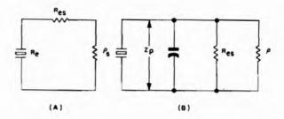
Figure 1-258. Equivalent circuit during build-up period of generalized negative-resistance crystal oscillator.
