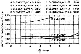
Figure 1-95. Approximate values of the ratio of capacitances,  $r_c = \frac{C_c}{C}$ , for various plated crystal elements
