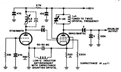
Figure 2-26. Schematic diagram of typical oscillator designed for use with Crystal Unit CR-32/U
