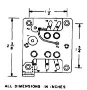
Figure 4-21. Dimensions of Bendix Radio Crystal Oven L205628
