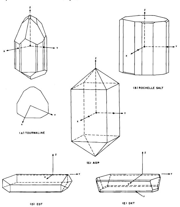
Figure 1-2. Commercially used piezoelectric crystals other than quartz
