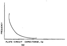
Figure 1-125. Variation of activity and frequency in Pierce oscillator as plate-circuit capacitance is increased
