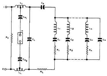
Figure 1-90. Equivalent circuit of crystal unit
