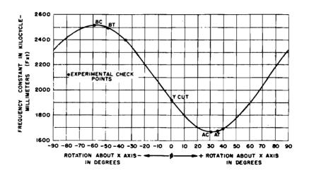
Figure 1-43. Frequency constant versus angle of rotation about X axis for thickness-shear elements of Y group.
