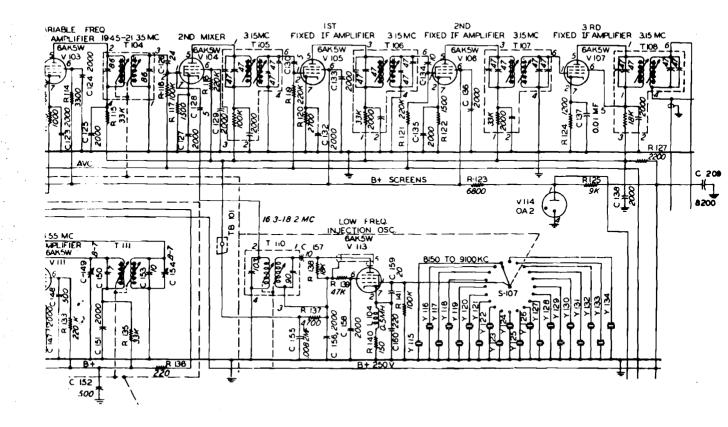
Figure 1-200. Block diagram of the Collins crystal-controlled, multichannel, frequency-control system as employed in the double-conversion superheterodyne circuit of Radio Receiver R-252A/ARN-14
