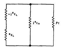
Figure 1-122. Generalized Pierce oscillator.  $Xz_L$  and  $X_{cn}$  represent the positive magnitudes of the equivalent reactances of the load and the dynamic effects of the tube, respectively.  $\rho_T$  is the same as the  $\rho_T$  in figure 1-121
