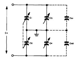
Figure 1-134. Ganged capacitances to enable adjustment of C<sub>p</sub>/C<sub>p</sub> ratio of Pierce circuit without changing total load capacitance
