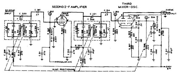
Figure 1-208. Second i-f amplifier unit in Radio Receiver R-278/GR. Schematic diagram
