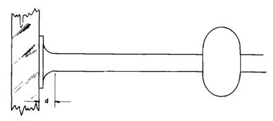
Figure 1-87. Headed-wire crystal support \*
