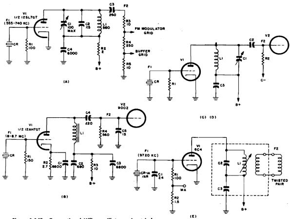
Figure 1-149. Conventional Miller oscillators using triodes
