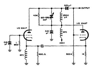
Figure 2-40. Schematic diagram of typical oscillator designed for use with Crystal Unit CR-40/U
