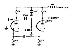
Figure 2-78. Schematic diagram of typical oscillator designed for use with Crystal Unit CR-60/U
