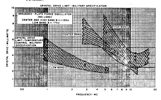
Figure 1-245. Typical drive levels and operating tolerances to be expected for crystal units connected in the grounded-plate Pierce circuit of Gruen packet series. The values shown assume no resistance losses in the output load
