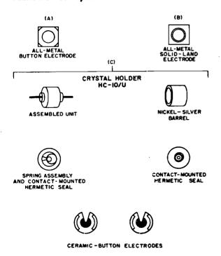
Figure 1-79. Button electrodes and methods of mounting
