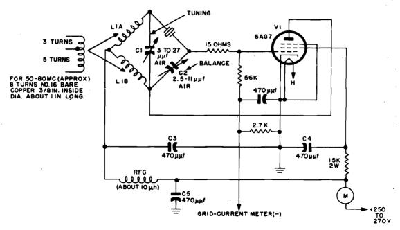
Figure 1-169. A capacitance-bridge oscillator for higher power output which is practical for operation in the 50-80-mc frequency range. Resistors not otherwise specified are ½ w. All fixed capacitors have mica dielectrics
