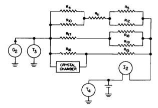
Figure 4-14. Thermal D-C path of heater power
