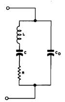
Figure 1-91. Simplified equivalent circuit of crystal unit
