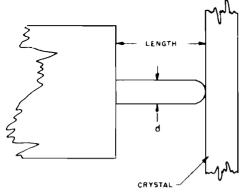
Figure 1-81. Cantilever clamp for providing a resonant-pin support for the crystal \*
