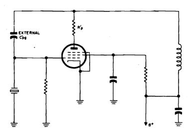
Figure 1-142. The large resistance,  $R_\mu$ , connected in plate circuit effectively increases  $R_\mu$  of the tube. This method can be used to improve the frequency stability of a Miller oscillator employing a screen-grid tube and an externally connected feed-back capacitance,  $C_{\mu\mu}$
