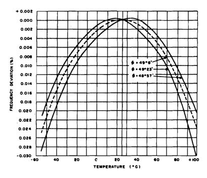
Figure 1-50. Temperature-frequency characteristics of element 8
