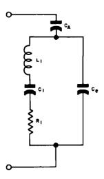
Figure 1-92. Simplified equivalent circuit of air-gap crystal unit
