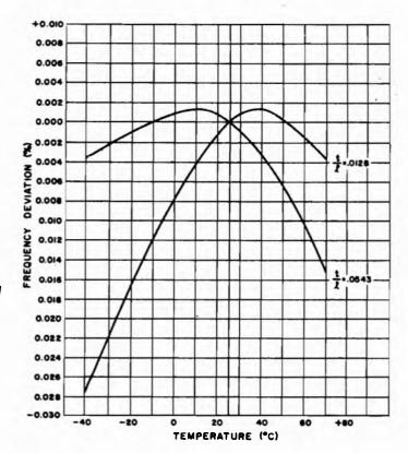
Figure 1-31. Percentage frequency deviation for J elements. The smaller t/l ratio is representative of a 1.2-kc element, and the larger t/l ratio is representative of a 10-kc element
