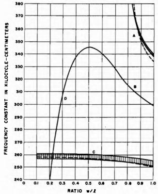
Figure 1-32. Frequency constant versus w/l ratio for various resonances of —18° X-cut crystal. A is the width-extensional mode. B is the face-shear mode, which, at small w/l ratios, is strongly coupled to D, the second flexural mode. C represents the band between the antiresonant (upper curve) and the resonant (lower curve) frequencies of the length-extensional mode of element F. Note the weak coupling between C and D-B \*
