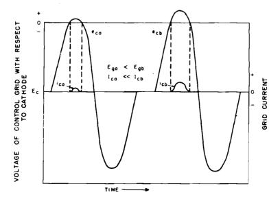
Figure 1-107. How a small percentage change in excitation voltage can cause a large percentage change in grid-leak current of CI meter. Bias does not actually remain constant as indicated, but follows the percentage changes of excitation voltage. Nevertheless, the relative percentage variations of grid current and excitation voltage can be approximately as shown when the greater part of the bias is developed across the cathode resistance
