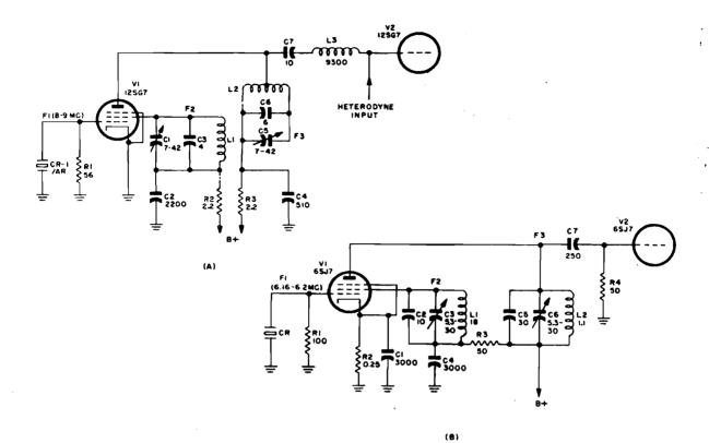
Figure 1-152. Electron-coupled Miller oscillators. All circuits except (A), (B), and (C) are tri-tet modifications
