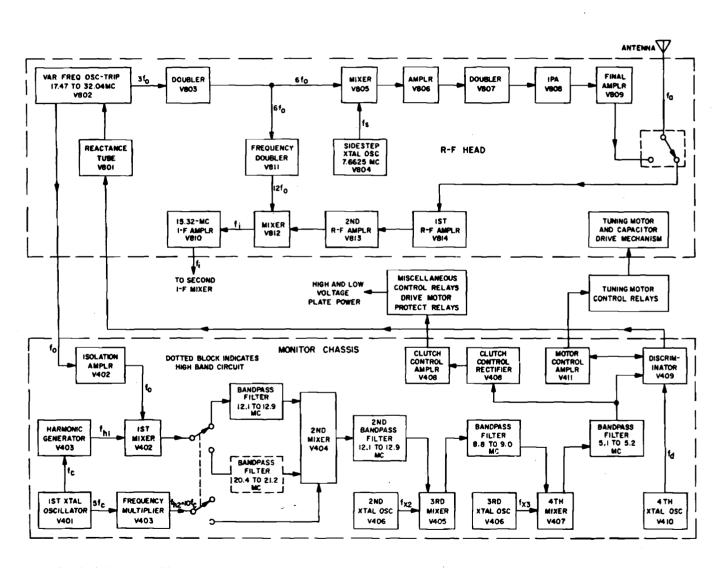
Figure 1-192. Block diagram of frequency control section of Radio Set AN/ARC-33 showing modified version of Bendix synthesizing system
