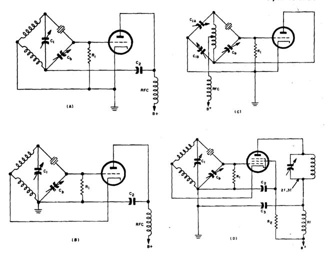
Figure 1-172. Miscellaneous capacitance-bridge oscillators
