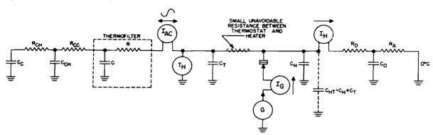
Figure 4-16. Oven thermal A-C circuit
