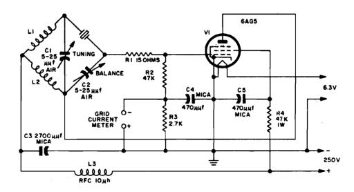
Figure 1-167. A single-tube capacitance-bridge oscillator which is practical for operation in the 50-90-mc frequency range. Resistors not otherwise specified are ½ w. L-1 and L-2 are a single center-tapped coil of suitable inductance
