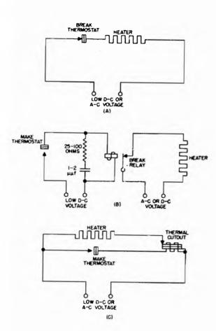
Figure 4-6. Bimetallic thermostat circuits
