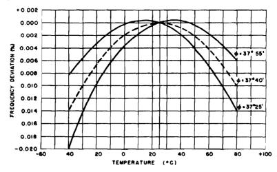
Figure 1-51. Temperature-frequency characteristics of element C
