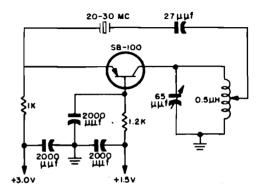
Figure 1-227. High-frequency transistor oscillator
