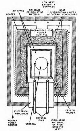
Figure 4-1. General construction features of typical crystal oven
