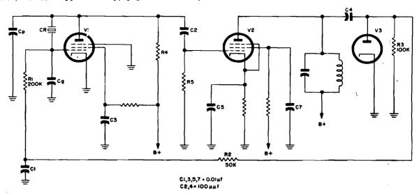
Figure 1-131. Pierce oscillator with automatic gain control
