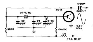
Figure 1-257. Schematic diagram of crystal-controlled transistor circuit employed in James Knights m-f and h-f (0.1 to 10 mc) oscillators. Relatively pure sinewave output
