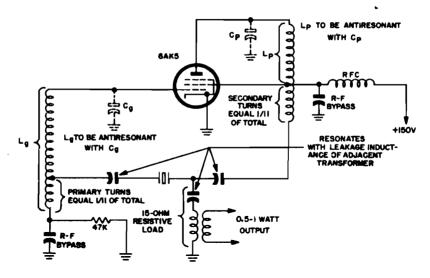
Figure 2-60. Schematic diagram of typical oscillator designed for use with Crystal Unit CR-51/U
