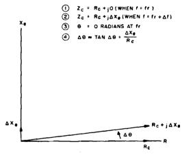
Figure 1-111. Phasor diagram, showing change in reactance,  $\Delta X_c$ , of series-mode crystal required to produce a small change in phase,  $\Delta \theta_c$ , where the resistance of the crystal circuit is equal to  $R_c$
