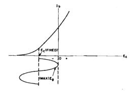
Figure 1-127. Point on E<sub>c</sub> I<sub>b</sub> curve at which stable oscillations can be achieved with fixed bias. For minimum grid losses, the peak of the maximum excitation voltage must not exceed the fixed E<sub>c</sub>
