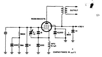
Figure 2-32. Schematic diagram of typical oscillator designed for use with Crystal Unit CR-36/U
