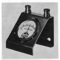
Fig. 1-5. A Weston center zero galvanometer.
