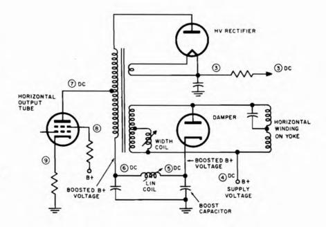
Fig. 12-27. Typical horizontal output system and high-voltage supply.
