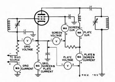
Fig. 13-2. Class-C r-f amplifier for transmitter, current, and valtage measurements.
