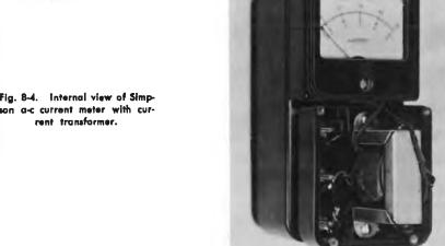
Fig. 8-4. Internal view of Simpson a-c current meter with cur-
