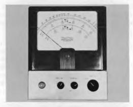
maximum. It is an obvious advantage here to have a meter whose pointer will indicate only between the limits of interest and will thus allow the meter to be read much more easily and definitely. This is accomplished by a suppressed-zero type of meter, which was introduced previously in Chap. 2. A commercial version featuring the open scale is seen in Fig. 15-2.
