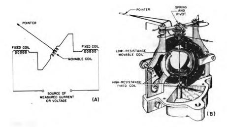
Fig. 2-8. The electrodynamometer: (A) schematic showing how the magnetic fields of the fixed and movable coils interact to cause the latter to rotate; (B) constructional details.
