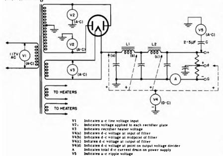
Fig. 12-23. Conventional full-wave B supply.
