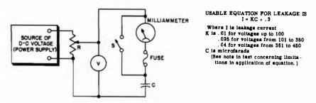
Fig. 11-8. Arrangement for measuring leakage current of capacitors.
