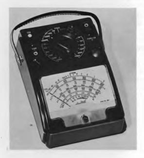
Fig. 15-3. Burnout-proof multimeter. Hickok model 455
