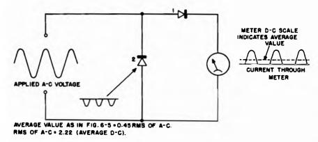
Fig. 6-3. Double-rectifier arrangement, which minimizes "back-current."
