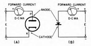
Fig. 12-36. Connection for forward-resistance check of: (A) tube diade, and (B) crystal diade.
