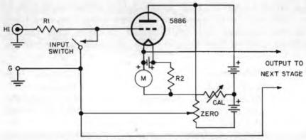
Fig. 14-7. Simplified input circuit of electrometer. Keithley
