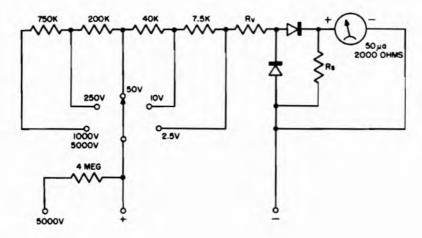
Fig. 8-8. Multiplier arrangement for a multi-range a-c voltmeter.
