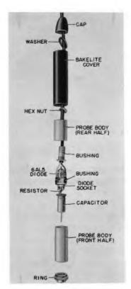
Fig. 9-19. Disassembled RCA duo-diade probe used for measurements from audio frequencies up to about 250 mc.
