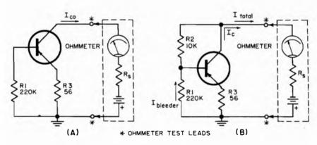
NOTE: The meter resistor  $\mathbf{R_S}$  and battery are integral parts of the ahmmeter used on its RXIOO range
