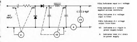
Fig. 12-24. Selenium rectifier power supply (full-wave voltage doubler).
