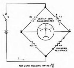
Fig. 11-4. Wheatstone-bridge circuit for measuring resistances.
