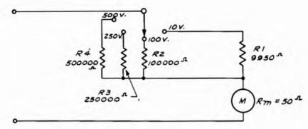
Fig. 8-6. Simple switching system for selecting multi-range voltmeter multipliers.
