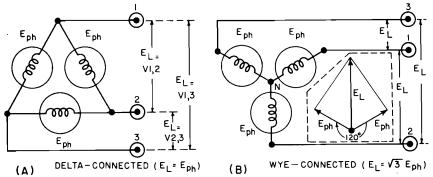
Fig. 5-6. Three-phase, three-wire generator connections showing relation of line voltage E<sub>L</sub> to phase voltage E<sub>PH</sub>: (A) delta-connected; (B) wye-connected.
