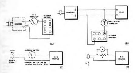
Fig. 11-3. (A) An ammeter connected to indicate rate of battery charge. (B) A centerzero meter used as a charge-discharge instrument. (C) and (D) Ammeter and voltmeter connected to measure current drain and power of device operated from the power line.
