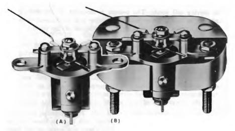
Fig. 1-3. Assembly of commercial moving-cail meter: (A) full double-bridge suspension of D'Arsonval movement; (B) movement assembled on permanent magnet without scale.
