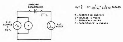
Fig. 11-10. Use of a-c source and current meter to measure capacitance. The a-c voltage source can be an isolation transformer with a 120-volt output.
