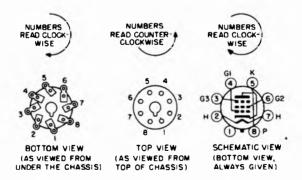
Fig. 12-4. Relation between the top and bottom views of an actal socket and schematic diagram of the tube as it would appear on a circuit diagram.
