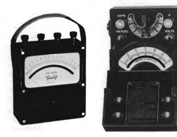
Fig. 8-1. Photos of multi-range instruments with terminals and with switch selector.
