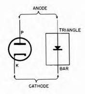
Fig. 12-35. Crystal-diode symbol corresponding to tube-diode symbol.
