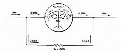
Fig. 3-1. How the current range of a meter is increased by addition of a shunt resistar.
