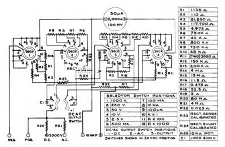
Fig. 8-12. Schematic of Simpson model 260 VOM.
