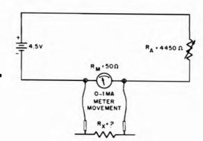
Fig. 4-4. Circuit of shunt type ohmmeter.
