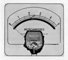
Fig. 1-9. Cutaway view of "taut-band" suspension-type meter. Hickok
