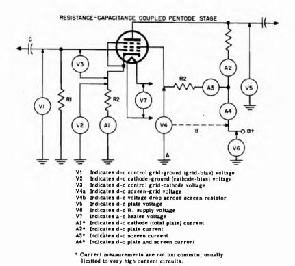
Fig. 12-15. A pentode resistance-copacitance-coupled amplifier stage and typical meter reading locations. For a triode in the same circuit, simply eliminate the screen grid and suppressor circuits.
