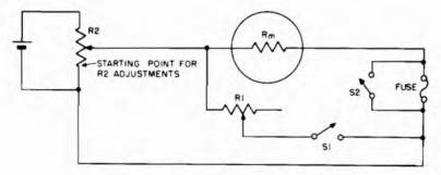
Fig. 3-10. Method for determining meter resistance.
