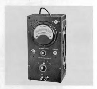
Fig. 14-3. Logarithmic-type meter, Ballantine a-c VIVM model 300
