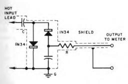
Fig. 9-21. Simple peak-to-peak r-f probe for VTVM.
