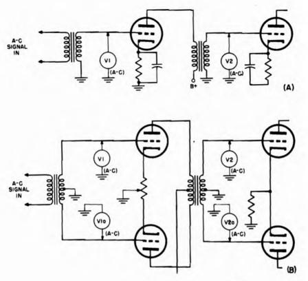
Fig. 12-32. Measuring gain in transformer-coupled amplifier.
