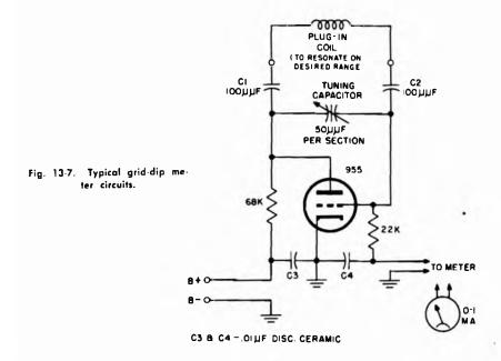
circuit to which the coil is coupled, the grid current "dips." The dial connected to the variable capacitor is calibrated to read frequency. Thus, the resonant frequency of a circuit in a transmitter or receiver can be determined.
