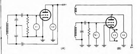
Fig. 12-19. Examples of operating voltages: (A) d-c in Colpitts oscillator; (B) d-c and a-c in tickler feedback oscillator.
