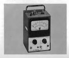
Fig. 14-6. Electrometer. Keithley model 210
