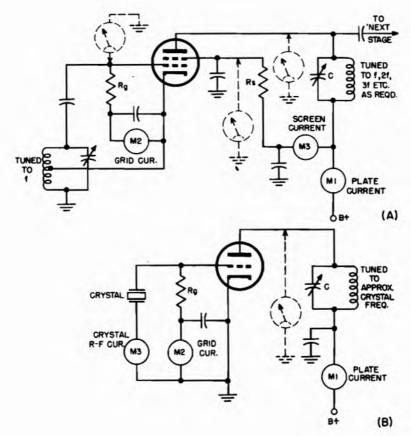
Fig. 13al. Oscillator circuits: (A) electron coupled circuit such as is used for the frequency-controlling circuit of transmitters, and locations of typical meter measurements;
