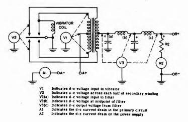
Fig. 12-25. Full-wave synchronous vibrator power supply.
