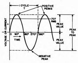
Fig. 2-2. Basic sine wave, showing how the current or/voltage builds up in one direction, returns to zero and then builds up in the other direction, finally returning to zero at the end of a complete cycle.
