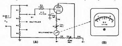
Fig. 9-3. (A) A center-zero instrument. (B) Typical scale calibration.
