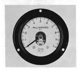
Fig. 1-6. Long-arc (250°) meter scale. Weston
