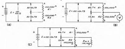
Fig. 3-12. Effect of voltmeter resistance an circuit resistance: (A) with voltmeter not present; (B) with voltmeter connected across R2; (C) equivalent circuit of B with voltage connected across R2 shows how the voltage drops across R1 and R2 are changed from those shown without the voltmeter.
