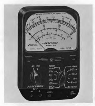
Fig. 15-4. Packet-size multimeter. Precision Apparatus model 110
