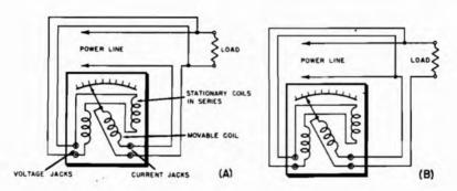
Fig. 5-4. Organization of dynamometer type wattmeter.
