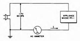
Fig. 5-3. Diagram of arrangement which measures power with an ammeter providing the voltage is constant and the power factor of the load is 1.
