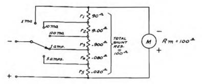
Fig. 8-3. A universal shunt operated by means of a single-gang switch.
