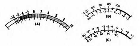
Fig. 6-8. Db scale and standard VU meter scales. The scale at (B) emphasizes arbitrary units proportional to voltage. The scale at (C) emphasizes the VU calibration.
