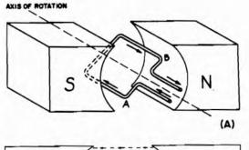
Fig. 1-1. Illustration of the basic motor principle employed in moving-call permanent-magnet meters.
