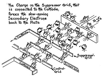
secondary electrons. In the absence of the suppressor-grid these secondary electrons would, because of the positive potential on the screengrid, flow to the screen-grid. The suppressor is, however, at cathode (or ground) potential and therefore exerts a retarding effect upon these secondary electrons so that they are forced to return to the plate.
