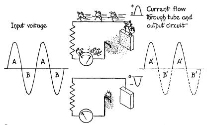
Plate current flows during positive alternation and plate is positive with respect to cathode. Plate current does not flow when plate is negative with respect to the cathode. Thus output current and voltage is unidirectional although input is alternating.
