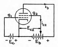
and the control-grid perform in the tetrode the same as they do in the triode.
