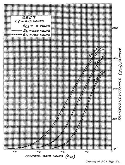
FIG. 12-11. These curves show how the transconductance of the 6SJ7 pentode varies for changes in control-grid and suppressor-grid voltages.
