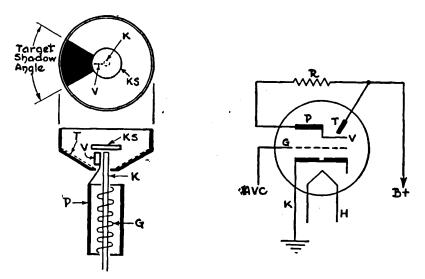
FIGS. 15-39 (left), 15-40 (right). The arrangements of the elements of a visualindicator tube are shown on the left, and the way this tube is connected in a circuit is shown on the right.
