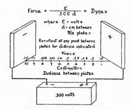
evident that increasing the separation between the plates to 20 centimeters would decrease the force to 0.05 dyne, assuming, of course, that the voltage between the plates remains 300 volts.
