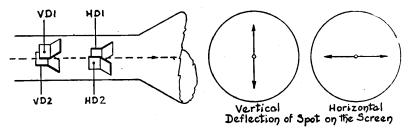
Fig. 15-29. VD1 and VD2 represent the plates that deflect the electron stream vertically, and HD1 and HD2 the plates that deflect the electron stream horizontally.
