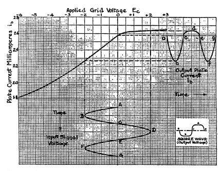
FIG. 11-14. By including a large resistance in the grid circuit, and driving the grid voltage into the positive region, the output waveform will have one side considerably flattened.
