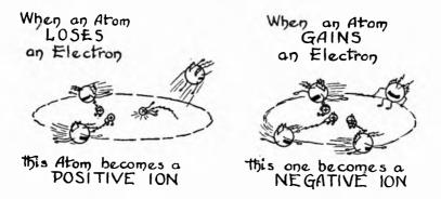
An atom which has an excess of positive electricity within it, due to loss of one or more planetary electrons, is called a *positive ion*; whereas an atom which has an excess of electrons, and which, therefore, is electrically negative, is identified as a negative ion. The process of producing ions is known as ionization.
