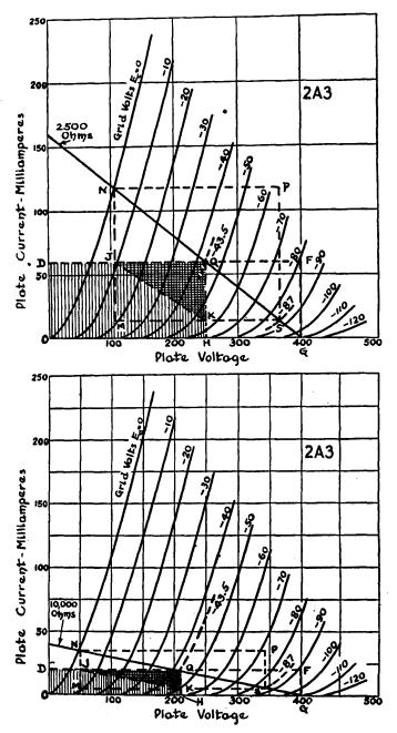
FIGS. 14-6 (above), 14-7 (below). In these four sets of curves, observe how the proportion of power output area (QJK) and the plate dissipation area (ODJKH) changes as the load resistance is changed.
