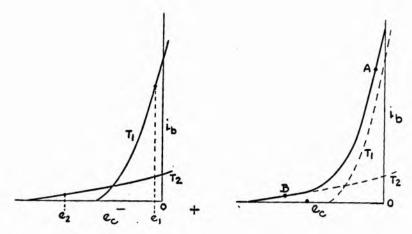
FIGS. 15-17 (left), 15-18 (right). The curves marked  $T_1$  and  $T_2$  are the dynamic transfer characteristics of tubes  $T_1$  and  $T_2$  respectively of Fig. 15-16. The curve on the right is a combination of the two curves on the left and is the characteristic of a variable-mu amplifier.
