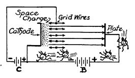
electrons, it must be in a direction which is *away* from the control grid. Thus the arrows which originate at each of the grid wires point away from the grid.
