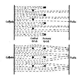
of the two grids are not arranged in this fashion, electrons are forced out of their paths by the negative charge on the control-grid and a large number of these are attracted by the positive charge of the screen-grid, thus forming the screen current, while other electrons, although deviating from their paths, miss the screen-grid and continue on to the plate. This action is illustrated in Fig. 14-12, wherein the lines indicate the paths of a few of the electrons.
