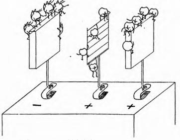
charged will have a field which will act in such direction as to attract a negative charge and repel a positive charge, while a plate which is negatively charged will attract a positive charge and repel a negative charge.
