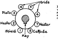
FIG. 15-4 (right). Diagram of an 11-prong tube base used with a cathode-ray tube. F10. 15-3 (left). Bottom view of an octal tube base showing prongs to which elements are sometimes connected.
