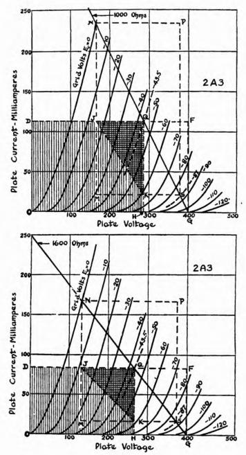
FIGS. 14-4 (above), 14-5 (below). In these two and the two graphs on the next page, different load lines are drawn on the plate family of a 2A3 for different values of loads as indicated, in order to indicate the power output and plate dissipation.
