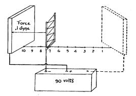
voltage required upon the original plates, which were separated by 10 centimeters in order to create the same change in the force upon the unit charge, is 540 volts. Thus we see that this third electrode is about 3.3 times as effective as the positive plate in controlling the force upon the test charge.
