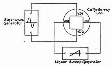
FIG. 15-36. When the sine-wave voltage and the linear sweep voltage have the same frequency, then a single cycle of the sine wave will be traced on the screen, as shown in Fig. 15-37.
