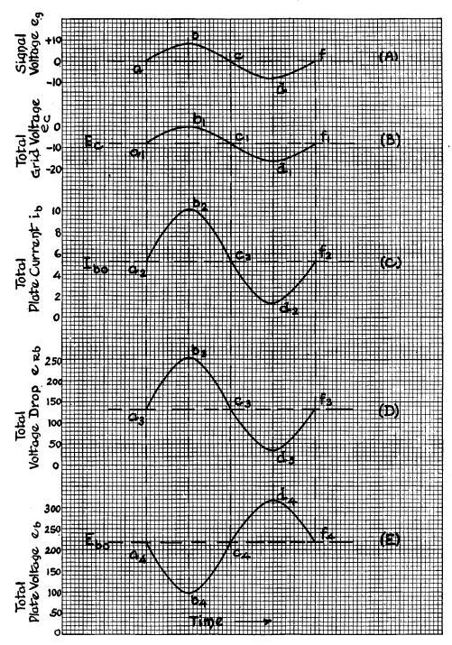
Fig. 11-8. This series of waves shows that the input voltage  $e_s$  is in phase with the plate current  $i_b$  and that  $e_s$  is 180° out of phase with the plate voltage  $e_b$ .
