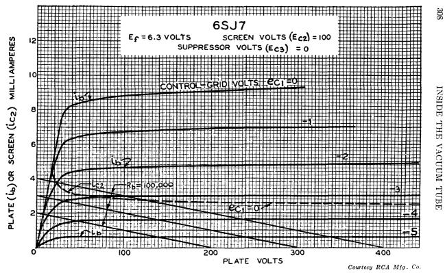
FIG. 12-19. The three load lines, for the same 100,000-ohm load, are drawn for three different values of plate-supply voltage, 200, 300, and 400 volts.
