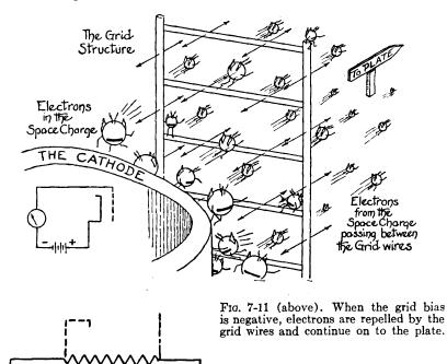
FIG. 7-12 (left). A negative grid bias is the equivalent of a very high resistance between the cathode and grid that prevents any current flow.
