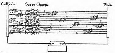
With a certain voltage impressed between the Plate and Cathode and with a certain Cathode temperature, as many Electrons enter the Space Charge from the Cathode as leave it for the Plate
