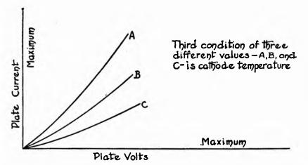
It is because of the above that you will usually see at least three quantities given in connection with any one vacuum-tube characteristic curve: the two variables illustrated in the curve and a third, each indicating the exact condition the other factor contributes to the behaviour illustrated in the characteristic curve.
