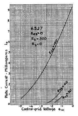
actual working conditions, insofar as they represent more nearly ideal operation than would be the case with a resistive load of high magnitude. Since, as we have already indicated, audio-frequency voltage amplifiers are generally operated at low screen-grid voltages, we observe how limited the permissible control-grid swing becomes. This partly accounts for the rule that the input signal to a voltage amplifier pentode should never exceed several tenths of a volt.
