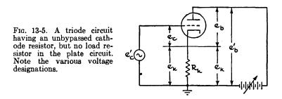
signal voltage applied between grid and ground is designated  $e'_{c}$  in order to indicate that it is equivalent in nature to the actual instantaneous grid voltage  $e_{c}$ , but that  $e'_{c}$  is the instantaneous grid-to-ground voltage, whereas  $e_{c}$  represents the instantaneous grid-to-cathode voltage. Similarly,  $e'_{b}$  signifies the instantaneous plate-to-ground voltage, as compared with  $e_{b}$  which is the instantaneous plate-to-cathode voltage.
