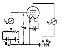
the plate voltage at a low value, we slide the movable arm of the potentiometer towards the middle, making the grid voltage less and less negative. While this is being done, the plate milliammeter shows an increasing plate current, but still nothing is indicated on the grid microammeter. More electrons go to the plate (as indicated by the increasing plate current) because the plate-cathode field is less and less counteracted by the gradual reduction of the grid-cathode field.
