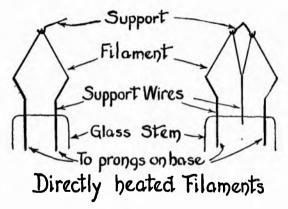
form of an inverted V or W, being mounted and held in place by suitable metal supports which rest in the glass stem of the tube. The filament voltage is applied across the prong terminals of the filament in the tube base and the current flowing in the filament heats it to the electron-emitting temperature.
