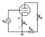
FIG. 13-1. The plate current returning to the cathode passes through the cathode resistor  $R_k$  and causes a voltage drop equal to the product of the current and the value of the resistance.
