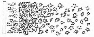
creases. When this increase in density nas again reached such a value that the repelling force of the electrostatic field of the space charge is sufficient to overcome the higher average velocity of the electrons emitted at the increased cathode temperature, and is again repelling the emitted electrons, a new state of equilibrium has again been established and *emission saturation* again exists.
