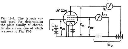
the graph of Fig. 12-6. The tetrode used in this test was the now obsolete filament-type UY-224, because it exhibits certain properties of fundamental interest which later types of tetrodes do not show. Curves for just one control-grid and screen-grid voltage setting are shown in Fig. 12-6 for illustrative purposes: the control-grid voltage  $e_{ct}$  is equal to -1.5 volts and the screen-grid voltage  $e_{ct}$  is equal to +75 volts.
