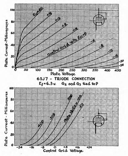
FIGS. 12-23 (above), 12-24 (below). The plate and grid families of a 68J7 connected as a triode with the screen and suppressor grids connected.
