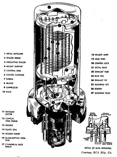
FIG. 15-8. Constructional details of a metal pentode.
