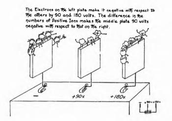
to an intermediate terminal, which happens to be 90-volts plus, then has the deficiency of electrons which would charge that plate 90-volts plus with respect to the negative plate. If the third plate is connected to the plus 180-volt terminal of the voltage source, that terminal has a deficiency of electrons (a preponderance of positive ions) equal to the surplus upon the negative plate, but twice as many positive ions as the plate which is joined to the 90-volt terminal of the voltage source.
