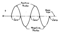
voltage and the signal voltage. Assuming for the moment that the signal voltage  $e_{\sigma}$  is of alternating character, you can see that in a wave of alternating voltage, as well as current, there are instants when the value of the alternating component of voltage or current is zero. These contrast with the other instantaneous values, which reach their maximum at the peaks of the positive and negative half cycles, as shown in Fig. 10-3.
