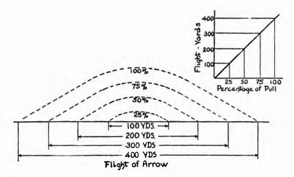
can easily realize that the further back from the bow the archer stretches the string on which the arrow is notched, the further will the arrow travel when it is released. For the sake if illustration, let us say that if he draws the string to  $\frac{1}{4}$  of its full capacity, the arrow
