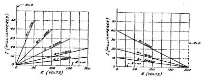
FIGS. 9-3 (left), 9-4 (right). A resistance having a fixed value can be represented by a straight line; those in Fig. 9-3 are for resistance when the voltage is unknown, and those in Fig. 9-4 are for resistance when the supply voltage is known.
