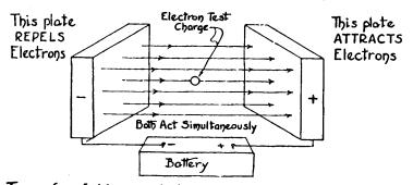
The uniform field is due to the existence of two forces acting on the electron and the fact that the sum of these forces remains the same no matter where the electron may be located between the two fixed charged plates.
