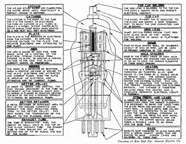
Constructional details of a duo-diode triode indirectly-heated tube.
