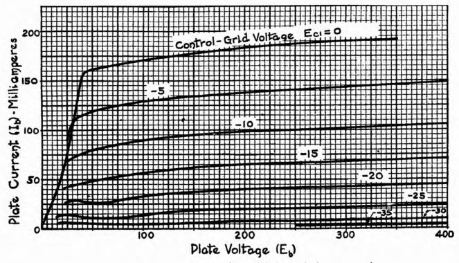
FIG. 14-15. Plate voltage-plate current characteristic curves of a beam power tube.
