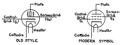
FIG. 12-2. The use of zigzag lines representing the grids in tube symbols has been replaced by dashed lines making for simpler representation of multi-element tubes.
