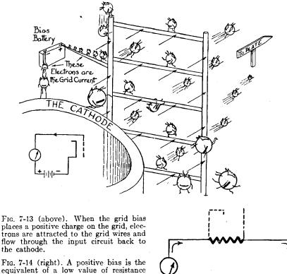
FIG. 7-14 (right). A positive bias is the equivalent of a low value of resistance between the cathode and grid through which electrons can easily flow.
