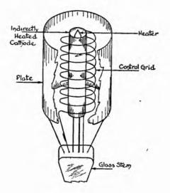
FIG. 7-2. In general, the control grid is a helix that surrounds the cylindrical cathode and in turn is surrounded by the cylindrical plate. These electrodes are supported by wires embedded in the glass stem of the tube base.
