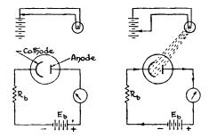
FIGS. 15-47 (left), 15-48 (right). When no light energy falls on the cathode of a photocell, no electrons flow through the anode circuit in which is connected the load  $R_h$ . In Fig. 15-48 light is indicated hitting the cathode of the photocell with a resulting current flow through the anode circuit.
