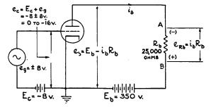
a comparison, we have included a companion circuit, Fig. 9-2(A), which is the same as Fig. 8-2. As was stated before, the triode has many other possible functions beside serving as an amplifier, but as long as the tube is used as a triode, its inherent property of amplification is employed and this particular function must be understood.
