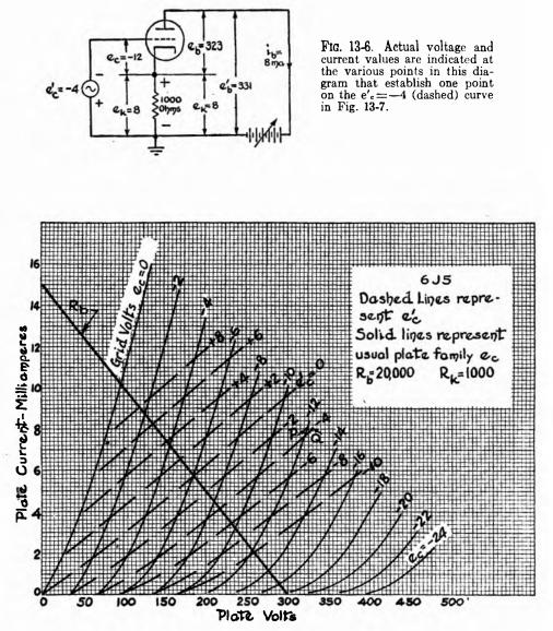
FIG. 13-7. The new plate family (dashed lines) when a cathode resistor of 1000 ohms is used, is drawn upon the usual plate family (solid lines) of a 6J5 triode. The load line is for a plate load resistance of 20,000 ohms. Refer to Table A (page 331) for values of new plate family.
