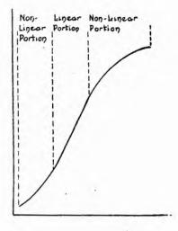
On the other hand, the entire characteristic may be non-linear, depending upon the conditions of operation. A quantitative example of a non-linear curve is given herein and it can be compared with the linear example also given. In contrast to the linear example, the conditions in the non-linear case are such that the change in effect is not directly proportional to the change in the cause. Stated differently, a uniform change in voltage does not produce a uniform change in current.
