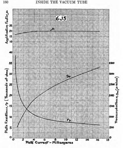
FIG. 8-13. These three curves show the relationship between the amplification constant  $\mu$ , the transconductance  $g_m$ , and the plate resistance  $r_p$  for a 6J5 triode.
