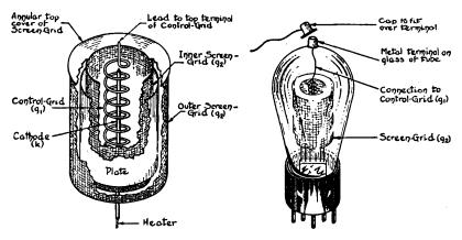
FIG. 12-1. The arrangement of the four elements of the tetrode is shown at the left. The control grid is connected to the metal cap at the top of the glass envelope, as shown on the right.
