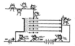
FIG. 7-10. When the grid circuit is open, the grid is said to be "floating." Electrons on their way to the plate, strike the grid wires and remain there. As there is no circuit through which they can flow, they accumulate on the grid and build up a negative charge.
