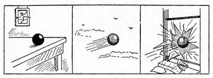
A Ball at rest on a table has no Kinetic Energy
