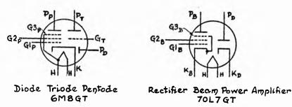
FIGS. 15-13 (left), 15-14 (right). On the left is the symbol of one type of a triple function tube, and that on the right is the schematic of one type of dual purpose tube.
