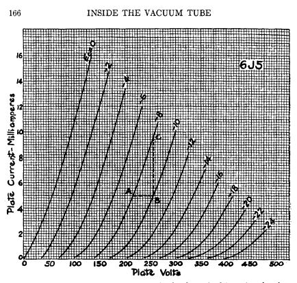
F16. 8-8. The amplification constant can also be determined by using the plate family of characteristic curves as outlined in the accompanying text.
