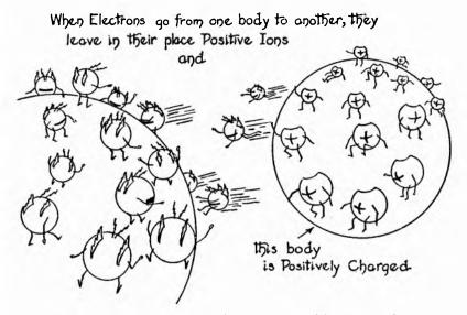
altered whether or not our conception is correct. If, during other operations, this positively charged plate is again made neutral, this is accomplished by supplying electrons to the plate, and not by the movement of positive ions from the plate to some other place in the system.
