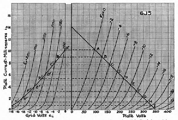
F10. 9-8. The 25,000-ohm load line drawn on the plate family is projected onto the grid family of characteristics, as described in the accompanying text, in order to construct the dynamic transfer characteristic.
