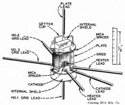
FIG. 15-22. Arrangement of the elements and leads of a pentode tube of the acorn type.
