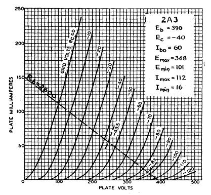
FIG. 14-3. The load line is used to determine the power output of a tube. Here the load line is for a resistor of 2600 ohms, the usable portion of which lies within the boundaries specified in Fig. 14-2.
