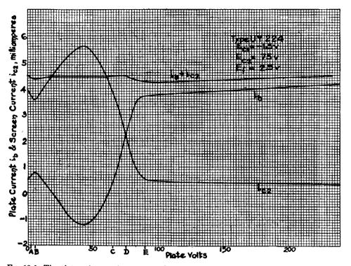
F10. 12-6. The plate voltage—plate current characteristic curves showing the variations of current flow in the plate and screen-grid circuits, (curves marked  $i_b$  and  $i_{c2}$  respectively) and the total current flow, which is the sum of these two currents.
