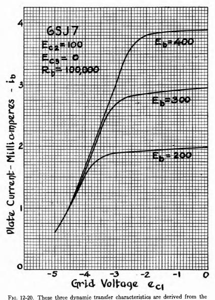
F16. 12-20. These three dynamic transfer characteristics are derived from the load lines of Fig. 12-19 on the opposite page.
