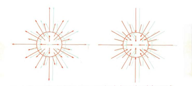
**PLATE** 2. The arrows indicate that the lines of force are away from the electron and towards the proton; the direction of the force exerted upon a negative test charge is indicated by the arrows. The lines of force radiate in all directions.
