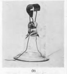
Fig. 72.—Improved Electrode for Fluorescent Lamps: (a) Without Shield (mag. ×2); (b) With Shielding Cylinder (natural size) (Osram HN 120).
