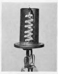
Fig. 68.—Directly Heated Double Spiral Cathode with Heat Shield Used in High-voltage Rectifiers (part of shielding cylinder cut away). (Current density 0.2 amp./cm.²; AEG G 10/4d; ¾ natural size.)
