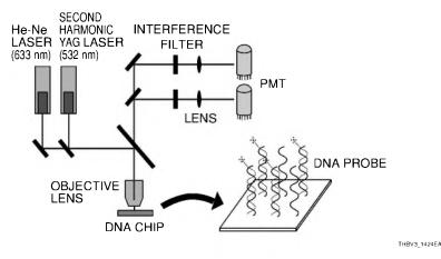
Figure 14-24: DNA microarray scanner
