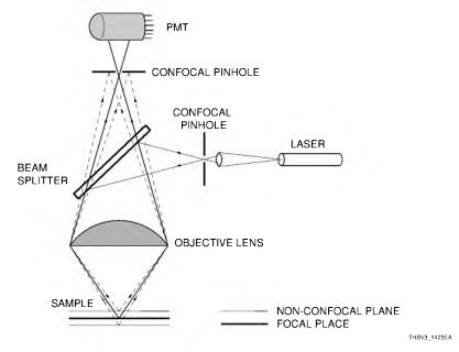
Figure 14-23: Confocal laser microscope
