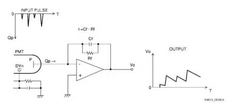
Figure 5-33: Pulse input type charge-sensitive amplifier
