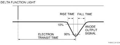
Figure 4-16: Definitions of rise/fall times and electron transit time
