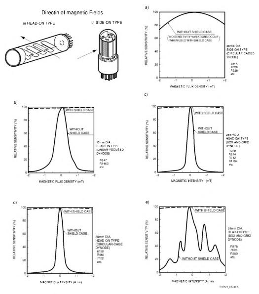
Figure 5-44: Effect of magnetic shield case
