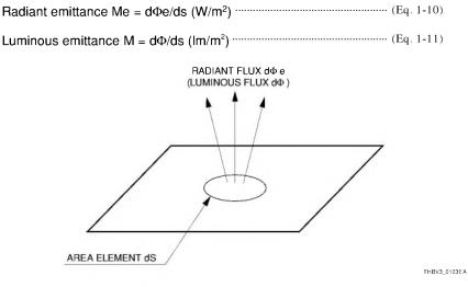
Figure 1-3: Radiant emittance (Luminous emittance)
