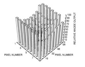
Figure 9-7: 64-channel multianode output uniformity
