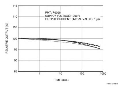
Figure 4-35: Examples of drift data
