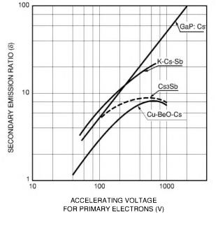
Figure 2-7: Secondary emission ratio
