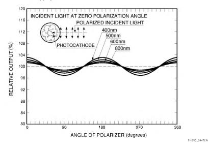
Figure 4-47: Typical polarization-light dependence of a side-on photomultiplier tube
