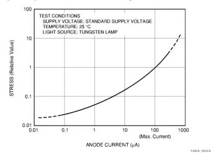
Figure 13-24: Current stress on photomultiplier tubes (at different anode currents)
