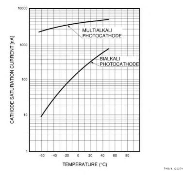
Figure 13-2 shows typical cathode saturation current versus temperature for transmission type bialkali and multialkali photocathodes.
