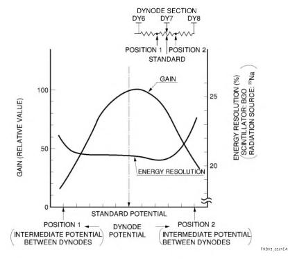
Figure 5-19: Gain variation and energy resolution as a function of dynode potential
