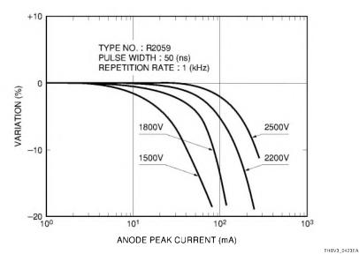
Figure 4-23: Voltage dependence of linearity
