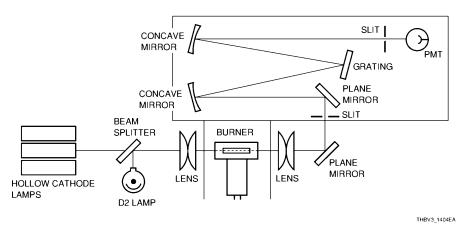
Figure 14-4: Optical system used in atomic absorption spectrophotometers
