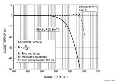
Figure 6-8: Linearity of count rate
