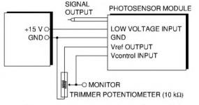
When using a trimmer potentiometer, adjust sensitivity while monitoring Vcontrol (control voltage)
