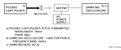
Figure 10-13 (a): Block diagram for MCP-PMT pulse linearity measurement
