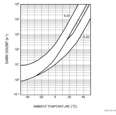
Figure 10-11: Dark count vs. ambient temperature
