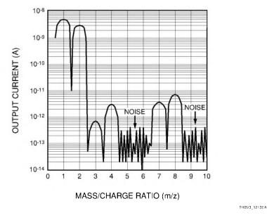
Figure 12-13: Ion source noise measured with an off-axis ion detector
