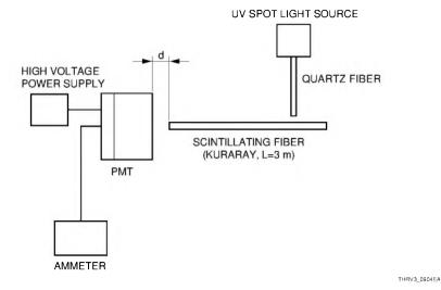
Figure 9-4: Crosstalk measurement method
