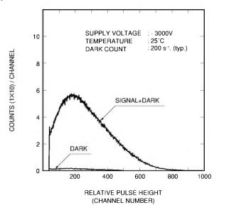
Figure 10-14: Typical pulse height distribution in single photon counting
