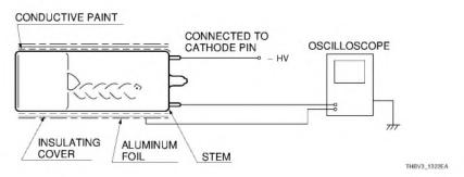
Figure 13-22: Observing the effect of external electric potential on HA coating
