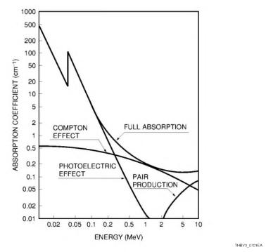
Figure 7-1: Gamma-ray absorption characteristics of Nal(TI) scintillator
