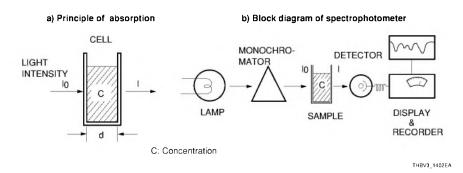
The principle and simplified block diagram<sup>1)</sup> of a spectrophotometer are shown in Figure 14-2.
