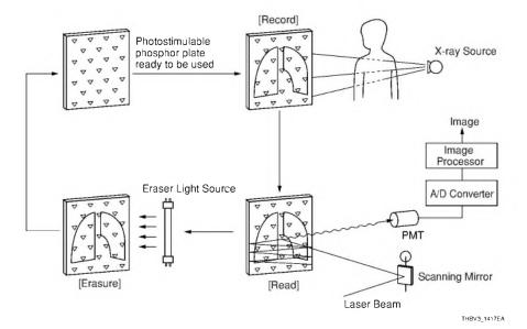
Figure 14-17: X-ray image acquisition using photostimulable phosphor plate
