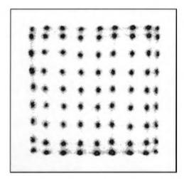
Figure 9-24: Scintillation image obtained by gamma-rays irradiated on mosaic pattern scintillators (BGO)
