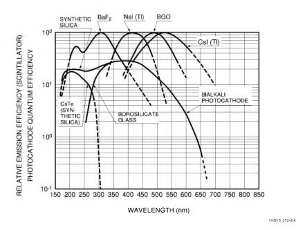
Figure 7-4: Photocathode quantum efficiency and emission spectra of major scintillators
