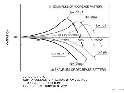
Figure 13-25: Typical time stability of photomultiplier tubes (at different anode currents)
