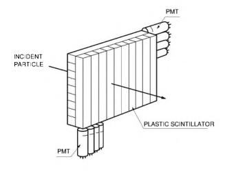
Figure 14-27: Simplified diagram of a hodoscope
