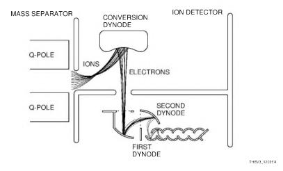
Figure 12-3: Ion detection by an ion detector with a conversion dynode
