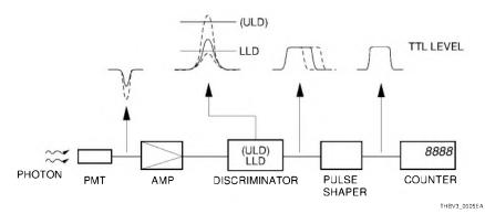
Figure 6-5: Circuit configuration for photon counting
