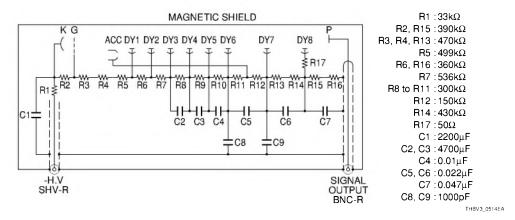
Figure 5-13: Fast-response voltage-divider circuits
