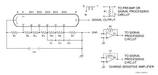
Figure 5-23: Anode grounding scheme in pulse operation
