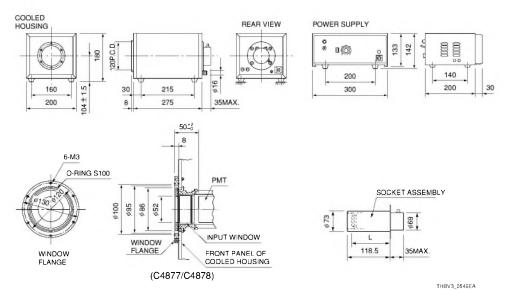
Figure 5-46: Thermoelectric cooler (manufactured by Hamamatsu Photonics)
