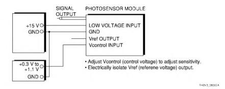
Figure 8-6: Sensitivity adjustment by changing voltage
