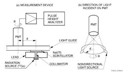
Figure 7-9: Measurement method for azimuth uniformity
