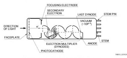
Figure 2-1: Construction of a photomultiplier tube
