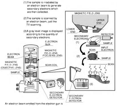
narrowed into a needle-like form and focused onto the sample by the focusing lens and objective lens.
