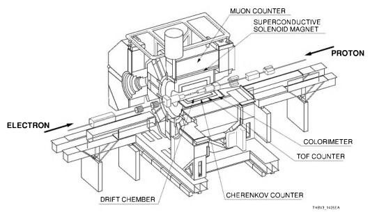
Figure 14-26: Example of collision experiment setup
