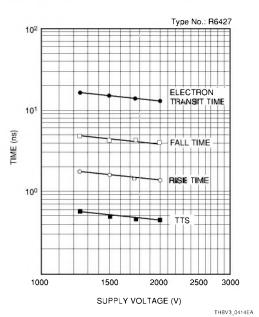
Figure 4-14: Time characteristics vs. supply voltage
