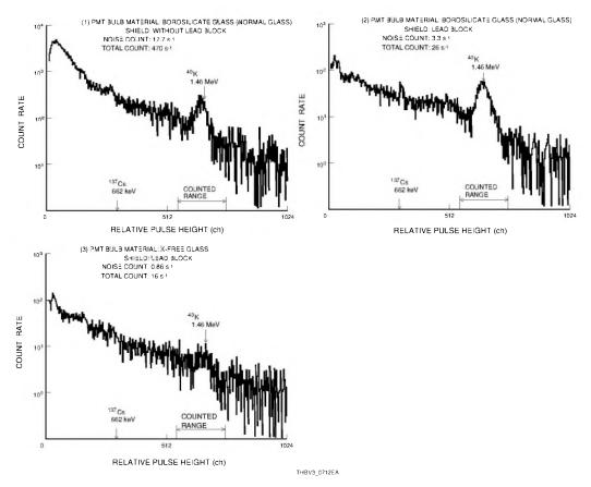
Figure 7-12: Background noise of 5-inch photomultiplier tube + Nal(TI)
