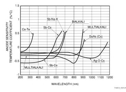
Figure 13-1: Temperature coefficients of photomultiplier tube photocathodes
