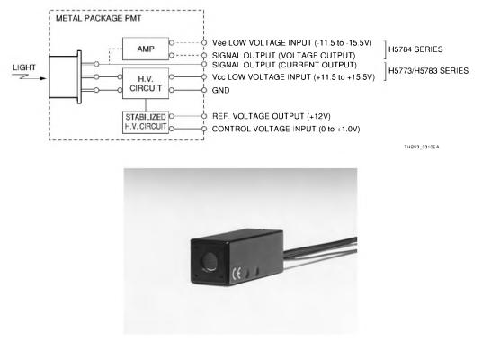
Figure 3-10: Structure of an integral power supply module
