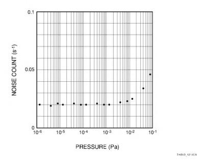
Figure 12-14: Typical noise count vs. pressure level for electron multiplier tubes
