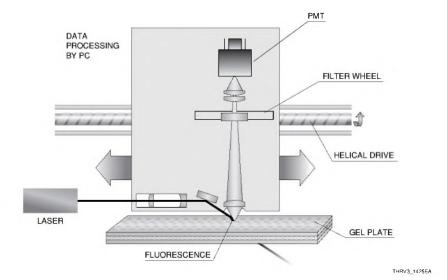
Figure 14-25: Principle of a DNA sequencer
