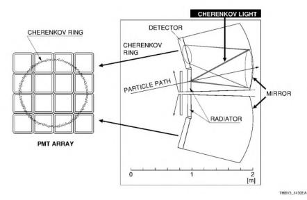
Figure 14-30: Schematic diagram of RICH
