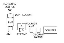
Figure 7-13 (a): Block diagram for plateau characteristic measurement
