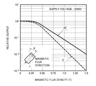
Figure 13-10: Magnetic characteristics of photomultiplier tubes for highly magnetic fields (2)
