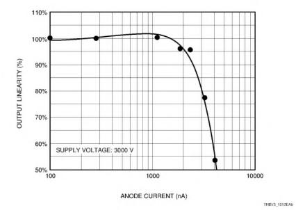
Figure 10-12 (b): Saturation characteristics of MCP-PMT (11 mm effective diameter, 6 μm channel diameter) in DC operation (2)
