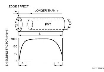
Figure 5-43: Edge effect of a magnetic shield case
