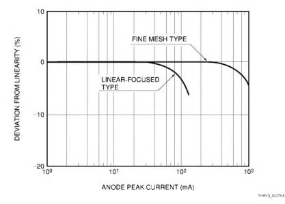
Figure 4-27: Pulse linearity
