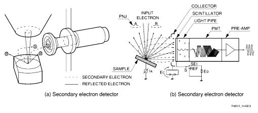
Figure14-49: Structure and operation of a secondary electron detector
