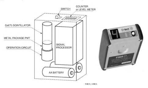
Figure 14-38: Structural view of a handheld radiation monitor
