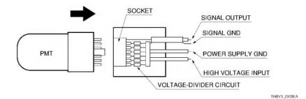
Figure 3-5: D-type socket assembly
