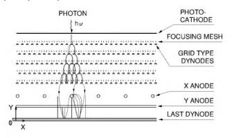
Figure 9-25: Electrode structure and electron trajectories
