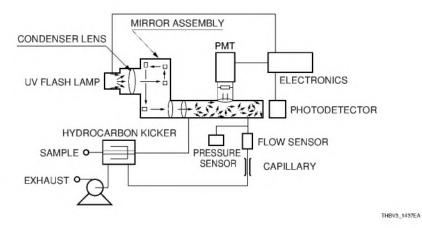
Figure 14-37: Typical setup of a UV fluorescent sulfur dioxide analyzer
