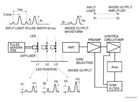
Figure 4-26: Block diagram for pulse mode linearity measurement
