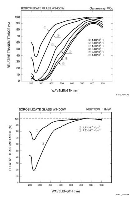
Figure 13-17: Transmittance change of borosilicate glass window irradiated by gamma rays/neutrons
