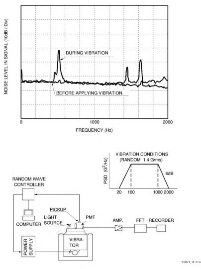
Figure 13-11: Resonance noise in the output signal of a photomultiplier tube subjected to vibration
