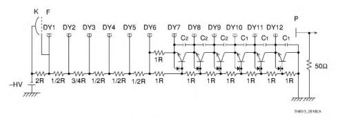
Figure 5-15: Voltage-divider circuit using transistors
