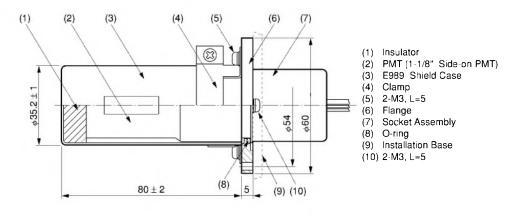
[Flange Fastening Positions to Installation Base]
