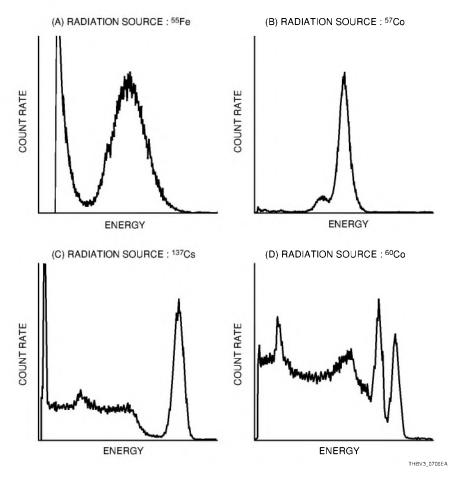
Figure 7-6: Typical pulse height distributions
