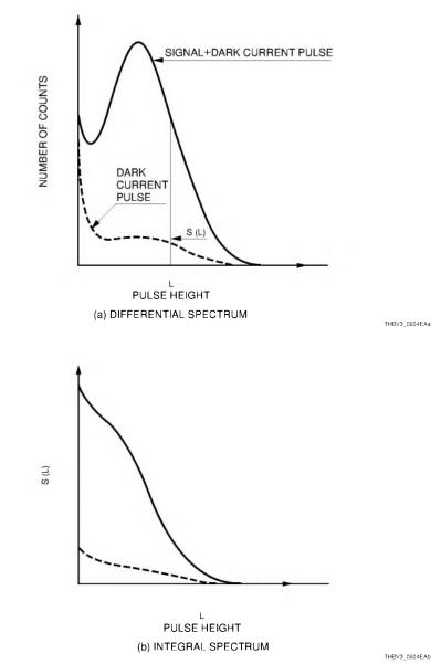
Figure 6-4: Differential and integral representations of pulse height distribution
