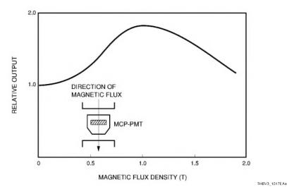
(a) When in magnetic fields parallel to tube axis Figure 10-17: Typical magnetic characteristics of an MCP-PMT (1)
