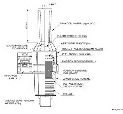
Figure 14-44: X-ray detector (GIS detector) mounted in ASUKA
