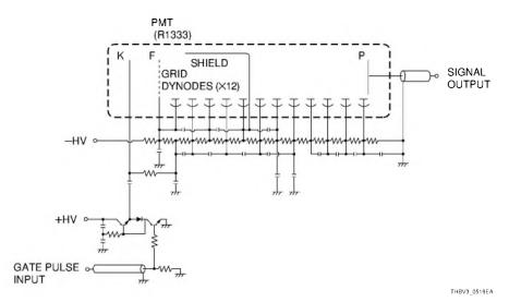
Figure 5-19: Circuit diagram of the C1392 socket assembly with a gating circuit
