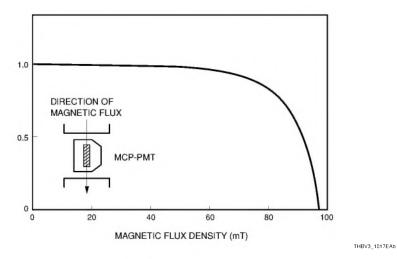
(b) When in magnetic fields perpendicular to tube axis Figure 10-17: Typical magnetic characteristics of an MCP-PMT (2)
