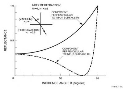
Figure 4-45: Angle dependence of reflectance
