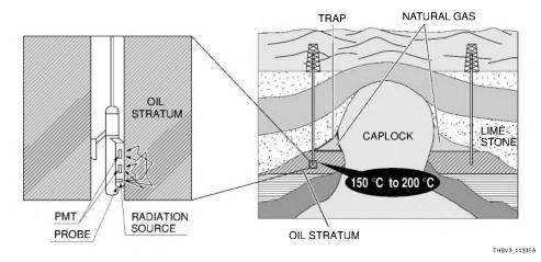
Figure 14-33: Oil well logging using radiation probe and cross sectional view of strata layers
