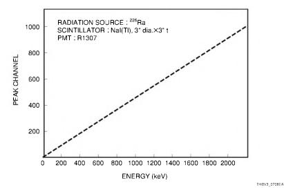
Figure 7-8: Relation between peak channel and gamma-ray energy
