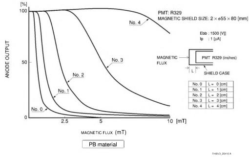
Figure 5-41: Magnetic characteristics of a photomultiplier tube used with magnetic shield case (PB material)
