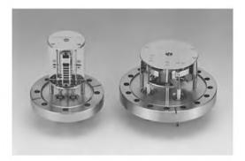
Figure 12-2: Ion detectors with conversion dynode
