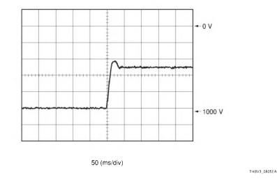
Figure 8-5: Changes in cathode voltage when control voltage is changed from +1.0 V to +0.5 V
