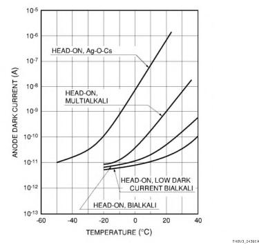
Figure 4-39: Temperature characteristics of anode dark current
