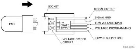
(3) DP-type socket assembly with built-in voltage divider and power supply
