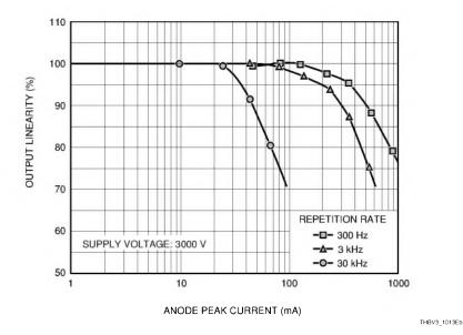
Figure 10-13 (b): Pulse linearity of an MCP-PMT (11 mm effective diameter, 6 mm channel diameter)
