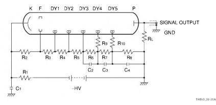
Figure 5-12: Voltage-divider circuit with countermeasure against pulse output linearity, ringing and high-voltage power supply noise
