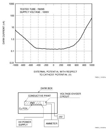
Figure 13-19: Dark current vs. external electric potential
