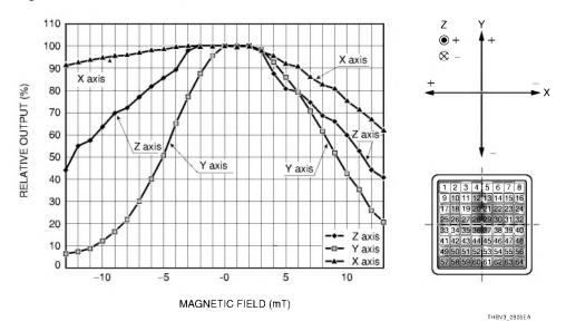
Figure 9-6: Effects of external magnetic fields on anode output (anode channel No. 29)
