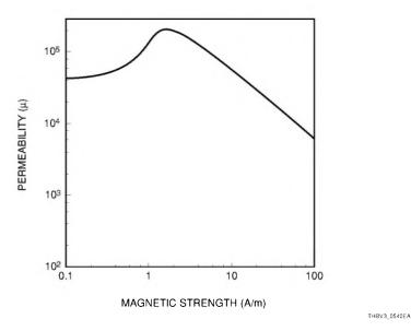
Figure 5-40: Permeability and external magnetic field
