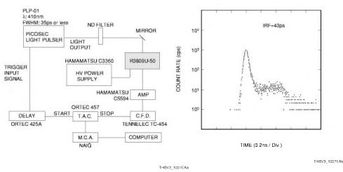
Figure 10-7: IRF measurement using MCP-PMT (R3809U-50)
