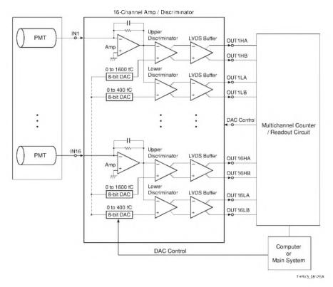
Figure 8-12: Block diagram of photon counting ASIC
