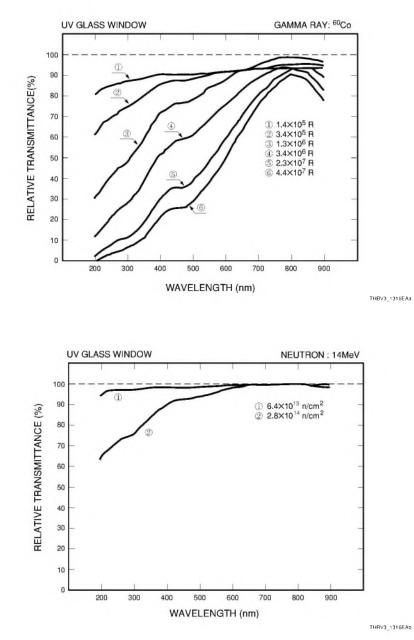
Figure 13-16: Transmittance change of UV glass window irradiated by gamma rays/neutrons
