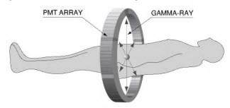
Figure 14-8: Concept view of a PET scanner
