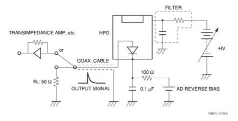
Figure 11-12: DC mode connection example
