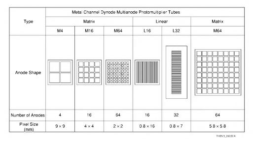
Figure 9-3: Anode patterns for metal channel dynode type multianode photomultiplier tubes
