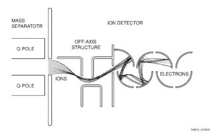
Figure 12-12: Ion detection in an off-axis ion detector
