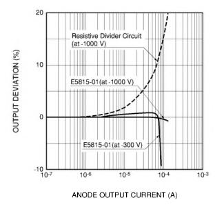
Figure 5-16: Output linearity of a voltage-divider circuit (E5815-01) using transistors
