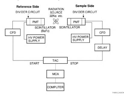
Figure 4-22: Block diagram for CRT measurement
