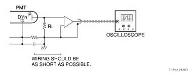
Figure 5-36: Waveform observation using an oscilloscope
