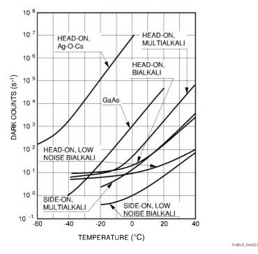
Figure 4-40: Temperature characteristics for dark current pulse
