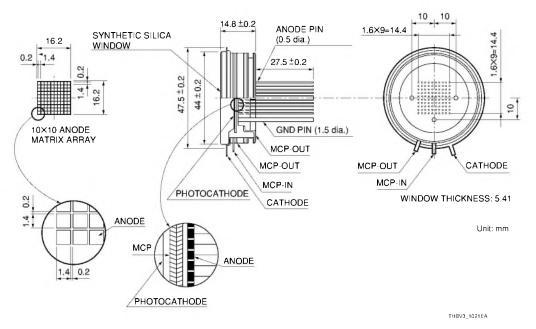
Figure 10-21: Multianode MCP-PMT with 10×10 anode format
