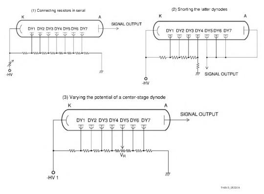
Figure 5-20: Anode sensitivity adjustment circuits
