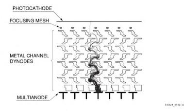
Figure 9-2: Electrode structure and electron trajectories
