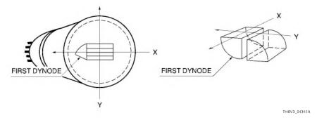
Figure 4-31: Spatial uniformity measurement for head-on types
