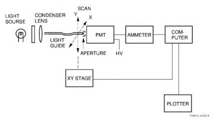
Figure 4-30: Schematic diagram for spatial uniformity measurement
