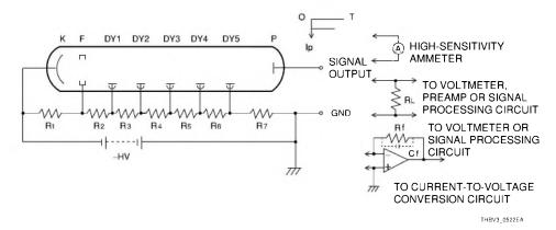
Figure 5-22: Anode grounding scheme in DC operation
