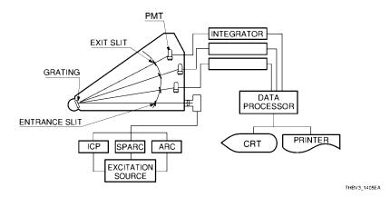
Figure 14-5: Block diagram illustrating a photoelectric emission spectrophotometer
