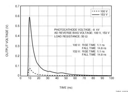
Figure 11-6: Time response waveform
