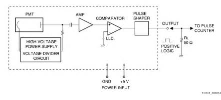
Figure 8-8: Block diagram of photon counting head
