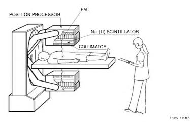
Figure 14-13: External view of a gamma camera
