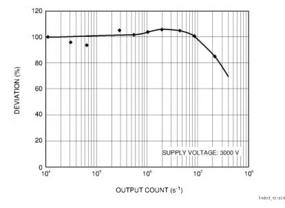
Figure 10-16: Count-rate linearity of an MCP-PMT (11 mm effective diameter, 6 mm channel diameter) in photon counting mode
