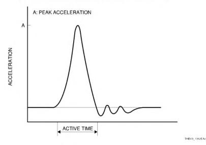
Figure 13-12: Vibration and shock pattern curves (2)
