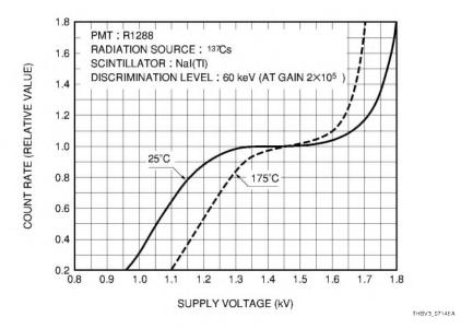
Figure 7-14: Typical plateau characteristics of a high-temperature photomultiplier tube
