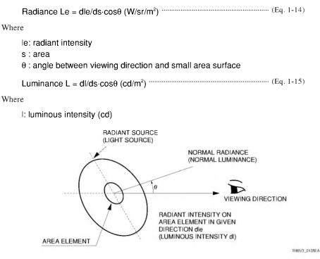
Figure 1-5: Radiant intensity (Luminous intensity)
