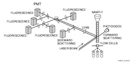
Figure 14-22: Major components of a flow cytometer
