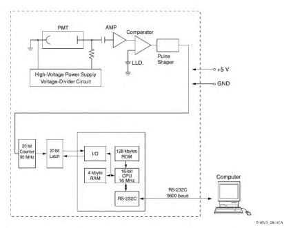
Figure 8-14: Block diagram of photon counting type module
