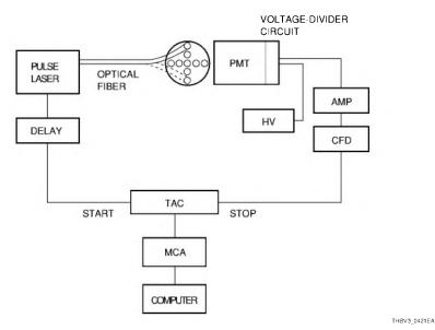
Figure 4-21: Block diagram for CTTD measurement
