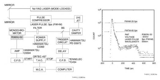
Figure 10-8: Accurate TTS measurement of MCP-PMT (R3809U-50)
