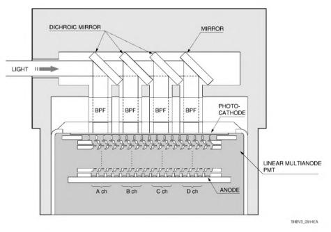
Figure 9-14: Multianode photomultiplier tube assembled with dichroic mirrors
