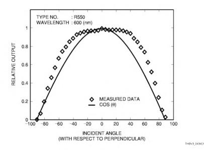
Figure 4-34: Typical angular response
