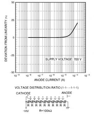
Figure 4-25: DC linearity (side-on type)
