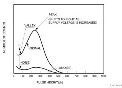
Figure 6-6: Typical example of pulse height distributions
