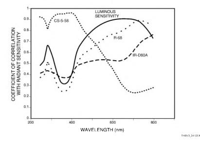
Figure 4-10: Correlation between luminous sensitivities and radiant sensitivity
