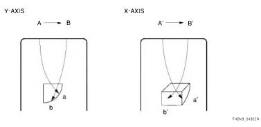
Figure 4-32: Position of photoemission and the related position on the first dynode
