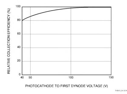
Figure 4-12: Collection efficiency vs. photocathode-to-first dynode voltage
