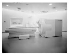
Figure 14-9: [Reference example] External view of a whole-body PET scanner (Hamamatsu Photonics SHR-92000)
