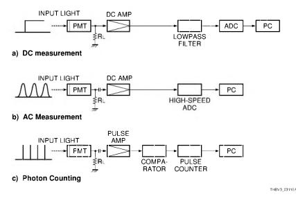
Figure 3-11: Light measurement methods using PMT
