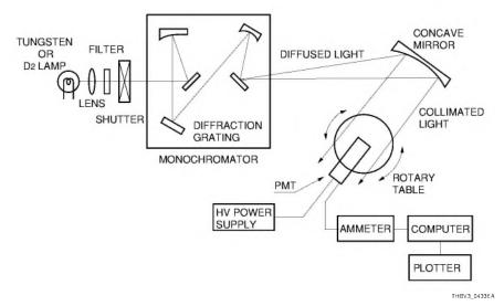
Figure 4-33: Schematic diagram for angular response measurement
