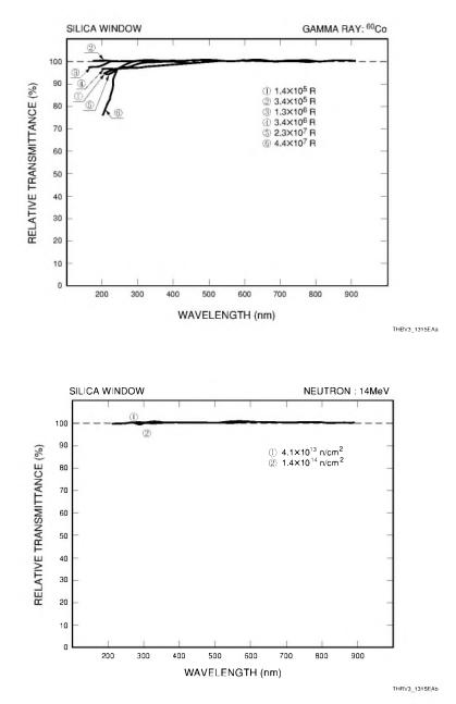
Figure 13-15: Transmittance change of silica window irradiated by gamma rays/neutrons
