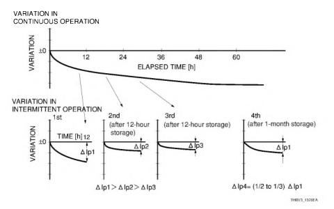
Figure 13-26: Effects of intermittent operation (aging effect)
