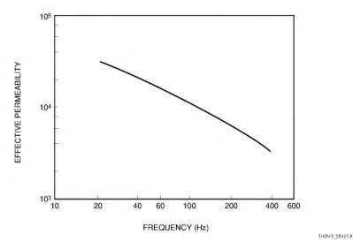
Figure 5-42: Frequency characteristics of a magnetic shield case
