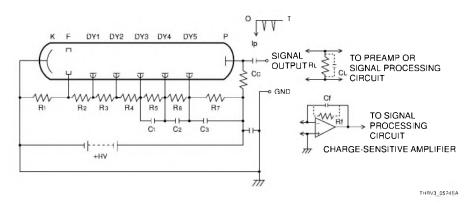
Figure 5-24: Cathode grounding scheme in pulse operation
