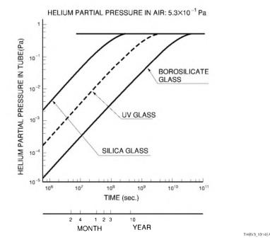
Figure 13-14: Bulb materials and variations in helium partial-pressure inside a tube
