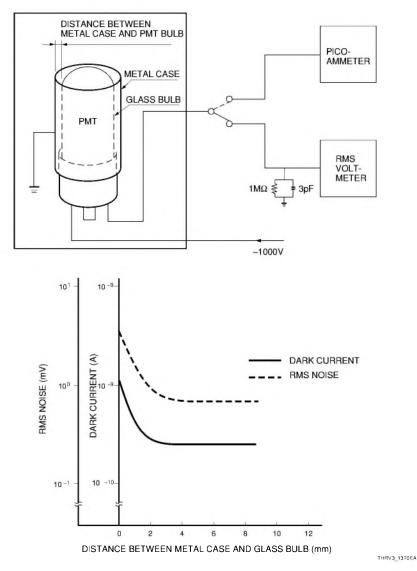
Figure 13-20: Dark current vs. distance to grounded case
