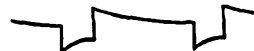
FIG. 8-19.—Typical wave form of condenser current or suppressor voltage for the circuit of Fig. 8-18.
