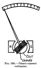
centage of accuracy from an error of the same number of volts at a high position on the scale. For instance, at 20 volts on the scale an error of 2 volts corresponds to a percentage of 10, while an error of 2 volts at a scale reading of 400 volts corresponds to an error of  $\frac{1}{2}$  per cent.
