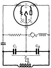
Fig. 417.—Modified Colpitts oscillator circuit.
