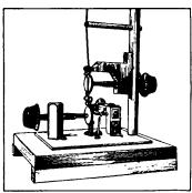
FIG. 120.—Oscillator for 100-centimeter wave lengths.
