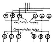
FIG. 475.—Arrangement of commutator tubes and rectifier tubes for grid control in thyratron motor.
