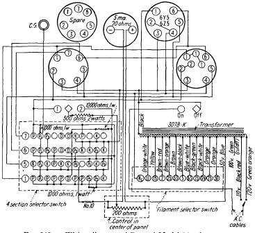
FIG. 242a.-Wiring diagram of Dayrad Model 14 tube tester.
