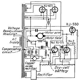
FIG. 461.—Circuit diagram of voltage-controlled rectifier for motor operation.
