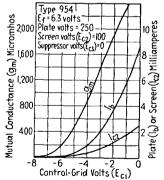
FIG. 133.—Average characteristics of midget pentode tube (type 954).
