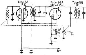
FIG. 406.—Autodyne frequency converter.
