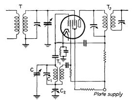
FIG. 410.—Pentagrid-converter tube in oscillator-mixer circuit.
