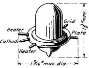
FIG. 122.—Acorn-type triode for use on wave lengths between 0.5 and 5 meters.
