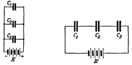
FIG. 25.—Condensers in parallel. FIG. 26.—Condensers in series.
