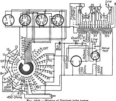
FIG. 242b.—Wiring of Triplett tube tester.
