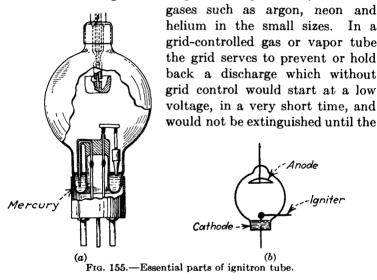
voltage was removed at least temporarily. The ignitron tube combines the overload capacity of the mercury-arc rectifier with the control characteristics of a grid-controlled gas or vapor tube. An additional advantage is that the ignitron as compared with the mercury-arc rectifier has a lower arc loss due to the closer spacing of its electrodes.
