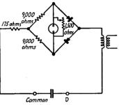
FIG. 207.—Simplified circuit of typical capacity meter.
