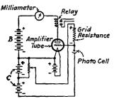
FIG. 381.—Typical direct-current reverse circuit.
