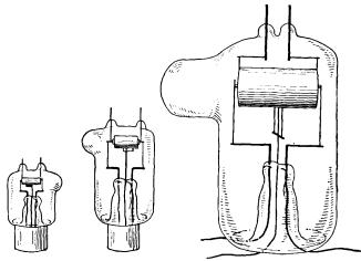
FIG. 426.-Three positive-grid oscillator tubes of spiral-grid type.
