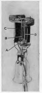
FIG. 66.—Typical dualgrid power amplifier.
