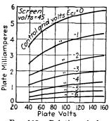
FIG. 118.-Relation of plate current to plate voltage for short-wave tetrode tube.
