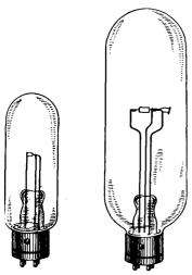
FIG. 476.—Typical arc-oscillator tubes.
