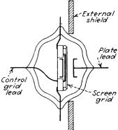
114.-Bulb and shield for midget tetrode tube.
