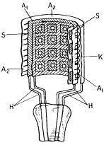
FIG. 166.—Cold-electrode tube with cylindrical electrodes.
