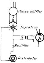
FIG. 474.—Circuit connections of thyratron motor with grid circuit.
