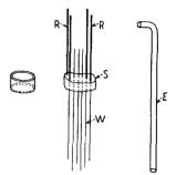
which is in the form of an inverted Fig. 7.—Construction of sup-V is covered with insulation except porting posts and lead-in wires. at the top and the ends. This filament wire fits snugly in
