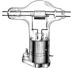
FIG. 423.-Typical positive-grid oscillator tube.
