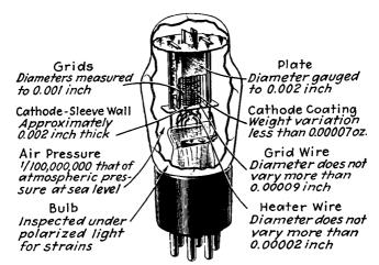
FIG. 4.—Materials used in typical radio receiving tubes.
