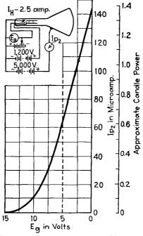
FIG. 441.—Characteristic curve of kinescope.
