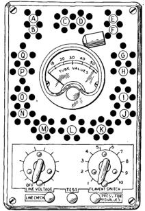
FIG. 237.—Panel of Weston Model 661 tube tester.
