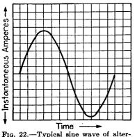
Fig. 22.—Typical sine wave of alternating current.
