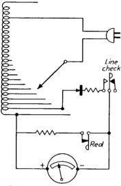
FIG. 239.—Circuit in line-voltage adjustment for Weston Model 661 tube tester.
