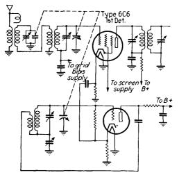
FIG. 407.—Typical all-wave superheterodyne oscillator circuit.
