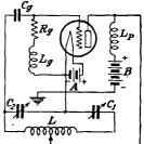
FIG. 405.—Colpitts oscillating circuit arranged for practical operation.
