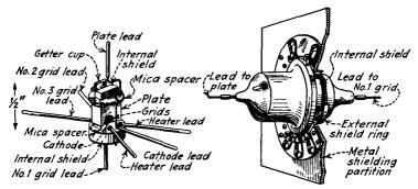
FIG. 129.—Details of construction of Findget pentode tube (type 954).
