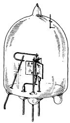
FIG. 421.—Oscillator tube for frequencies up to 740 megacycles per second.
