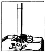
FIG. 121.—Transmitter for 100-centimeter wave lengths.
