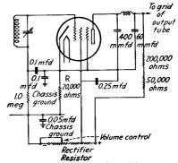
FIG. 285.—Circuit for using type 77 tube with self-biasing resistance as detector.
