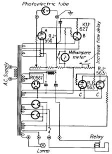
FIG. 451.—Photoelectric controller with time delay.
