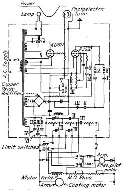
FIG. 462.-Circuit diagram of regulator of paper-coating machine.
