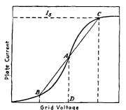
FIG. 404.—Variation of oscillation with grid voltage.
