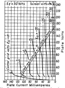
FIG. 339.—Power-output tetrode used as class A amplifier.
