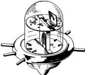
the usual construction is the method of connecting the tube elements to the leads and of using these leads as the base pins. Special directions are given for mounting the tube in order that leakage losses may be kept at a minimum. Connections should be made to FIG. 123.-Midget triode tube (type the terminal leads by means of clips-the heat of solder-
