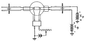
FIG. 424.-Typical positive-grid oscillator circuit.
