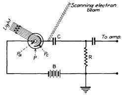
FIG. 429.—Circuit of photoelectric elements in iconoscope.
