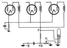
FIG. 367a.-Circuit of visual tuning indicator for amplifier.
