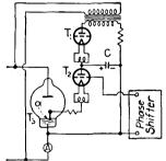
FIG. 467.—Circuit diagram of ignitron used for variablespeed controlled device.
