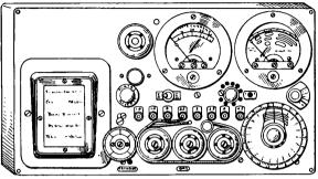
FIG. 232 .--- Panel of Hickok Model AC-47 tube tester.
