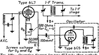
FIG. 108c.—Operating diagram for type 6L7 tube (first method).
