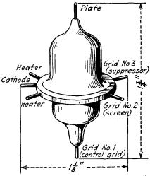
FIG. 128.—Midget pentode tube (type 954).
