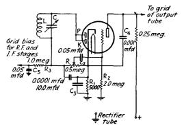
Fig. 262.—Circuit arrangement of duplex-diode-triode type 2A6 or 75 when used as detector-amplifier tube.
