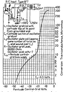
Fig. 104.—Relation between conversion transconductance and control-grid voltage in pentode section of triode-pentode (type 6F7).
