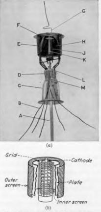
FIG. 59.-Typical variable-mu tube.
