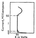
FIG. 159.—Relation of voltage to current of glow lamp as used in small-unit voltage regulation.
