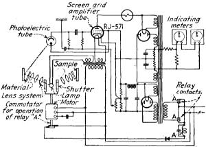
FIG. 455.—Circuit diagram of concentration indicator.
