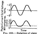
FIG. 269.—Relation of plate current to grid voltage at *B* in Fig. 267.
