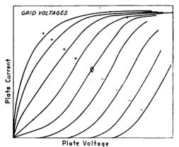
FIG. 47.—Relation of plate current to plate voltage for a series of values of grid voltage.
