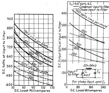
FIG. 301.—Regulation curves of two tubes in a full-wave rectifier with filter.
