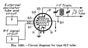
which is connected the output of an external oscillator. The fourth grid, connected within the tube to the second grid, acts as a screen, increasing the plate resistance of the tube, and reducing the capacity between the third grid and the plate. The fifth grid, used as a suppressor, is connected within the tube to the cathode, and serves to limit the effects of secondary emission from the plate.
