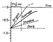
FIG. 430.—Rate of element charging for different degrees of brightness.
