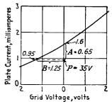
F10. 219.—Amplification factor determined by slope of characteristic curve of tube.
