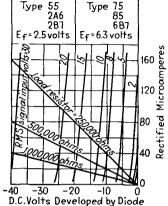
FIG. 84.-Relation of directcurrent voltage to rectified current for single diode unit in halfwave rectification.
