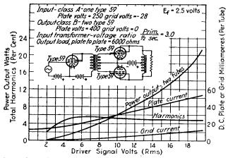
F10. 341.—Operation characteristics of type 59 triple-grid power amplifier tube in class B service.
