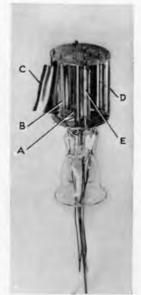
FIG. 90.—Twin triode (complete class B amplifier).
