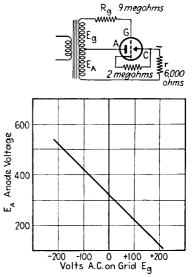
FIG. 135.—Relation of breakdown voltage to grid voltage in gaseous tube (type KU-618).
