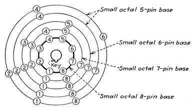
**Bottom View** FIG. 243c.—General pin arrangement for metal tubes.
