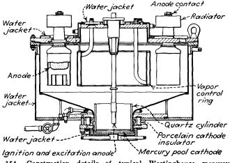
FIG. 154.—Construction details of typical Westinghouse mercury-arc rectifier.
