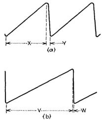
FIG. 443.-Intensity of magnetic fields for unidirectional scanning.
