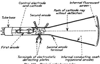
FIG. 183.-Typical cathode-ray tube.
