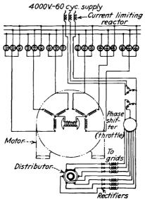
FIG. 473.—Circuit connections of thyratron motor with grid circuit omitted.
