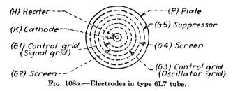
is designed for a remote cut-off characteristic in order that radio-frequency distortion and cross-modulation effects may be minimized when the grid-bias voltage is obtained from an automatic volume-control system. The second grid acts like the screen in a tetrode tube, accelerating the movement of electrons toward the plate, and reducing the capacity between the first and third grids. The third grid, designed to have a sharp cut-off characteristic, is used as a second control grid to
