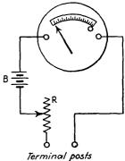
Fig. 199.—Simple ohmmeter.
