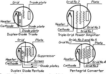
FIG. 65.—Usual representations of multi-electrode and multi-unit tubes.
