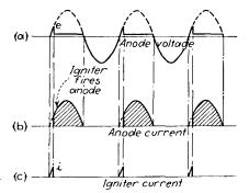
FIG. 314.—Relation of anode voltage to rectified anode current in ignitron rectification circuit in Fig. 313.
