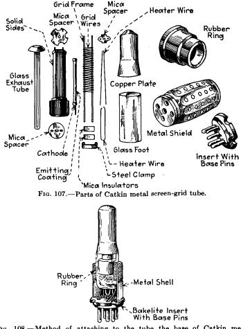
FIG. 108.—Method of attaching to the tube the base of Catkin metal vacuum tube.
