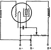
FIG. 253.—Volume-control arrangement using screen-grid voltage variation.
