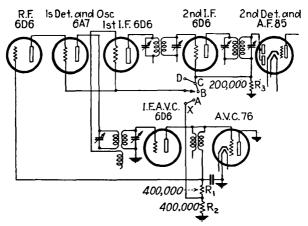
FIG. 356.—Circuit for double-automatic-volume control.
