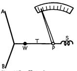
alternating current. As shown in Fig. 197, the resistance wire fastened between points A and B will stretch when it is heated by the passage of an electric current. The change in length of the wire is taken up by the spring S and causes a movement of the pointer. The position of the pointer may be adjusted by a regulating screw.
