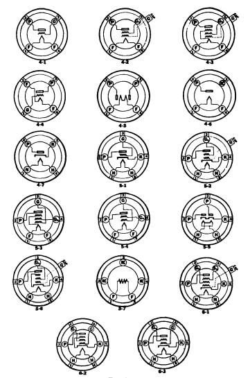
FIG. 243a. FIGS. 243a and b.—Diagrams of typical tube bases (viewed from bottom of base).
