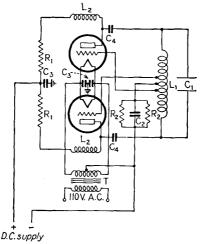
FIG. 415.—Oscillating push-pull circuit for three-electrode tubes.
