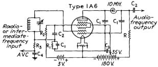
F16. 97.—Circuit of diode tetrode for half-wave detection, automatic volume control, and fixed grid-biased audio-frequency amplification.
