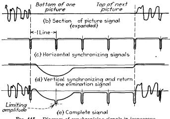
FIG. 445.—Diagram of synchronizing signals in iconoscope.
