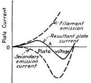
FIG. 186.—Relation of plate current to plate voltage in typical dynatron connection for three-element tube.
