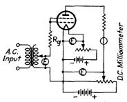
FIG. 217.—Power-output test of tetrode for class B operation.
