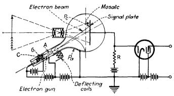
FIG. 428.—Iconoscope circuit.
