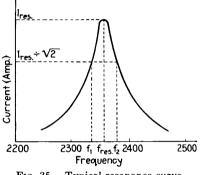
FIG. 35.—Typical resonance curve.
