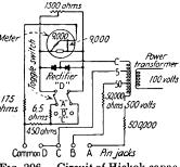
FIG. 206.-Circuit of Hickok capacity meter.
