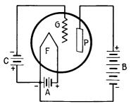
FIG. 44.—Conventional representation of three-element tube.
