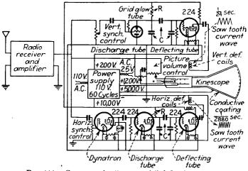
FIG. 444.—Generator for "saw-tooth" deflection current.
