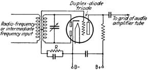
FIG. 260.—Full-wave rectification with duplex-diode triode.
