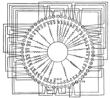
FIG. 229.—Filament circuit of "Confidence" No. 6 tube tester.
