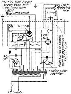
FIG. 450.—Lock-in type photoelectric controller with amplifier tube.
