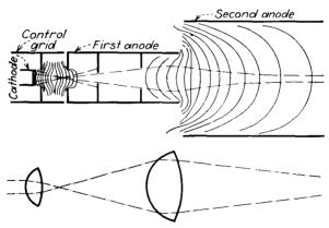
Approx. Optical Analogy FIG. 436.—Distribution of electrostatic fields in electron gun.
