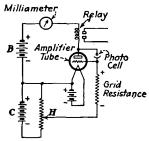
FIG. 378.—Typical directcurrent forward circuit. are for the operation of relays.
