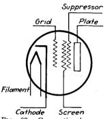
FIG. 63.—Conventional representation of pentode.
