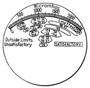
234.--Mutual conductance meter in Hickok Model AC-47 tube tester.
