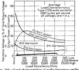
FIG. 210.—Load characteristics of audio-frequency oscillator.
