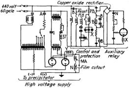
FIG. 458.—Circuit diagram of precipitation apparatus.
