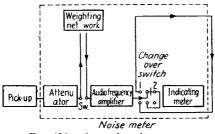
FIG. 482.—Acoustic noise meter.
