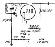
Fig. 282.—Application of screengrid tube type 32 as detector in Spartan model 81A receiver.
