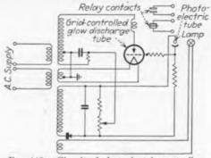
FIG. 448.-Circuit of photoelectric controller.
