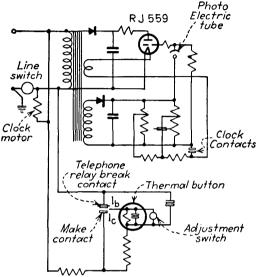
FIG. 452.--Circuit diagram for lighting control.
