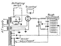
FIG. 457.—Circuit diagram of electronic timer.
