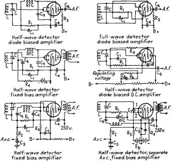
FIG. 83.-Typical duplex-diode triode in circuits (types 85 or 55).
