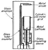
FIG. 169.—Reich and Hesselberth's cold-electrode glow-discharge tube.
