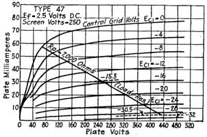
FIG. 64.—Average plate characteristics of type 47 power-output pentode.
