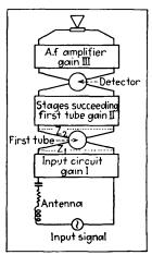
FIG. 394.—Diagrammatic representation of typical radio receiver.
