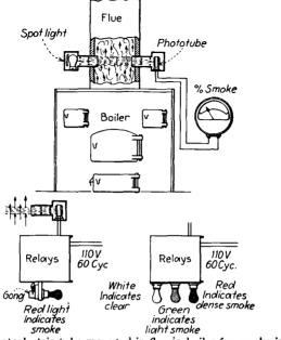
FIG. 468.—Photoelectric tube mounted in flue in boiler for smoke indication.
