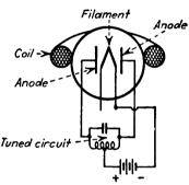
FIG. 189.—Magnetron for generation of high-frequency power. increases to a maximum.
