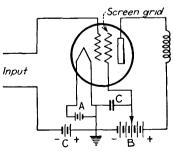
FIG. 54.—Connection of electrodes of screen-grid tube.
