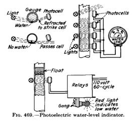
beam and one photoelectric cell are sufficient. In another alarm arrangement a float is used which blocks the light beam when a certain water level is reached in the gage glass, and thus causes a relay to ring a bell or to turn on a red light.
