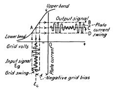
FIG. 325.—Static characteristic curve of simple amplifier.
