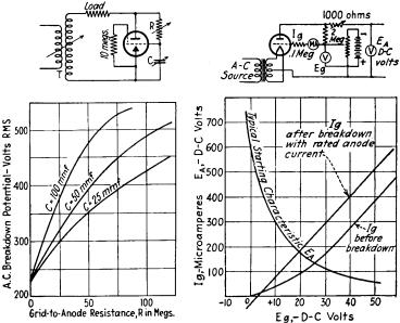
FIG. 136.—Relation of breakdown voltage to anode-to-grid resistance of gaseous tube (type KU-618).
