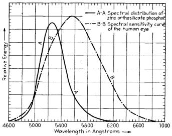
F1G. 442.—Relative energy over light band of (A) iconoscope, (B) human eye.
