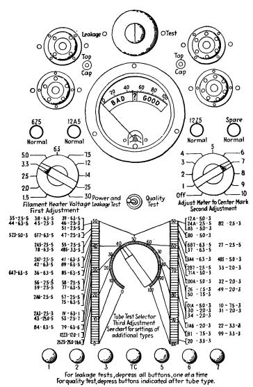
FIG. 230.—Panel of "Supreme" Model 85 tube tester.
