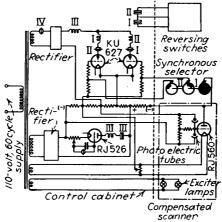
FIG. 463a.—Circuit diagram of regulator with compensated scanner.
