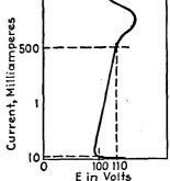
FIG. 160.—Relation of voltage to current in glow lamp in largeunit voltage regulation.
