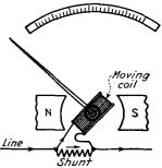
ranges by the use of a number of FIG. 194.—Direct-current amdifferent shunts each to be conmeter with shunt connection.
