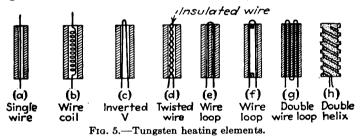
which a reversed coil winding is baked in the insulator or threaded into it is intended not only to reduce the electromagnetic field responsible for the production of hum but also to reduce the heating time by placing the heater wire nearer to the cathode sleeve. The insulator also appears in various forms, such as the solid single-hole type, the solid double-hole type, and the perforated type; the materials used include porcelain, magnesia compounds, and alumina compounds.
