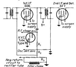
FIG. 358.—Retroactive circuit for automatic volume control.
