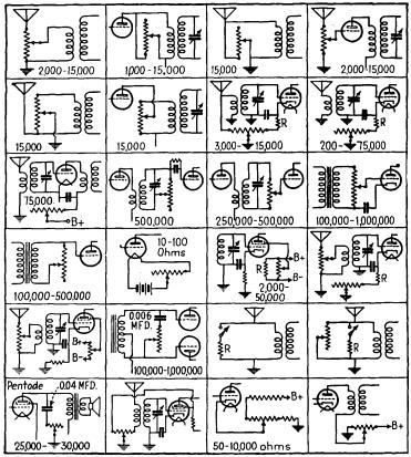
FIG. 349.—Typical volume-control arrangements.
