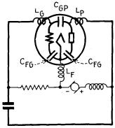
FIG. 418.—Limiting circuit of Colpitts oscillator.
