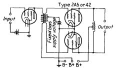
FIG. 247.-Fixed grid-bias arrangement using battery-supply current.
