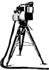
FIG. 437.—Portable iconoscope camera and pick-up equipment.
