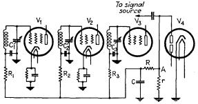
FIG. 355.—Automatic-volume-control circuit with filters.
