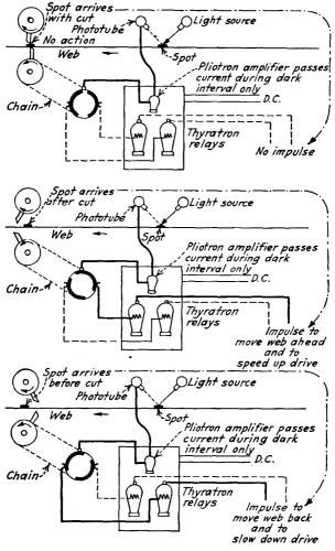
FIG. 463b.—Arrangement of apparatus for register control.
