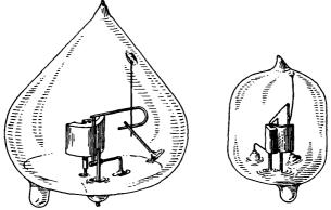
Smaller one will oscillate at FIG. 422.-Experimental oscillator designs. 1200 megacycles per second.
