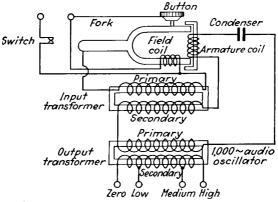
FIG. 209.—Circuit of audio-frequency oscillator.
