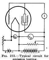
its value cannot be measured because if the current is increased to its maximum the tube may be damaged and the emitting conditions may be changed. Consequently a test of emission is made at a lower voltage which will not injure the tube. Comparisons of tests are valueless if the operating conditions are not alike.
