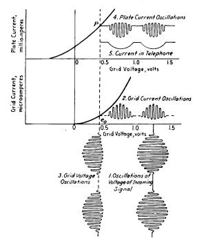
FIG. 274.—Use of detector tube with grid condenser on modulated continuous oscillations.
