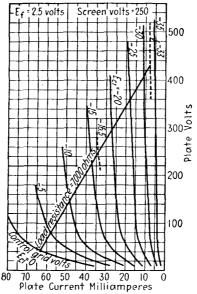
FIG. 340.—Power-output pentode used as class A amplifier.
