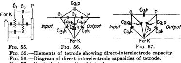
FIG. 57.—Equivalent capacity of tetrode.
