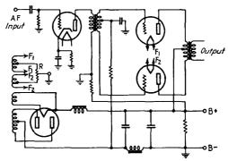
FIG. 250.—Circuit for semi-fixed grid-bias method.
