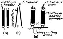
FIG. 10.—Construction of cathode heaters.
