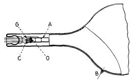
FIG. 434.—Electron gun of iconoscope.
