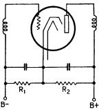
FIG. 245.—Circuit for providing a combination of variable and fixed grid-bias voltage.
