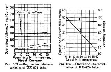
electrical equipment from a surge of high voltage in the supply circuit. It is used also in connection with a rectifier unit (page 361) to maintain a constant direct-current output for varying load currents. In this application the tube maintains an approximately constant direct-current voltage of 90 volts for a current change of 10 to 50 milliamperes.
