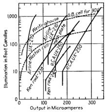
FIG. 180.—Photoelectric response for various tubes (floating grid).
