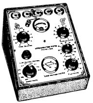
FIG. 224.—Panel view of Model 304 tube tester.
