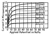
FIG. 176.—Relation of current and applied voltage at different light intensities for high-vaccum photoelectric tube (SR-50).
