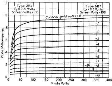
FIG. 88.—Average characteristics of duplex-diode pentode (type 6B7).
