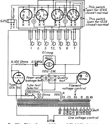
FIG. 231.—Wiring diagram of "Supreme" Model 85 tube tester.
