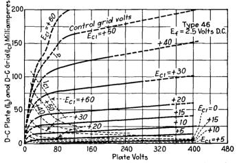
FIG. 68.—Average plate characteristics of type 46 tube used as class B amplifier.
