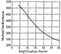
FIG. 50.—Relation of mutual conductance to amplification factor.
