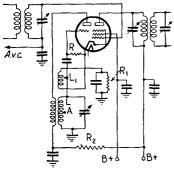
FIG. 408.—Triode-pentode tube in oscillator-mixer circuit.
