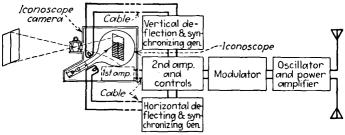
FIG. 438.—Iconoscope transmitting equipment.
