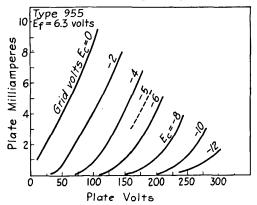
FIG. 127.—Relation of plate current to plate voltage in midget triode (type 955).
