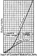
FIG. 395.—Relation of audiofrequency output voltage to applied signal input voltage at constant modulation.
