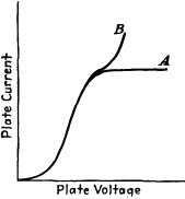
FIG. 16.—Curve showing relation between plate current and plate voltage with and without gas ionization,
