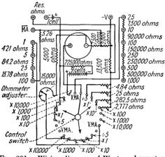
F1G. 201.—Wiring diagram of Weston ohmmeter.
