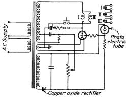
FIG. 454.—Circuit diagram for heater control.
