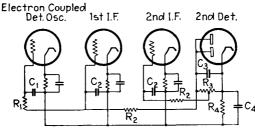
FIG. 361.—Circuit providing grid-bias voltage for automatic volume control on intermediate-frequency stages.
