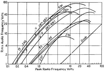
FIG. 275.—Average performance of typical detector tubes.
