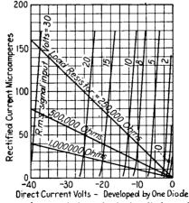
FIG. 261.—Average characteristics of single diode unit for half-wave rectification.
