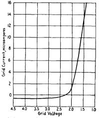
FIG. 280.—Characteristic curve showing best point of operation of UX-200A tube.
