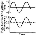
FIG. 268.—Relation of plate current to grid voltage at A in Fig. 267.
