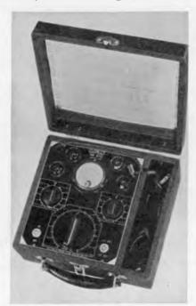
FIG. 241.-Panel of Dayrad Model 14 tube tester.
