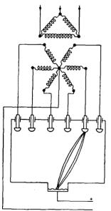
FIG. 319.—Simple method of connecting mercury-arc rectifier to transformer.
