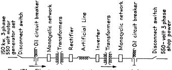
Fig. 471.-Direct-current constant-current transmission system.
