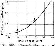
FIG. 267.—Characteristic curve typical triode vacuum tube.
