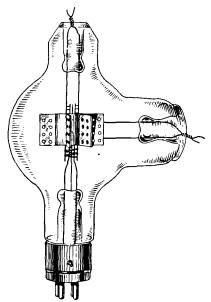
FIG. 419.-Typical air-cooled high-frequency oscillator.
