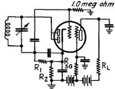
FIG. 279.—Typical detection circuit for duplex-diode high-mu triode tubes.
