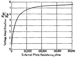
FIG. 344.—Theoretical relation of load resistance to voltage amplification in typical radio receiving tube.
