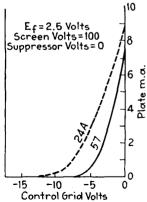
FIG. 74.—Relation of plate current to control-grid voltage (types 24 and 57).
