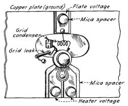
FIG. 124.—Typical mounting assembly for midget triode (type 955).
