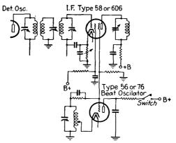
FIG. 413.—Beat-frequency oscillator circuit.
