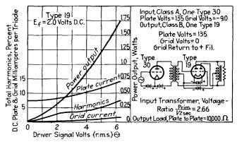
FIG. 91.—Circuit and performance characteristics of type of twin triode used as class B power amplifier (type 19).
