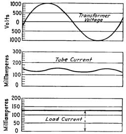
FIG. 298.—Oscillograph record of UX-280 tube with choke-input type of filter.
