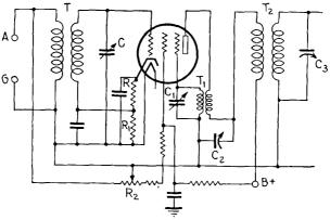
FIG. 409.—Triple-grid tube in oscillator-mixer circuit.
