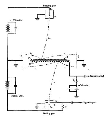
Fig. 15. Signal-converter storage tube (Graphechon). A, accelerating anodes; C, writing-gun control grid; G, collector;  $i_C$ , collected current;  $i_{pr}$ , primary current;  $K_r$ , reading-gun cathode;  $K_w$ , writing-gun cathode; M, target-supporting mesh; P, backplate (aluminum foil);  $R_i$ , input resistor;  $R_0$ , output resistor; T, insulating target.
