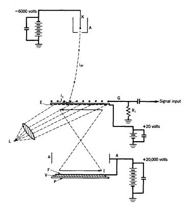
Fig. 23. Photoelectric viewing storage tube (Schroeter).
