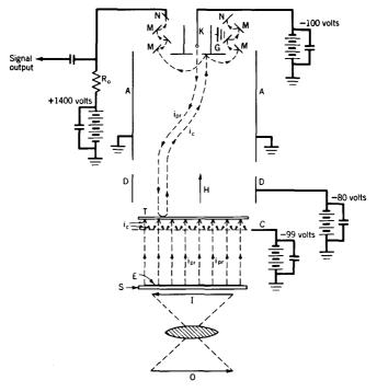
Fig. 32. Television-camera storage tube (Image Orthicon).
