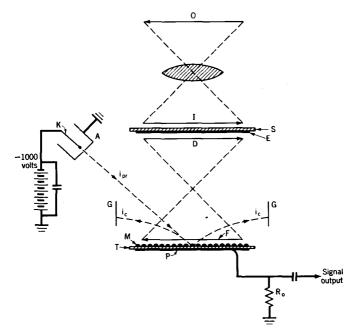
Fig. 31. Television-camera storage tube (Image Iconoscope).
