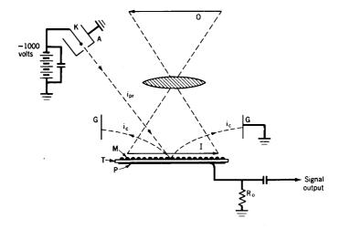
Fig. 28. Television-camera storage tube (Iconoscope).
