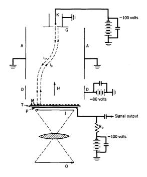
Fig. 29. Television-camera storage tube (Orthicon).
