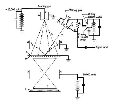
Fig. 20. Viewing storage tube (Knoll and Randmer). A, accelerating anodes; C, control grid; G, collector cylinder; I, image of secondary currents;  $i_{C}$ , secondary current;  $i_{pr}$ , primary current;  $K_{r}$ , reading-gun cathode;  $K_{w}$ , writing-gun cathode; M, insulating mosaic; P, target foil;  $R_{i}$ , input resistor; V, viewing phosphor.
