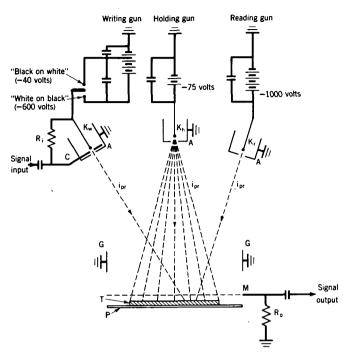
Fig. 16. Signal-converter storage tube (Memory Tube). A, accelerating anodes; C, writing-gun control grid; G, collector cylinder;  $i_{pr}$ , primary current;  $K_h$ , holding-gun cathode;  $K_r$ , reading-gun cathode;  $K_w$ , writing-gun cathode; M, collector grid; P, transparent supporting insulator;  $R_i$ , input resistor;  $R_o$ , output resistor; T, insulating target (phosphor if used for visual output).
