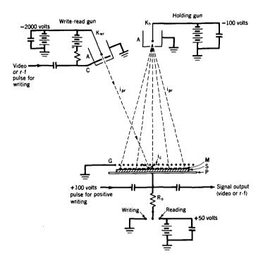
Fig. 27. Computer storage tube (Dodd, Klemperer, and Youtz).
