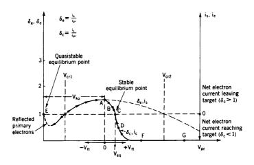
Fig. 6. Curve of instantaneous collected current as a function of floating target potential  $V_{ft}$  showing equilibrium points C and E.  $V_{ft}$ , floating-target potential with respect to collector.  $V_{ft}=0$  represents target potential equal to collector potential.
