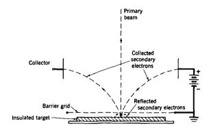
Fig. 8b. Barrier grid for reducing electron redistribution.
