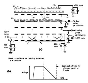
Fig. 26. Computer storage tube (Rajchman). (a), electrode system; (b), pulse applied to writing plate.
