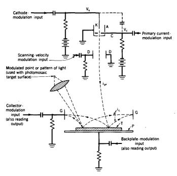
Fig. 9. Methods of applying input signals to a storage tube. A, accelerating anode; C, control grid; D, deflection plates; G, collector;  $i_{\rm C}$ , collected current;  $i_{\rm pr}$ , primary current; K, cathode; P, backplate; T, target;  $V_{\rm C}$ , control-grid bias voltage;  $V_{\rm k}$ , cathode bias voltage.
