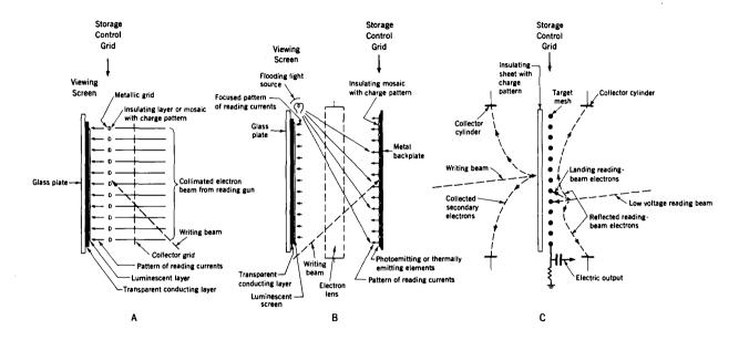
Fig. 12. Grid-control reading systems.
