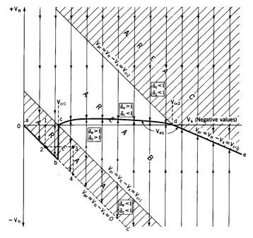
Fig. 4. Potential shift of a floating target under electron bombardment as a function of its initial potential  $V_{ft}$  and the cathode voltage  $V_k$ .  $V_{ft}$ , instantaneous potential of target surface;  $V_{eq}$ , particular value of  $V_{ft}$  at equilibrium potential of target surface;  $V_k$ , cathode potential of bombarding primary beam.
