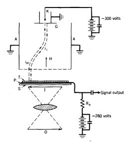
Fig. 30. Television-camera storage tube (Vidicon).
