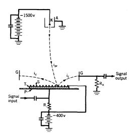
Fig. 18. Signal-converter storage tube (Radechon).
