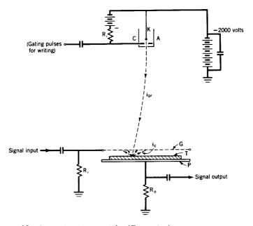
Fig. 25. Computer storage tube (Forrester).
