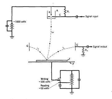
Fig. 13. Signal-converter storage tube (Krawinkel, Kronjäger, and Salow).
