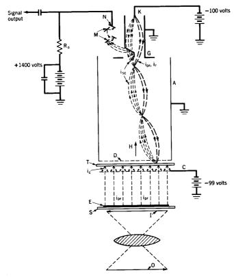
Fig. 33. Television-camera storage tube (Image Isocon).
