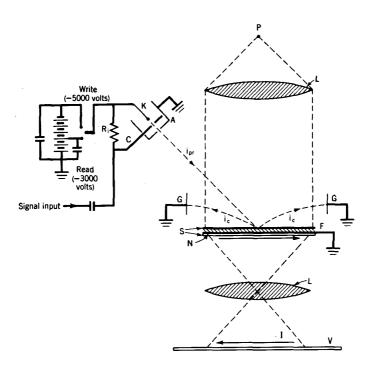
Fig. 21. Light-valve viewing storage tube (Donal and Langmuir).
