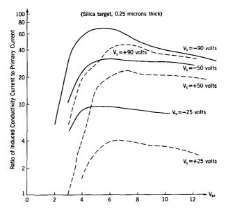
Fig. 7. Typical curves showing change in bombardment-induced conductivity with primary beam energy  $V_{pr}$ .  $V_{pr}$ , primary beam energy in kilovolts;  $V_{s}$ , potential of target surface with respect to backplate (Pensak, Ref. 17).
