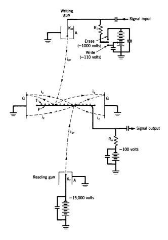
Fig. 17. Signal-converter storage tube (Knoll and Randmer). A, accelerating anodes; G, collector;  $i_{pr}$ , primary current;  $i_{c}$ , collected current;  $K_{r}$ , reading-gun cathode;  $K_{w}$ , writing-gun cathode; P, backplate (aluminum foil);  $R_{i}$ , input resistor;  $R_{o}$ , output resistor; T, insulating mosaic.
