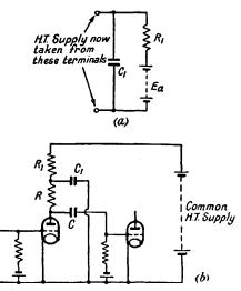
FIG. 44. ANODE-CIRCUIT DECOUPLING
