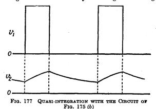
when fed with input voltages having a waveform which includes a flat horizontal portion.
