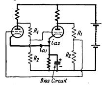
FIG. 117. RESISTANCE-COUPLED KIPP RELAY
