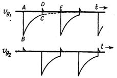
FIG. 114. MULTIVIBRATOR WAVEFORMS
