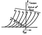
FIG. 129. DYNAMIC-CHARACTERISTICS OF DIODE
