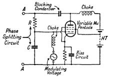
FIG. 165. REACTANCE-VALVE CIRCUIT
