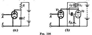
(a) Production of triangular pulses(b) Triggered blocking-oscillator
