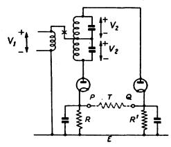
FIG. 151. PRINCIPLE OF THE FOSTER-SEELEY DISORIMINATOR
