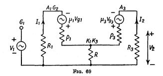
180°. Thus we may draw the equivalent circuit as in Fig. 69, omitting the second stage, but taking the alternating input voltage to the third stage as  $\left(-\frac{\mu_2 R_3}{\rho_2 + R_2}\right) \times V_{a_1}$  or  $-(VA)_2 V_{a_1}$ . Since  $V_a$  is equal to  $-R_1 I_1$  this gives  $V_{\sigma_3} = (VA)_2 R_1 I_1 - R(I_1 + I_2)$ Also  $V_{\sigma_1} = V_1 - R(I_1 + I_2)$
