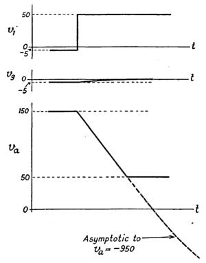
FIG. 217. WAVEFORMS OCCURRING IN FIG. 216
