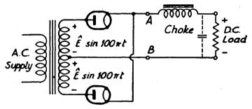
FIG. 142. SERIES-CHOKE FULL-WAVE RECTIFIER
