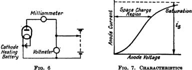
Note. The cathode heating battery is often omitted from circuit diagrams
