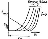
FIG. 136. RECTIFICATION CHARACTERISTICS OF ANODE-BEND DETECTOR
