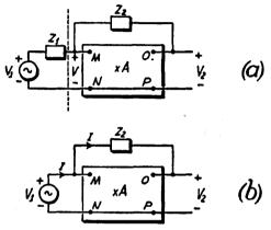
FIG. 75. SHUNT-CONNECTED FEEDBACK
