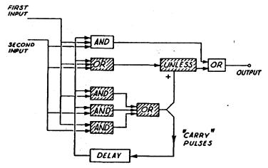
FIG. 230, BINABY ADDING CIRCUIT
