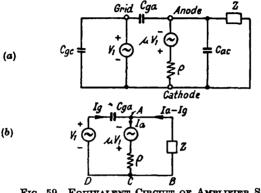
FIG. 59. EQUIVALENT CIRCUIT OF AMPLIFIEB SHOWING INTER-ELECTRODE CAPACITANCES
