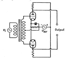
FIG. 149. PHASE-SENSITIVE DETECTOR
