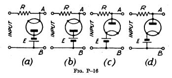
**VIII.12.** How would the answers to the previous question be changed if R = 9 K, the output resistance of the source were 10 K, and the resistance of the diode when conducting were 1 K?
