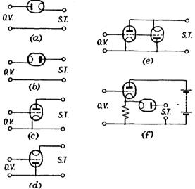
FIG. 196. ELECTRONIC SWITCH CIRCUITS (All are unidirectional switches except (e) which is bi-directional) O.V. = Operating Voltage S.T. = Switch Terminals
