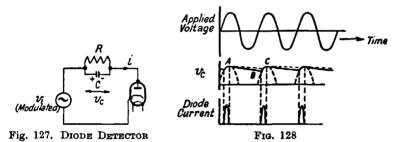
of a high resistance across the condenser, making the circuit as shown in Fig. 127, provides such a path, and the circuit is then that of a diode detector.
