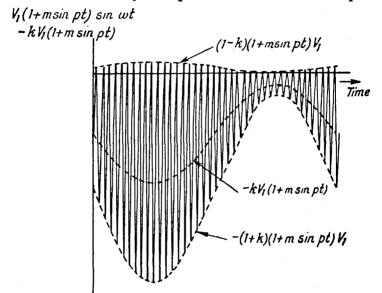
FIG. 135. RESULTANT GRID-VOLTAGE OF CUMULATIVE-GRID DETECTOR WITH MODULATED INPUT
