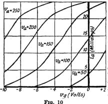
it is convenient to express the characteristics in one form  $(i_a/v_a)$  for various fixed values of  $v_{a}$ ) and for other purposes in the other form  $(i_a/v_a$  for various fixed values of  $v_{\sigma}$ ). The two forms are sometimes referred to as the "Anode-characteristics" (Fig. 11) and the "Mutual-characteristics" (Fig. 10). See also page 358.
