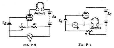
**\*III.39.** Fig. P-7 shows a circuit which is used for the direct measurement of the mutual conductance,  $g_m$ , of a valve. V represents an audio-frequency e.m.f. and R a calibrated variable resistance. The procedure is to adjust R until no sound is heard in the high-resistance headphones (which indicates that the alternating component of the anode-voltage is zero).
