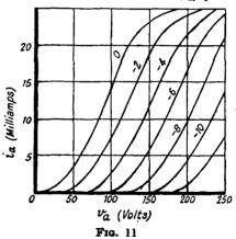
The figure attached to each curve indicates the value of  $v_{\sigma}$  for which it applies
