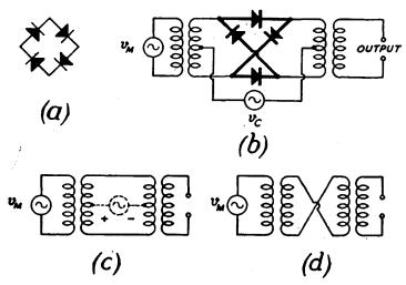
FIG. 158. THE RING MODULATOR
