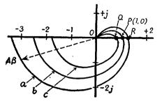
its own input voltage. It is shown in Chapter V (page 154) that under these conditions the "amplifier" will generate oscillations whose amplitude increases with time, the amplitude eventually reaching equilibrium at a value which makes the valve parameters such that the magnitude of  $A\beta$  is reduced exactly to unity.
