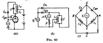
which will be balanced if  $C_n/C_{ga}$  equals  $L_1/L_2$ . When this condition obtains the anode generator can send no current through the grid circuit (denoted in our bridge by the generator  $V_1$ ). Thus the feedback from anode circuit to grid circuit is prevented.
