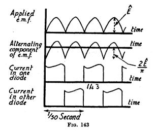
this half-cycle. The p.d. between the points A and B in the circuit of Fig. 142 must therefore be as shown in Fig. 143 and the circuit may be considered as supplying this specified pulsating e.m.f.
