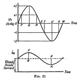
taking the mean of the positive peak, FG, and the negative peak, HK, in Fig. 21,
