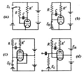
FIG. 218. INITIATING THE RUN-DOWN IN A MILLER Sweep Generator
