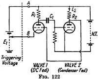
condenser voltage reaches a certain value the first valve shall conduct.
