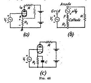
For some purposes it is necessary to have a grid-bias voltage large enough to cut-off the flow of anode-current. Clearly, this cannot be achieved with this circuit since the grid-bias voltage is produced by the flow of anode-current. Cut-off bias can, however, be provided by connecting an additional resistance (shown dotted) between K and h.t. positive.
