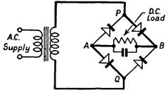
FIG. 144. BRIDGE RECTIFIER
