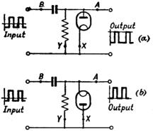
FIG. 208. D.C. RESTORATION CIRCUITS
