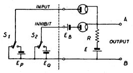
FIG. 229. INHIBITION GATE
