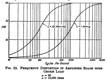
with choke coils of inductance 10 henrys and 1 henry. From equation (III.10) it is easy to show that the cut-off frequency, defined as the frequency at which the gain is 3 decibels below the asymptotic value, is given by  $f_c = \rho/2\pi L$ .
