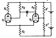
FIG. 119. CATHODE-COUPLED FLIP-FLOP
