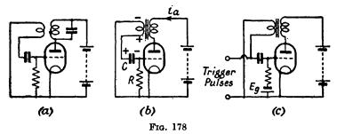
(a) Orthodox tuned-anode mutual-coupled oscillator
