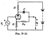
(a) What is the phase-relationship between the output-voltage (potential of anode above h.t. negative) and the input-voltage (potential of cathode above h.t. negative)?
