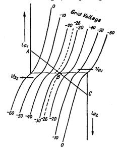
FIG. 88. COMPOSITE CHARACTERISTICS FOR CLASS B STAGE (Incorrect Bias-voltage)
