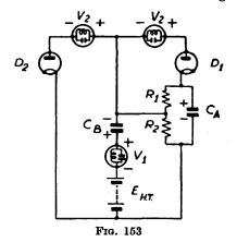
conducting direction of the diode. Applying this rule to the lefthand closed circuit (formed of  $D_2$ ,  $V_2$ ,  $C_B$ ,  $V_1$  and  $E_{HT}$ ) we see that  $v_{C_B} = E_{HT} + |V_1 - V_2|$
