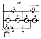
FIG. 146. VOLTAGE-QUADRUPLING RECTIFIER
