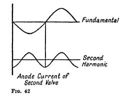
of the resultant anode-current (viz. the sum of fundamental and second harmonic) should have a larger positive excursion than negative excursion. This criterion applies equally to the two valves, since the effect of curved characteristics upon the waveform will be the same for both valves. The anode-current of the second valve is, therefore, given by
