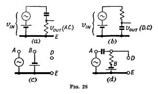
used is essentially that of paragraph (b) above, and the design rule is  $R > 1/\omega C$  as enunciated for the a.c./d.c. separating circuit. This is an important method of applying grid-bias voltage, whether fixed or derived from an A.G.C. circuit.
