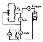
FIG. 130. CIRCUIT FOR MEASURING DYNAMIC-CHARACTERISTICS
