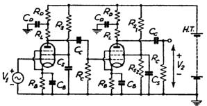
FIG. 48. TWO-STAGE PENTODE AMPLIFIER
