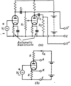
FIG. 49. PHASE INVERTERS (Push-pull input circuits)
