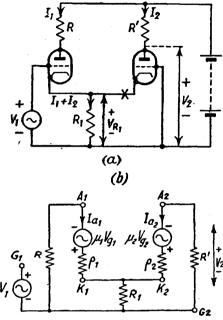
FIG. 51. CATHODE COUPLING
