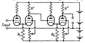
FIG. 52. LONG-TAILED PAIRS IN & D.C. AMPLIFIER
