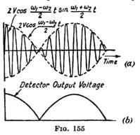
where  $V_1$  and  $V_2$  are respectively the peak values of the signal voltage and oscillator voltage. To determine the exact shape of the envelope we must revert to mathematical treatment and proceed to find the equation of the envelope, i.e. the equation of the curve passing through the maxima and minima of the sum curve,
