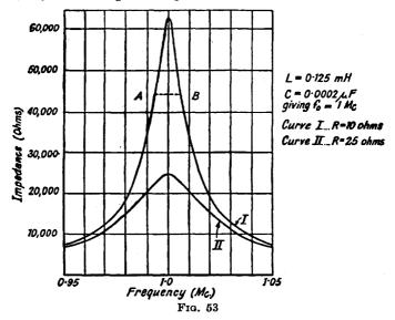
$\omega_0/2\delta\omega$  where  $\delta\omega$  is the change of  $\omega$  required to reduce the amplification from  $|(VA)|_{max}$  to  $|(VA)|_{max}/\sqrt{2}$ . In view of the use of the factor  $1/\sqrt{2}$ , the range of frequency corresponding to  $2\delta\omega$  is often called "the 3 decibel bandwidth" of the amplifier, and we may write—
