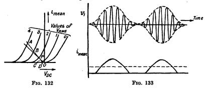
for modulation depths less than a certain value, this value becoming smaller as the difference between the slopes of the two lines increases.
