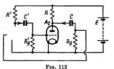
C. This condenser C is connected, in series with the resistor  $R_o$ , directly between  $A_2$  and h.t. negative. As a result of the landslide an increased current is now flowing through R and hence the p.d. between  $A_2$  and h.t. negative has been reduced. The condenser C must therefore discharge, the discharge current flowing in the direc-
