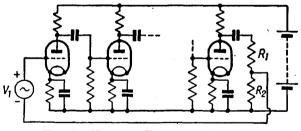
FIG. 64. NEGATIVE FEED-BACK AMPLIFIER WITH AN ODD NUMBER OF STAGES
