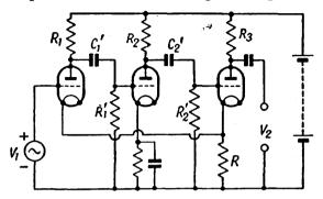
FIG. 68 NEGATIVE FEED-BACK AMPLIFIER WITH AN ODD NUMBER OF STAGES (Permitting earthing of one input terminal)
