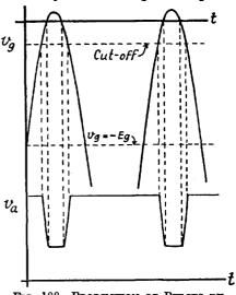
FIG. 188. PRODUCTION OF PULSES BY SHAPING OF SINE WAVE
