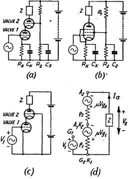
FIG. 61. THE CASCODE CIRCUIT
