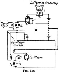
alternating electrical quantities of nearly equal frequency—the envelope of the sum curve having the difference frequency.
