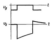
pulse-sides to differ from the shape of the input-pulse sides. Amplifiers in which the anode-current is cut off by the negative excursion of the input
