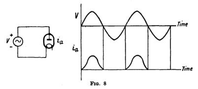
of unidirectional current from alternating current is known as Rectification.
