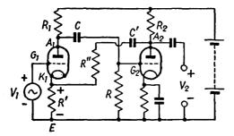
FIG. 65. NEGATIVE FEED-BACK AMPLIFIER WITH EVEN NUMBER OF STAGES
