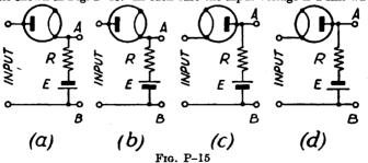
peak amplitude 100 v, E is 60 v, and R is very large compared to the internal impedance of the a.c. source supplying the input terminals. The diode may be considered to have negligible resistance when conducting, and to be non-conducting for negative values of anode-voltage.
