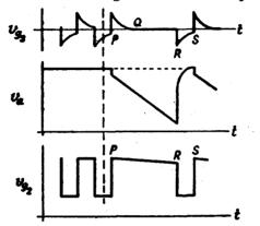
FIG. 225. WAVEFORMS IN SCREEN-COUPLED PHANTASTRON OF FIG. 224 (b)
