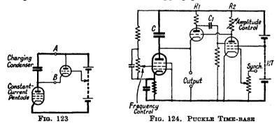
rapidly towards the positive end of  $E_1$ . This causes the anodecurrent of valve 1 to be cut off, which in turn precipitates a return to the stable condition with valve 2 conducting. The whole process of sliding the tapping point down the battery  $E_1$  then recommences.
