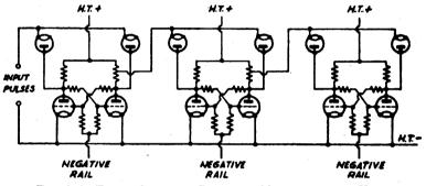
FIG. 226. THREE CASCADED BI-STABLE MULTIVIBRATORS USED AS A BINARY COUNTING CIRCUIT
