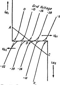
FIG. 90. COMPOSITE CHARACTERISTICS FOR CLASS B STAGE (Correct Bias Voltage)
