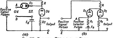
FIG. 199. Two-diode Time-selection Circuit
