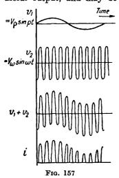
sinusoidal current together with unwanted harmonics of carrier and sidebands. By including in series with the sum voltage and the diode a parallel L-C circuit tuned to the carrier frequency, the desired modulated voltage (being a narrow band of frequencies whose mean value is the carrier frequency) may be separated from the unwanted components, for the parallel L-C circuit has a large impedance at frequencies near the carrier frequency, and a small impedance at other frequencies.
