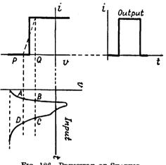
line in the top left part of the figure. The application to such a circuit of the nonrectangular pulse voltage shown in the lower part of the figure will then give a rectangular output pulse as shown.
