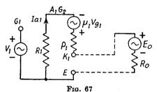
may be made large compared to unity with quite small values of n. It has the further advantage over the circuits of Fig. 64 that one side of the input voltage,  $V_1$ , may be earthed to the common negative.
