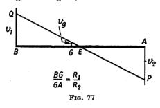
of this circuit. This diagram is simply the graph of the potential distribution along the total resistance  $R_1 + R_2$ , the ordinates being potentials with respect to h.t. negative and AB being a scale of resistance. The letters ABEGcorrespond to the lettering on Fig. 76. Since the potentials of points A and B are
