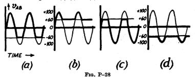
A useful rule for such circuits is that, if terminal A is connected to the anode of the diode, the potential of A will be prevented from rising above a limiting value given by E, whereas if terminal A is connected to the cathode of the diode, the potential of A will be prevented from falling below a limiting value given by E.
