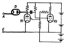
FIG. 197. DIODE SWITCH FOR TRIGGER-ING MONOSTABLE MULTIVIBRATOR
