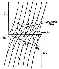
FIG. 43. COMPOSITE CHARACTERISTICS FOR PUSH-PULL CIRCUIT
