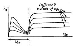
FIG. 17. CHARACTERISTICS OF SCREEN-GRID TETRODE
