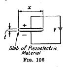
piezo-electric crystal has the two following properties. First, if two opposite faces of the slab are coated with conducting material to form a condenser, then a voltage applied to the plates of this condenser produces a mechanical stress in the slab. For example, the application of a voltage, V, as shown in Fig. 106, would produce a stress tending to increase the length, x. The magnitude of this mechanical stress would be the product of the electrical stress, V/t, and the piezo-
