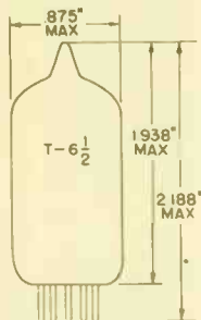
GLASS BULB MINIATURE BUTTON 9 PIN BASE E9-1 OUTLINE DRAWING JEDEC 6-2
