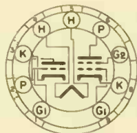
BOTTOM VIEW MINIATURE BUTTDN 9 PIN BASE
