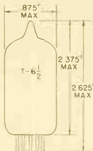
CLASS 9ULB MINIATURE BUTTON 9 PIN BASE E9-1 OUTLINE DRAWING JEDEC 6-3
