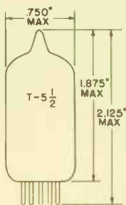
GLASS BULB MINIATURE BUTTON 7 PIN BASE E7-1 OUTLINE DRAWING JEDEC 5:2
