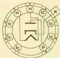
BOTTOM VIEW SMALL-BUTTON 9 PIN NOVAL 9CB
