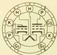
BOTTOM VIEW MINIATURE BUTTON 9 PIN BASE 9FX
