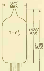
GLASS BULB SMALL-BOTTOM NDVAL 9 PIN BASE E9-1 OUTLINE DRAWING JEDEC 6-2
