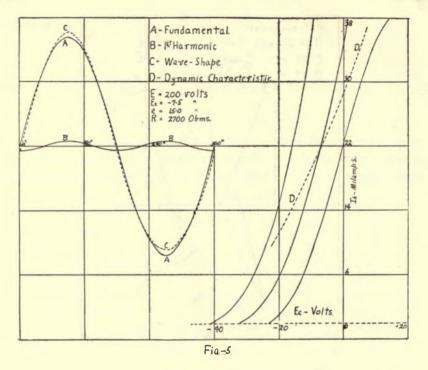
Fig. 5 represents the wave-shape of the plate current obtained when a pure sine wave e.m.f. of 15 volts is impressed on the grid, the plate and grid potentials being the same as stated above. The fundamental and first harmonic are the only components included in the wave-shape. The
