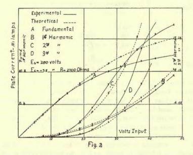
Resistance in Plate Circuit.—When a resistance of 2,700 ohms was placed in series with the plate, and the value of  $E_b$  reduced to 200 volts, the plate current was 21.5 milliamperes. Using these values of potential and resistance the curves shown in Fig. 2 were obtained. The amplitude of the input e.m.f. was varied from 0 up to 50 volts. The latter maximum loaded the tube rather heavily, and the larger currents were maintained just long enough to obtain the necessary readings.
