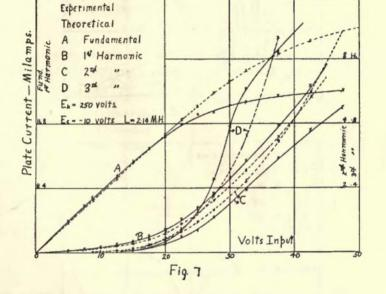
The reactive load in the plate circuit was 2,700 ohms. Fig. 7 shows the variation of the harmonics with the alternating e.m.f. on the grid, under the conditions given above.
