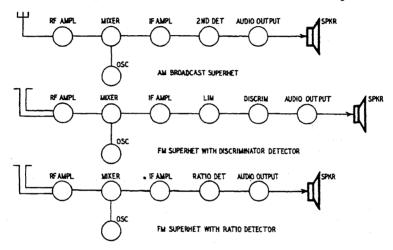
Fig. 711. Block diagrams of three superheterodyne receivers.
