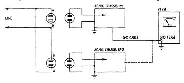
Fig. 502. If both a.c.-d.c. chassis are plugged into the power line, as shown, a connecting link between the two chassis (or if the two are tied together through the v.t.v.m.) would result in a short circuit.
