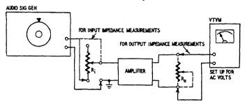
Fig. 806. Test method for determining the input and output impedances of an audio amplifier. The same procedure can be used for impedance measurements of circuits other than audio amplifiers.
