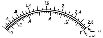
Fig. 304. Some low a.c. voltage scales are also nonlinear, a situation caused by the nonlinearity characteristic of the rectifying diode (used in the v.t.v.m.) at low a.c. signal levels.
