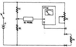
Fig. 1008. The v.t.v.m. can be used as a sensitive null indicator.
