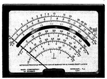
Fig. 301. In this illustration we have the dial scales of a modern v.t.v.m. The use of a number of scales having various ranges gives the instrument considerable versatility, extends its usefulness.
