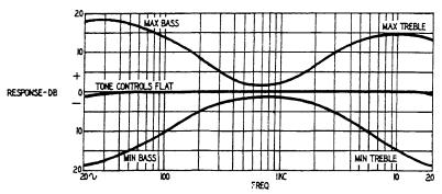
Fig. 805. Typical curves obtained for various settings of the audio-amplifier controls.
