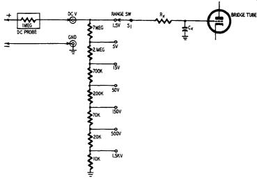
Fig. 204. Voltage-divider network at the d.c. input to a v.t.v.m. The input resistance, including the resistance of the external probe, is 11 megohms.
