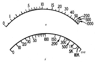
Fig. 303-a, b. Typical resistance scales shown above are nonlinear. The right-hand end of such scales is so crowded that it is often difficult to read. It is easier to make an error reading these than when reading voltage or current
