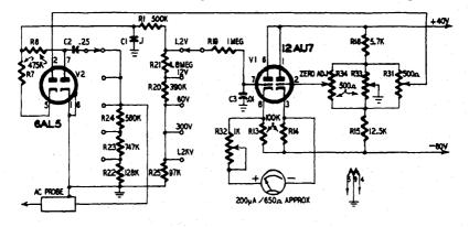
Fig. 1107. A.c. voltage section of the v.t.v.m. The diode rectifies the a.c., passes it on to the triode in the form of a d.c. voltage.
