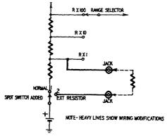
Fig. 1009. Modification of v.t.v.m. for resistance matching.
