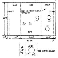
Fig. 1018. Chassis layout of the preamplifier unit.
