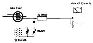
Fig. 705. Test setup for checking the local oscillator.
