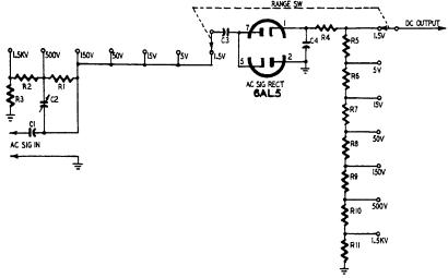
Fig. 210. A.c. measuring circuit of a peak-to-peak type of v.t.v.m. This circuit enables the instrument to measure the peak-to-peak values of complex waveforms.
