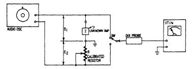
Fig. 1012. The v.t.v.m. and a generator can be used to measure the impedance of a coil or a capacitor, or combination of resistance, inductance and capacitance.
