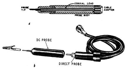
Fig. 401-a, -b. Direct probe (a) shields the test lead almost up to the probe tip.
