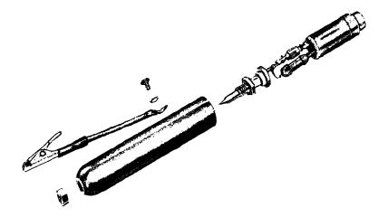
Fig. 410. Internal construction of a crystal rectifier probe. The ground lead is an important part of the crystal probe circuit.
