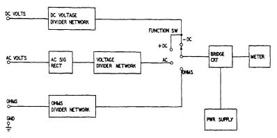
Fig. 1103. This block diagram represents the circuit arrangement in many v.t.v.m.'s.
