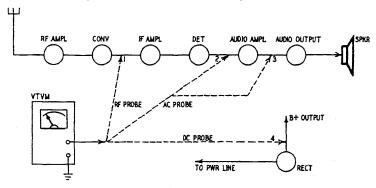
Fig. 709. An intermittent receiver can be monitored by connecting the v.t.v.m. to the check points shown in this block diagram.
