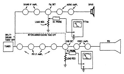
Fig. 610. The v.t.v.m. (set to read d.c. volts) and a d.c. probe can be used to monitor the picture or sound sections of a TV receiver. For servicing intermittents, it is generally preferable to use a signal generator rather than depend upon a television station as the signal source.
