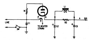
Fig. 706. Test points in simple half-wave power supply.
