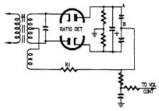
Fig. 713. Ratio-detector circuit.
