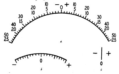
Fig. 305-a, -b, -c. Typical zero-center scales used in some v.t.v.m.'s. Some scales are calibrated, others simply have a center marker and a plus-minus indication. Calibrated scales are helpful in the alignment of circuits such as FM detectors.
