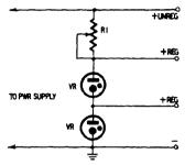
Fig. 908. VR tubes connected in series.
