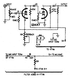
Fig. 1019. Diagram of the v.t.v.m. preamplifter. The circuit is that of a resistancecoupled amplifier.
