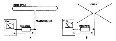
Fig. 1011-a, -b. Technique for testing transmission lines and TV antennas. Disconnect the line from the receiver terminals before making the check.
