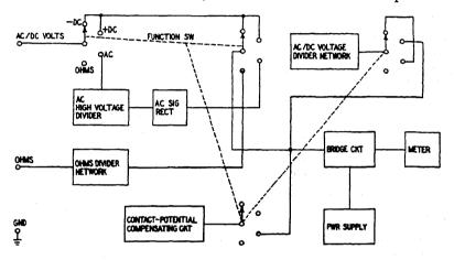
Fig. 1104. Block diagram of the various circuits of a v.t.v.m. This instrument uses a contact-potential compensating circuit for a.c. voltage measurements.
