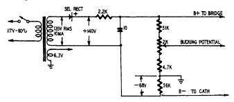
Fig. 216. Power supply for the v.t.v.m. is small, uses selenium rectifier and simple R-C filter. A vacuum-tube rectifier is sometimes used in place of the selenium unit.
