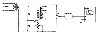
Fig. 1013. Method for determining the impedance of a transformer winding. The test frequency should be that at which the transformer will be used.
