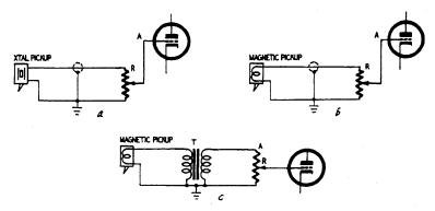
Fig. 1031-a, -b, -c. The v.t.v.m. can be used to check the output of phonograph cartridges. Use a constant amplitude test record for making these measurements.
