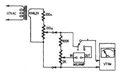
Fig. 1022. Calibration of the v.t.v.m. using the preamplifier.
