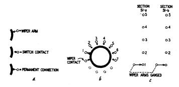
Fig. 1101-a, -b, -c. Rotary switches used in v.t.v.m.'s can be represented in these three different ways in circuit diagrams.
