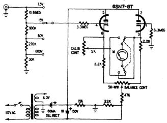
Fig. 1027. Schematic diagram of simplified v.t.v.m.
