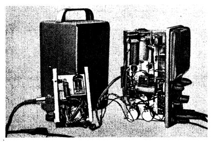
Fig. 1020. Underchassis view of the preamplifier shows connections to the v.t.v.m.
