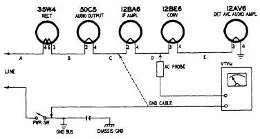
Fig. 701. The v.t.v.m. can be used to check the heater wiring of filament circuits.
