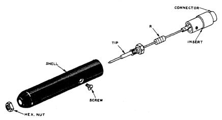
Fig. 403. Exploded view of a d.c. (or isolating) probe. The resistor, R, most often has a value of one megohm. The probe, held together by a single screw and hex nut, can easily be taken apart when repairs are needed.
