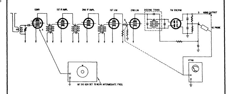
Fig. 712. Simplified circuit diagram of FM receiver using two limiter stages and discriminator-type detector. This arrangement is gradually being replaced by FM sets using ratio detectors. Such receivers do not ordinarily have limiter circuits. Various test points are shown in the FM circuit above. The audio stages have been eliminated since these are checked in the same manner for all receivers.
