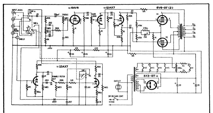
Fig. 801. Representative circuit diagram of a high-fidelity amplifier. The v.t.v.m. can be used to service the amplifier (in the event of component failure) or can be used to get optimum performance. For servicing and maintenance of such units the v.t.v.m. is practically indispensable. Checking techniques are described in the text.
