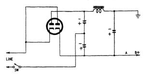
Fig. 707. Full-wave voltage doubler circuit.
