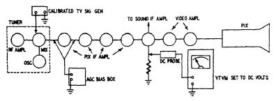
Fig. 611. Setup for plotting the bandpass of a TV i.f. amplifier.
