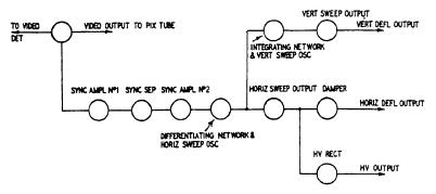
Fig. 614. Block diagram of the various sweep circuits used in a TV receiver. These circuits can be checked through with a v.t.v.m. by making voltage and resistance measurements. A.c. voltages are best measured with a peakto-peak reading v.t.v.m.
