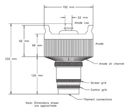
Figure 3.13 Principal dimensions of 4CX15000A tetrode.
