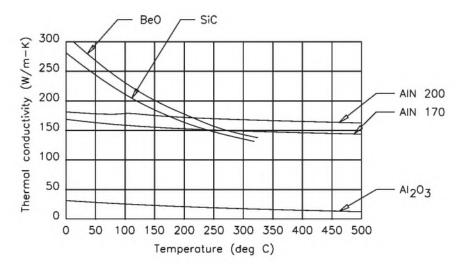
Figure 3.37 Thermal conductivity of common ceramics.
