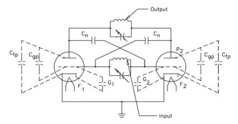
Figure 3.41 Push-pull grid neutralization.
