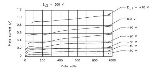
**Figure 3.11** Tetrode plate current characteristics. Plate current is plotted as a function of plate voltage, with grid voltages as shown.
