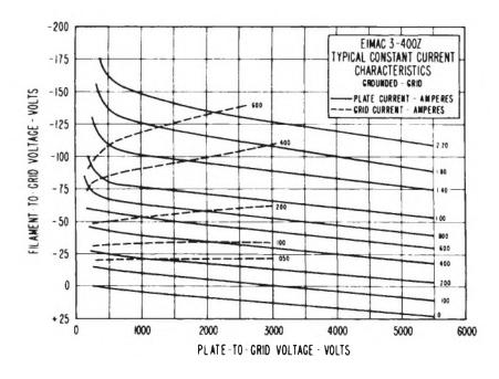
Figure 3.9 Grounded-grid constant-current characteristics for a zero-bias triode with a  $\mu$  of 200.
