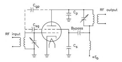
Figure 3.46 Single-ended plate neutralization.
