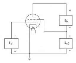
Figure 3.33 Series power supply configuration for swamping the screen circuit of a tetrode.
