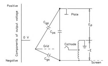
**Figure 3.54** Components of the output voltage of a tetrode neutralized by adding inductance common to the screen and cathode return.
