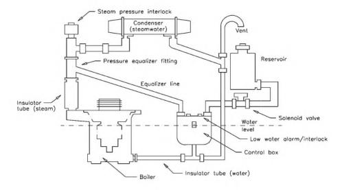
Figure 3.22 Typical vapor-phase cooling system.
