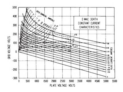
Figure 3.8 Constant-current characteristics for a triode with a  $\boldsymbol{\mu}$  of 20.
