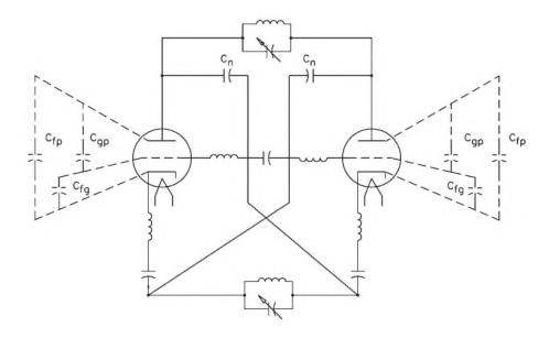
Figure 3.50 Neutralization by cross-connected capacitors of a symmetrical cathode-excited amplifier wth compensation of lead inductance.
