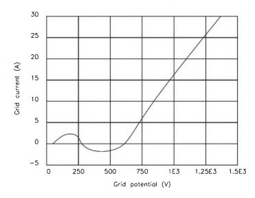
**Figure 3.34** Typical curve of grid current as a function of control grid voltage for a high-power thoriated-tungsten filament tetrode.
