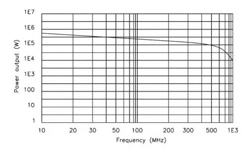
Figure 3.16 Continuous wave output power capability of a gridded vacuum tube.
