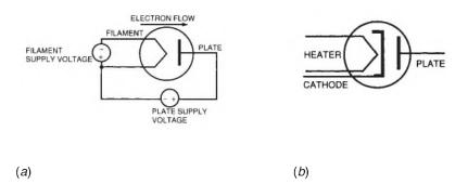
**Figure 3.4** Vacuum diode: (a) directly heated cathode, (b) indirectly heated cathode. (*From* [2]. *Used with permission*.)
