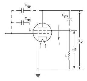
Figure 3.39 The elements involved in the neutralization of a tetrode PA stage.
