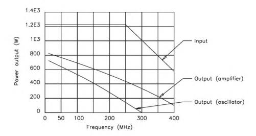
$\textbf{Figure 3.17} \ \ Performance of a class C amplifier as the operating frequency is increased beyond the design limits of the vacuum tube.$
