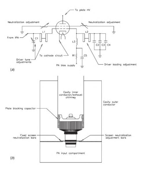
**Figure 3.48** A grounded-screen PA stage neutralized through the use of stray inductance between the screen connector and the cavity deck: (a) schematic diagram, (b) mechanical layout of cavity.
