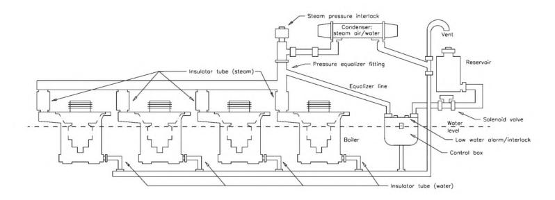
Figure 3.23 Vapor-phase cooling system for a 4-tube transmitter using a common water supply.
