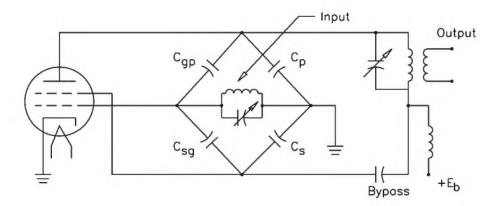
Figure 3.47 Single-ended plate neutralization showing the capacitance bridge present.
