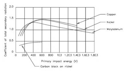
**Figure 3.35** Secondary emission characteristics of various metals under ordinary conditions.
