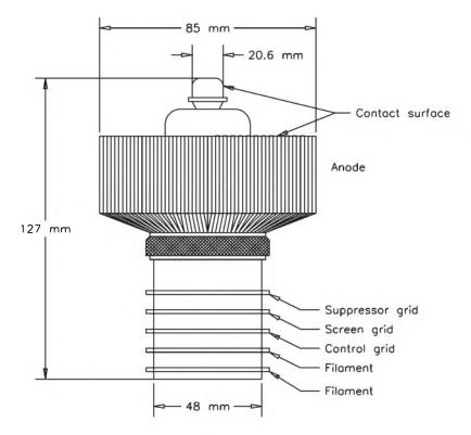
Figure 3.15 Principal dimensions of 5CX1500B pentode.
