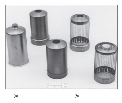
**Figure 3.29** Pyrolytic graphite grid: (a) before laser processing, (b) completed assembly. (Courtesy of Varian.)
