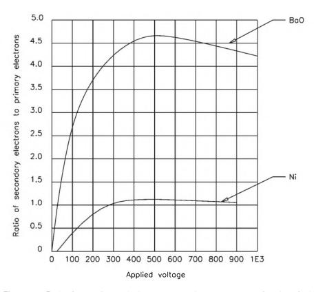
**Figure 3.3** Ratio of secondary emission current to primary current as a function of primary electron velocity.
