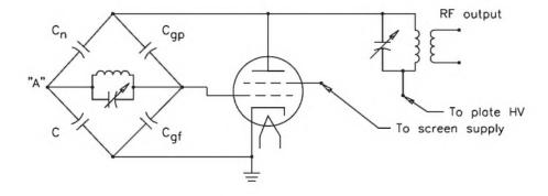
Figure 3.45 The previous figure redrawn to show the elements involved in neutraliza-
