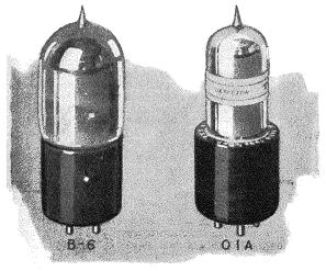
Left: The B-6 tube is a new type of detector operating on a different principle from the standard vacuum tube. It is very sensitive and can be used in any but a regenerative circuit. 01-A, and G, at the right, are high-impedance tubes with high amplification factors designed for use in resistance- and impedancecoupled A.F. amplifiers. Type F is a power amplifier for use in the last stage of any type of A.F. amplifier.
