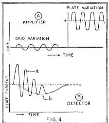
When a tube is employed as an amplifier the plate current variation is a magnification of the grid voltage variation, except for the fact that the plate current is a positive variation only as shown at A. When a tube is employed as a detector the plate current flows only during positive variations of grid voltage. This is shown in B; a is the plate current variation and b the effective telephone current.
