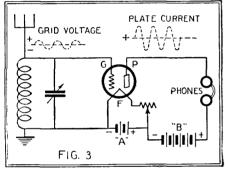
Illustrating the action of a vacuum tube in a radio receiving circuit. For every positive and negative variation of the signal voltage, impressed on the grid of the tube, there is a resultant positive variation of the plate current which is always flowing when the tube is lighted. The grid voltage and plate current are represented by dotted lines directly above the diagram. It will be noted that the plate current variation corresponds to that of the grid voltage, but is greatly amplified.
