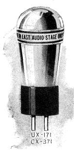
A new storagebattery type power amplifier tube, for use in the last stage audio amplifier only. Th is tube takes the same filament voltage and filament current as the No. 112 tube shown above, but employs a "B" voltage of 180 and a 40<sup>3</sup>/<sub>2</sub> volt "C" battery. Special means should be prov i d e d for handling it s heavy output. Two arrangemenn in Fig. 6.
