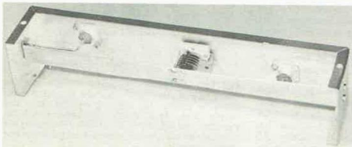
Fig. 15-12 — A half-wave strip line is used in the 220-MHz filter. It is grounded at both ends and tuned at the center.
