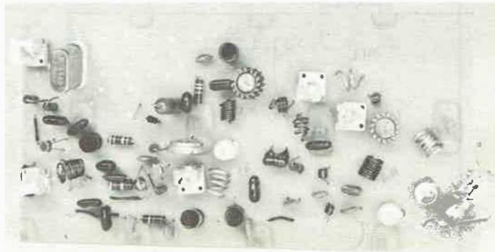
Fig. 11-29 — Top view of the solid-state 1-W transmitter for 220 MHz.
