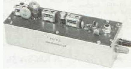
Fig. 11-4 - The solid-state fm adapter is constructed on a 6 x 2-inch etched-circuit board, mounted on a homemade chassis.
