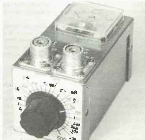
Fig. 14-16 — Simple vhf impedance bridge. Settings of the variable control, marked on the front of the case, represent values of impedance corresponding to nulls in meter indication.
