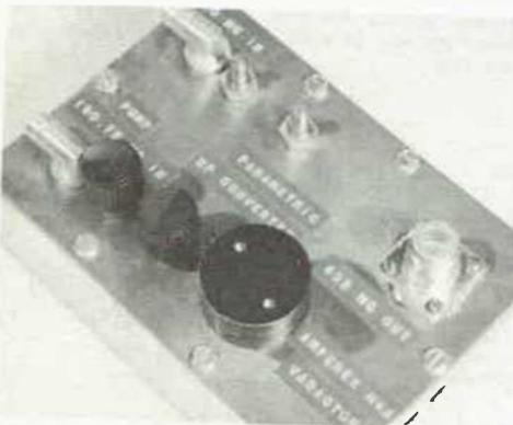
Fig. 13-26 — Parametric up-converter for transferring a 50-MHz ssb signal to 432 MHz. The large black object, a heat-dissipating cap for the varactor, taken from a 2C39A tube, is not needed if an all-metal chassis is used.
