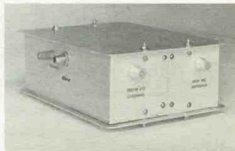
Fig. 4-15 — The twin vhf converters are housed in a homemade aluminum box which has removable top and bottom covers for easy access to the circuit boards. Each converter has its own input and output jacks so that simultaneous operation is possible.
