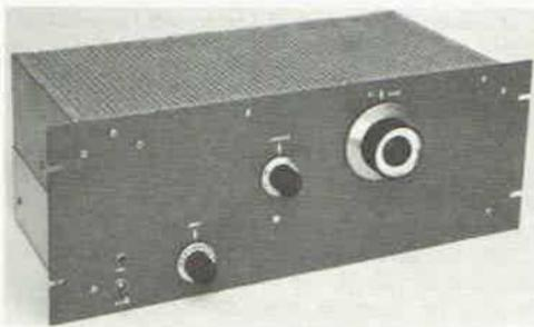
Fig. 6-49 — The 144-MHz amplifier is built in conventional rack and panel style, with the entire top of cane metal, to provide free air flow. Controls are grid-circuit tuning, C2, lower left; output loading capacitor, C5, center; and plate-circuit tuning, C4, with vernier dial, right. The slotted end of the Teflon shaft on C1 is visible as a white spot just below the loading control.
