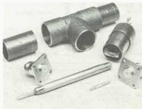
Fig. 14-20 — Major components of the line sampler. The brass T and two end sections are at the back of the picture. A completed probe assembly is at the right. The N connectors have their center pins removed. The pins are shown with one inserted in the left end of the inner conductor and the other lying in the right foreground.
