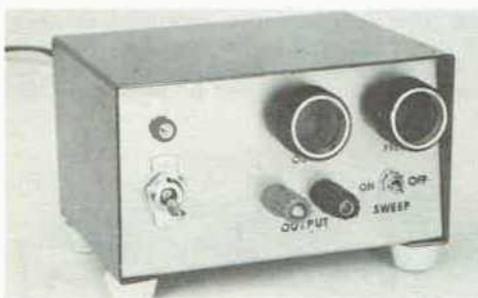
Fig. 11-43 — The sweep generator for fm i-f alignment.
