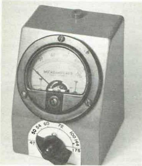
Fig. 14-7 — A field-strength indicator and wavemeter for 50 and 144 MHz. The coil size is set so that the tuning range is approximately 47 to 175 MHz.
