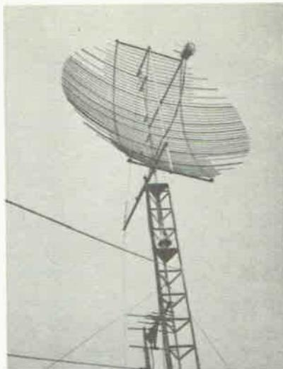
Fig. 16-6 — The WA9HUV 12-foot dish for 432 and 1296 MHz atop its 50-foot tower.
