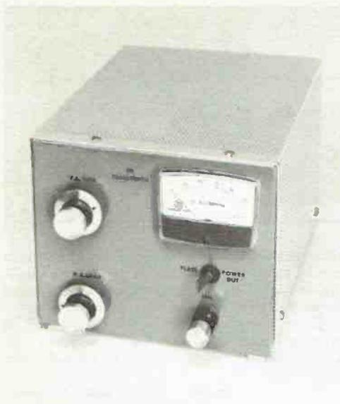
7-8 — The 6-meter transverter, with shield cover in place. Large knobs are for amplifier tuning and loading. Small knob, lower right, is for a meter sensitivity control. The meter switch is just above it.
