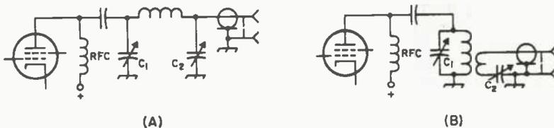
Fig. 5-8 — Basic functions of tuning and impedance matching are performed equally well in the pi-network, A, and inductively coupled output circuit, B. Choice in single-band vhf amplifiers is mainly a matter of convenience in a particular design.
