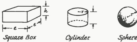
Fig. 13-6 — Forms of cavity resonators. The square and cylindrical types are merely closed-off sections of waveguide.
