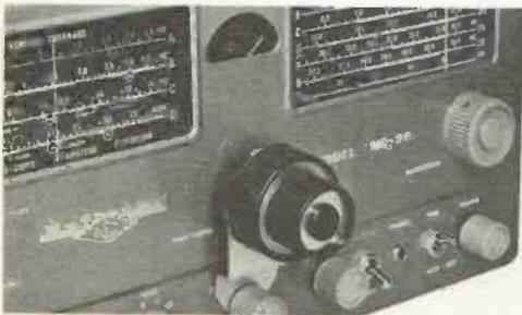
Fig. 3-9 — Example of use of a two-speed planetary mechanism to slow down the tuning rate on the general-coverage dial of an inexpensive communications receiver.
