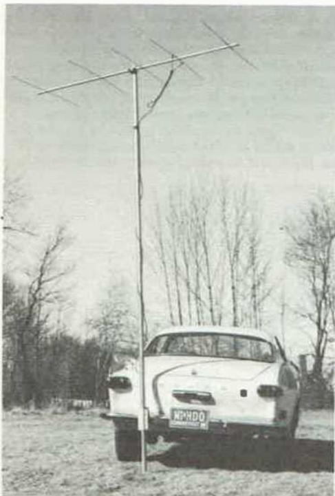
Fig. 9-54 — Portable beam set up for 144 MHz, using the bumper bracket of Fig. 9-46.
