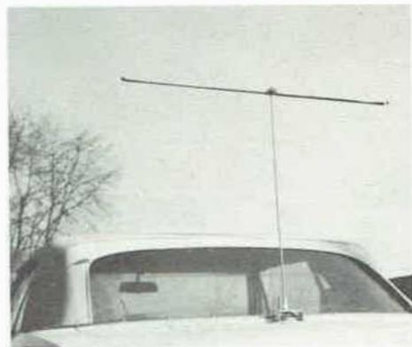
Fig. 9-53 — Horizontal dipole for 2-meter mobile. The vertical support is 1/4-inch tubing, with small coax inside, thus serving as a 1:1 balun.
