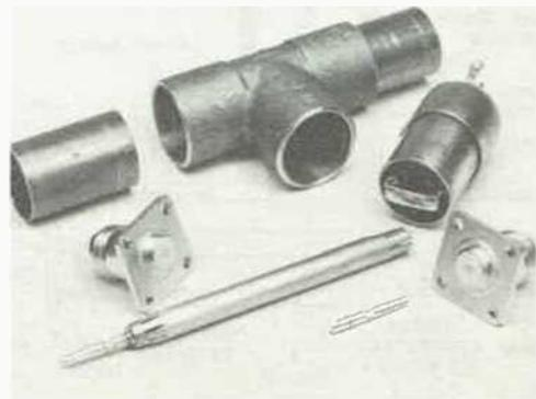
Fig. 14-20 — Major components of the line sampler. The brass T and two end sections are at the back of the picture. A completed probe assembly is at the right. The N connectors have their center pins removed. The pins are shown with one inserted in the left end of the inner conductor and the other lying in the right foreground.
