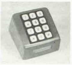
Fig. 12-29 — The homemade Touch-Tone generator is housed in a plastic box. The keyboard is a Chromerics EF-20457 which has no moving parts. Electrical contact is made by chemical means.
