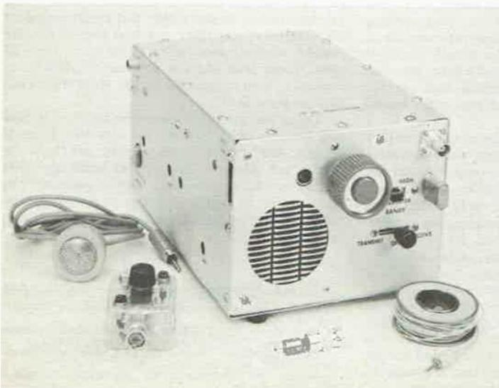
Fig. 7-19 — The 50-MHz portable station, complete with all necessary operating accessories — total weight: under 5 pounds. Accessories grouped around the transceiver: the microphone, miniature antenna coupler, pilot-lamp dummy load, and a 35-foot "long-wire" antenna.
