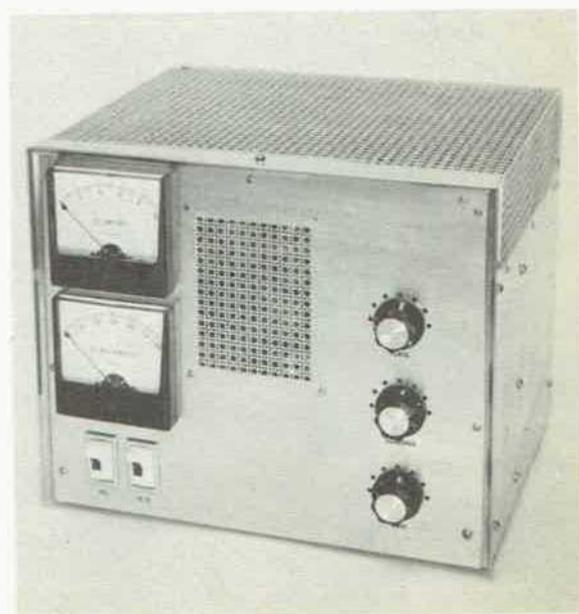
Fig. 6-45 — Table-top 50-MHz amplifier of grounded-grid design, only 10 X 12 inches in size. Grid and plate current are monitored simultaneously. Knobs at the right are for input tuning, bottom, amplifier loading, center, and plate tuning, top.
