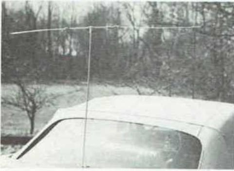
Fig. 9-51 — Shortened dipole for 50-MHz mobile service. Loading coils are inserted either side of a solid center section. Inserts are 19 inches long, threaded into forms that support the loading coils. See Fig. 9-52.
