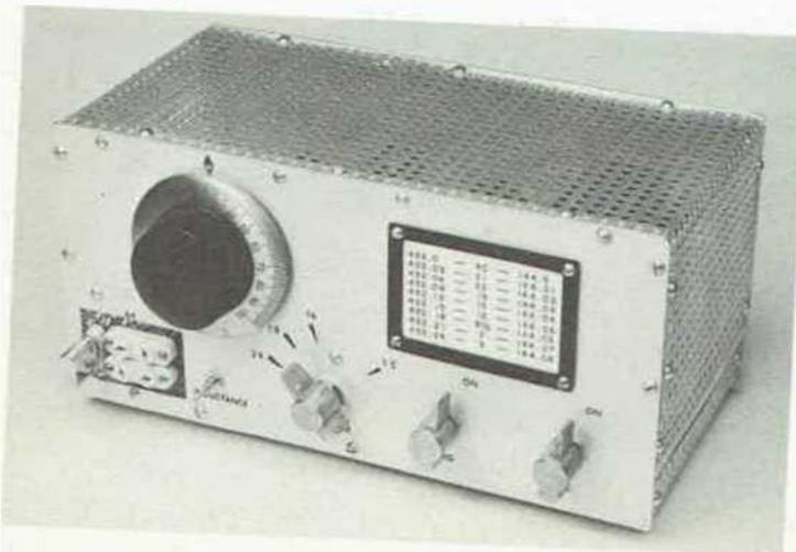
Fig. 6-1 — A VXO especially for vhf use. Calibration on the front panel is for a favorite crystal used for cw work on 144 and 432 MHz. Crystal sockets at the lower left are mounted on insulating material, to reduce circuit capacitance to the lowest possible value. Frequency variation per crystal depends on which socket is used. Pointer knobs are for the output plate circuit and the spotting and power switches.
