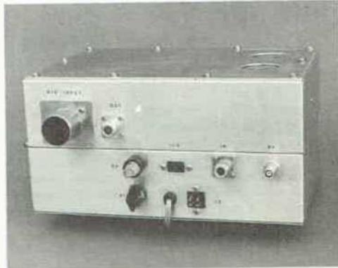
Fig. 13-49 — Rear view of the K2RIW 432-MHz kilowatt amplifier.
