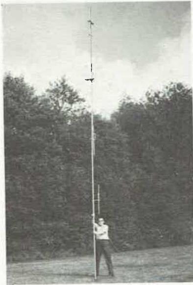
Fig. 12-9 — An array of dipole elements which provides approximately 6 dB of gain.
