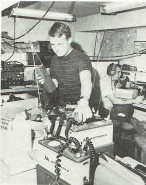
Fig. 10-1 – One advantage of the fm mode is the large amount of surplus equipment which can be converted for amateur use. AREC and civil-defense groups increasingly are using vhf fm for local communications networks because of the low cost and high reliability of surplus commercial gear. Here WA6ECK checks Motorola Handi-Talkies which have been modified for 6-meter operation at the San Fernando Emergency Operating Center during an earthquake emergency.
