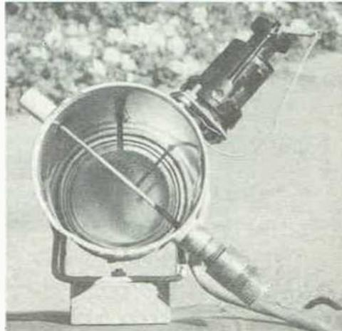
Fig. 13-13 — Looking into the open end San Bernardino Microwave Society 3300-MHz polaplexer. The klystron oscillator is mounted at a 45-degree angle, with its "antenna" in the same plane inside the beer-can waveguide section. Perpendicular to it is the receiving probe, connected to the crystal mixer, upper left. The vertical screw, upper center, is the mixer injection adjustment.
