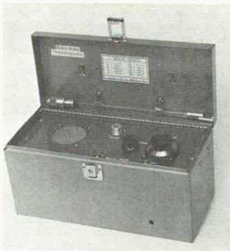
Fig. 7-29 — The 2-meter transceiver is housed in a legal-bond box. A dial-calibration chart for the receiver is pasted on the inside of the lid. Two plastic cable clamps serve as holders for the two-section 1/4-wavelength whip antenna (inside lid) when the unit is not in use. The antenna is held together at the center by a 1/4-inch-diameter threaded coupling.
