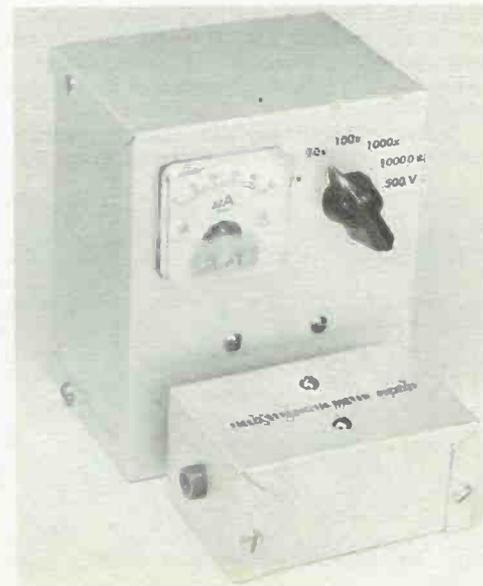
Fig. 14-10 — A vhf field-strength indicator and general-purpose test instrument for dc measurement. The small pickup unit can be plugged into the indicator as shown, or connected to it by a 2-wire cable of any desired length. Antenna rods or wires plug into jacks at each end of the small box. The meter can be used with test leads for measuring direct current and voltage. Ranges are 0 to 50 and 500 microamperes, 5, 50, and 500 milliamperes, and 0 to 500 volts dc.
