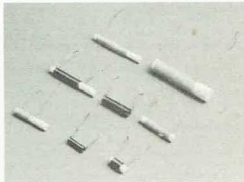
Fig. 16-10 — Typical handmade vhf chokes. At the rear are closewound and spacewound chokes for 50 MHz wound on 1/4-inch and 1/2-inch Teflon rod, drilled and tapped for end-mounting. Three 144-MHz chokes are seen in the center row, the two at the left being excellent for high-current applications. Similar types to these, but for the 220-MHz band, are in front.
