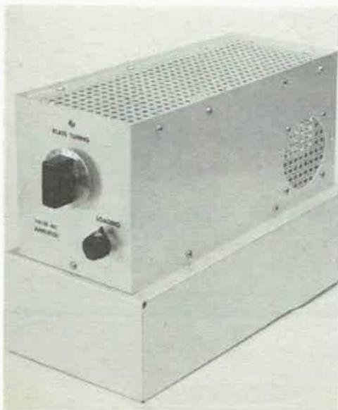
Fig. 6-33 — The 829-B amplifier, with its shield cover in place. Air circulation is provided by the screened holes and cover.
