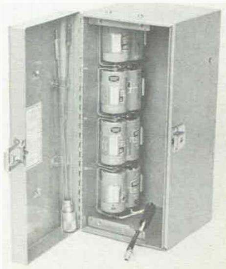
Fig. 7-33 — Eight size-D cells are series connected to provide 12 volts. They are mounted in Keystone holders on the back wall of the bond box. The 1/4-inch-diameter hole in the front of the cabinet (upper right of photo) permits final calibration of the receiver (C20) after the installation is completed. The hole is opposite the shaft of C20.
