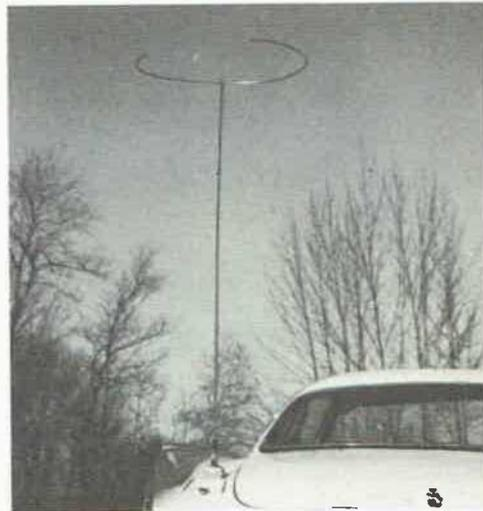
Fig. 9-49 — This 144-MHz halo appears to have no transmission line or matching device. Attached off-center to the whip of Fig. 9-47, it uses the whip as a single-wire transmission line. Optimum whip length is approximately 40 inches, so top section is telescoped when the halo is used. Very little vertical polarization is in evidence.
