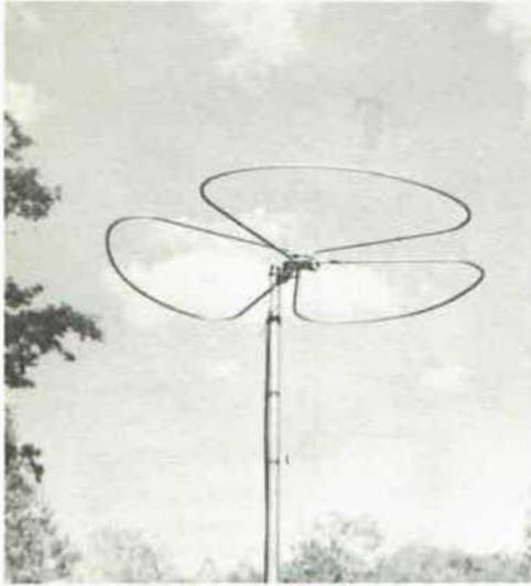
Fig. 9-41 — The Big Wheel, an omnidirectional horizontal antenna for the 144-MHz band designed by W1FVY and W1IJD. Radiating elements occupy an area approximately 40 inches in diameter.
