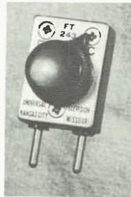
Fig. 16-2 — An FT-243 surplus crystal, modified for variable frequency control.
