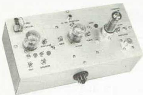
Fig. 7-4 — Transmitting converter for duplicating a 50-MHz signal on 144 MHz. Two tubes at the left and center comprise the oscillator, multiplier, amplifier, and mixer stages. At the right is the 144-MHz output amplifier. Provision is made for metering all stages by means of tip jacks and test points. Note crystals taped together to prevent loss of the one not in use.
