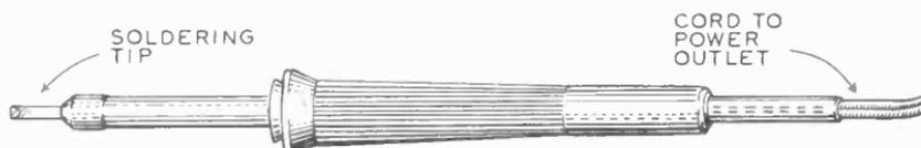
SMALL SOLDERING IRON (25-WATT) FOR TRANSISTOR CIRCUITS
