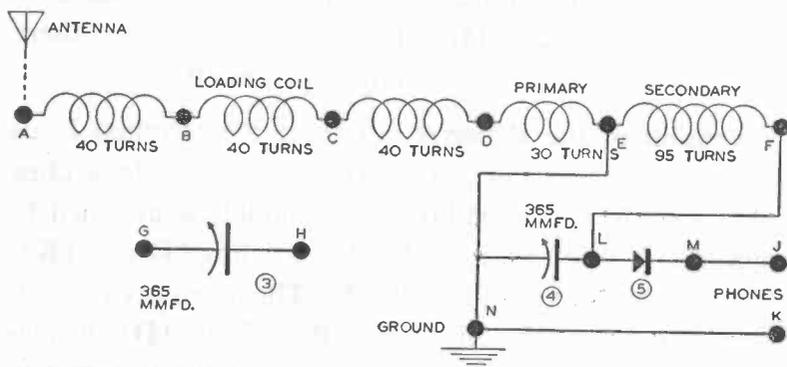
CIRCUIT DIAGRAM OF THE CRYSTAL RECEIVER
