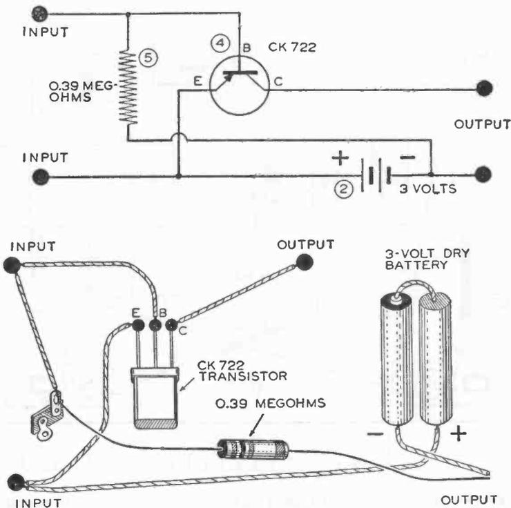
The components can be purchased for \$1.75 or less. When connected to either of the crystal detector receivers described in Chapter Three, this amplifier will greatly increase the strength of the signals.
