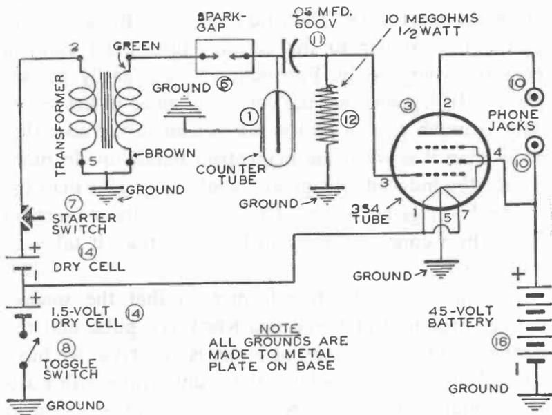
**SCHEMATIC CIRCUIT DIAGRAM OF THE "GAMMA SNIFFER"**
