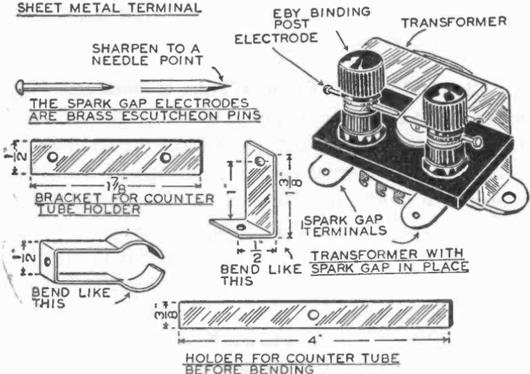
**DETAILS OF THE SPARK GAP, BRACKET AND HOLDER FOR G-M TUBE**
