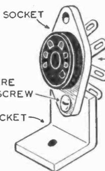
SOCKET IS FASTENED TO BRACKET BY A SCREW AND NUT
