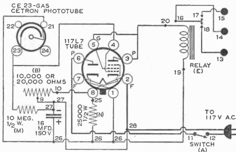
117L7 tube operates directly from the 117-v AC power supply without any form of resistor in series.
