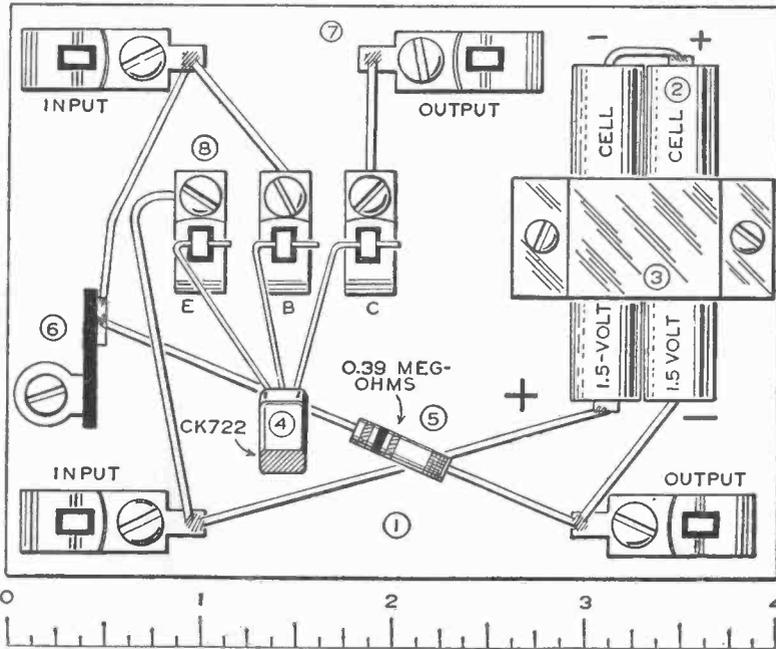
PLAN OF THE ONE-STAGE TRANSISTOR AUDIO AMPLIFIER
