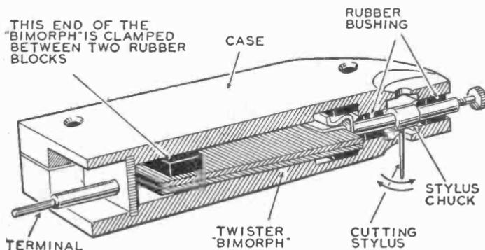
**THE CARTRIDGE IN A PHONOGRAPH PICKUP IS A TINY ELECTRICAL GENERATOR**
