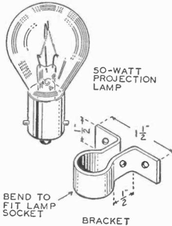
PROJECTION LAMP. SOCKET, RESISTOR AND HOMEMADE BRACKET FOR LIGHT SOURCE
