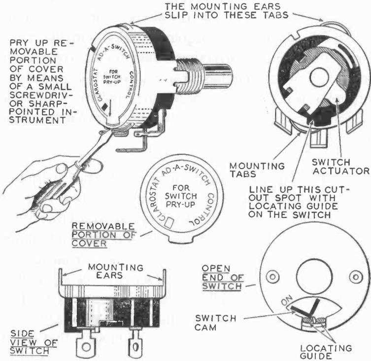
**HOW TO ATTACH AN "ON-OFF" SWITCH TO A CONTROL**
