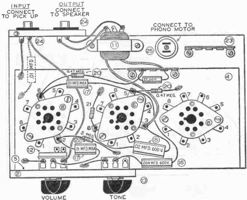
PLAN OF THE AMPLIFIER SHOWING THE WIRING OF THE AUDIO CIRCUIT
