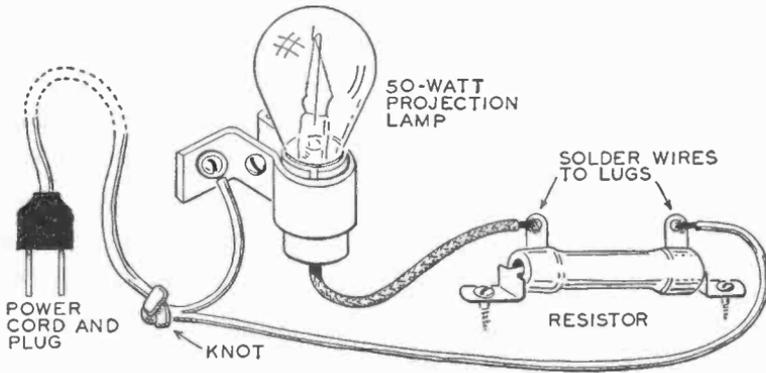
CONNECT LAMP IN SERIES WITH RESISTOR
