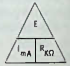
(B) Optional units (volts, kilohms, and milliamperes).
