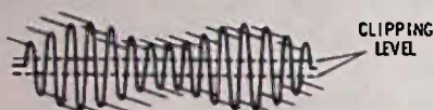
FM SIGNALS CAN BE CLIPPED (CALLED LIMITING) TO REMOVE NOISE BUT SIGNAL STILL RETAINS ITS FREQUENCY CHANGE AND THIS CAN BE DETECTED BY THE FM DEMODULATOR
