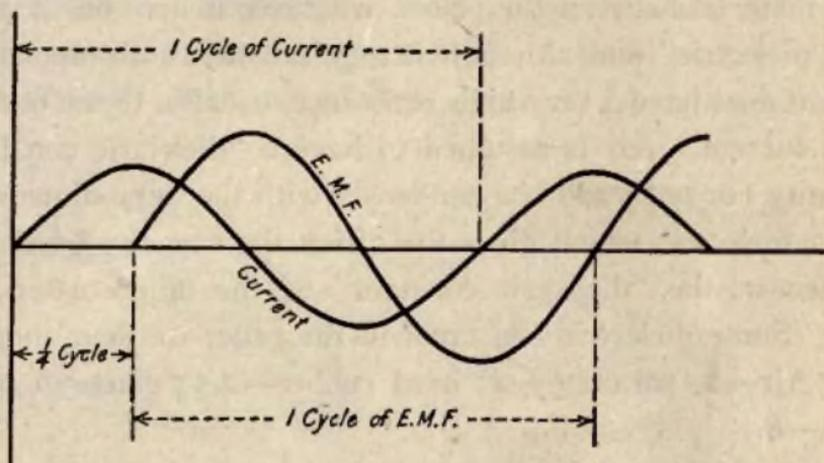
Fig. 5—Effect of capacitance in an alternating current circuit.
