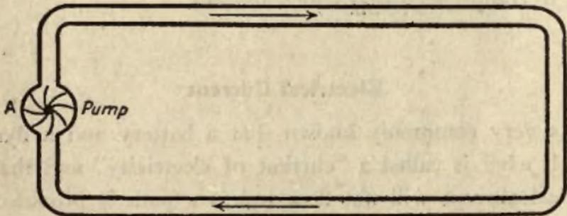
Fig. 2—Water analogy of simple electrical circuit.
