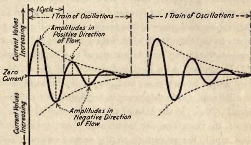
Fig. 10—Damped oscillations.
