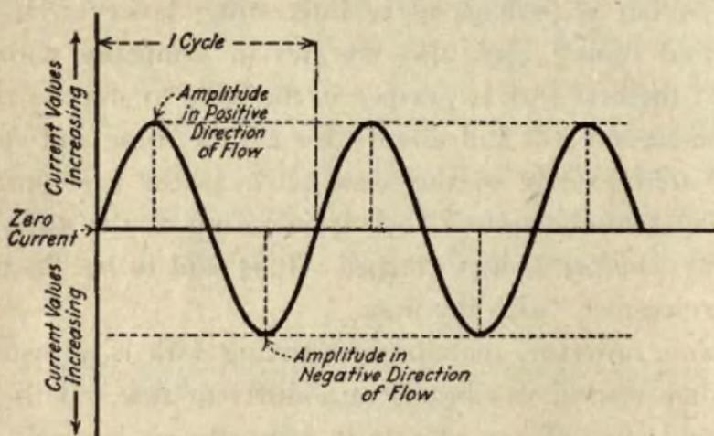
Fig. 9—Continuous oscillations.
