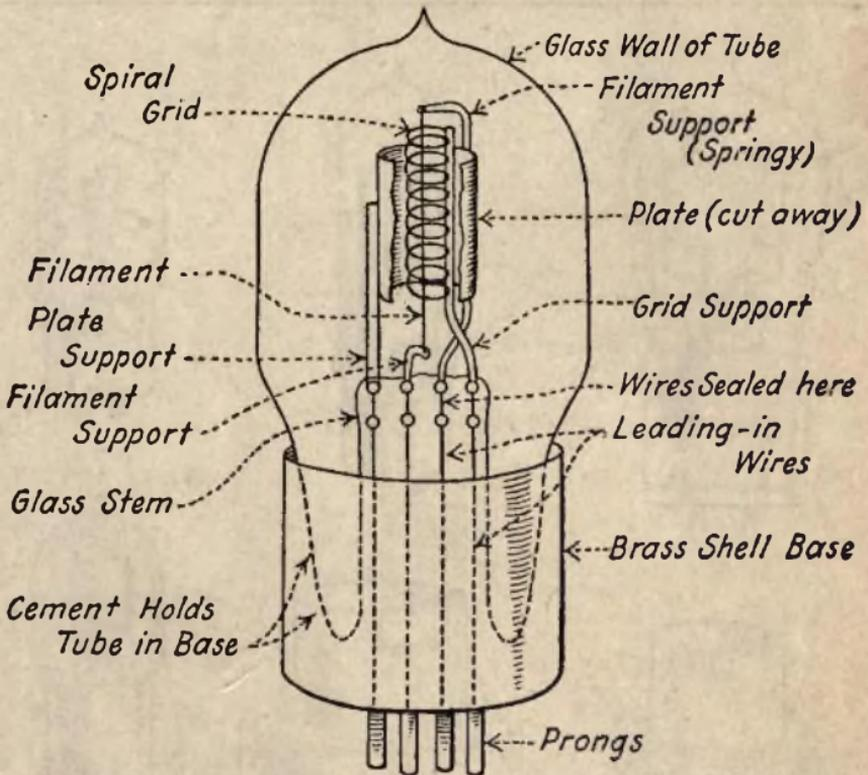
Fig. 12—Construction of a typical vacuum tube.
