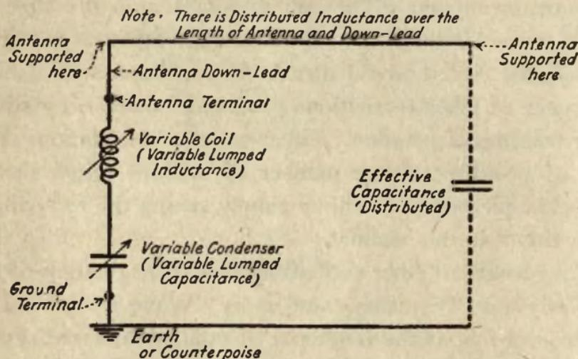
Fig. 11.—Scheme of antenna as a complete circuit.
