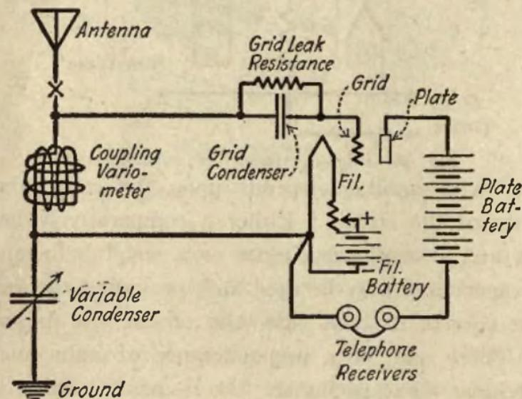
Fig. 37.—Simple Single Circuit Receiver.
