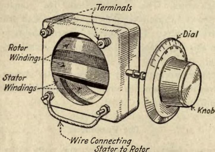
Fig. 35—Construction of a typical variometer.
