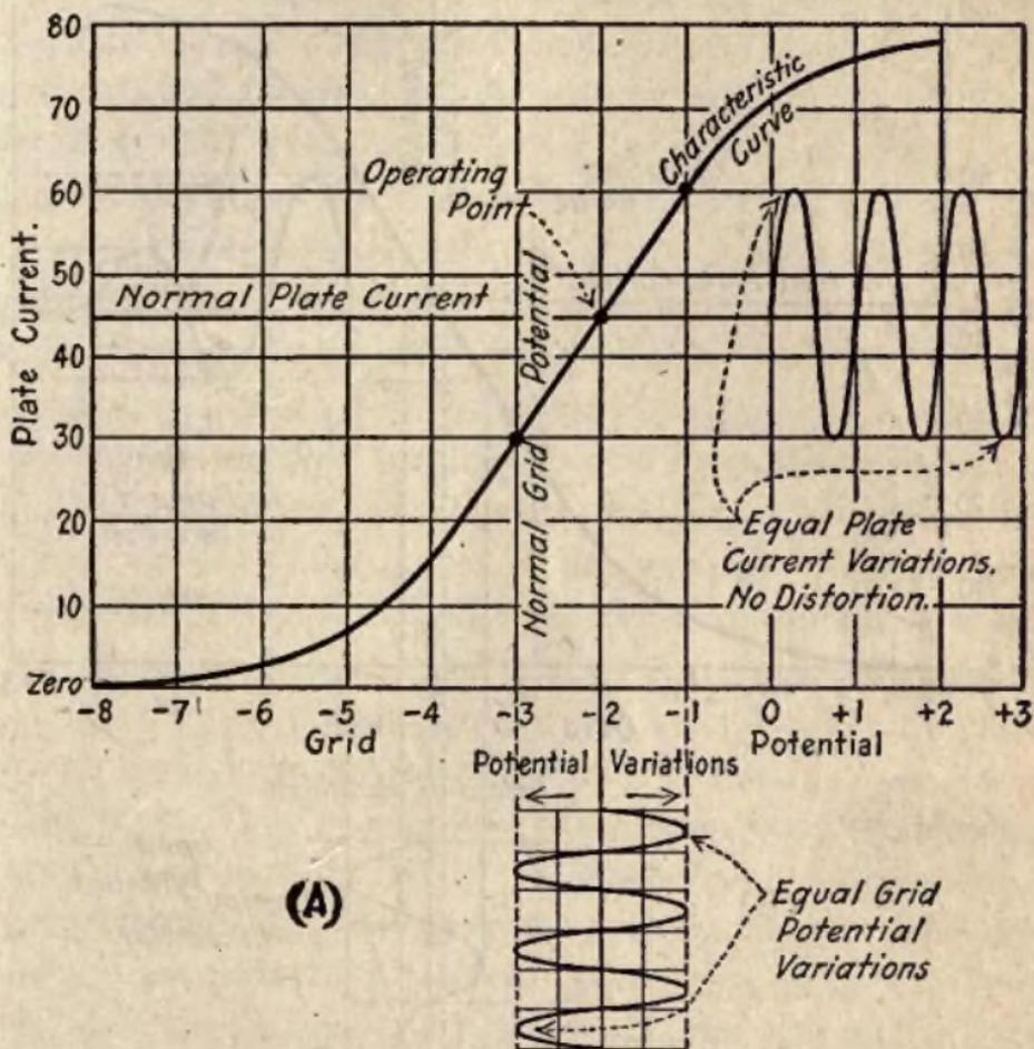
Fig. 29 (a)—Amplification of continuous oscillations.
