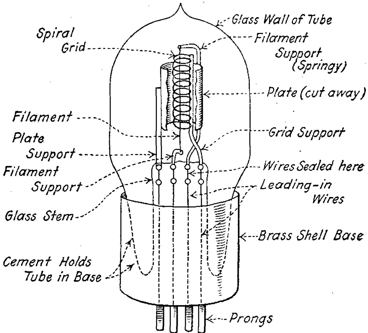
Fig. 12—Construction of a typical vacuum tube.
