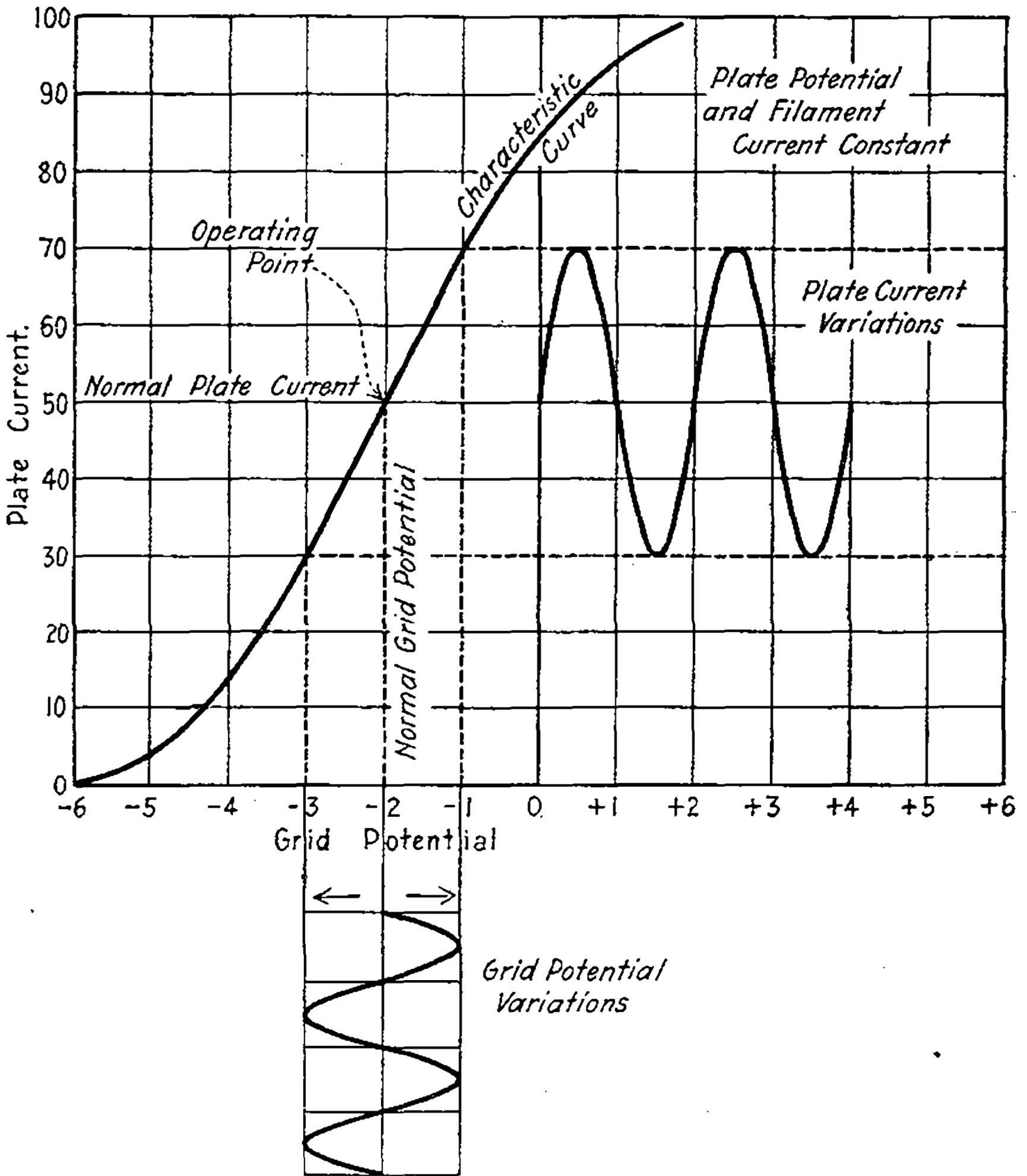
Fig. 30—Amplification of continuous oscillations
