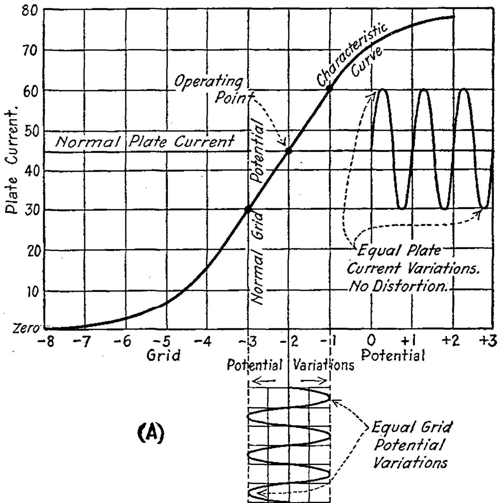
Fig. 29 (a)—Amplification of continuous oscillations.
