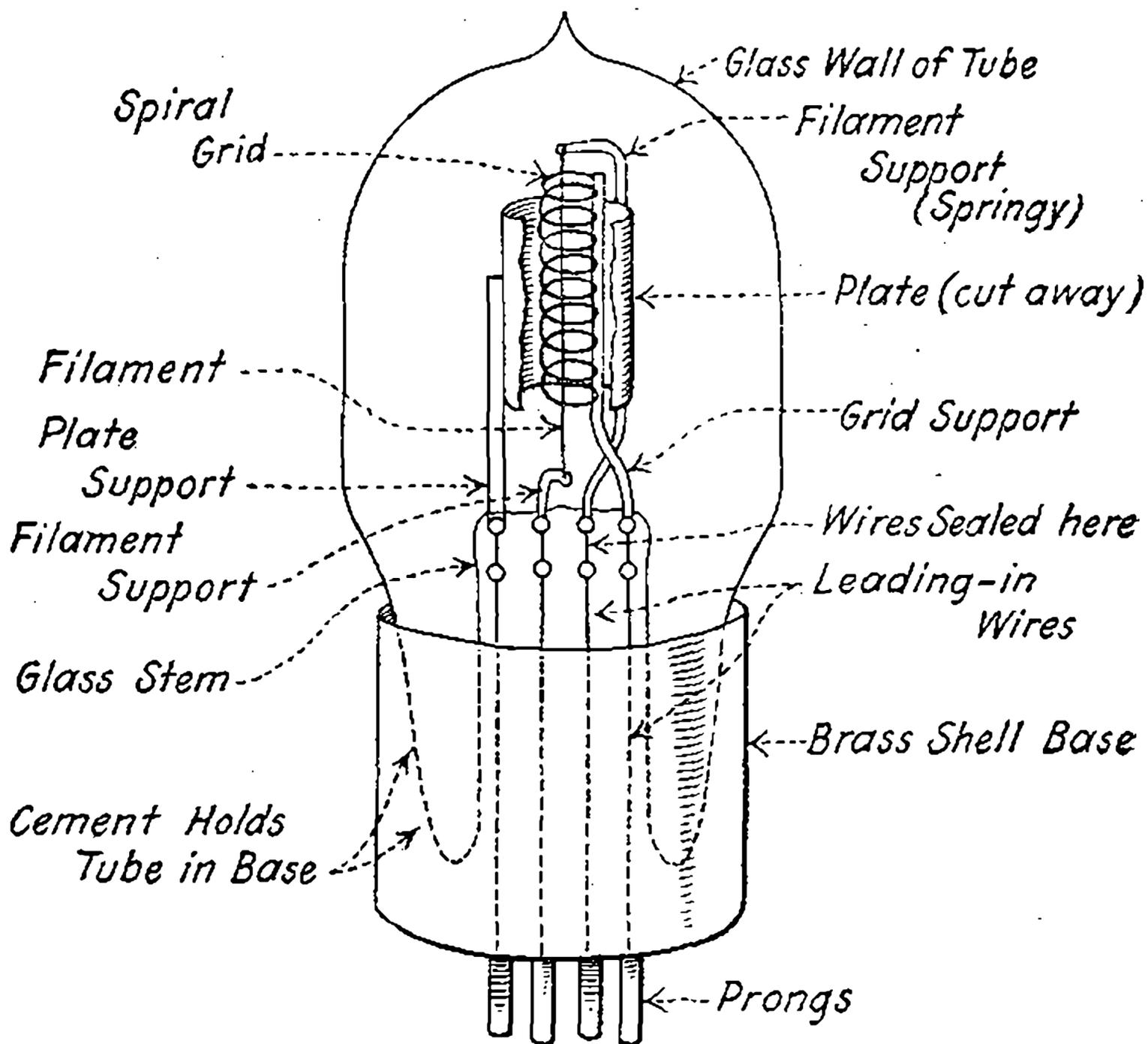
Fig. 12—Construction of a typical vacuum tube.
