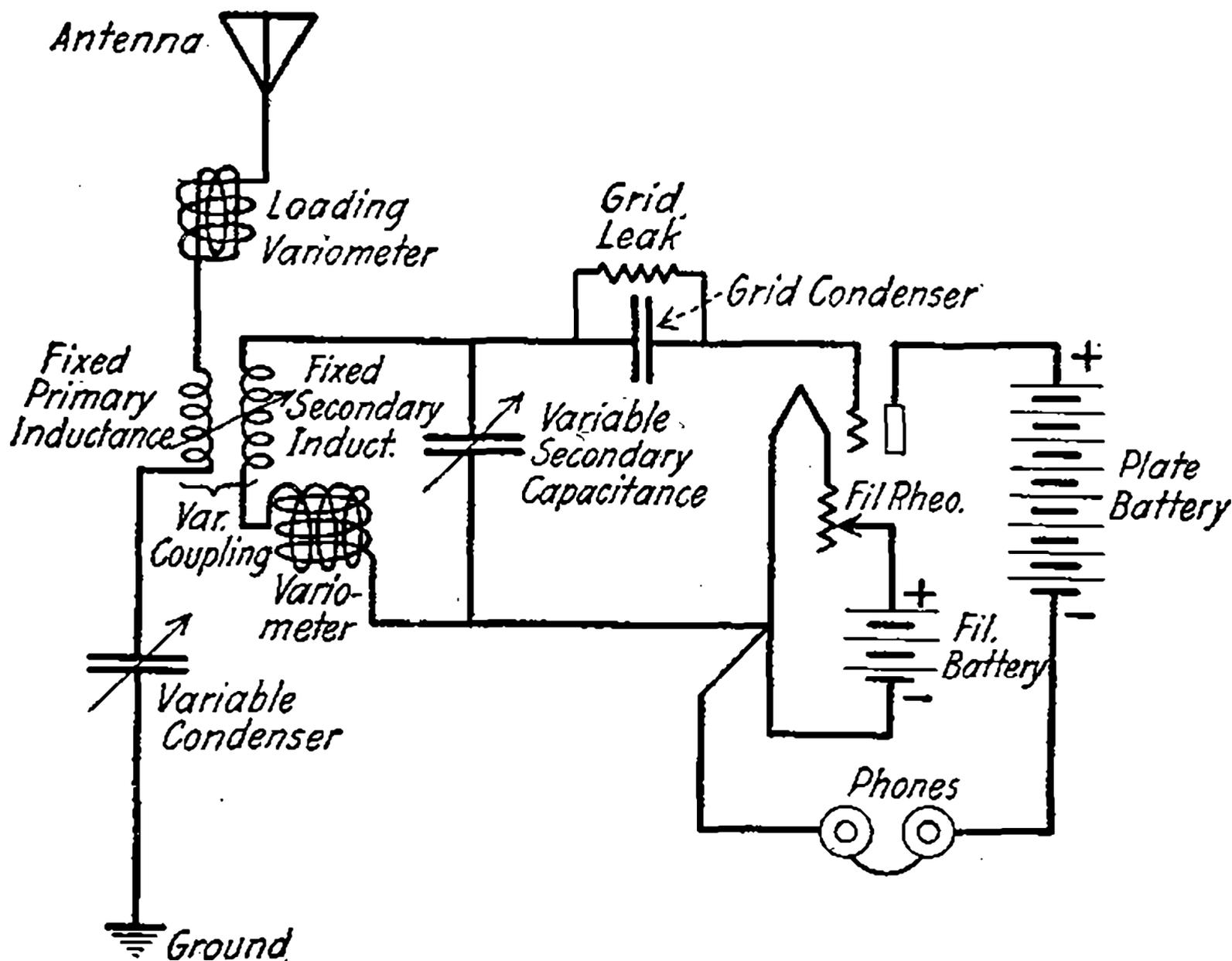
Fig. 39—Two Circuit Receiver, Inductive Coupling.
