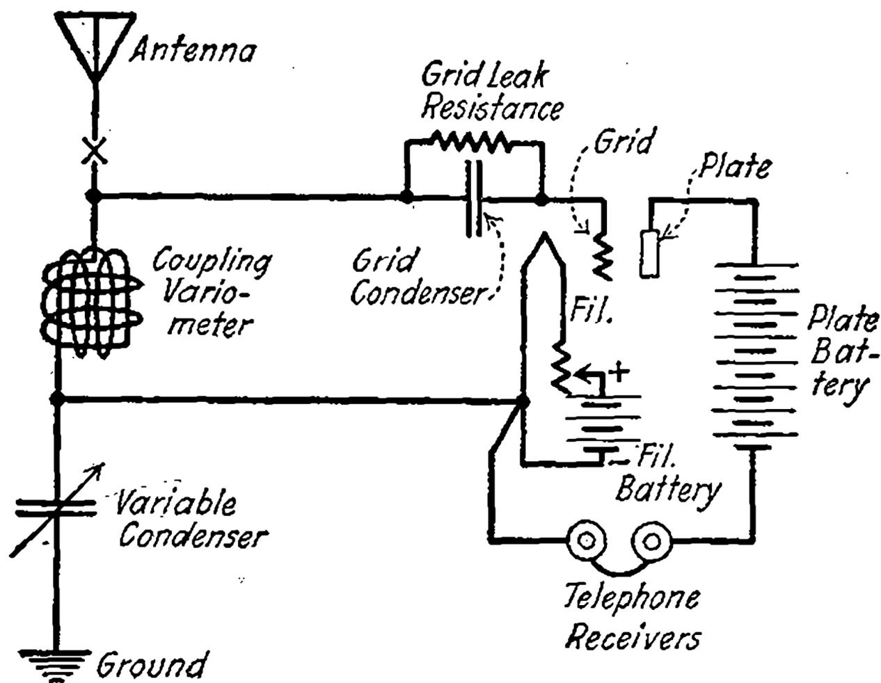
Fig. 37—Simple Single Circuit Receiver.
