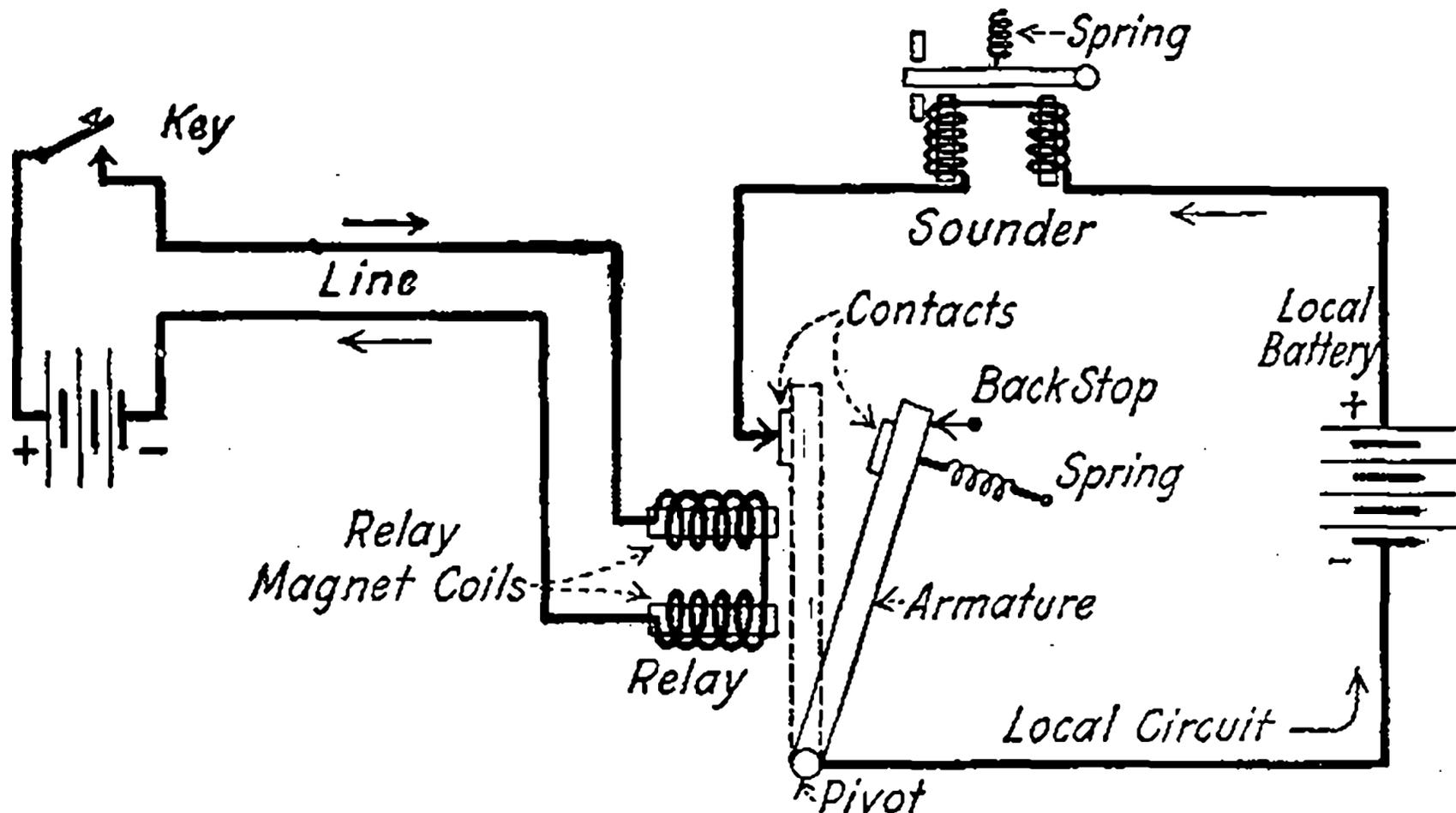
Fig. 17—Circuits of telegraph relay.
