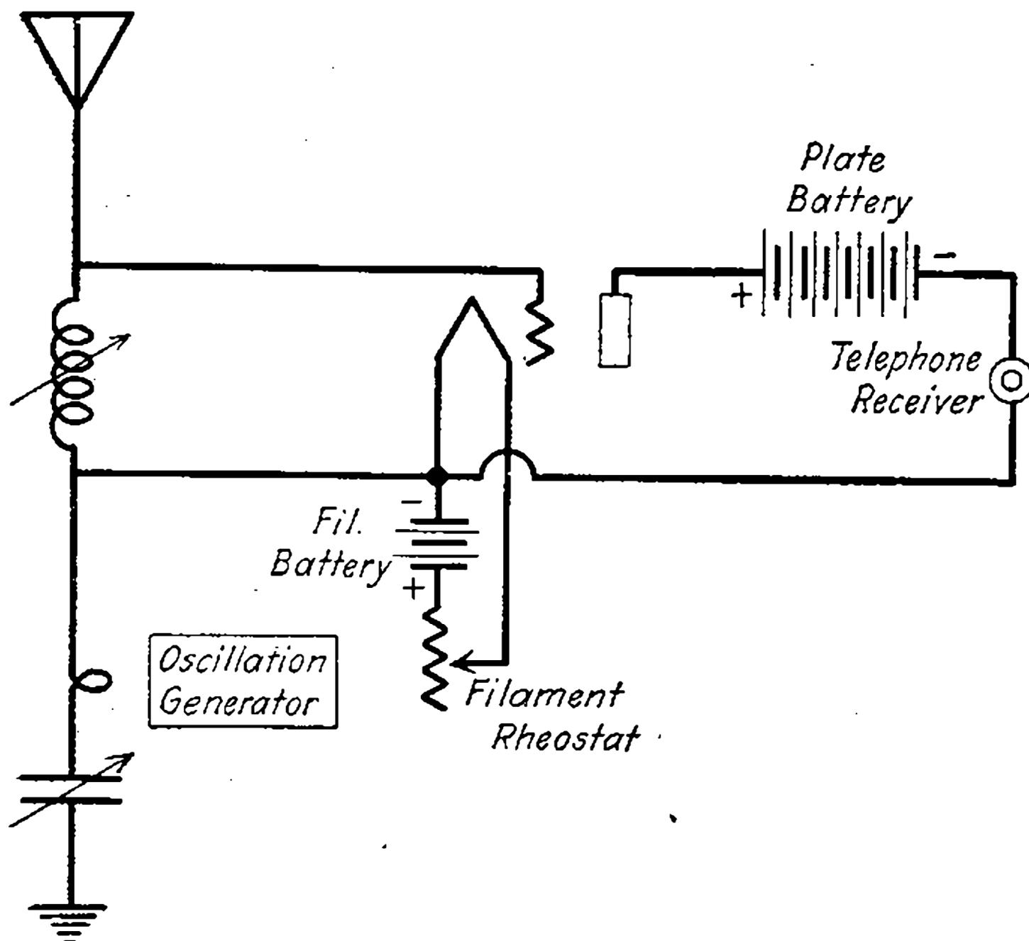
Fig. 28—Schematic circuit for the production of beats.
