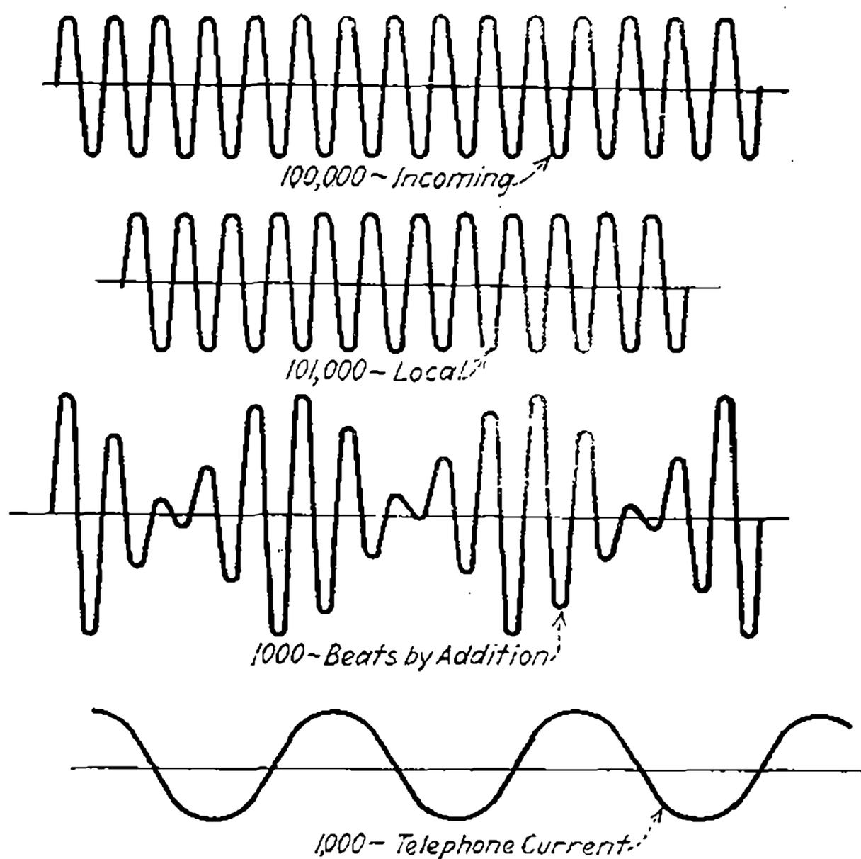
Fig. 27—The principle of heterodyne action.
