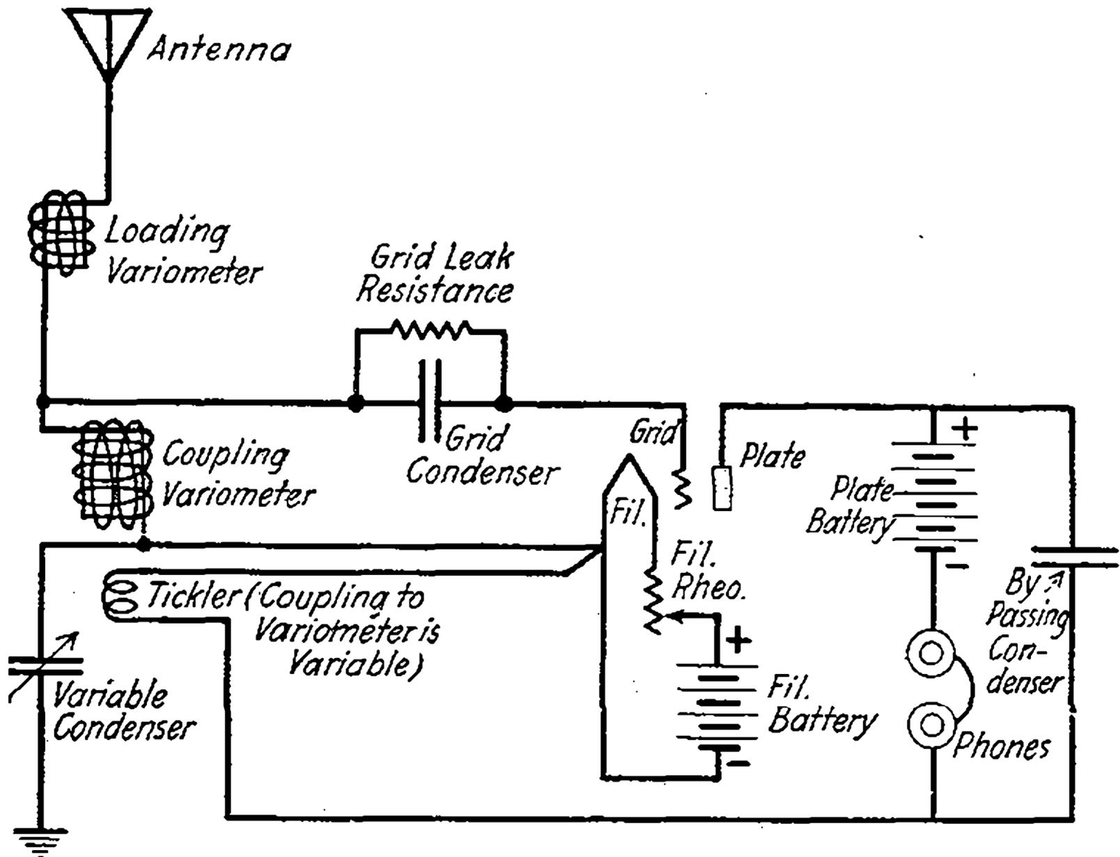
Fig. 38—Single Circuit Regenerative Receiver.
