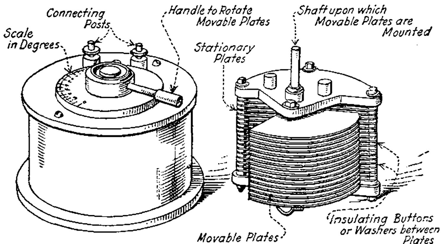
Fig. 7—Typical variable condenser with air dielectric.
