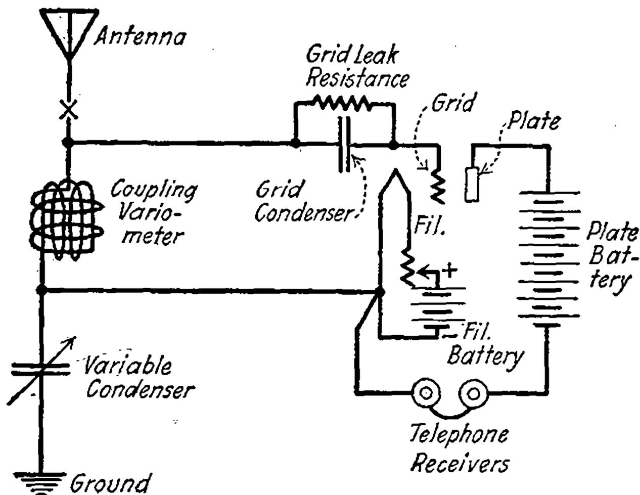
Fig. 37—Simple Single Circuit Receiver.
