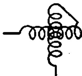
Fixed Coupling of Coils (Fixed Inductive Coupling) -----
