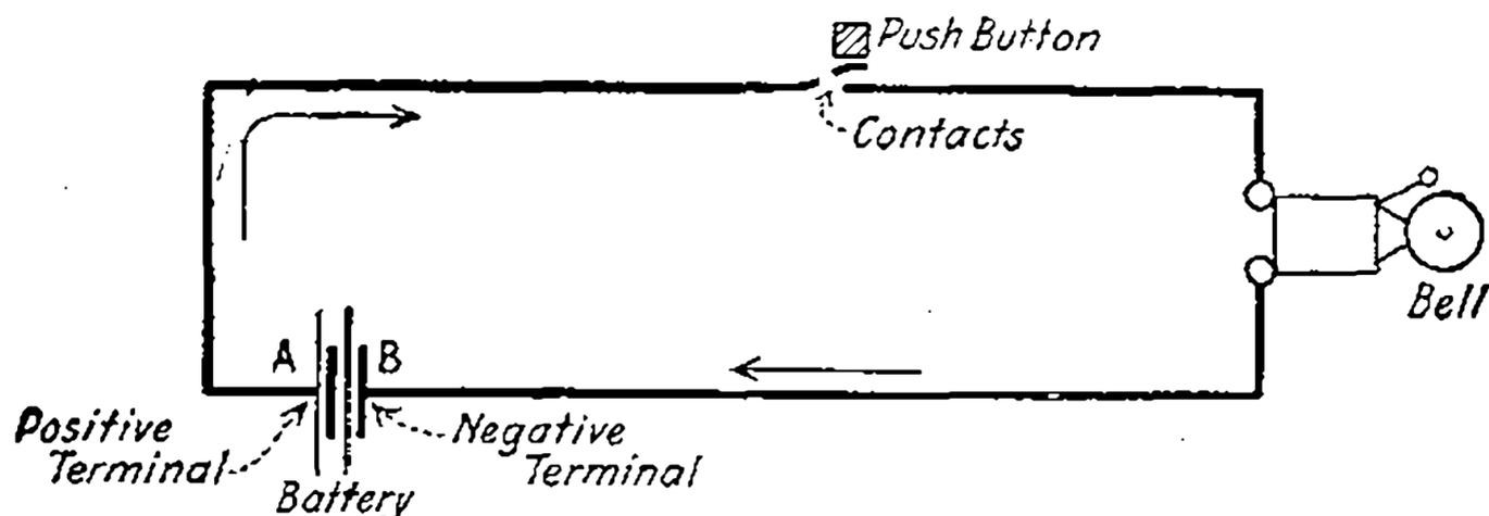
Fig. 1—Simple electrical path or circuit.
