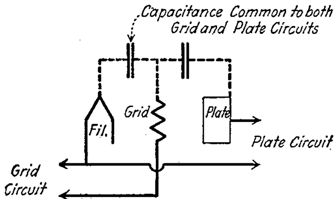
Fig. 36—Inter-electrode tube capacitance.
