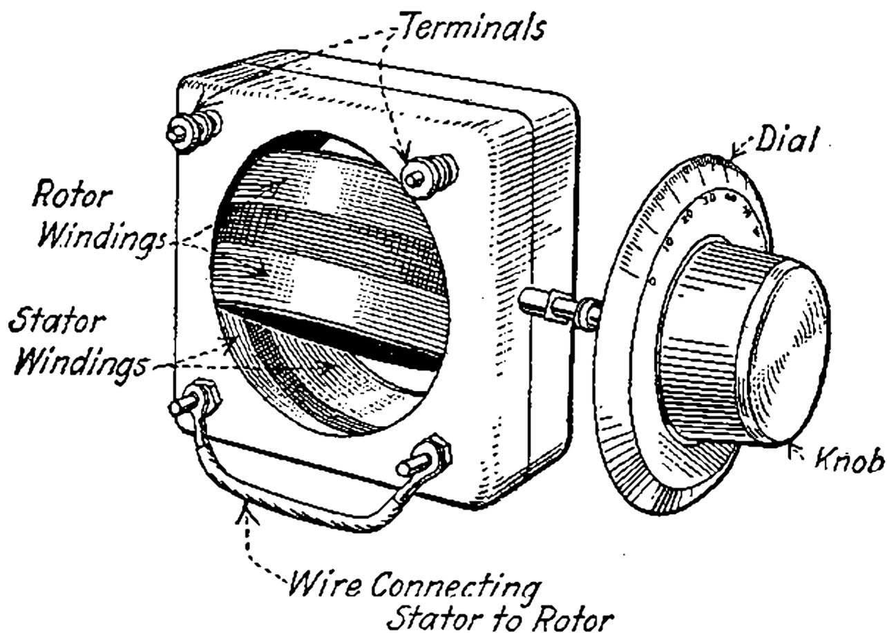
Fig. 35—Construction of a typical variometer.
