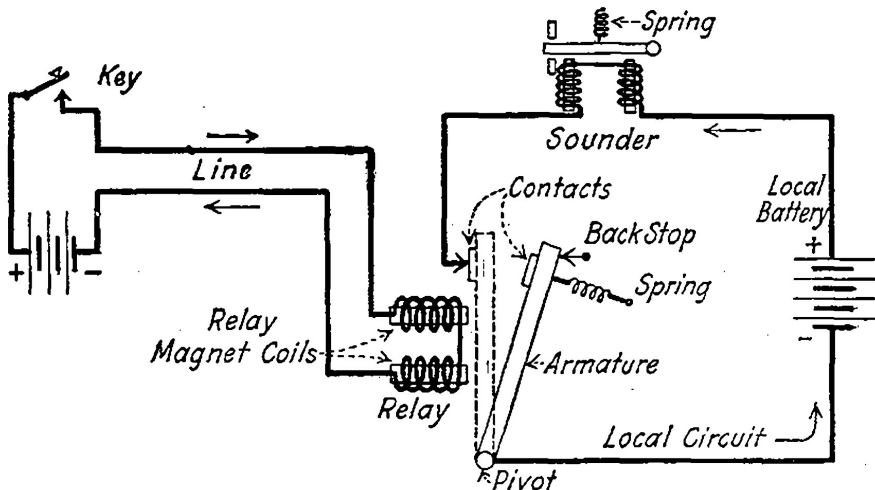
Fig. 17—Circuits of telegraph relay.
