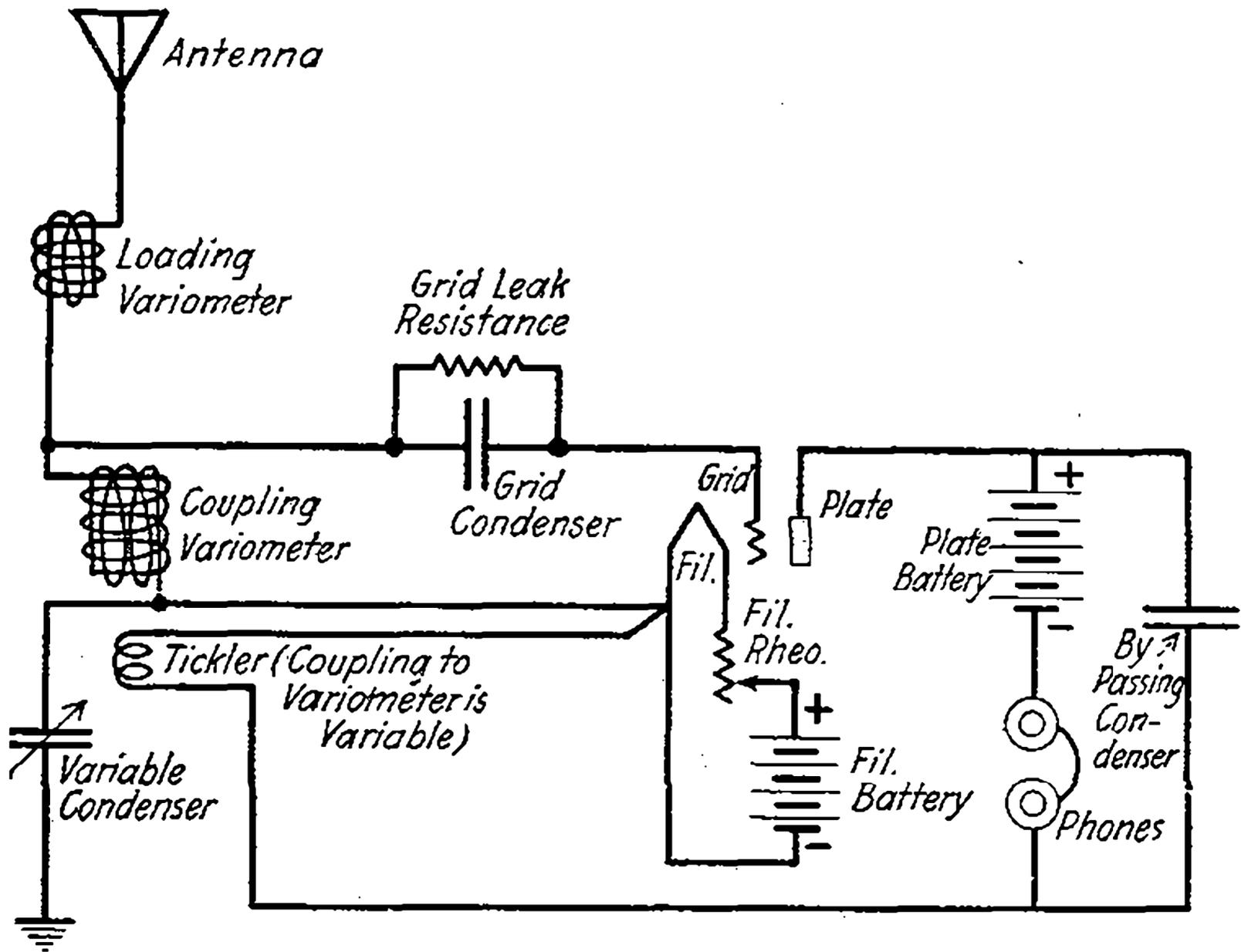
Fig. 38—Single Circuit Regenerative Receiver.
