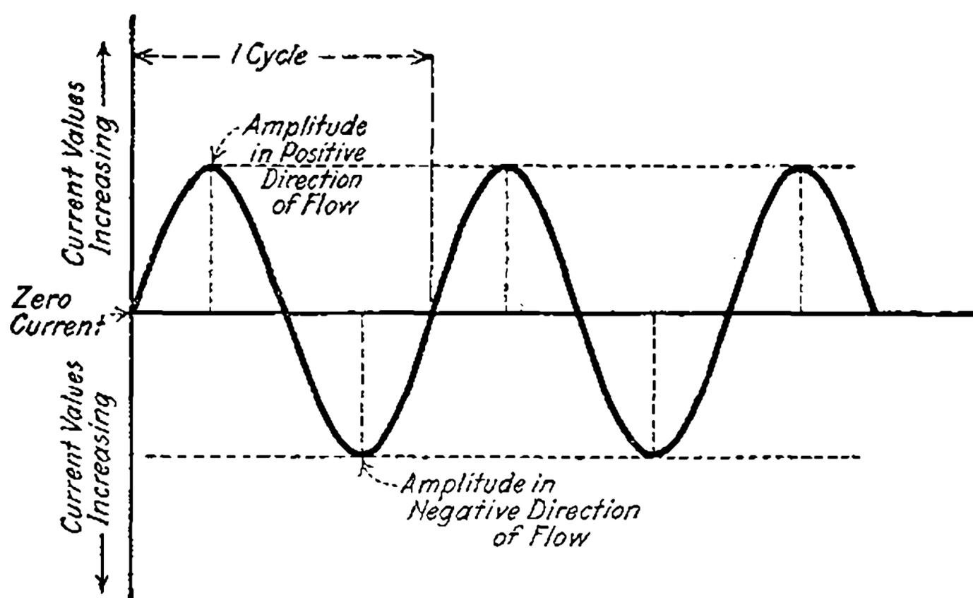
Fig. 9—Continuous oscillations.
