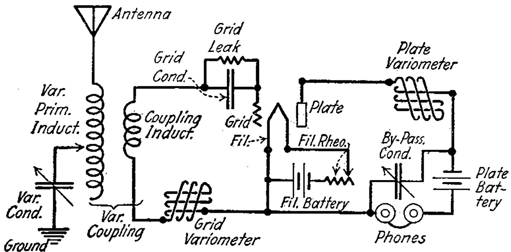
Fig. 41—Three Circuit Regenerative Receiver for Short Waves.
