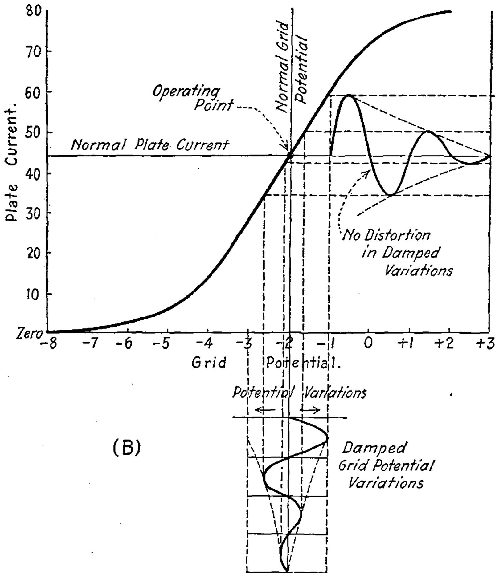
Fig. 29 (b)—Amplification of damped oscillations.
