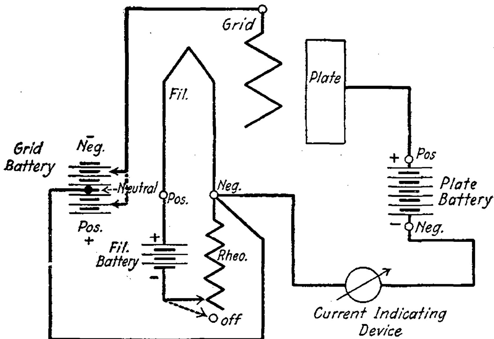
Fig. 15—One method of varying the grid potential.
