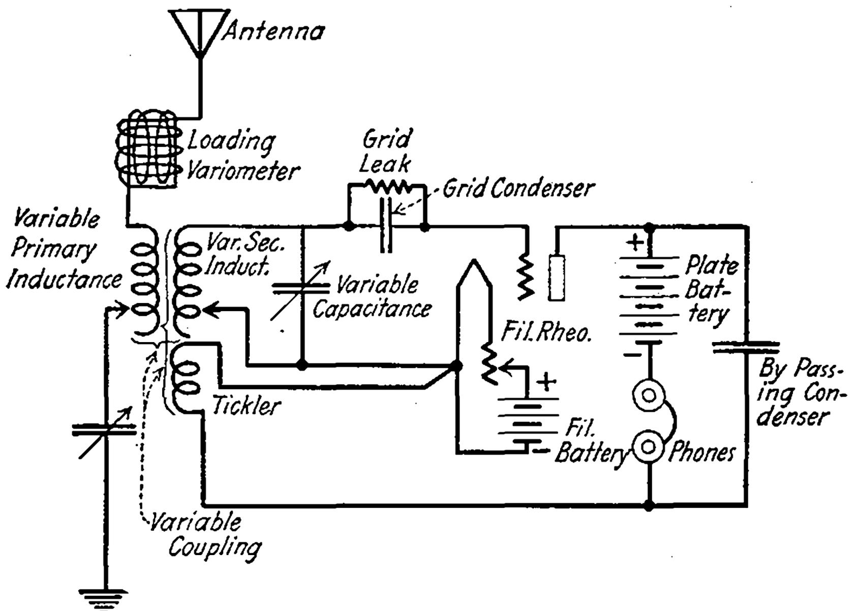
Fig. 40—Two Circuit Regenerative Receiver, Inductive Coupling.
