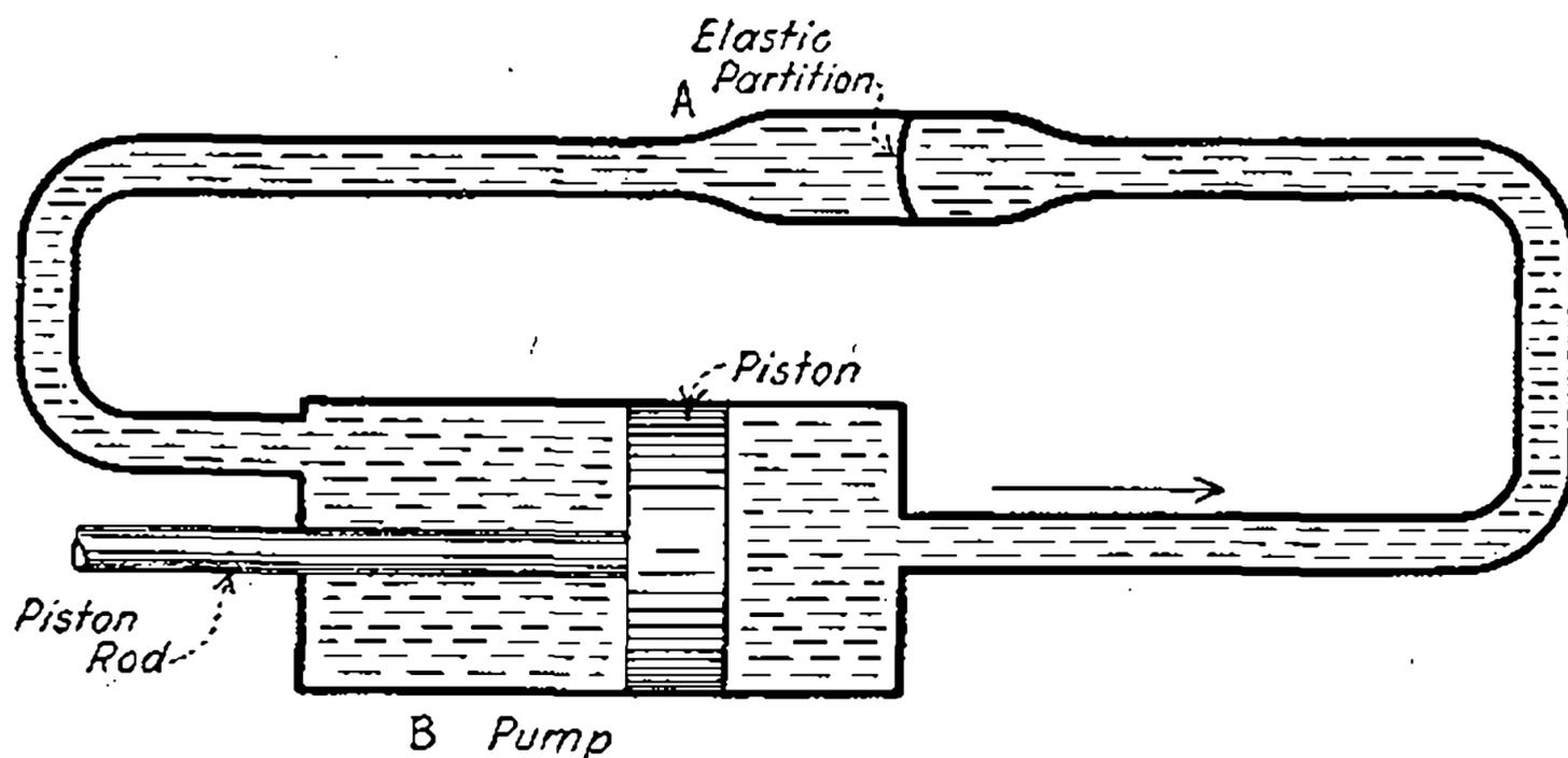
Fig. 8—Water analogy of alternating current in a circuit containing a condenser.
