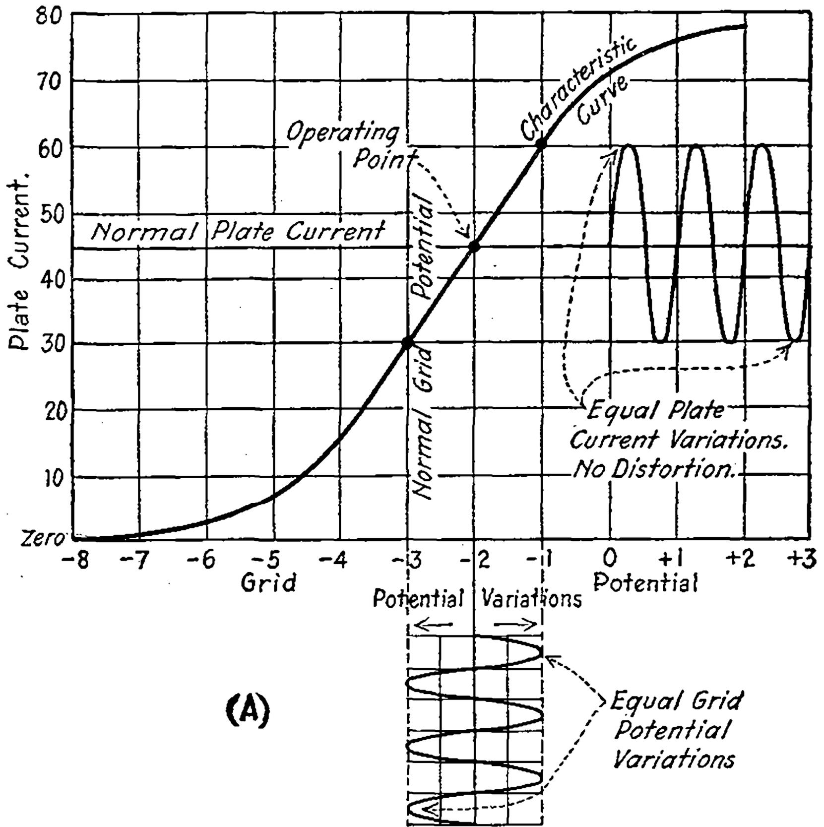
Fig. 29 (a)—Amplification of continuous oscillations.
