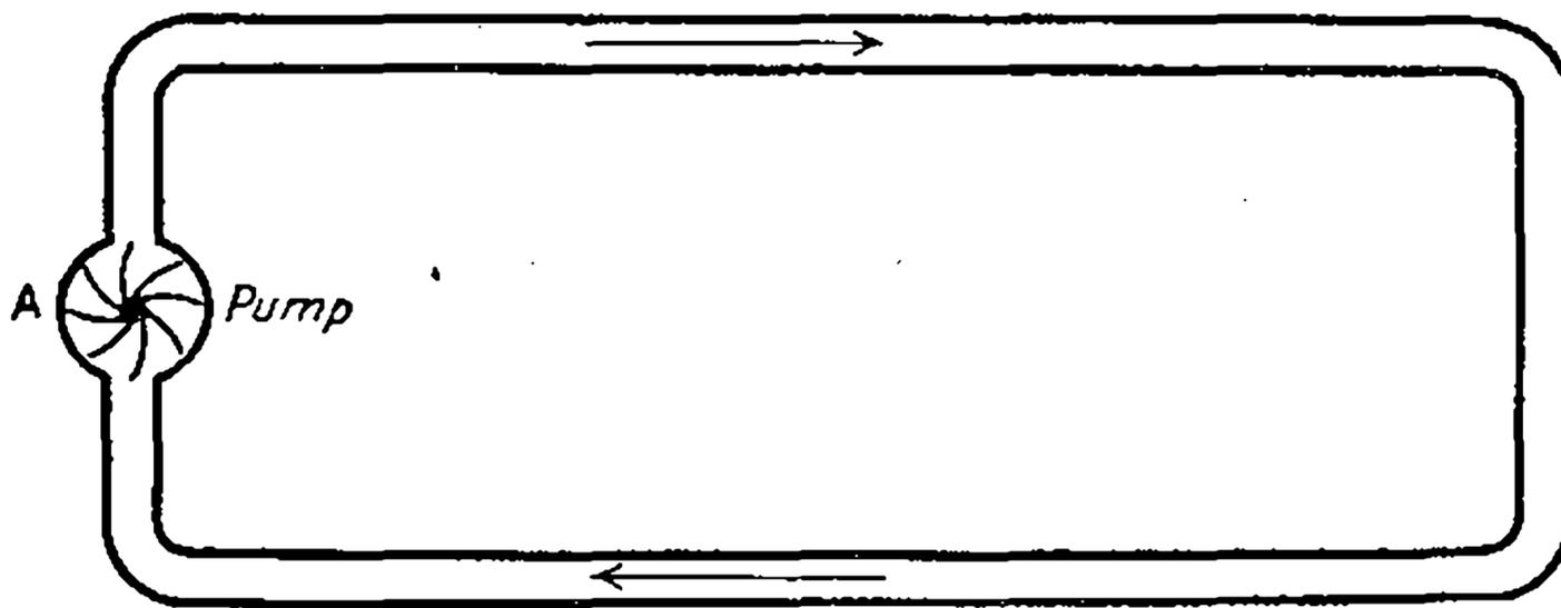
Fig. 2—Water analogy of simple electrical circuit.
