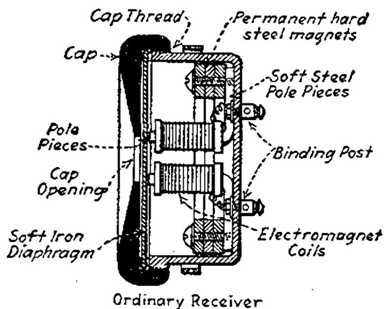
Fig. 21—Construction of a typical telephone receiver.
