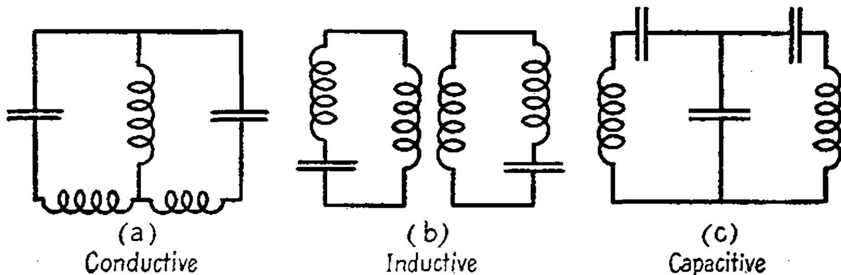
Fig. 34—Methods of coupling.
