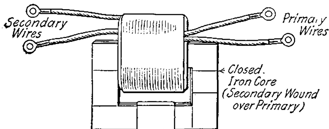
Fig. 44—Typical audio-frequency coupling transformer.
