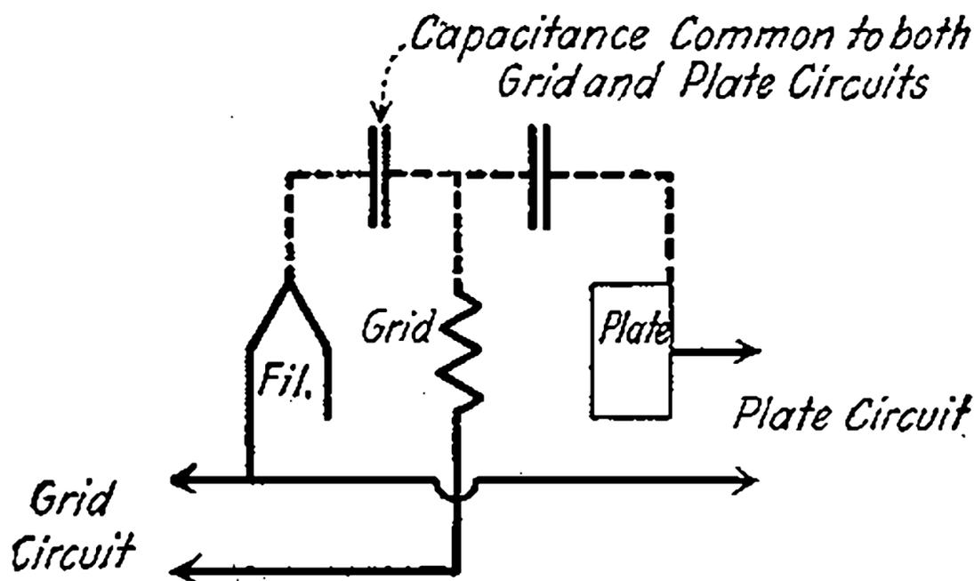
Fig. 36—Inter-electrode tube capacitance.
