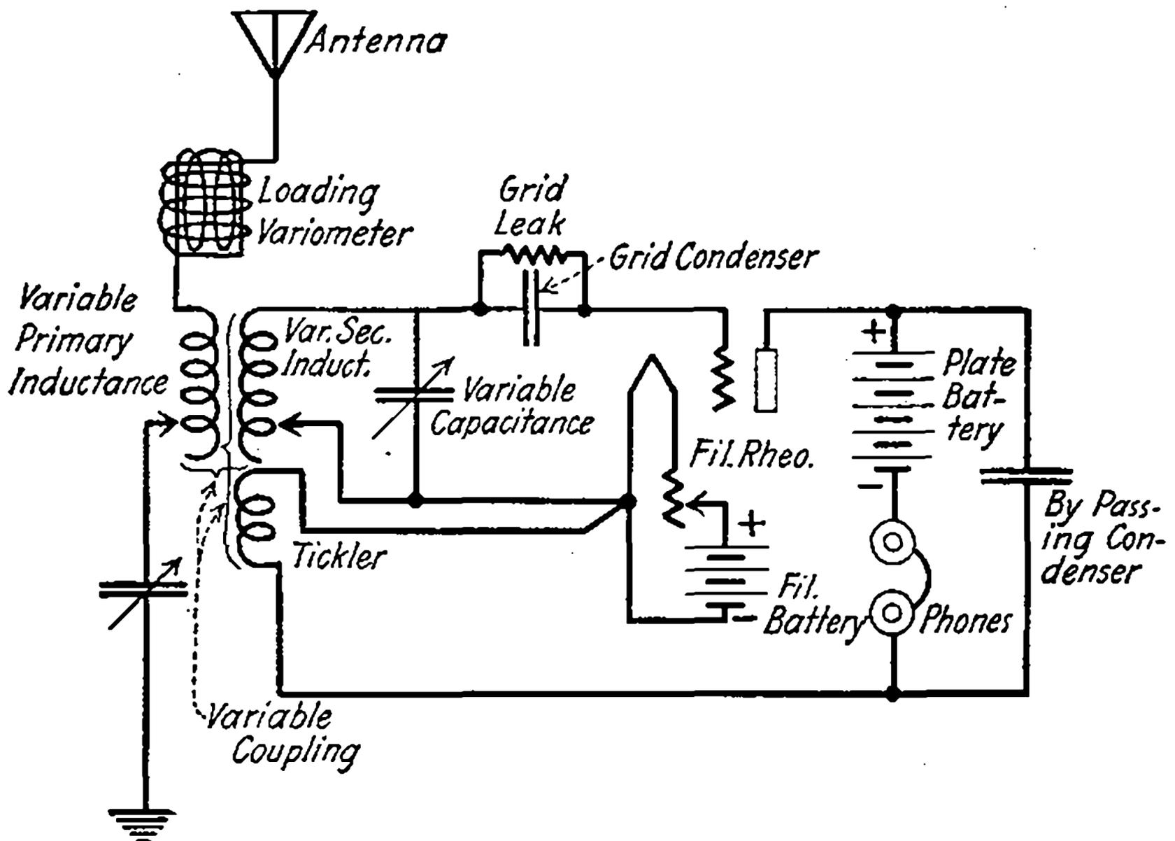
Fig. 40—Two Circuit Regenerative Receiver, Inductive Coupling.
