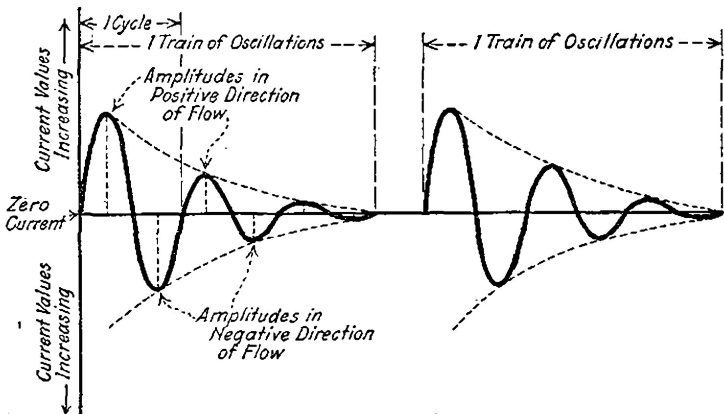
Fig. 10—Damped oscillations.
