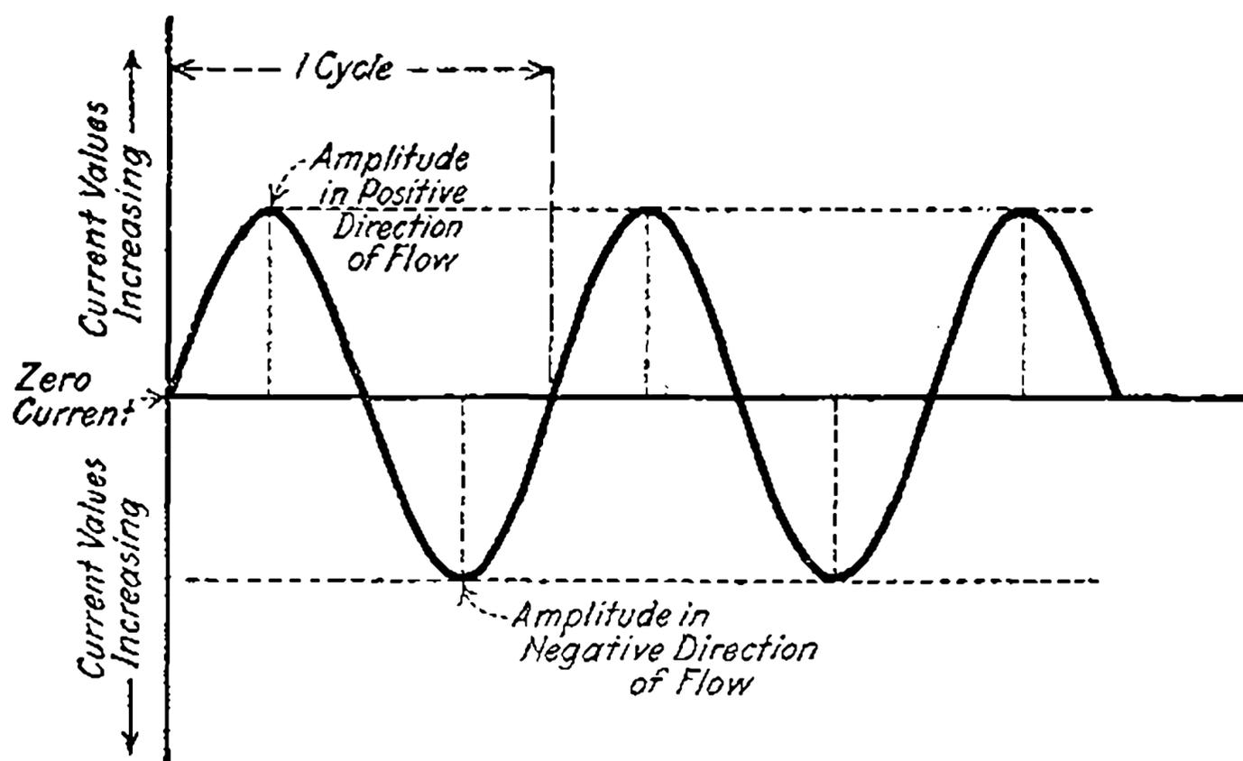
Fig. 9—Continuous oscillations.
