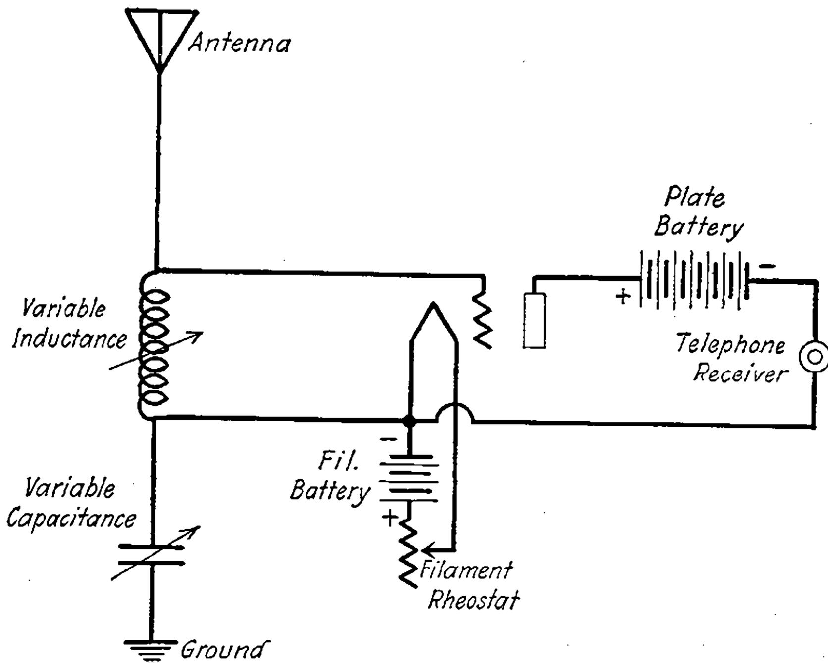
Fig. 22—Simple detector circuit.
