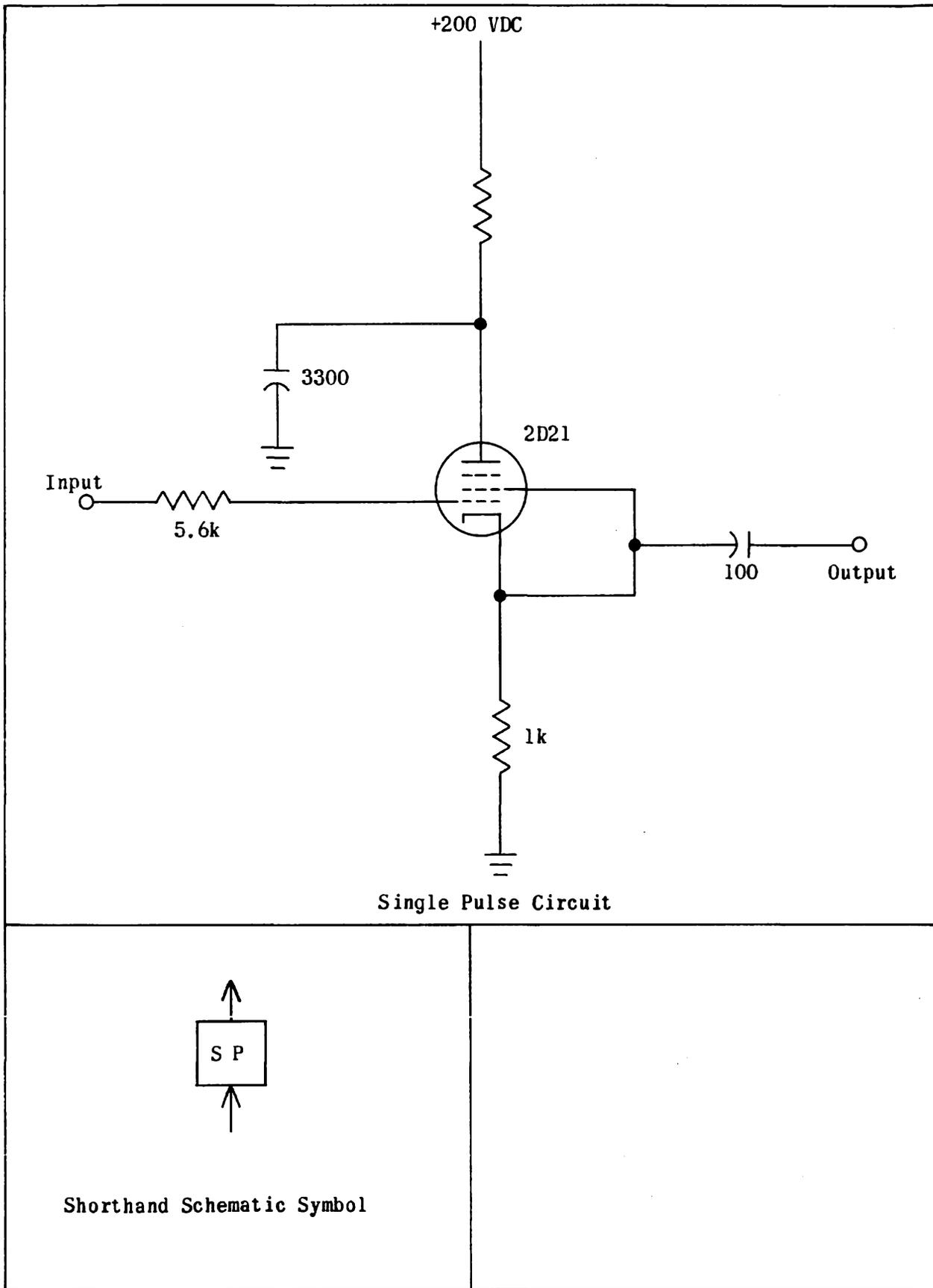
Figure 10. STANDARD Single Pulse Circuit
