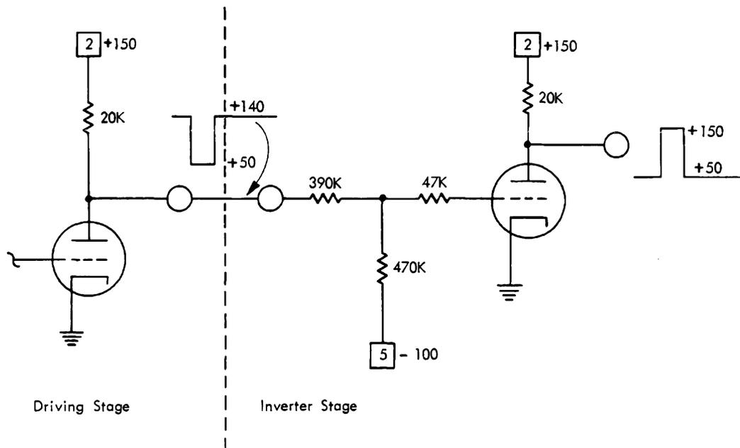
Figure 23. A Practical Inverter Circuit
