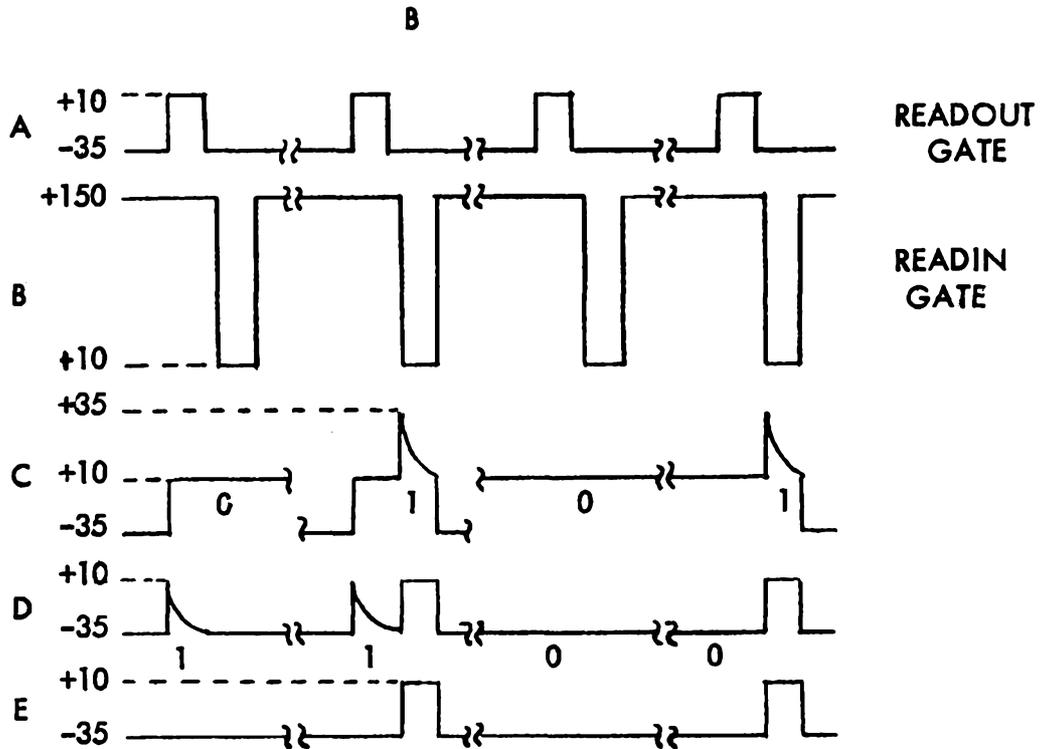
Fig. 28 - Capacitor storage
