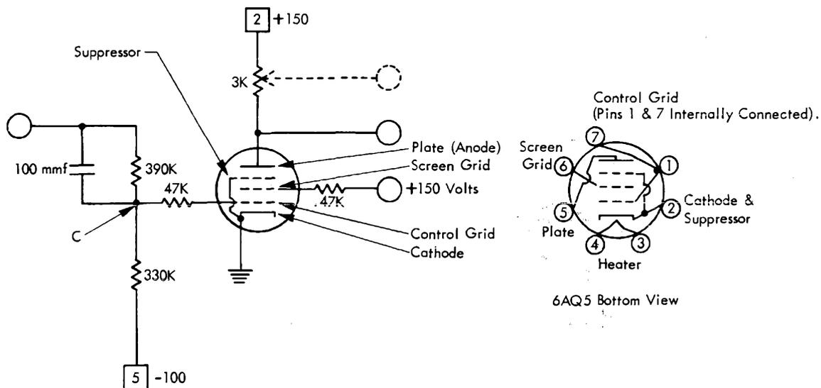
Figure 41. A Power Unit Using a 6AQ5
