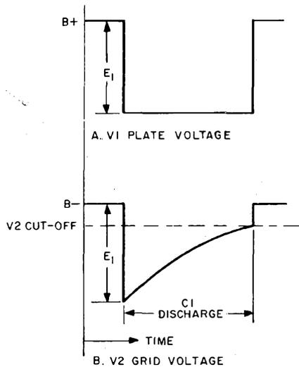
$E_1 = I_1 \times R_1 =$  VOLTAGE FALL AT PLATE OF V1 WHEN V1 CONDUCTS
