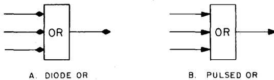
Figure 3-28. Diode OR Circuit, Logic Block Symbols
