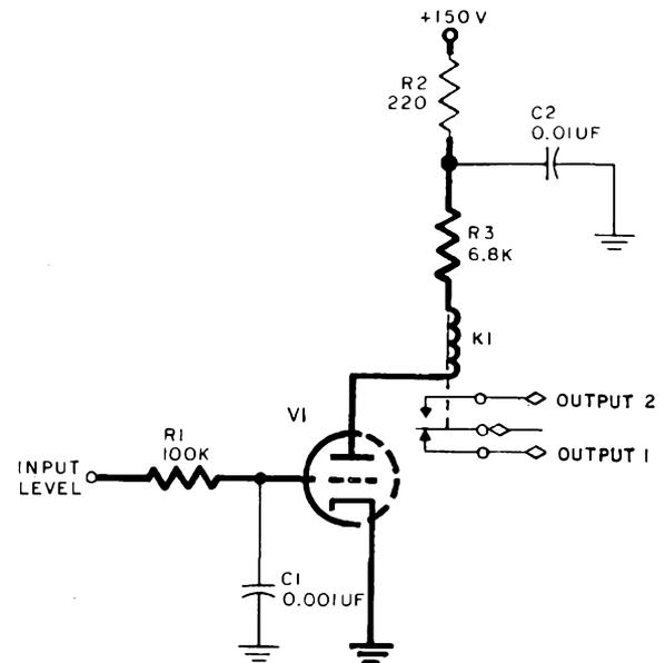
Figure 3-19. Vacuum-Tube Relay Driver, Model B, Schematic Diagram
