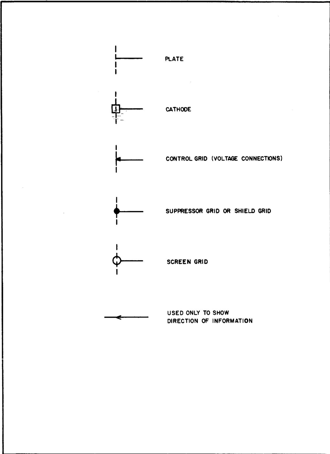
Figure 2. Tube Element Connections.
