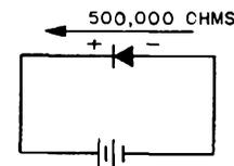
Figure 3-24. Backward Resistance of Crystal Diode, Schematic Diagram
