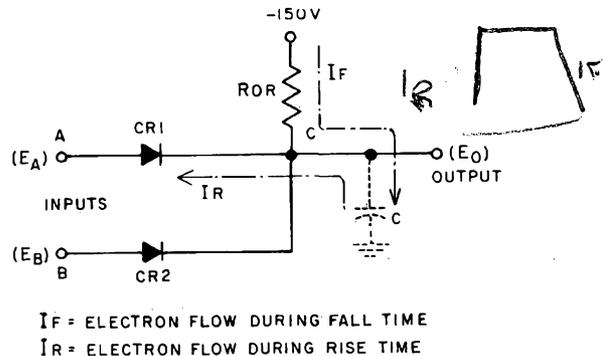
load capacitance gives the circuit a slow rise time. Figure 3-31 shows a pulsed OR circuit. In order for this circuit to function with pulse inputs, the fall time must be speeded up. This is accomplished by replacing resistor  $R_{OR}$  with an inductor,  $L$ . Resistor  $R_L$  is used to prevent oscillation between  $L$  and  $C$  (stray capacitance). Resistor  $R_L$  is of low ohmic value.
