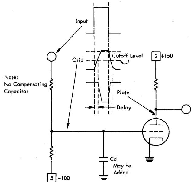
Figure 35. Signal Delay
