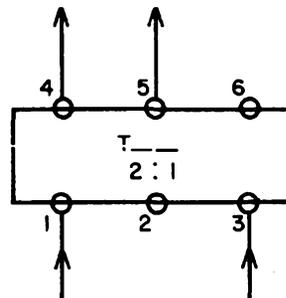
SYMBOL SERIES NUMBERS T01 THROUGH T99 ARE ASSIGNED TO THE PULSE TRANSFORMERS. TURNS RATIOS USED ARE PRINTED BELOW THE SYMBOL SERIES NUMBERS. (TYPE 130AI IS INTERCHANGEABLE WITH TYPE 130A2. TYPE 131AI IS INTERCHANGEABLE WITH TYPE 131A2.)
