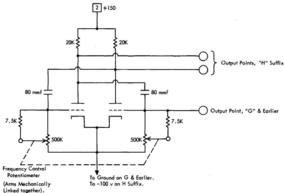
Figure 67. 604 Multivibrator Circuit
