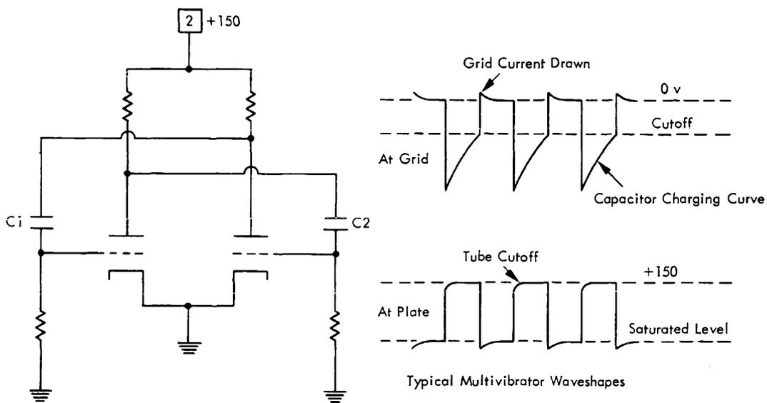
Figure 66. The Basic Multivibrator and Typical Waveshapes
