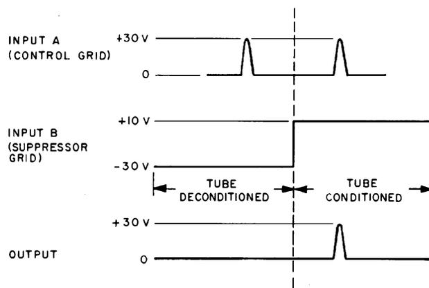
Figure 3-35. Gate Tube, Model A,
