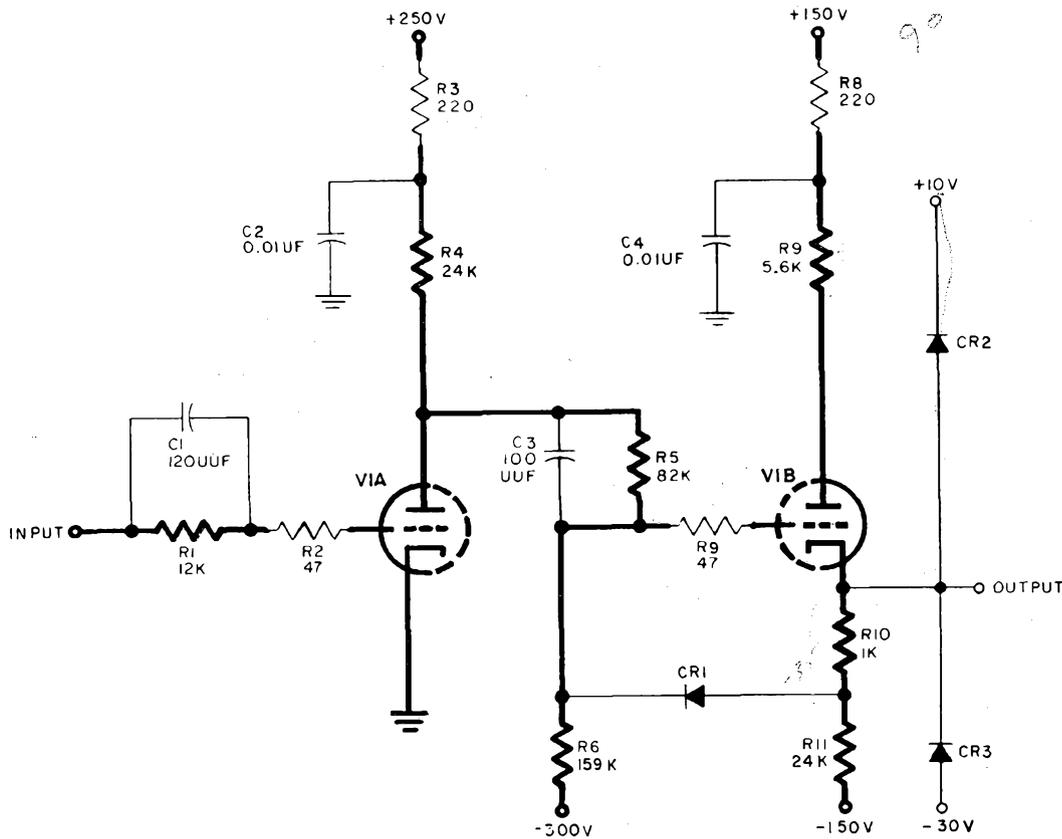
Figure 3-38. D-C Inverter, Model A, Schematic Diagram
