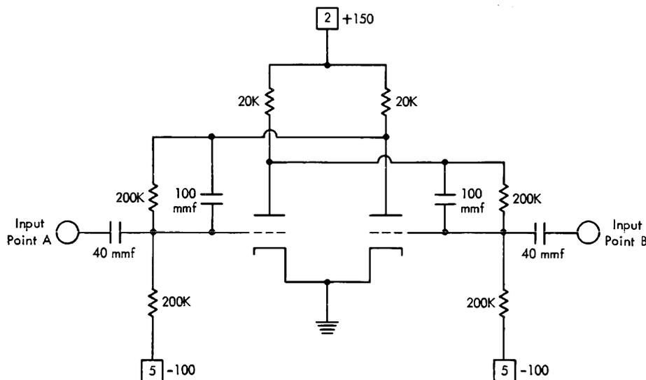
NOTE: Capacitive input triggers in the 604 respond only to negative shifts.
