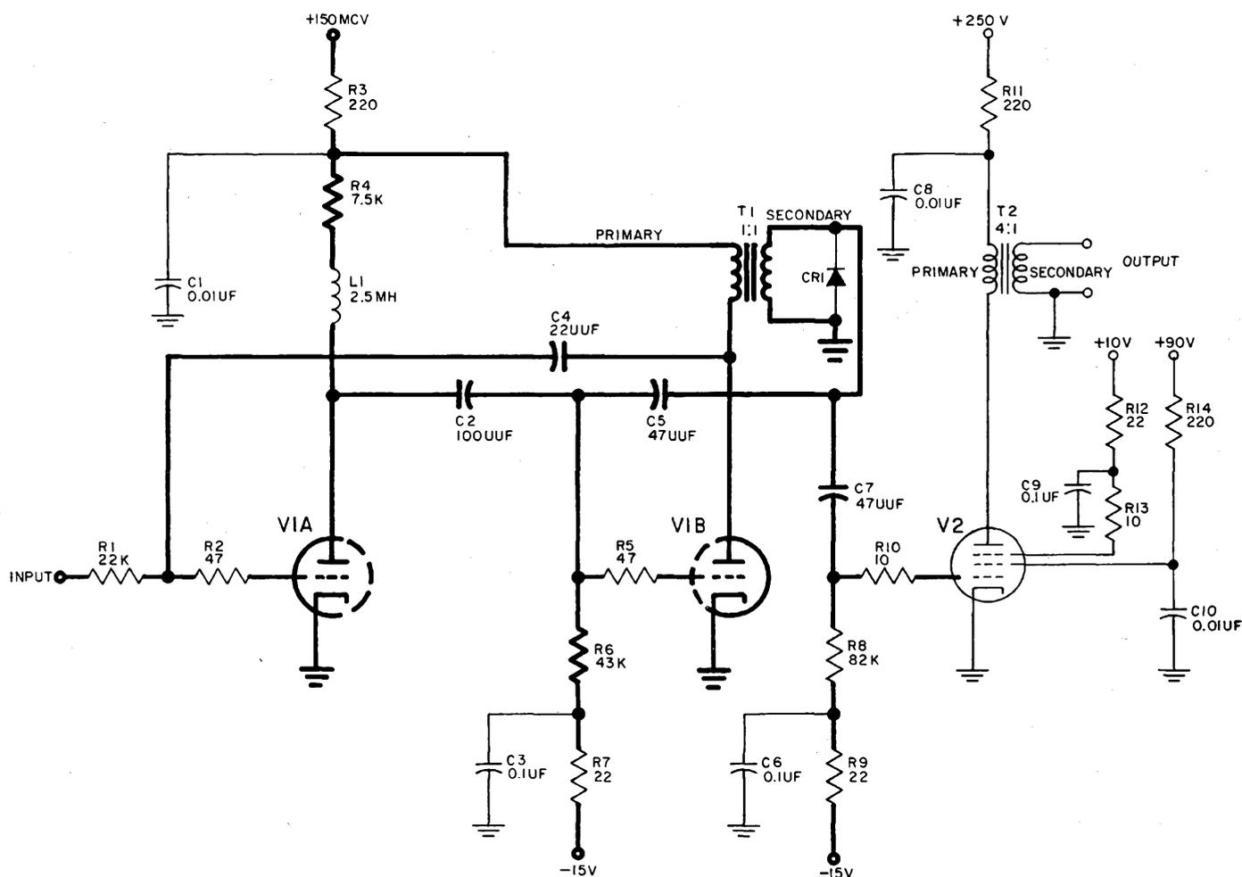
Figure 3-56. Pulse Generator, Model E, Schematic Diagram
