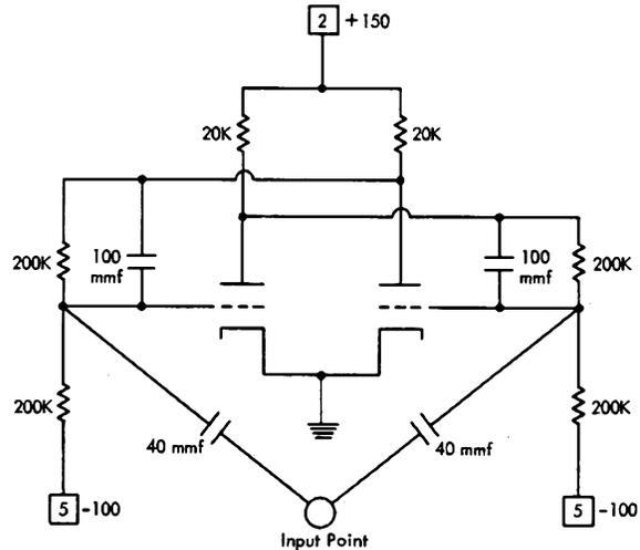
Figure 64. A Binary. Commoned Input Trigger
