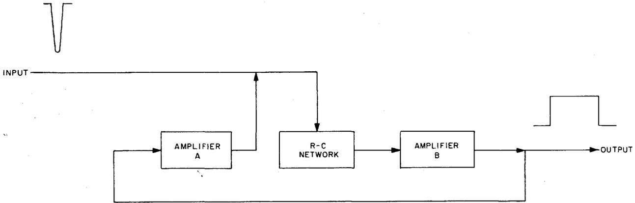
Figure 3-46. Single-Shot, Simplified Block Diagram
