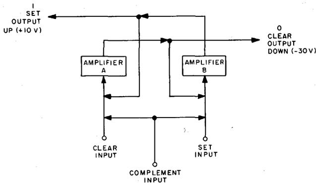
Figure 3-39. Flip-Flop, Block Diagram
