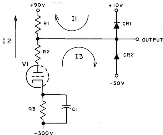
Figure 2-13. Diode Clamped Output Levels, Simplified Schematic Diagram
