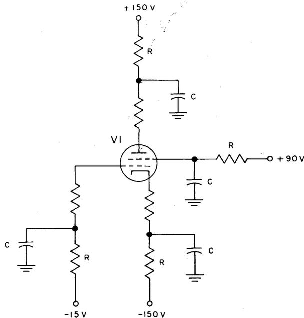
Figure 2-10. RC Decoupled Returns, Simplified Schematic Diagram
