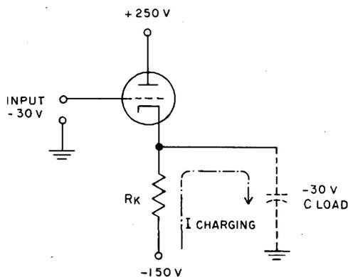
Figure 3-4. Cathode Follower with Capacitive Load, Simplified Schematic Diagram
