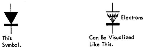
Figure 53. Derivation of the Symbol for Solid State Diodes
