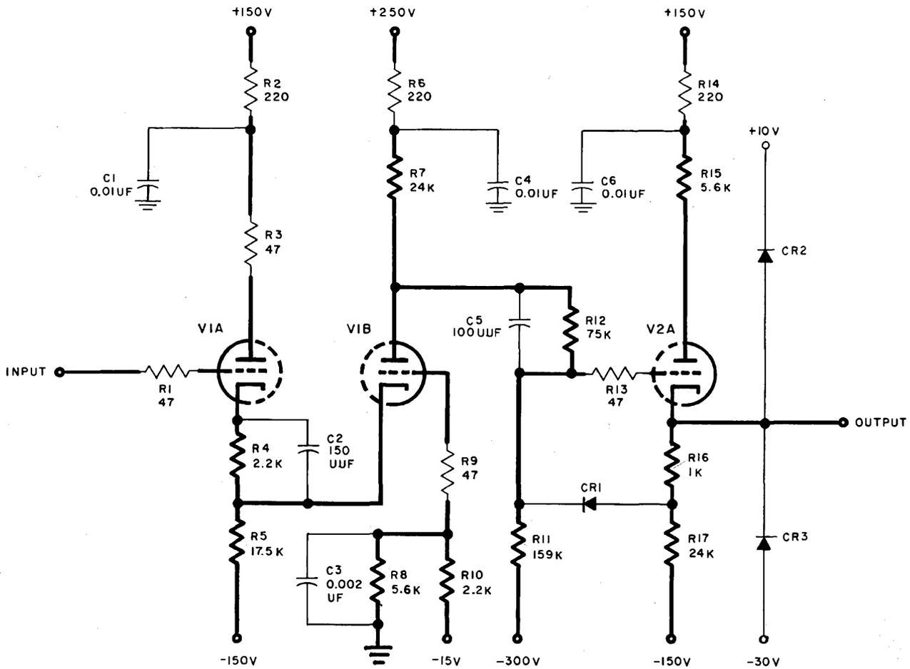
Figure 3-11. D-C Level Setter, Model B, Schematic Diagram
