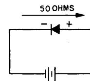
Figure 3-23. Forward Resistance of Crystal Diode, Schematic Diagram
