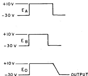
Figure 3-30. Effect of Load Capacitance in OR Circuit
