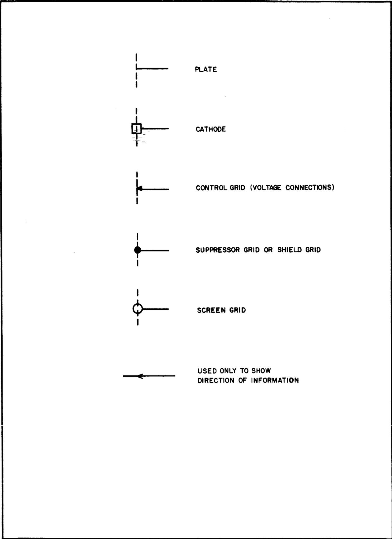
Figure 2. Tube Element Connections.
