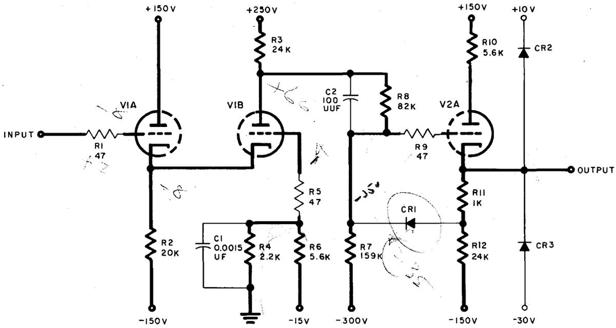
Figure 3-10. D-C Level Setter, Model A, Schematic Diagram
