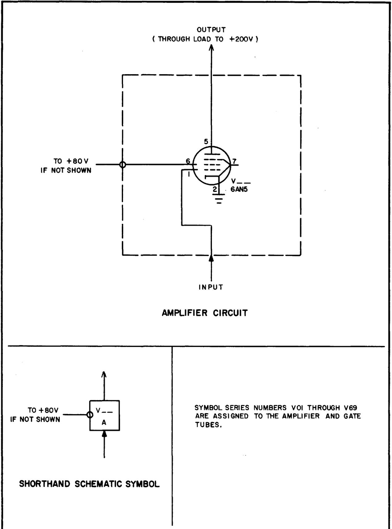
Figure 7. STANDARD Amplifier Stage
