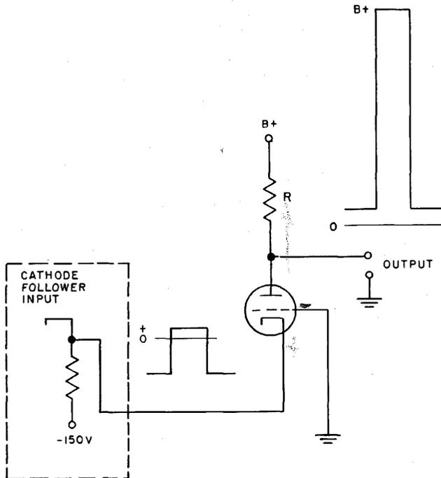
Figure 3-9. Grounded Grid Amplifier, Simplified Schematic Diagram
