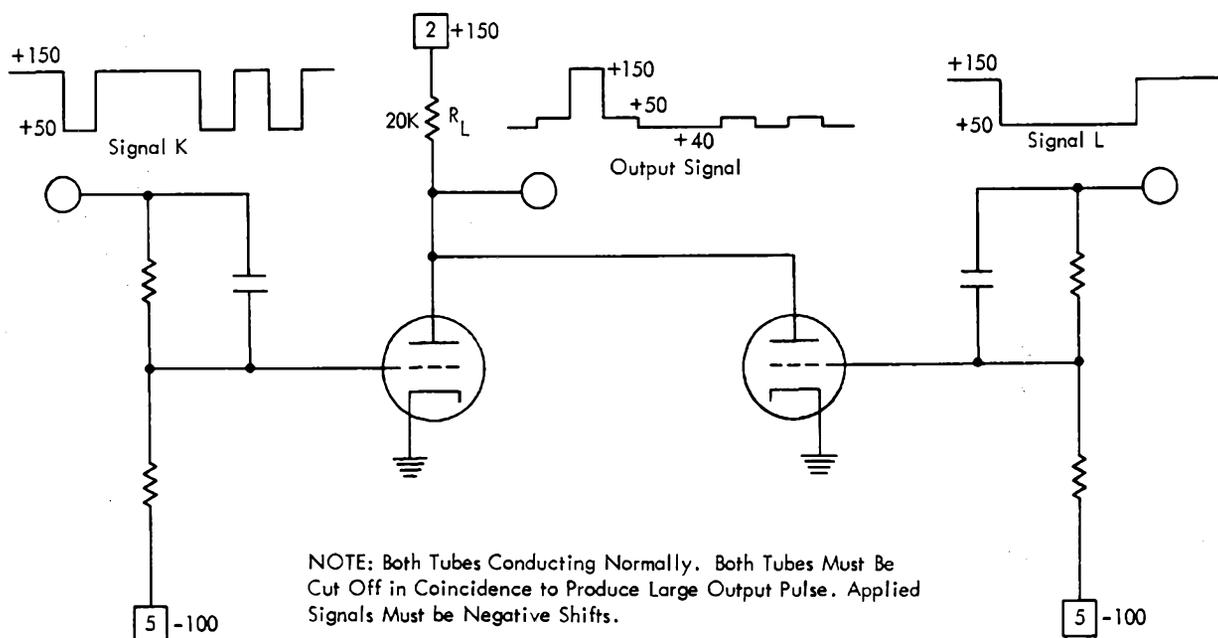
Figure 39. The Inverter AND Circuit (Switch)
