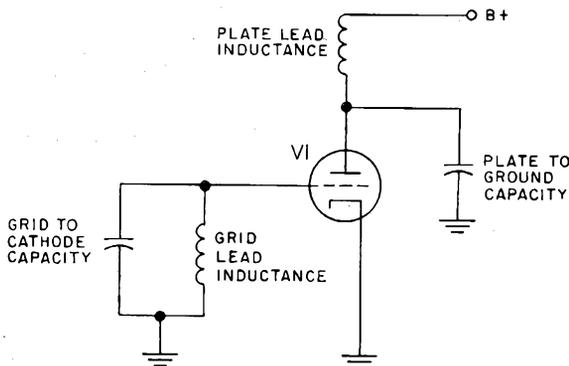
Figure 2-7. Lumped Constants, Equivalent Circuit, Simplified Schematic Diagram
