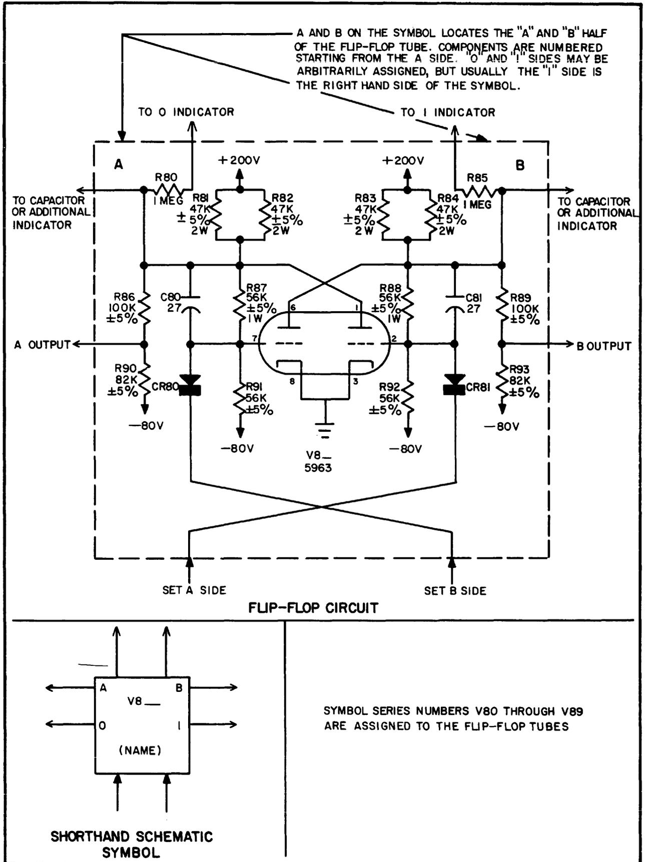
Figure 3. STANDARD Flip-flop Stage
