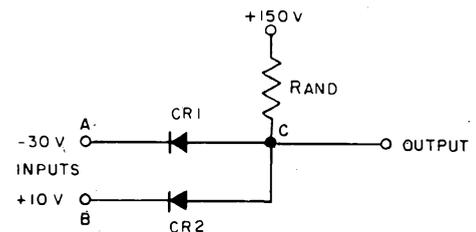
Figure 3-25. Two-way AND Circuit, Simplified Circuit Diagram
