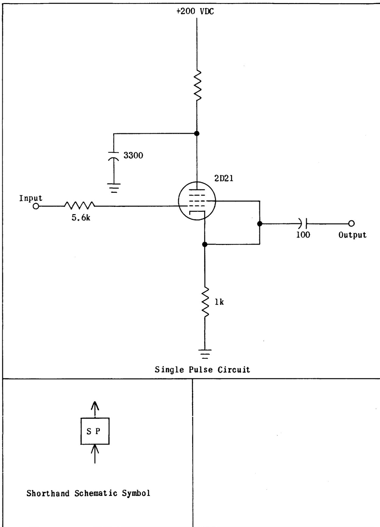
Figure 10. STANDARD Single Pulse Circuit
