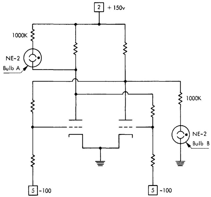
Figure 69. Neon Indicator Bulb Circuits for Triggers
