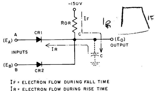
Figure 3-30. Effect of Load Capacitance in OR Circuit
