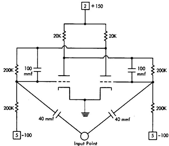
Figure 64. A Binary. Commoned Input Trigger
