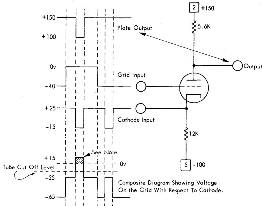
Note: Portion shown shaded (where grid goes plus with respect to cathode) will, if cathode is hot, be swamped due to grid current flow.
