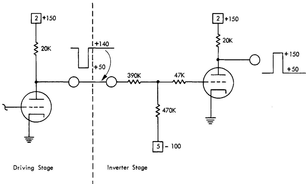
Figure 23. A Practical Inverter Circuit
