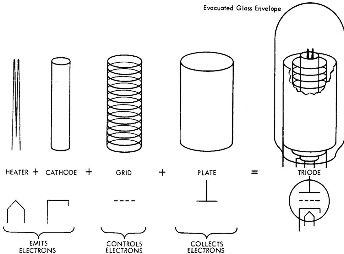
Figure 20. Development of the Triode Tube
