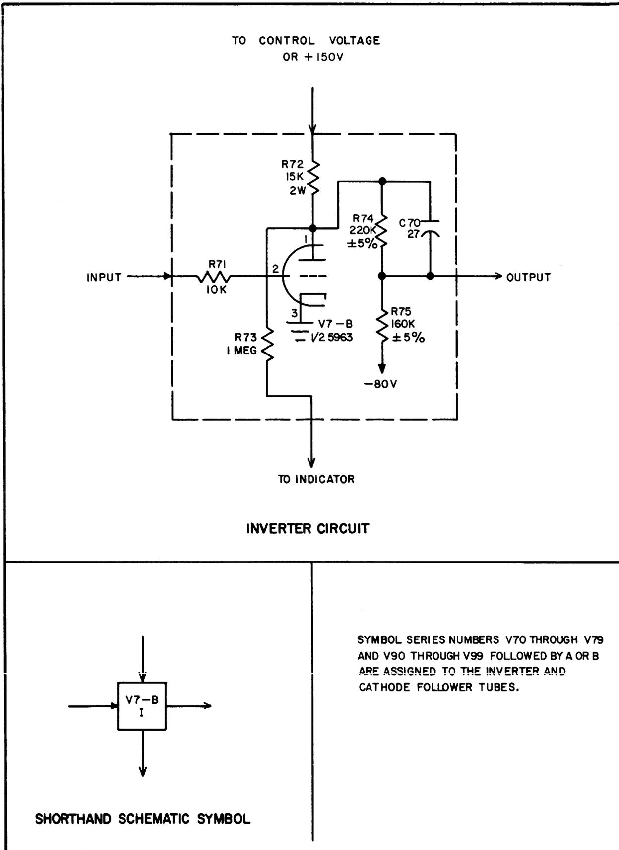
Figure 5. STANDARD Inverter Stage
