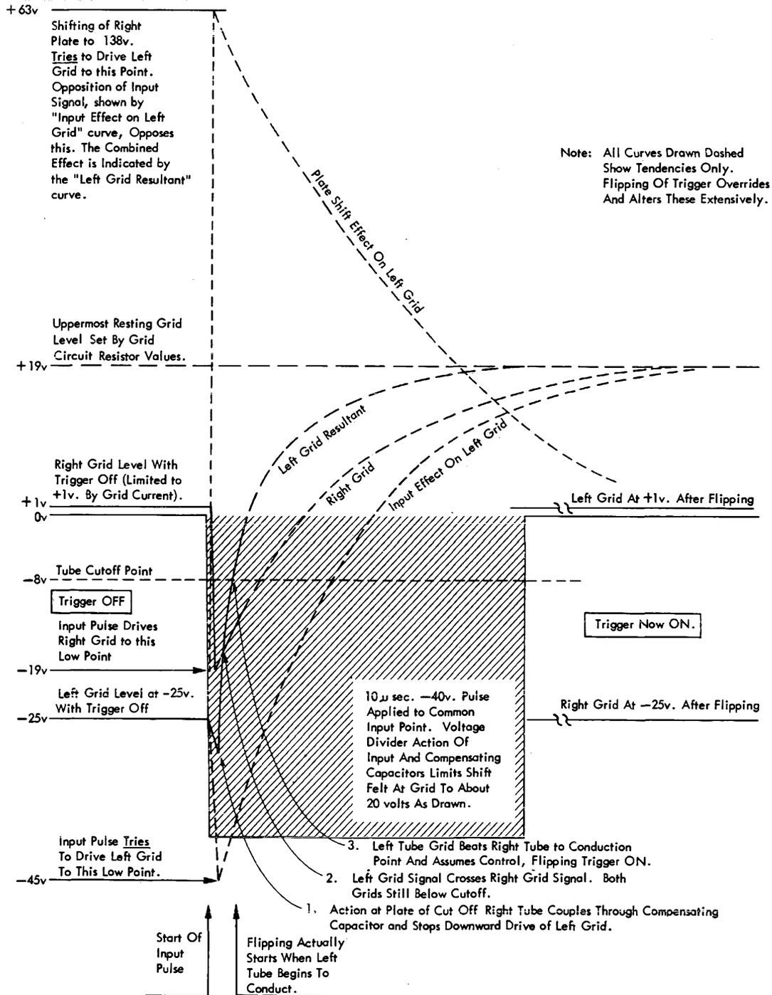
Figure 65a. Waveforms of Binary Trigger Action With Compensating Capacitors
