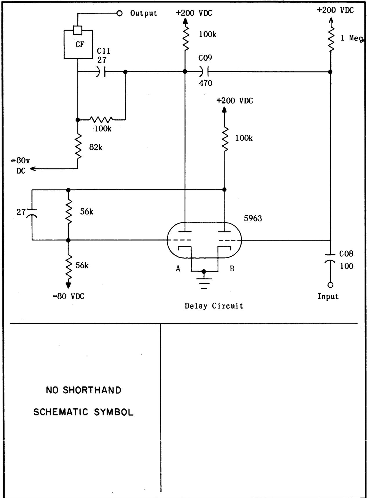
Figure 11. STANDARD Delay Circuit (Vacuum Tube)
