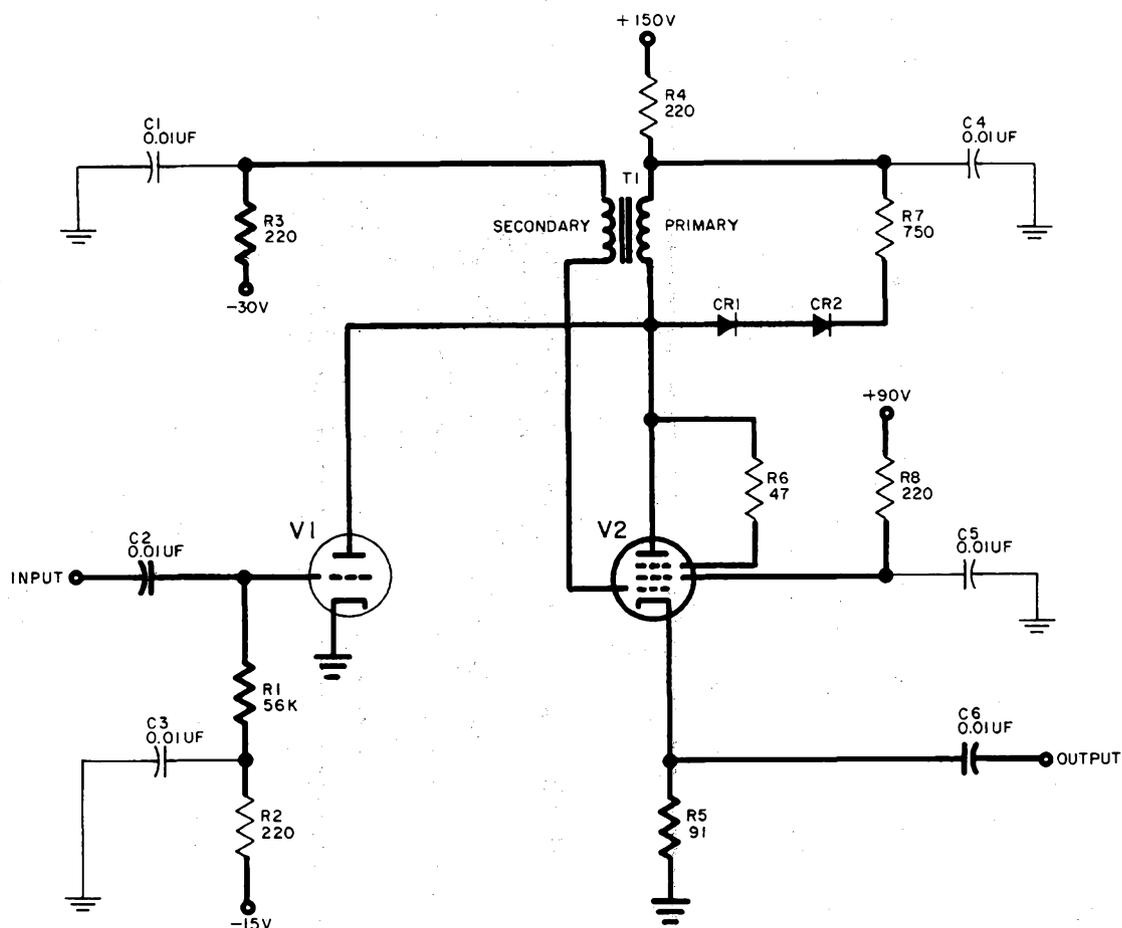
Figure 3-55. Pulse Generator, Model D, Schematic Diagram
