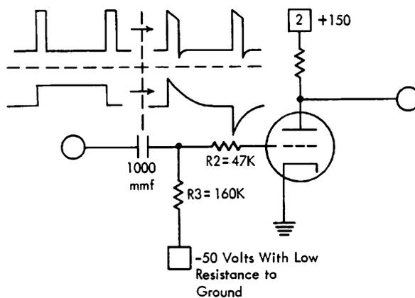
Figure 28. The Coupling Capacitor
