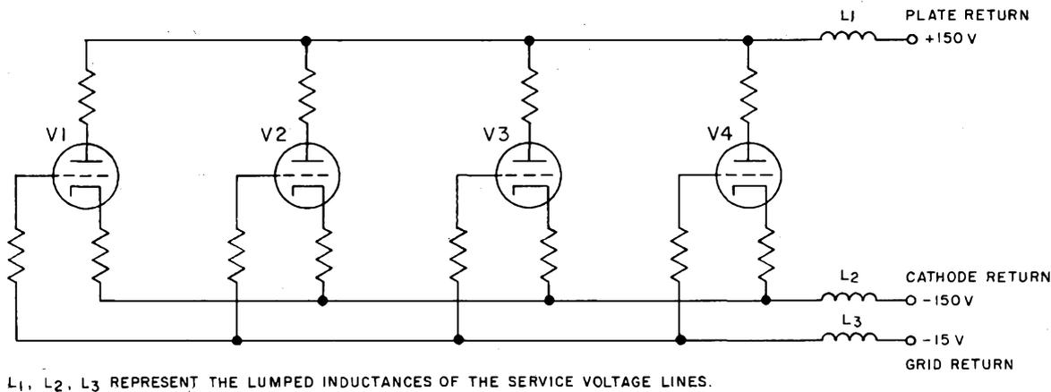
L<sub>1</sub>, L<sub>2</sub>, L<sub>3</sub> REPRESENT THE LUMPED INDUCTANCES OF THE SERVICE VOLTAGE LINES.
