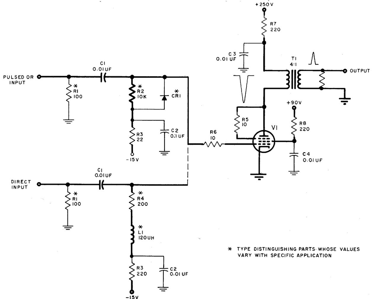
Figure 3-13. Pulse Amplifier, Model B, Schematic Diagram
