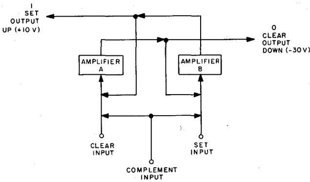
Figure 3-39. Flip-Flop, Block Diagram
