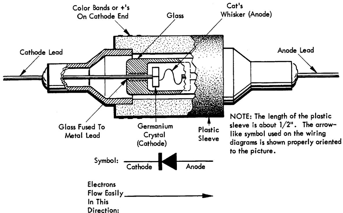
Figure 52. An Enlarged Diagram of a Germanium Diode Showing Construction
