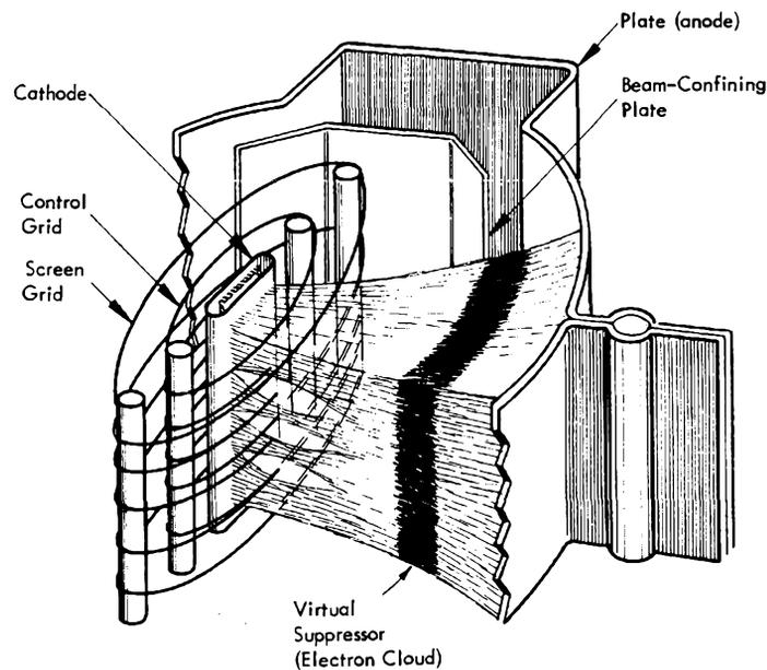
Figure 42. A Beam Power Pentode
