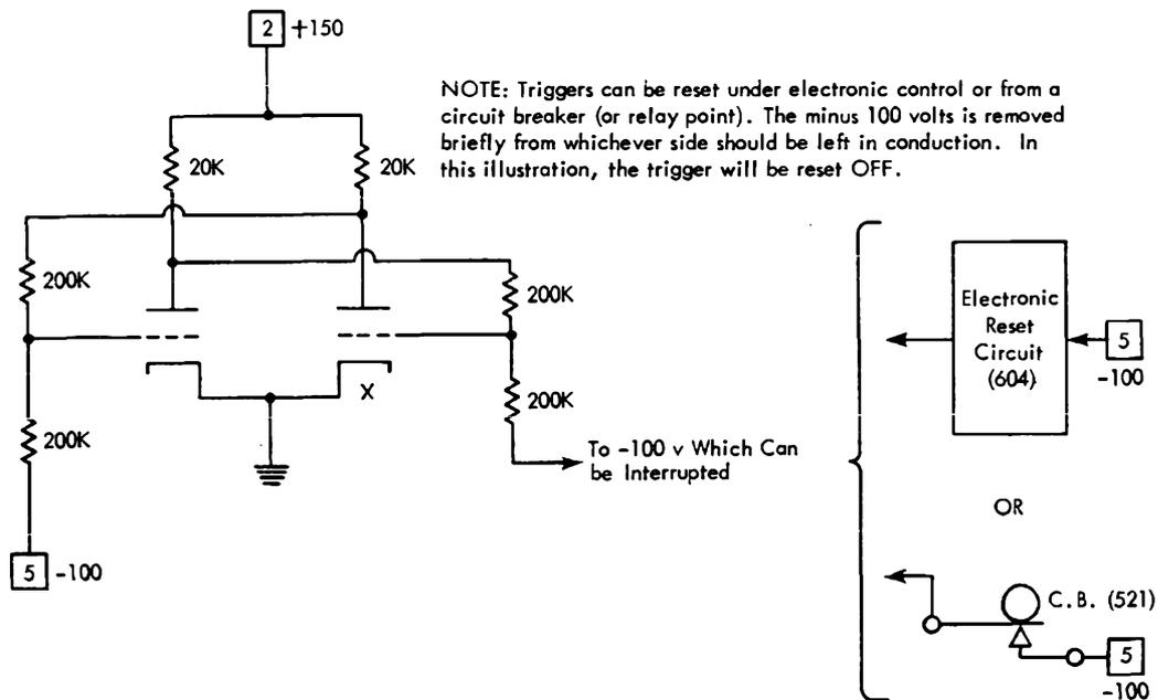
Figure 59. Trigger Unit Reset
