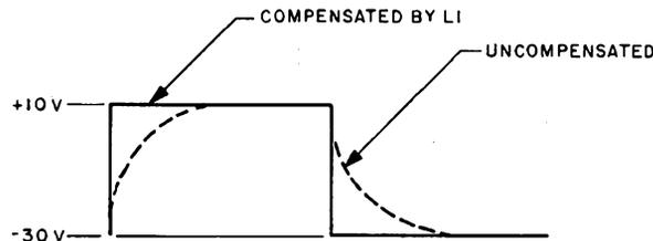
Figure 2-17. Peaking Coil Compensated Plate Circuit, Simplified Schematic Diagram with Waveform
