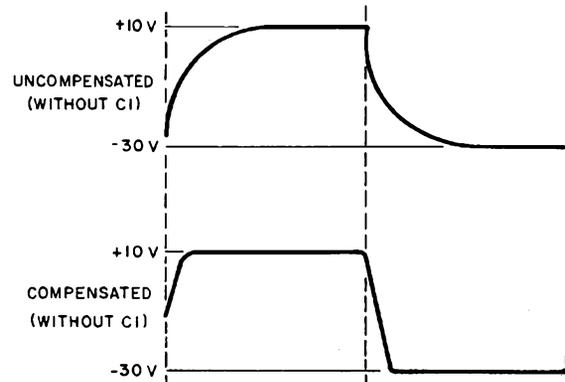
Figure 2-16. Output Waveform (V2 in Figure 2-15)
