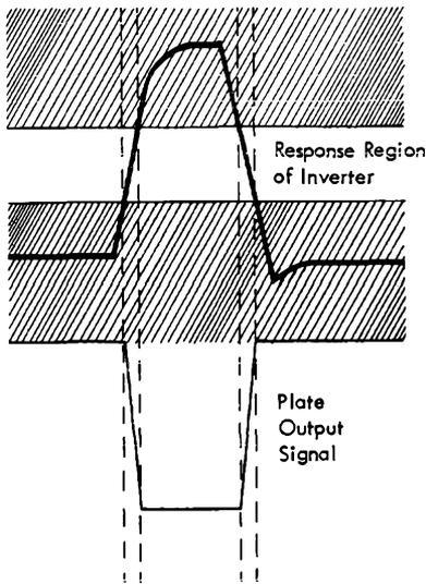
Figure 34. Signal Reshaping
