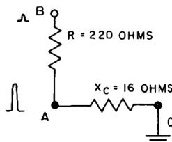
AN ALTERNATING VOLTAGE (PULSE) AT A, WILL CAUSE CURRENT TO FLOW IN TWO PATHS A-B AND A-C.
