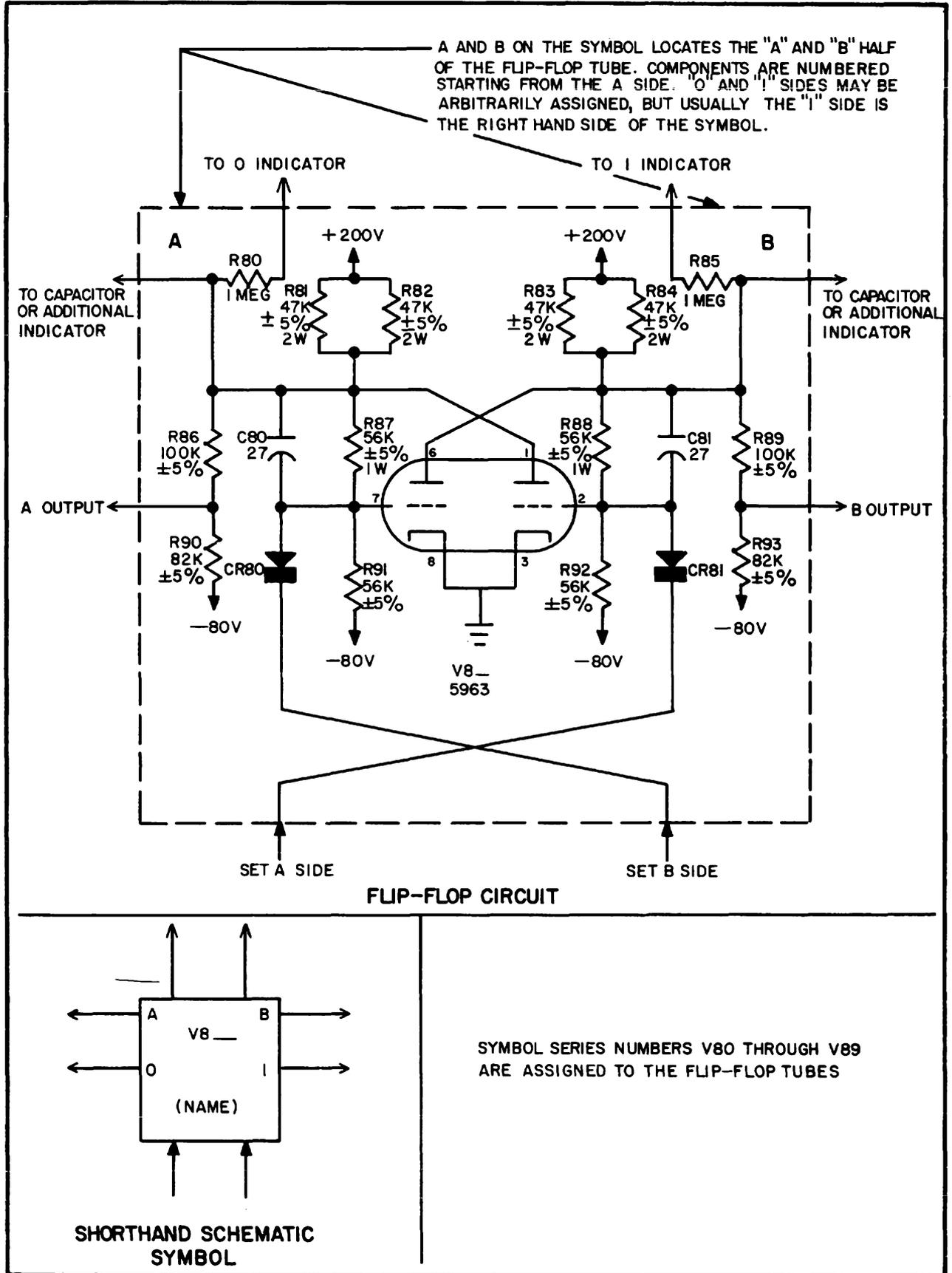
Figure 3. STANDARD Flip-flop Stage
