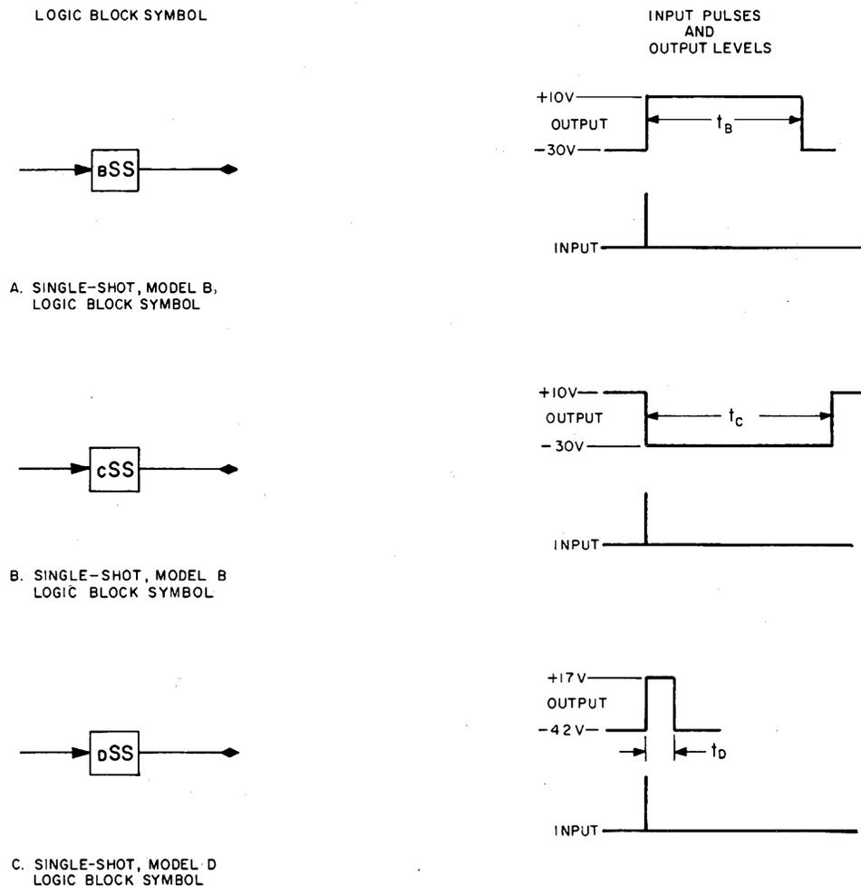
**Figure 3-45. Single-Shot, Logic Block Symbols and Output Waveforms**
