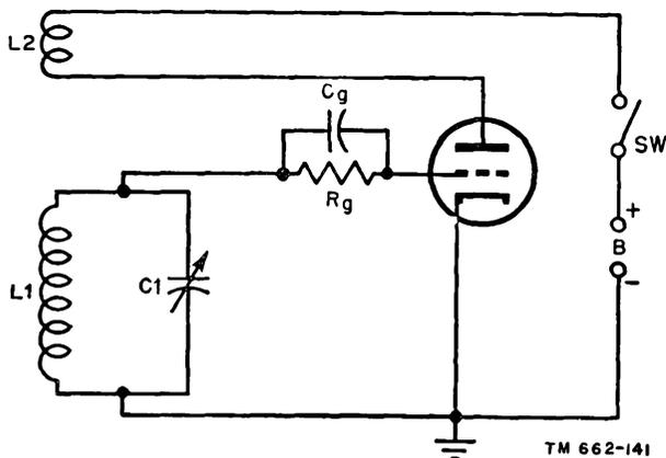
Figure 132. Tuned-grid oscillator.
