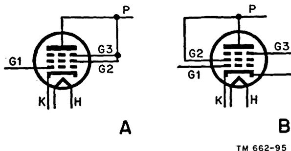
Figure 86. Typical example showing pentode connection to triode.
