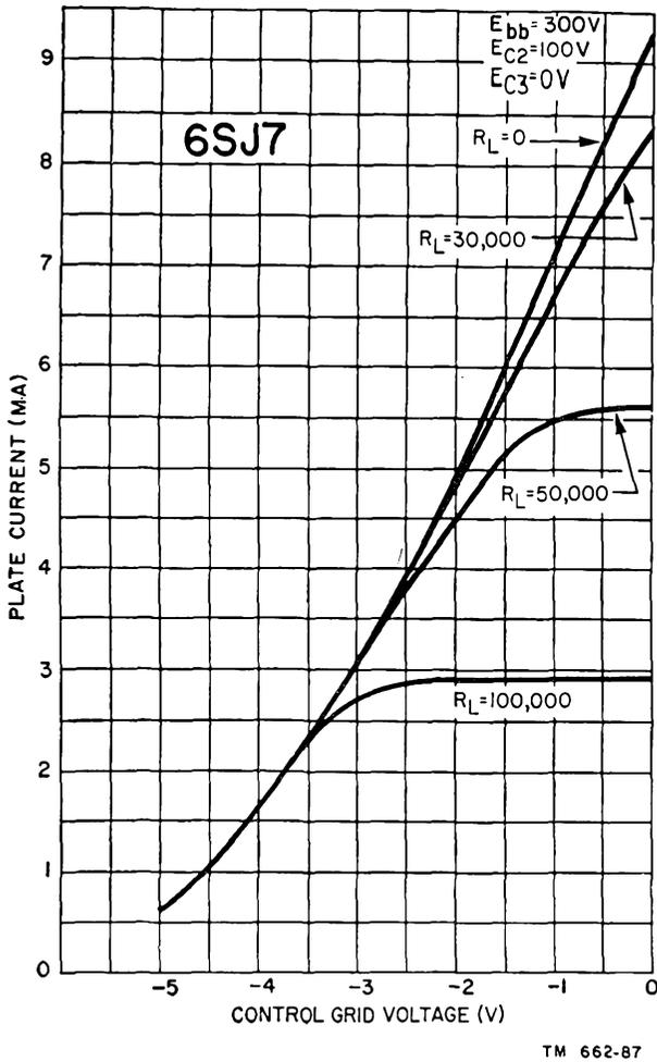
Figure 78. Dynamic transfer characteristic curves of 6SJ7 pentode.
