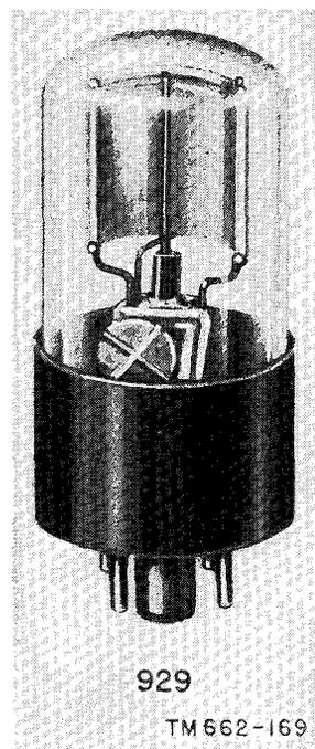
Figure 160. Typical phototube.
