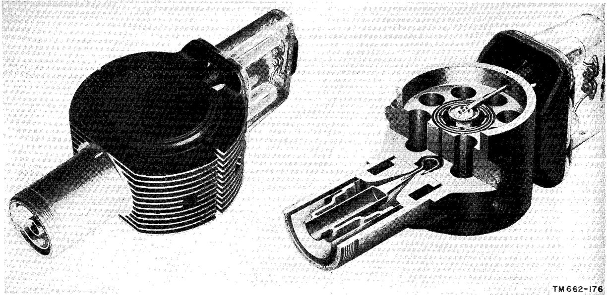
Figure 167. Operational and cutaway view of typical magnetron.
