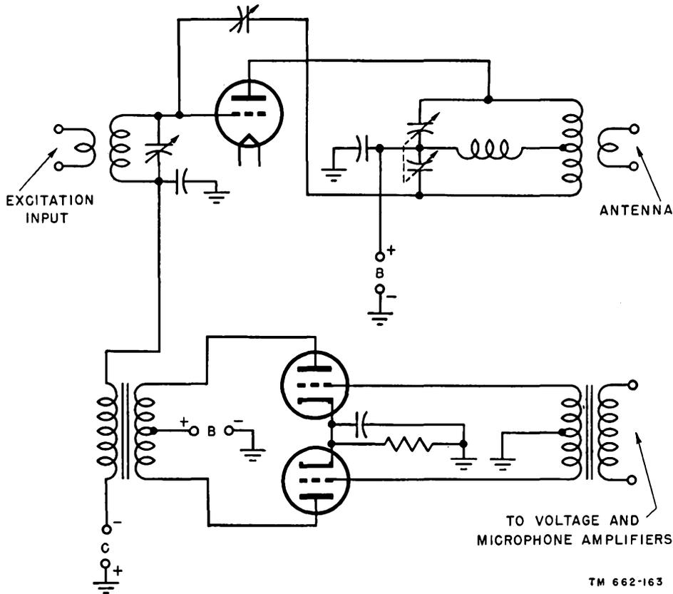
Figure 154. Grid-modulated amplifier.
