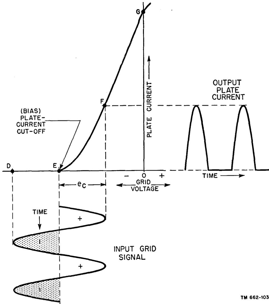
Figure 94. Class B operation on dynamic characteristic.
