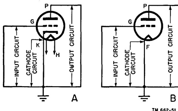
Figure 42. Input, output, and cathode circuits of indirectly and directly heated triodes.
