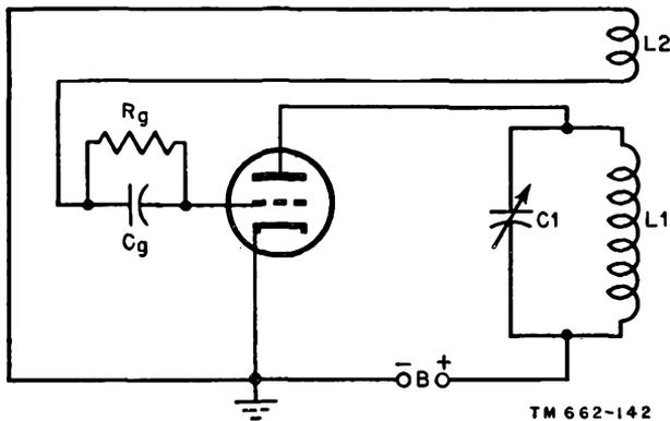
Figure 133. Tuned-plate oscillator.
