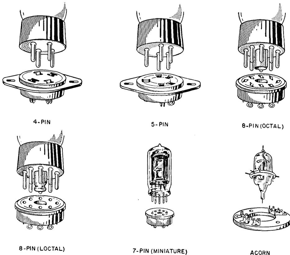
Figure 171. Receiving-type electron-tube bases and corresponding sockets.
