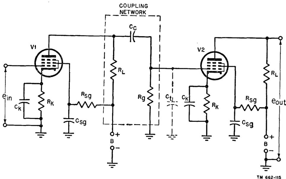
Figure 106. Typical R-C coupled amplifier using pentodes.
