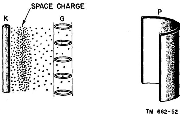
Figure 43. Imaginary view of electrodes in a triode.
