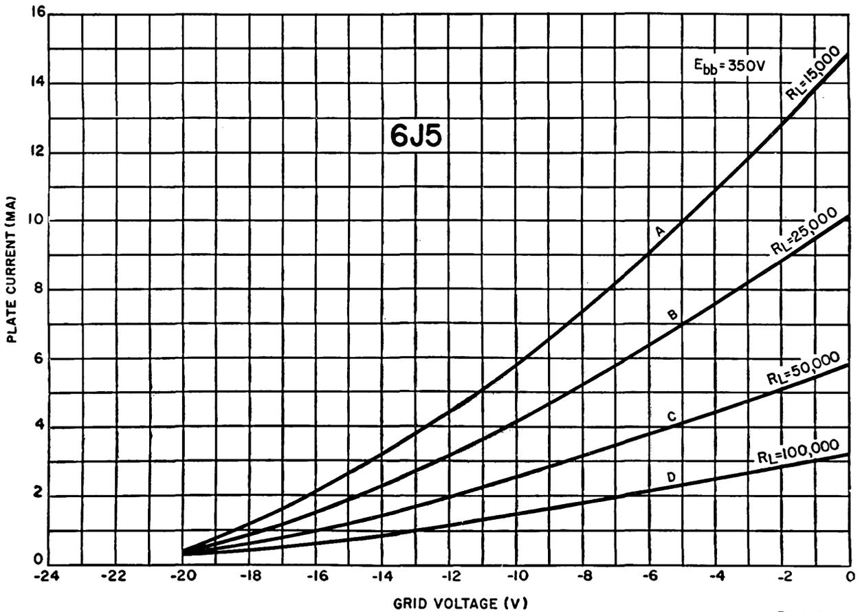
Figure 63. Dynamic transfer characteristic curves for different loads.
