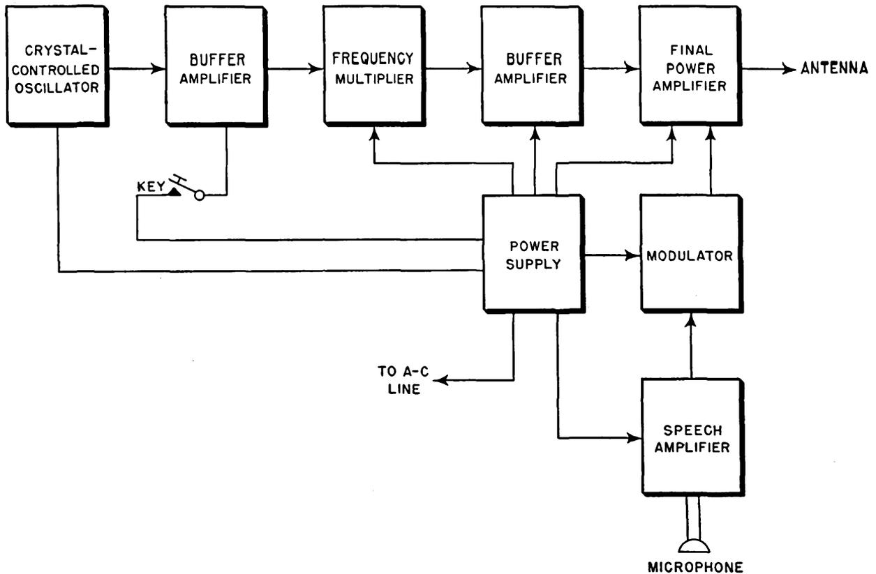
Figure 141. Block diagram of typical transmitter.
