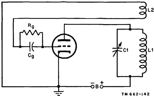
Figure 133. Tuned-plate oscillator.
