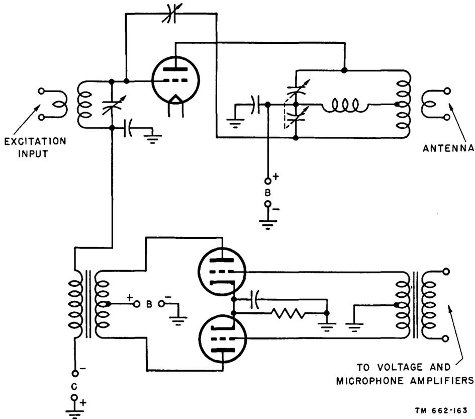
Figure 154. Grid-modulated amplifier.
