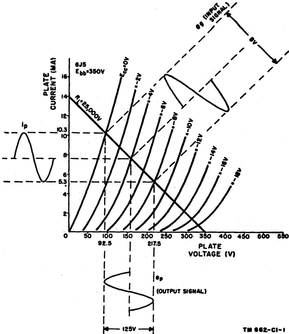
Figure 61.1. (Added) Plate characteristics showing signal voltage amplification.
