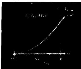
Fig. 6—Transfer characteristic of a typical power pentode.
