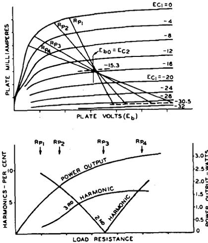
Fig. 11—Performance characteristics of a typical power pentode.
