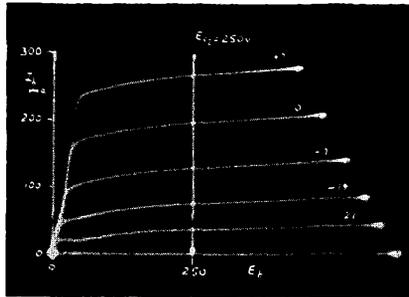
Fig. 21—Plate family of type 6L6 beam power tube.
