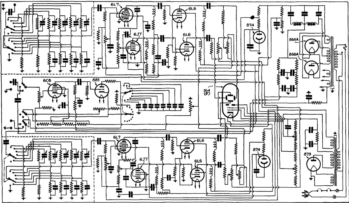
Fig. 32. Schematic of RCA 9" Oscillograph TMV 168A.
