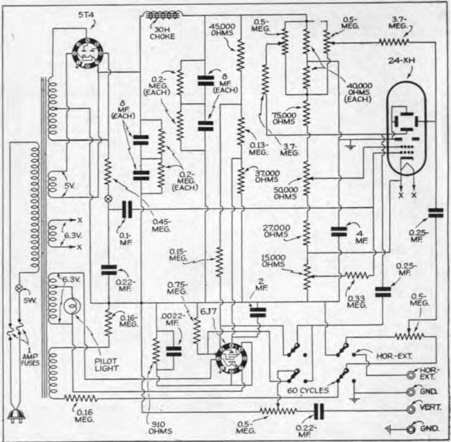
Fig. 11. Schematic of Model 530 Supreme Oscilloscope.
