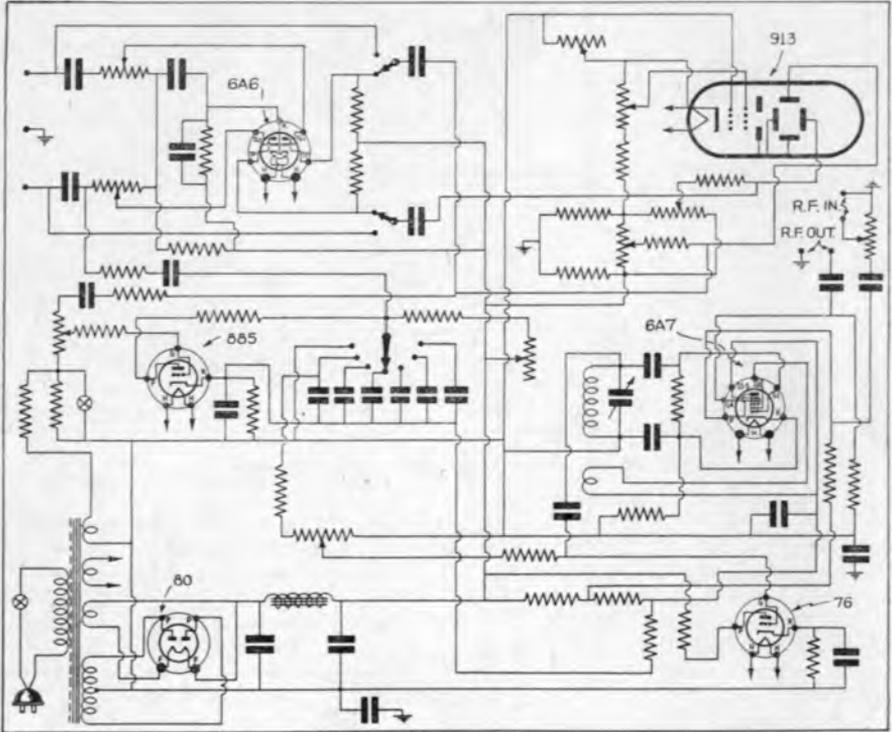
Fig. 48. Above. Triumph Oscillograph Wobbulator and Schematic.
