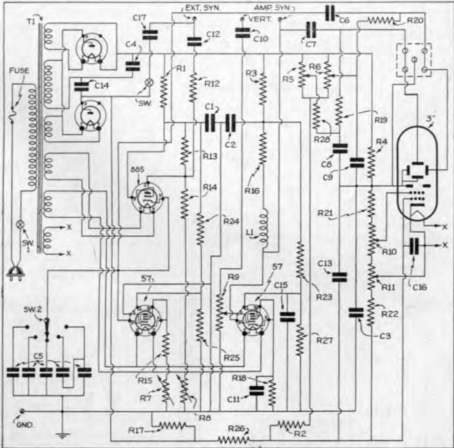
Fig. 56. Schematic of Model 154 Dumont 3" Oscillograph.
