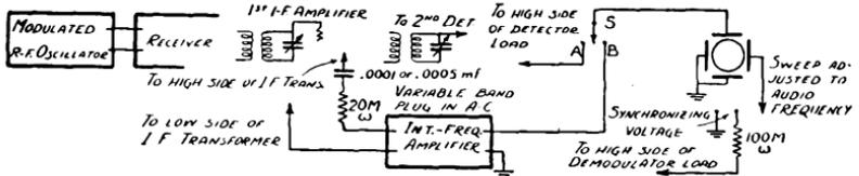
Fig. 195. Circuit for checking overloading in i-f. amplifiers.
