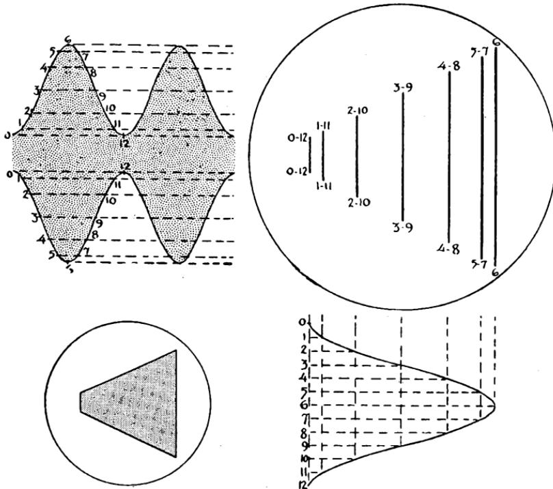
*Figs. 386-A, above, 386-B, below. How a trapezoidal pattern is developed on the screen of a cathode-ray tube. The pattern enclosed in the small circle, Fig. 386-B, is what actually appears on the screen. The sweep voltage is in phase with the modulated wave.*
