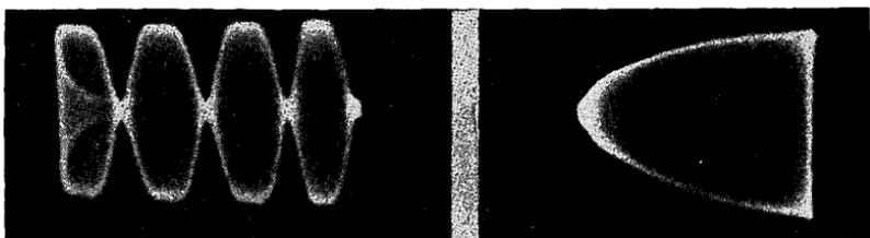
*The wave envelope and trapezoid patterns indicating insufficient excitation of the Class C stage are shown in Figs. 396 (left) and 397 (right). All other operating conditions are correct. Note the clipped peaks in figure 396 and the non-linearity of the pattern in Fig. 397.*
