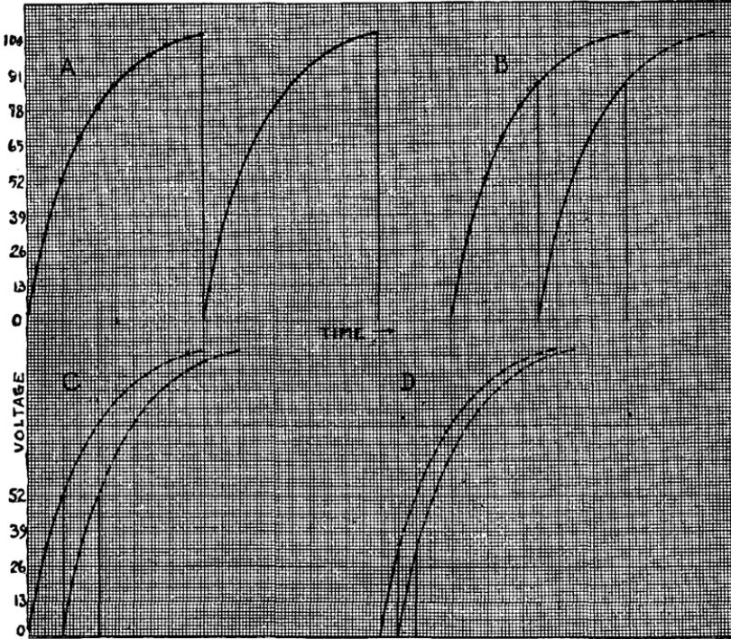
*Fig. 33-A. Two cycles of a theoretical saw-tooth wave such as would be developed by a resistor-condenser-discharge tube combination with the tube tripping at 105 volts. Fig. 33-B shows the waveform when the tube flashes at 87.7 volts and Fig. 33-C shows the wave when the tube flashes at 52 volts. When the flashing voltage is reduced to 32.5 volts, Fig. 33-D, the charging portion of the wave is fairly linear.*
