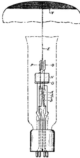
*Fig. 2. The various elements of the Western Electric type 224 cathode-ray tube are designated in the table on the right. The glass tube is first evacuated and then argon is introduced. As is explained fully in the text, this gas is an aid in concentrating the beam of electrons so that when it strikes the screen a small spot will result.*
