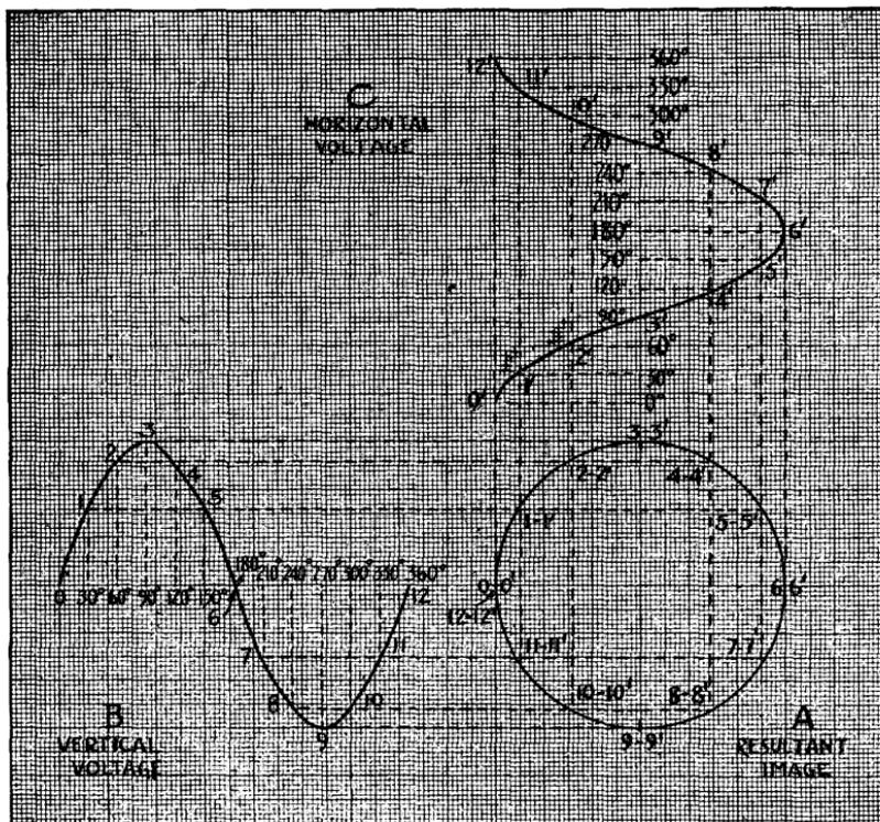
Fig. 48. The sine wave at B is  $90^\circ$  out of phase with the one shown at C, so that the resulting pattern is a circle. Note that the time axis here is divided into degrees of a circle instead of fractions of a second as in previous drawings.
