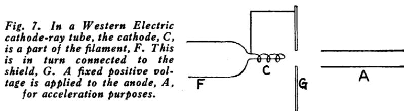
*Fig. 7. In a Western Electric cathode-ray tube, the cathode, C, is a part of the filament, F. This is in turn connected to the shield, G. A fixed positive voltage is applied to the anode, A, for acceleration purposes.*
