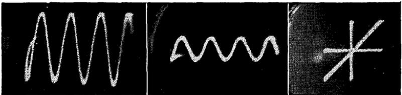
*Figs. 207, left, 208, middle, 209, right. The output wave of the Class A stage is shown in Fig. 207. The input voltage wave to the Class B stage is shown in Fig. 208. The correct phase relation of  $180^\circ$  between the two voltages to the Class B input is indicated in Fig. 209.*
