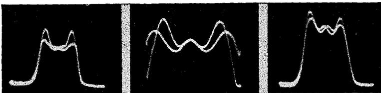
*Figs. 306, left, 307, middle, 308, right. The resonance curve of Fig. 306 indicates incorrect alignment. Note that the bases of the two patterns coincide, but not the peaks. The incomplete curve in Fig. 307 was caused by the frequency band of the circuit being greater than the signal frequency sweep. The corrected condition is shown in Fig. 308.*
