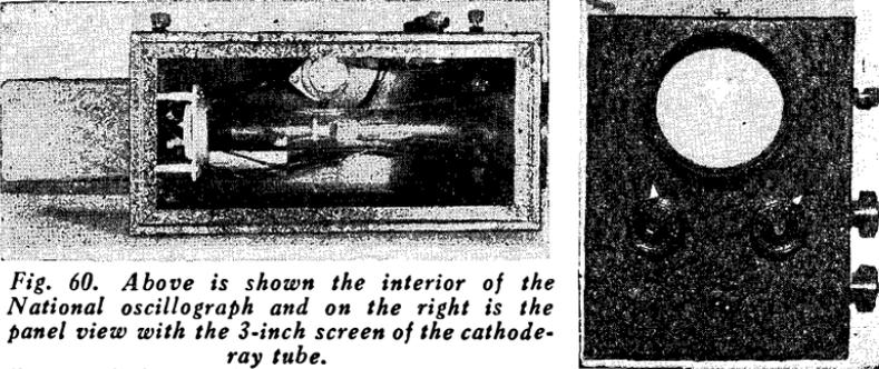
Fig. 60. Above is shown the interior of the National oscilloscope and on the right is the panel view with the 3-inch screen of the cathode-ray tube.
