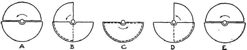
*Fig. 259. Five positions of the rotating plates of a variable condenser used in a frequency modulator. When the capacity is minimum (plates unmeshed completely), the frequency is maximum and vice versa. It is essential that the plates be in positions B or D when the oscillator delivers the mean frequency of the circuit under test.*
