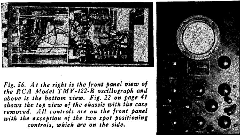
*Fig. 56. At the right is the front panel view of the RCA Model TMV-122-B oscillograph and above is the bottom view. Fig. 22 on page 41 shows the top view of the chassis with the case removed. All controls are on the front panel with the exception of the two spot positioning controls, which are on the side.*
