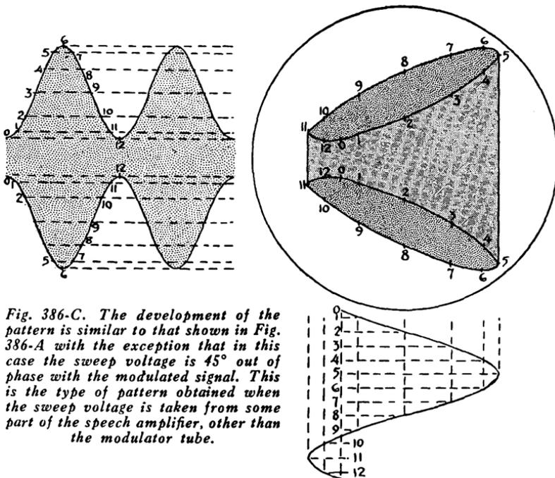
*Fig. 386-C. The development of the pattern is similar to that shown in Fig. 386-A with the exception that in this case the sweep voltage is 45° out of phase with the modulated signal. This is the type of pattern obtained when the sweep voltage is taken from some part of the speech amplifier, other than the modulator tube.*
