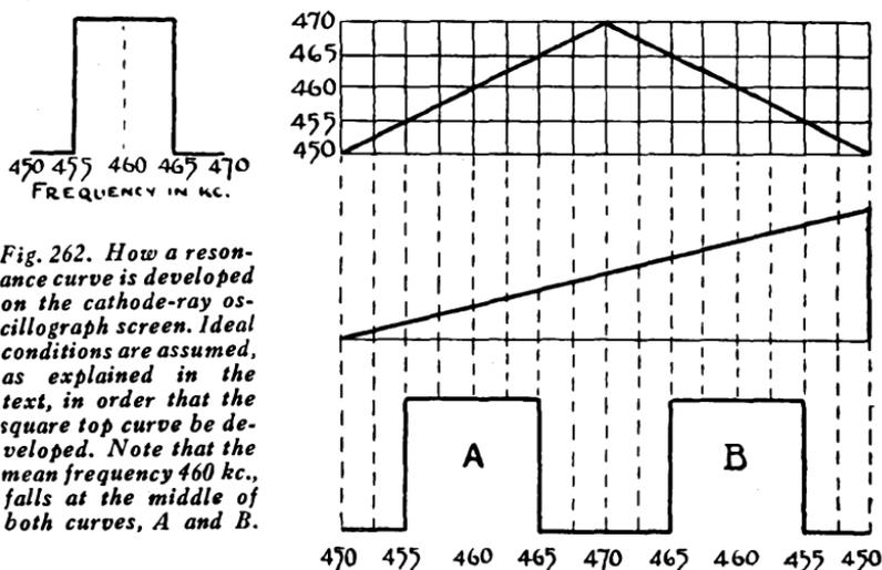
Fig. 262. How a resonance curve is developed on the cathode-ray oscilloscope screen. Ideal conditions are assumed, as explained in the text, in order that the square top curve be developed. Note that the mean frequency 460 kc., falls at the middle of both curves, A and B.
