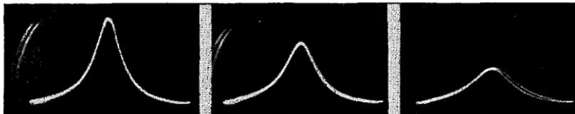
*Figs. 329, left, 330, middle, 331, right. When R-2 of Fig. 328 was 0, the curve of Fig. 329 was obtained. When R-2 was 2 ohms and 6 ohms, the curves obtained are shown in Figs. 330 and 331, respectively.*
