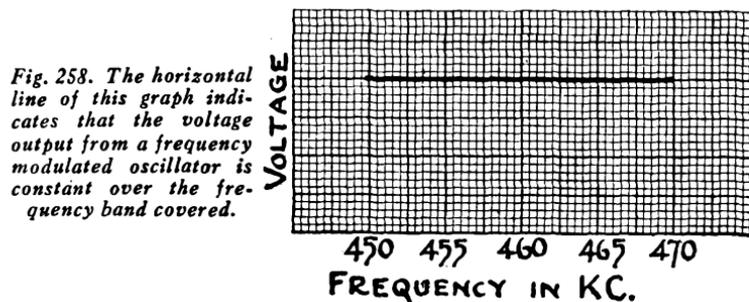
*Fig. 258. The horizontal line of this graph indicates that the voltage output from a frequency modulated oscillator is constant over the frequency band covered.*
