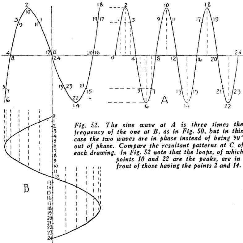
*Fig. 52. The sine wave at A is three times the frequency of the one at B, as in Fig. 50, but in this case the two waves are in phase instead of being 90° out of phase. Compare the resultant patterns at C of each drawing. In Fig. 52 note that the loops, of which points 10 and 22 are the peaks, are in front of those having the points 2 and 14.*
