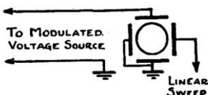
*Fig. 385. The modulated wave envelope of Fig. 382 is developed with the arrangement shown on the left. For frequencies above 100 kc., it is necessary to connect directly to the free vertical plate. See text.*
