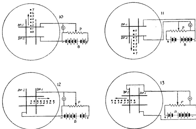
*Figs. 10, 11, 12, 13. The circles indicate the viewing screen of a cathode-ray tube. The dots, numbered 0 to 7, show the successive positions of the spot formed by the electron beam when it strikes the screen and various voltages are applied to the deflecting plates, the voltages from the battery, B, being controlled by a potentiometer, P, and their values being read by the voltmeter, V.*
