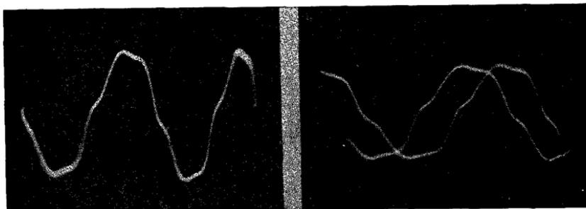
*Fig. 81, left, Fig. 82, right. Even though the wave impressed on the vertical plates of the cathode-ray tube is distorted, as in Fig. 81, the same need for proper synchronization exists. Improper adjustment of the synchronizing control is responsible for the pattern of Fig. 82*
