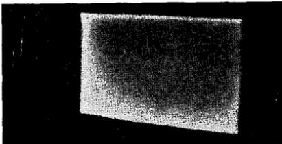
*Fig. 135. Theoretically this pattern, obtained with magnetic deflection applied vertically and electrostatic deflection horizontally, should be a perfect rectangle, but it is not, due to tube distortion.*
