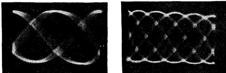
*Fig. 126, left, Fig. 127, right. The pattern in Fig. 126 shows two loops and two lines of intersections. By adding one to the number of intersections, the ratio of 2-3 or 3-2 is established for the pattern. The five loops and five intersections of Fig. 127 indicates a ratio of 5-6 or 6-5, by adding one to the number of intersections.*
