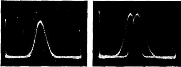
*The left pattern shows the circuit in resonance and that on the right, the circuit out of resonance. These oscillograms made with the Supreme 555.*
