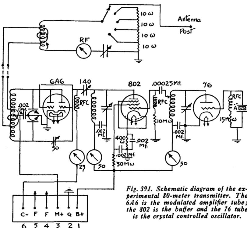
Fig. 391. Schematic diagram of the experimental 80-meter transmitter. The 6A6 is the modulated amplifier tube; the 802 is the buffer and the 76 tube is the crystal controlled oscillator.
