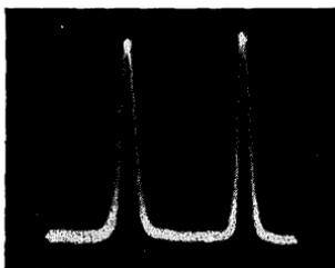
*Fig. 265. An example of symmetrical resonance curves. Note that the base of the right hand curve is less wide than the one on the left. As explained in the text, this is due to the variation of the sweep from true linearity. The sweep frequency here is the same as the motor frequency.*
