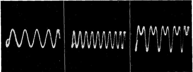
*Figs. 154, left, 155, middle, 156, right. A 1000-cycle sine wave, shown in Fig. 154, and a 2000-cycle sine wave, Fig. 155, result in the composite wave, Fig. 156. Note that the 2000-cycle wave (the second harmonic of the 1000-cycle wave) is almost equal in amplitude to the fundamental frequency.*
