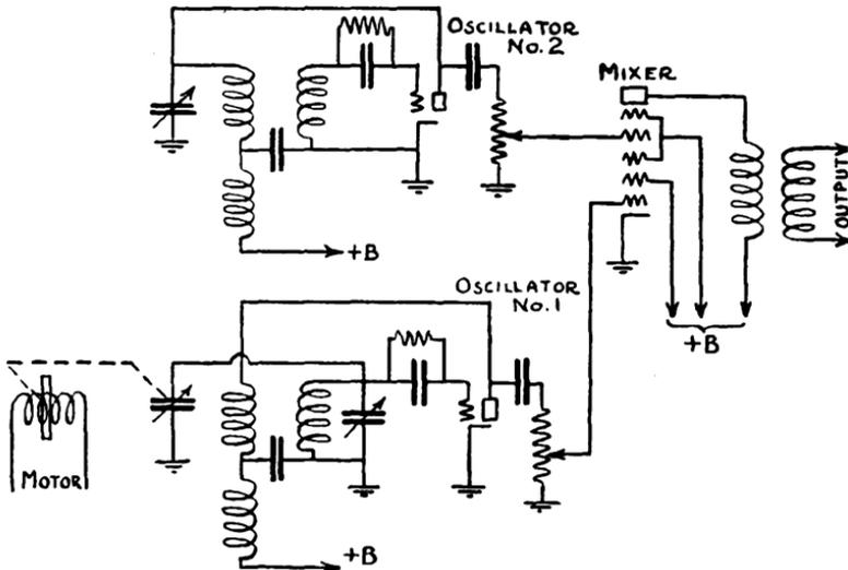
*Fig. 252. Schematic diagram of a beat frequency oscillator which is frequency modulated by the motor driven variable condenser in the lower left corner of the diagram. This type of oscillator, when frequency modulated, provides a band width that is constant for any output frequency.*
