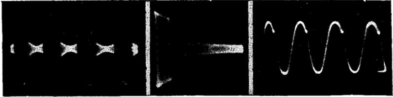
*Fig. 415 (left) indicates the modulated wave. Fig. 416 (middle) shows the equivalent trapezoidal pattern and 417 (right) shows the audio wave across the modulator output. Note that the oscillation starts suddenly, persists for awhile and then dies out during each cycle. Note the resulting dip in the audio wave*
