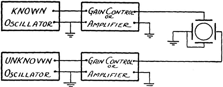
Fig. 94. The basic circuit used for producing Lissajous figures, which are used in the comparison of two frequencies or for frequency calibration.
