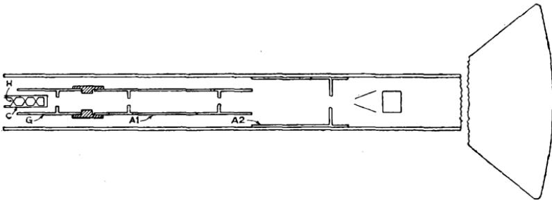
*Fig. 4. In the sketch of the RCA type 906 tube the following letters indicate the various elements: H, the heater; C, cathode; G, shield grid; A1, first anode; A2, second anode. The two pairs of deflecting plates are to the right of A2. It will be noted that these plates are at an angle to the main axis of the tube. This arrangement of elements in a glass envelope or bulb constitutes what is sometimes referred to as an "electron gun."*
