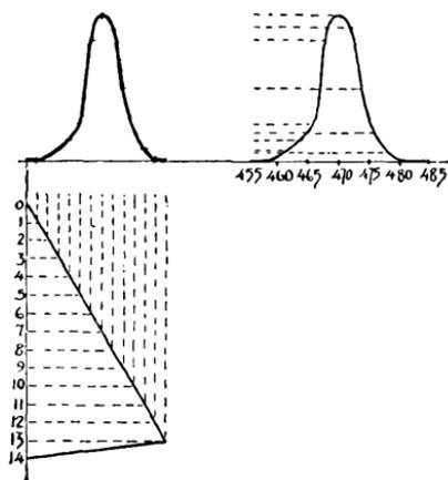
*Fig. 53. The sweep frequency is such that one cycle occurs during the time that the oscillator's frequency varies from 455 to 485 kc. The tuned circuit to which this band of frequencies is applied is resonant at 470 kc. The frequency response curve taken across the detector load appears at the right and its image, as seen on the screen is at the left, above the sweep.*
