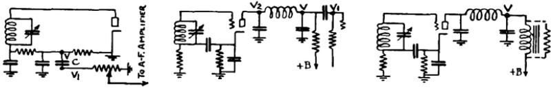
*Figs. 288, left, 289, middle, 290, right. Schematic diagrams showing two types of demodulator circuits with three types of load circuits. The correct points for connecting to the deflection plates are indicated by V. The results obtained when connections are made to other points are explained in the text.*
