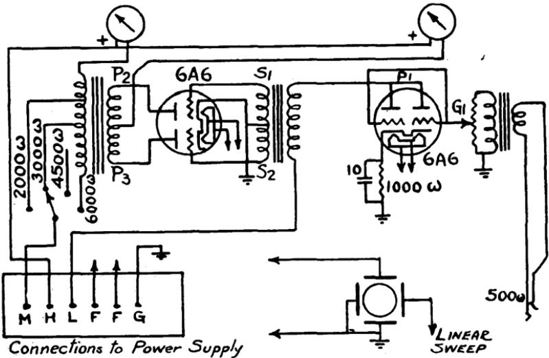
Fig. 206. A typical Class B amplifier, which can be employed either for amplification or for the modulation of a transmitter.
