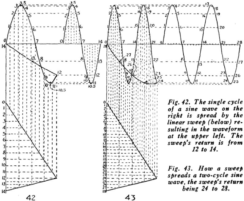
*Fig. 42. The single cycle of a sine wave on the right is spread by the linear sweep (below) resulting in the waveform at the upper left. The sweep's return is from 12 to 14.*
