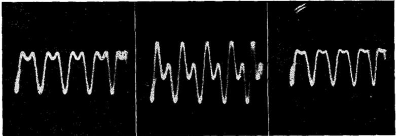
*Figs. 157, left, 158, middle, 159, right. The amplitude of the wave in Fig. 155 was reduced and caused the reduction of the dip in the composite wave of Fig. 157. Compare Fig. 156. By shifting the phase between the waves of Figs. 154 and 155, the composite wave of Fig. 158 was obtained. Fig. 159 was obtained by reducing the amplitude of the wave of Fig. 154 and making that of Fig. 155 about one-half its amplitude. Compare Figs. 156 and 157.*
