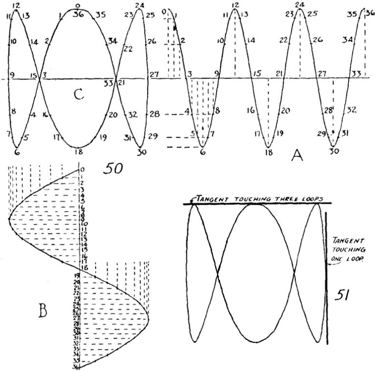
Fig. 50. The sine wave at A is three times the frequency of that at B and is  $90^\circ$  out of phase. Both waves are divided into equal time intervals. The numbers on the resultant image at C indicate the amplitude displacement of each wave at the same instant.
