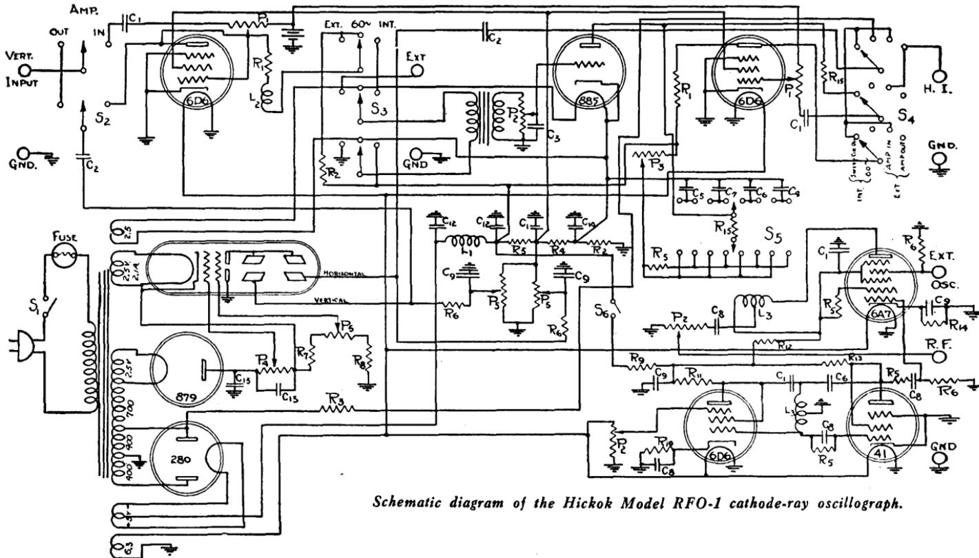
*Schematic diagram of the Hickok Model RFO-1 cathode-ray oscillograph.*
