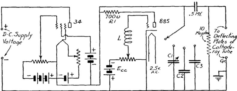
*Fig. 38. The type 34 tube replaces the resistor,  $R$ , (Fig. 34) as a current limiting device in this relaxation oscillator sweep circuit. The constant current flow tends to charge whatever condenser is in the circuit at a constant rate, making the voltage rise constant thereby supplying a linear output to the deflecting plates.*
