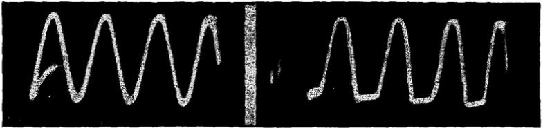
*Figs. 213, left, 214, right. The waveform of the voltage across the secondary circuit is shown in Fig. 213. The waveshape of the voltage, showing cut-off, in the plate circuit of one of the sections of the 6A6 tube in the Class B stage.*
