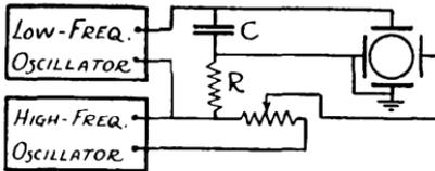
*Fig. 120. This circuit is used for separating the front and rear portions of a pattern, making the interpretation of high ratio figures much simpler. For a circular pattern the reactance of  $C$  should equal resistance of  $R$  at the base frequency.*
