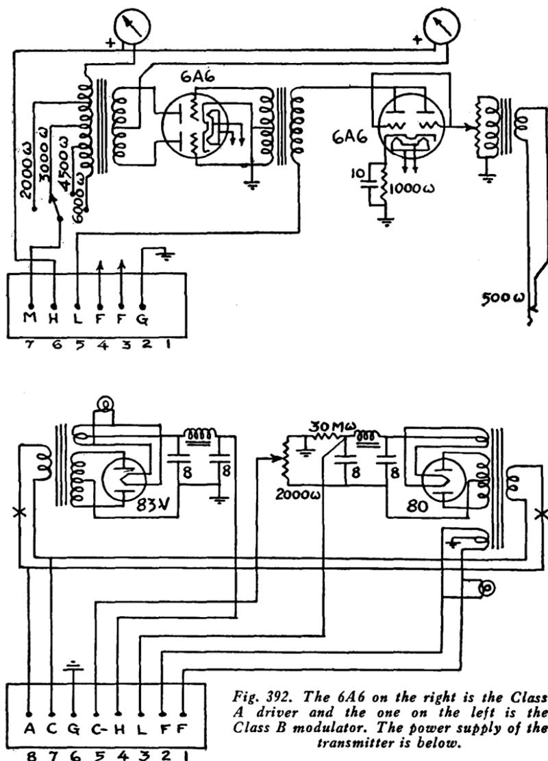
Fig. 392. The 6A6 on the right is the Class A driver and the one on the left is the Class B modulator. The power supply of the transmitter is below.
