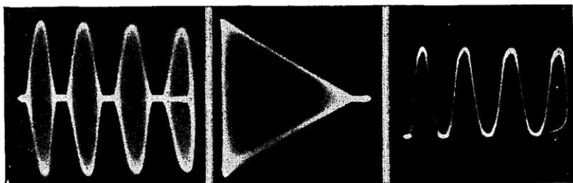
*Fig. 425 (left) shows the modulated wave envelope when the modulator is matched to a 6000-ohm load. The corresponding trapezoidal pattern is shown in Fig. 426 (middle). The audio wave across the modulator load is shown in Fig. 427 (right). Compare these images with Figs. 393 and 394.*
