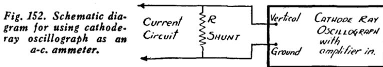
is shown in figure 152. The cathode-ray tube is arranged for independent voltages to the horizontal and vertical plates. The vertical
