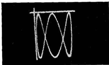
*Fig. 118. The tangent that is drawn parallel to the X axis touches the loops that result from the voltage applied to the vertical plates and the tangent drawn vertically touches those loops that are produced by the voltage applied to the horizontal plates. As the former was 3000 cycles and as the figure shows a 3-1 ratio, the other voltage must be 1000 cycles.*
