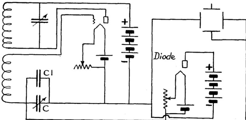
*Fig. 40. This circuit is capable of producing frequencies of a fairly high order. It is an ordinary oscillator circuit so arranged that the grid circuit will block periodically. The filament temperature of the diode is the rough frequency adjustment and the condenser  $C$  is the fine frequency adjustment.*
