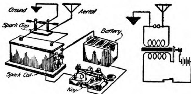
The instruments necessary for a simple radio telegraph transmitter.
