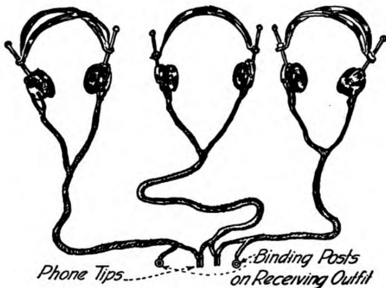
How telephone receivers should be connected when more than one pair are used.
