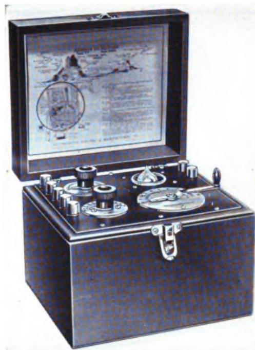
A simple vacuum tube receiver which operates from a single dry cell
