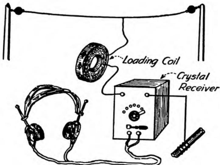
How a loading coil is connected between the aerial and ground of a crystal receiver to increase the wave-length.
