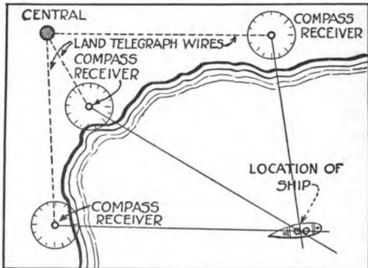
Showing how the radio compass functions.
