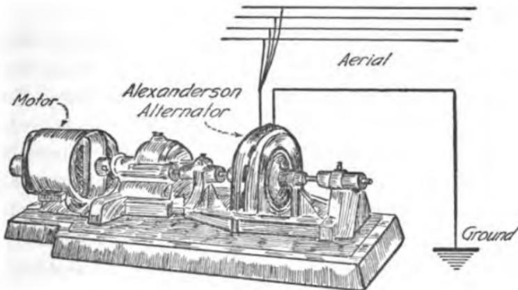
The Alexanderson high-frequency alternator now used in trans-oceanic radio communication.
