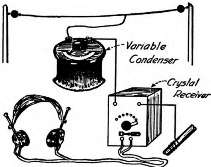
How a variable condenser is connected between the aerial and receiving outfit to reduce the wave-length.
