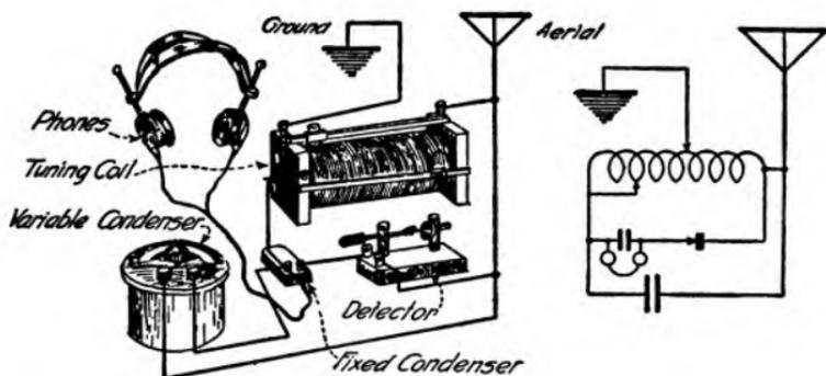
The instruments used in a simple radio receiving outfit.
