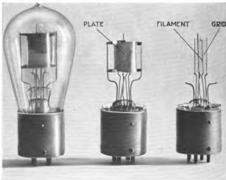
The various parts of a vacuum tube
