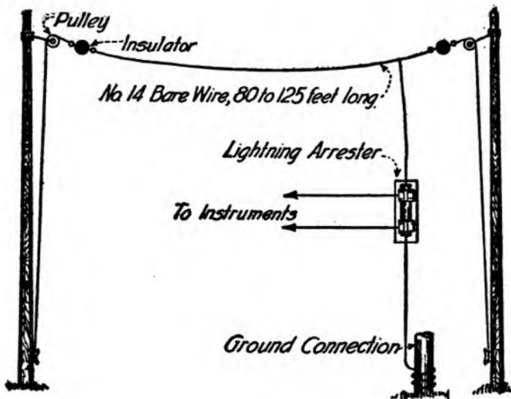
Constructional details of a simple one-wire aerial.
