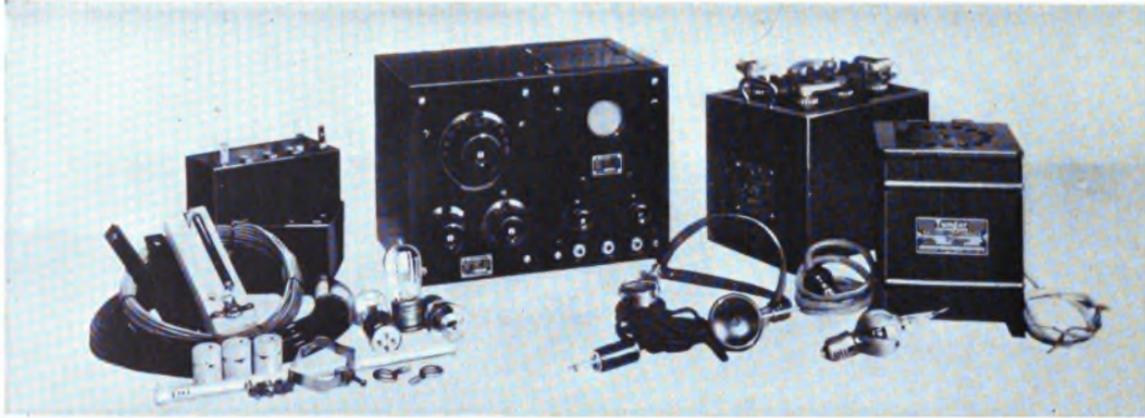
Complete set of apparatus necessary for a two-stage amplifying receiver. The auxiliary apparatus pictured follows: Storage battery, "B" batteries, three vacuum tubes, charging outfit for storage battery, telephones, aerial wire, lightning arrester, and insulators. A loud speaker can be used in place of the telephones
