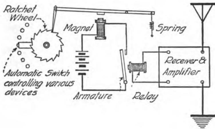
This diagram illustrates the principle of radiodynamics.
