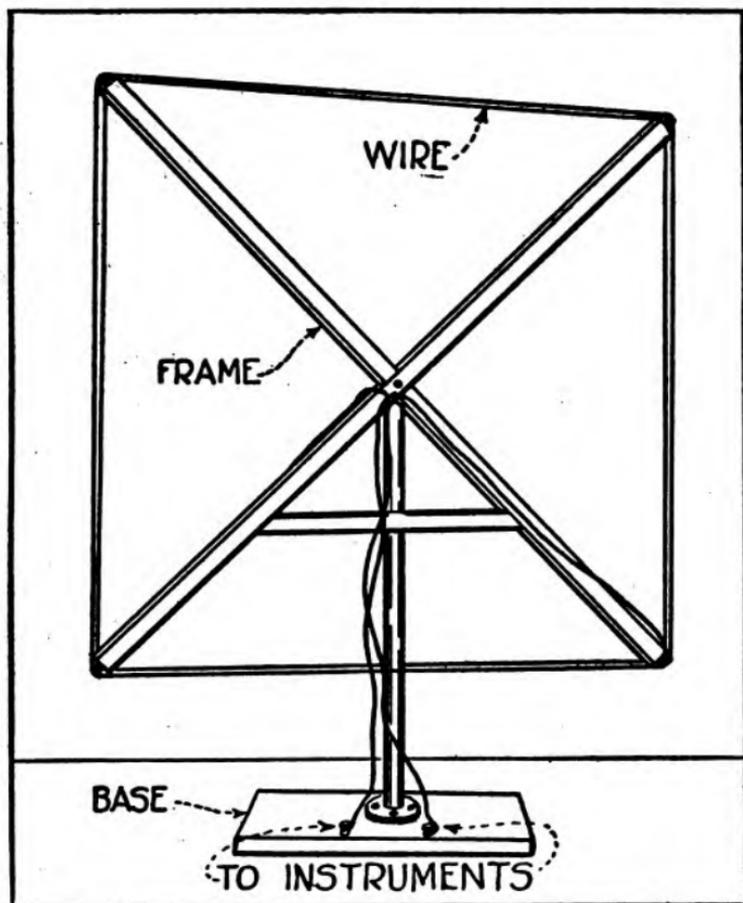
Construction of a loop antenna. It is made by winding several turns of wire around a four-foot frame.
