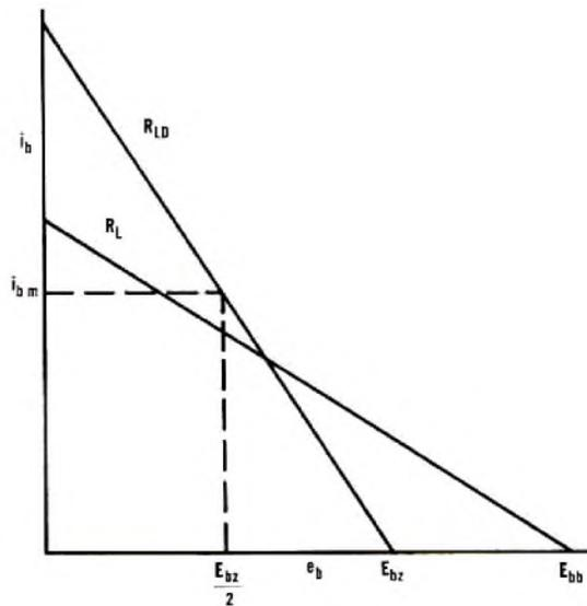
NOTE. if  $R_L$  and  $R_{LD}$  coincide,  $E_{bb} = E_{bz}$ .
