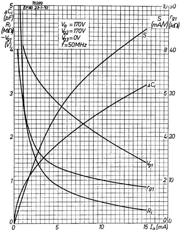
Fig. 18 Control-grid voltage, mutual conductance, internal resistance, input capacitance variation and input damping (at 50 Mc/s) plotted against anode current for anode and screen-grid voltage of 170 V.
