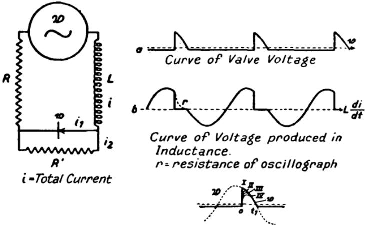
FIG. 45.—Valve in Series with Resistance and Inductance, and in Parallel with Resistance.
