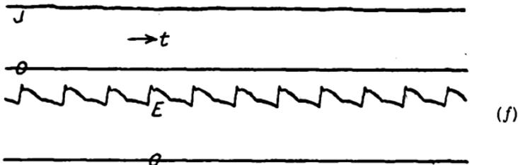
*D.C. voltage (550 volts) and current (460 amps.) of a large rectifier connected to a tram network.*
