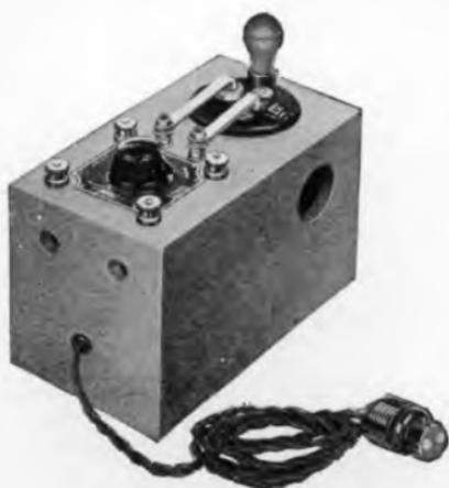
FIG. 55.—TANTALUM RECTIFIER FOR TRICKLE CHARGING.
