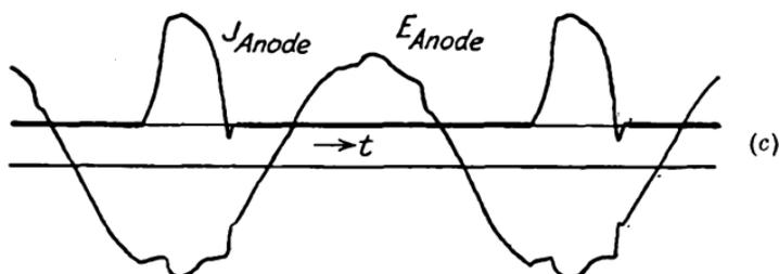
*Anode voltage (454 volts efficiency) and anode current (135 amps. efficiency) of a large rectifier with inductionless load.*
