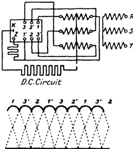
FIG. 36.—Connections and Output Curve of Hexaphase Rectifier.
