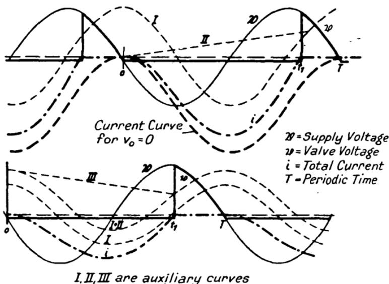
FIG. 44.—Valve in Series with Resistance and Inductance.
