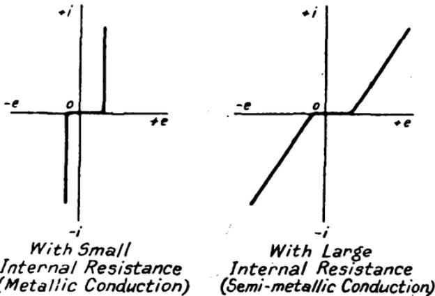
FIG. 30.—Theoretical Current Voltage characteristic of a Detector (after Schottky).
