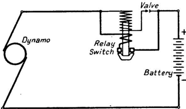
FIG. 92.—Use of Tantalum Valve as cut out in Wind-driven Electric Light Installations.
