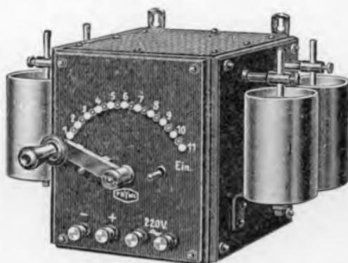
FIG. 53.—Aluminium Electrolytic Rectifier with Tapped Transformer; made by the Physikalische Werkstätten of Göttingen.
