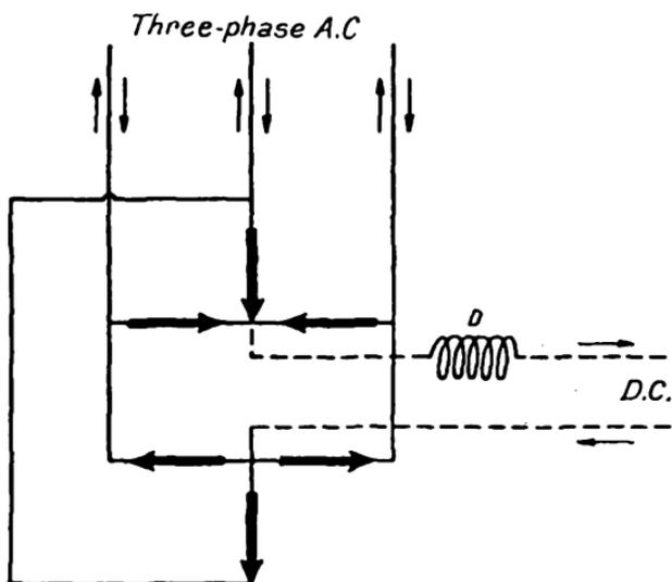
FIG. 33.—Grätz Circuit for Three-phase A.C.
