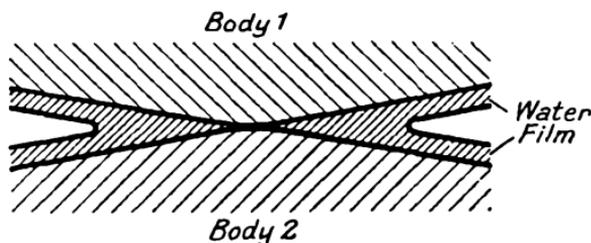
FIG. 28.—Diagram of Water Film between Two Bodies in contact.
