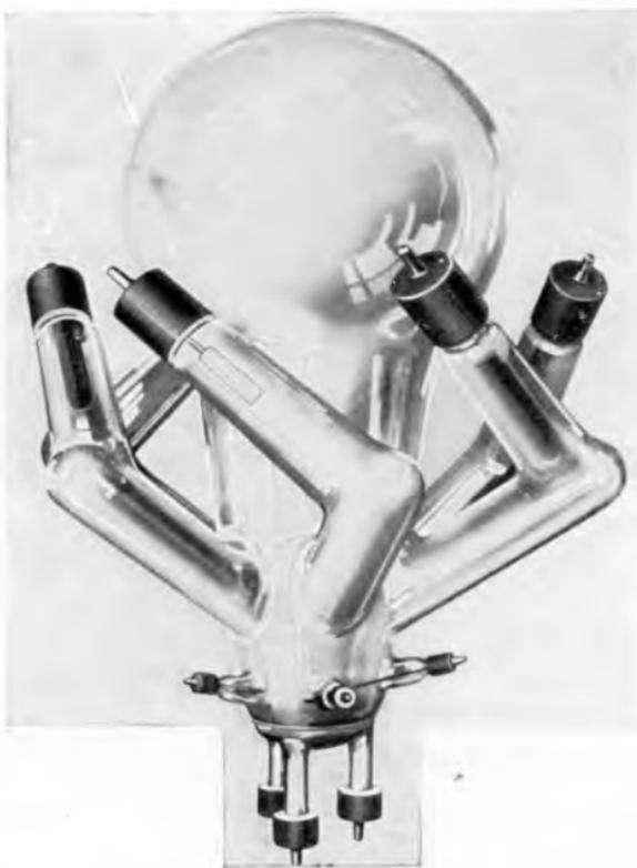
FIG. 69.—A.E.G. HEXAPHASE GLASS BULB RECTIFIER.
