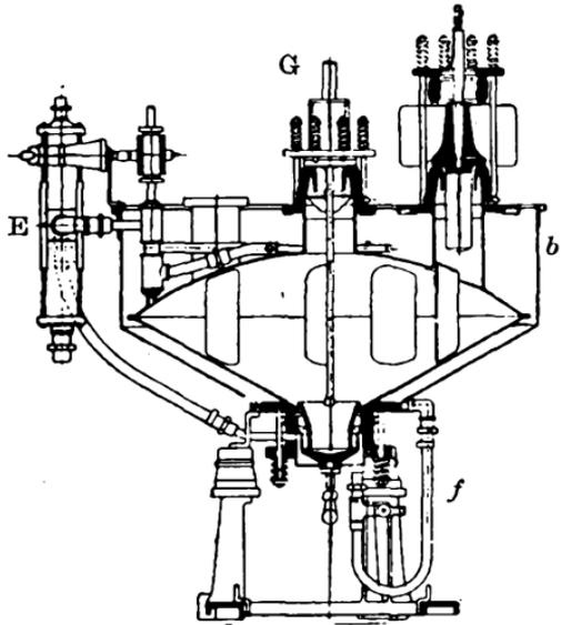
FIG. 84.—A.E.G. Rectifier for 500 amps.
