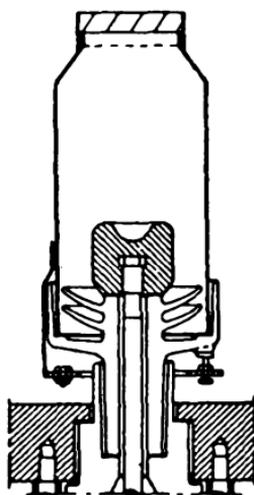
FIG. 83.—Construction of Anode in B.B.C. Rectifier.
