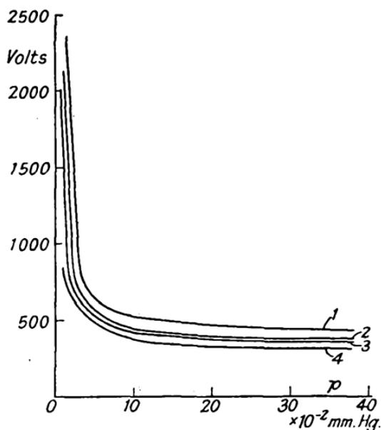
FIG. 24.—Dependence of Back-firing Voltage on pressure with Cathode covered with Sodium Chloride.
