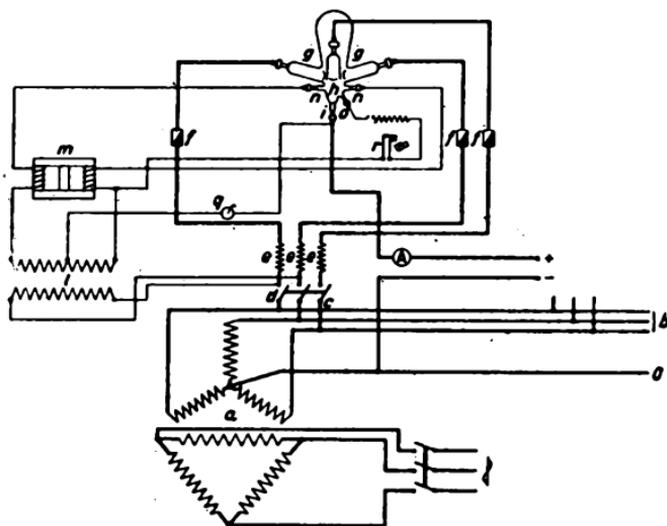
*a*-Main Transformer. *b*-3-phase Mains. *e*-Primary Choke Coils. *l*-Exciter Transformer. *o*-Mains Neutral Wire. *r*-Exciting Switch.
