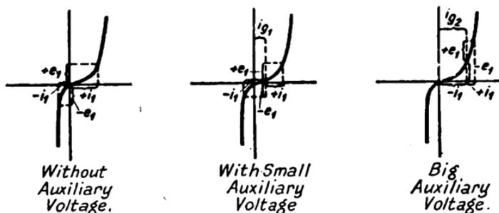
FIG. 31.—Influence of Auxiliary Voltage on Rectification.
