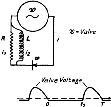
FIG. 46.—Inductance and Resistance in Parallel with each other and in Series with the Valve.
