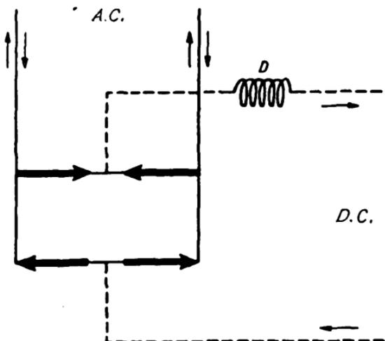
FIG. 32.—Grätz Circuit for Single-phase A.C.
