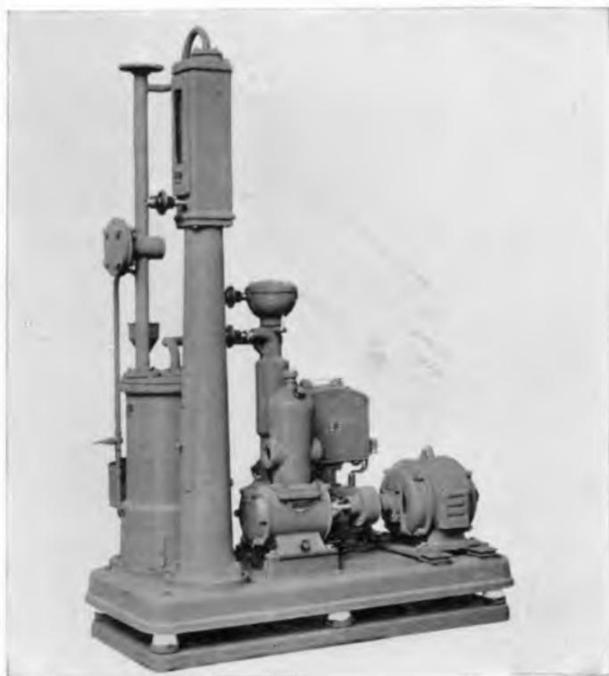
FIG. 70.—PUMPING EQUIPMENT OF METAL CASED MERCURY
