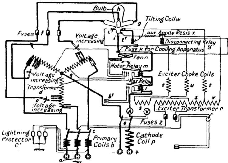
FIG. 66.—Normal Connections of Glass Bulb Rectifier.
