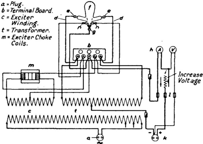
FIG. 80.—Connections of 5-10 amps. Accumulator Charging Rectifier.
