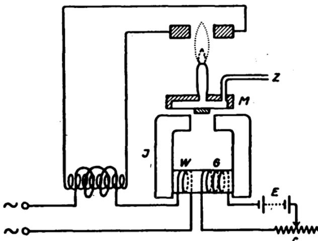
FIG. 52.—Connection of Vibrating Flame Rectifier of Dowling and Harris.
