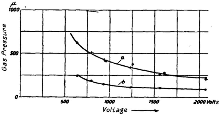
FIG. 64.—Dependence of Back-firing Voltage on Pressure.
