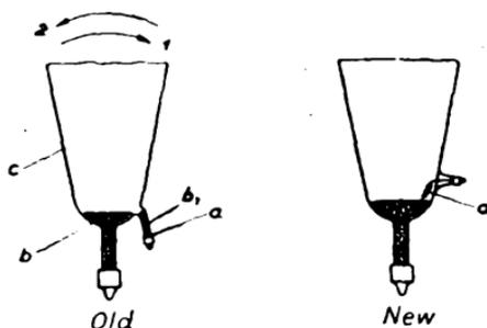
FIG. 67.—Old and New Construction of Exciting Anode.
