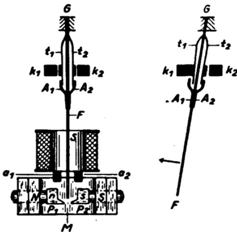
FIG. 49.—Construction of Pendulum Rectifier.
