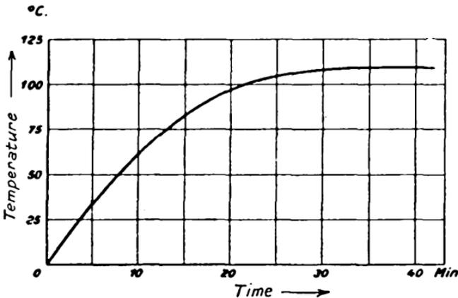
FIG. 71.—Rise of Temperature in a large Glass Bulb Rectifier.
