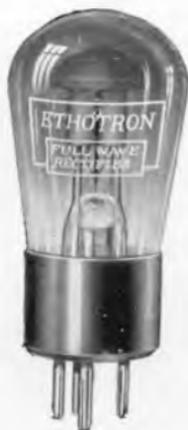
FIG. 59.—GLOW DISCHARGE RECTIFIER FOR H.T. BATTERY ELIMINATOR.
