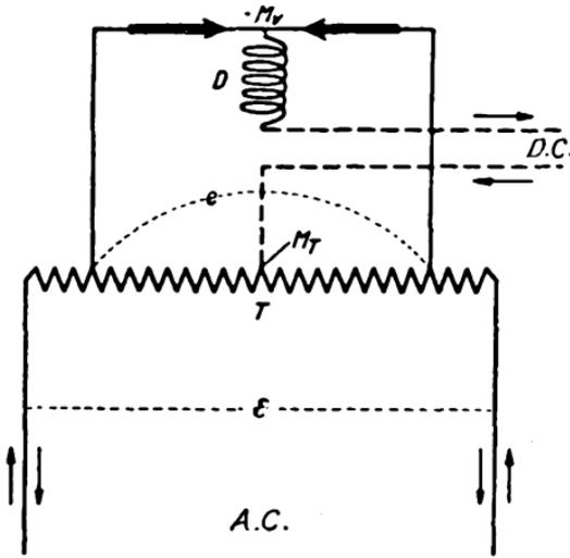
FIG. 34.—Transformer Circuit for Single-phase A.C.
