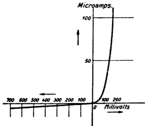
FIG. 27.—Current Voltage characteristic of a Lead Sulphide—Nickelin Detector (after Ettenreich).
