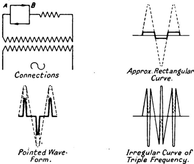
FIG. 94.—Production of any Wave Form.
