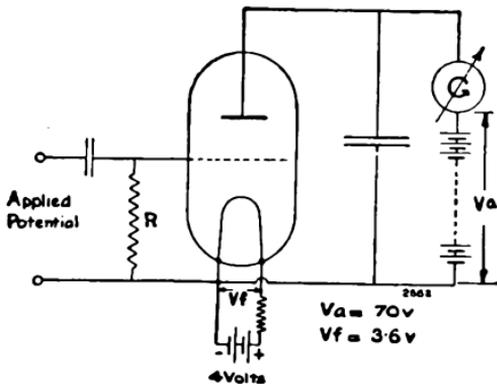
FIG. 91.—Connections of Moullin Voltmeter, Type B.
