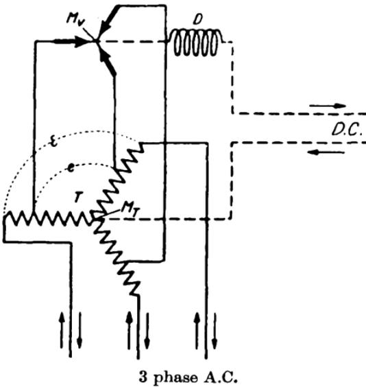
FIG. 35.—Transformer Circuit for Three-phase A.C.
