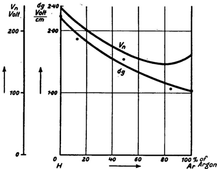
FIG. 7.—Variation of Normal Cathode Fall  $V_n$  and Normal Gradient  $\sigma_g$  with Composition of the Mixture of H<sub>2</sub>-Ar.
