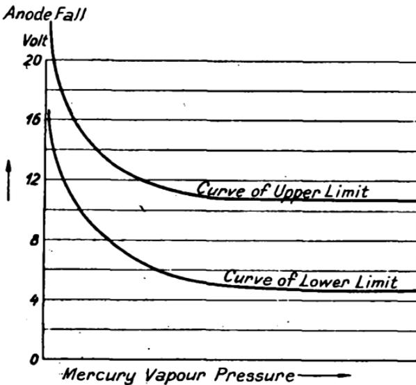
FIG. 11.—Dependence of Anode Fall on Mercury Vapour Pressure.
