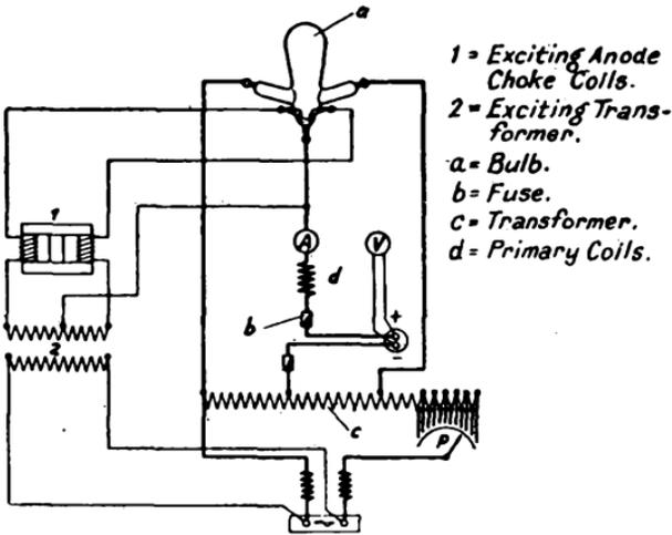
FIG. 77.—Single-phase Glass Bulb Rectifier, with Tapped Auto-transformer, for 20–60 Amps.
