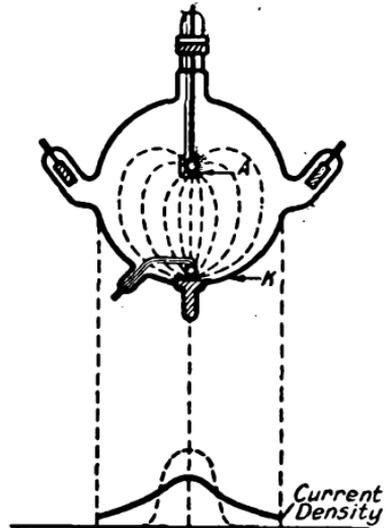
FIG. 9.—Current Lines of an Arc in a Large Vessel containing Pure Mercury Vapour.
