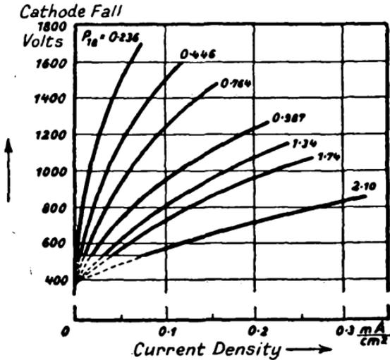
FIG. 23.—Dependence of Cathode Fall (Iron Cathode in Mercury Vapour) on Current Density and Pressure.
