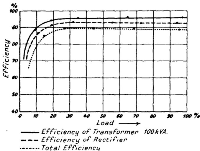
FIG. 68.—Efficiency of Transformer and Glass Bulb Rectifier.
