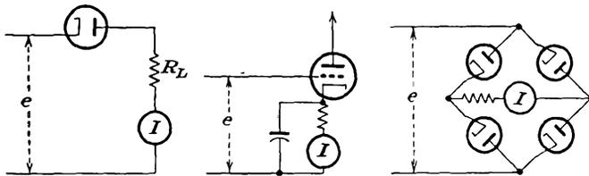
FIG. 22-4. The circuits of several average-reading vacuum-tube voltmeters.
