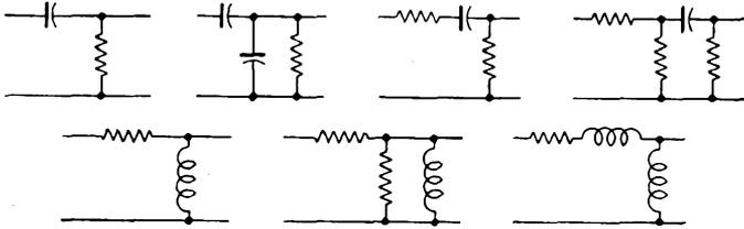
FIG. 7-17. Differentiation circuits with similar response characteristics.
