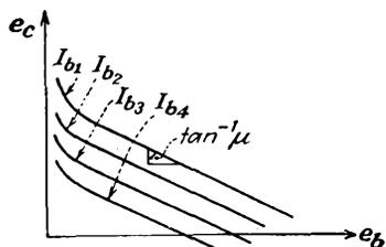
FIG. 2-8. The constant-current characteristics of a triode.
