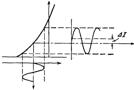
FIG. 22-3. Illustrating the operation of an rms voltmeter.
