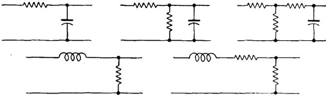
FIG. 7-18. Integrating circuits with similar response characteristics.
