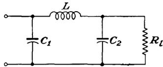
FIG. 14-15. A  $\Pi$ -section filter.
