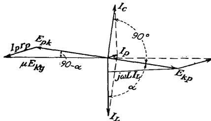
FIG. 12-6. The sinor diagram of a tuned-plate oscillator.
