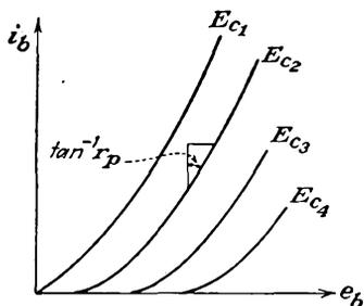
FIG. 2-6. The plate characteristics of a triode.
