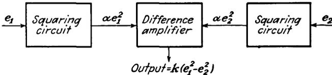
FIG. 8-13. Circuit for obtaining the difference of squares.
