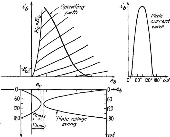
FIG. 11-7. The construction for determining the plate-current pulses in a class C amplifier.
