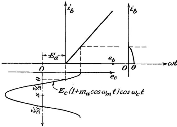
FIG. 16-5. The approximate action of a diode detector.
