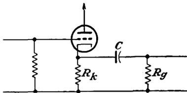
FIG. 6-13. The l-f circuit of the cathode-follower amplifier.
