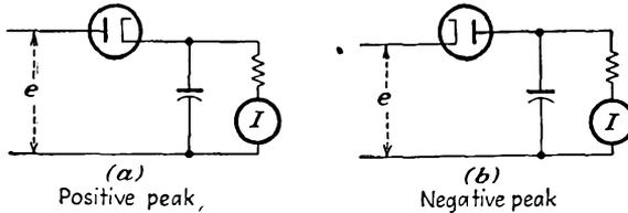
FIG. 22-5. Peak-reading voltmeters.
