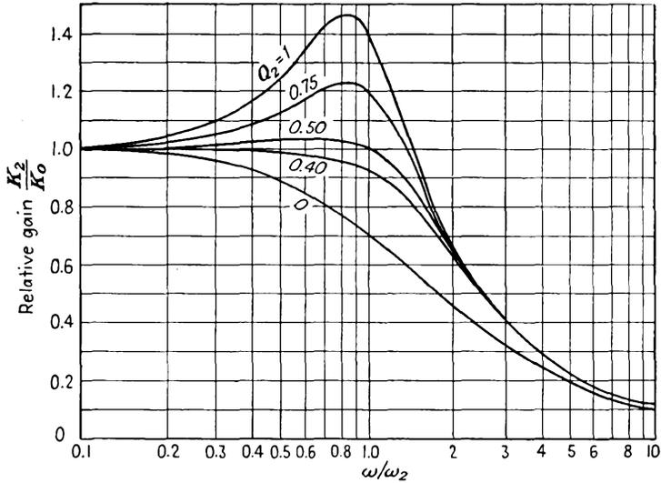
FIG. 6-5. Dimensionless relative gain curves for the shunt-compensated amplifier. (Adapted from Bedford and Fredendall.<sup>1</sup>)
