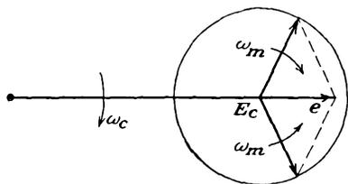
FIG. 17-20. The sinor representation of an a-m wave.
