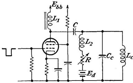
FIG. 21-5. An oscillatory sweep-current circuit with arrangements for adjusting the zero position of the sweep.
