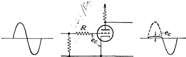
FIG. 7-6. Grid-circuit limiter.
