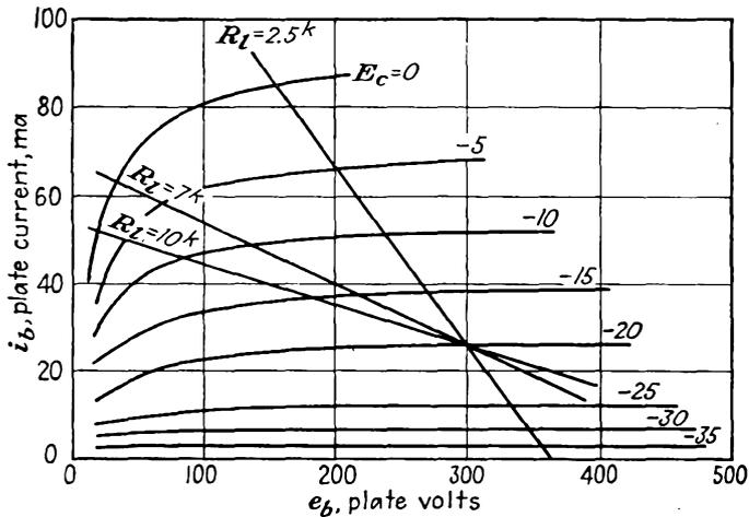
FIG. 9-11. Plate characteristics of a 6F6 power pentode.
