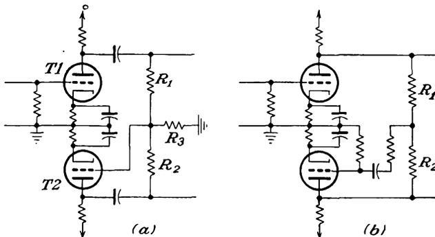
FIG. 9-27. Two forms of floating paraphase amplifiers.
