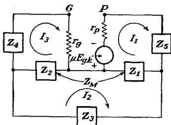
FIG. 12-9. The basic circuit of impedance stabilization.
