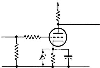
FIG. 7-8. A self-biased grid-circuit limiter.
