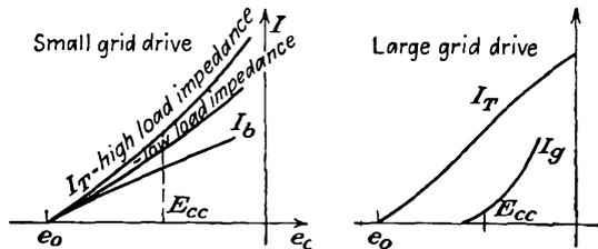
FIG. 15-13. Typical linearity curves of a grid-bias modulated class C amplifier under different conditions.
