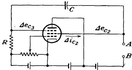
FIG. 12-23. A pentode circuit that exhibits a negative output resistance.
