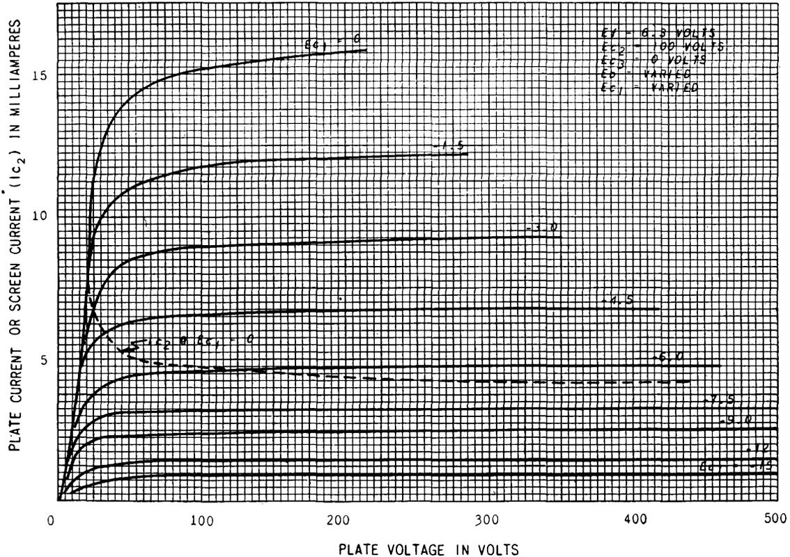
Fig. B-13. 6SK7 variable-mu pentode.
