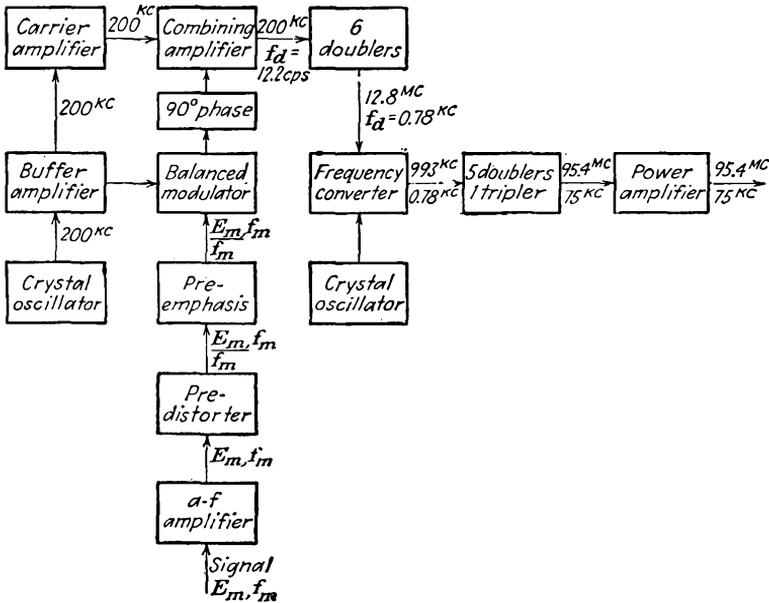
FIG. 17-22. Block diagram of an Armstrong f-m transmitter.
