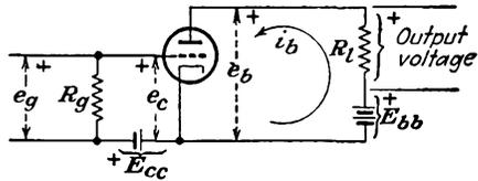
FIG. 3-1. The basic circuit of a triode amplifier.
