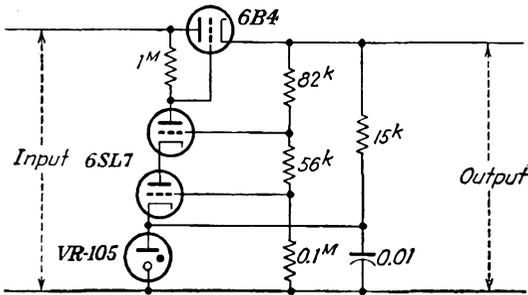
FIG. 14-24. A voltage regulator employing a "cascode" amplifier.
