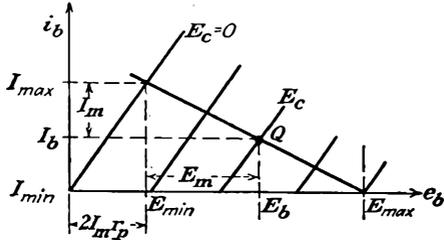
FIG. 9-10. The plate characteristics of an ideal tube.
