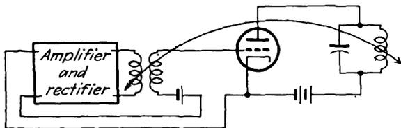
FIG. 12-14. A linear-stabilized oscillator.
