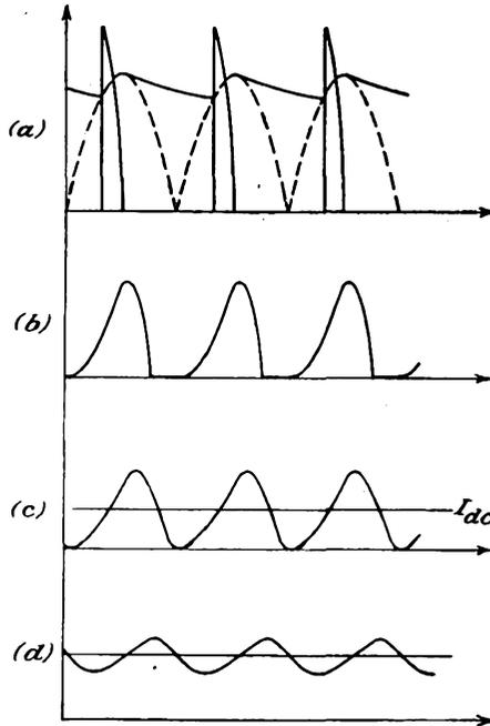
FIG. 14-10. The tube current in the full-wave rectifier with  $L$ -section filter, for (a)  $L = 0$ , (b)  $L$  less than critical inductance  $L_c$ , (c)  $L$  equal to  $L_c$ , (d)  $L$  greater than  $L_c$ .
