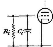
FIG. 4-5. The equivalent input circuit of a triode.
