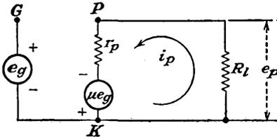
FIG. 3-6. The equivalent circuit of a triode.
