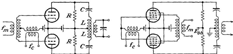
FIG. 15-8. Balanced modulators for producing suppressed carrier modulation.
