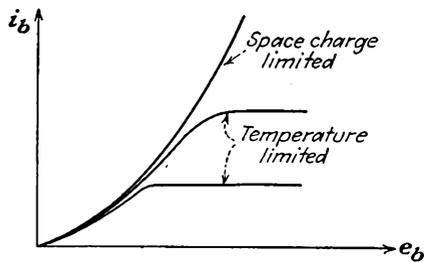
FIG. 2-2. The volt-ampere characteristics of a typical diode.
