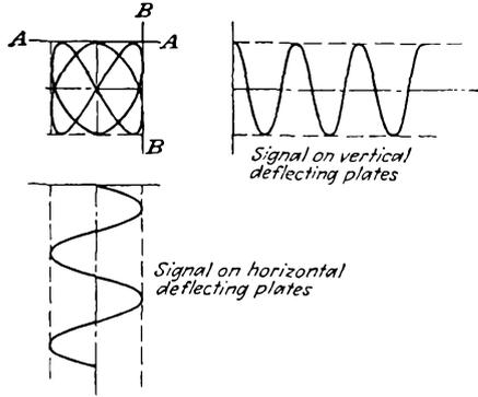
FIG. 22-21. Lissajous pattern for 2:3 frequency ratio.
