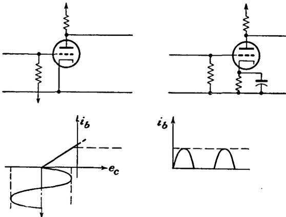
FIG. 7-10. Cutoff limiting in a strongly biased amplifier.
