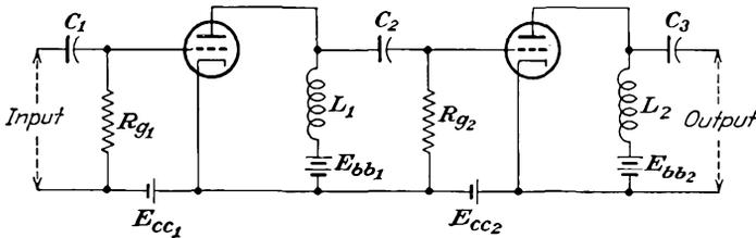
FIG. 5-9. Schematic diagram of an inductance-capacitance coupled amplifier.
