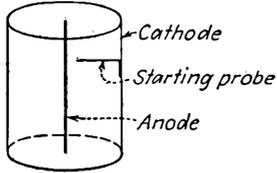
FIG. 2-20. Electrode structure in a VR tube.
