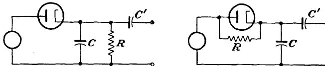
FIG. 16-3. Two circuits for envelope detection.
