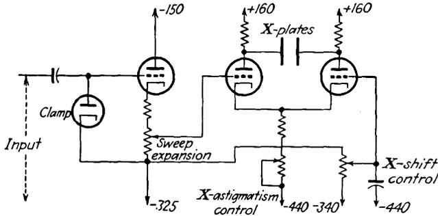
FIG. 20-28. A cathode-coupled paraphase amplifier with sweep expansion.
