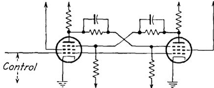
FIG. 19-16. Eccles-Jordan type of trigger circuit using pentodes.
