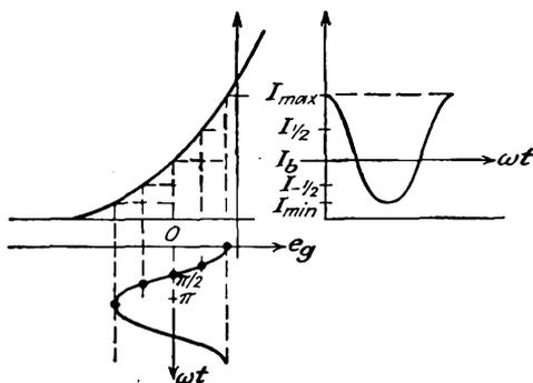
FIG. 3-12. The construction for obtaining the plate-current values to be used in the five-point schedule for determining the Fourier coefficients.
