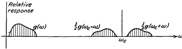
FIG. 15-4. The frequency spectrum of a complex wave.
