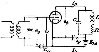
FIG. 11-1. Schematic diagram of a tuned power amplifier.
