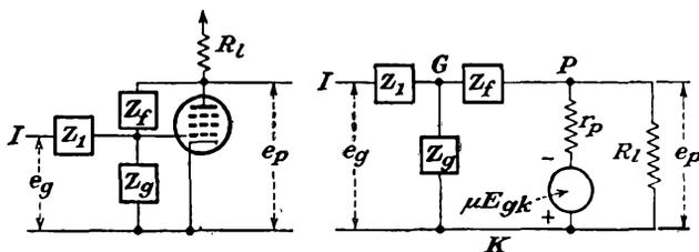
Fig. 6-15. A general feed-back circuit, and its equivalent circuit.
