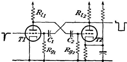
FIG. 19-1. A gate circuit with two a-c couplings.
