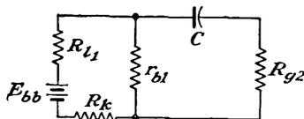
FIG. 19-7. The discharge circuit of the capacitor  $C$ .
