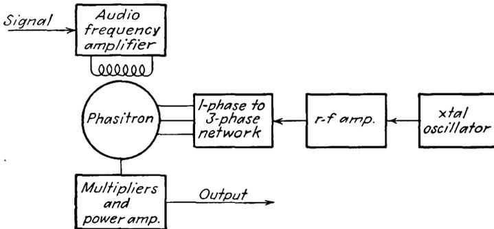
Fig. 17-26. The General Electric phasitron f-m transmitter.
