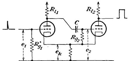
FIG. 19-5. A cathode-coupled gate.
