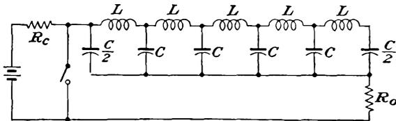
FIG. 19-39. The basic circuit incorporating a pulse-forming line.
