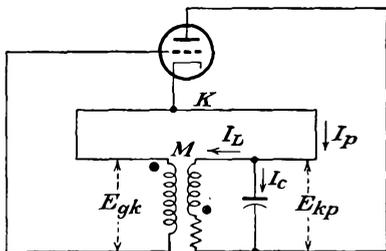
FIG. 12-5. Tuned-plate oscillator.
