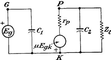
FIG. 4-8. The equivalent circuit of a pentode amplifier.
