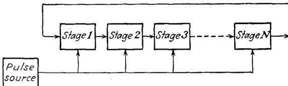
FIG. 19-21. Block diagram of a conventional ring counter.
