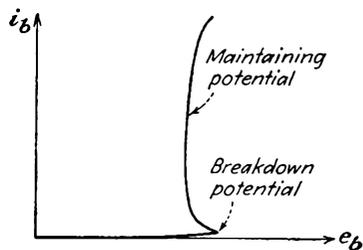
FIG. 2-19. Volt-ampere characteristic of a glow discharge.
