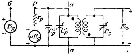
FIG. 10-5. The equivalent circuit of a double-tuned amplifier.
