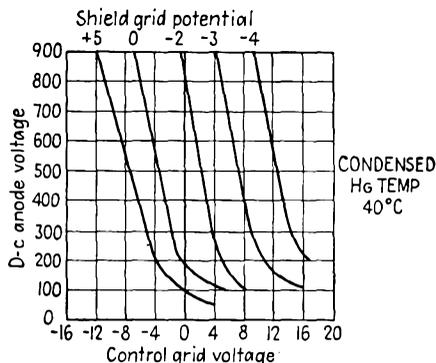
FIG. 2-29. Control characteristics of an FG-98 shield-grid thyatron.
