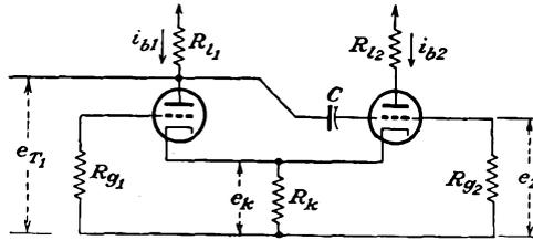
FIG. 18-13. A cathode-coupled multivibrator using direct coupling.
