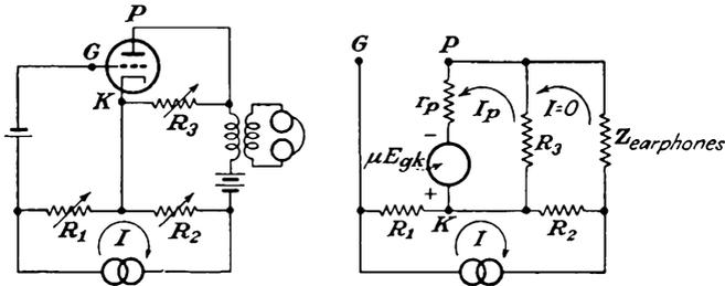
FIG. 3-9. The Miller bridge from determining the transconductance of a triode under operating conditions.
