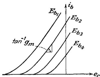
FIG. 2-7. The transfer characteristics of a triode.
