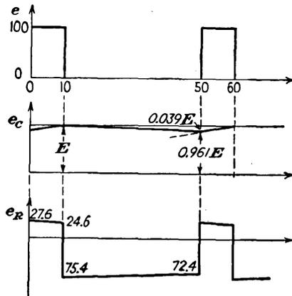
figure. These sketches show the potential variations across the capacitor and across the grid-cathode resistor after steady-state conditions have been reached.
