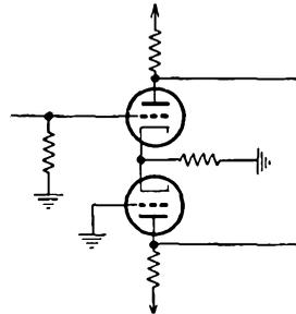
FIG. 20-27. A cathode-coupled paraphase amplifier.
