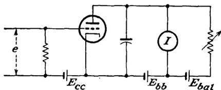
FIG. 22-1. The basic circuit of a vacuum-tube voltmeter.
