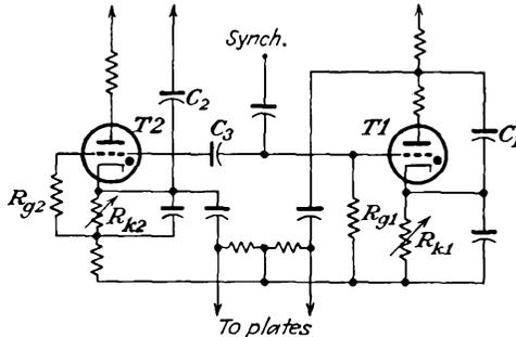
FIG. 20-31. Two thyatron saw-tooth generators operating in push-pull.
