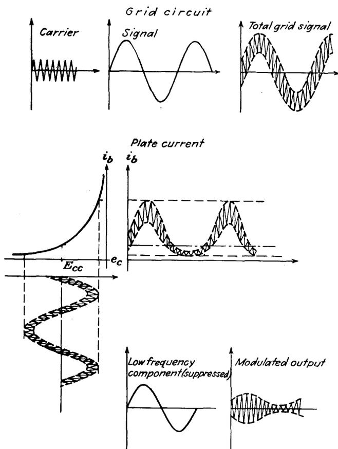
FIG. 15-6. The wave shapes at various points in the van der Bijl modulator.
