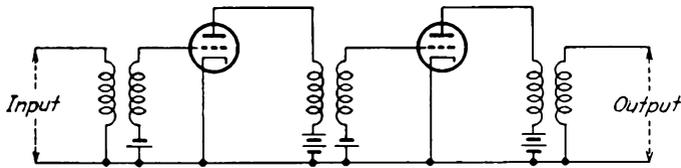
FIG. 5-11. Schematic diagram of a transformer-coupled amplifier.
