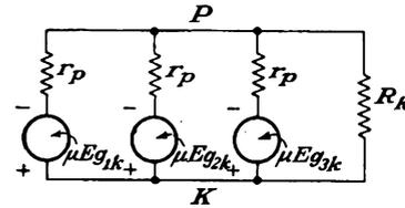
FIG. 8-8. The equivalent circuit of Fig. 8-7.
