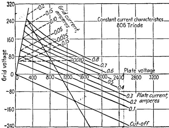
Fig. 11-12. Constant-current characteristics of an 806 triode.
