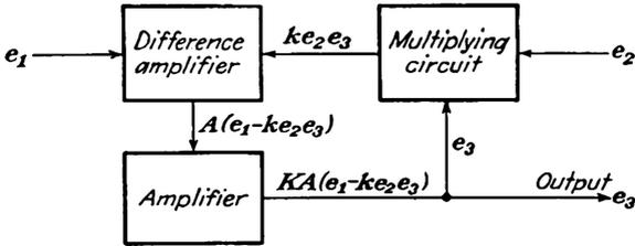
FIG. 8-15. A circuit which divides two voltages.
