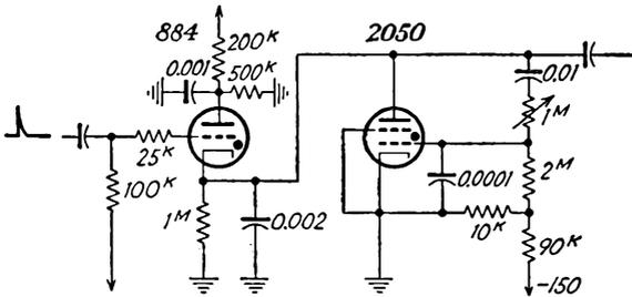
FIG. 19-37. A thyatron pulse generator with thyatron clipper.
