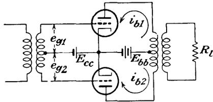
FIG. 9-14. The basic push-pull circuit.
