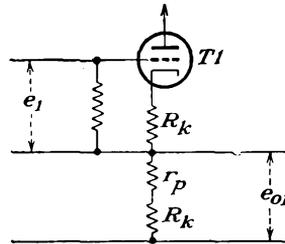
FIG. 8-4. The operating circuit of tube  $T_1$ .
