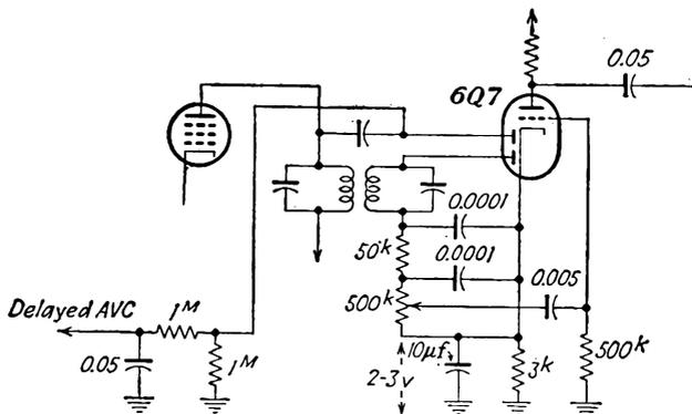
FIG. 16-13. A diode detector and delayed automatic-volume-control circuit.
