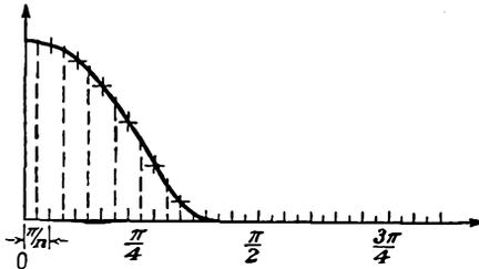
FIG. 11-11. Current wave form and its approximate representation.
