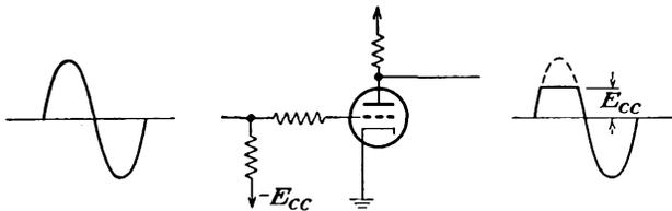
FIG. 7-7. Grid-circuit limiting about a fixed potential level.
