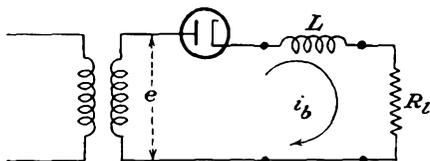
FIG. 14-1. Half-wave rectifier circuit with choke filter.
