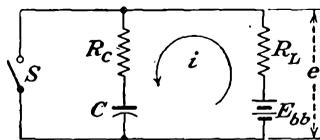
FIG. 21-9. A circuit for generating a trapezoidal wave.
