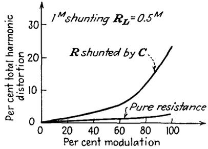
FIG. 16-10. Variation of distortion with per cent modulation. (From F. Langford Smith, "Radiotron Designer's Handbook," Chap. 18.)
