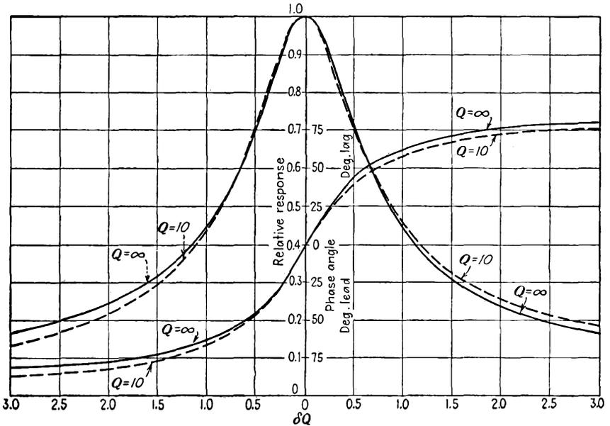
FIG. 10-3. Plots showing the amplitude  $K/K_{res}$  and phase of the output of the single-tuned direct-coupled amplifier. (From Terman, F. E., *Radio Engineering*, 3d ed., McGraw-Hill Book Company, Inc., New York, 1947.)
