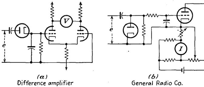
FIG. 22-6. Diode peak voltmeters with d-c amplifier.
