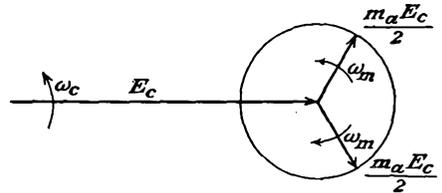
FIG. 15-3. The sinor representation of an a-m wave.
