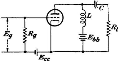
FIG. 9-4. A parallel or shunt-fed power amplifier.
