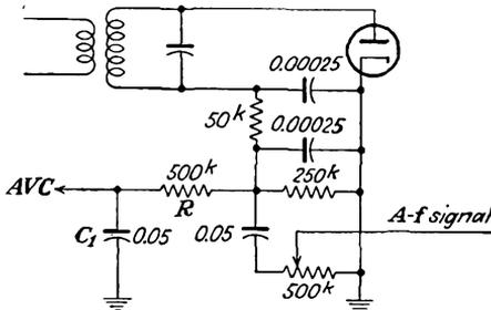
FIG. 16-12. A diode detector and automatic-volume-control circuit.
