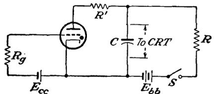
FIG. 20-6. A saw-tooth generator employing a thyatron.
