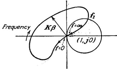
FIG. 5-25. The polar plot of an amplifier.
