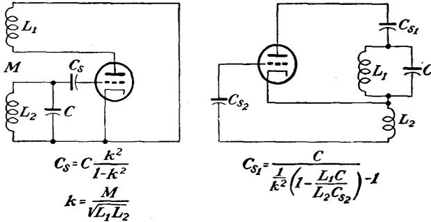
FIG. 12-11. Impedance-stabilized oscillators.
