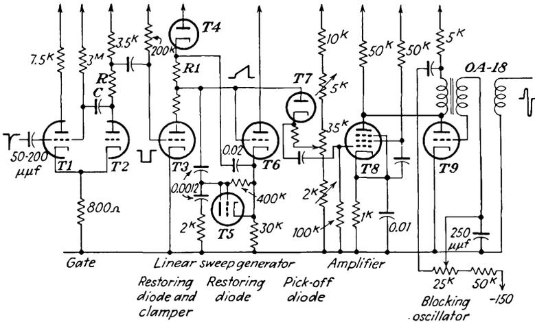
FIG. 19-35. A 150- $\mu$ sec linear-sweep delay circuit.
