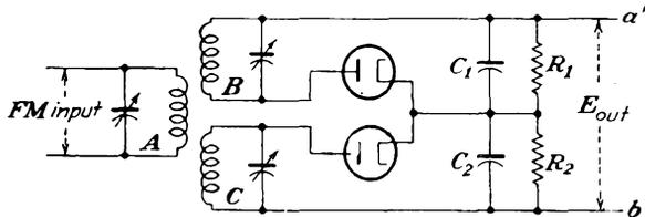
FIG. 17-30. A discriminator employing two stagger-tuned circuits.
