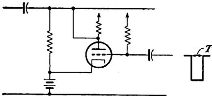
FIG. 7-33. A one-way clamp using a single triode.
