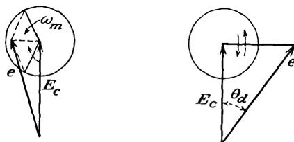
FIG. 17-21. The sinor representation of a p-m wave.
