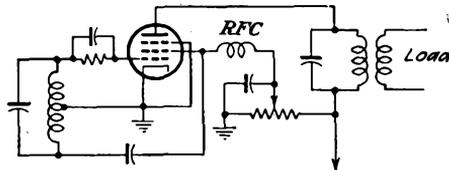
FIG. 12-8. Electron-coupled oscillator.
