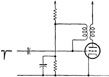
FIG. 19-38. A triggered blocking oscillator for pulse generation.
