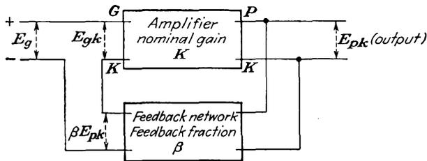
FIG. 5-16. The principle of feedback in amplifiers.
