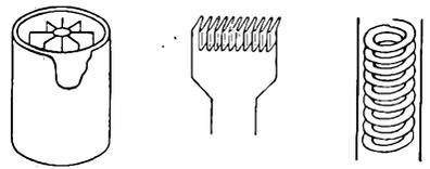
FIG. 1-4. Different types of heat-shielded cathodes.
