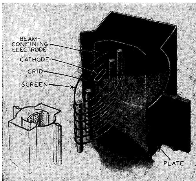
FIG. 2-18. Schematic view of the shapes and arrangement of the electrodes in a beam power tube. (RCA Mfg. Co.)
