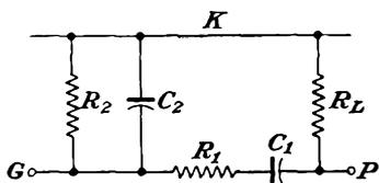
FIG. 12-16. An RC coupling network for an oscillator.
