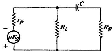
FIG. 5-5. The l-f equivalent circuit of the RC amplifier.
