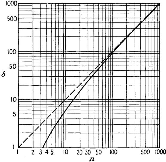
FIG. 17-8. Values of  $n$  for a given value of  $\delta$  to make  $J_n(\delta) < 0.01$ . Note that  $n$  may assume only integral values. (From L. Mautner, "Mathematics for Radio Engineers," Pitman Publishing Corp., New York, 1947.)
