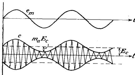
FIG. 15-1. The modulating signal and a modulated carrier.
