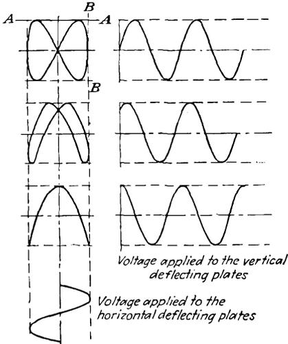
FIG. 22-20. Lissajous figure for 1:2 frequency ratio.
