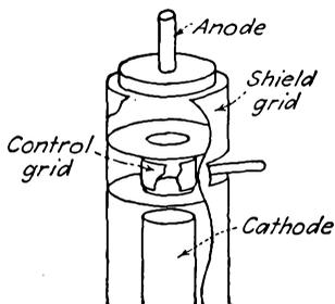
FIG. 2-28. Electrode structure of the FG-98 shield-grid thyatron.
