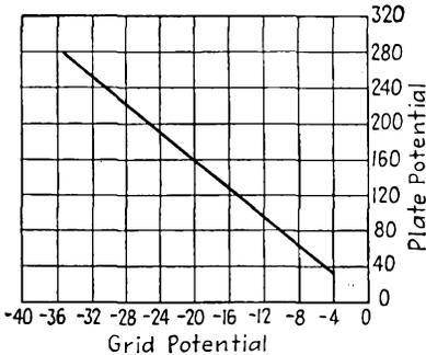
FIG. 2-27. Critical grid characteristic of an 884 argon-filled thyatron.
