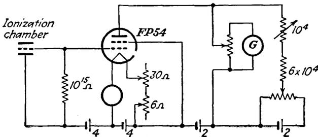
FIG. 22-13. An electrometer circuit using an FP-54 tube.
