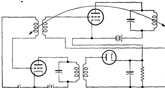
FIG. 12-15. The circuit of a linear-stabilized oscillator.
