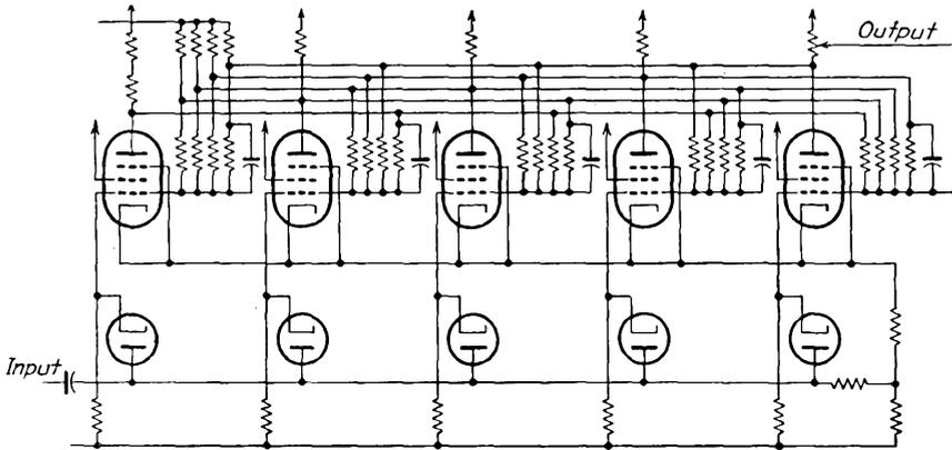
FIG. 19-22. The General Electric scale-of-5 ring circuit.
