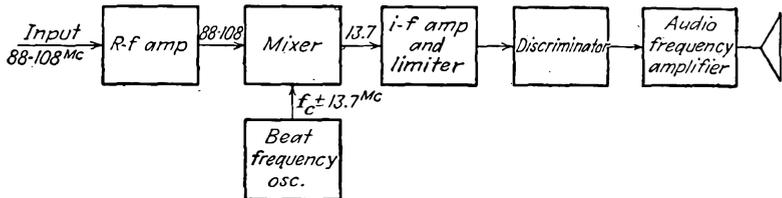
FIG. 17-27. Block diagram of a typical f-m receiver.
