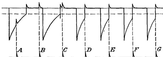
FIG. 18-25. Synchronizing a multivibrator with positive pulses.
