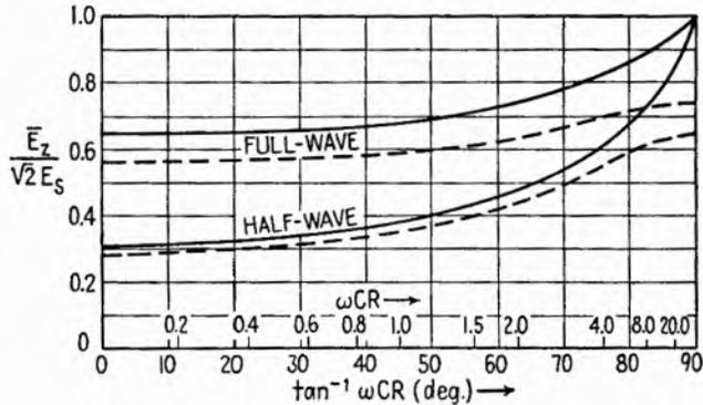
FIG. 2.6.—Relation between average load voltage and characteristic angle of parallel  $RC$  circuit supplied by a rectifier (average load voltage  $\bar{E}_z = \bar{E}_R$  is referred to peak of applied voltage,  $\sqrt{2} E_s$ ). Solid curves are for tube drop = 0; dotted curves are for load resistance/rectifier resistance = 10.
