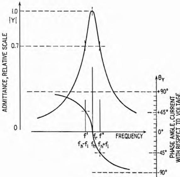
FIG. 10.1.—Admittance and phase-angle curves for a high- $Q$  LC circuit, with an amplitude spectrum of the induced voltage of (10.1) shown on the frequency axis.
