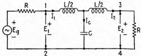
FIG. 2.2.—Filtering network introduced between generator and load of Fig. 2.1.
