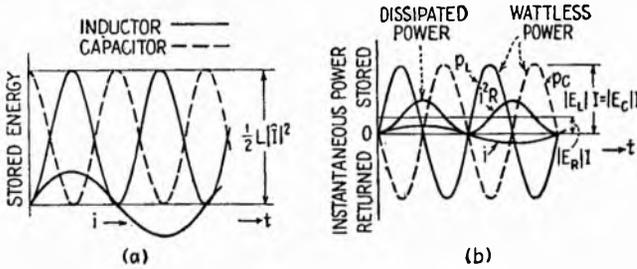
FIG. 9.1.—Stored energy and power variations at resonance.
