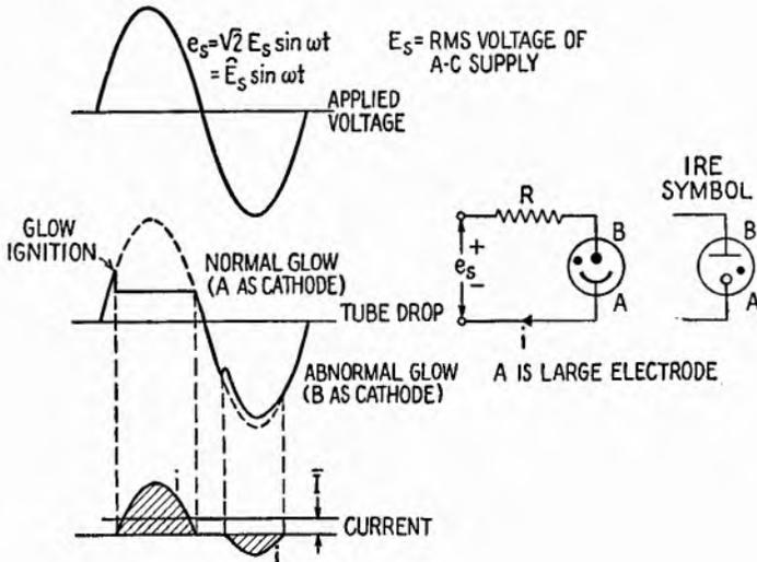
FIG. 2.3.—Glow-tube rectification.
