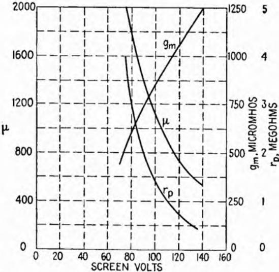
FIG. 15.3.—Effects of screen-grid voltage on  $\mu$ ,  $g_m$ , and  $r_p$  for a screen-grid tetrode
