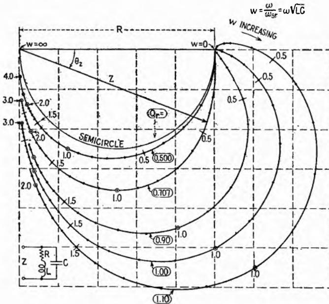
FIG. 16.2.—Impedance variations for parallel circuits having very low values of  $Q_r$ . of  $Q_r$  (approx. 0.57) would ensure linear variation of the phase angle over a wide range of frequencies beginning at zero.<sup>1</sup>
