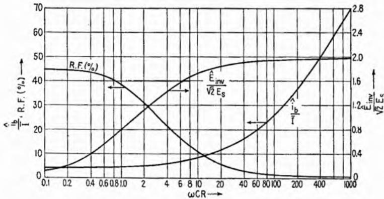
FIG. 4.4.—Full-wave-voltage-doubler characteristics. R.F. = ripple factor;  $\hat{E}_{inv}$  = peak inverse voltage;  $\hat{i}_b$  = peak current per tube;  $\bar{I}$  = average load current;  $E_s$  = rms applied voltage.
