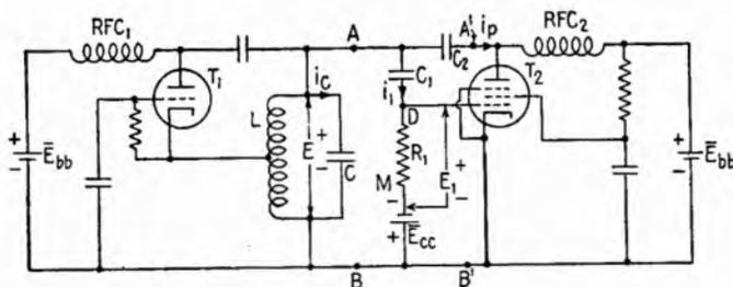
FIG. 10.1.—Reactance-tube circuit attached to a Hartley oscillator.
