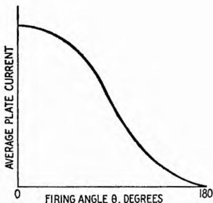
FIG. 5.4.—Control of average current of a thyatron.
