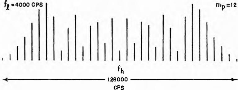
FIG. 8.3.—Amplitude spectrum for a phase-modulated wave as the modulation frequency  $f_1$  increases;  $m_p$  is constant and chosen to yield at  $f_1 = 1,000$  cps the same spectrum as in Fig. 8.2a.
