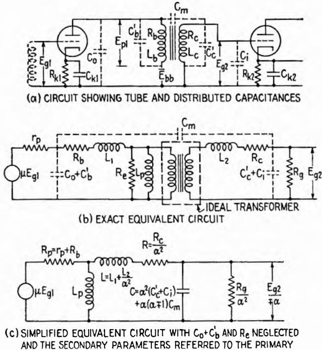
FIG. 22.2.—Untuned transformer-coupled amplifier stage and equivalent circuits.
