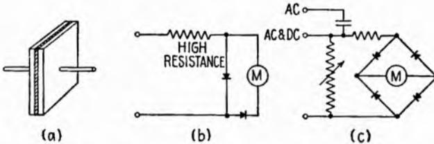
FIG. 5.1.—Rectifier units employed for a-c measurements.
