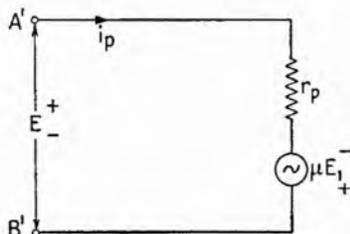
FIG. 10.2.—Equivalent plate circuit of a reactance tube.
