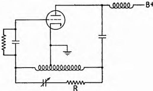
FIG. 6.1.—Output obtained by loading the tank circuit.
