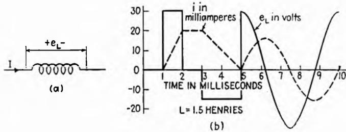
FIG. 7.1.—Ideal inductor and its instantaneous current-voltage relations.
