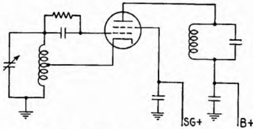
FIG. 6.3.—Electron-coupled oscillator.
