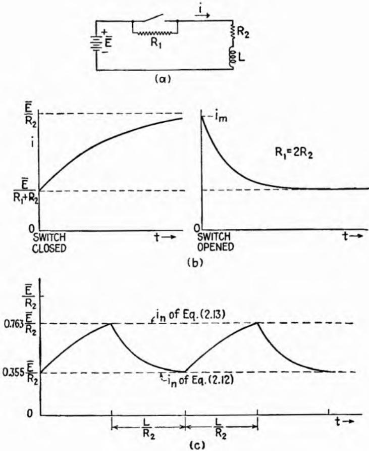
FIG. 2.6.—(a) Circuit containing resistance and inductance; (b) graph of current through  $R_2$  and  $L$  when the switch is closed and opened again; (c) graph of current through  $R_2$  and  $L$  when the switch is closed and opened repeatedly at the interval indicated.
