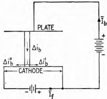
FIG. 3.1.—Division of space current in the filament.
