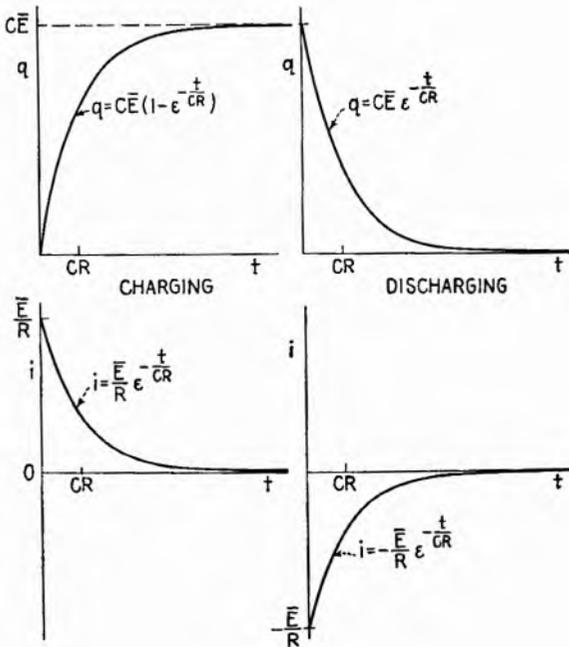
FIG. 3.14.—Curves of charge and current for a charging operation and a discharging operation.
