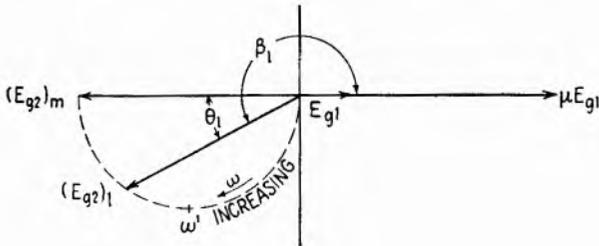
FIG. 10.3.—Polar relation of  $E_{o2}$  to  $E_{o1}$  at low frequencies in a resistance-coupled stage.
