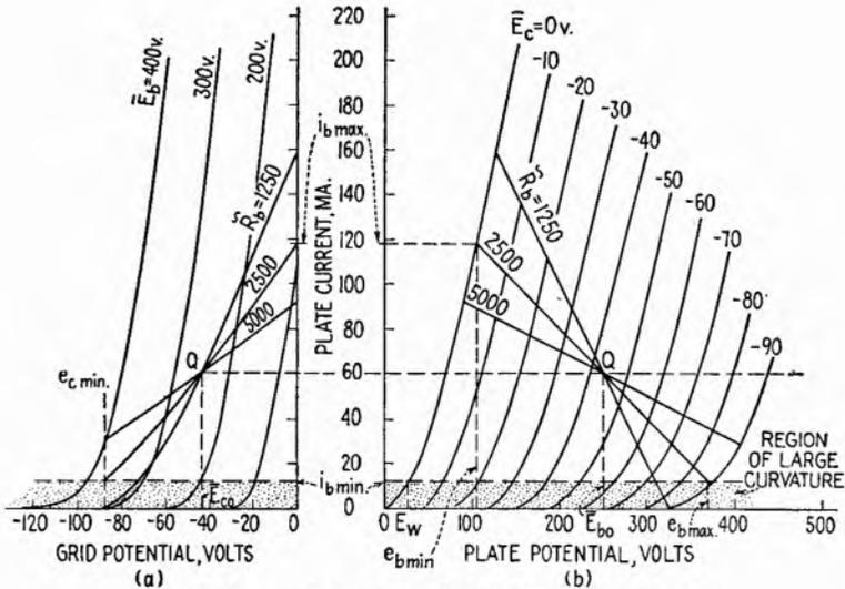
FIG. 23.1.—A typical power triode in Class A<sub>1</sub> operation.
