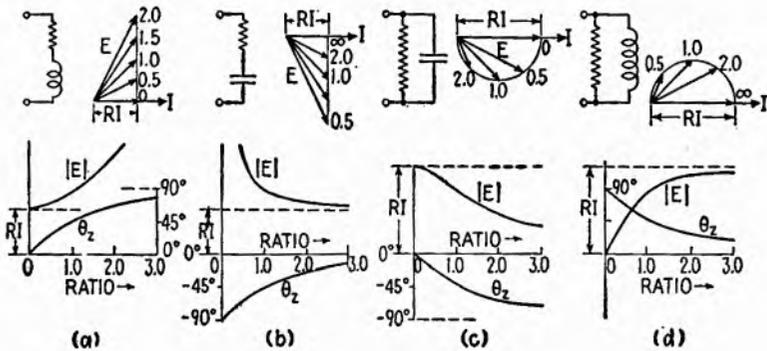
FIG. 3.1.—Voltage variation across  $LR$  and  $CR$  loads driven by a constant-current generator.  $R$  is constant. Numerical scale is ratio  $\omega/\omega'$ ,  $L/L'$ , or  $C/C'$ , according to which is the variable.
