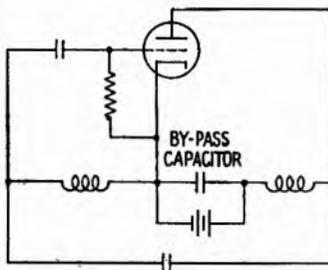
FIG. 4.1.—Series feed with battery at cathode potential.
