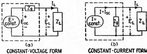
FIG. 16.1.—Alternative descriptions of a linear a-c generator.
