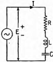
FIG. 8.1.—Series circuit.
