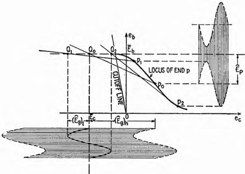
FIG. 18.2.—Grid modulation of a Class C amplifier.
