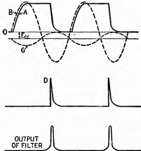
FIG. 12.2.—Performance of thyatron pulse circuit of Fig. 12.1.
