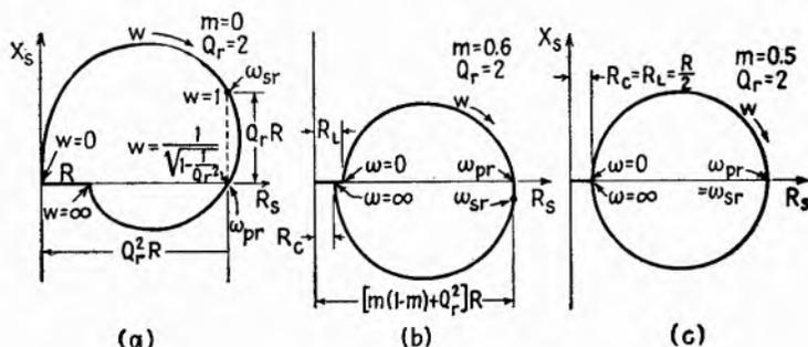
FIG. 17.1.—Impedance variations for a parallel circuit (a) with all the resistance in the capacitive branch,  $m = 0$ ; (b) with unequal division of resistance,  $m = 0.6$ ; (c) with equal division of resistance,  $m = 0.5$ .
