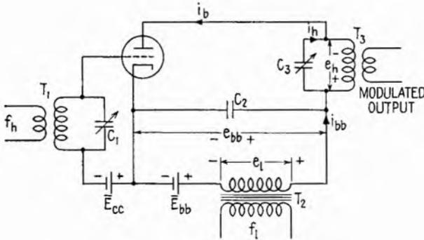
FIG. 2.1.—Basic diagram of a plate-modulated Class C amplifier.
