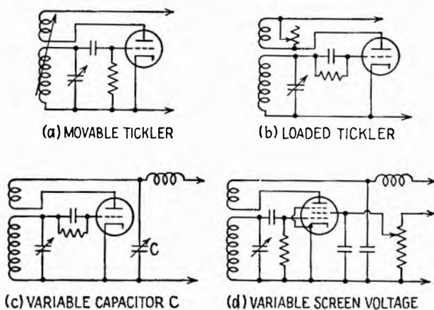
FIG. 2.2.—Methods for control of regeneration.
