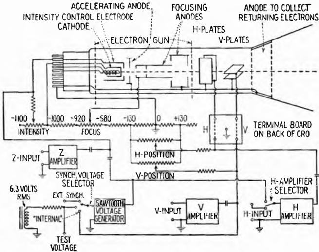
FIG. 8.1.—Block and circuit diagram of composite oscillograph.
