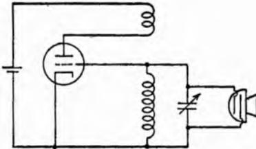
FIG. 9.1.—Condenser-microphone method of frequency modulation.
