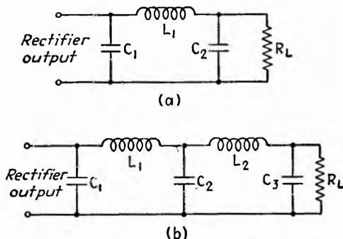
FIG. 11.1.—Capacitor-input filters: (a) one-section and (b) two-section.
