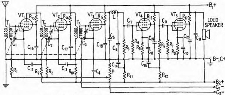
FIG. 4.1.—Tuned-radio-frequency (TRF) receiver.
