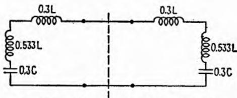
FIG. 19.5.—Example of  $m$ -derived II section.
