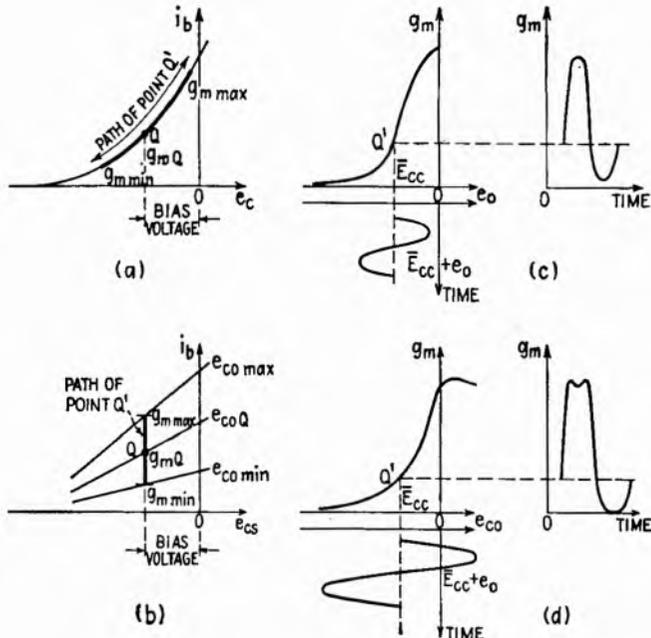
FIG. 6.1.—Operation of frequency converters; (a) and (b): movement of  $Q$  point in single- and double-input converters; (c) and (d): variation in value of  $g_m$  in single- and double-input converters.
