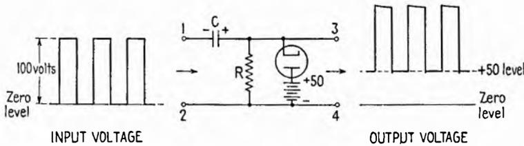
FIG. 20.4.—Bottom of wave clamped at +50-volt level.
