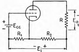
FIG. 13.3.—Amplification-factor stabilizer.
