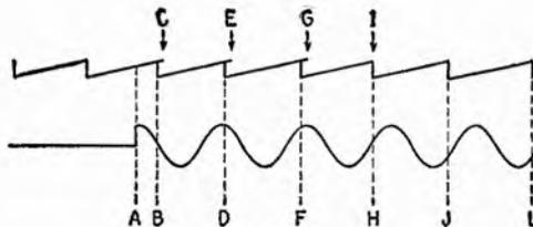
FIG. 4.2.—Synchronization process.
