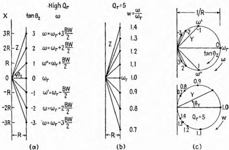
FIG. 11.2.—Variation of  $Z$  and  $Y$  as related to  $\tan \theta_z$  and  $\omega$  for a high- $Q_r$  series  $LCR$  circuit and to  $w$  for a low- $Q_r$  series circuit.
