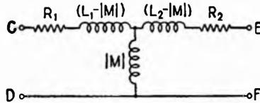
FIG. 4.3.—Equivalent T for the transformer of Fig. 3.1.
