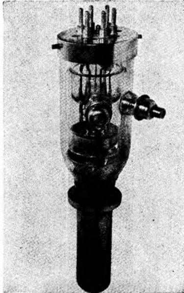
FIG. 1.2.—Water-cooled tube.
