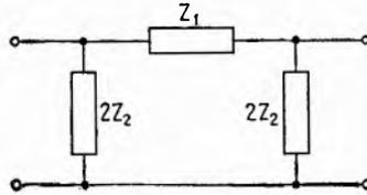
FIG. 15.1.—Symmetrical  $\Pi$ -section filter.
