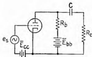
FIG. 3.4.—Vacuum-tube circuit in which the a-c load resistance is less than the d-c load resistance ( $\bar{R}_L < \bar{R}_L$ ).
