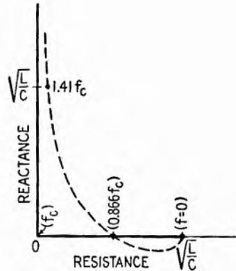
FIG. 4.4.—Variations with frequency of the characteristic impedance  $Z_c$  (heavy solid lines) of a one-section low-pass filter, and of the input impedance  $Z_i$  (dotted line) when the termination is  $R = \sqrt{L/C}$  as in Fig. 3.4.
