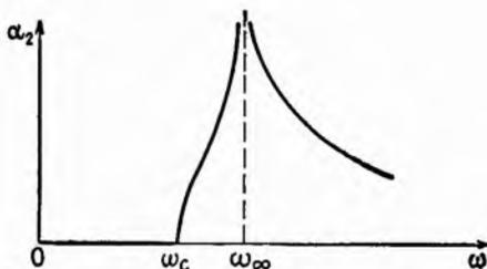
FIG. 19.2.—Attenuation constant of  $m$ -derived filter section.
