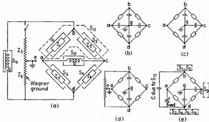
FIG. 4.1.—(a) Bridge with shielded impedances and a Wagner ground; (b) Wagner ground disconnected and all shields grounded; (c) terminal  $a$  grounded also; (d) Wagner ground connected and adjusted; (e) Wagner ground removed,  $S_{12}$  added and connected to terminal  $d$ , and other shields connected as shown.
