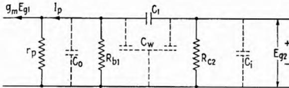
FIG. 8.2.—Equivalent plate circuit using a constant-current generator.
