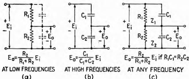
FIG. 6.1.—Voltage-divider circuits.
