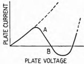
FIG. 13.5.—Dynatron characteristics.
