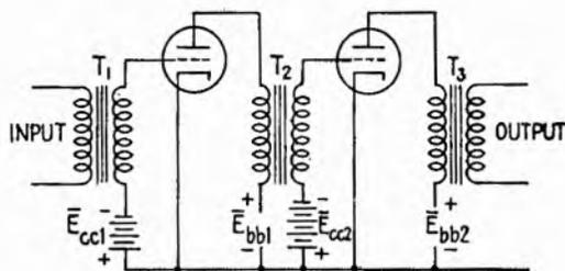
FIG. 22.1.—Two-stage audio-frequency transformer-coupled amplifier.
