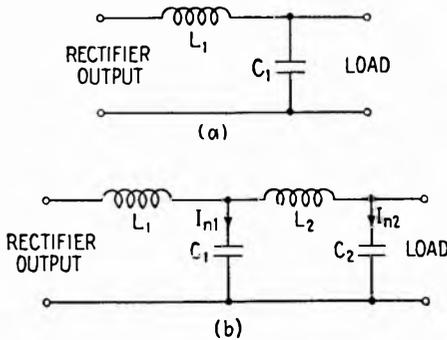
FIG. 8.1.—Choke-input filters: (a) one-section and (b) two-section.
