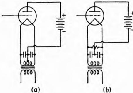
FIG. 3.2.—Plate-circuit connections to the cathode heating circuit.
