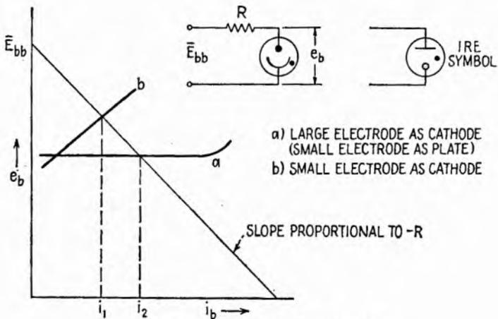
FIG. 2.2.—Glow-tube characteristics.
