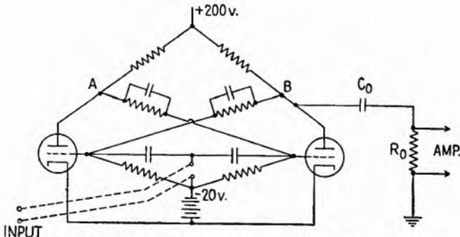
FIG. 27.6.—One method of obtaining an output voltage.
