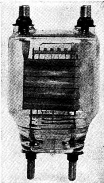
FIG. 1.1.—Radiation-cooled tube.
