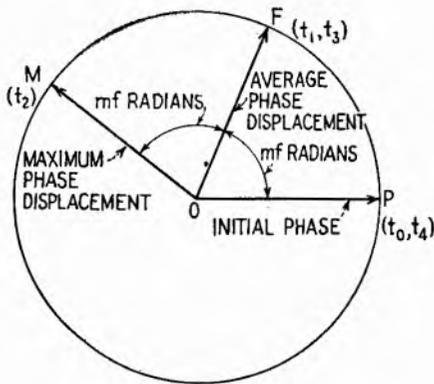
Fig. 8.1.—Motion of a vector representing a frequency-modulated current resulting from sinusoidal modulation, with  $f_h$  rps subtracted from its motion.
