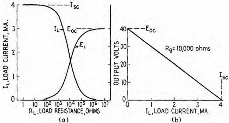
FIG. 1.2.—Load characteristics of a particular d-c generator.
