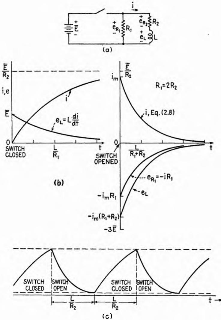
FIG. 2.5.—(a) Circuit containing resistance and inductance; (b) graph of current through  $R_2$  and  $L$  when the switch is closed and opened again; (c) graph of current through  $R_2$  and  $L$  when switch is closed and opened repeatedly at the interval indicated.
