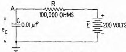
FIG. 2.1.—Basic circuit.
