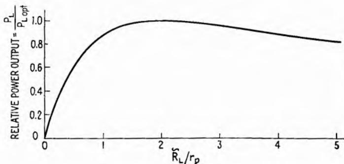
FIG. 23.2.—Theoretical relative power output from a triode in Class  $A_1$  linear operation as a function of  $\bar{R}_L / r_p$ .
