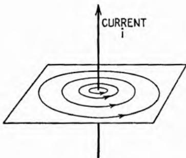
FIG. 11.2.—Magnetic field about a long straight current.
