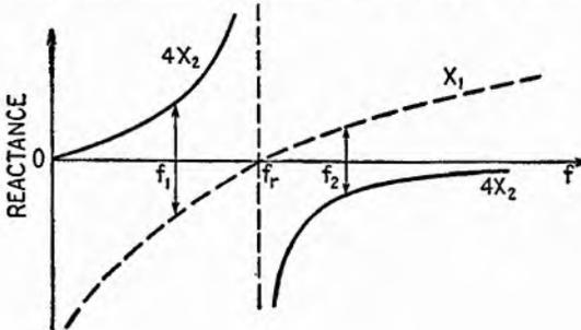
FIG. 13.2.—Variations with frequency of  $X_1$  and  $4X_2$ .
