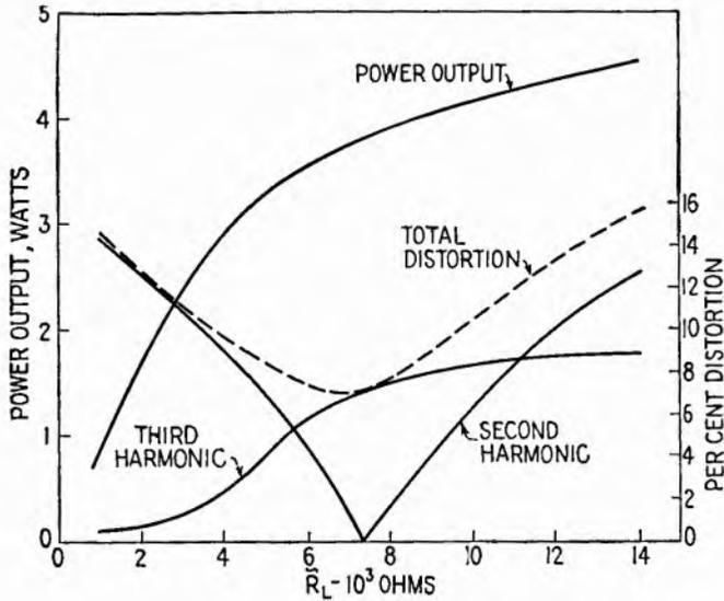
FIG. 23.6.—Power output of the pentode of Fig. 23.5.
