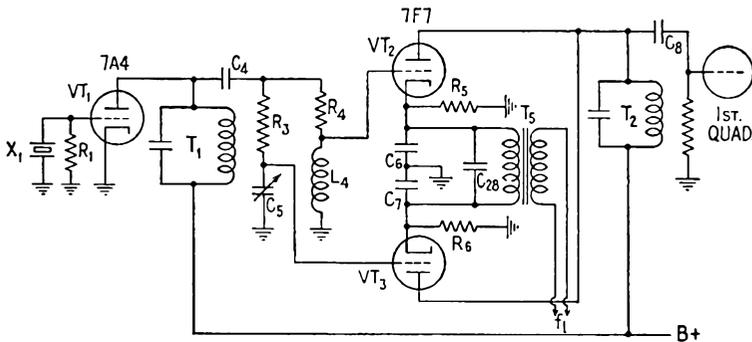
FIG. 11.2.—An example of a phase-shift modulator circuit.
