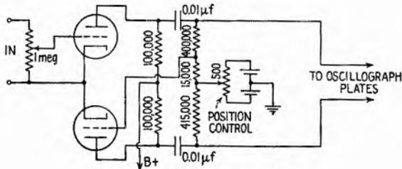
FIG. 11.3.—Phase inverter.
