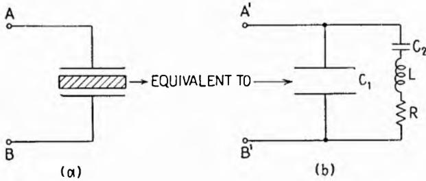
FIG. 8.1.—Equivalent circuit of crystal in its holder.
