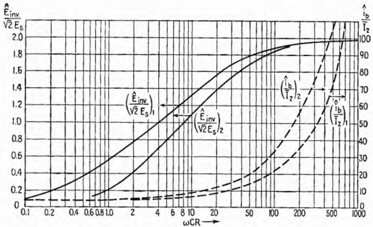
FIG. 4.7.—Peak inverse voltage and peak tube currents of half-wave voltage doubler.  $E_s =$  rms a-c supply voltage;  $\hat{E}_{inv}$  = peak inverse voltage per tube;  $\hat{i}_b$  = peak tube current;  $I_2 =$  average load current; subscripts 1 and 2 refer to tubes  $T_1$  and  $T_2$ .
