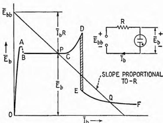
FIG. 1.1.—Gas-discharge characteristics.
