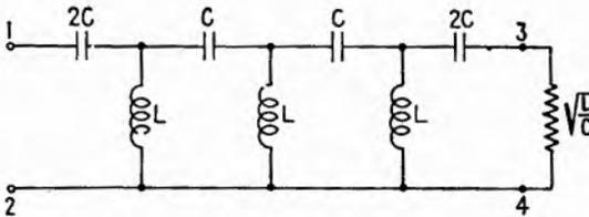
FIG. 8.4.—A three-section high-pass filter.
