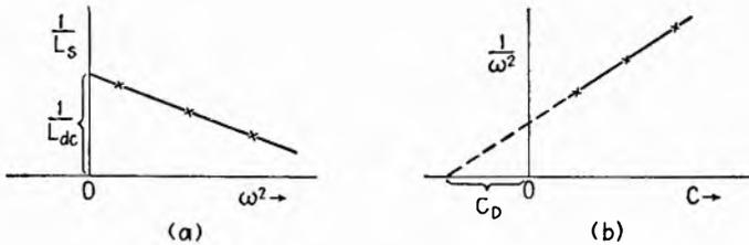
FIG. 7.1.—Evaluation of equivalent circuit constants.
