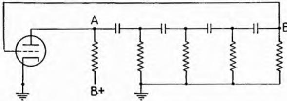
FIG. 11.1.—Phase-shift oscillator.
