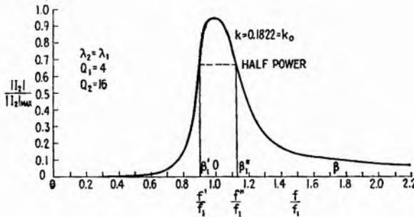
FIG. 18.1.—Variations in secondary current at optimum coupling.
