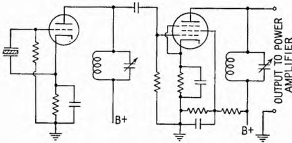
FIG. 6.2.—Use of buffer amplifier to isolate oscillator.
