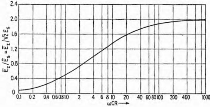
FIG. 4.3.—Ratio of average output voltage of full-wave voltage doubler to peak a-c, as function of load  $\omega CR$ ;  $\omega$  = supply fundamental,  $2\pi f$ .
