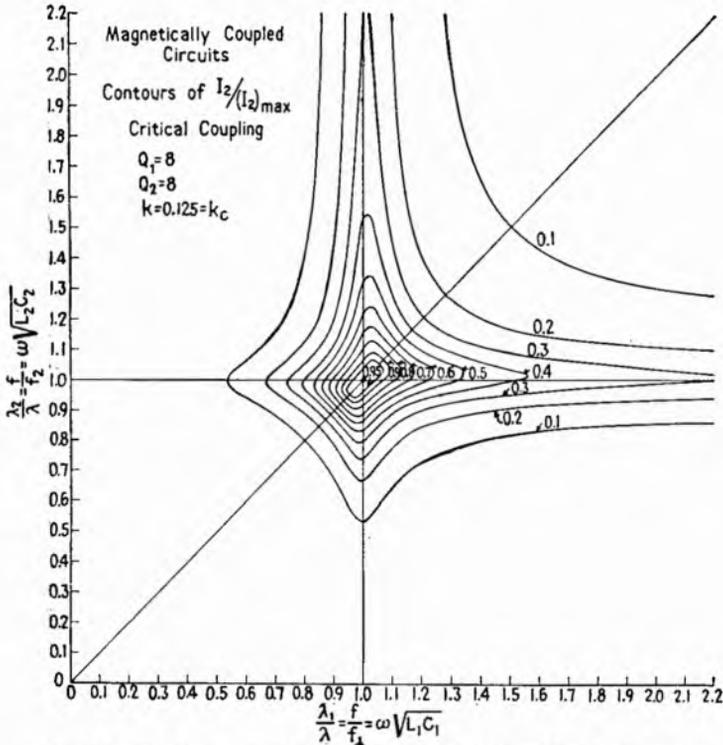
FIG. 9.6.—Contour curves of model of Fig. 9.2;  $Q_1 = Q_2$ ,  $k = k_{critical}$ .
