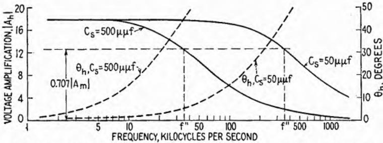
FIG. 11.2.—High-frequency response of a resistance-coupled amplifier stage.
