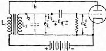
FIG. 14.1.—Blocking oscillator.
