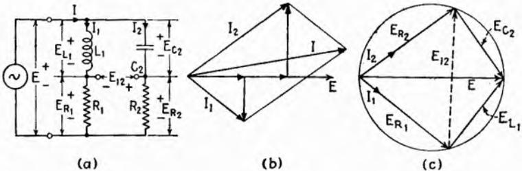
FIG. 15.1.—Two-branch parallel circuit and its current-voltage relations.
