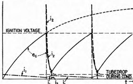
FIG. 4.4.—For the circuit of Fig. 4.3, graphs versus time of voltage  $e_c$  across the capacitor (solid line), current  $i_2$  through  $R_2$  (dash line), and current  $i_1$  through  $R_1$  (dot-dash line).
