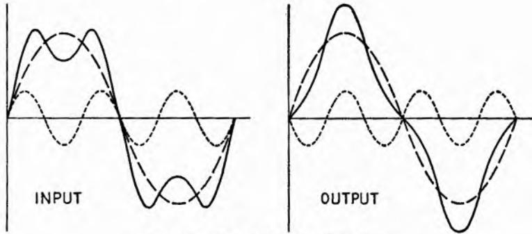
FIG. 3.3.—Effect of phase distortion.
