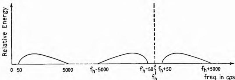
FIG. 4.2.—Possible time-average energy spectrum of a complex modulating wave and of the r-f wave produced by amplitude modulation.
