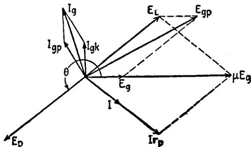
FIG. 14.2.—Vector diagram showing negative conductance.
