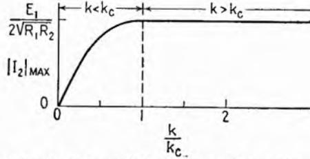
FIG. 13.1.—Variation of  $|I_2|_{\max}$  with coefficient of coupling.
