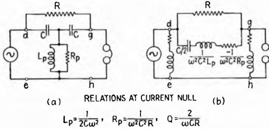
FIG. 5.3 — (a) Bridged T; (b) equivalent circuit.
