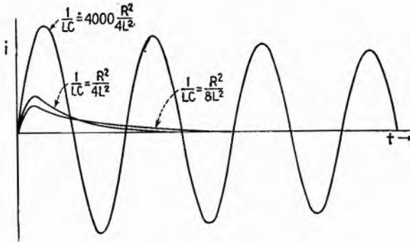
FIG. 5.2.—Graphs of equations (5.12), (5.14), (5.15) with  $q_0 = 0$  plotted for three values of  $R/L$ ;  $L$  and  $C$  are held constant. All curves have the same initial slope  $E/L$  and enclose the same total area from zero to infinity of time. Areas above the time axis are considered positive, and areas below, negative.
