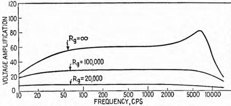
FIG. 22.8.—Effect on frequency response of varying  $R_g$ .
