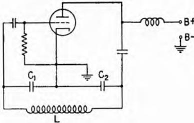
FIG. 3.2.—Colpitts oscillator circuit.
