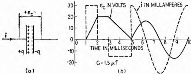
FIG. 5.1.—Ideal capacitor and its instantaneous current-voltage relations.
