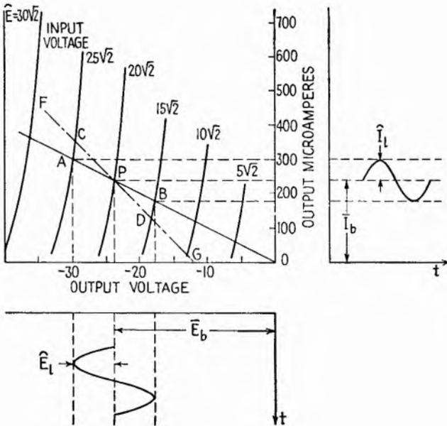
FIG. 6.1.—Diode-rectification diagram showing d-c load line  $OBPA$  and a-f resistance load line  $FCPDG$ . Waveforms of output a-f current  $I_t$  and a-f voltage  $E_t$  are shown for the condition where the d-c resistance and a-f impedance of the load are equal.
