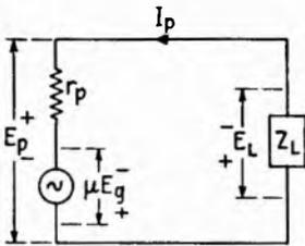
FIG. 9.2.—Equivalent plate circuit (constant-voltage form).
