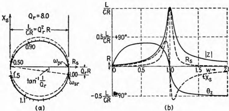
FIG. 15.1.—Impedance variations for a parallel circuit of intermediate  $Q_r$ , described in polar and rectangular form as a function of the frequency ratio  $w = \omega/\omega_{sr} = \omega \sqrt{LC}$ .
