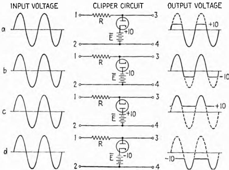
FIG. 17.1.—Diode clipper circuits.
