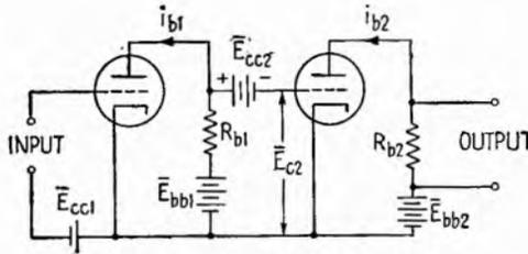
FIG. 5.1.—Direct-coupled amplifier.
