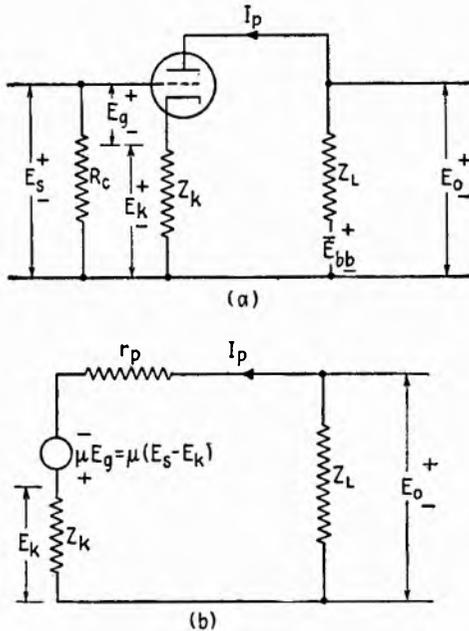
FIG. 31.1.—Cathode degeneration.
