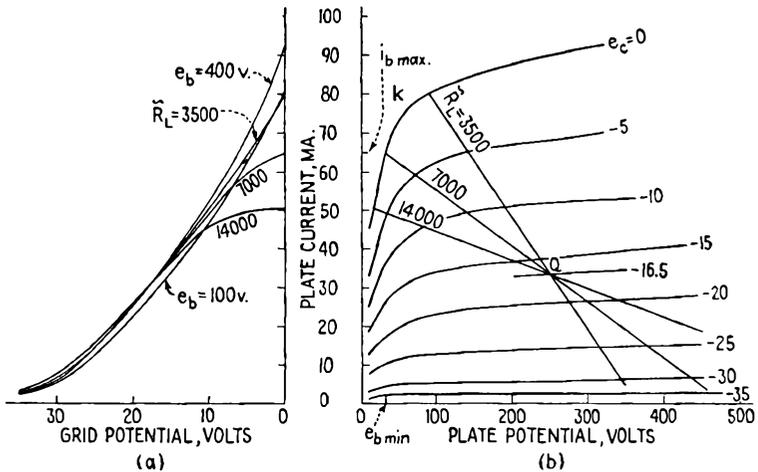
FIG. 23.5.—A typical power pentode in Class A<sub>1</sub> operation.
