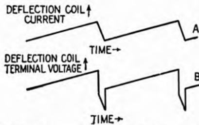
FIG. 6.1.—Deflection-coil current and terminal voltage as functions of time.
