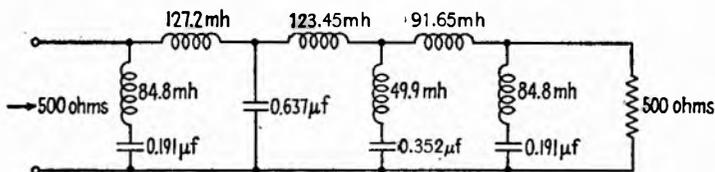
FIG. 19.6.—Composite filter.
