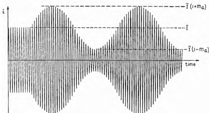
FIG. 2.1.—Amplitude-modulated current.
