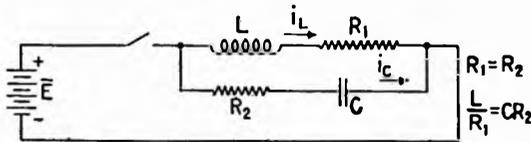
FIG. 4.5.—Spark-suppressor circuit.
