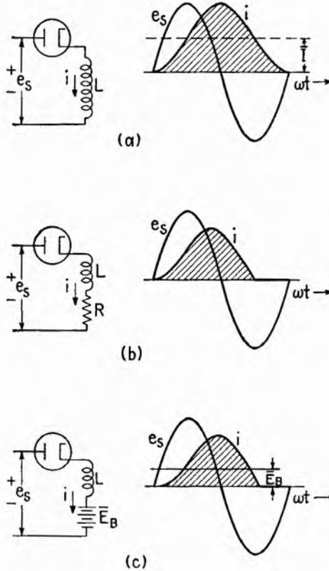
FIG. 2.9.—Half-wave rectifier with inductive load. (a) Pure inductance,  $\sqrt{2} E_s/\omega L = 1$ ; (b)  $\omega L/R = 4$ ,  $\sqrt{2} E_s/\sqrt{R^2 + \omega^2 L^2} = 1$ ; (c)  $E_B = \sqrt{2} E_s/4$ ,  $\sqrt{2} E_s/\omega L = 1$ .
