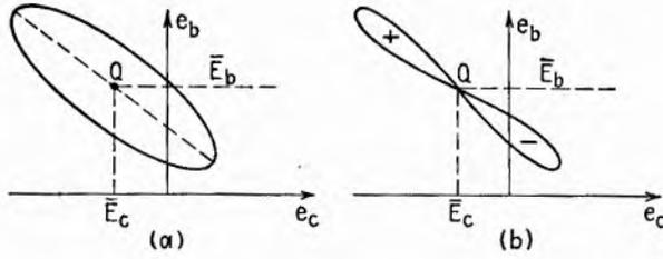
FIG. 10.2.—(a) Path of operation when  $E_p$  and  $E_o$  are not opposite in phase; (b) path of operation when  $E_p$  and  $E_o$  are opposite in phase, but  $e_p$  contains a second-harmonic component.
