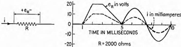
FIG. 6.1 —Ideal resistor and its instantaneous current-voltage relations.
