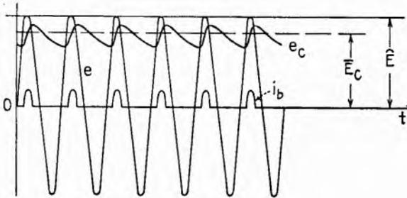
FIG. 4.2.—Showing the voltage across the capacitor and the current in the diode with the  $RC$  load of Fig. 4.1.
