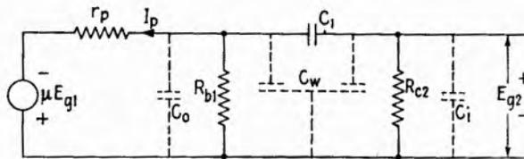
FIG. 8.1.—Equivalent plate circuit using a constant-voltage generator.
