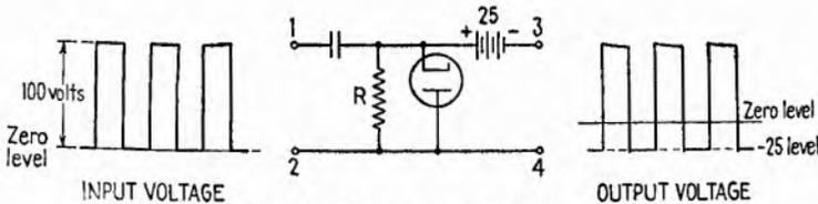
FIG. 20.5.—Bottom of wave clamped at -25-volt level.
