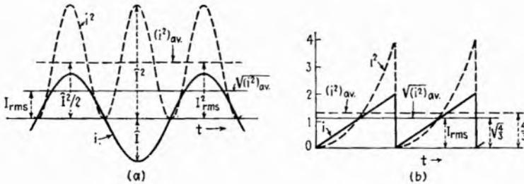
FIG. 3.2.—Root-mean-square (rms) values of sinusoidal and nonsinusoidal waves. variations of double the frequency of the current  $i$  displaced vertically and has an average value  $|\hat{I}|^2/2$ . The rms value of the current is indicated.
