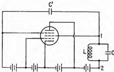
FIG. 13.7.—Transitron oscillator.
