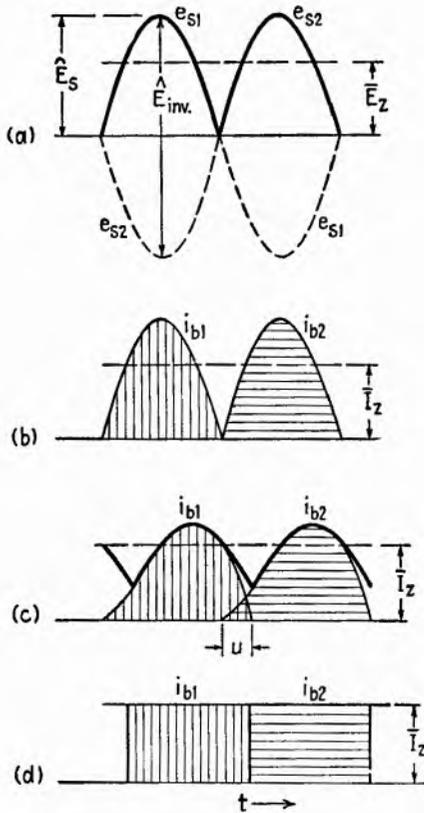
FIG. 3.2.—Full-wave-rectifier waveforms. (a) Voltages for pure resistance load; (b) current for pure resistance load; (c) current for load of  $R$  and  $L$ ,  $u$  = period of overlap; (d) idealized current for highly inductive load with no inductance in anode leads.
