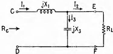
FIG. 7.5.—Matching section for which  $R_c < R_L$ .
