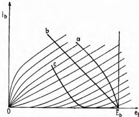
FIG. 22.2.—Load characteristics of Fig. 22.1 reversed and superimposed as load lines on the  $i_b$ - $e_b$  diagram of a modulator tube.
