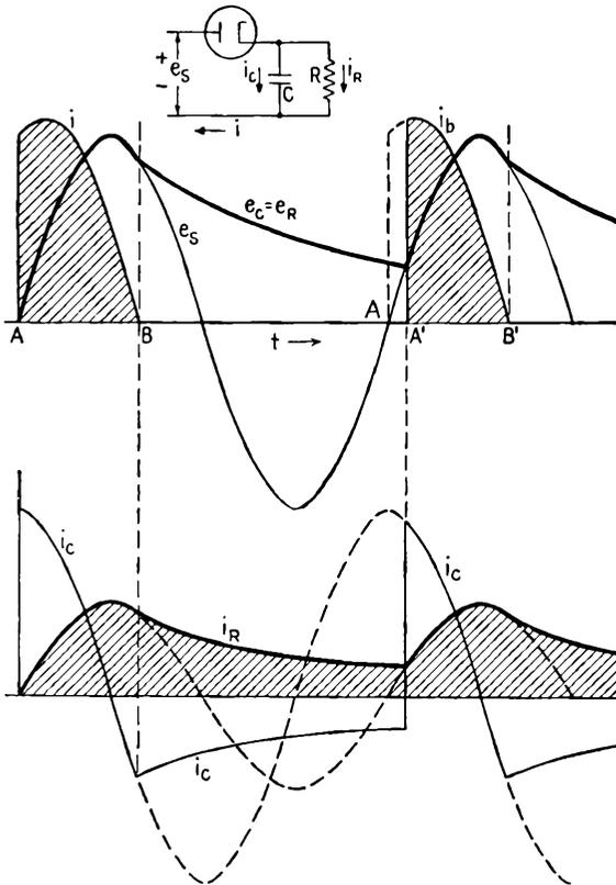
FIG. 2.5.—Current and voltage relations in load of  $R$  and  $C$  in parallel. Solid, heavy lines show rectifier-circuit quantities; dotted lines show normal steady-state quantities (rectifier short-circuited).
