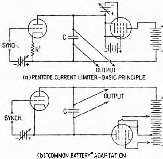
FIG. 11.2.—(a) Relaxation oscillator with pentode current limiter; (b) "common battery" adaptation. In practice, rectifiers with potential dividers replace the batteries.
