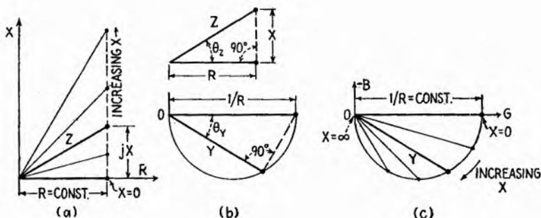
FIG. 1.1.—Impedance and admittance relations in a series circuit with constant  $R$ : (a) values of  $Z$  as  $X$  is varied; (b) relation between  $Z$  and its corresponding  $Y$ ; (c) values of  $Y$  corresponding to indicated values of  $Z$ .
