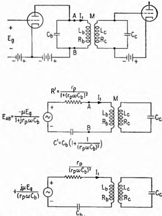
FIG. 20.1.—Parallel-fed coupled system and its equivalent circuit.
