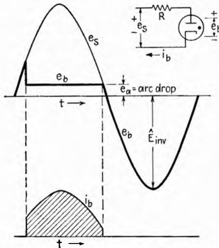
FIG. 1.3.—Waveform of current with an arc rectifier.
