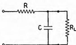
FIG. 12.1.—Resistance-capacitance filter.
