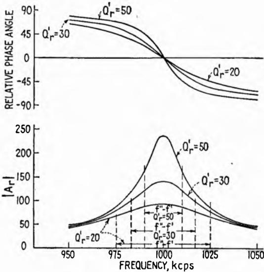
FIG. 26.3.—Frequency and phase response near resonance for a capacitance-coupled r-f amplifier stage.
