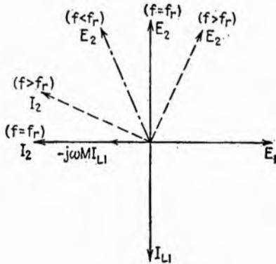
FIG. 22.2.—Phase relationships in the discriminator circuit of Fig. 22.1. Position of  $E_2$  at resonance given by solid line; at a higher frequency, by the dashed line; at a lower frequency, by the dot-dash line.
