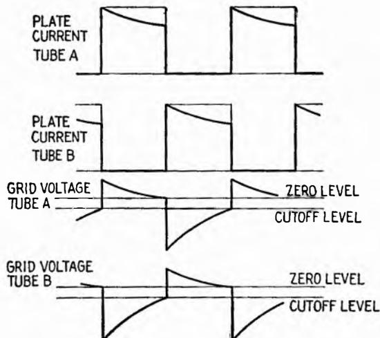
FIG. 28.3.—Multivibrator waveforms in the circuit of Fig. 28.1.
