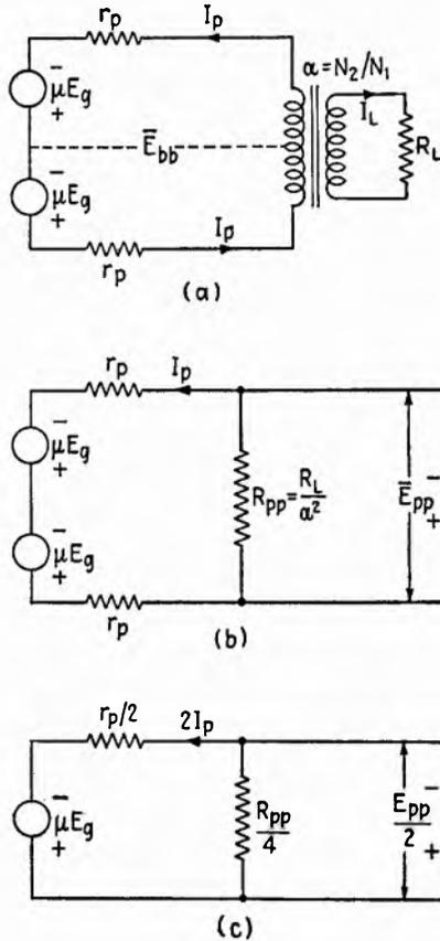
FIG. 24.2.—Equivalent plate circuits for push-pull linear operation.
