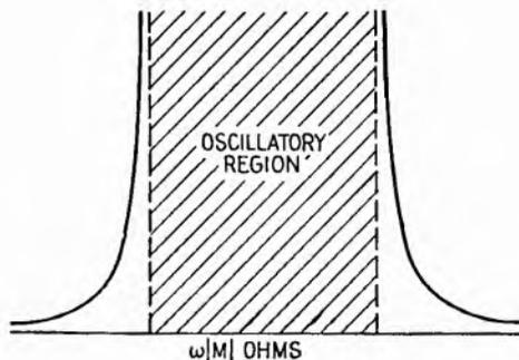
FIG. 2.3.—Variation of current in regenerative tuned-grid circuit.
