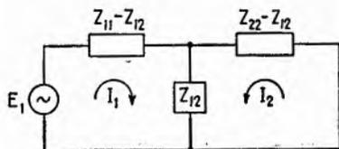
FIG. 6.1.—General form of two coupled circuits.
