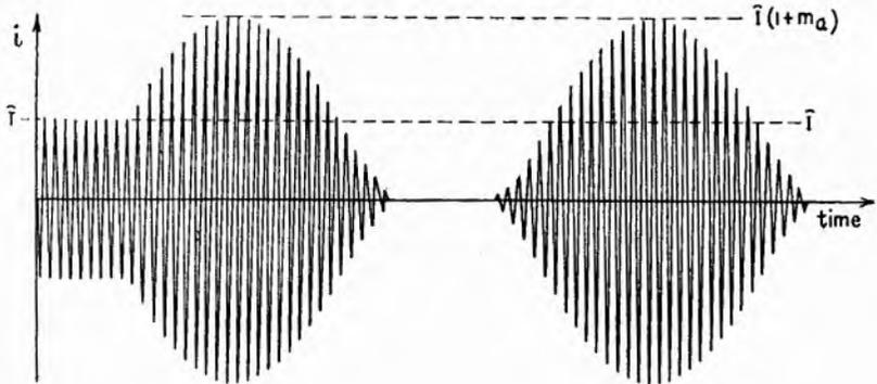
FIG. 2.2.—Overmodulated current.
