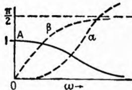
FIG. 12.3.—Frequency characteristics of the network of Fig. 12.1.
