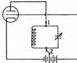
FIG. 13.6.—Dynatron oscillator.
