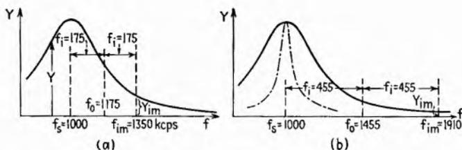
FIG. 9.1.—Image-frequency response in a converter: (a) intermediate frequency = 175 kcps; (b) intermediate frequency = 455 kcps.
