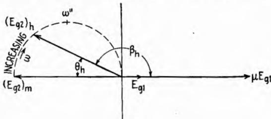
FIG. 11.3.—Polar relation of  $E_{o2}$  to  $E_{o1}$  at high frequencies in a resistance-coupled stage.
