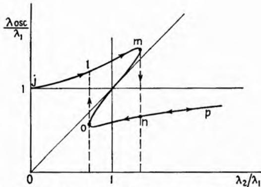
FIG. 20.4.—Wavelength of oscillation with  $k > (1/Q_2)$ .
