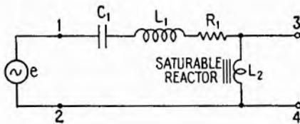
FIG. 23.2.—Saturable-reactor circuit.
