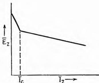
FIG. 9.3.—Voltage-regulation curve of a choke-input power supply.
