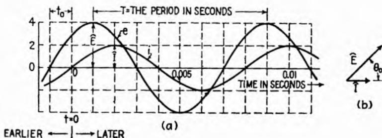
FIG. 1.1.—Sinusoidal voltage and current variations of different amplitudes and phases. For the curve marked  $e$ ,  $\hat{E} = 4$ ,  $T = 0.008$  sec,  $t_0 = 0.001$  sec,  $f = 125$  cycles/sec,  $\omega = 78.5$  radians/sec.
