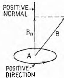
FIG. 10.1.—Conventions for determining flux of induction  $\phi$ .
