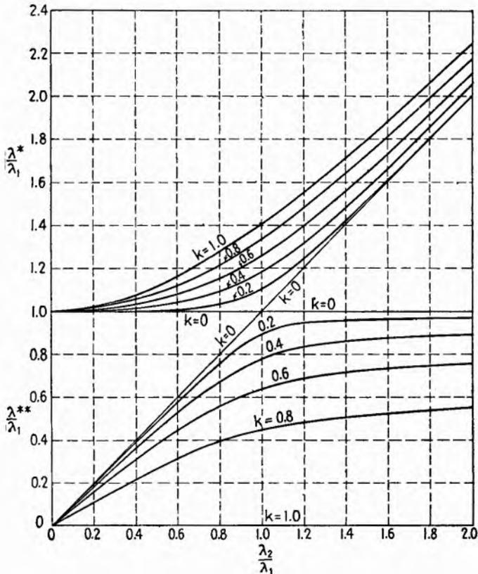
FIG. 4.1.—Wavelengths of a freely oscillating coupled system.
