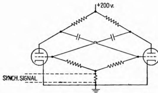
FIG. 28.5.—Injection of synchronizing signal for division by an even number.
