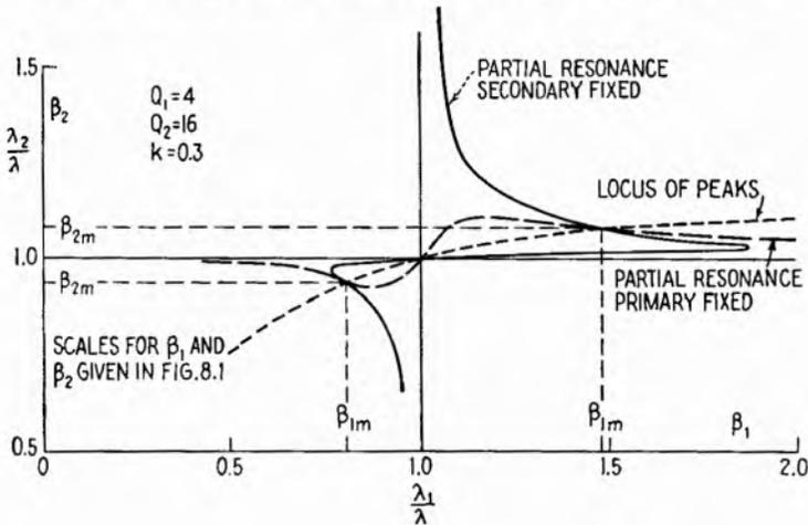
FIG. 10.1 —Partial-resonance conditions in magnetically coupled circuits.
