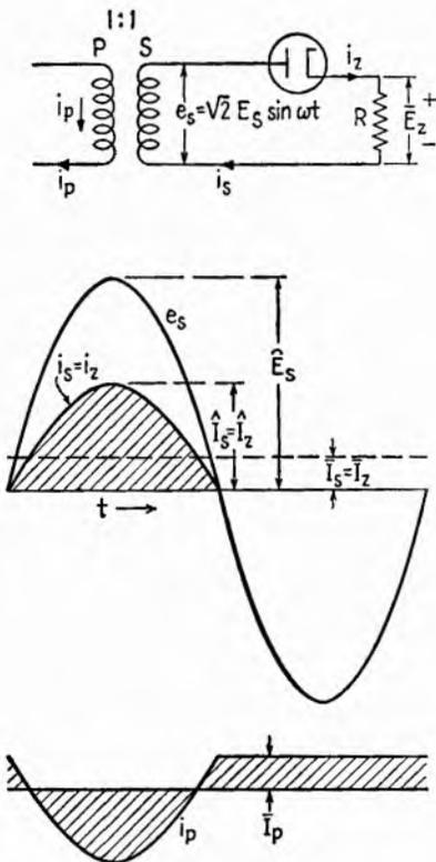
FIG. 7.1.—Primary and secondary currents of a rectifier transformer.
