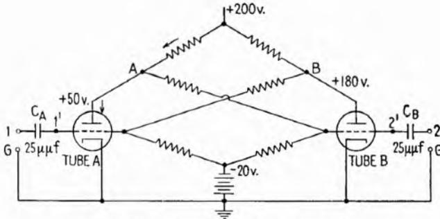
FIG. 27.4.—Separate triggering controls.
