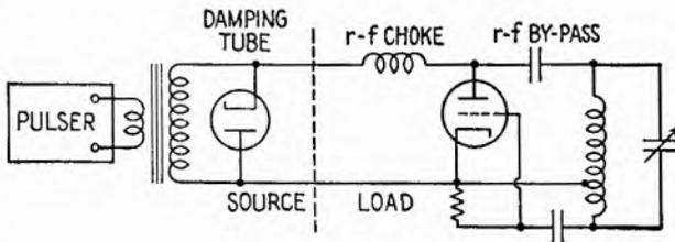
FIG. 19.2.—Pulsed oscillator.
