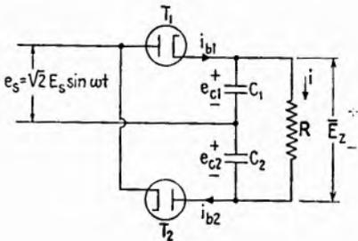
FIG. 4.1.—Full-wave-voltage-doubler circuit.
