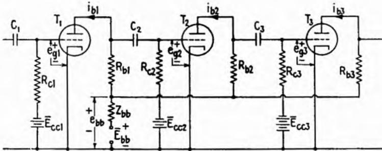
FIG. 33.1.—Feedback through the impedance of a common plate power supply. and any added impedance that is in series with the plate power supply. Since  $Z_{bb}$  is common to the plate circuits of both tubes, it provides a feedback path.
