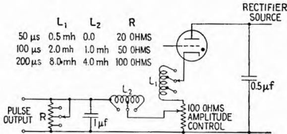
FIG. 12.3.—Pulse-shaping filter.
