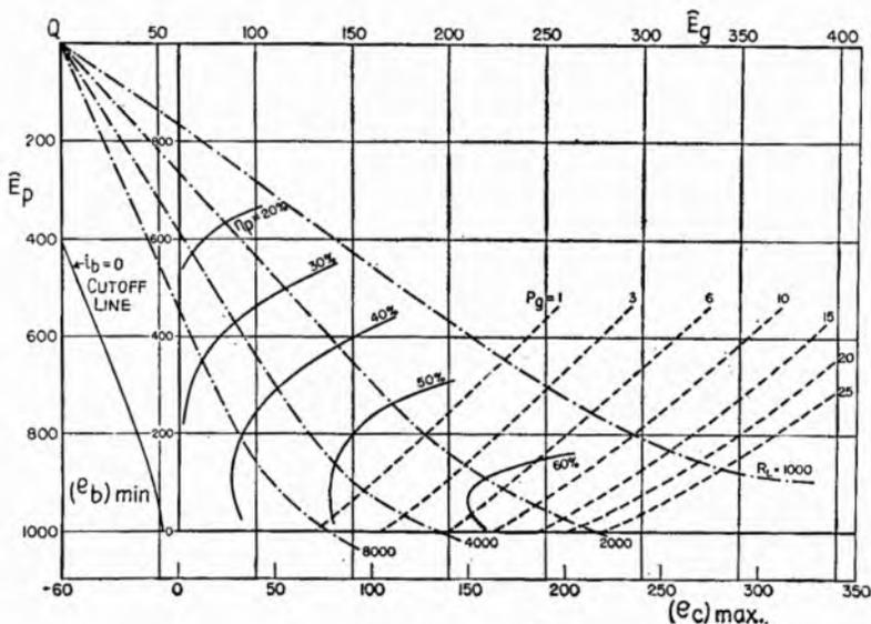
FIG. 12.7.—Chart showing contours of constant  $P_g$ ,  $\eta_p$ , and  $R_L$  for the type 211 tube. Class B operation;  $\hat{E}_c = -60$  volts.
