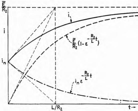
FIG. 2.7.—Graph of equation (2.12) showing the terms plotted separately and in total.
