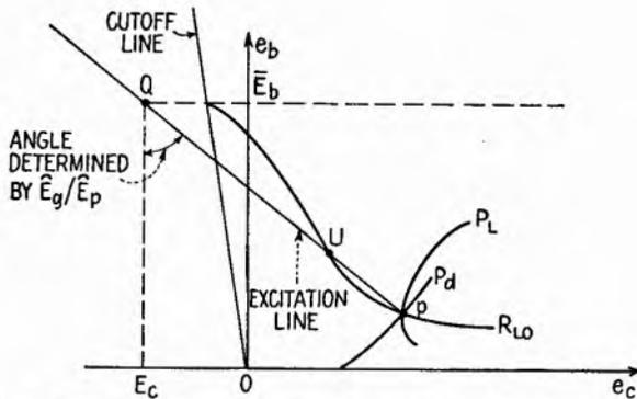
FIG. 20.1.—Contour chart showing conditions for an oscillator.
