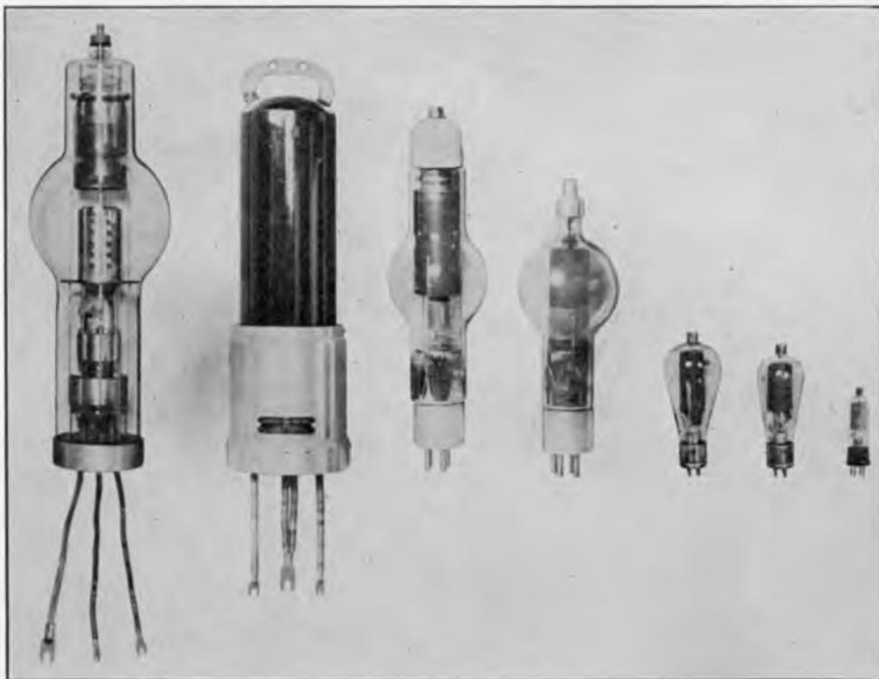
FIG. 6. A group of three-electrode, mercury-vapor-filled tubes. The ratings of these tubes range from 15,000 volts and 75 amperes down to 1,000 volts and 0.125 ampere.
