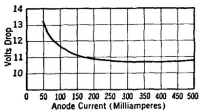
FIG. 60. Arc drop curve for a tube filled with argon.
