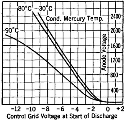
FIG. 67. The breakdown characteristic of one form of shield-grid, mercury-vapor-filled tube.
