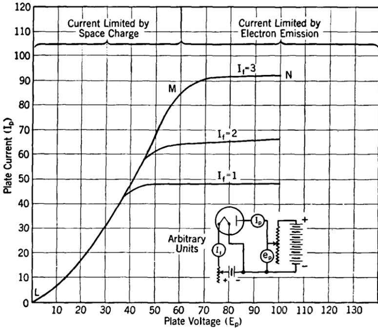
FIG. 8. Volt-ampere characteristic of a high-vacuum, two-electrode tube.
