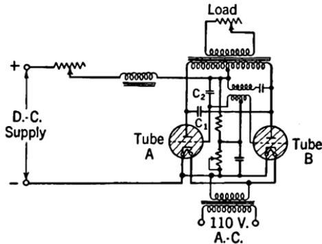
FIG. 79. The circuit for one form of inverter using two grid-controlled, gas-filled tubes.
