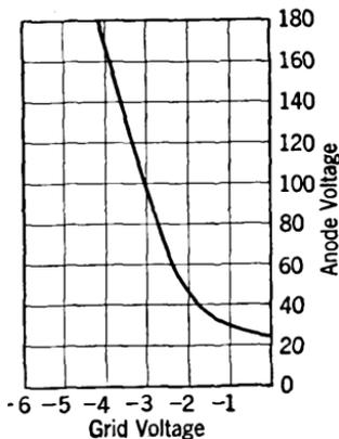
FIG. 59. The breakdown characteristic of an argon-filled tube.
