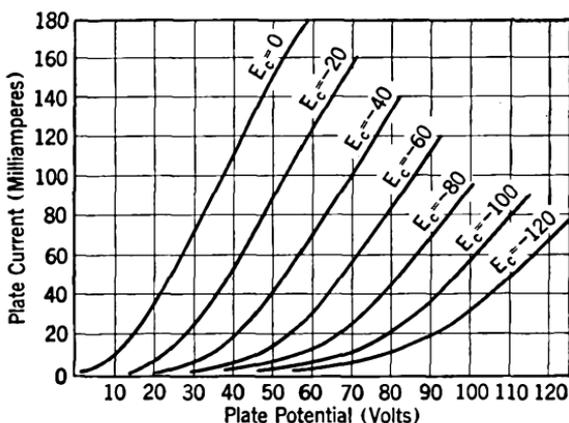
FIG. 34. Plate characteristic of an internal-grid tube.
