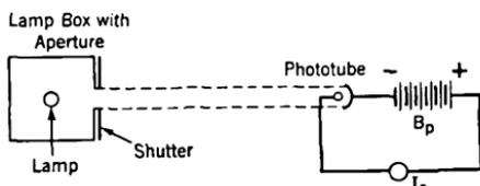
FIG. 16. Apparatus for determining the relation between light intensity and anode current in a phototube.
