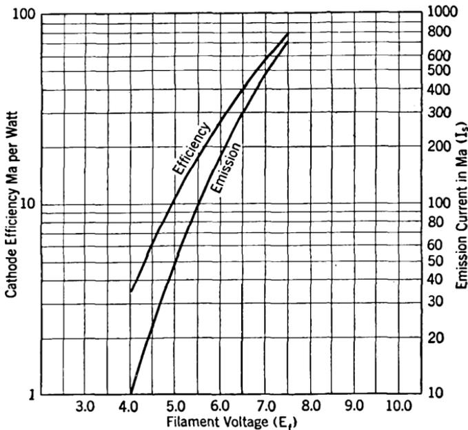
FIG. 11. Emission and emission efficiency for a tube using a thoriated-tungsten filament. The tube with which these data were taken has a filament rating of 7.5 volts.
