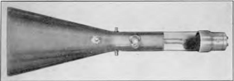
FIG. 82. A cathode-ray oscillograph tube.
