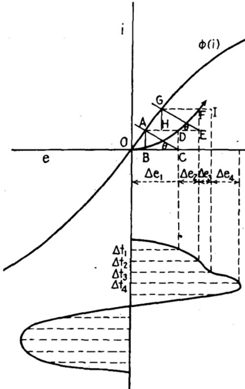
FIG. 47.—Graphical solution for  $Lr$  nonlinear circuit.
