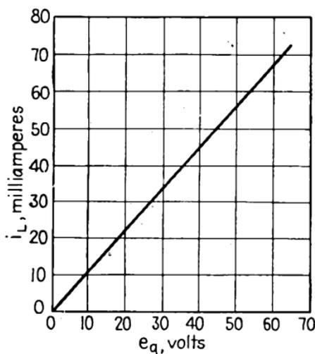
FIG. 82.—Output characteristic for 6F6 balanced amplifier.
