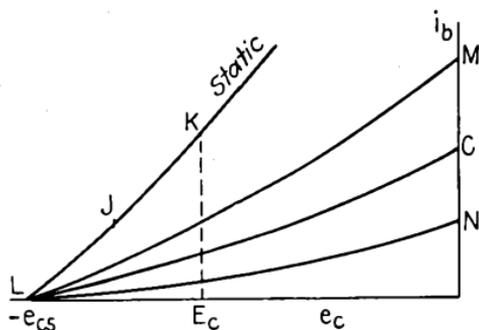
FIG. 25.—Comparison of various dynamic characteristics.
