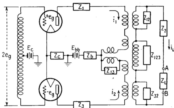
FIG. 89.—Generalized balanced-amplifier circuits.
