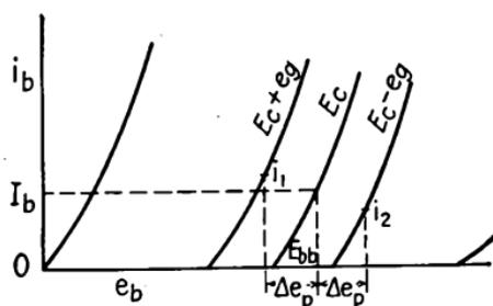
FIG. 73.—Graphical construction on plate family of tube characteristics.
