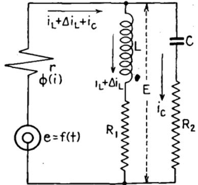
FIG. 57.—Parallel resonant nonlinear circuit
