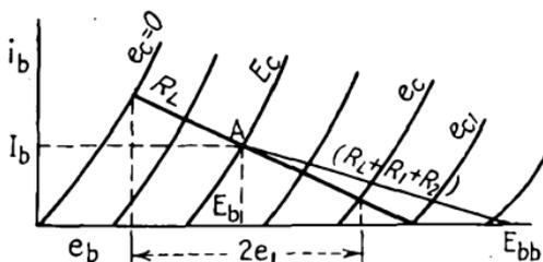
FIG. 124.—Graphical construction for plate-isolation circuit.
