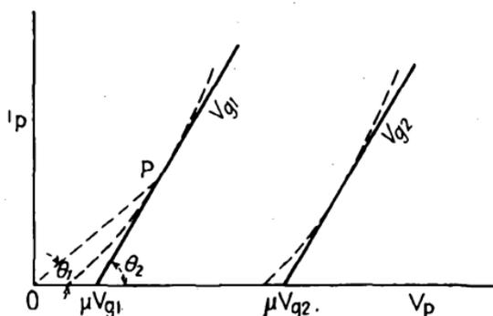
FIG. 7.—Linear and actual tube-plate characteristics.
