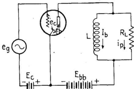
FIG. 27.—Inductive plate-feed circuit.
