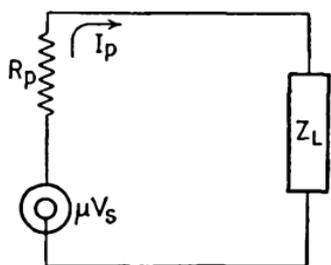
FIG. 8.—Equivalent plate circuit for a.c. component.
