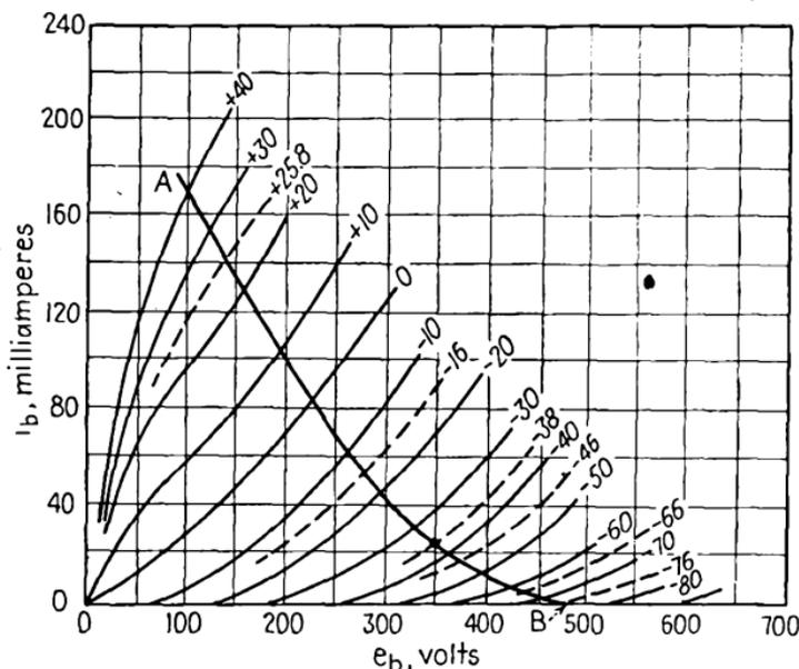
FIG. 79.—Push-pull load line for 6F6 tube—sliding-rule method.
