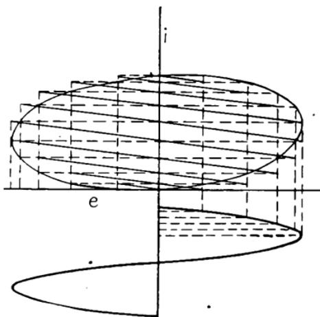
FIG. 48.—Displaced ellipse obtained for pure linear inductance.
