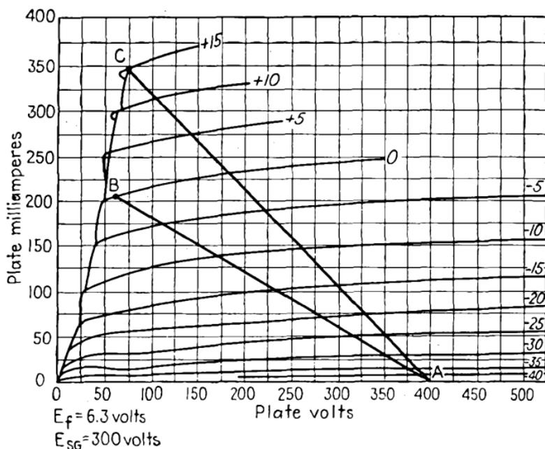
FIG. 85.—Push-pull characteristics for a 6L6 tube.
