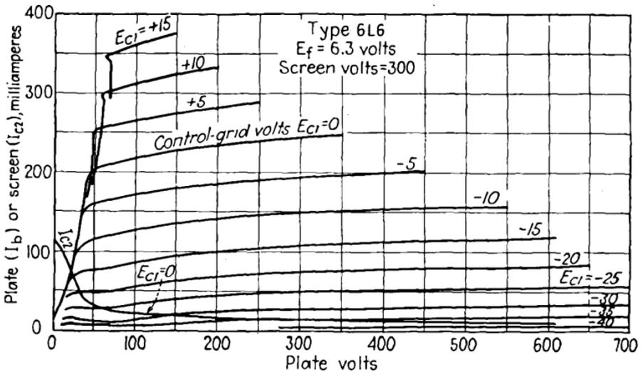
FIG. 36.—Beam power-tube characteristic.
