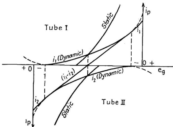
FIG. 94.—Push-pull operation beyond cutoff for parabolic tubes.
