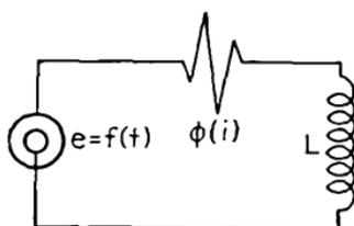
FIG. 46.—Simple  $Lr$ -series nonlinear circuit.
