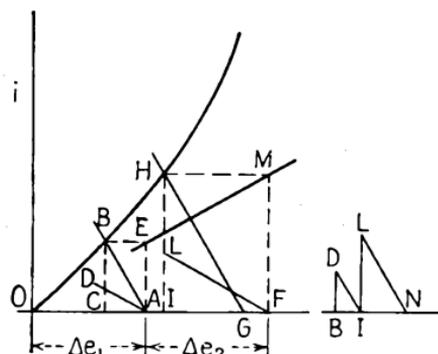
FIG. 56.—Graphical construction for parallel RC linear parameters.
