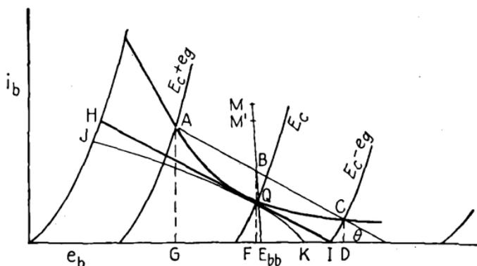
FIG. 86.—Graphical construction for the case of a mid-branch resistance.
