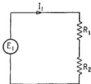
FIG. 13.—Two linear resistances in series.
