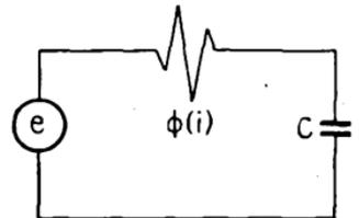
FIG. 49.—Simple  $rC$ -series nonlinear circuit.
