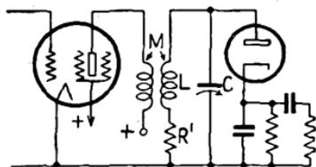
FIG. 112.—Complete diode circuit including h.f. source.
