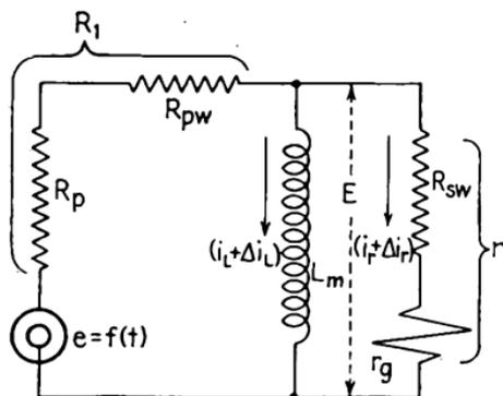
FIG. 59.—Circuit having nonlinear parallel resistor.
