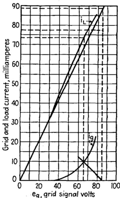
FIG. 101.—Determination of the driver resistance, 6F6 tube.
