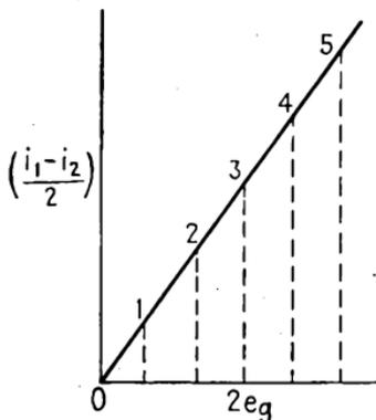
FIG. 75.—Transfer, or output, characteristic for balanced amplifier.
