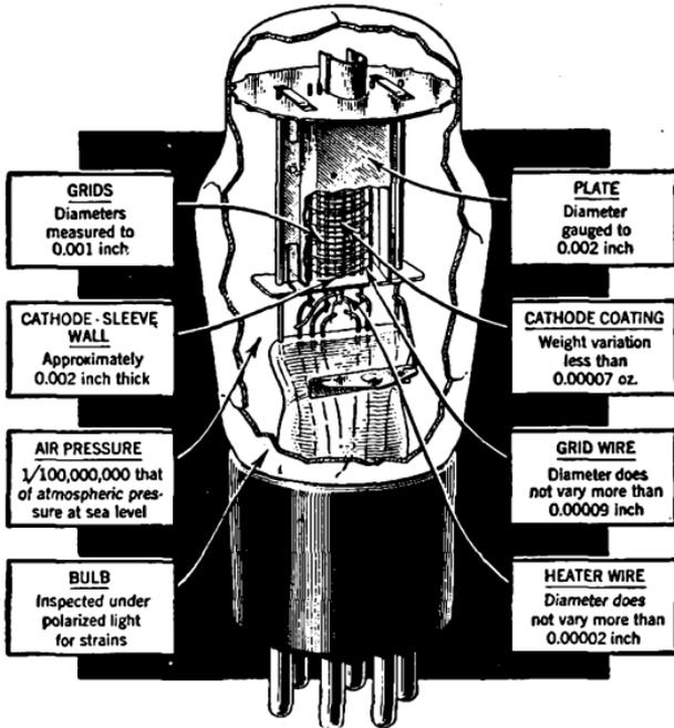
FIG. 4.—Typical triode construction. (Courtesy of RCA.)
