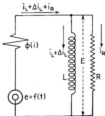
FIG. 54.—Parallel  $LR$  in series with nonlinear  $r$ .
