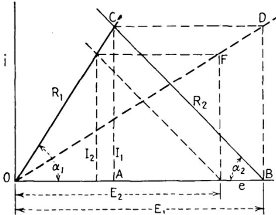
FIG. 14.—Graphical constructions for linear series circuit.
