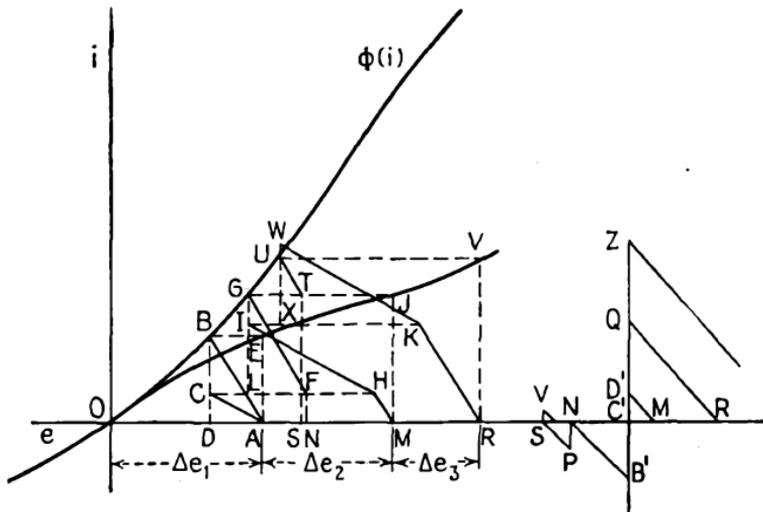
FIG. 58.—Graphical solution for parallel resonant circuit.
