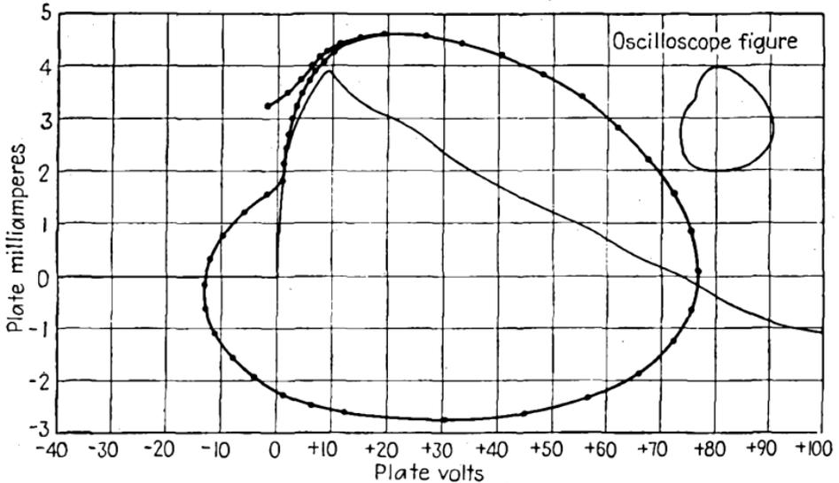
FIG. 70.—Path of operation for dynatron oscillator—22.5-volt plate supply.
