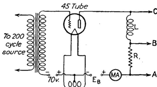
FIG. 63.—Experimental setup to check graphical construction of type 45 triode with inductive load.
