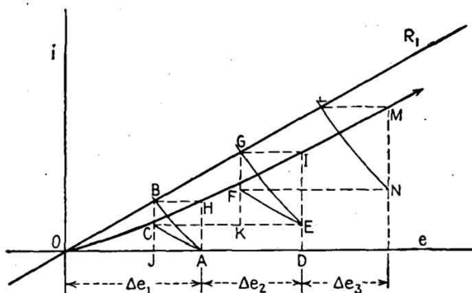
FIG. 61.—Graphical solution for nonlinear parallel resistor.
