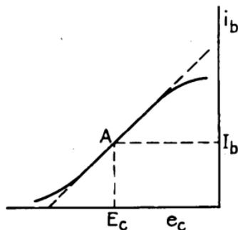
FIG. 38.—Dynamic characteristic for a pentode tube.
