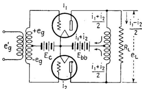
FIG. 72.—Idealized push-pull circuit.
