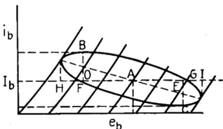
FIG. 44.—Reactive load line, plate characteristics.
