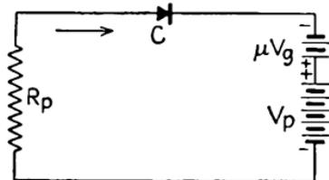
FIG. 11.—Equivalent circuit for a triode.
