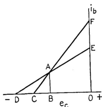
FIG. 31.—Power-output behavior for a linear tube.
