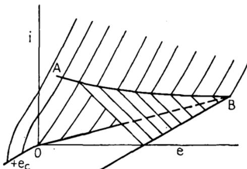
FIG. 21.—Three-dimensional graphical solution for triode circuit.
