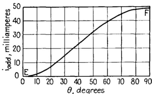
FIG. 81.—Wave shape for additional direct current.
