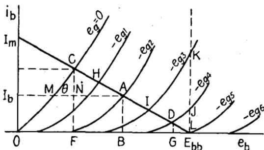
FIG. 22.—Two-dimensional graphical solution for triode circuit.
