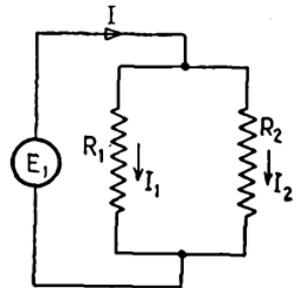
FIG. 16.—Parallel circuit.
