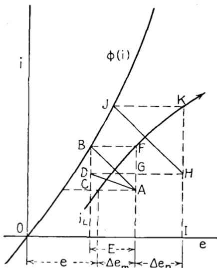
FIG. 55.—Graphical construction for parallel  $LR$ .
