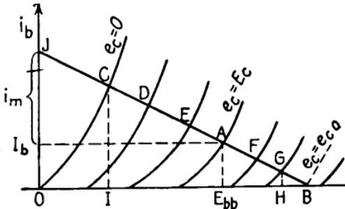
FIG. 28.—Path of operation for inductive plate feed.
