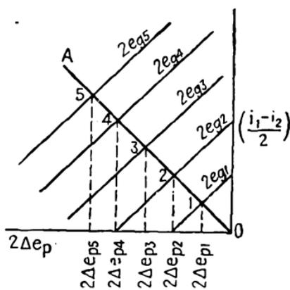
FIG. 74.—Push-pull family of characteristics.
