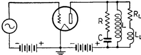
FIG. 39.—Loud-speaker compensating circuit, pentode output tube.
