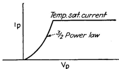
FIG. 3.—Temperature-saturation characteristic.
