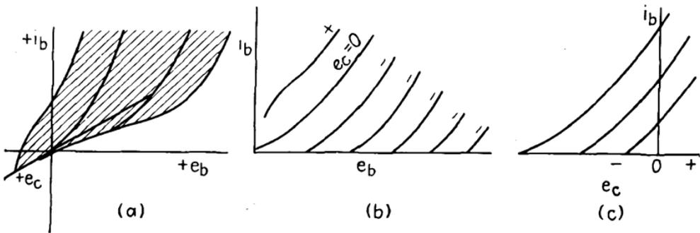
FIG. 18.—Triode surface and characteristic curves.
