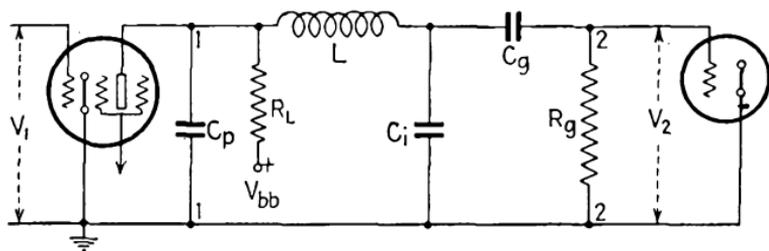
FIG. 9.—Series-peaking video circuit.
