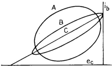
FIG. 45.—Reactive load line, grid characteristics.
