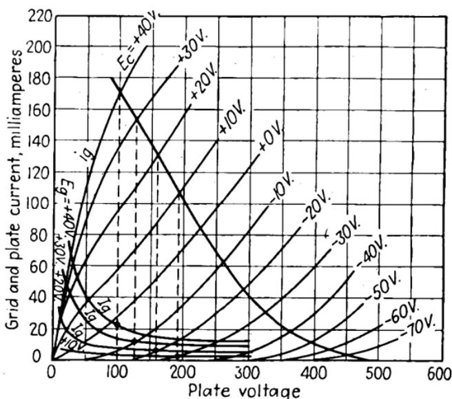
FIG. 100.—Grid-current determination for a 6F6 tube.
