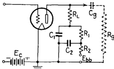
FIG. 123.—Two-stage plate-isolation circuit.
