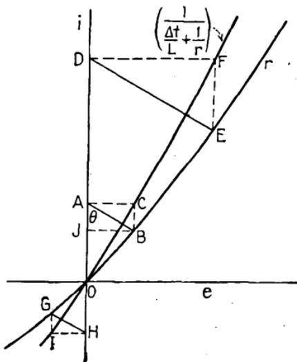
FIG. 60.—Parallel  $Lr$  finite operator—auxiliary graphical construction.
