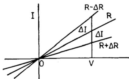
FIG. 12.—Terminal characteristics for a carbon-button microphone.
