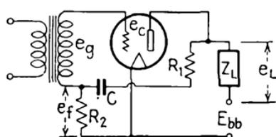
FIG. 119.—Typical voltage feedback circuit.
