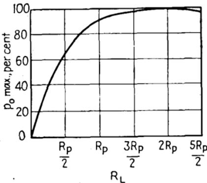
FIG. 32.—Power output vs. load resistance.
