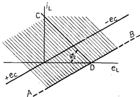
FIG. 20.—Load plane for linear resistor.
