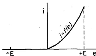
FIG. 1.—Diode-rectifier terminal characteristic.
