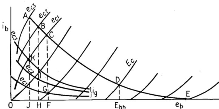
FIG. 95.—Determination of operating grid current.
