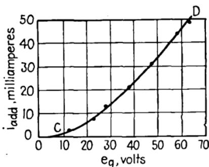
FIG. 80.—Interpolation curve—additional direct current vs. grid-signal swing.
