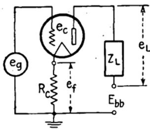
FIG. 121.—Typical current feedback circuit.
