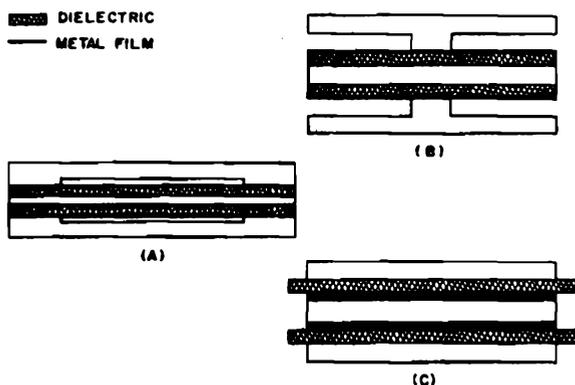
**Figure 1-78.** (A) Air-gap mounting using dielectric sheets having conducting films on each major surface. (B) Air-gap mounting using dielectric sheets having a conducting film on major surface in contact with electrode. (C) Dielectric sandwich in which leaves of metal foil are inserted between dielectric and crystal
