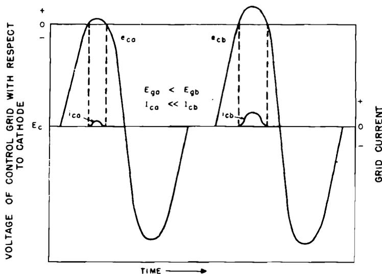
**Figure 1-107.** How a small percentage change in excitation voltage can cause a large percentage change in grid-leak current of  $C_1$  meter. Bias does not actually remain constant as indicated, but follows the percentage changes of excitation voltage. Nevertheless, the relative percentage variations of grid current and excitation voltage can be approximately as shown when the greater part of the bias is developed across the cathode resistance
