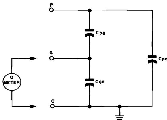
$$\begin{aligned} \textcircled{1} \quad C_{PG} &= C_{pg} + \frac{C_{gc} C_{pc}}{C_{gc} + C_{pc}} & \textcircled{3} \quad C_{PC} &= C_{pc} + \frac{C_{pg} C_{gc}}{C_{pg} + C_{gc}} \\ \textcircled{2} \quad C_{GC} &= C_{gc} + \frac{C_{pg} C_{pc}}{C_{pg} + C_{pc}} & * \textcircled{4-9} \quad C_{XY} &= C_{xy} + (C_{yz} \text{ OR } C_{xz}) \end{aligned}$$
