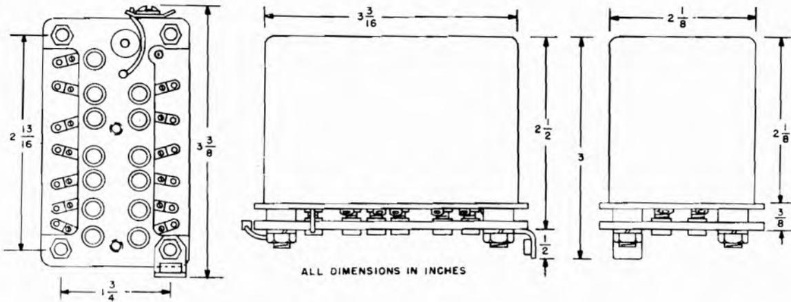
**Figure 4-23. Dimensions of Bendix Radio Crystal Oven N205651**
