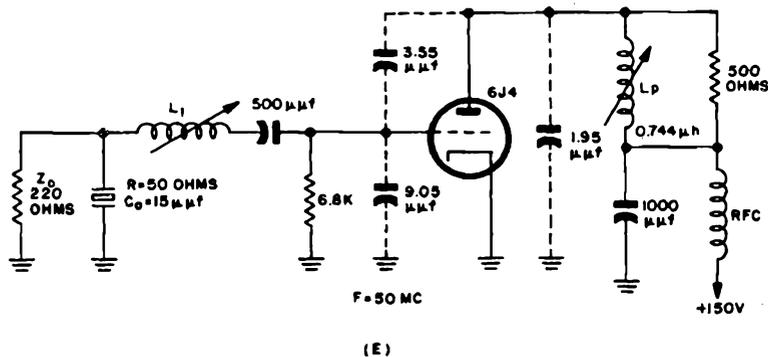
Figure 1-182. Impedance-inverting oscillator circuits. (E) Impedance-inverting Miller oscillator
