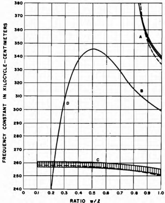
**Figure 1-32. Frequency constant versus  $w/l$  ratio for various resonances of  $-18^\circ$  X-cut crystal. A is the width-extensional mode. B is the face-shear mode, which, at small  $w/l$  ratios, is strongly coupled to D, the second flexural mode. C represents the band between the antiresonant (upper curve) and the resonant (lower curve) frequencies of the length-extensional mode of element F. Note the weak coupling between C and D-B \***
