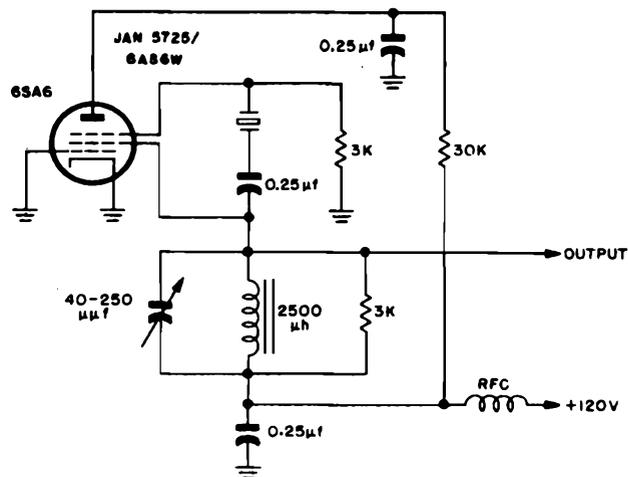
Figure 2-14. Schematic diagram of typical oscillator designed for use with Crystal Unit CR-25/U
