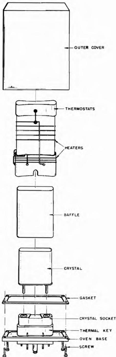
Figure 4-2. Small crystal oven equivalent to Military Type HD-54/U
