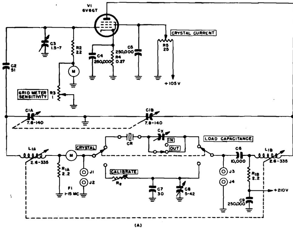
Figure 1-185. Colpitts circuits modified for series-mode crystal control
