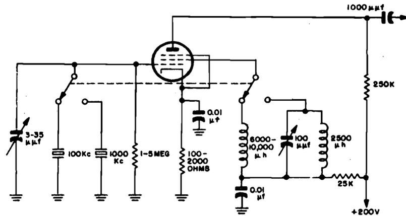
Figure 1-186. Typical design of single-tube general-purpose crystal calibrator circuit
