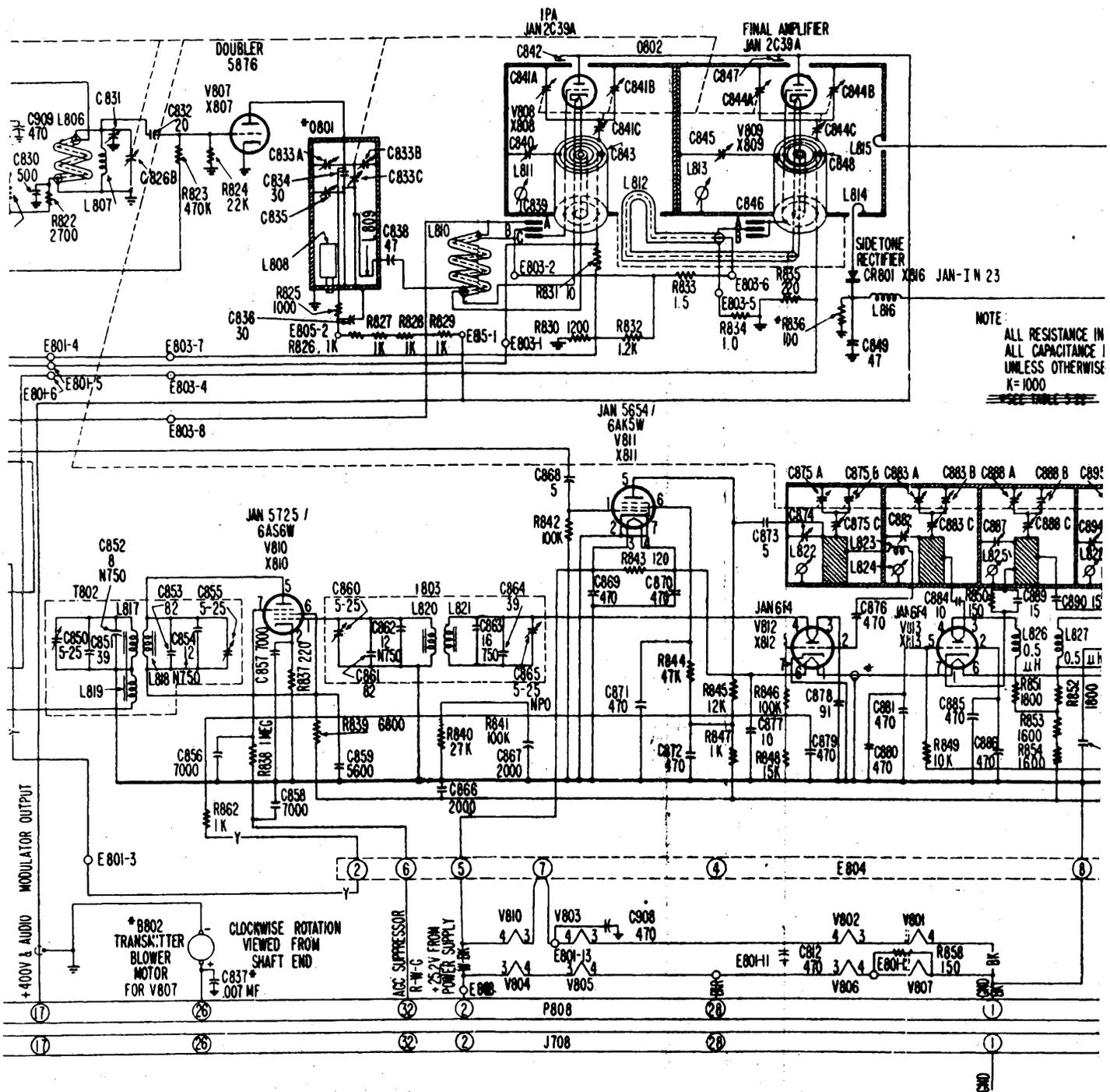
Figure 1-199. R-f head. Schemc transmitter and receiver r-f circ
