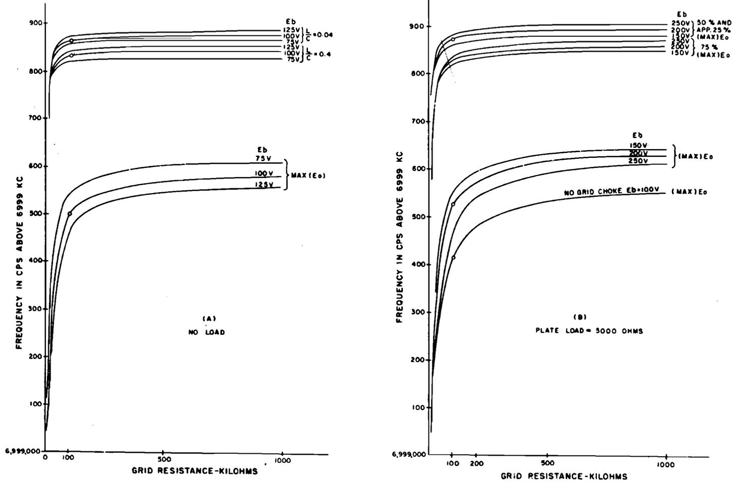
**Figure 1-146. Frequency of experimental Miller oscillator versus d-c plate voltage and grid resistance for various plate-tuned load capacitances. (Max) E<sub>o</sub> represents the plate tuning adjustment that provided maximum output voltage when grid resistance and d-c plate voltage were values indicated by zero reference point. A 7-mc CR-18/U crystal unit was used, having a P<sub>i</sub> of 49,000 ohms when operating into a rated load capacitance of 32 μμf**
