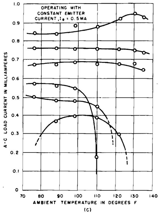
Figure 1-223. (A) Current amplification,  $\alpha$ , of point-contact transistor versus emitter current,  $I_e$ . (B) Collector characteristics of point-contact transistor. A-C load line indicates approximate operating region during oscillations. (C) Collector current characteristics for different point-contact transistors of type 1729, showing effects of temperature
