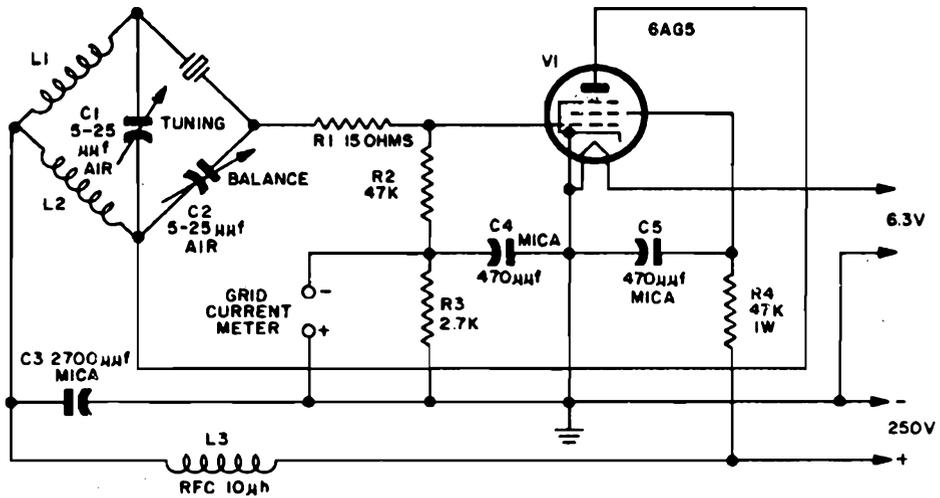
Figure 1-167. A single-tube capacitance-bridge oscillator which is practical for operation in the 50-90-mc frequency range. Resistors not otherwise specified are 1/2 w. L-1 and L-2 are a single center-tapped coil of suitable inductance
