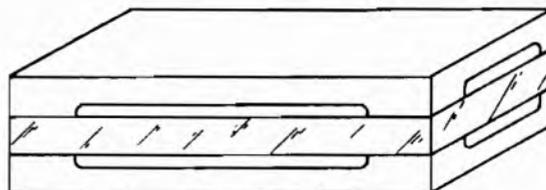
Figure 1-71. Typical corner-clamped, air-gap method of mounting crystals \*
