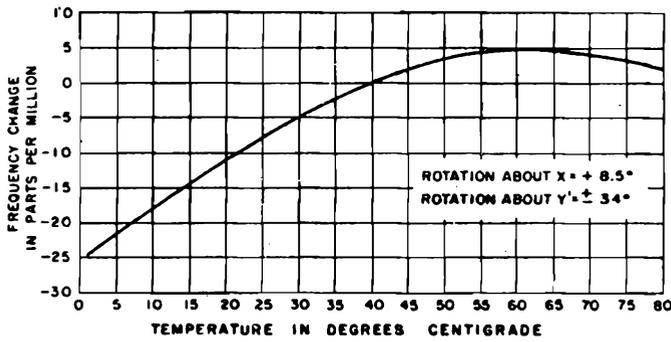
Figure 1-35. Frequency-temperature characteristics of element M \*
