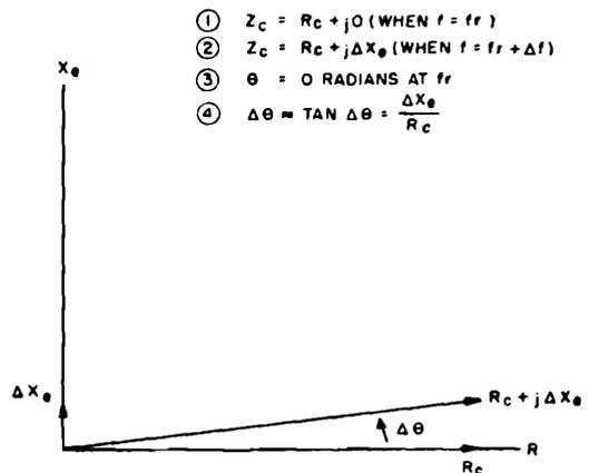
Figure 1-111. Phasor diagram, showing change in reactance,  $\Delta X_c$ , of series-mode crystal required to produce a small change in phase,  $\Delta\theta$ , where the resistance of the crystal circuit is equal to  $R_c$ .
