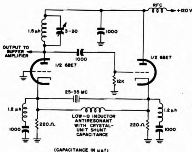
Figure 2-10. Schematic diagram of typical oscillator designed for use with Crystal Unit CR-23/U
