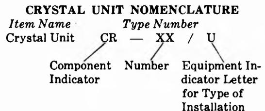
In the type number, the component, which is a crystal mounted in a holder, is identified by the symbol, CR. The component symbol is followed by a hyphen and 2 digits (-XX) which identify the mounted crystal as having been designed according to certain specified electrical and physical characteristics. The letter U, separated from the number by a slant sign, is the equipment indicator
