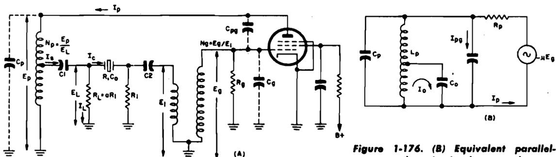
Figure 1-176. (A) Basic circuit of transformer-coupled oscillator
