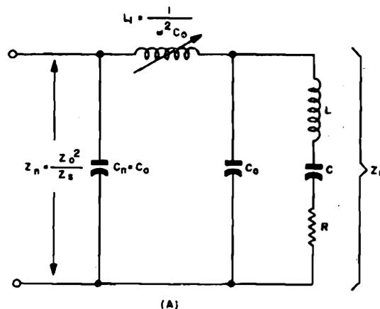
Figure 1-182. Impedance-inverting oscillator circuits.
