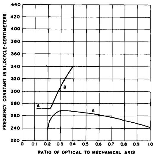
**Figure 1-20.** Frequency constant for length-extensional mode (curve A) of X-cut crystal where the width and length are parallel to the Z and Y axes, respectively. Curve B is the frequency constant of a face-shear mode coupled to a second flexural mode, whose interference makes the crystal useless for w/l ratios between 0.2 and 0.3, unless the thickness approaches the dimensions of the width \*
