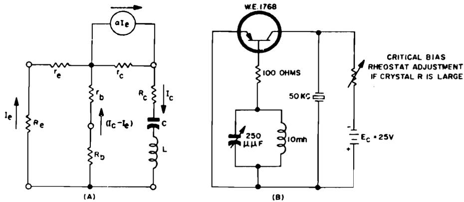
Figure 1-232. (A) Equivalent a-c circuit of tuned-collector negative-resistance oscillator. For crystal control,  $L$ ,  $C$ , and  $R_c$  can be interpreted as being the series-arm parameters of a crystal unit; (B) Crystal-controlled tuned-collector negative-resistance oscillator. The parallel tuned tank is inserted in the base circuit in lieu of a resistor in order to obtain negative resistance values in excess of 40,000 ohms
