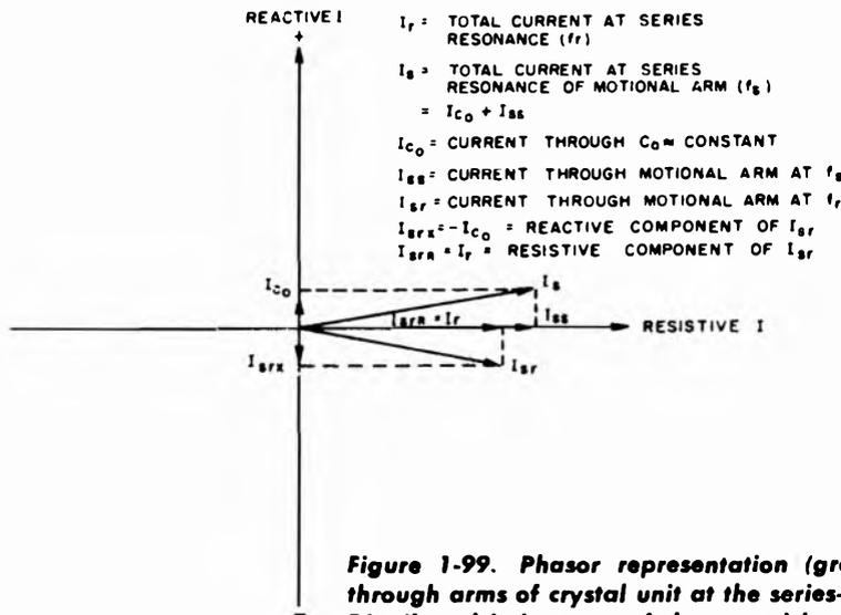
**Figure 1-99. Phasor representation (greatly exaggerated) of current through arms of crystal unit at the series-resonant frequencies,  $f_r$  and  $f_s$ . Distributed inductance of the crystal leads is assumed to be negligible**
