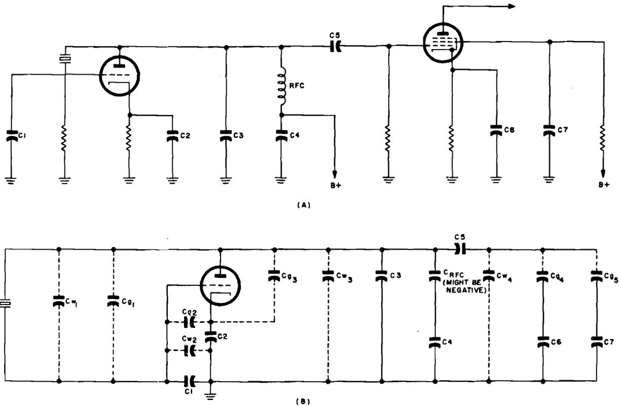
**Figure 1-124. (A) Conventional Pierce oscillator and buffer-amplifier circuit. (B) Static capacitances of circuit (A).  $C_y$  = interelectrode capacitances.  $C_w$  = distributed capacitances of wires**
