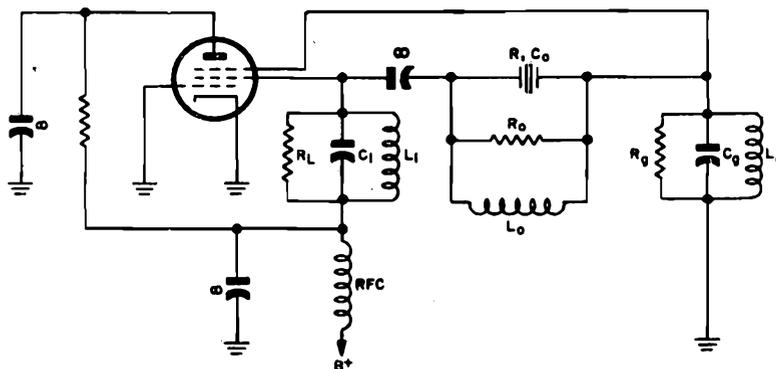
Figure 1-181. Transistron crystal oscillator
