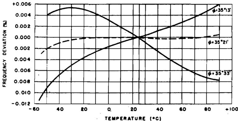
Figure 1-49. Temperature-frequency characteristics of element A
