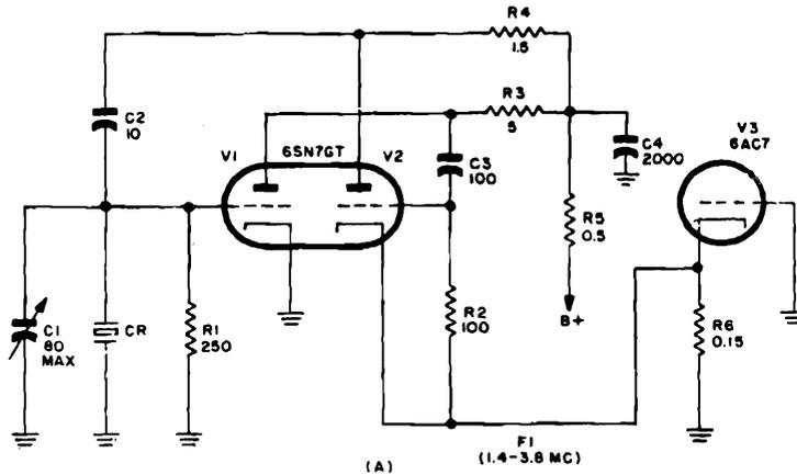
Figure 1-155. Two-stage parallel-resonant oscillators of the multivibrator type.
