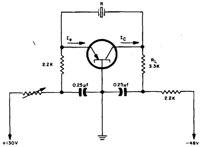
Figure 1-222. Basic circuit for crystal-controlled transistor oscillator
