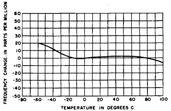
Figure 1-55. Temperature-frequency characteristics of element G \*
