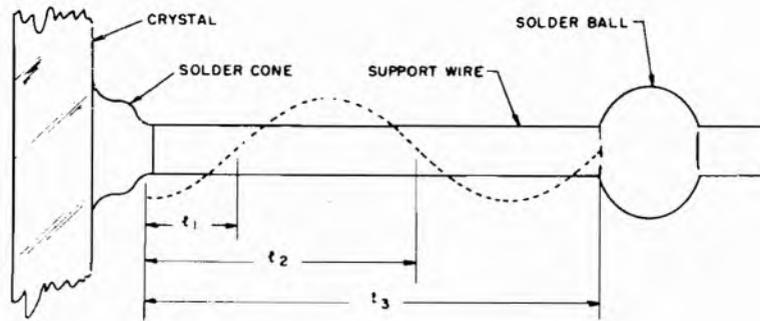
**Figure 1-84. Solder-cone resonant-wire support. The solder ball "tunes" the wire to the crystal frequency if it is placed at a distance equal to an odd multiple of a quarter wavelength ( $l_1, l_3$ , etc.) from the peak of the solder cone \***
