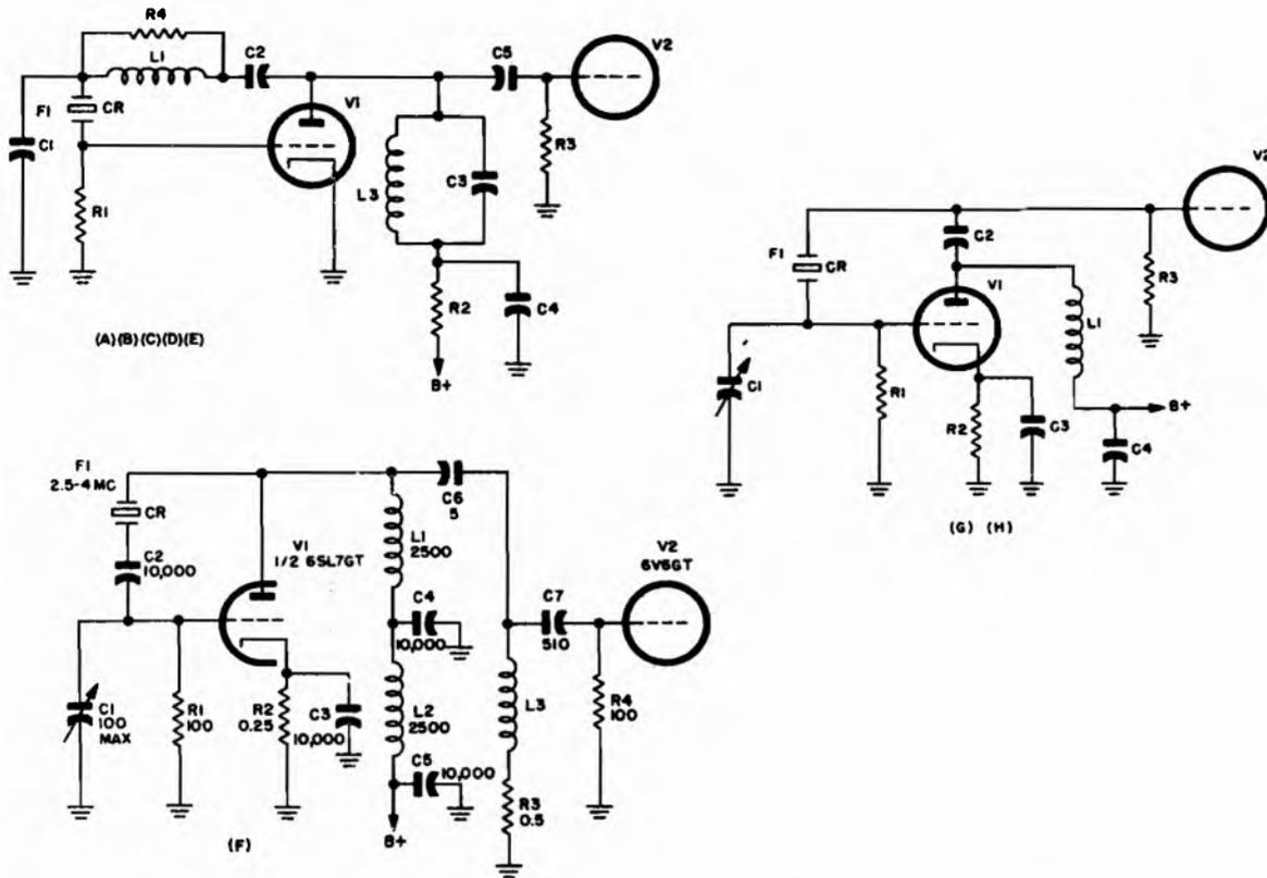
Figure 1-135. Modifications of Pierce oscillator using triodes
