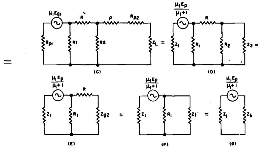
Figure 1-173. (A) Basic diagram of Butler two-stage cathode-coupled oscillator. (B) Equivalent r-f circuit of Butler oscillator. Current arrows indicate instantaneous electron flow when r-f voltages have polarities shown. (C) Simplified equivalent circuit where generator of grounded-grid amplifier is replaced by a negative resistance. (D), (E), (F), and (G) Progressive simplifications of equivalent Butler circuit
