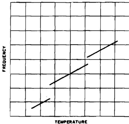
Figure 1-47. Temperature-frequency characteristics typical of the Y-cut, thickness-shear element. The frequency jumps are most apt to occur when small discrepancies are present in the thickness-dimension
