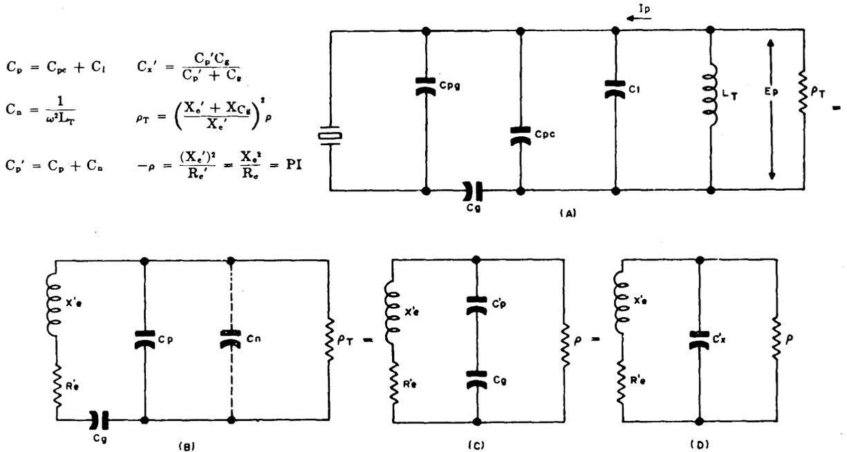
**Figure 1-121. Generalized Pierce oscillator.  $X_e'$  and  $R_e'$  are the effective impedance parameters of the crystal unit based upon the assumption that  $C_{pg}$  is a part of  $C_o$ .  $C_x$  is an equivalent negative capacitance having a positive reactance equal to that of  $L_T$ .  $I_p$  is the r-f plate current of the vacuum tube.**
