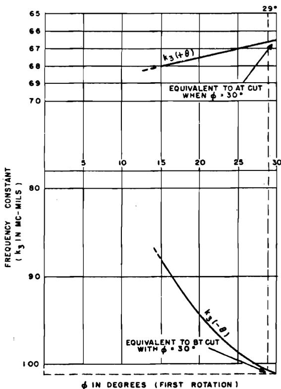
Figure 1-39. Frequency constant versus  $\phi$  (angle of rotation about Z axis) for the thickness-shear mode of V-cut crystals when  $\theta$ , the second angle of rotation, is so chosen that a zero temperature coefficient is obtained. The upper and lower curves are for positive and negative values of  $\theta$ , respectively
