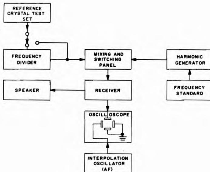
*Figure 2-92. System recommended for Government inspection measurements of crystal frequencies at room temperature. The measurements are made visually with the oscilloscope and interpolation oscillator. The speaker is used principally as an aid in determining whether the crystal frequency under test is greater or less than the standard harmonic*
