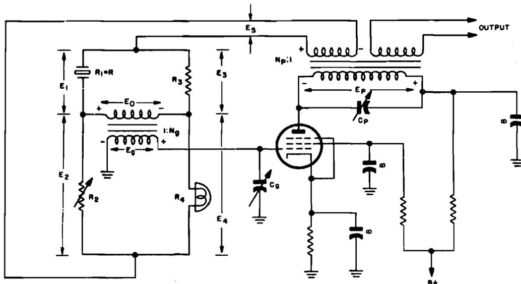
Figure 1-160. Basic circuit of Meacham bridge-stabilized oscillator
