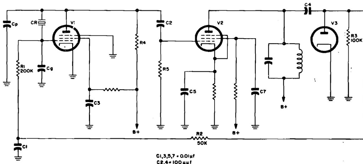
Figure 1-131. Pierce oscillator with automatic gain control
