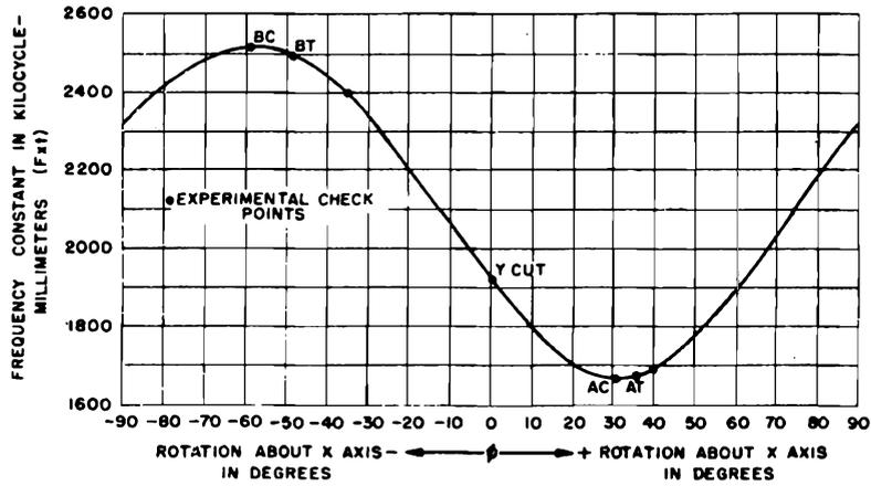
Figure 1-43. Frequency constant versus angle of rotation about X axis for thickness-shear elements of Y group. (Values shown for Y, BT, and BC cuts are smaller than the average) \*
