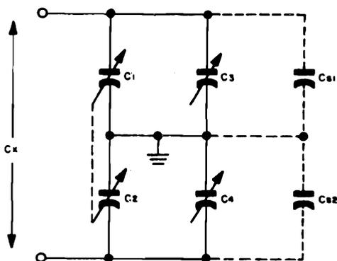
Figure 1-134. Ganged capacitances to enable adjustment of  $C_s/C_o$  ratio of Pierce circuit without changing total load capacitance
