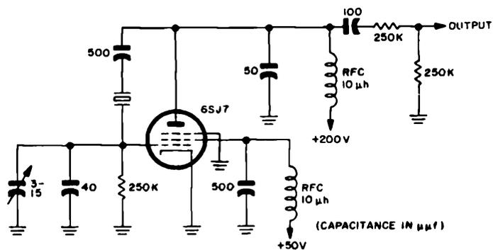
Figure 2-46. Schematic diagram of typical oscillator designed for use with Crystal Unit CR-44/U
