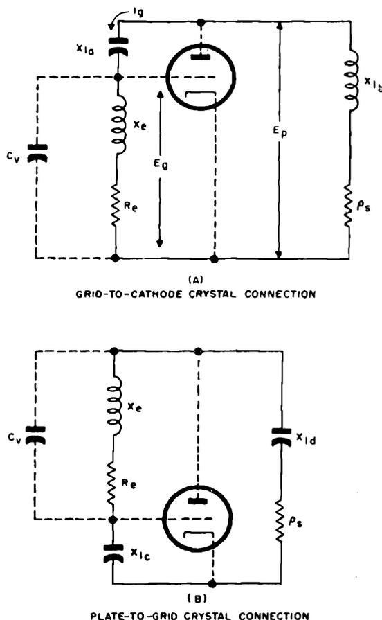
Figure 1-109. Generalized crystal oscillator circuits, showing two conventional methods for connecting crystal unit ( $X_c, R_e$ ) in feed-back circuit
