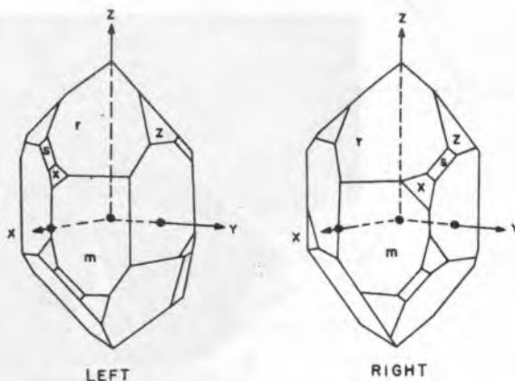
Figure 1-4. Left and right quartz crystals
