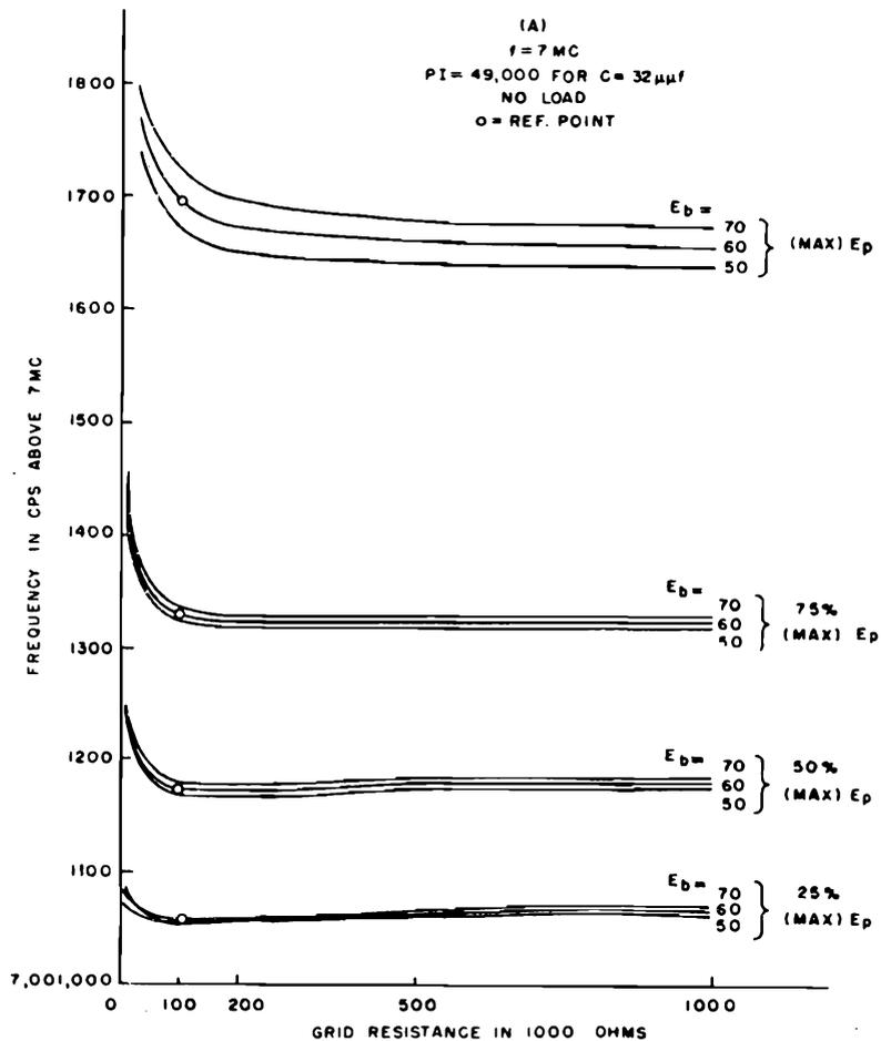
Figure 1-129. Frequency of tuned Pierce oscillator versus plate voltage and grid resistance for various plate-tuned load capacitances. (Max)  $E_p$  represents plate tuning adjustment that provided maximum r-f plate voltage when grid resistance and d-c plate voltage were values indicated by zero reference point. A 7-mc CR-18/U crystal unit was used, having a PI of 49,000 ohms when operating into a rated load capacitance of 32  $\mu\text{f}$
