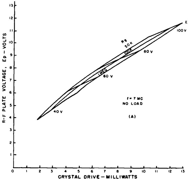
**Figure 1-130. Output curves of tuned Pierce oscillator for different values of grid resistance when reactance of tuned plate circuit is adjusted for output voltages equal to 50 percent of the maximum attainable. A 7-mc CR-18/U crystal unit was used, having a PI of 49,000 ohms when operating into its rated load capacitance of 32  $\mu\mu$ f**
