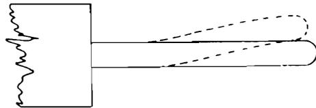
**Figure 1-82. Resonant motion of cantilever pin when its length is equal to one-quarter wave-length of clamp-free flexural vibration. Note that the effective free end of the pin is that end supporting the crystal (not shown) \***
