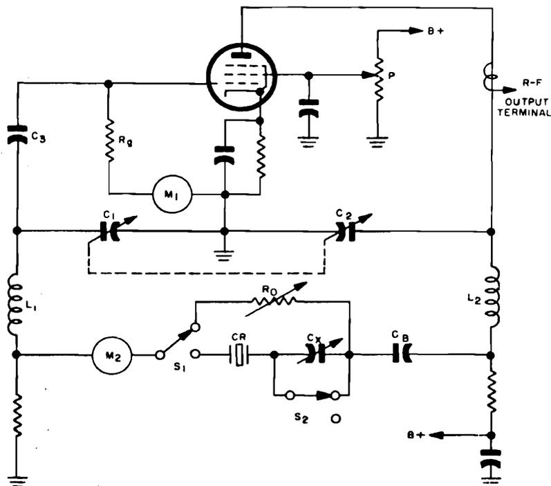
Figure 1-106. Simplified schematic diagram of CI meter
