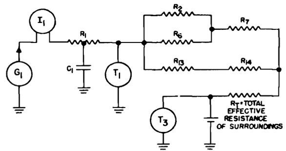
**Figure 4-13. Thermal D-C path of crystal power**
