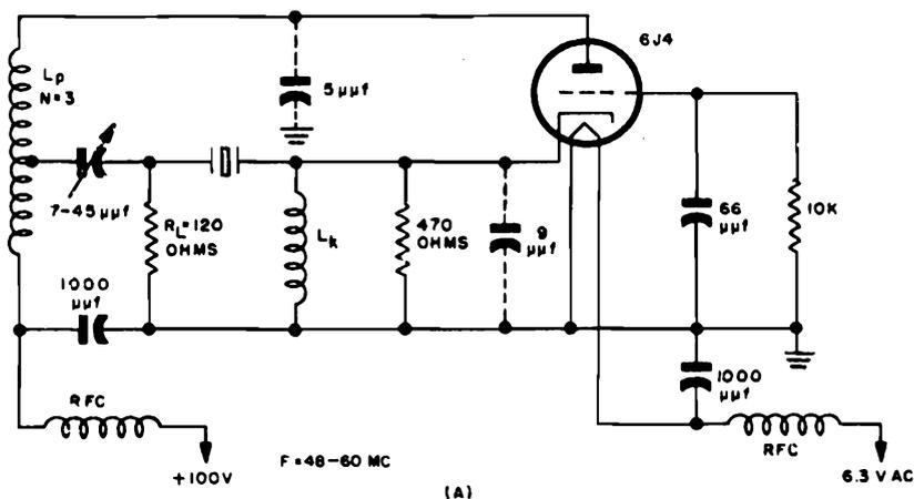
Figure 1-179. Modifications of grounded-grid oscillator. (A) Narrow-band circuit
