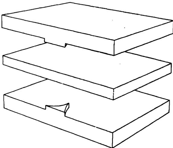
Figure 1-72. Typical nodal-clamped, air-gap method of mounting crystals
