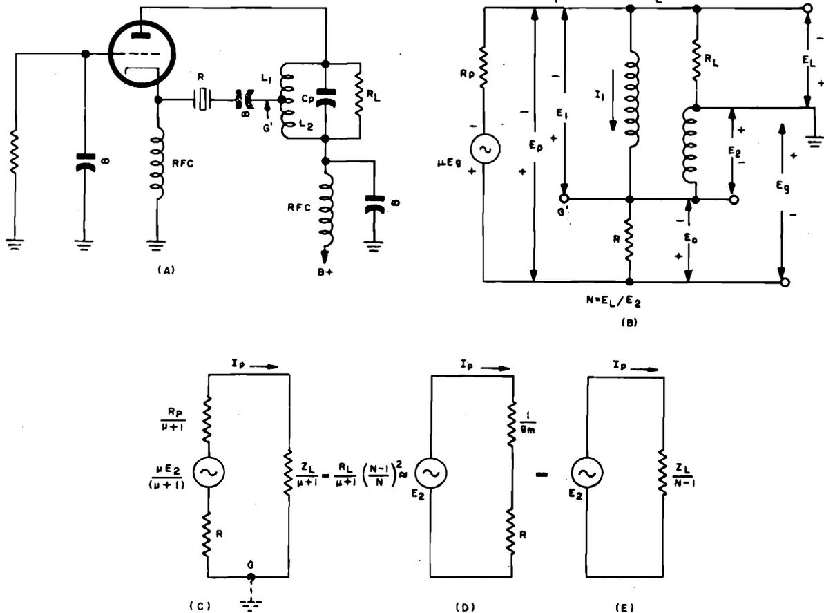
Figure 1-178. Basic grounded-grid oscillator and equivalent circuit progressively simplified
