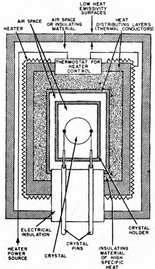
Figure 4-1. General construction features of typical crystal oven
