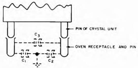
Figure 4-18. Pin-to-pin electrostatic capacitance of crystal oven
