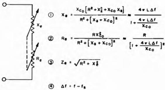
**Figure 1-98.** Equivalent circuit of crystal unit when represented as an effective reactance in series with an effective resistance. The ganged arrows indicate that  $X_e$  and  $R_e$  will vary together with changes in the frequency, as indicated by the approximate formulas given as functions of  $\Delta f$ . ( $X_{c0}$  is negative.)
