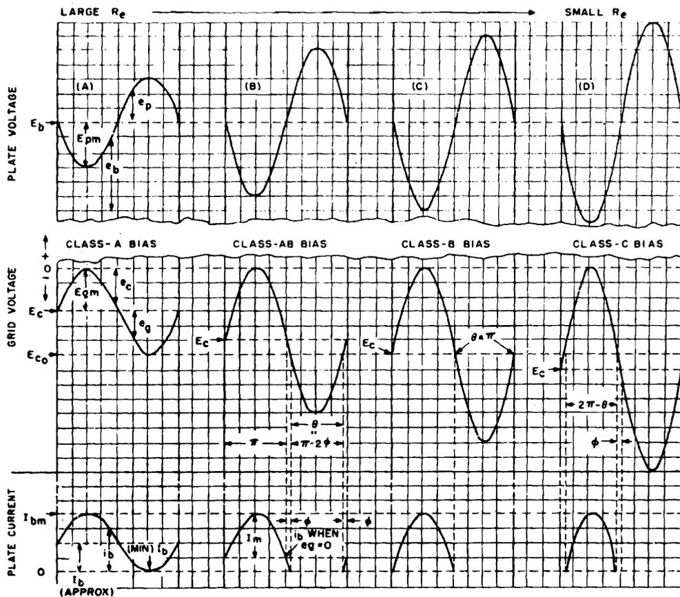
Figure 1-132. Change of state of Pierce oscillator with a  $C_g/C_p$  ratio of one, under no-load conditions when  $E_b$  is held constant and the effective resistance of the crystal changes
