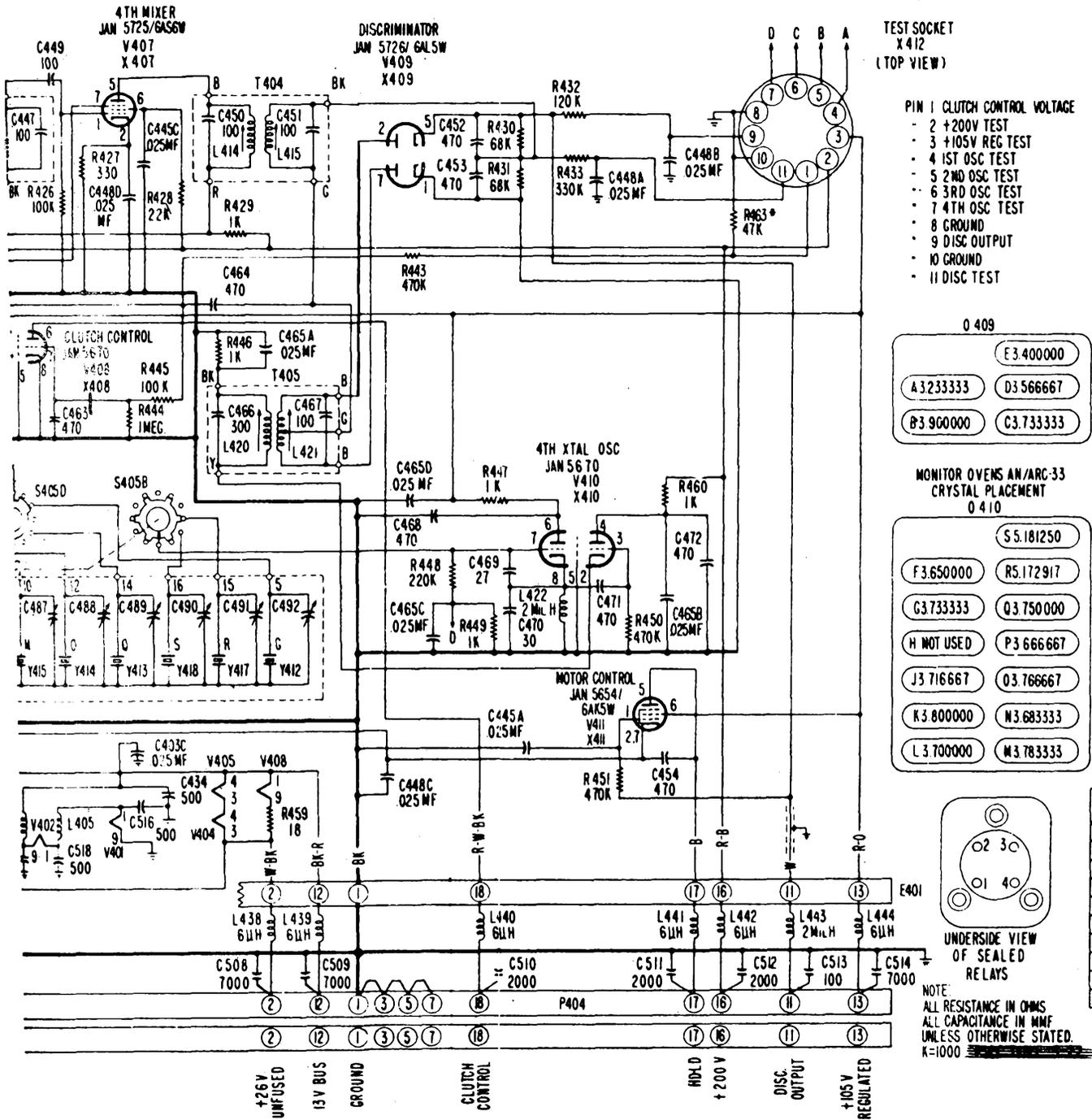
Figure 1-196. Monitor chassis. Schematic diagram of a-f-c system in Radio Set AN/ARC-33
