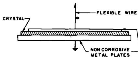
Figure 1-69. Gravity sandwich
