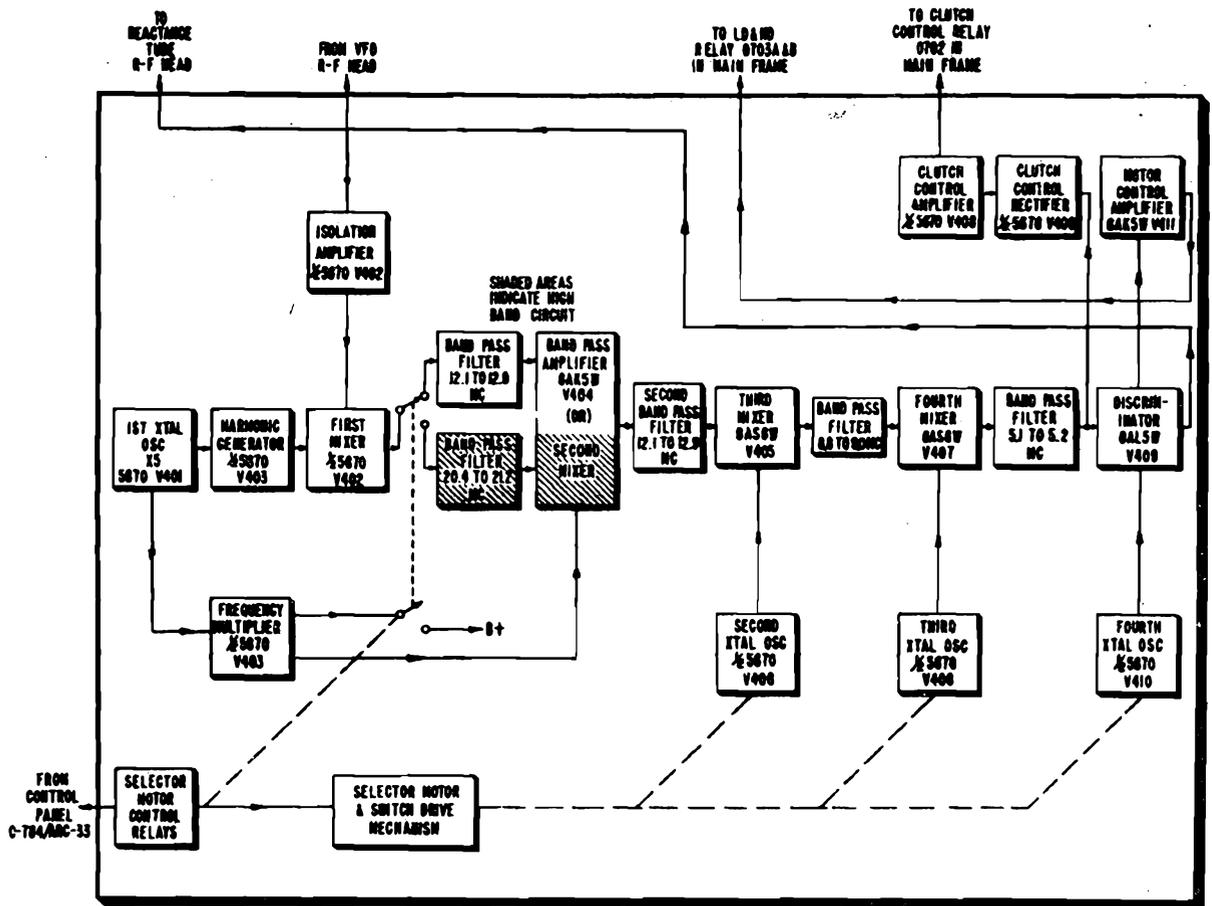
Figure 1-195. Monitor chassis. Block diagram of a-f-c system in Radio Set AN/ARC-33
