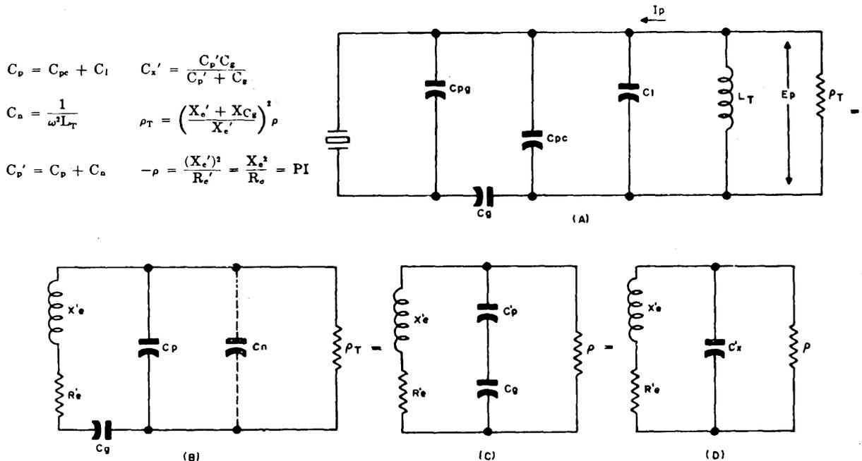
**Figure 1-121. Generalized Pierce oscillator.  $X_e'$  and  $R_e'$  are the effective impedance parameters of the crystal unit based upon the assumption that  $C_{pg}$  is a part of  $C_o$ .  $C_x$  is an equivalent negative capacitance having a positive reactance equal to that of  $L_T$ .  $I_p$  is the  $r$ - $\frac{1}{2}$  plate current of the vacuum tube.**
