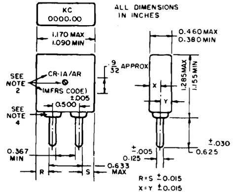
**Figure 3-23. Crystal Holder for Crystal Unit CR-1A/AR**
