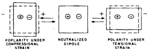
**Figure 1-7. Effective polarities resulting from sudden displacements of the centers of charge of a neutralized dipole. (If after displacement, the crystal were maintained indefinitely in the strained position, the effective polarity would eventually be neutralized by an accumulation of ions at the poles. A sudden return from such a state would thus result in an effective polarization in the unstrained position)**
