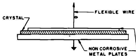
Figure 1-69. Gravity sandwich
