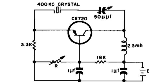
**Figure 1-236.** Frequency-stabilized circuit for single battery supply
