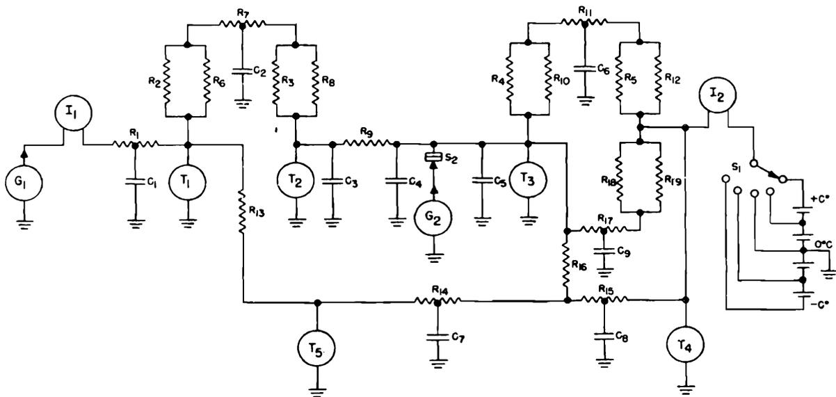
**Figure 4-12. Equivalent electrical circuit of crystal oven**
