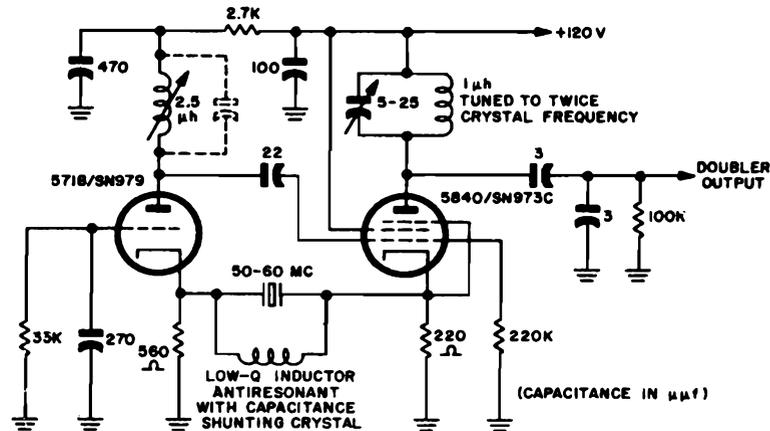
Figure 2-26. Schematic diagram of typical oscillator designed for use with Crystal Unit CR-32/U
