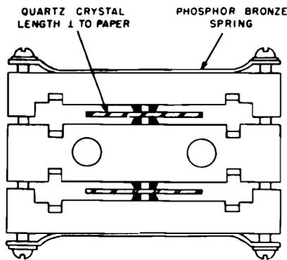
**Figure 1-83. Knife-edge clamp support for two crystal plates. Each crystal has two pairs of plated electrodes, and is so mounted that each pressure blade makes electrical contact with a different electrode. This arrangement effectively provides four crystal elements for use in a balanced filter circuit\*.**
