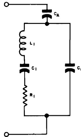
Figure 1-92. Simplified equivalent circuit of air-gap crystal unit
