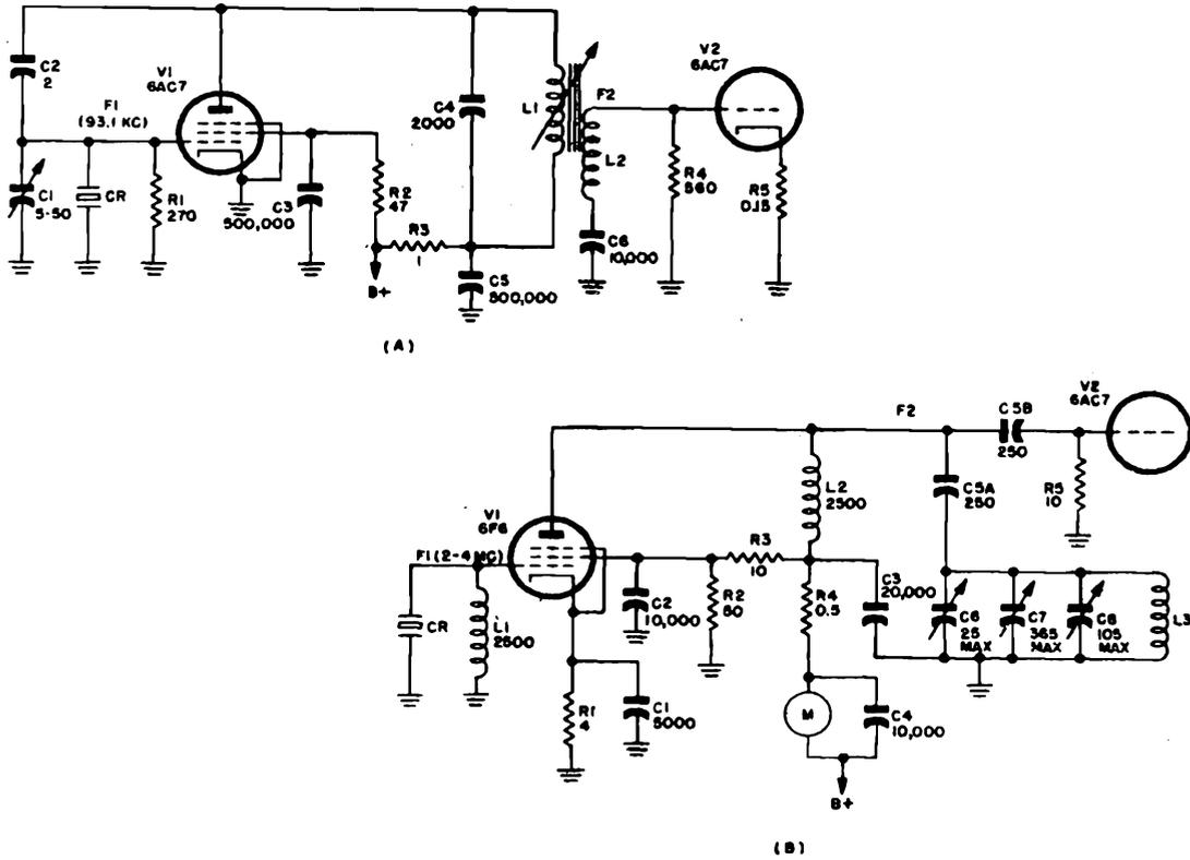
Figure 1-151. Miller oscillators using screen-grid tubes. (Effective suppressor in beam-power tubes is connected to cathode inside tube, although external connection may be indicated in diagram.)
