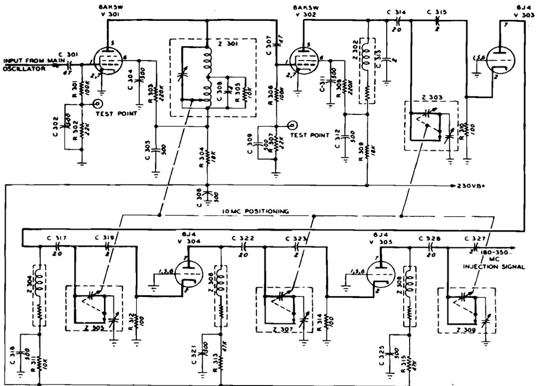
Figure 1-206. Multiplier-amplifier unit of 1st injection system in Radio Receiver R-278/GR. Schematic diagram
