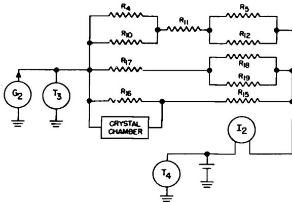
Figure 4-14. Thermal D-C path of heater power
