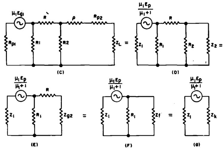
Figure 1-173. (A) Basic diagram of Butler two-stage cathode-coupled oscillator. (B) Equivalent r-f circuit of Butler oscillator. Current arrows indicate instantaneous electron flow when r-f voltages have polarities shown. (C) Simplified equivalent circuit where generator of grounded-grid amplifier is replaced by a negative resistance. (D), (E), (F), and (G) Progressive simplifications of equivalent Butler circuit
