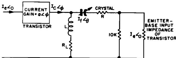
**Figure 1-225. Simplified equivalent circuit of junction transistor crystal-feedback oscillator, showing tuned tank in collector circuit for obtaining desired current amplification and loop phase shift for feedback to emitter input. For stable oscillations to be maintained**
