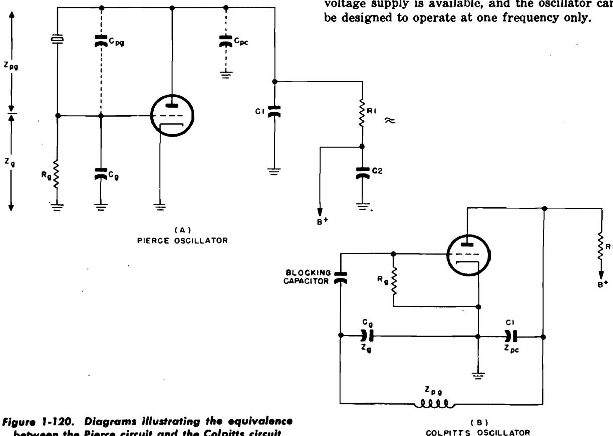
Figure 1-120. Diagrams illustrating the equivalence between the Pierce circuit and the Colpitts circuit
