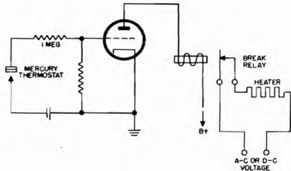
Figure 4-8. Heater control circuit using mercury thermostat
