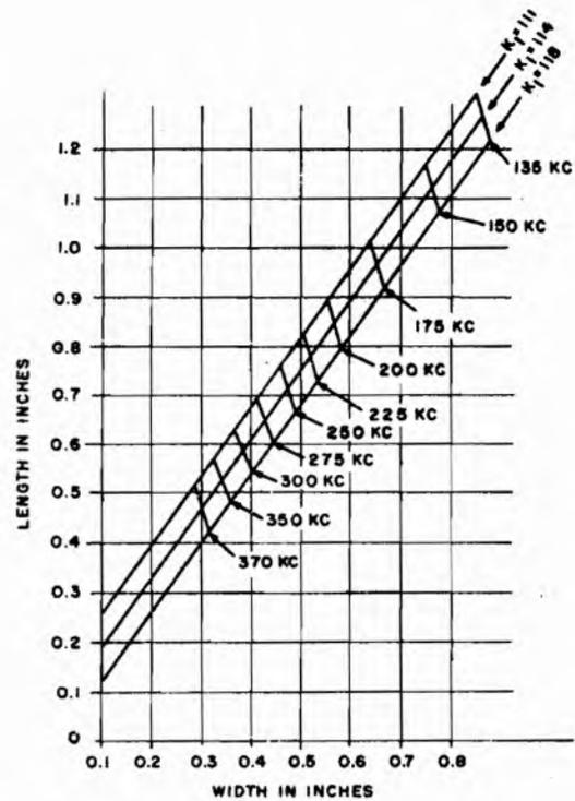
Figure 1-22. Frequency characteristics of X-cut crystal vibrating in width-extensional mode, where the width is parallel to the Y axis.  $w/l$  ratios not included between the two outer curves will have interfering modes.  $K_1$  is in kc-inches
