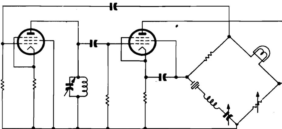
Figure 1-164. Two-stage Meacham bridge-stabilized oscillator
