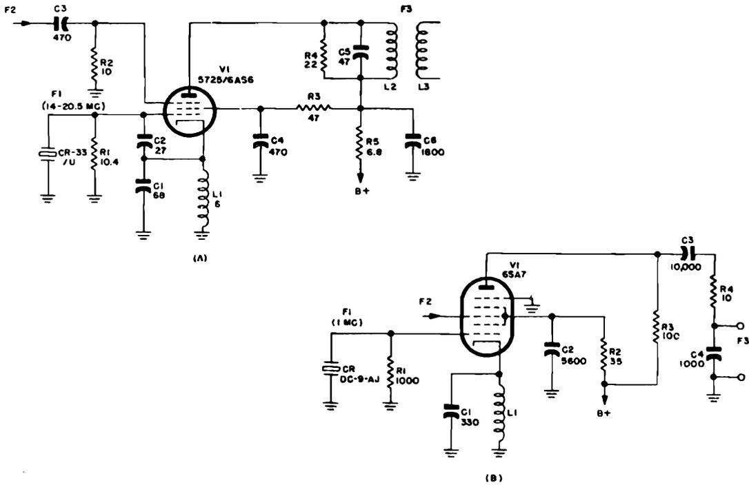
Figure 1-138. Electron-coupled Pierce oscillator modifications for heterodyne circuits
