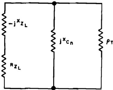
Figure 1-122. Generalized Pierce oscillator.  $X_{ZL}$  and  $X_{Cn}$  represent the positive magnitudes of the equivalent reactances of the load and the dynamic effects of the tube, respectively.  $\rho_T$  is the same as the  $\rho_T$  in figure 1-121
