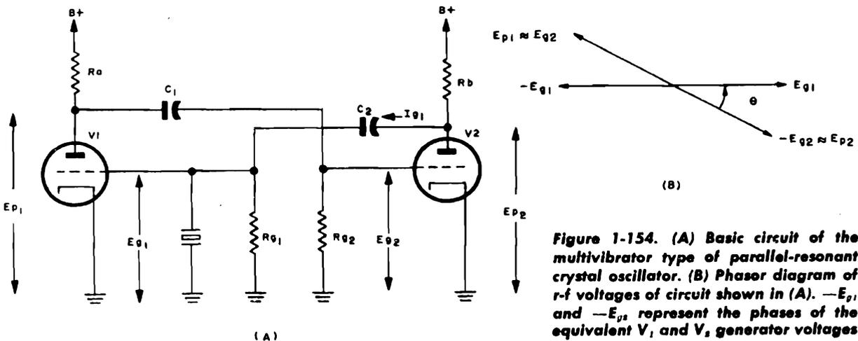
Figure 1-154. (A) Basic circuit of the multivibrator type of parallel-resonant crystal oscillator. (B) Phasor diagram of r-f voltages of circuit shown in (A).  $-E_{g1}$  and  $-E_{g2}$  represent the phases of the equivalent  $V_1$  and  $V_2$  generator voltages
