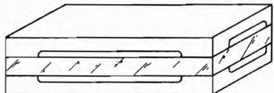
Figure 1-71. Typical corner-clamped, air-gap method of mounting crystals \*
