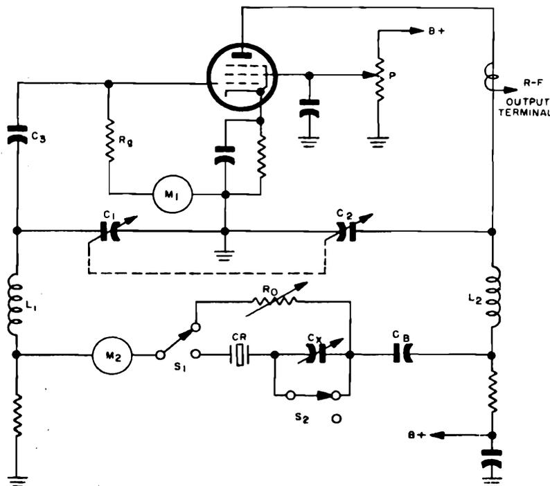
Figure 1-106. Simplified schematic diagram of CI meter
