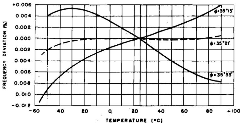
Figure 1-49. Temperature-frequency characteristics of element A
