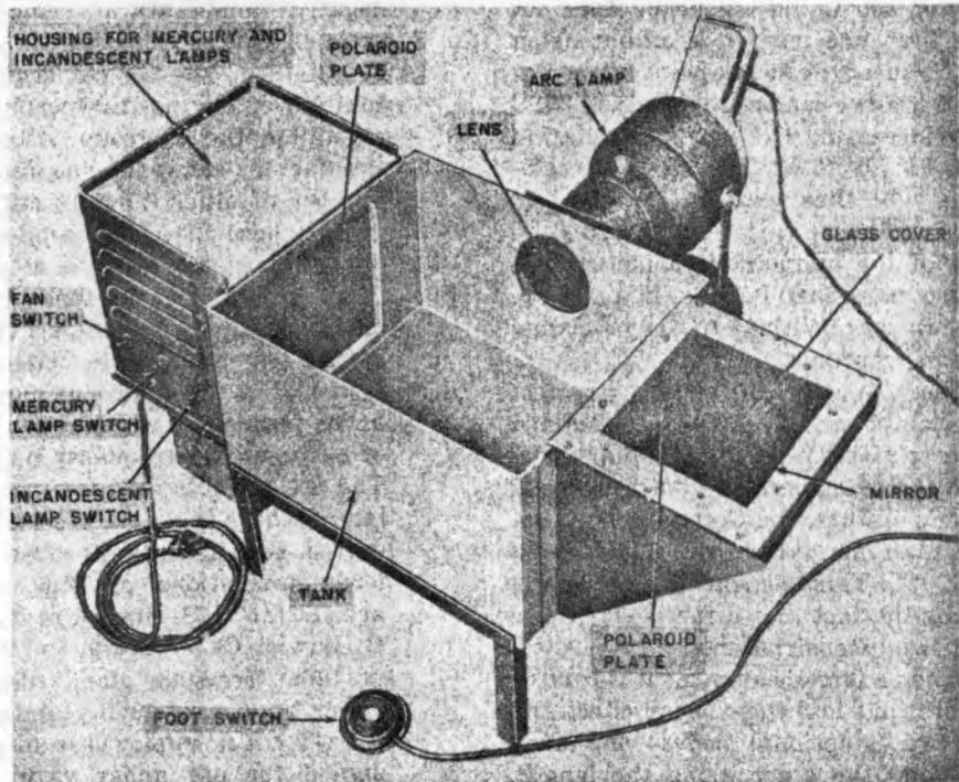
**Figure 1-57. Polariscope-Inspectoscope. Used for examining raw quartz**
