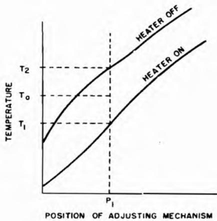
Figure 4-3. Typical differential curves of adjustable thermostat
