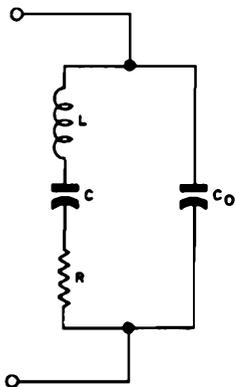
Figure 1-91. Simplified equivalent circuit of crystal unit
