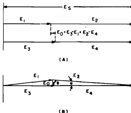
Figure 1-161. Phasor diagrams of bridge voltages in Meacham oscillator. Angles  $\phi$  and  $\theta$  (greatly magnified) represent small shifts in phase when crystal unit is operating slightly off series resonance
