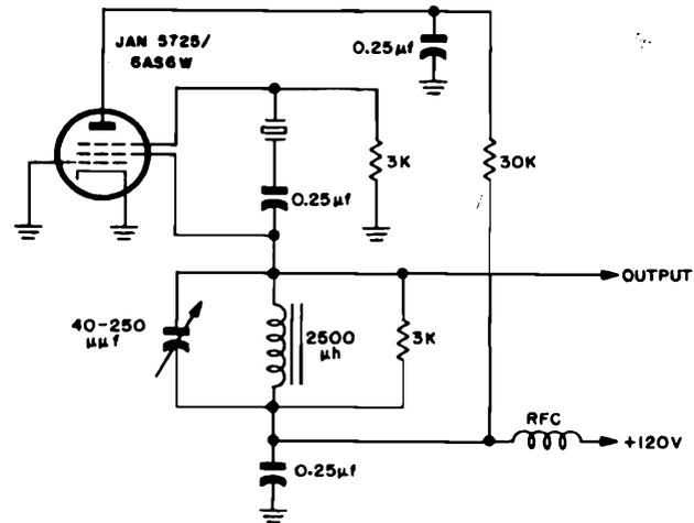
Figure 2-16. Schematic diagram of typical oscillator designed for use with Crystal Unit CR-26/U
