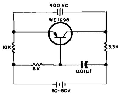
**Figure 1-238.** Crystal-feedback oscillator in which the resistance parameters have been selected empirically to provide maximum frequency stabilization for the particular 400-kc crystal unit and point-contact transistor being used
