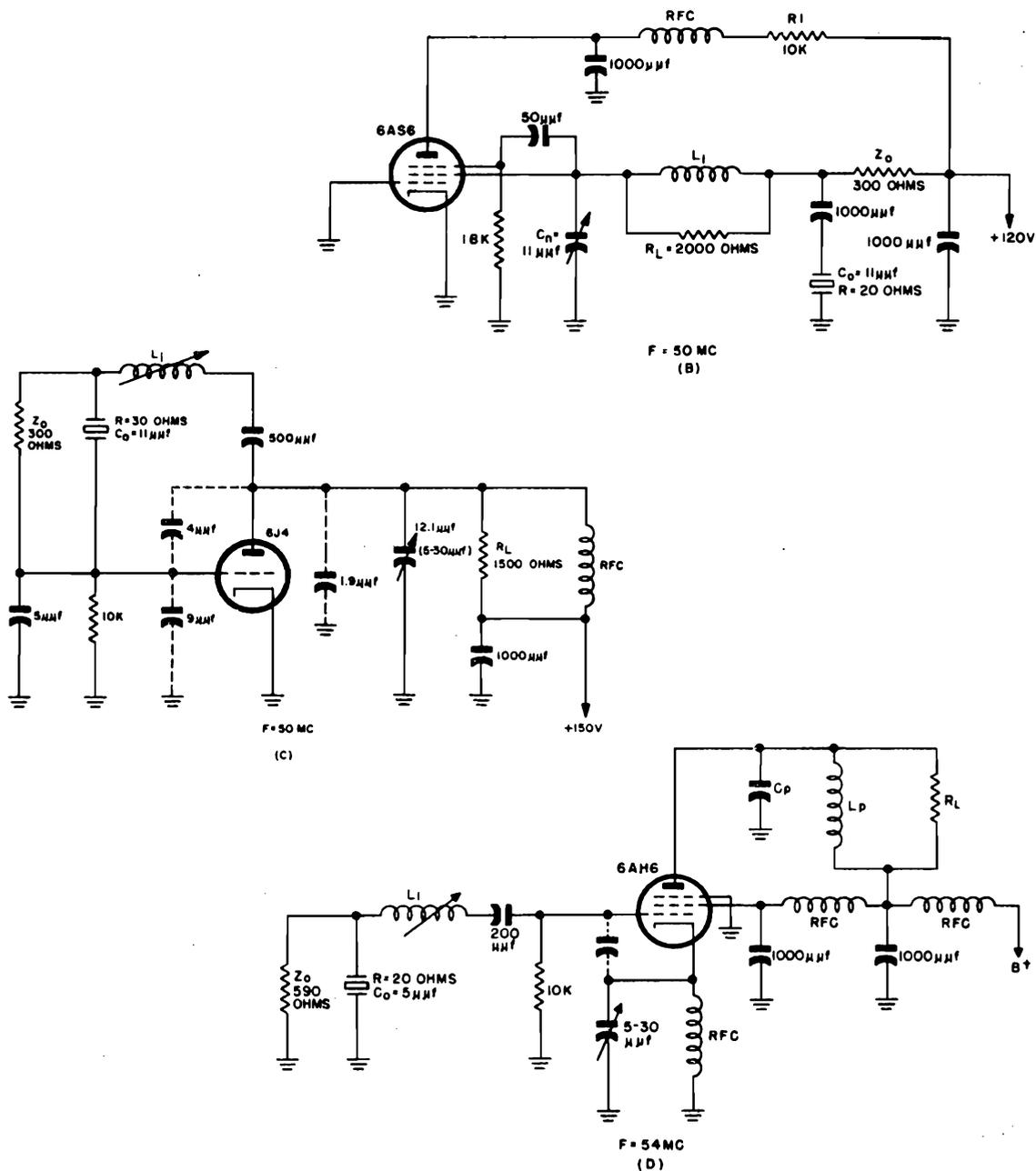
Figure 1-182. Impedance-inverting oscillator circuits. (B) Impedance-inverting transitron oscillator. (C) Impedance-inverting Pierce oscillator. (D) Impedance-inverting electron-coupled Pierce oscillator
