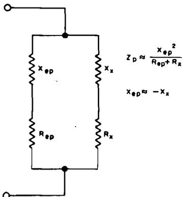
Figure 1-101. Equivalent parallel-resonant circuit of crystal unit ( $X_{cp}$ ,  $R_{cp}$ ) shunted by load ( $X_x$ ,  $R_x$ ). Normally  $f_r < f_p < f_a$ , so that  $X_{rp}$  is inductive and  $X_x$  is capacitive
