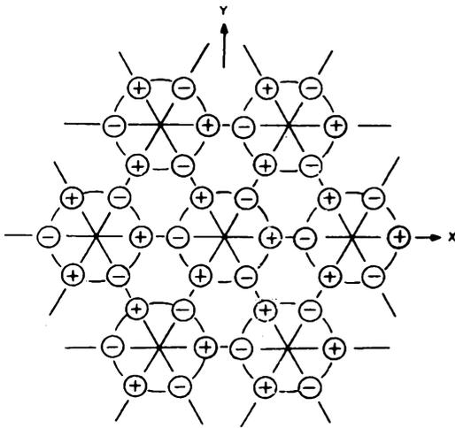
**Figure 1-9. Kelvin's molecular model of the charge distribution of alpha quartz. The positive direction shown for the X axis corresponds to that of right quartz, for a compression along that axis will cause the piezoelectric polarities to coincide in sign with the X-axial directions. For left quartz, the sign of the Y, as well as the X, axis must be reversed in order to maintain a right-handed coordinate system \***
