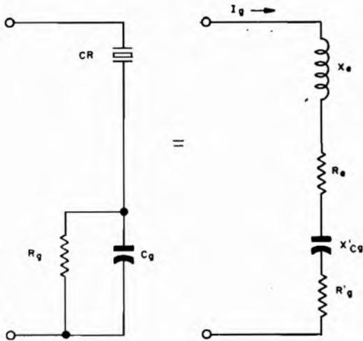
$$\textcircled{1} \quad Q_{pfc} = \frac{X_g + X'_{cg}}{R_g + R'_{g}} \quad \textcircled{3} \quad Q_f = \frac{Q_{pfc} Q_g - 1}{Q_{pfc} + Q_g}$$
