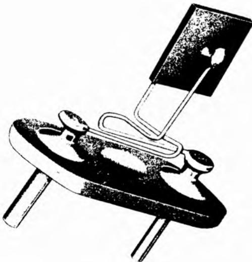
**Figure 1-85. Solder-cone wire mounting of face-shear element**
