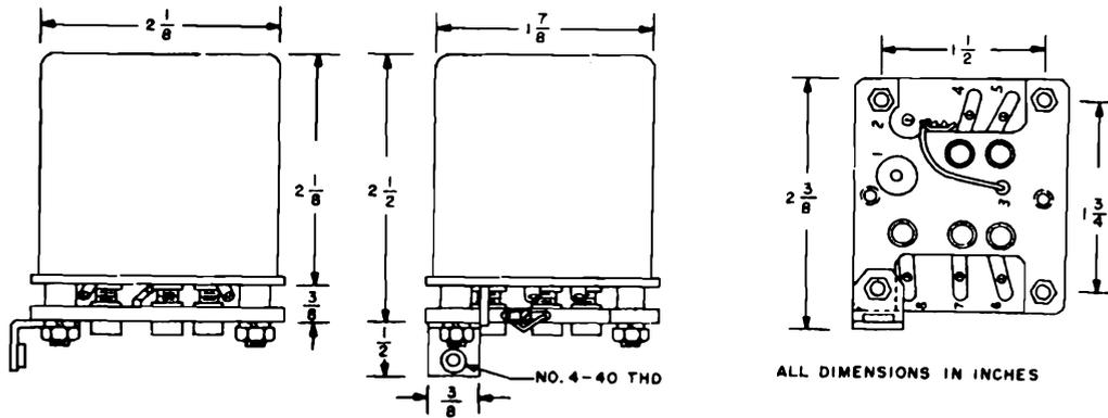
**Figure 4-21. Dimensions of Bendix Radio Crystal Oven L205628**
