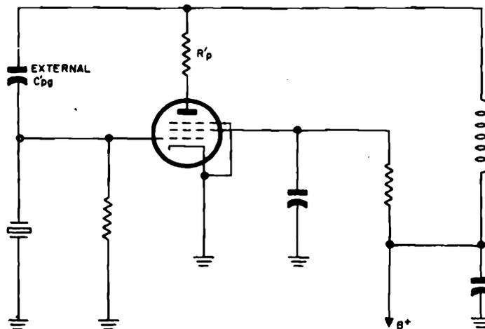
Figure 1-142. The large resistance,  $R_{p'}$ , connected in plate circuit effectively increases  $R_p$  of the tube. This method can be used to improve the frequency stability of a Miller oscillator employing a screen-grid tube and an externally connected feed-back capacitance,  $C_{bg}$
