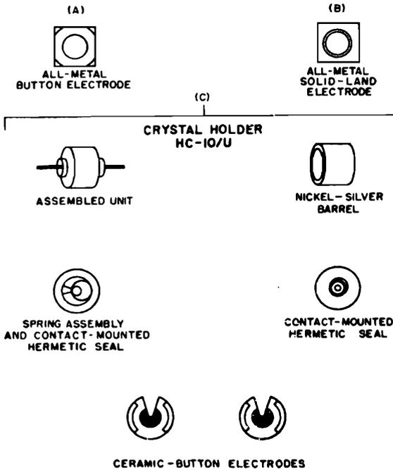
**Figure 1-79. Button electrodes and methods of mounting**
