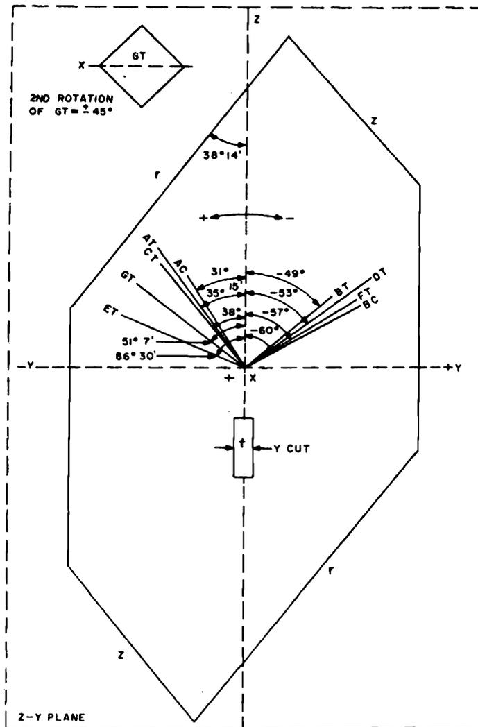
**Figure 1-42.** Rotation angles of Y cut about X axis which provide the principal members of the Y group. The GT cut is the only member having a second rotation ( $\pm 45^\circ$  about the Y' axis). The +X sign indicates that the positive end of the X axis points toward the observer
