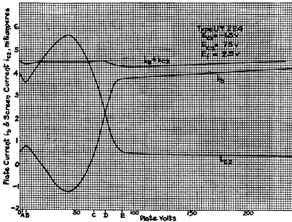
FIG. 12-6. The plate voltage—plate current characteristic curves showing the variations of current flow in the plate and screen-grid circuits, (curves marked  $i_b$  and  $i_{c2}$  respectively) and the total current flow, which is the sum of these two currents.
