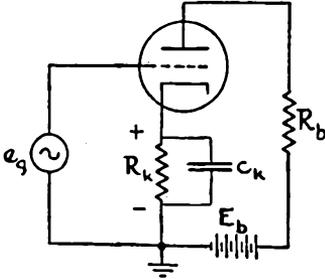
FIG. 13-3. The bypass condenser  $c_k$  in parallel with the cathode resistor bypasses the a-c component of the plate current and so only the d-c component flows through the resistor  $R_k$ . Thus the cathode-to-ground voltage remains constant.
