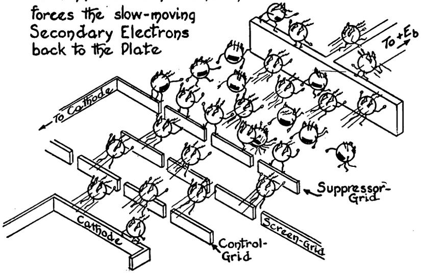
secondary electrons. In the absence of the suppressor-grid these secondary electrons would, because of the positive potential on the screen-grid, flow to the screen-grid. The suppressor is, however, at cathode (or ground) potential and therefore exerts a retarding effect upon these secondary electrons so that they are forced to return to the plate.
