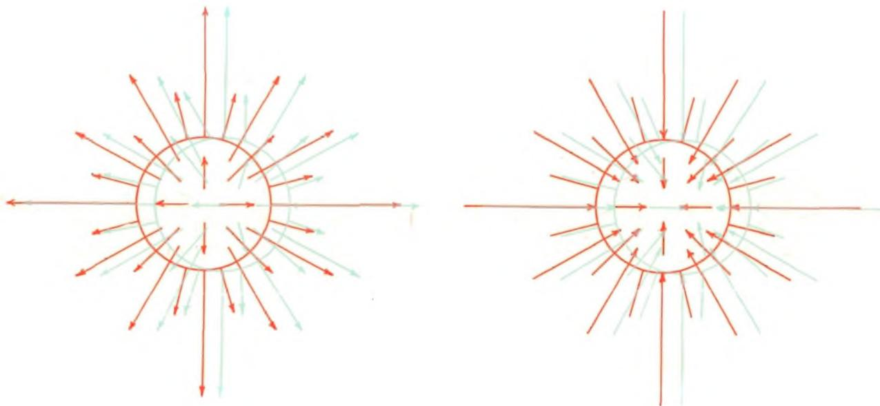
PLATE 2. The arrows indicate that the lines of force are away from the electron and towards the proton; the direction of the force exerted upon a negative test charge is indicated by the arrows. The lines of force radiate in all directions.
