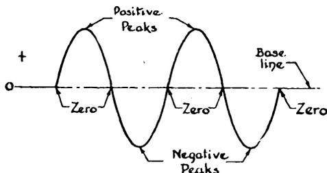
voltage and the signal voltage. Assuming for the moment that the signal voltage  $e_p$  is of alternating character, you can see that in a wave of alternating voltage, as well as current, there are instants when the value of the alternating component of voltage or current is zero. These contrast with the other instantaneous values, which reach their maximum at the peaks of the positive and negative half cycles, as shown in Fig. 10-3.
