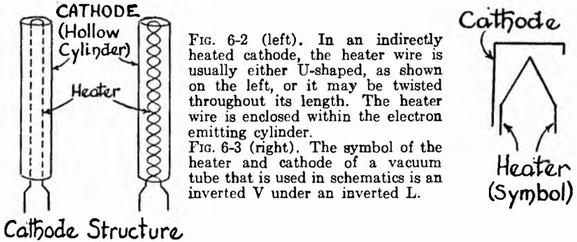
FIG. 6-2 (left). In an indirectly heated cathode, the heater wire is usually either U-shaped, as shown on the left, or it may be twisted throughout its length. The heater wire is enclosed within the electron emitting cylinder.
