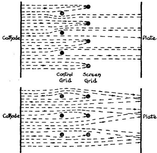
of the two grids are not arranged in this fashion, electrons are forced out of their paths by the negative charge on the control-grid and a large number of these are attracted by the positive charge of the screen-grid, thus forming the screen current, while other electrons, although deviating from their paths, miss the screen-grid and continue on to the plate. This action is illustrated in Fig. 14-12, wherein the lines indicate the paths of a few of the electrons.
