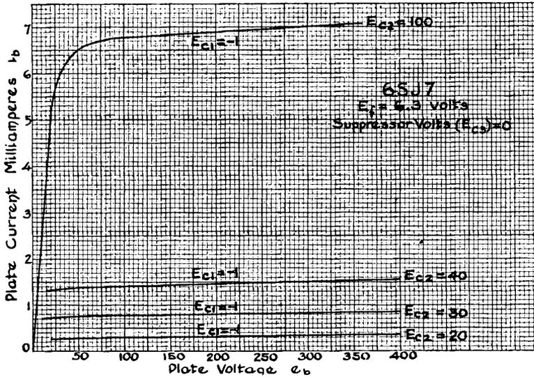
FIG. 12-12. These characteristics were made with the same control-grid voltage ( $-1$  volt) and different values of screen-grid voltage. Note that the plate current increases with an increase in  $E_{c2}$ .
