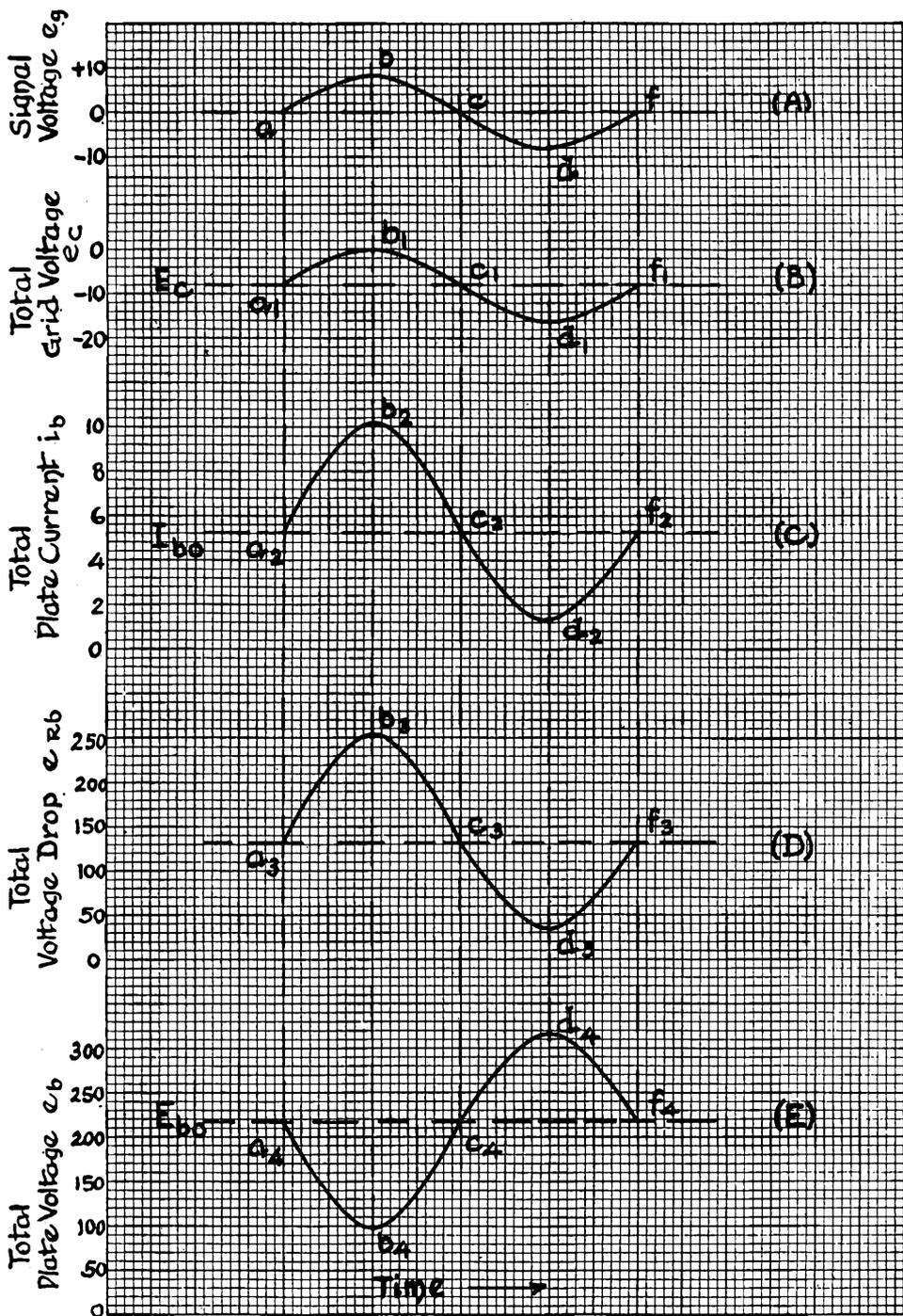
FIG. 11-8. This series of waves shows that the input voltage  $e_g$  is in phase with the plate current  $i_b$  and that  $e_c$  is  $180^\circ$  out of phase with the plate voltage  $e_b$ .
