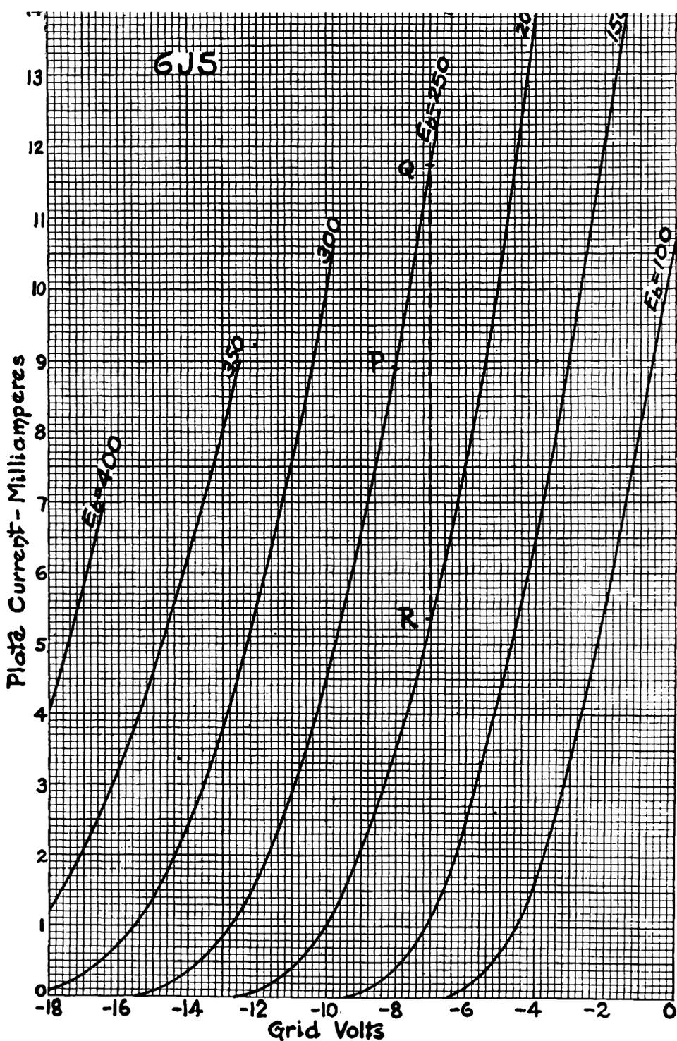
FIG. 8-9. The grid family of characteristic curves can be used to determine either the d-c or a-c plate resistance of a triode; here the resistance is found at point P, which is 250 volts on the plate and -8 volts on the grid.
