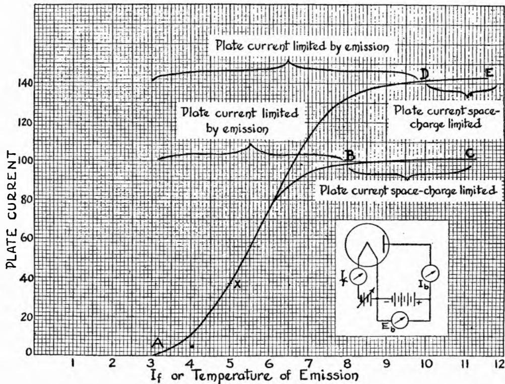
FIG. 6-9. Emitter temperature—plate current characteristic. These curves show that the plate current does not increase appreciably above a certain value even though the temperature of the emitter is increased.
