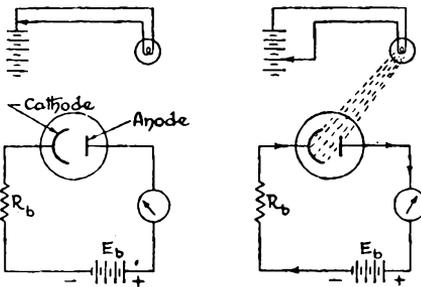
FIGS. 15-47 (left), 15-48 (right). When no light energy falls on the cathode of a photocell, no electrons flow through the anode circuit in which is connected the load  $R_b$ . In Fig. 15-48 light is indicated hitting the cathode of the photocell with a resulting current flow through the anode circuit.
