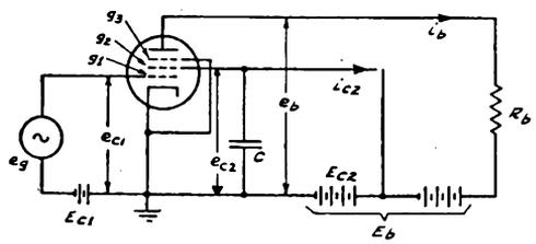
sired, the screen may be at the same potential as the quiescent plate voltage, since the harmful effects of secondary emission have been eliminated as a result of suppressor-grid action. With regard to signal voltages, however, the screen-grid is effectively at ground potential in virtue of the bypassing effect of condenser C.
