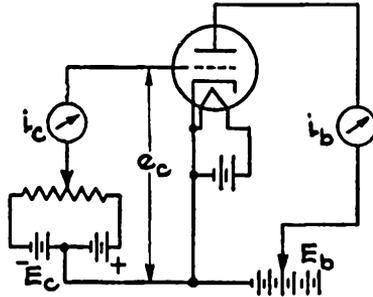
the plate voltage at a low value, we slide the movable arm of the potentiometer towards the middle, making the grid voltage less and less negative. While this is being done, the plate milliammeter shows an increasing plate current, but still nothing is indicated on the grid microammeter. More electrons go to the plate (as indicated by the increasing plate current) because the plate-cathode field is less and less counteracted by the gradual reduction of the grid-cathode field.
