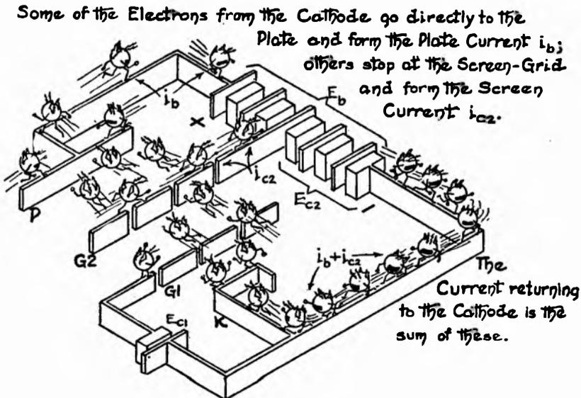
with a certain velocity. Some of these electrons will make direct hits on the wires of the screen-grid and flow out into its external circuit; this electron flow is the *screen current*  $i_{c2}$ . The rest of the electrons will travel on to the plate and form the plate current  $i_b$ . Most of the electrons pass through the openings of the screen-grid mesh and continue on to the plate. So by and large, the plate is a collector of electrons in the tetrode as it is in the triode.
