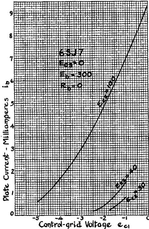
actual working conditions, insofar as they represent more nearly ideal operation than would be the case with a resistive load of high magnitude. Since, as we have already indicated, audio-frequency voltage amplifiers are generally operated at low screen-grid voltages, we observe how limited the permissible control-grid swing becomes. This partly accounts for the rule that the input signal to a voltage amplifier pentode should never exceed several tenths of a volt.
