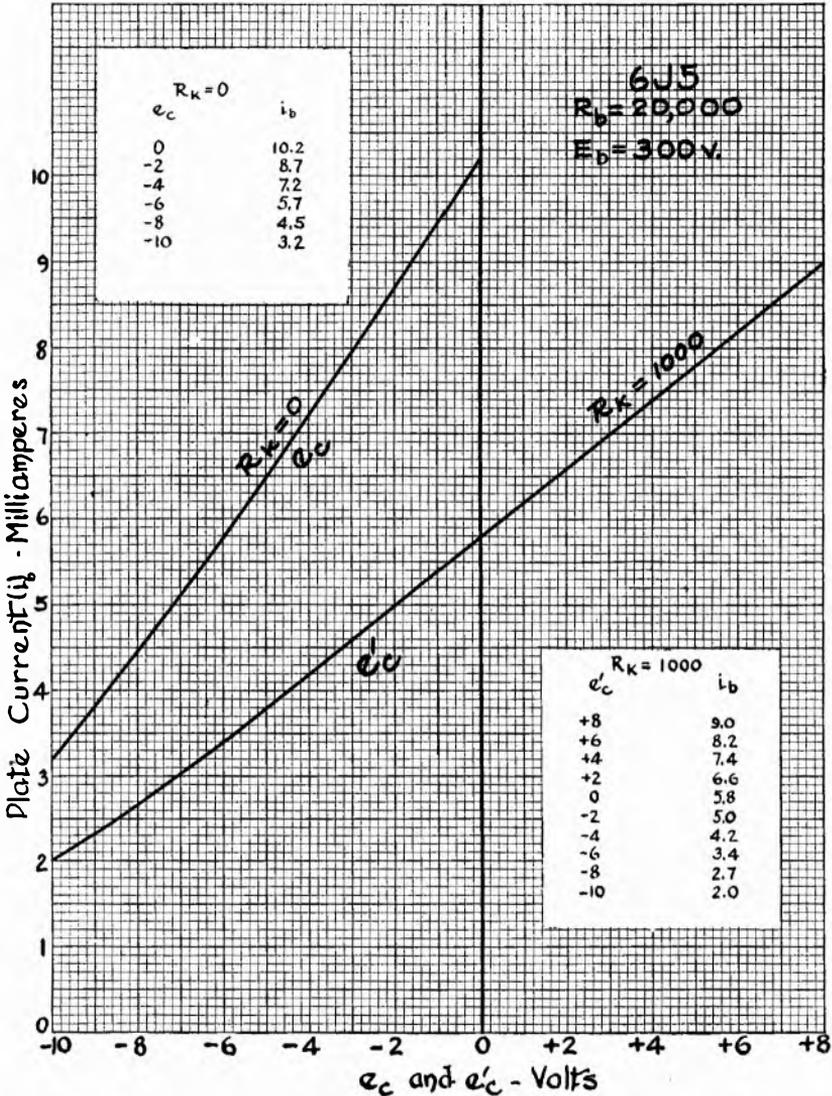
FIG. 13-8. The difference that a cathode resistor makes in the dynamic transfer characteristic of a triode is illustrated by these two curves. The curve marked  $e_c$  was derived when no cathode resistor was included, and the  $e'_c$  curve was derived when 1000 ohms was in the cathode circuit. In both instances a plate load of 20,000 ohms was used.
