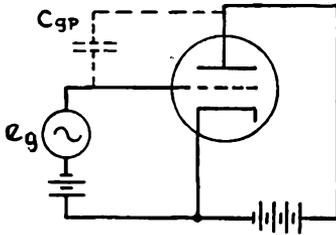
FIG. 12-3. The capacity  $C_{gp}$  existing between the grid and the plate in a triode can be disregarded at low frequencies, but at high frequencies (above 15,000 cycles) this capacity effect interferes with proper operation of the tube. The screen-grid of the tetrode greatly reduces this condition.
