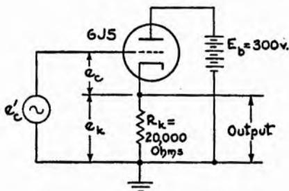
In order to find out the characteristics of a cathode follower circuit, let us examine the circuit of Fig. 13-9 more carefully. In particular, a 6J5 triode is shown, a cathode resistor  $R_k$  of 20,000 ohms, and a plate-supply voltage  $E_b$  of 300 volts. If a certain signal voltage  $e'_c$  is applied to the input, what will the output signal voltage  $e_k$  be?
