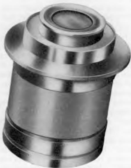
Fig. 16.1. Ceramic X-ray tube with a wide angle beryllium window for reproduction of Greuz Rays. Anode voltage 4 to 25 kv. Diameter of ceramic cylinder is 2 inch, over-all length  $3\frac{13}{16}$ "<sup>4</sup> (Courtesy Machlett Laboratories, Inc.)
