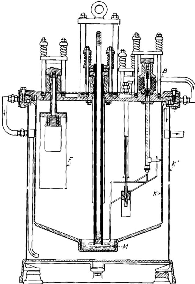
FIG. 99.—Cross-section of a Bergmann (Germany) rectifier.
