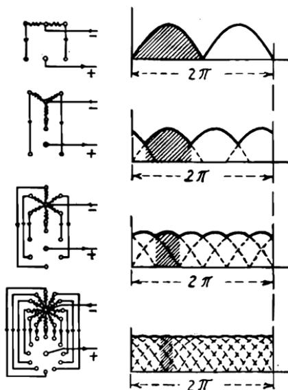
FIG. 15.—Current waves of single-phase and polyphase rectifiers.
