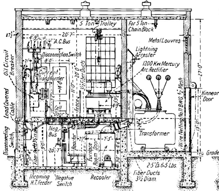
Cross-Section Through Rectifier Room
