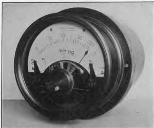
FIG. 128.— Brown Boveri contact-making vacuum meter.
