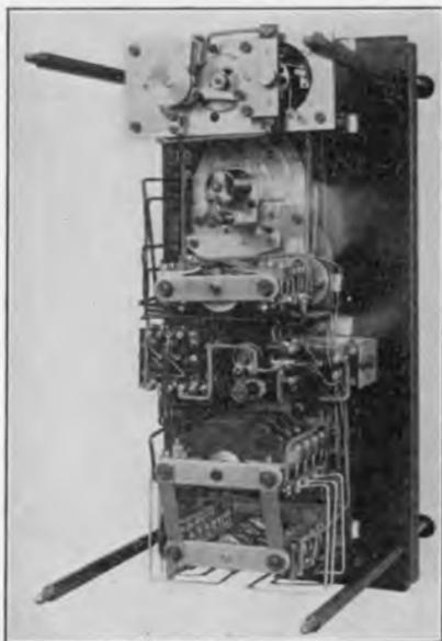
FIG. 171.—Brown Boveri automatic relay for controlling vacuum pump. The relay is denoted in Fig. 170 by device number 63VX.
