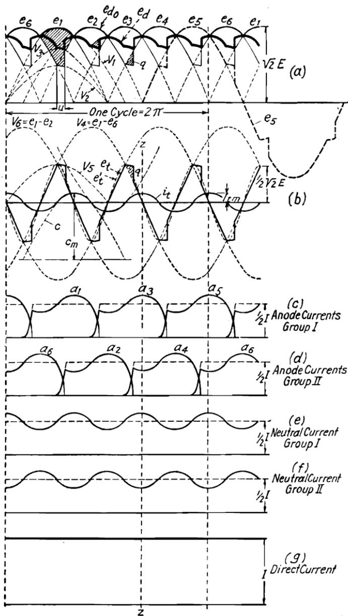
FIG. 57.—Waves of voltages and currents in the circuits of a rectifier having a 6-phase connection with interphase transformer, as shown in Fig. 55.
