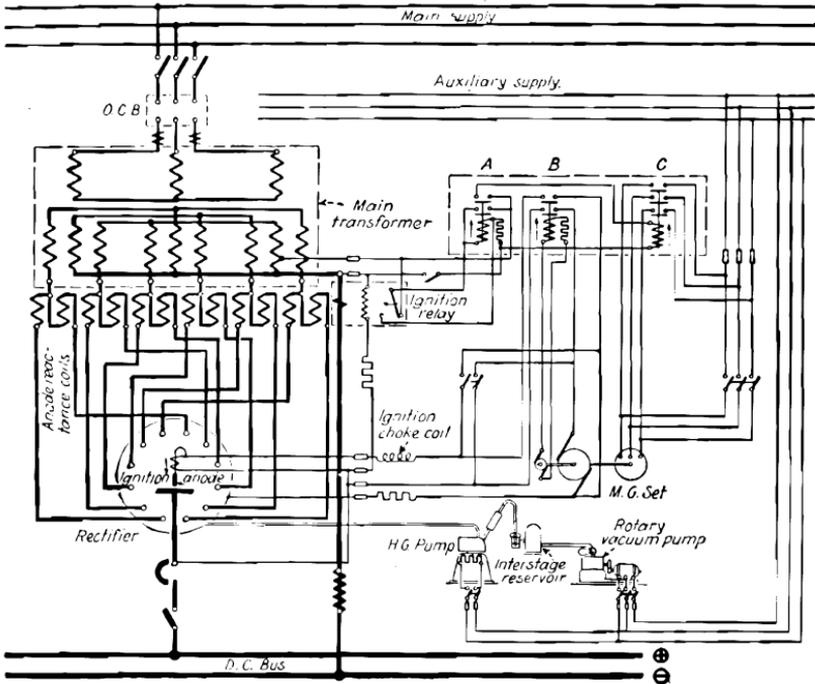
FIG. 134.—Connection diagram for a rectifier unit of the Allgemeine Elektrizitäts Gesellschaft (Germany), showing equipment and circuit for igniting arc.
