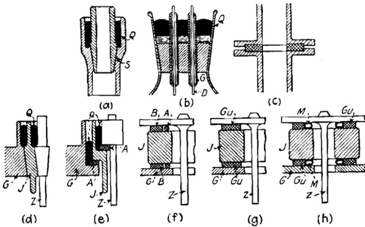
FIG. 104.—Schematic construction of several types of seals.
