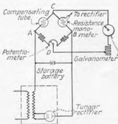
FIG. 132.—Connection diagram of General Electric hot-wire gage.
