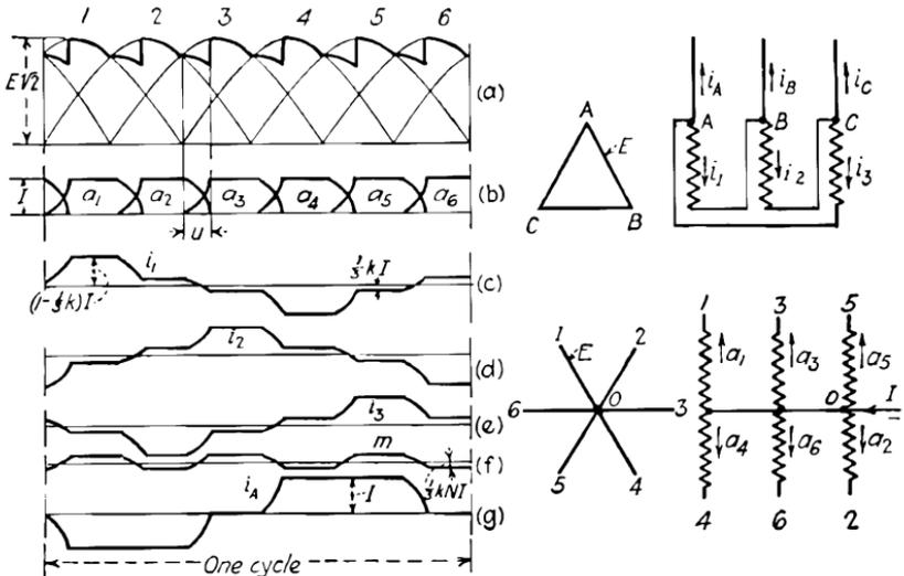
FIG. 49.—Diametrical 6-phase connection with delta primary.
