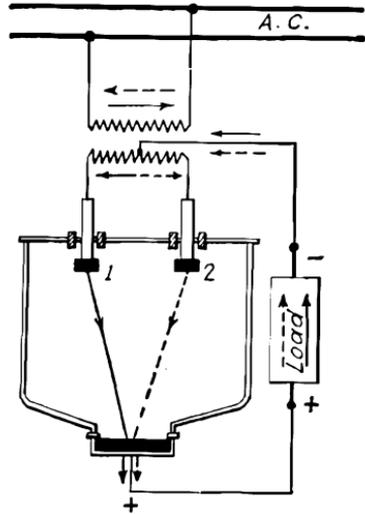
FIG. 12.—Diagram of single-phase, full-wave rectifier circuit.
