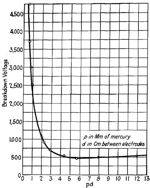
FIG. 9.—Curve showing the breakdown voltage of mercury vapor as a function of the vapor pressure and the distance between electrodes (349).
