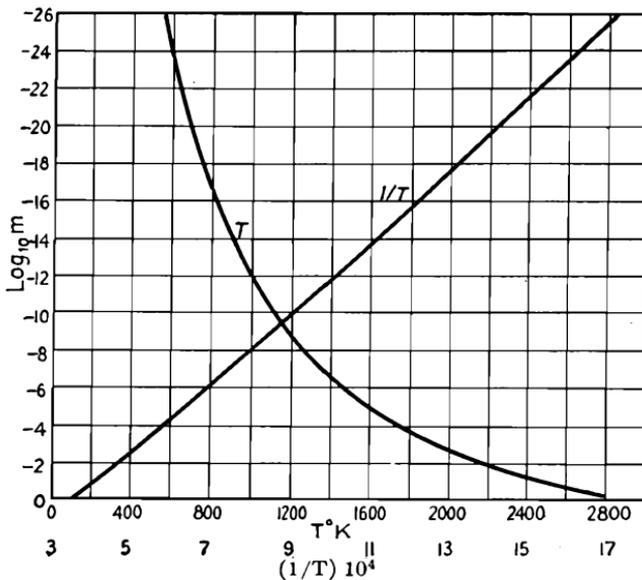
FIG. 11.—Rate of evaporation,  $m$ , of iron, in grams per square centimeter per second in vacuum, as function of the temperature in degrees Kelvin (335). (Degrees Kelvin = degrees C. + 273.13 degrees C.)
