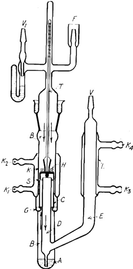
FIG. 115.—Gaede diffusion-type mercury vacuum pump.
