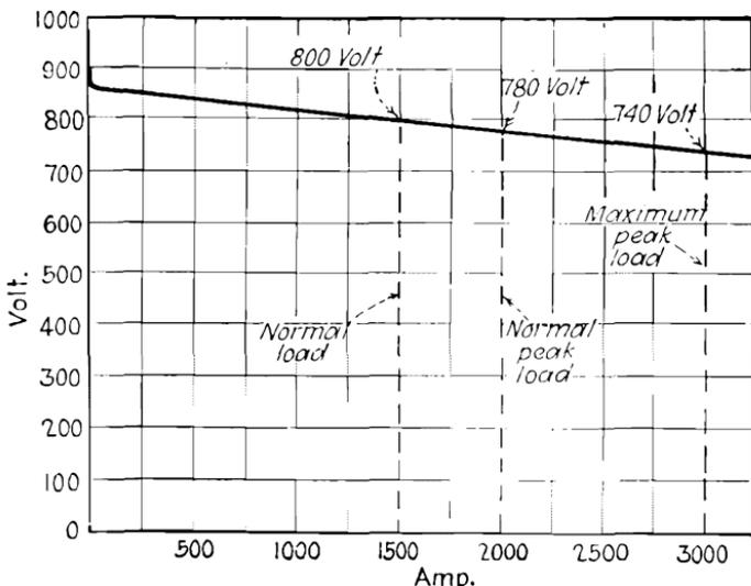
FIG. 163.—Voltage regulation curve of rectifiers on the Berlin elevated railways.
