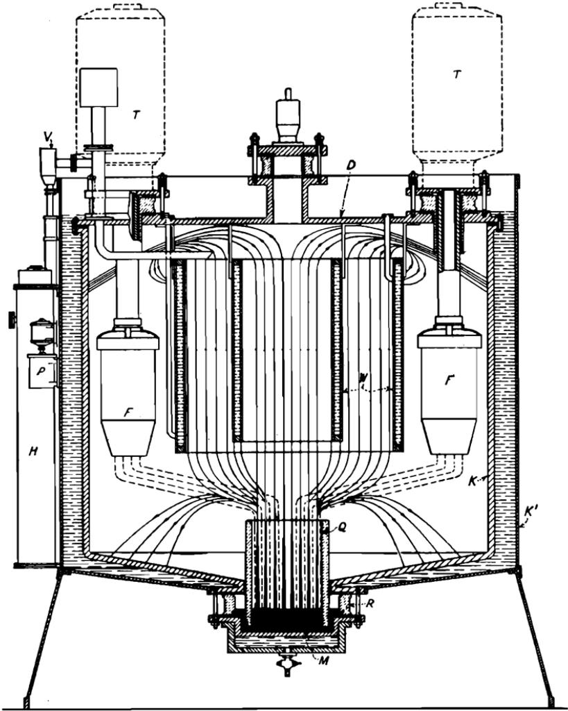
FIG. 96.—Cross-section of a Siemens-Schuckert (Germany) rectifier.
