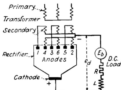
FIG. 41.—Rectifier connected to generalized direct-current load.
