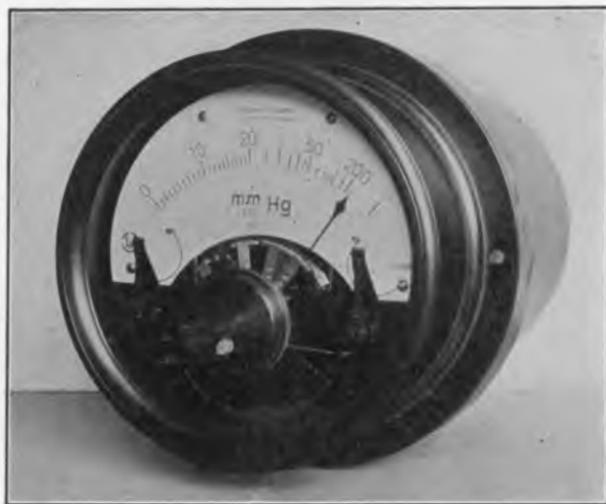
FIG. 128.— Brown Boveri contact-making vacuum meter.
