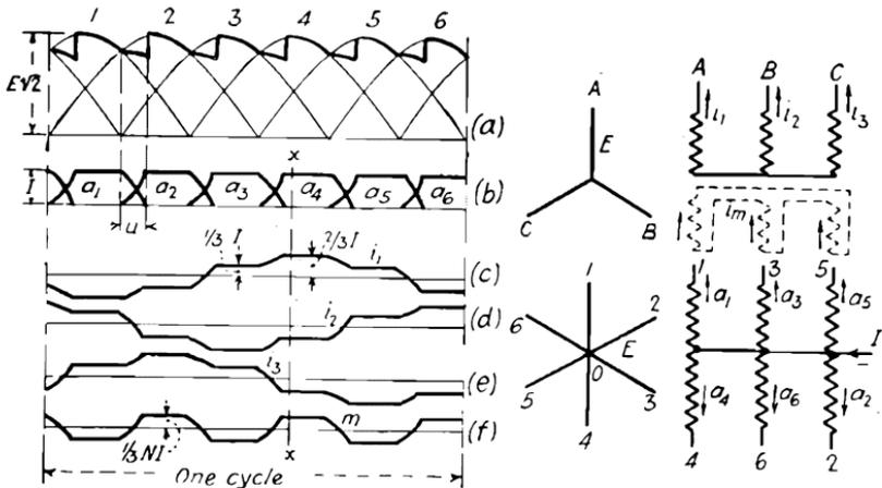
FIG. 50.—Diametrical 6-phase connection with Y-primary.
