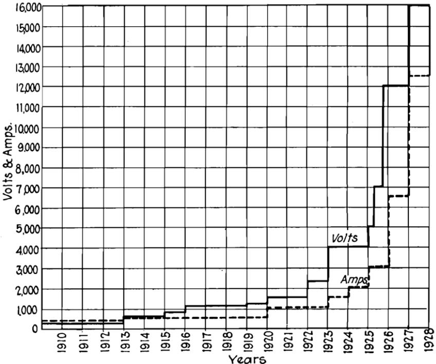
FIG. 1.—Graph showing increase of direct-current voltage and capacities of rectifiers.
