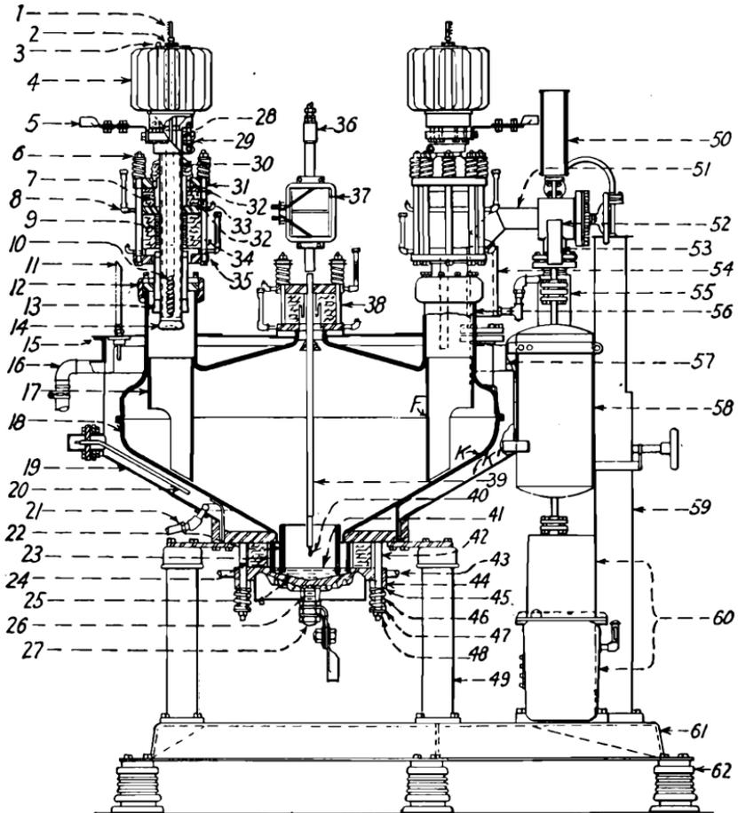
FIG. 90.—Cross-section of General Electric 6-anode rectifier.
