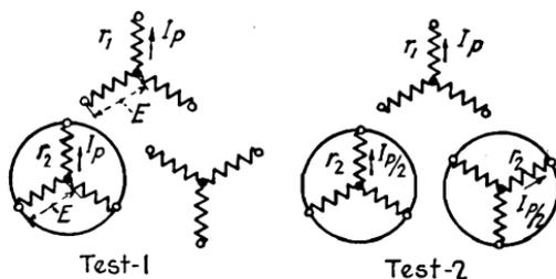
FIG. 77.—Tests for determining the copper losses of a rectifier transformer having a 6-phase connection with interphase transformer. (The resistances  $r_1$  and  $r_2$  are represented in Eqs. (174) to (178) by  $r_p$  and  $r_s$ , respectively.)
