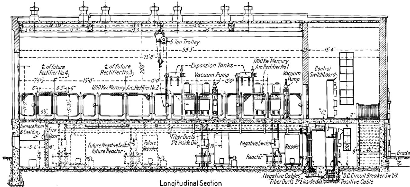
FIG. 185.—Longitudinal section through Rockfield substation.
