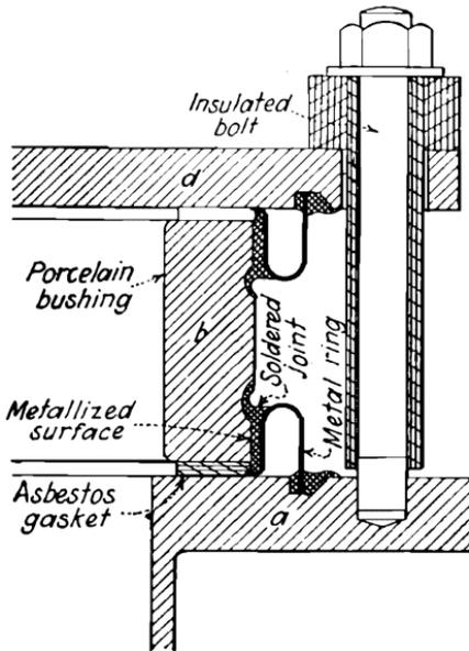
FIG. 105.—Fused seal used in the rectifier shown in Fig. 98.
