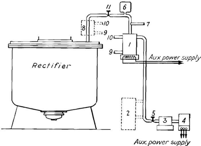
Fig. 110.—Schematic arrangement of vacuum pumping system.
