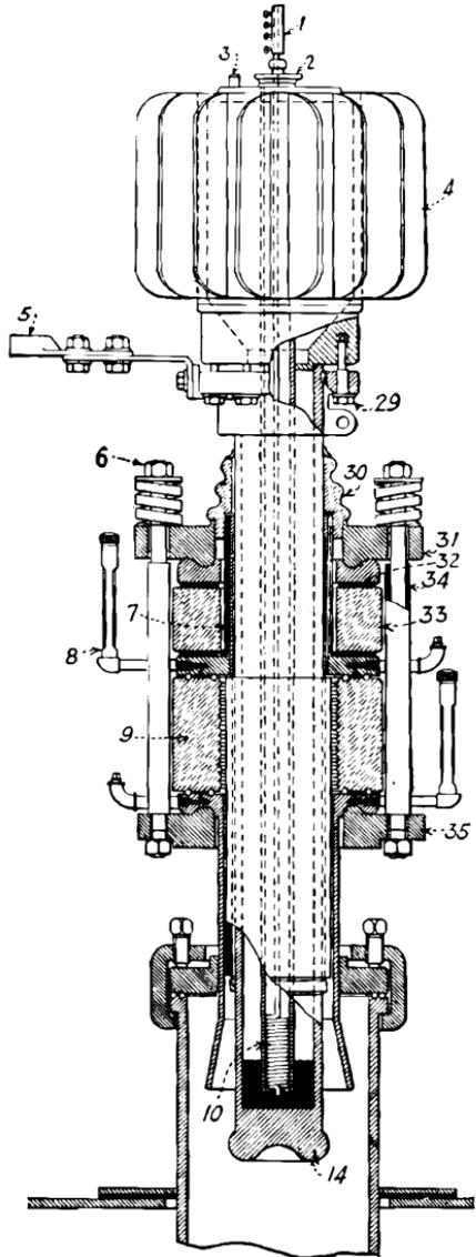
FIG. 108.—Assembly of anode used in the rectifier of Fig. 90, showing mercury seals.
