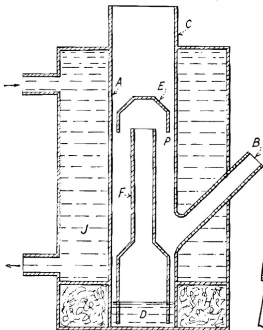
FIG. 117.—Schematic construction of Langmuir mercury-condensation vacuum pump.
