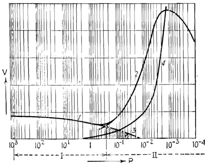
FIG. 111.—Curves of volumetric capacity of mercury and rotary vacuum pumps, in function of the pressure in millimeters mercury column.
